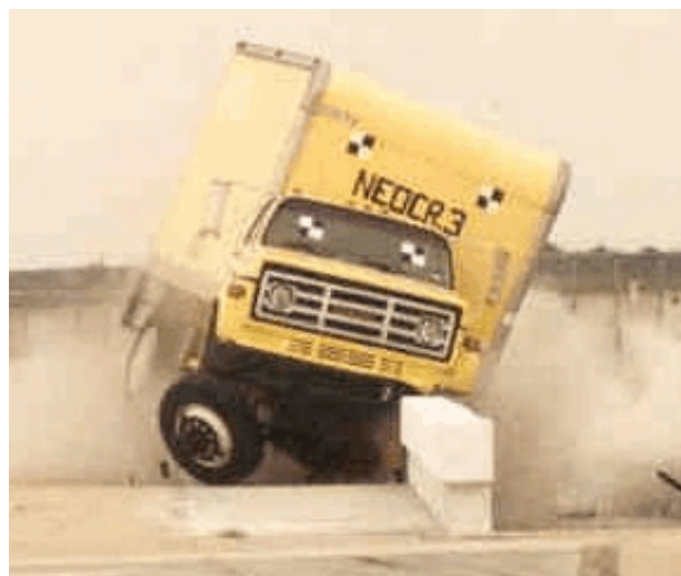
Figure 2. Single-Unit Truck Roll Motion Behavior
