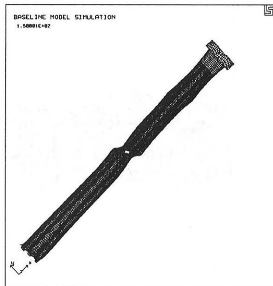
Figure 46. Failure geometry from simulation.
