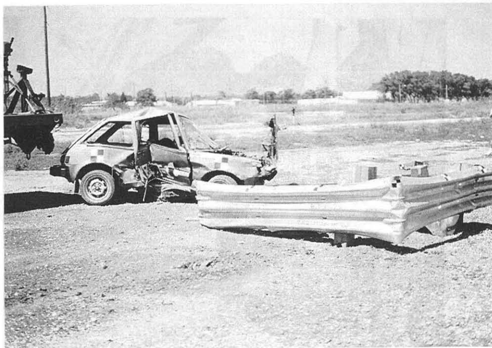
Figure 67. Vehicle trajectory, Test KBCT-1.
