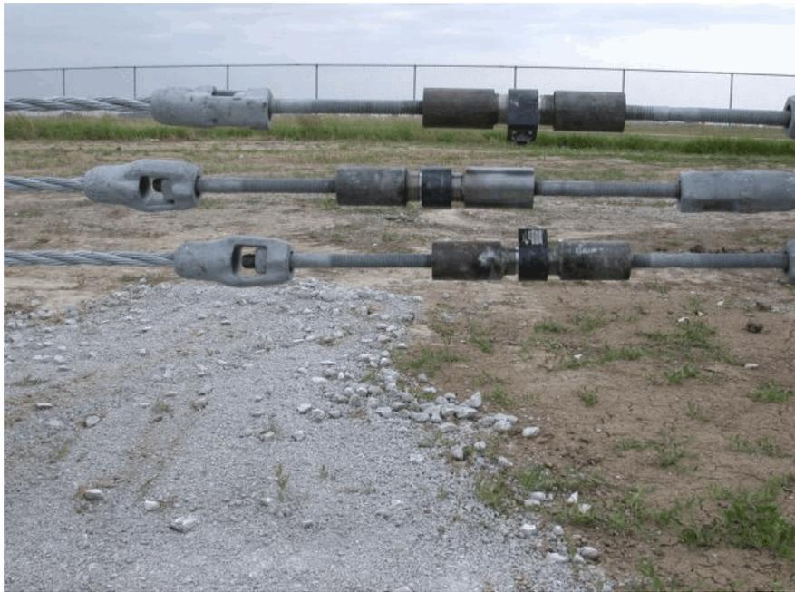
Figure 17. Load Cell Configuration, Test CT-1
