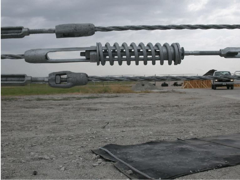
Figure 24. End Anchor, Load Cell, and Spring Compensator Details, Design No. 1
