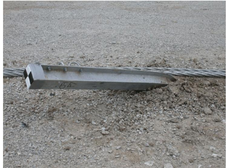
Figure 34. Post Nos. 6 and 7 Damage, Test CT-1
