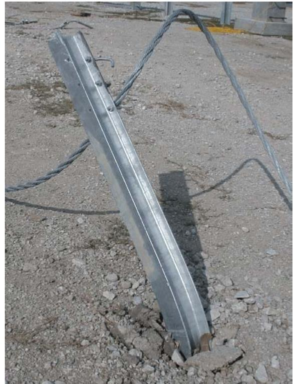
Figure 80. Post Nos. 6 and 7 Damage, Test CT-3
