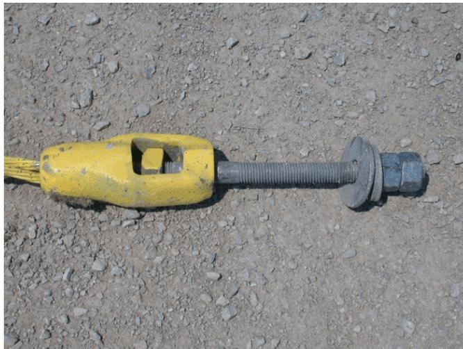
Figure 60. Threaded Rod Damage, Test CT-2
