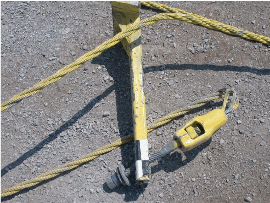
Figure 58. Cable Release Lever Damage, Test CT-2
