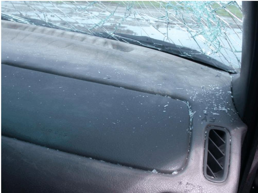
Figure 111. Occupant Compartment Damage, Test CT-4
