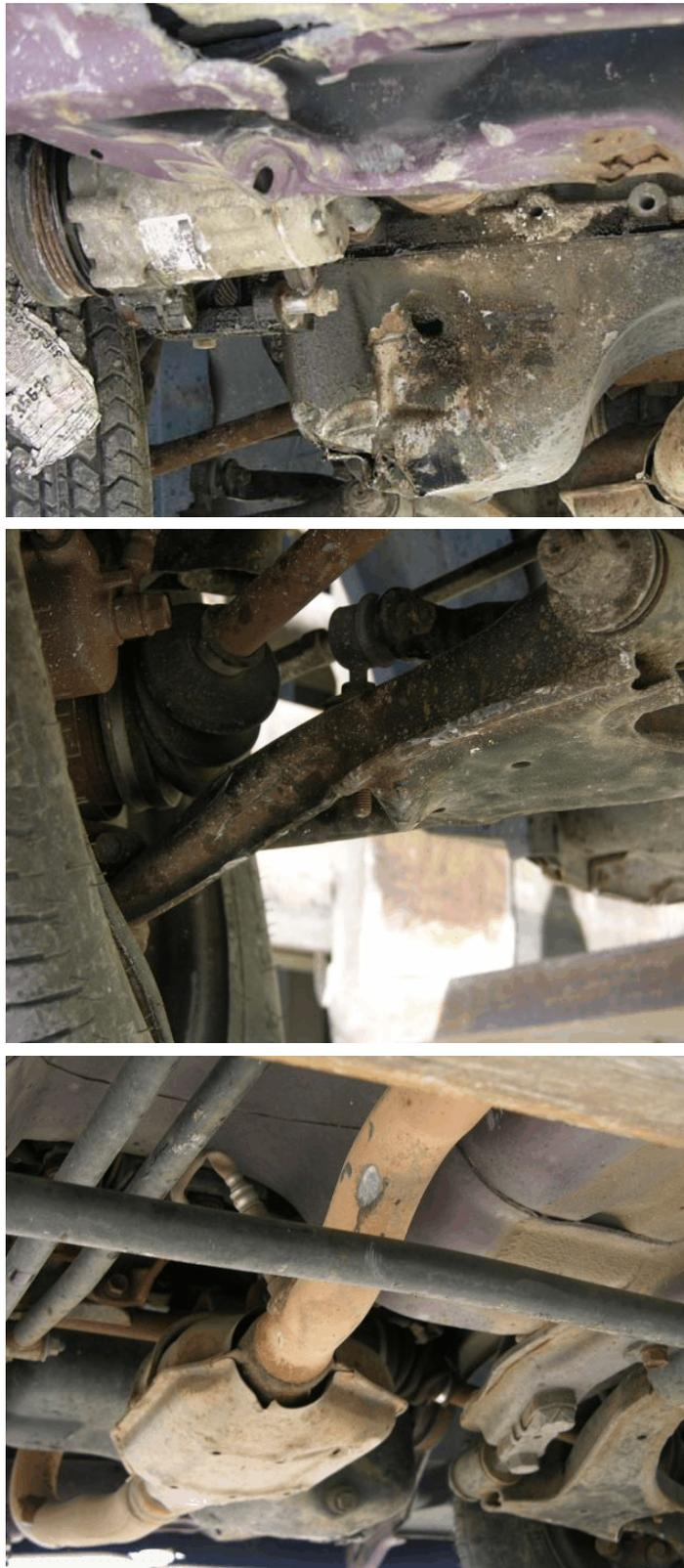
Figure 110. Undercarriage Damage, Test CT-4
