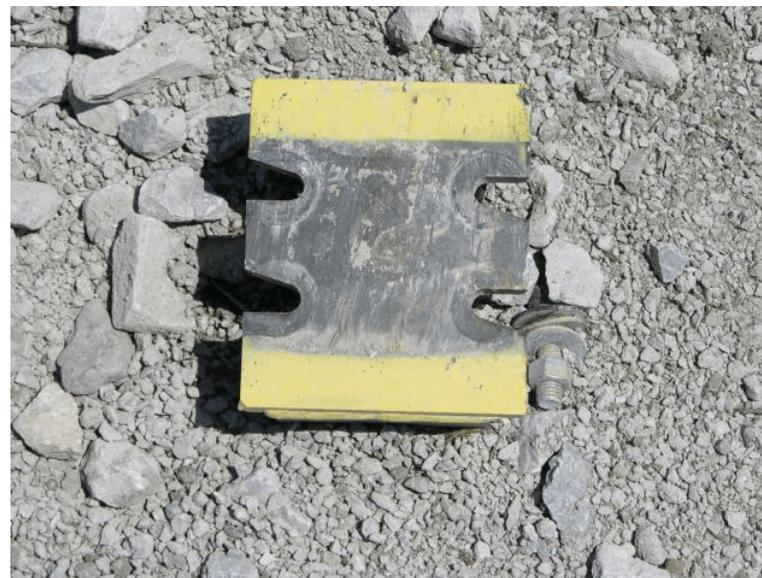
Figure 104. Post Nos. 1 through 3 Base Plate Damage, Test CT-4
