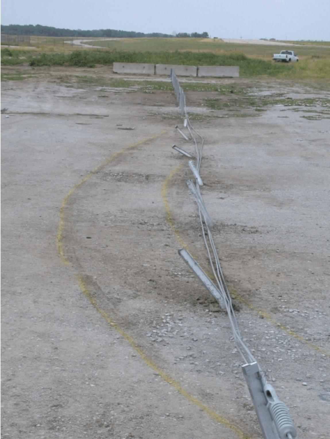
Figure 31. Vehicle Trajectory and Final Position, Test CT-1
