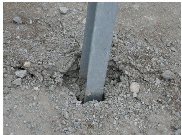
Figure 32. Post Nos. 2 and 3 Damage, Test CT-1
