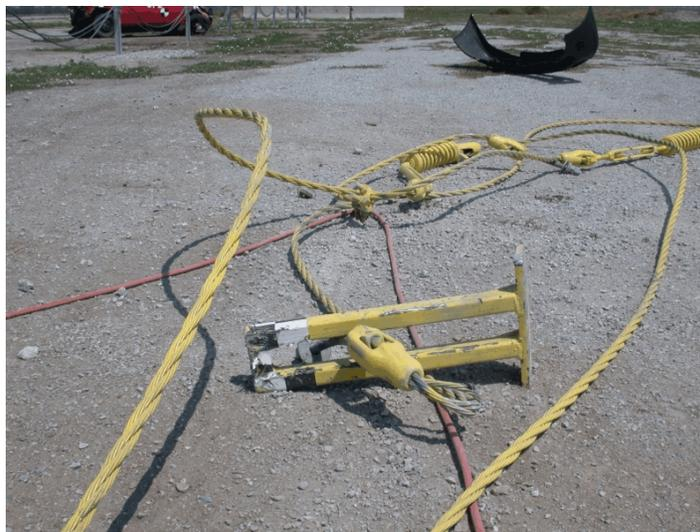
Figure 59. Cable Damage, Test CT-2
