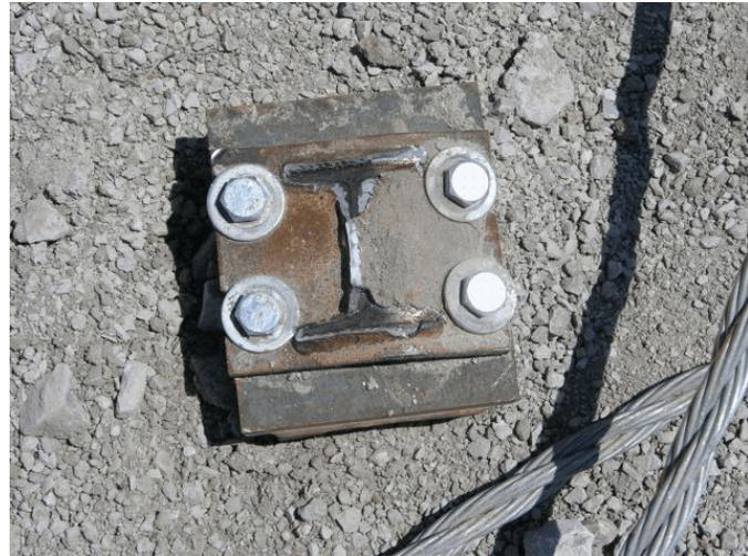
Figure 105. Post Nos. 4 through 7 Base Plate Damage, Test CT-4
