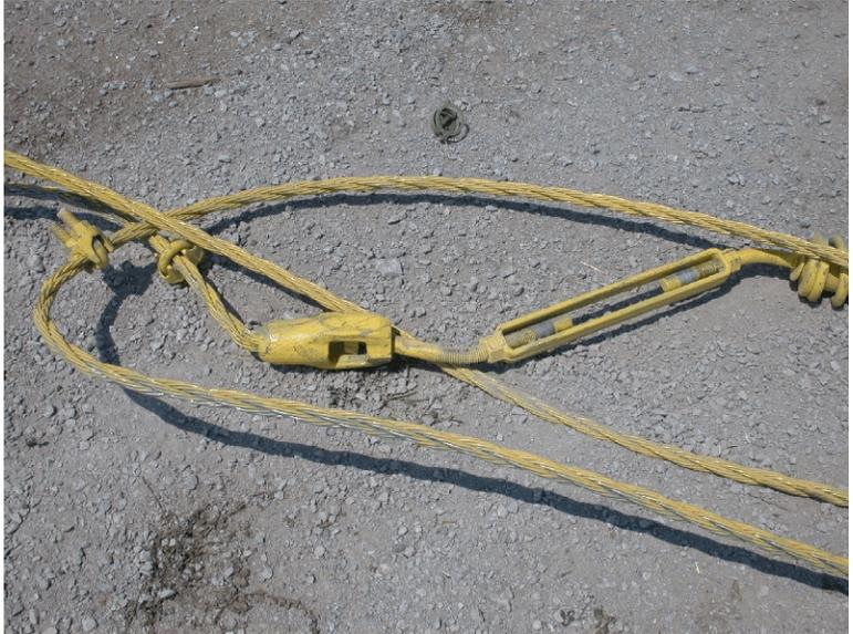
Figure 61. Cable Turnbuckle and Compensator Damage, Test CT-2
