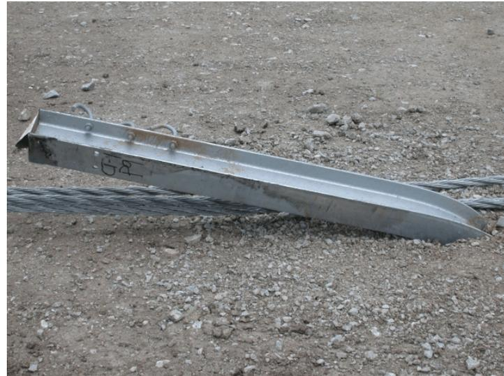
Figure 35. Post Nos. 8 and 9 Damage, Test CT-1
