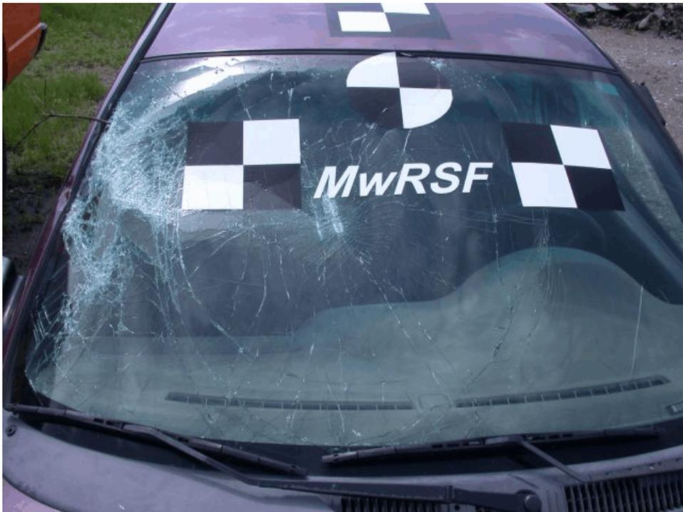
Figure 109. Windshield Damage, Test CT-4
