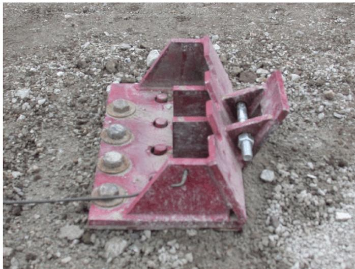
Figure 76. Post No. 1 and Cable Release Lever Damage, Test CT-3
