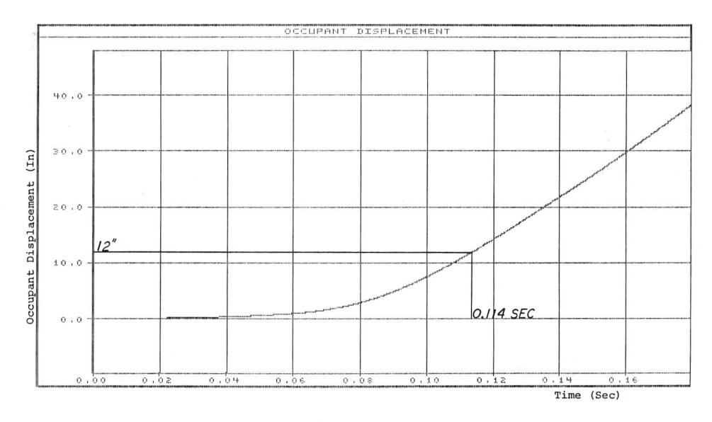
FIGURE C-12. GRAPH OF LATERAL OCCUPANT DISPLACEMENT, TEST 12-2
