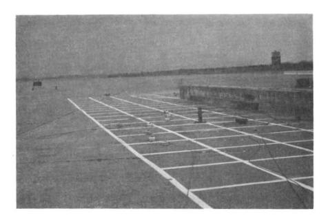
FIGURE 25. RETROFIT CONCRETE BARRIER RAIL DAMAGE, TEST 12-3
