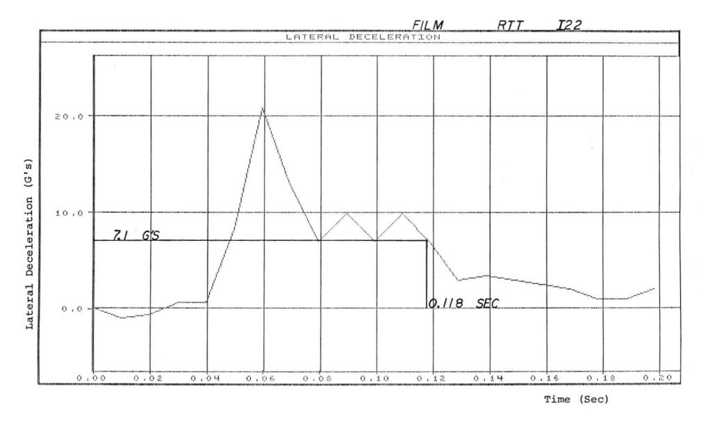
FIGURE C-13. GRAPH OF LATERAL DECELERATION, TEST 12-2
