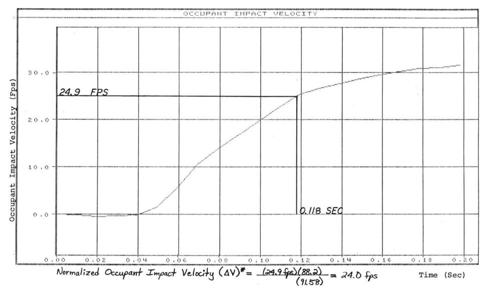
FIGURE C-14. GRAPH OF LATERAL OCCUPANT IMPACT VELOCITY, TEST 12-2
