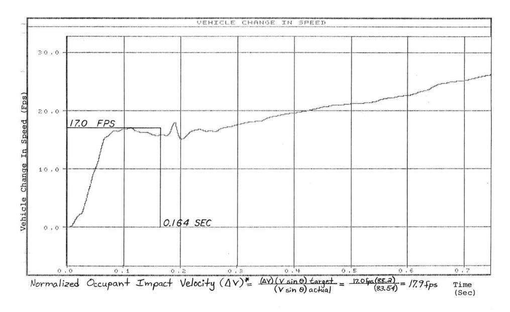
FIGURE C-2. GRAPH OF VEHICLE CHANGE IN SPEED, TEST 12-1
