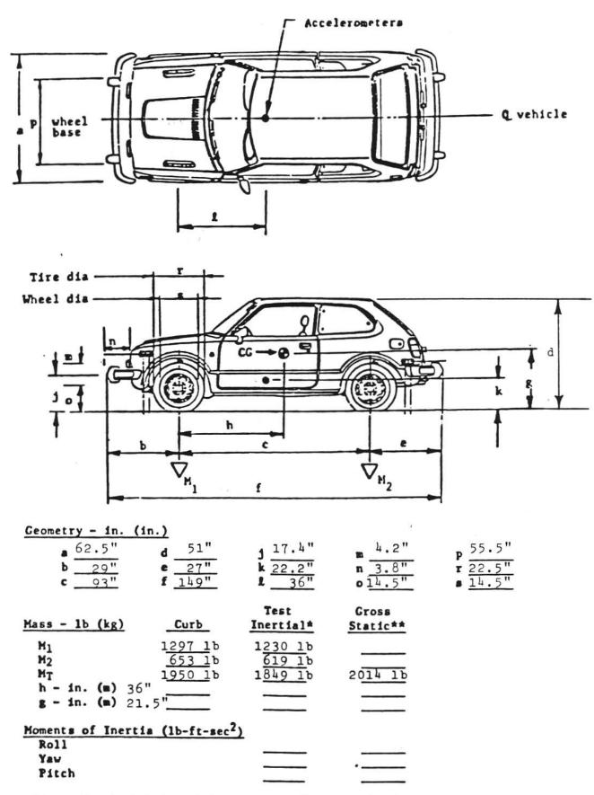
\*Ready for test but excludes passenger/cargo payload \*\*Gross ready for test including passenger/cargo payload
