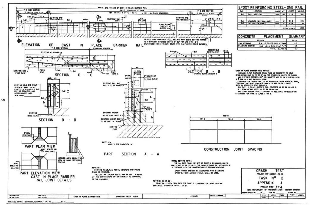
strength at the time of the crash tests (for the Box-Aluminum Bridge Rail) averaged about 6,000 psi (see Appendix A). The curb was 20-in. wide and 86 ft. in length. The curb was anchored 8-in. into the existing airport concrete apron by two L-shaped No. 5 rebar dowels, spaced at 14-in. on centers over the length of the curb. An epoxy grout material was used as the bonding agent for the dowels.
