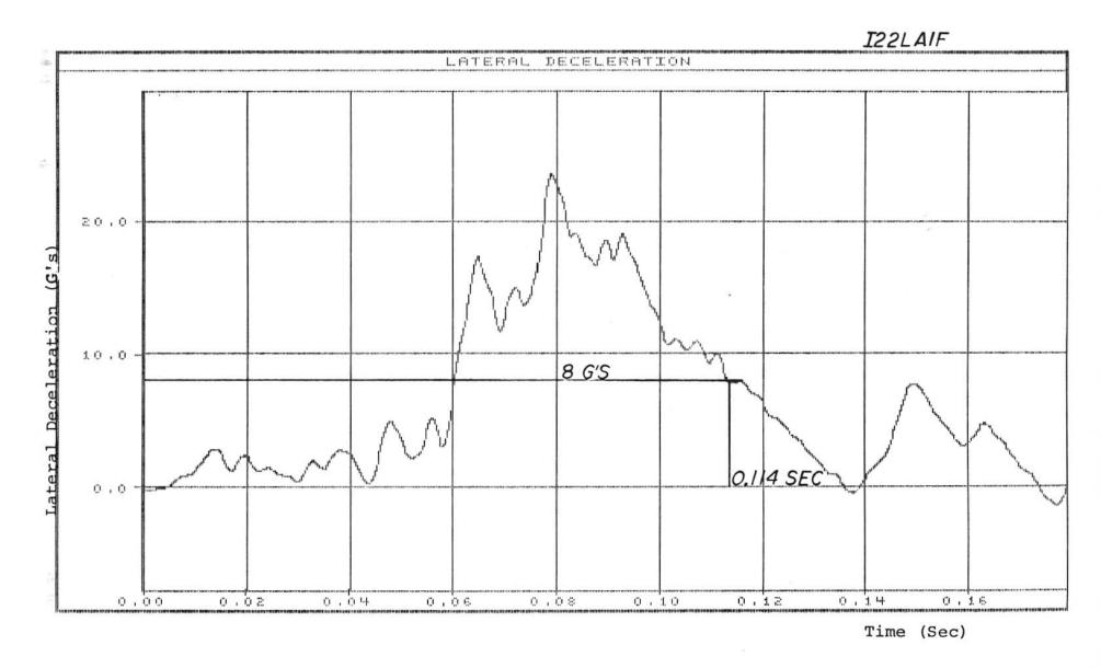
FIGURE C-10. GRAPH OF LATERAL DECELERATION, TEST 12-2
