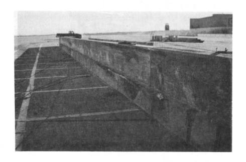
FIGURE 22. RETROFIT CONCRETE BARRIER RAIL DAMAGE, TEST 12-2
