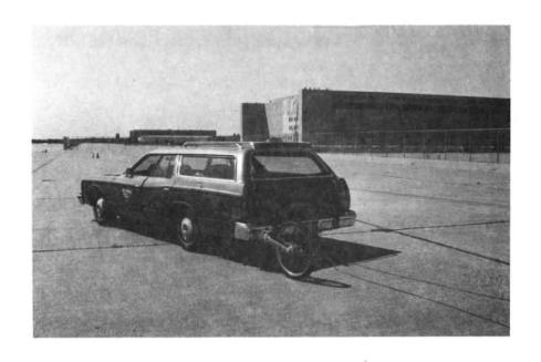
FIGURE 3. PHOTOGRAPHS OF TOW VEHICLE AND FIFTH WHEEL
