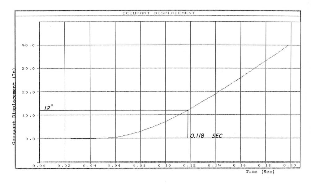
FIGURE C-15. GRAPH OF LATERAL OCCUPANT DISPLACEMENT, TEST 12-2
