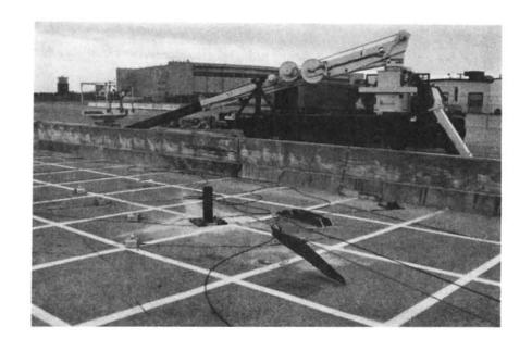
FIGURE 19. RETROFIT CONCRETE BARRIER RAIL DAMAGE, TEST 12-1
