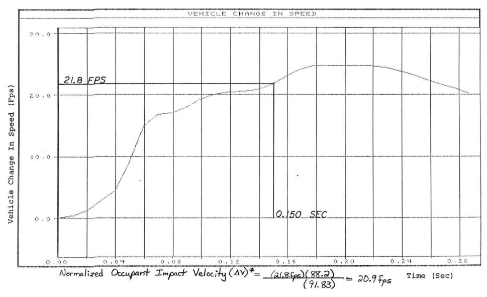
FIGURE C-17. GRAPH OF VEHICLE CHANGE IN SPEED, TEST 12-3
