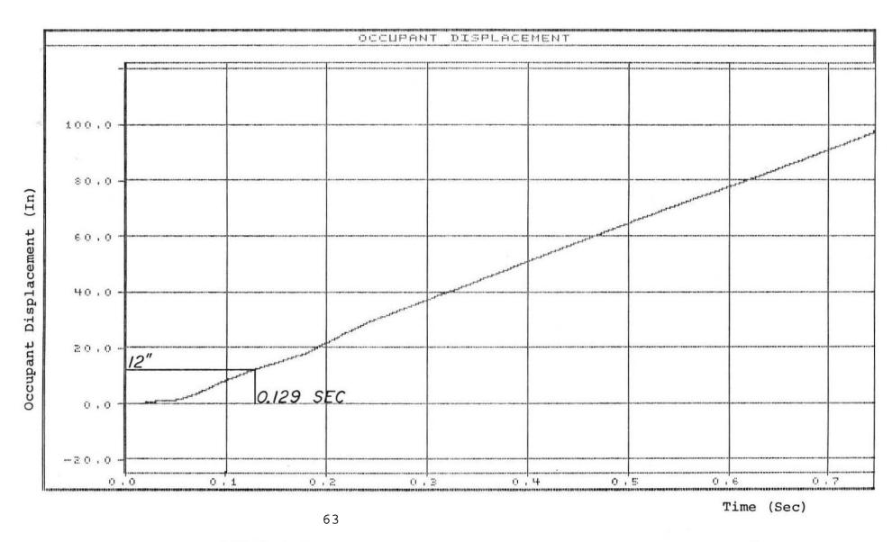
FIGURE C-6. GRAPH OF LATERAL OCCUPANT DISPLACEMENT, TEST 12-1
