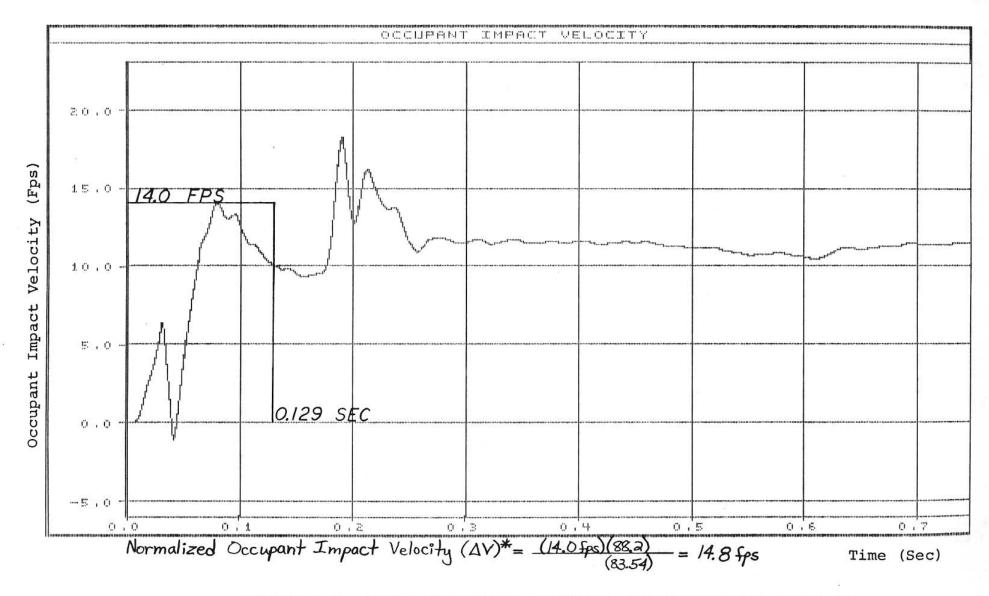
FIGURE C-5. GRAPH OF LATERAL OCCUPANT IMPACT VELOCITY, TEST 12-1
