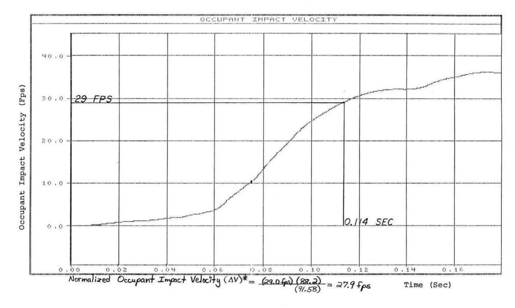
FIGURE C-11. GRAPH OF LATERAL OCCUPANT IMPACT VELOCITY, TEST 12-2
