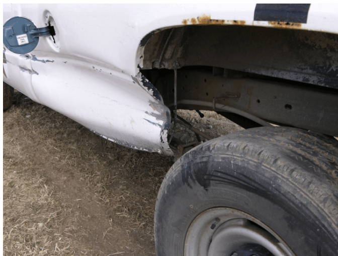
Figure 96. Vehicle Damage, Test CMB-3
