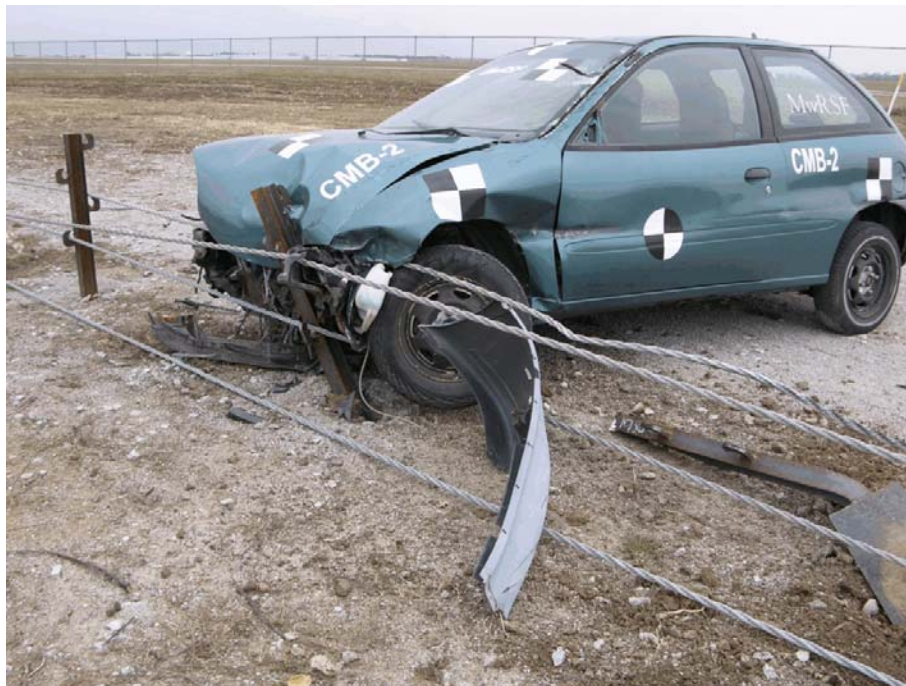
Figure 66. Vehicle Final Position and Trajectory Marks, Test CMB-2
