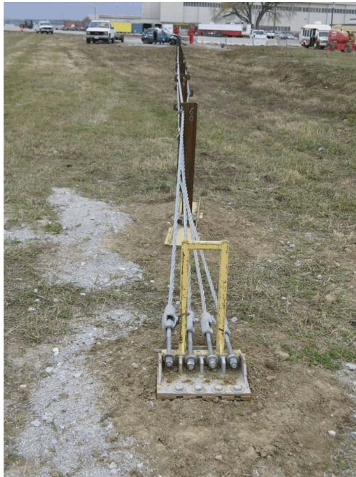
Figure 70. End Anchorage Damage, Test CMB-2
