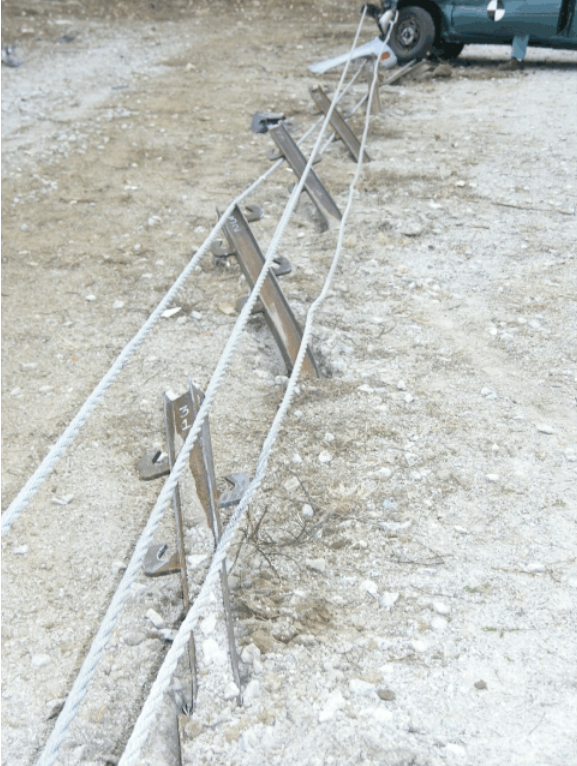
Figure 67. System Damage, Test CMB-2
