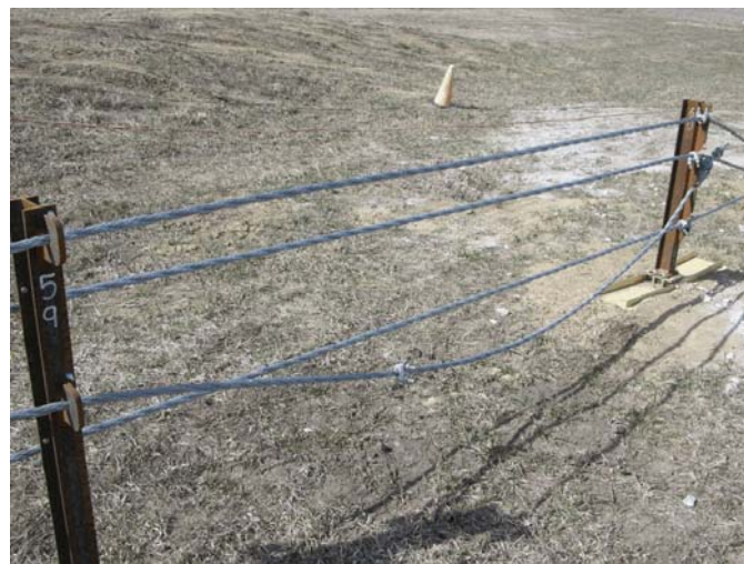
Figure 94. Downstream Anchorage Damage, Test CMB-3
