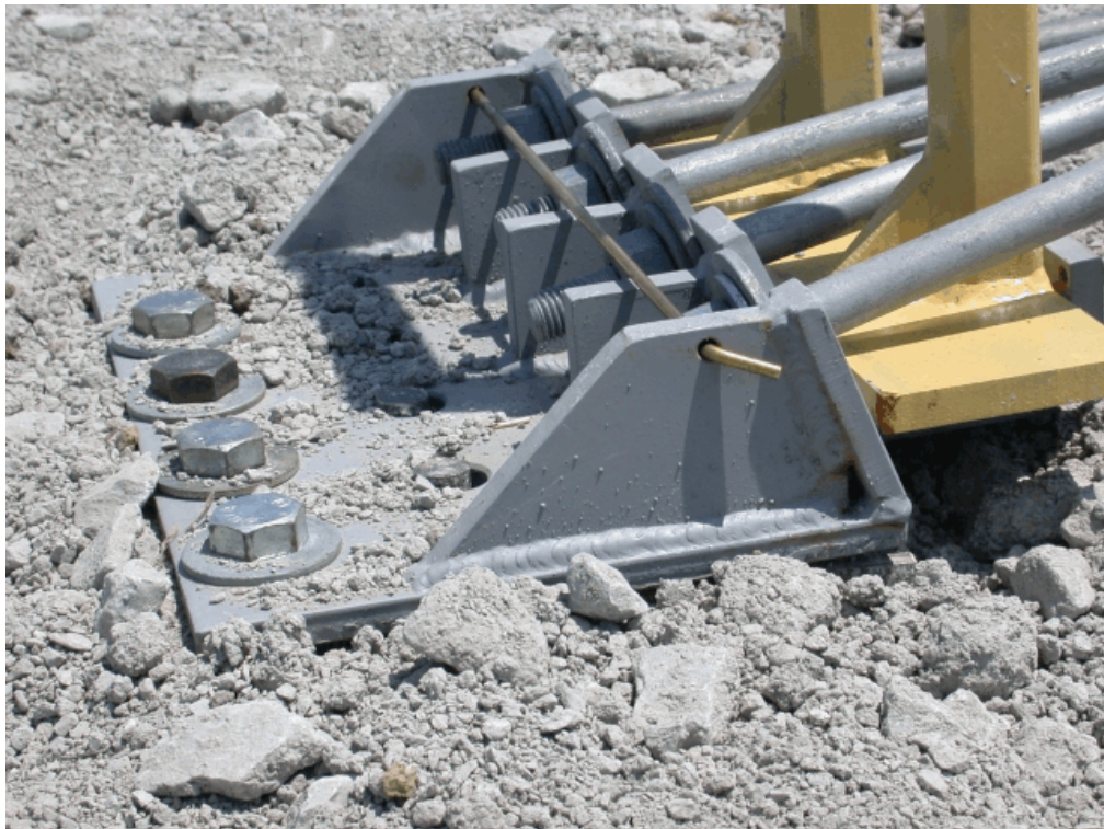
Figure 46. Downstream End Anchorage Damage, Test CMB-1
