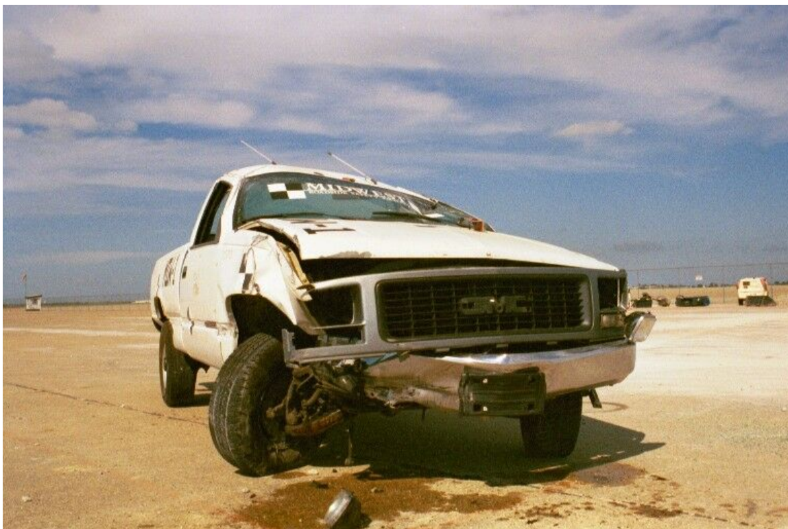
Figure 121. Bumper Deformation in Test MIW-1 (Failed)
