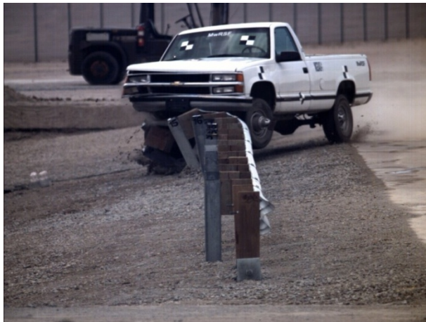
Figure 126. W-beam Rail Trapped Between the Front Wheel and the Bumper
