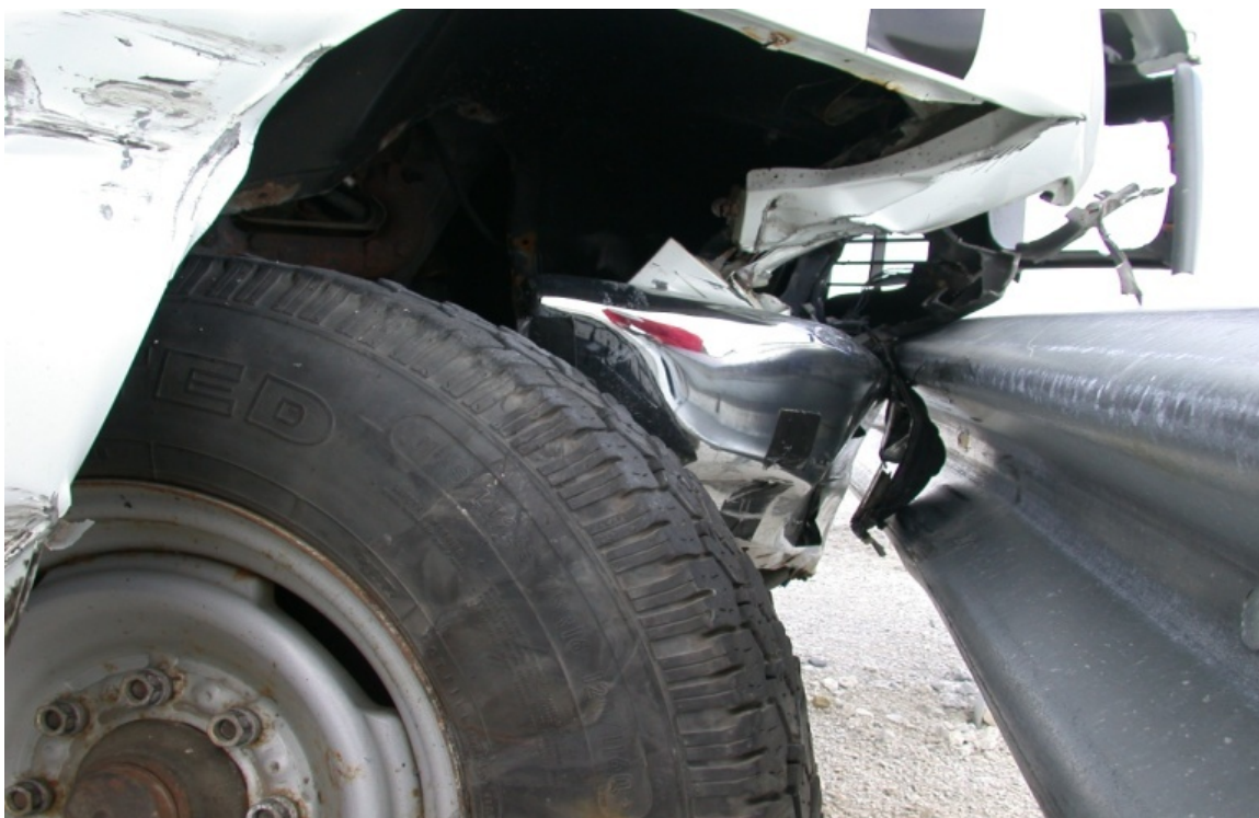
Figure 122. Bumper Deformation in Test NPG-4 (Passed)
