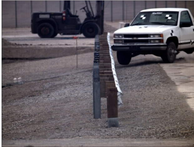
Figure 125. Vehicle's Front Suspension Extended Due to the Slope
