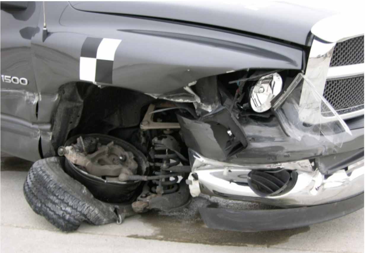
Figure 109. Only Middle Metallic Portion Actually Functions as a Bumper
