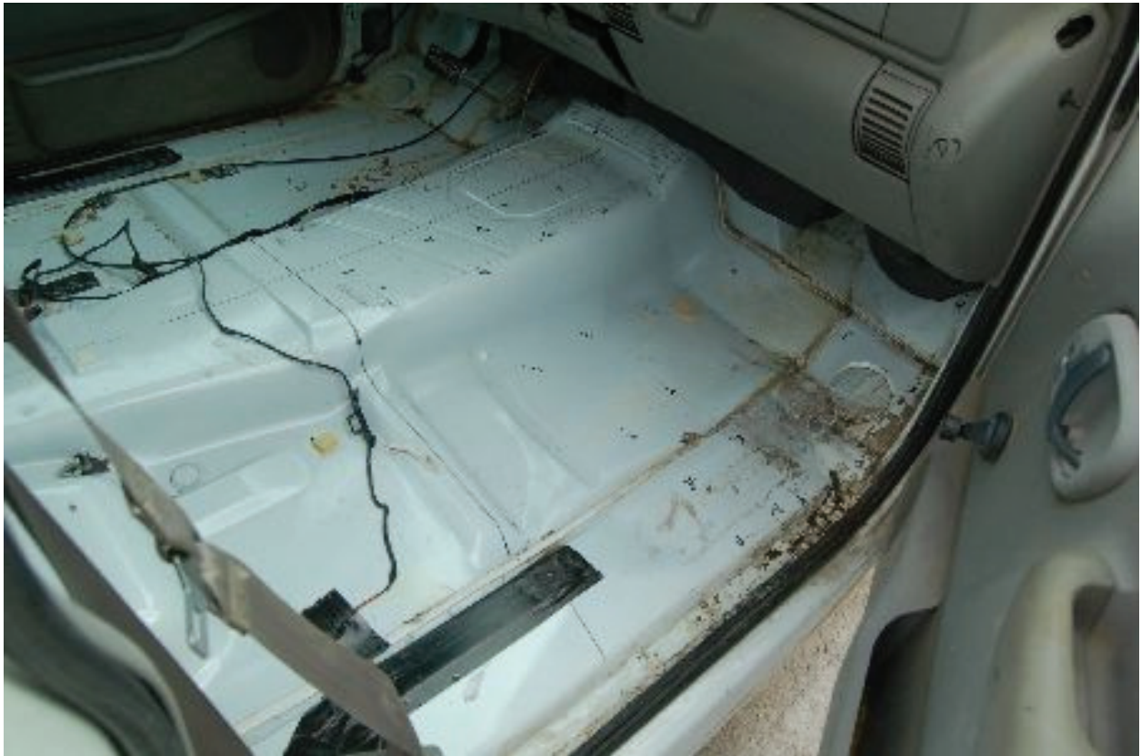
Figure 52. Vehicle Damage, Occupant Compartment, Test No. RSMG-1
