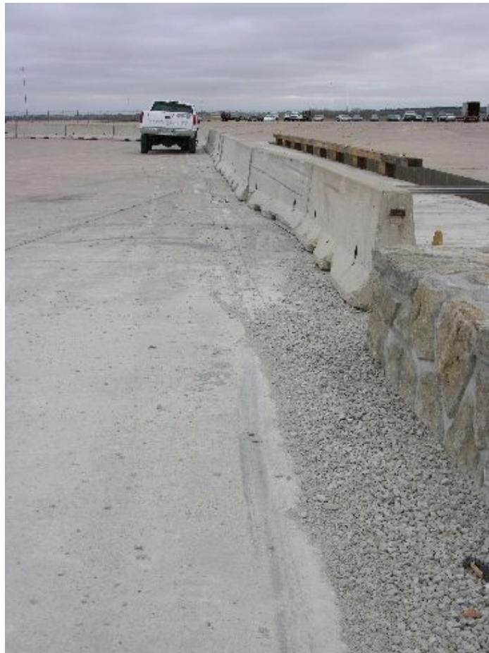
Figure 46. Vehicle Final Position and Trajectory Marks, Test No. RSMG-1
