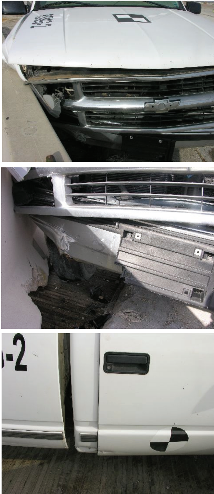
Figure 66. Vehicle Damage, Test No. RSMG-2
