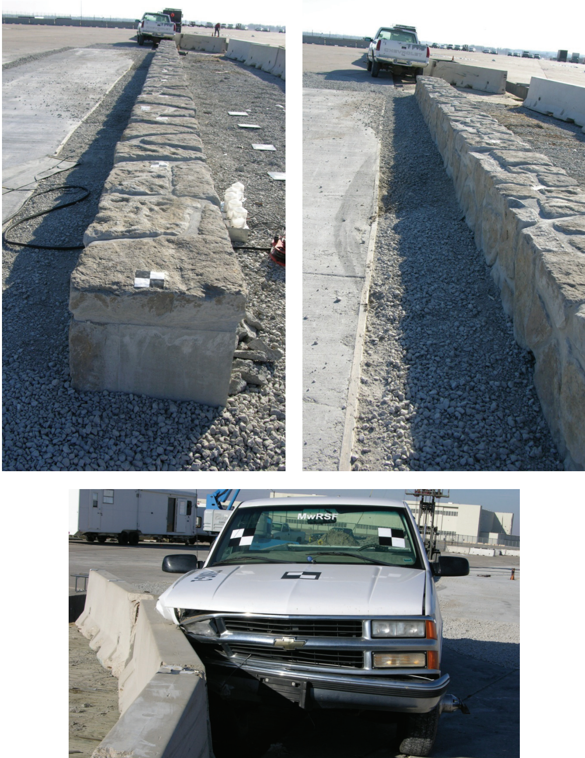
Figure 61. Vehicle Final Position and Trajectory Marks, Test No. RSMG-2
