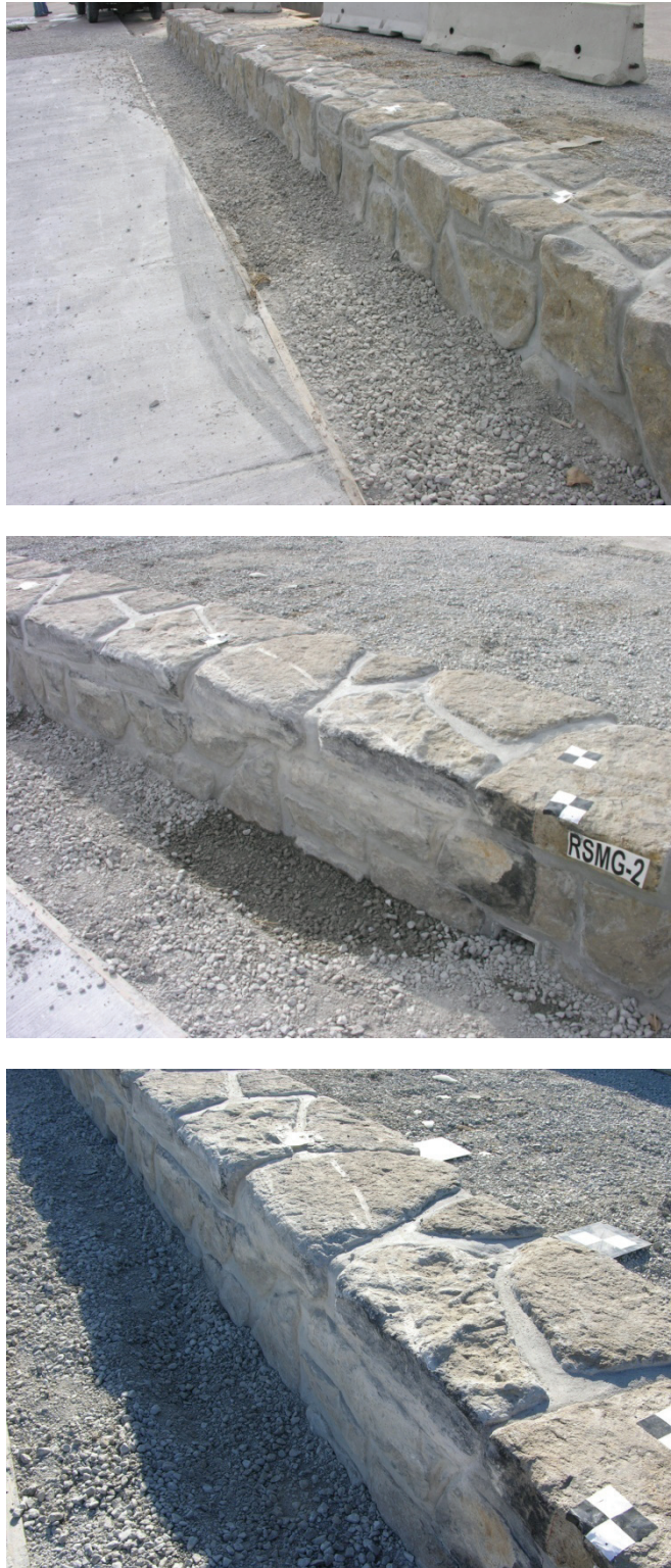
Figure 62. System Damage, Test No. RSMG-2
