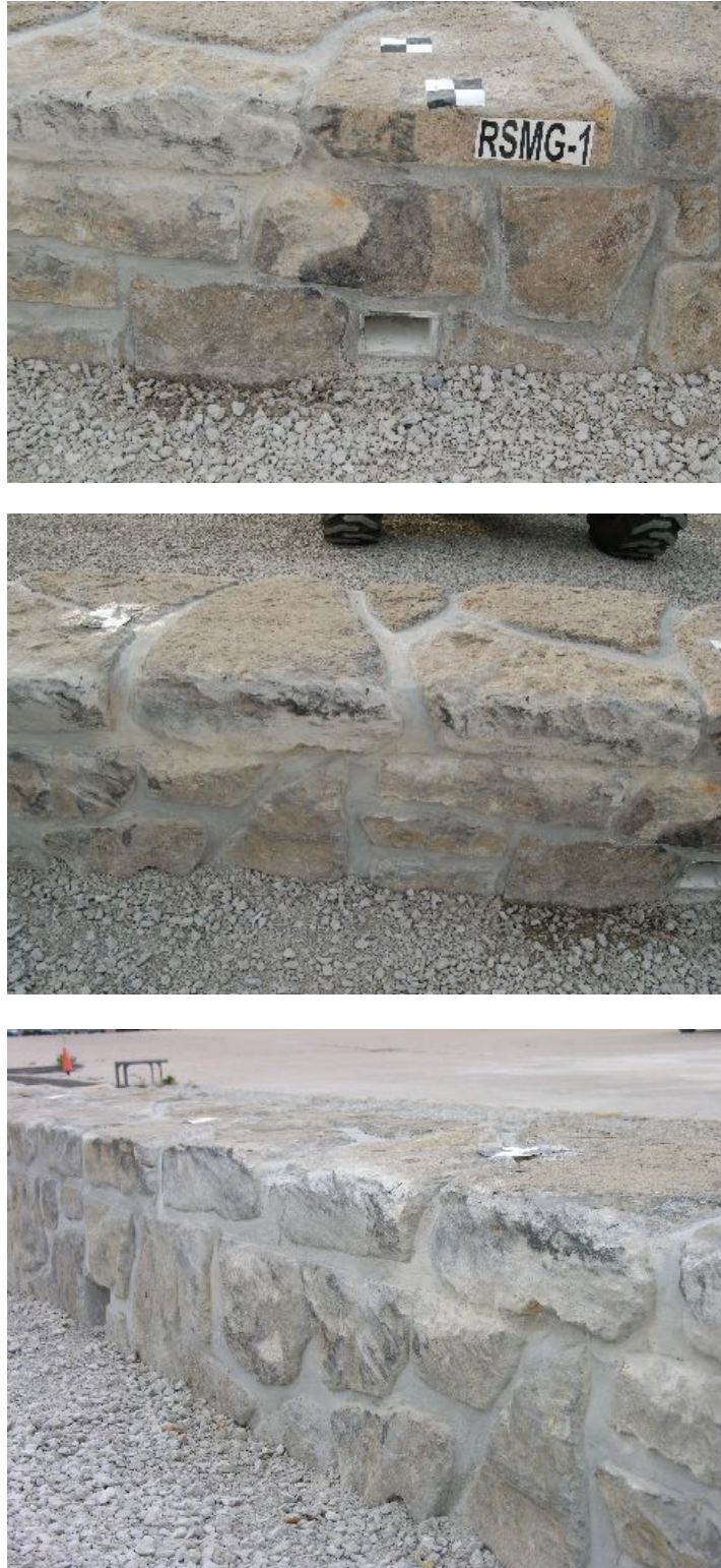
Figure 48. System Damage, Test No. RSMG-1
