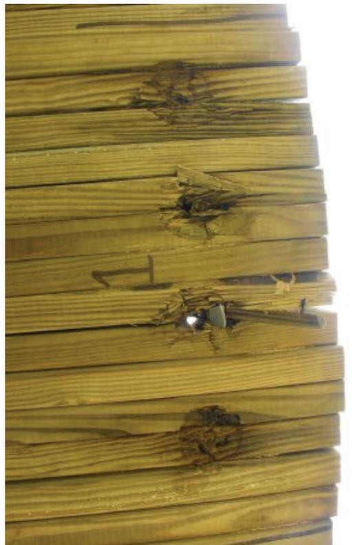
**Figure 11. Bridge Deck Damage, Test No. WVS-1**
