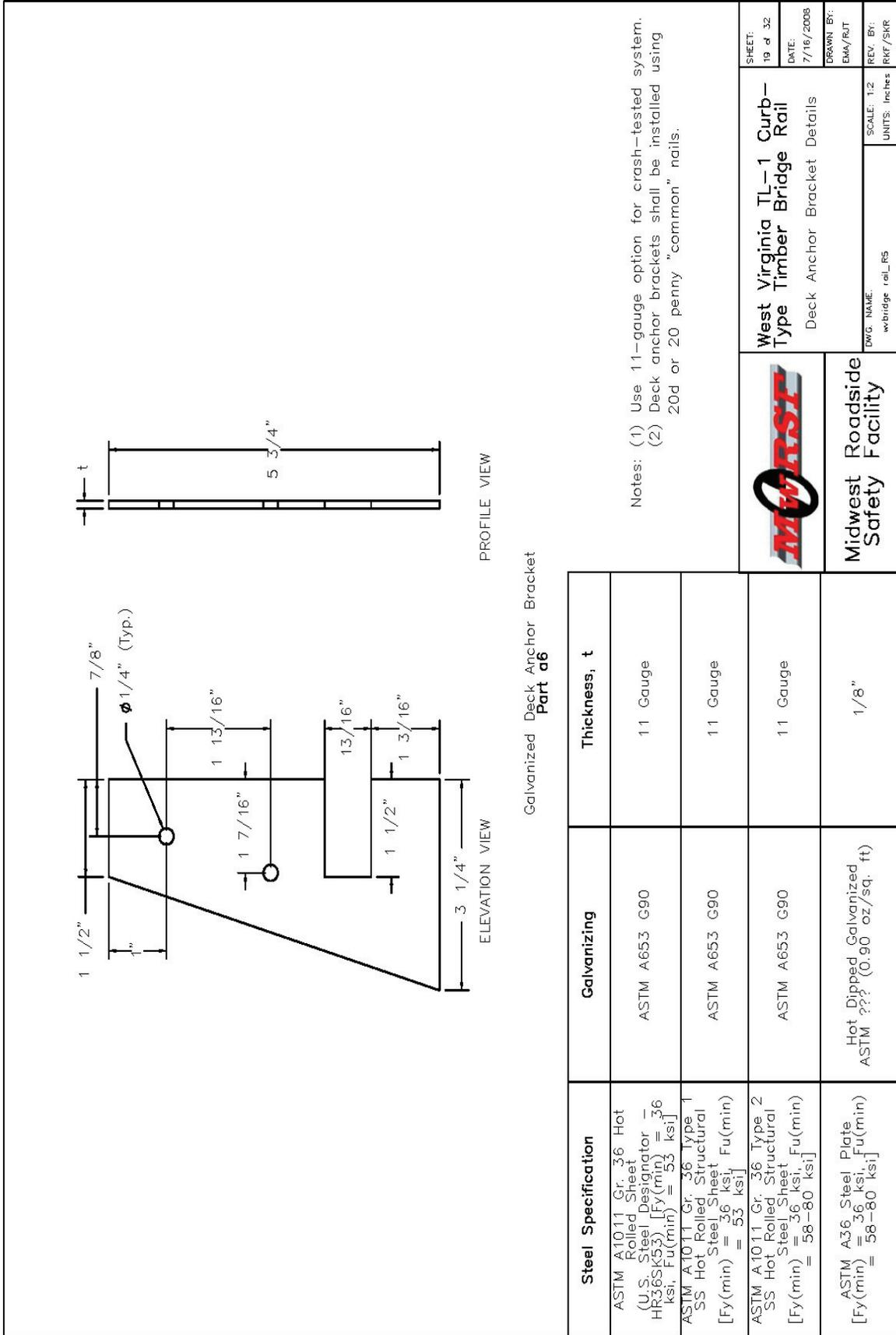
**Figure 43. Deck Anchor Bracket Details, Test No. WVBR-1**
