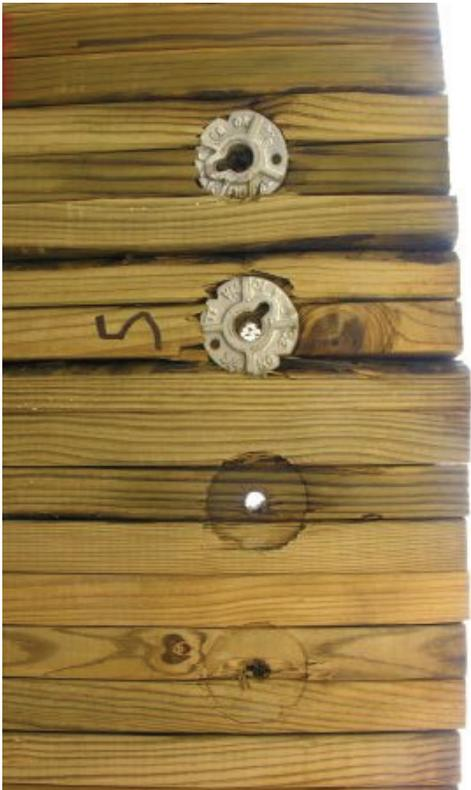
Figure 23. Bridge Deck Damage, Test No. WVS-5
