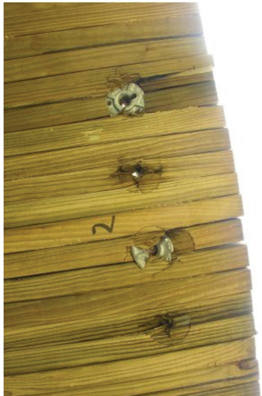
Figure 14. Bridge Deck Damage, Test No. WVS-2
