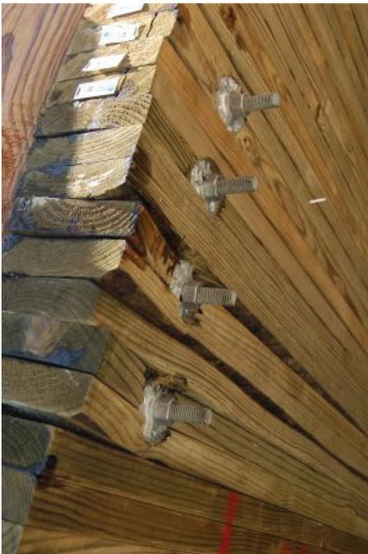
Figure 22. Component Damage and Permanent Set Deflection, Test No. WVS-5
