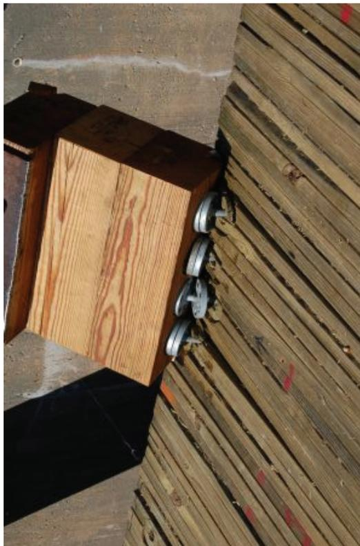
Figure 16. Component Damage and Permanent Set Deflection, Test No. WVS-3
