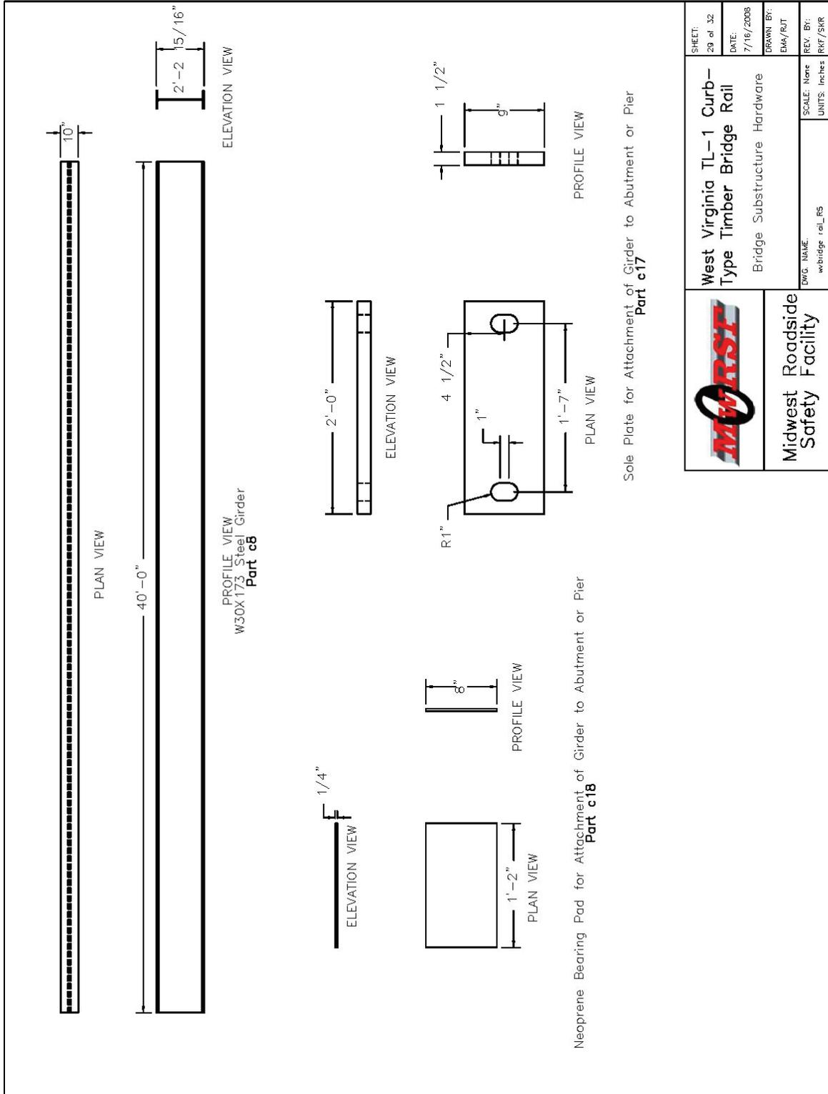
Figure 53. Bridge Substructure Hardware, Test No. WBR-1
