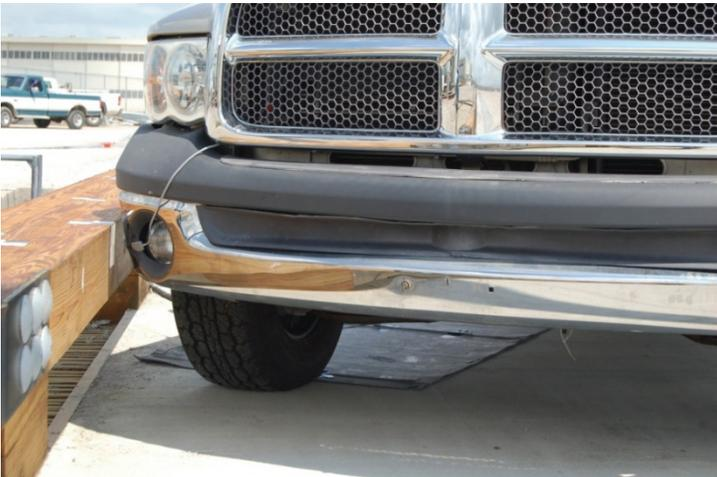
**Figure 70. Target Impact Location, Test No. WVBR-1**
