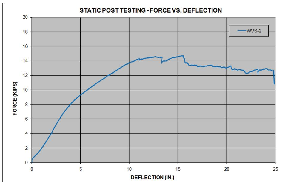
Figure 12. Force vs. Deflection Plot, Test No. WVS-2
