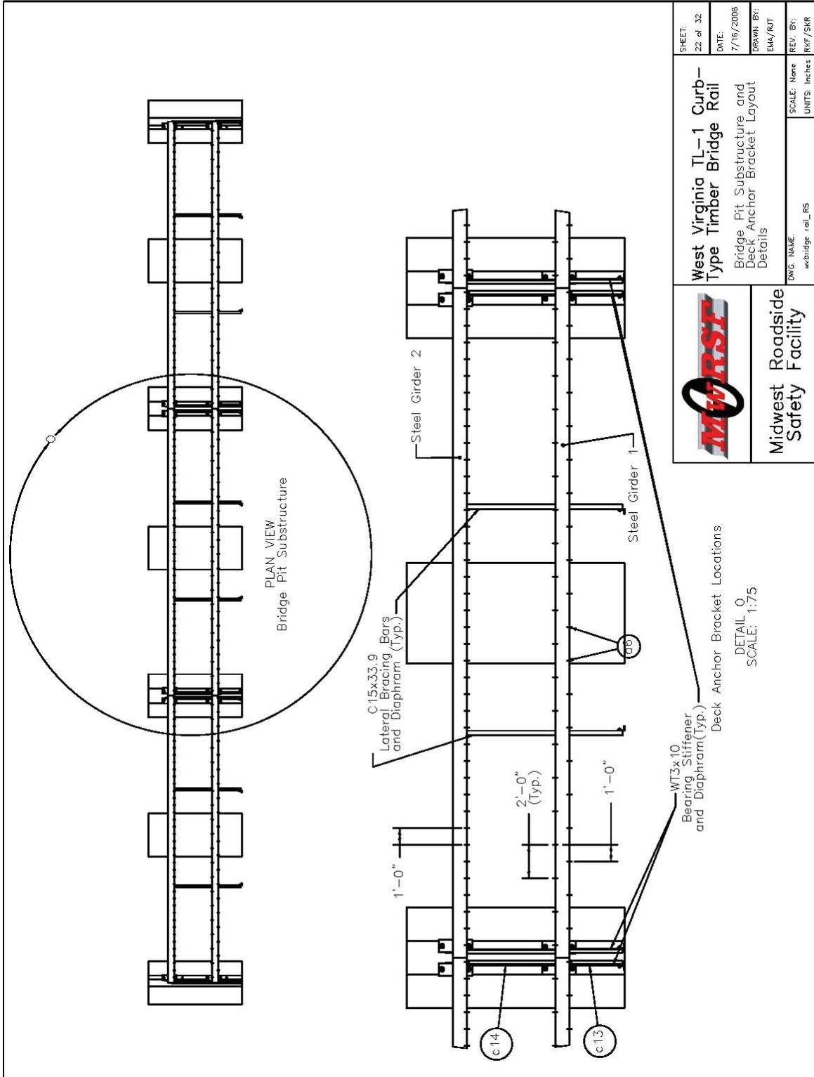
**Figure 46. Bridge Substructure and Deck Anchor Bracket Layout, Test No. WVBR-1**
