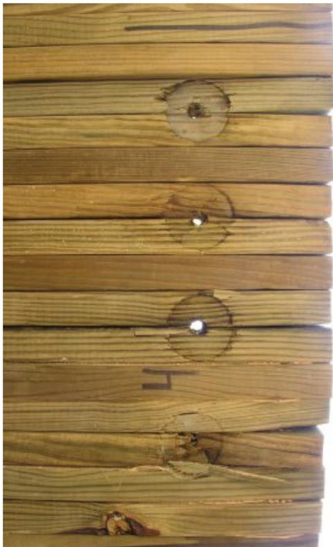
Figure 20. Bridge Deck Damage, Test No. WVS-4
