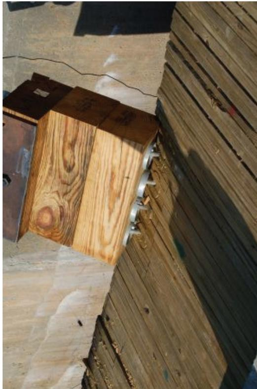
Figure 13. Component Damage and Permanent Set Deflection, Test No. WVS-2
