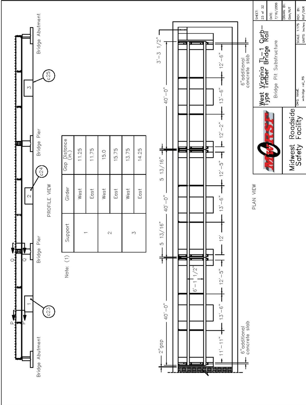
Figure 47. Bridge Pit Substructure, Test No. WVBR-1
