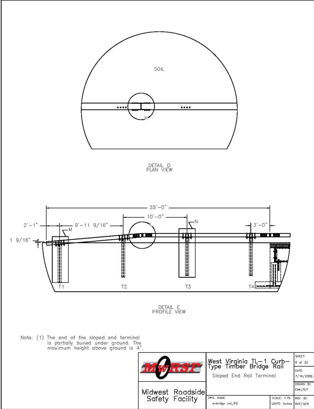
Figure 32. Rail End Treatment, Test No. WVBR-1
