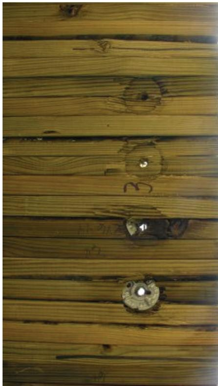
Figure 17. Bridge Deck Damage, Test No. WVS-3
