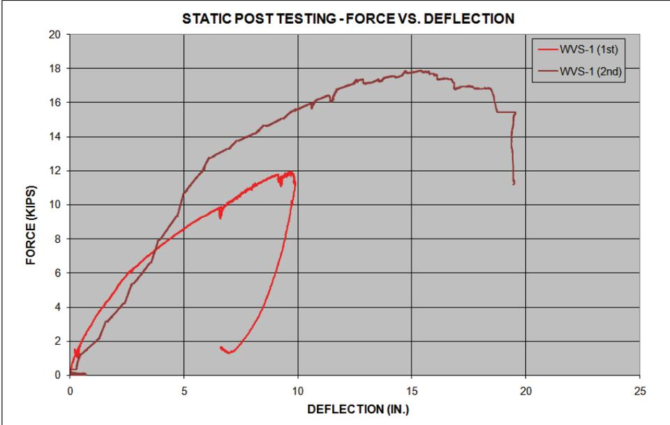
**Figure 9. Force vs. Deflection Curve, Test No. WVS-1**
