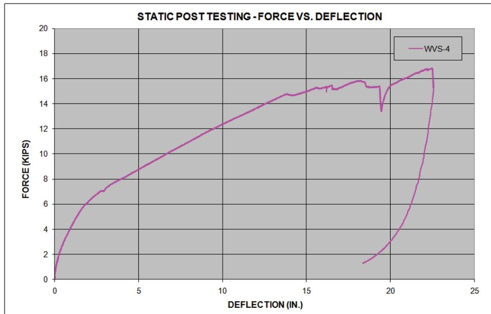
Figure 18. Force vs. Deflection Plot, Test No. WVS-4
