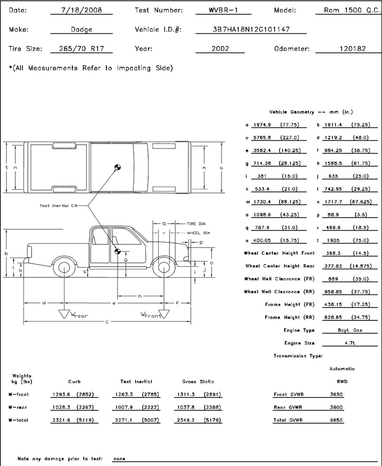
Figure 62. Vehicle Dimensions, Test No. WVBR-1
