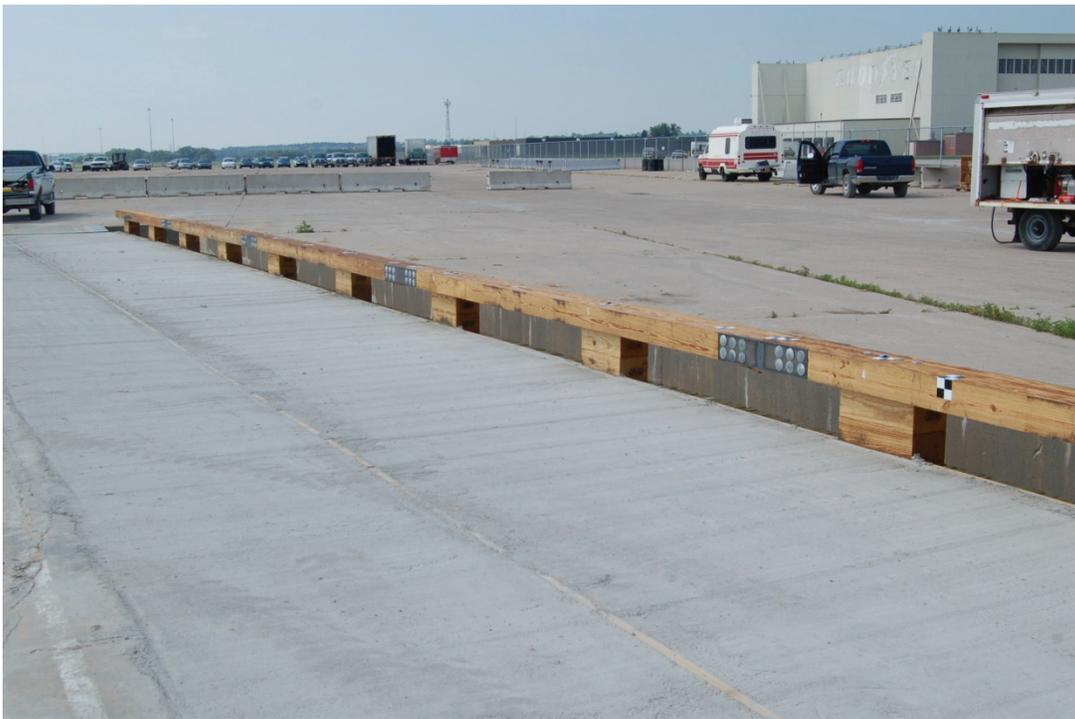
**Figure 57. Curb-Type Bridge Railing System, Test No. WVBR-1**
