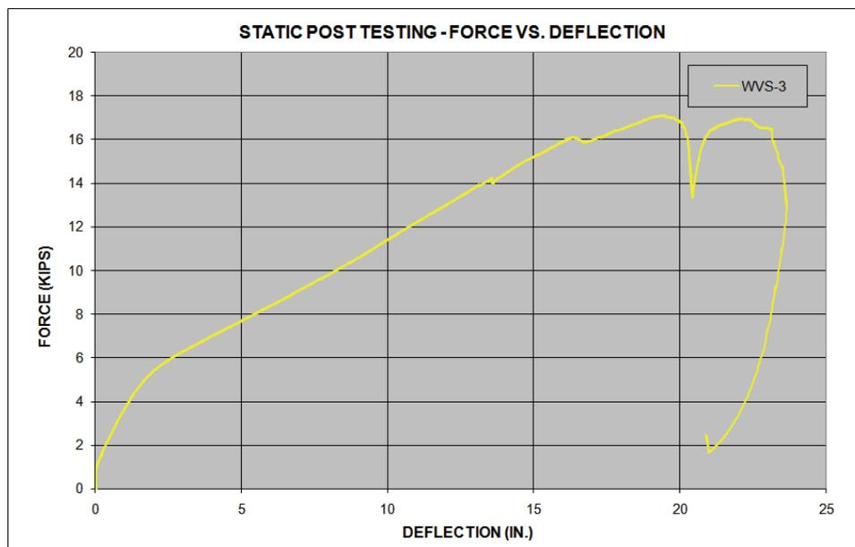
Figure 15. Force vs. Deflection Plot, Test No. WVS-3
