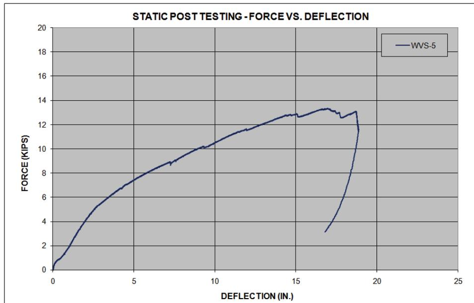
Figure 21. Force vs. Deflection Plot, Test No. WVS-5
