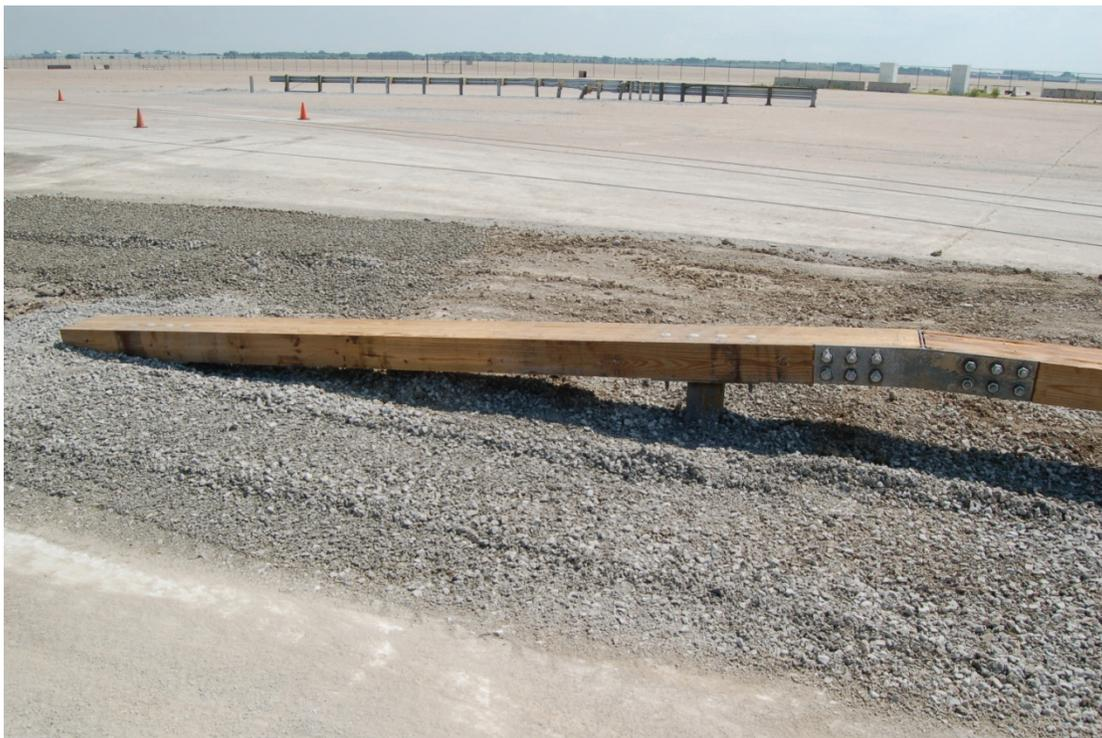
**Figure 60. Sloped End Treatment, Test No. WVBR-1**
