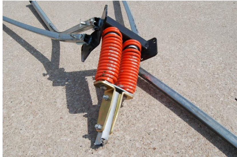
Figure 98. System Damage, Test No. WZ09-4B
