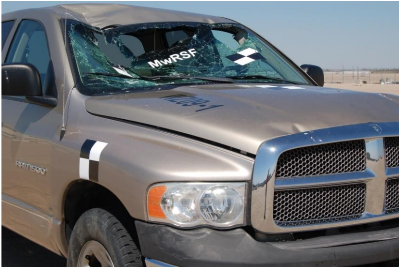
Figure 58. Vehicle Damage, Test No. WZ09-1
