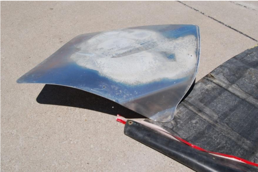
Figure 67. System Damage, Test No. WZ09-2A
