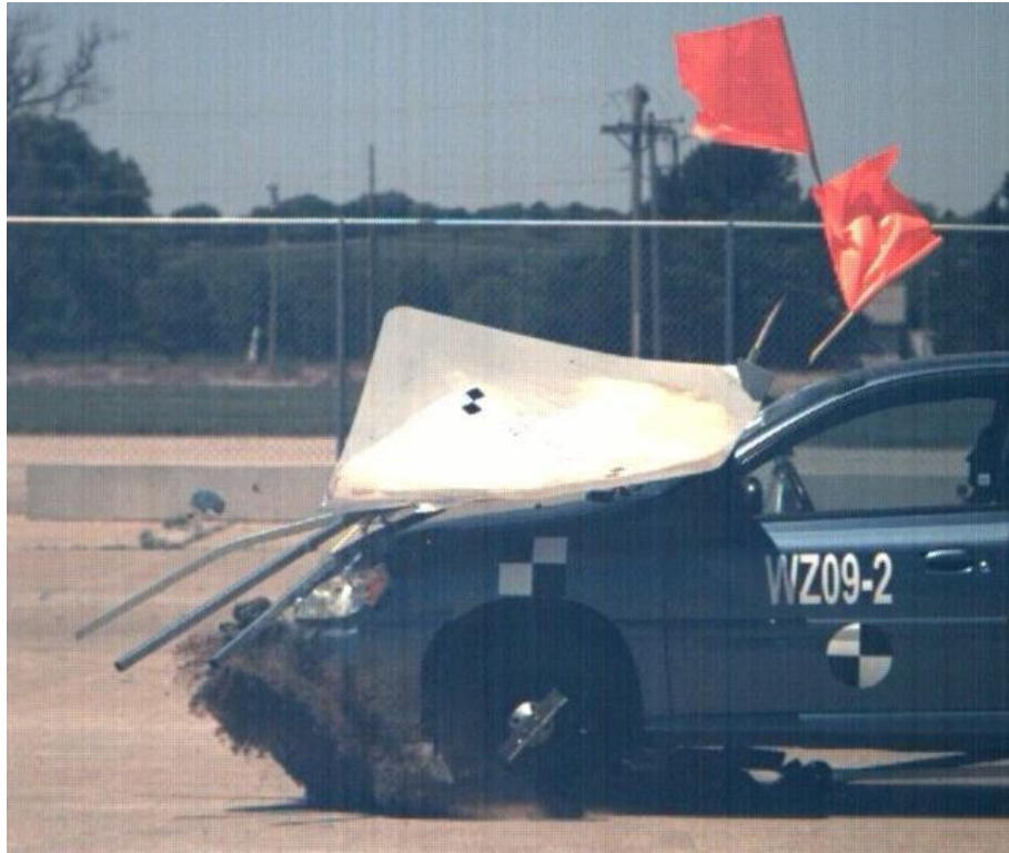
Figure 105. System No. 2B, Tripod Oriented at 90 Degrees
