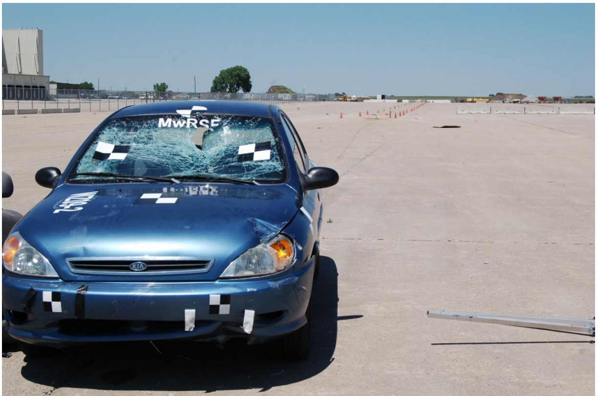
Figure 66. Vehicle Final Position and Trajectory Marks, Test No. WZ09-2
