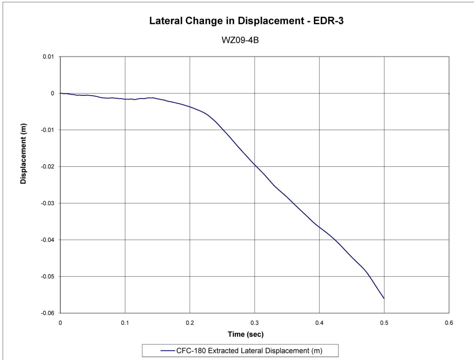
Figure I-13. Lateral Occupant Displacement (EDR-3), Test No. WZ09-4B
