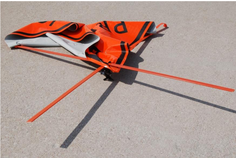
Figure 96. System Damage, Test No. WZ09-4A
