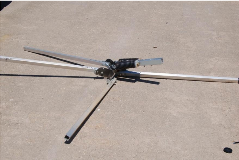
Figure 68. System Damage, Test No. WZ09-2A
