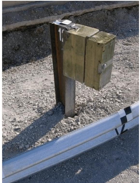
Figure 60. Post Nos. 9 through 12 Damage, Test No. MGS221-2
