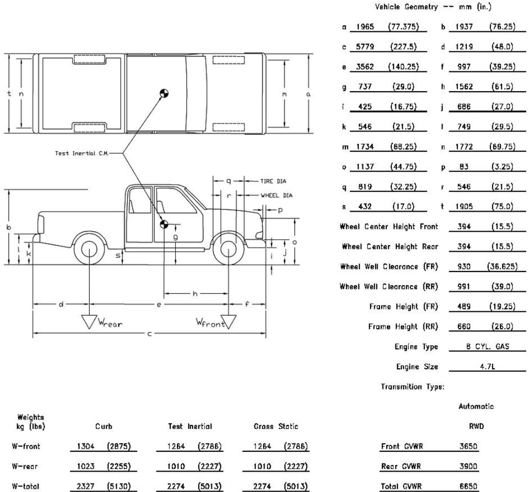
Figure 8. Test Vehicle Dimensions, Test No. MGS221-2
