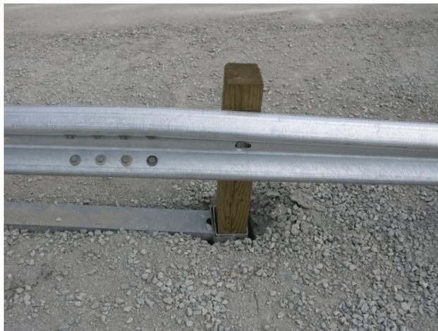
Figure 40. Upstream Anchorage Damage, Test No. MGS221-1
