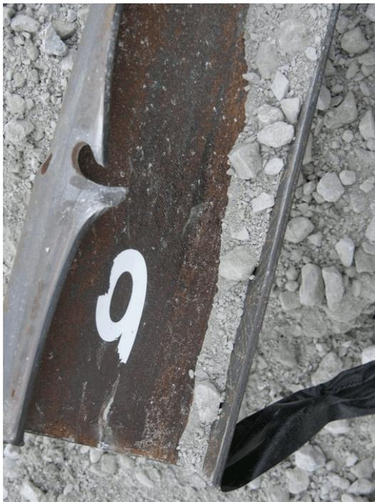
Figure 62. Post Nos. 16 through 18 Damage, Test No. MGS221-2
