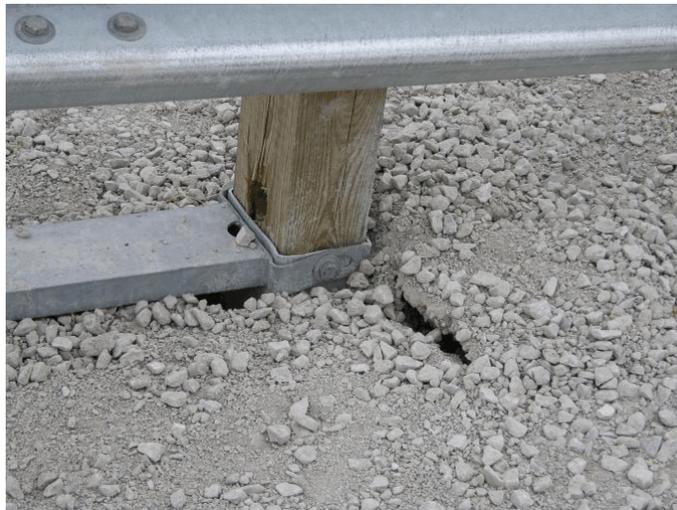
Figure 63. Upstream Anchorage Damage, Test No. MGS221-2
