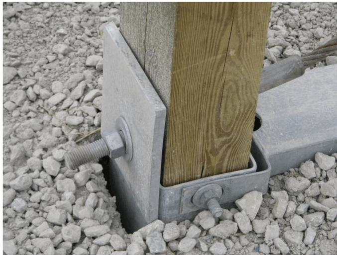
Figure 64. Downstream Anchorage Damage, Test No. MGS221-2
