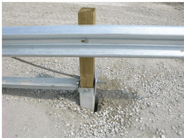
Figure 41. Downstream Anchorage Damage, Test No. MGS221-1
