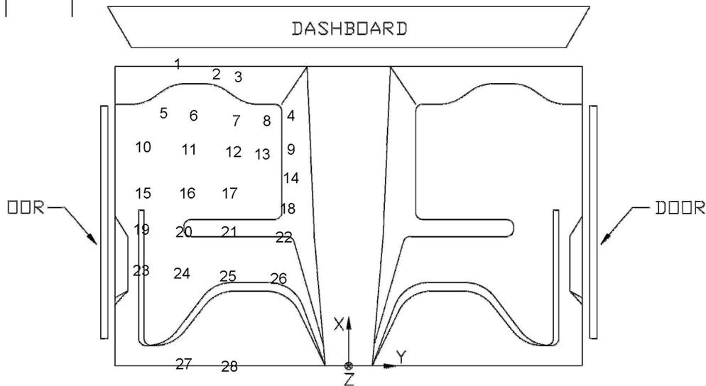
Figure H-1. Occupant Compartment Deformation Data - Set 1, Test MGS221-2
