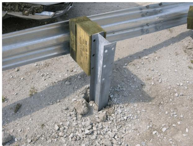
Figure 39. Post Nos. 25 through 27 Damage, Test No. MGS221-1
