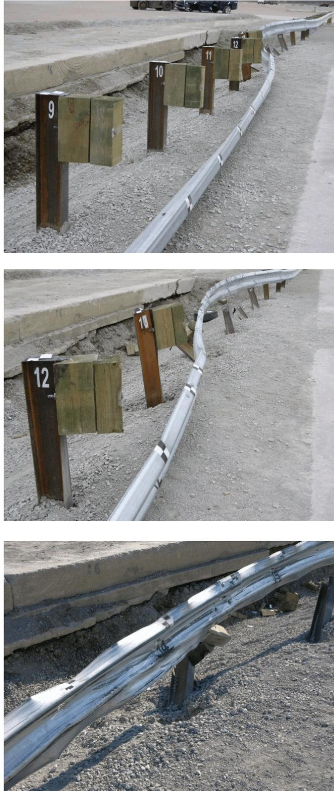
Figure 59. System Damage, Test No. MGS221-2
