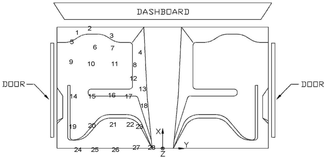
Figure E-1. Occupant Compartment Deformation Data - Set 1, Test MGS221-1
