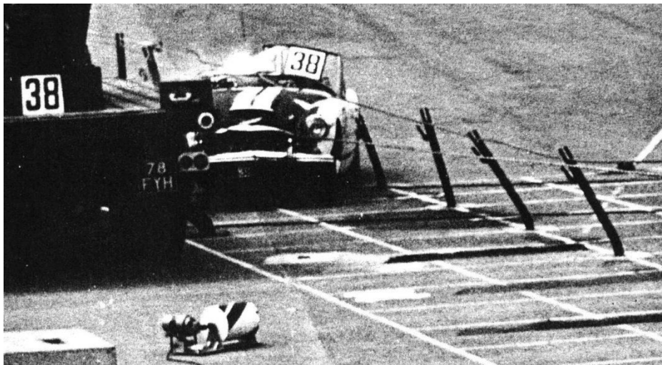
Figure 17. Upper Cable Impact Into Windshield, Test No. 38, 1967 [18]
