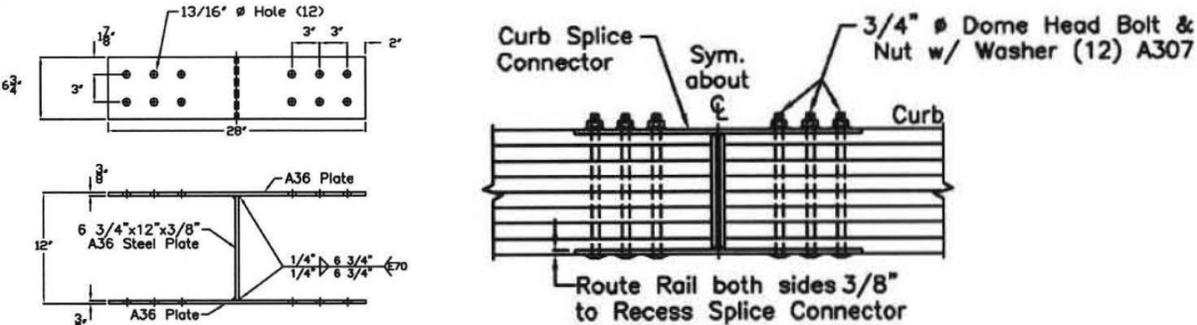
Figure 94. Curb Rail Splice Assembly for Glulam Rail and Curb on Transverse Glulam Deck [25]
