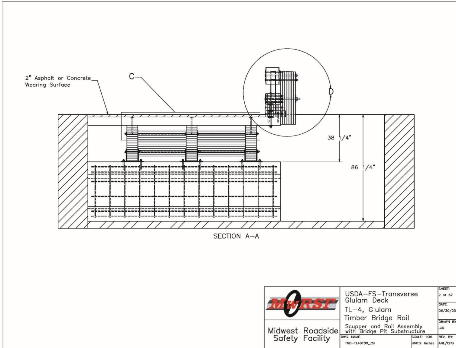
Figure O-2. Full-Scale Crash Test System Cross-Section View
