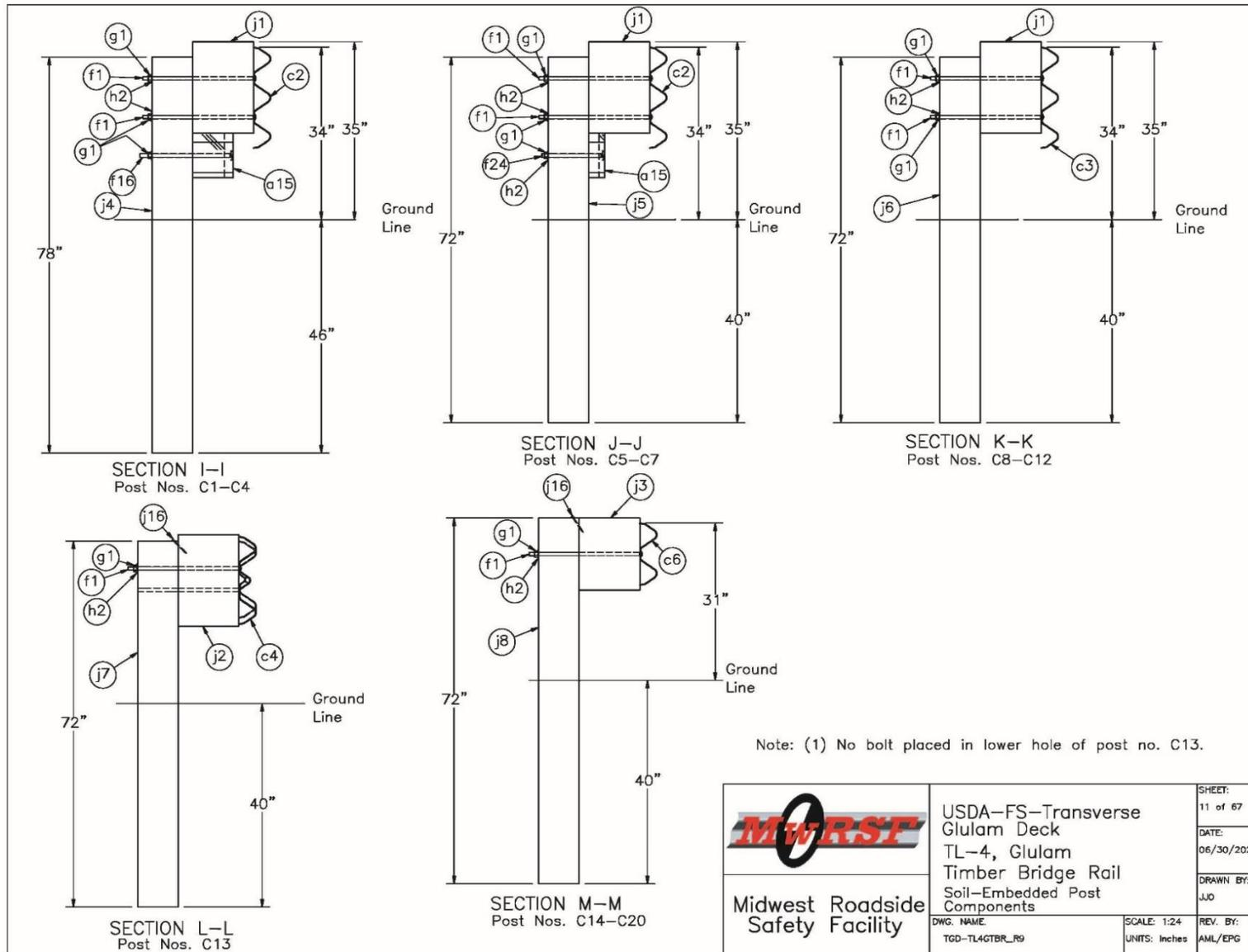
Figure O-11. AGT Post Cross-Section Views
