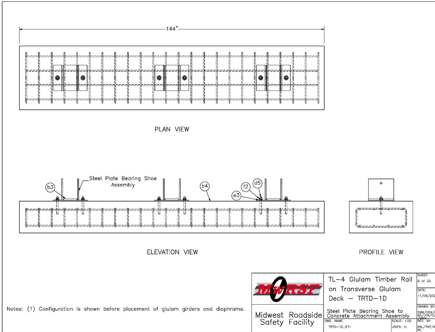
Figure 156. Concrete and Bearing Assembly Details, Test No. TRTD-1
