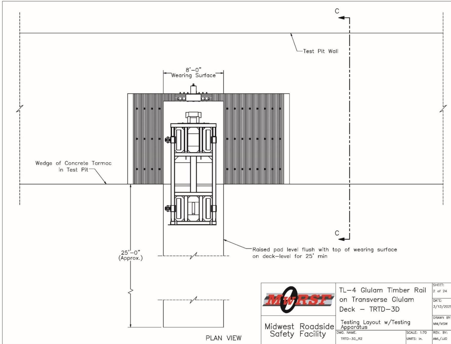
Figure N-2. Test No. TRTD-3 Layout with Bogie
