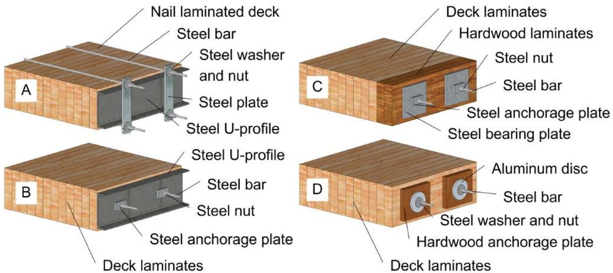
Figure 45. Stress-Laminated Deck Anchorage [68]
