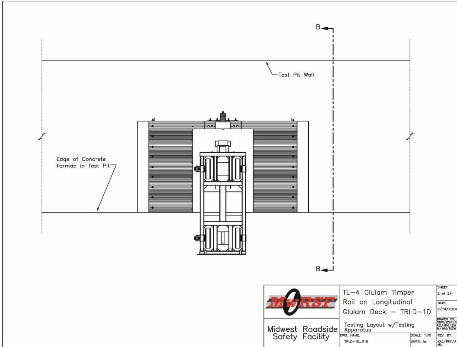
Figure 244. Layout with Bogie, Test No. TRLD-1
