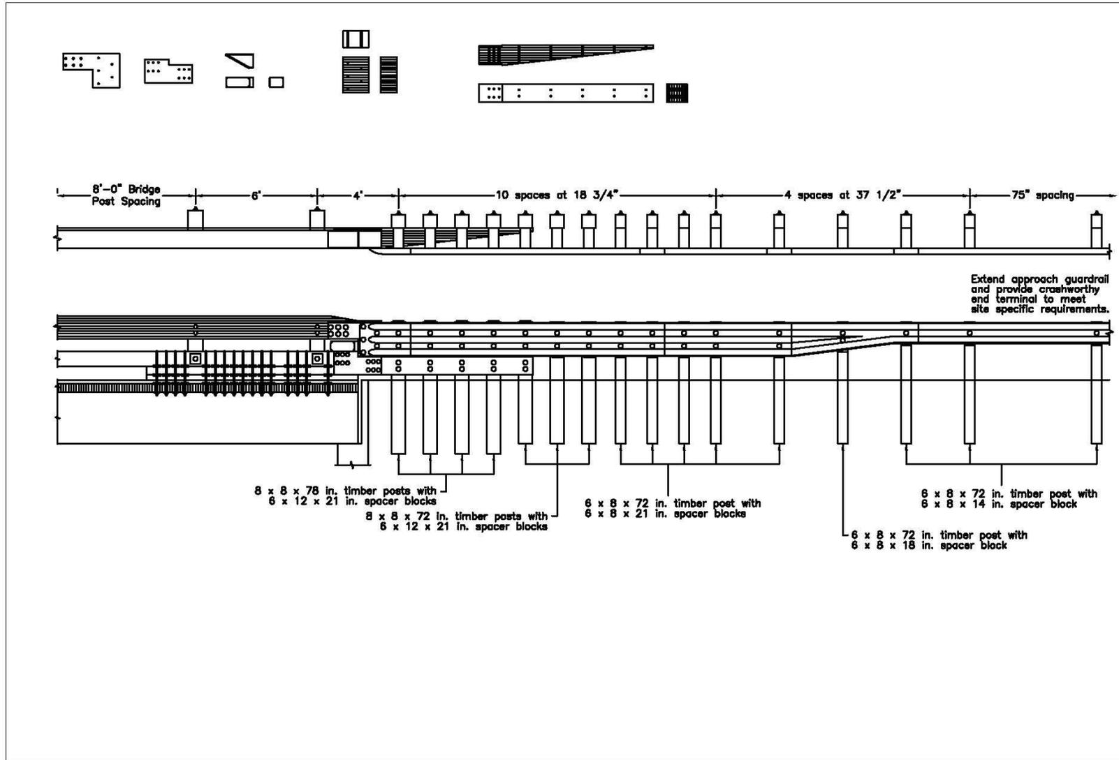
Figure K-4. Option 1.4 – Quarter-Post Spacing, 4-ft and 6-ft Gaps, L-Plate, Separated Block, Steel Reverse Taper, Thick Curb Taper
