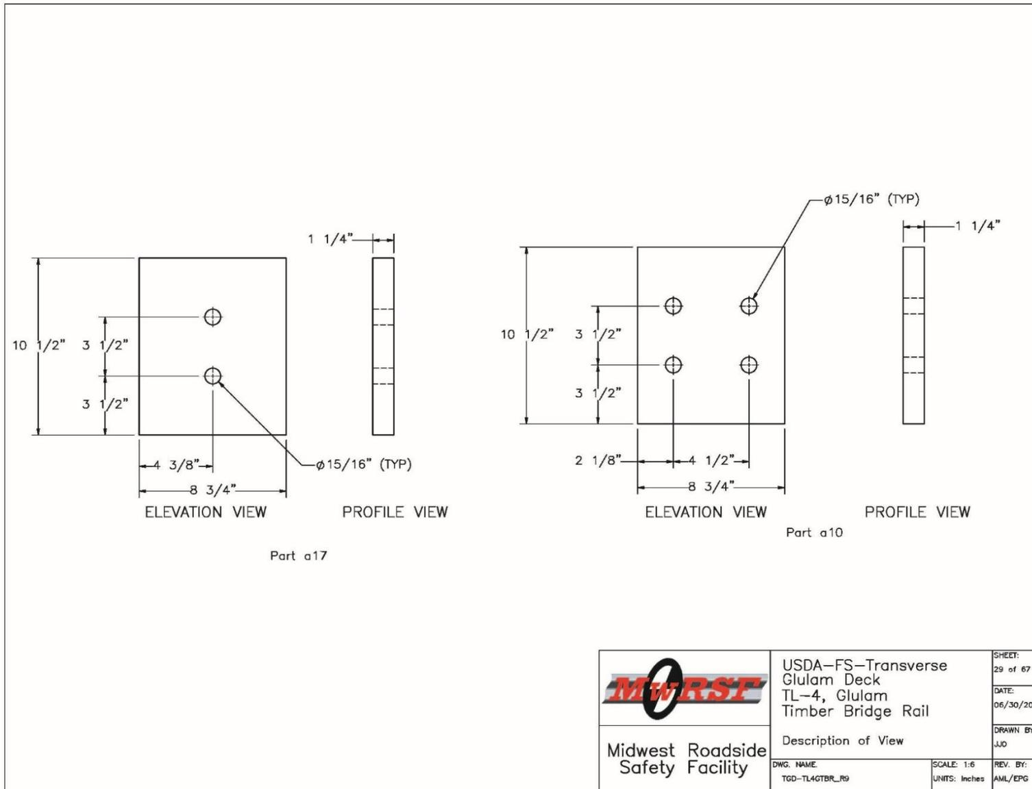
Figure O-29. Bridge Post Typical and Splice Blockout Details
