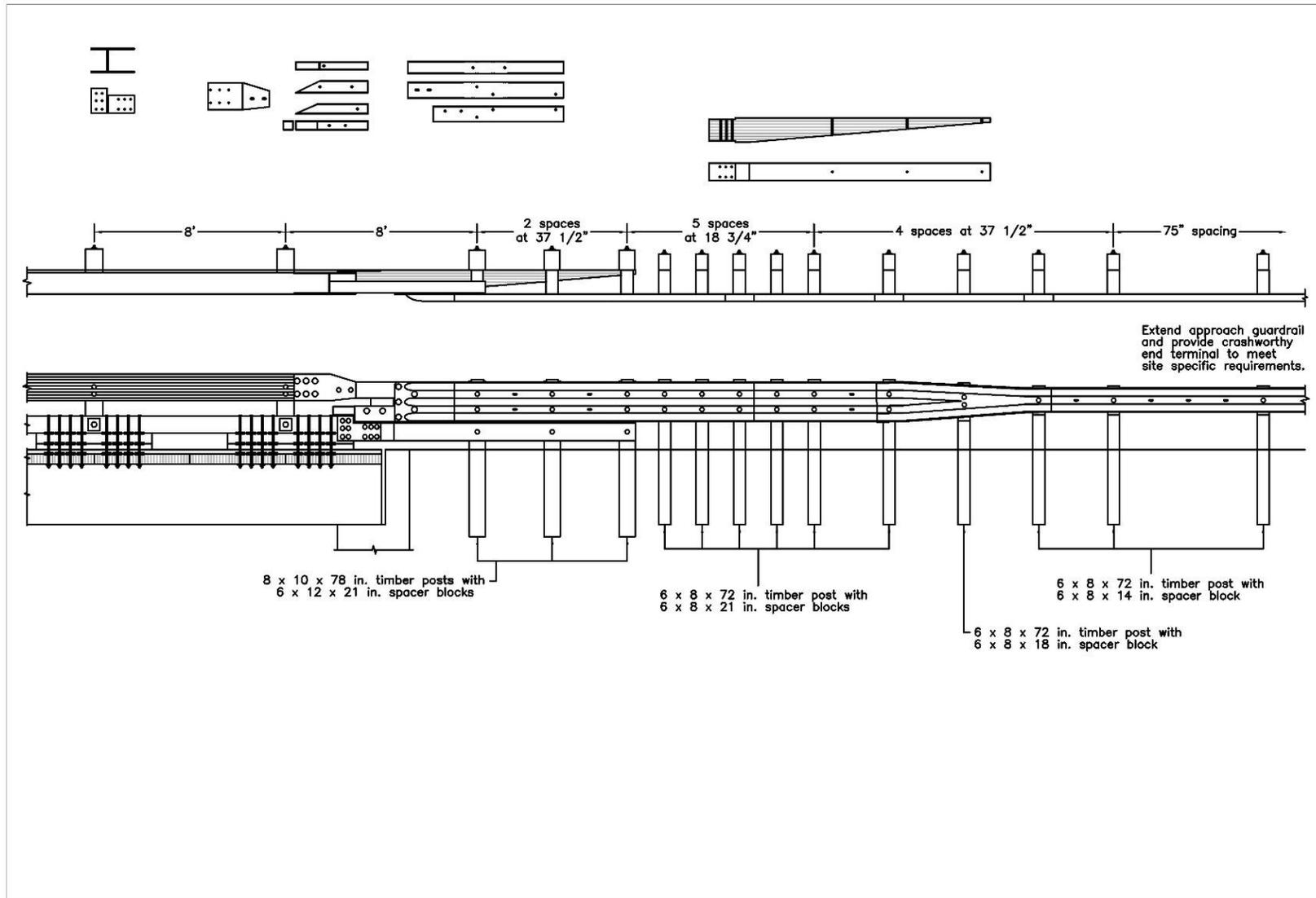
Figure K-22. Option 3.7 – Half-Post Spacing, 8-ft Gap, Steel Components, Partially Removed Blockout, Two Steel Reverse Tapers, Stepped Thick Curb Taper
