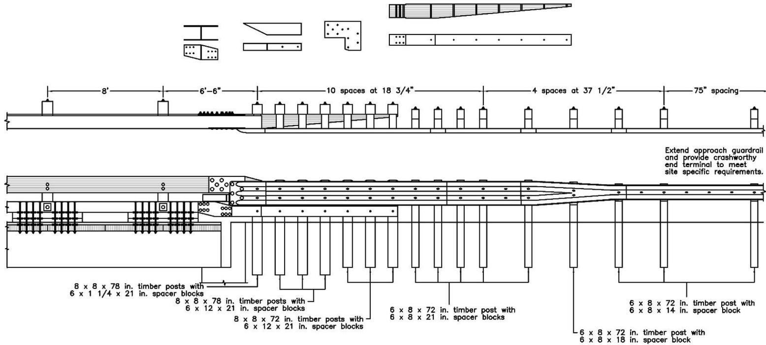
Figure K-45. Option 7.8 – Quarter-Post Spacing, 6.5-ft Gap, Notched L-Plate, Steel Reverse Taper, Stepped Curb Taper
