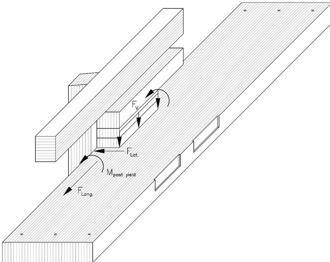
Figure 98. Longitudinal Deck External Force Diagram
