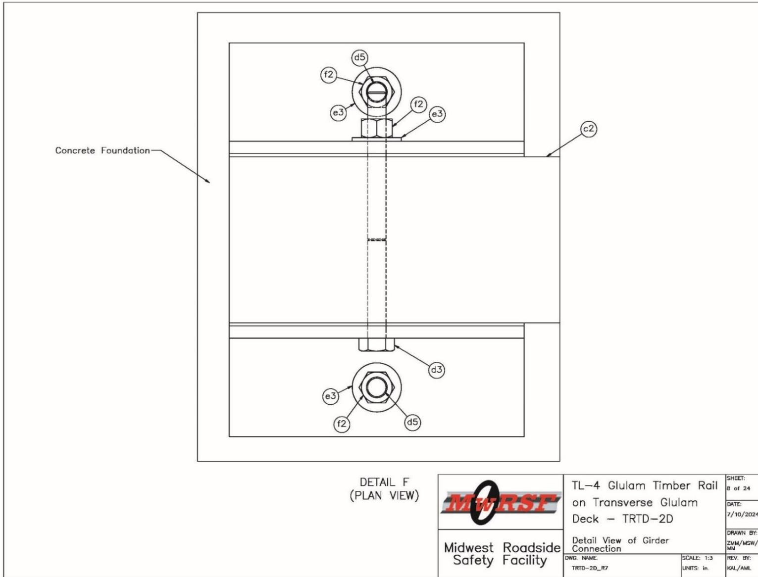
Figure 226. Girder Connection Details, Test No. TRTD-2
