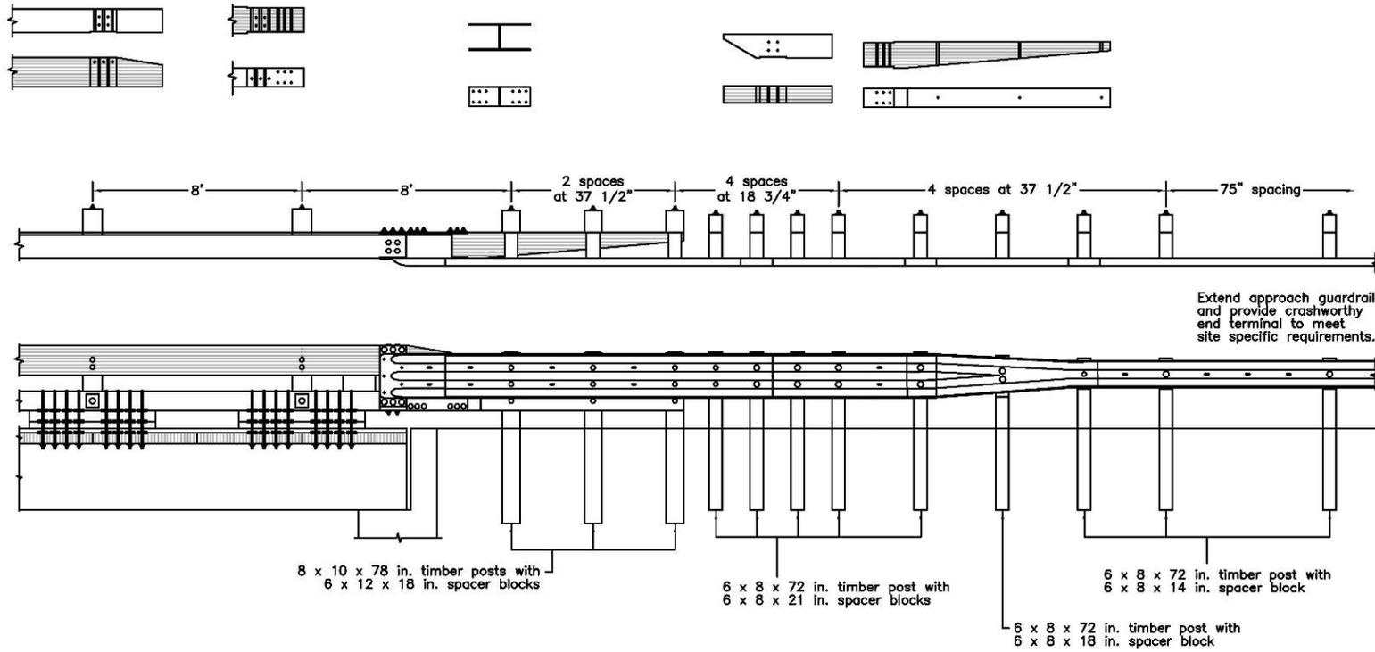
Figure K-28. Option 5.2 – Half-Post Spacing, 8-ft Gap, Welded End-Shoe, Wood Reverse Taper, Curb Taper Behind Thrie-beam
