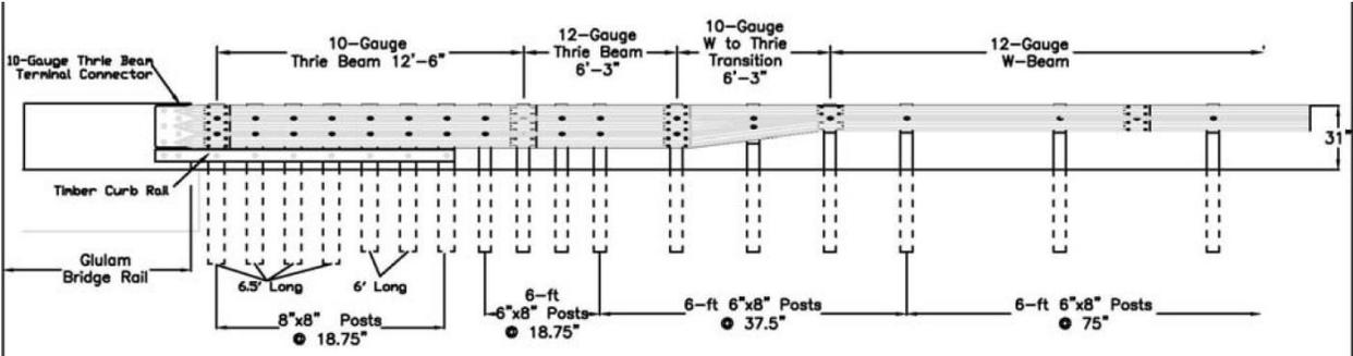
Figure 23. Proposed AGT Design Utilizing Quarter-Post Spacing [37]
