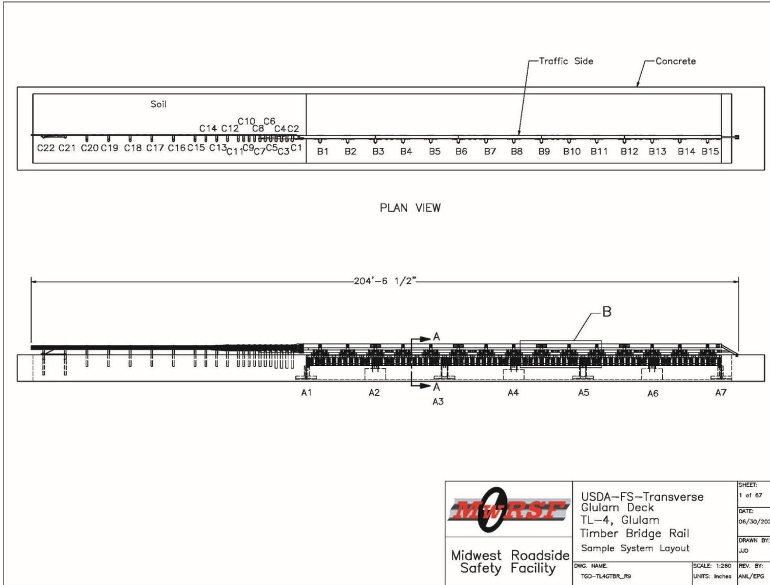
Figure O-1. Full-Scale Crash Test System Layout Plan and Elevation Views
