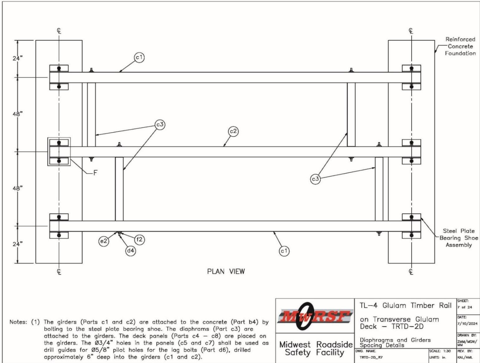
Figure 225. Diaphragm and Girder Spacing Details, Test No. TRTD-2
