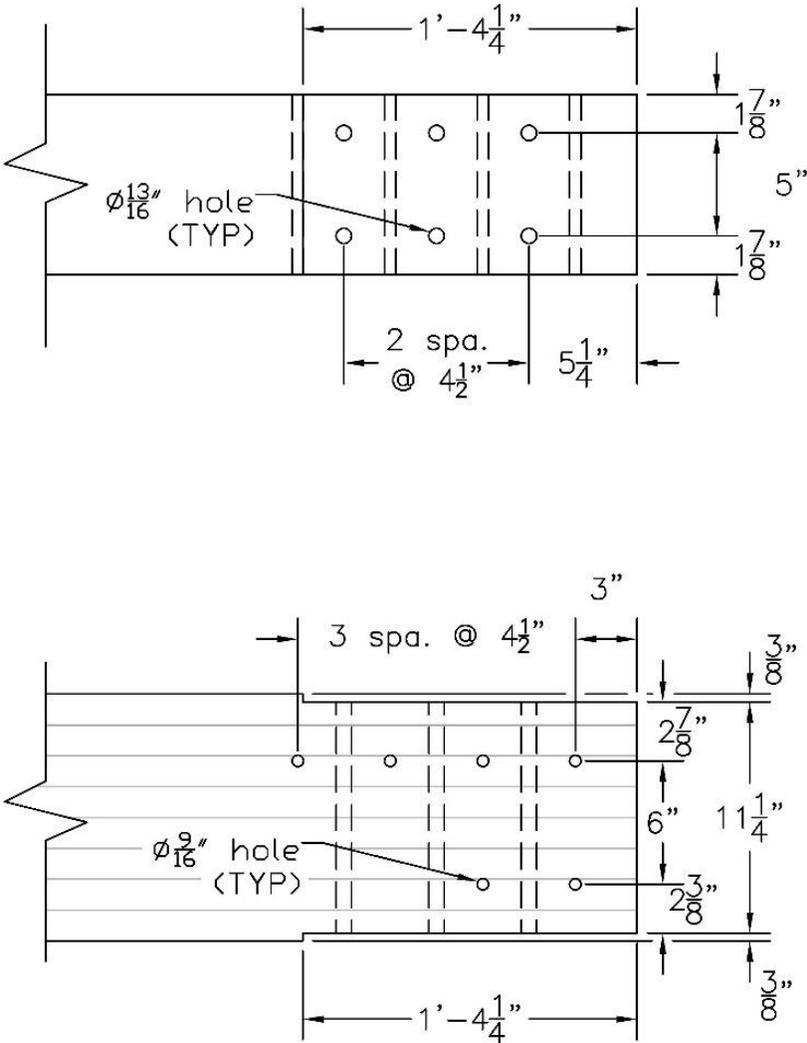
Figure 119. Cuts and Holes Needed at Curb Rail End for Both Systems
