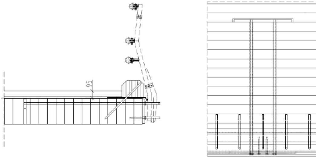
Figure 10. Bridge Railing Developed for Stress-Laminated Timber Decks in Norway: Cross-Section (left) and Plan View (right) [deck stressing rods not shown for clarity] [28]
