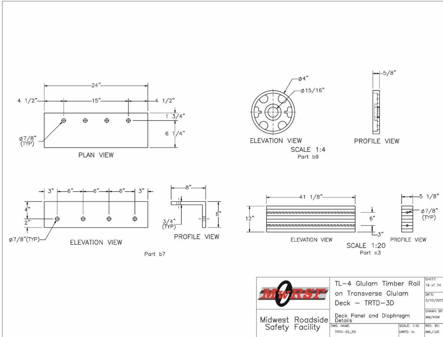
Figure 269: Test No. TRTD-3 Tarmac Angle Restraint, Diaphragm, and Shear Plate Details
