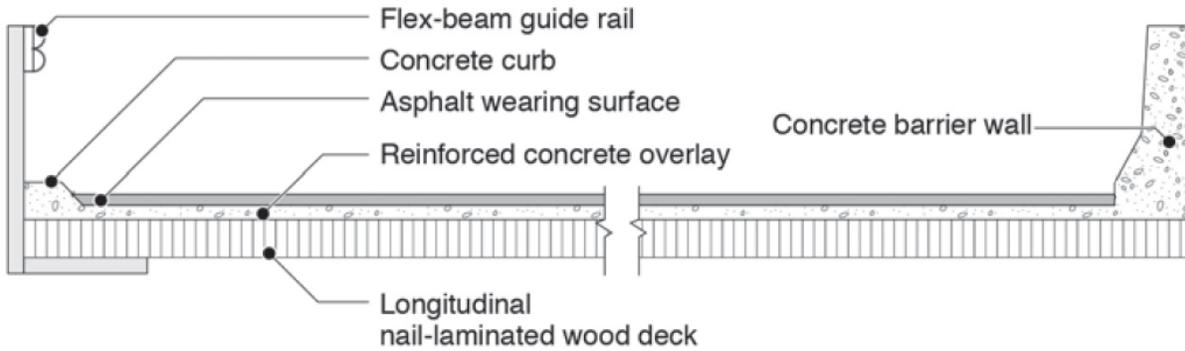
Figure 36. Cross-Section View of Timber-Concrete Composite Deck [51]
