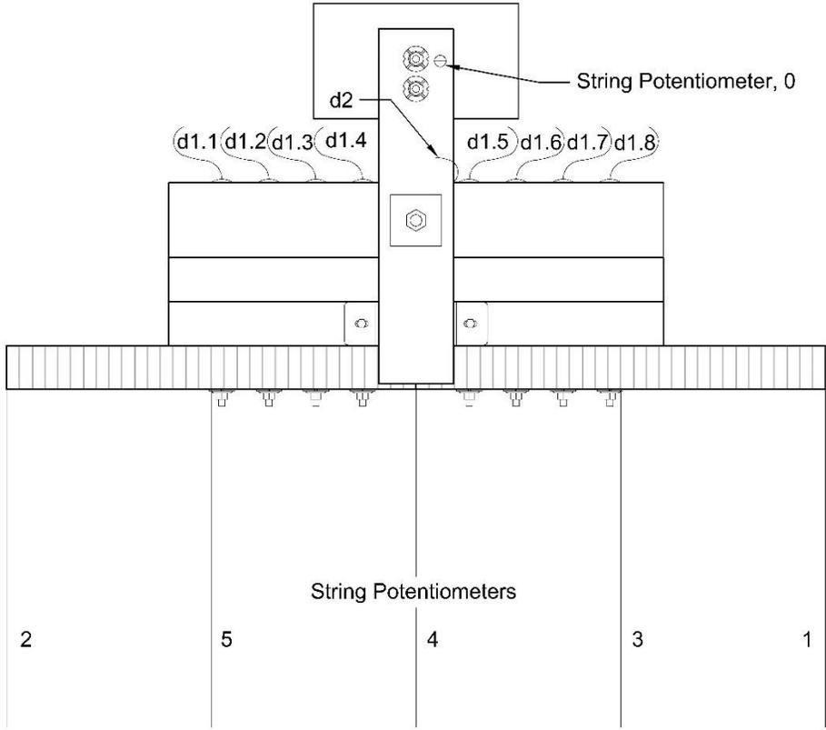
Figure 183. String Potentiometer and Bolt Axial Gauge Locations on Bridge Post System, String Potentiometers Numbered 0 to 5
