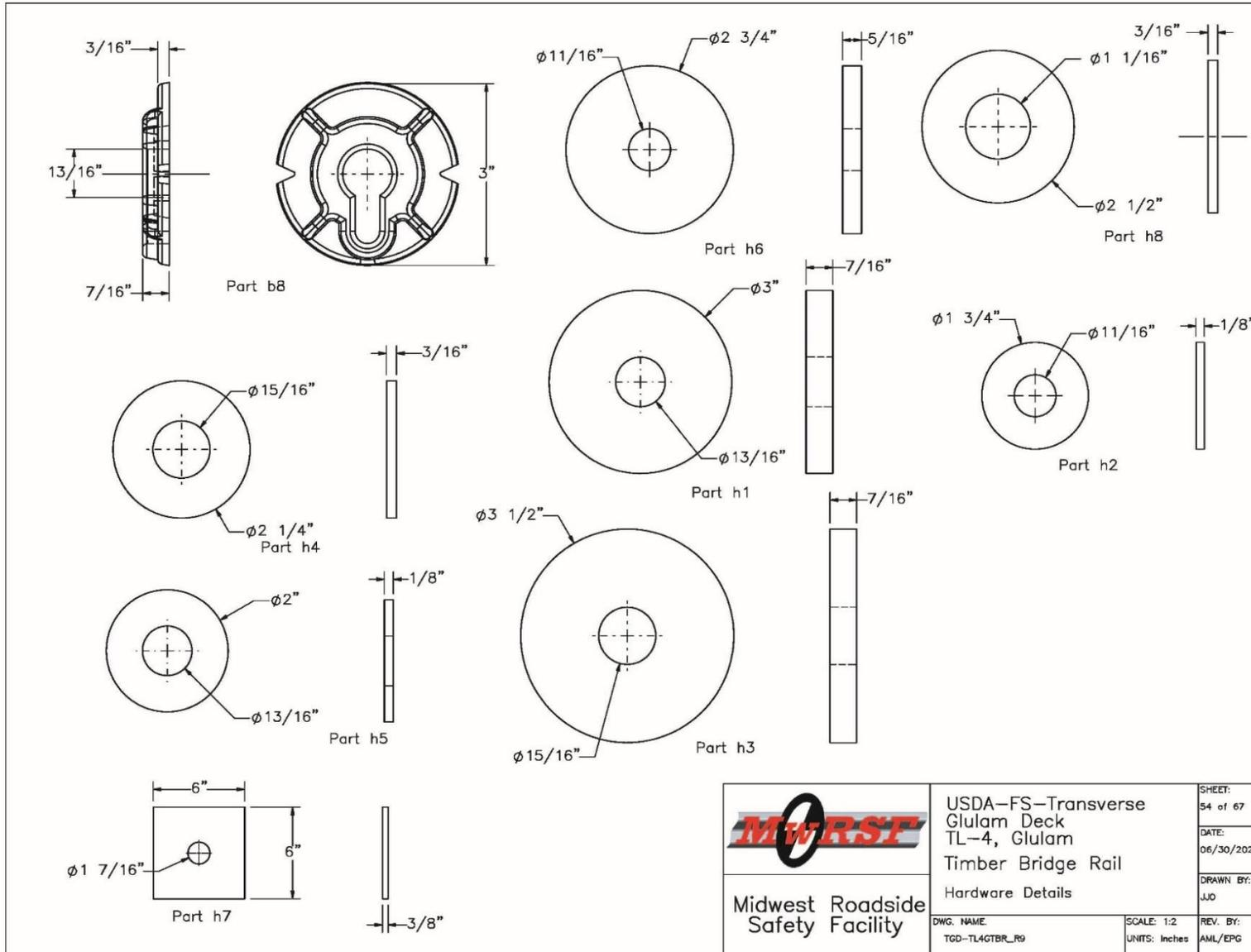
Figure O-54. Bridge Washer Hardware Details
