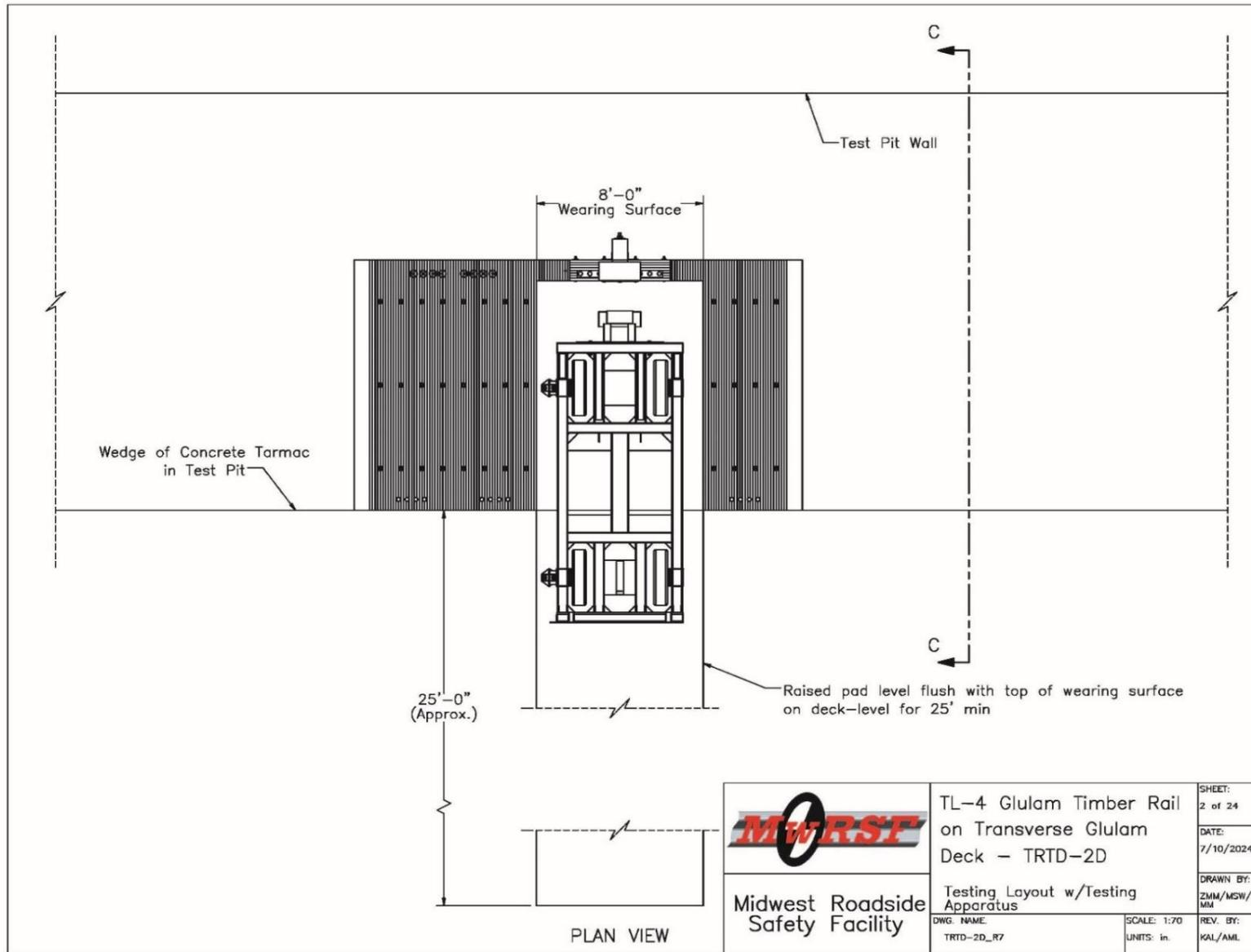
Figure 220. Test Layout with Bogie, Test No. TRTD-2
