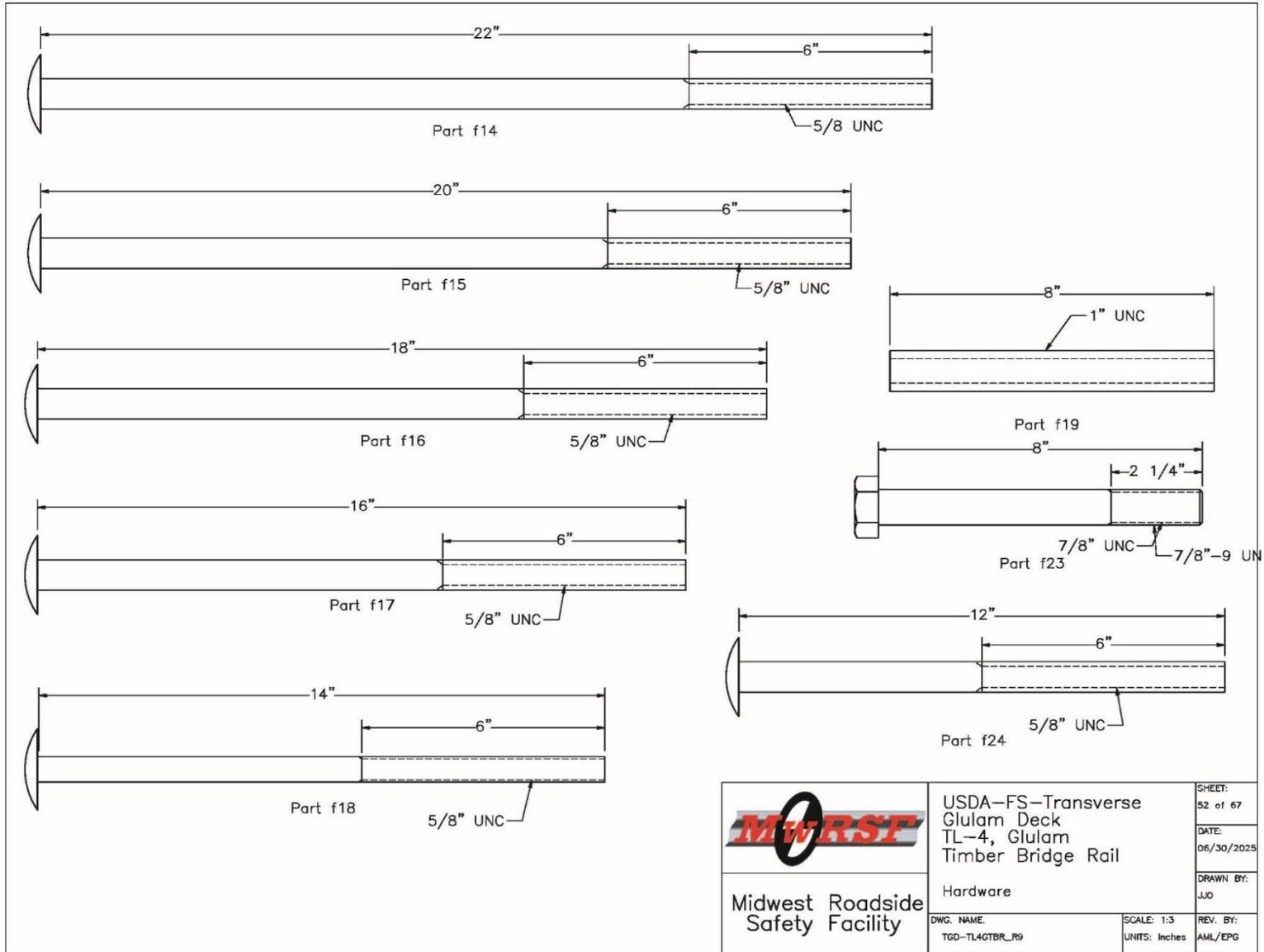
Figure O-52. Bridge Bolt Hardware Details, Page 3
