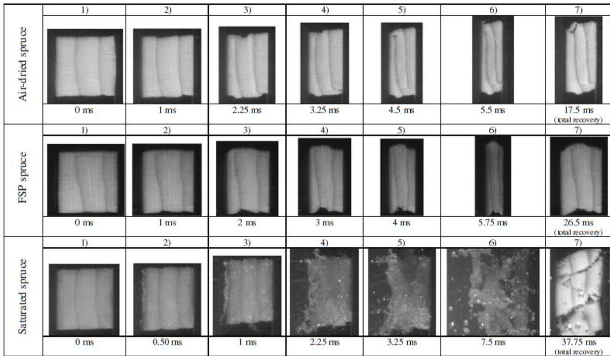
Figure 55. Results of Impact Compression Under Different Moisture Contents [88]
