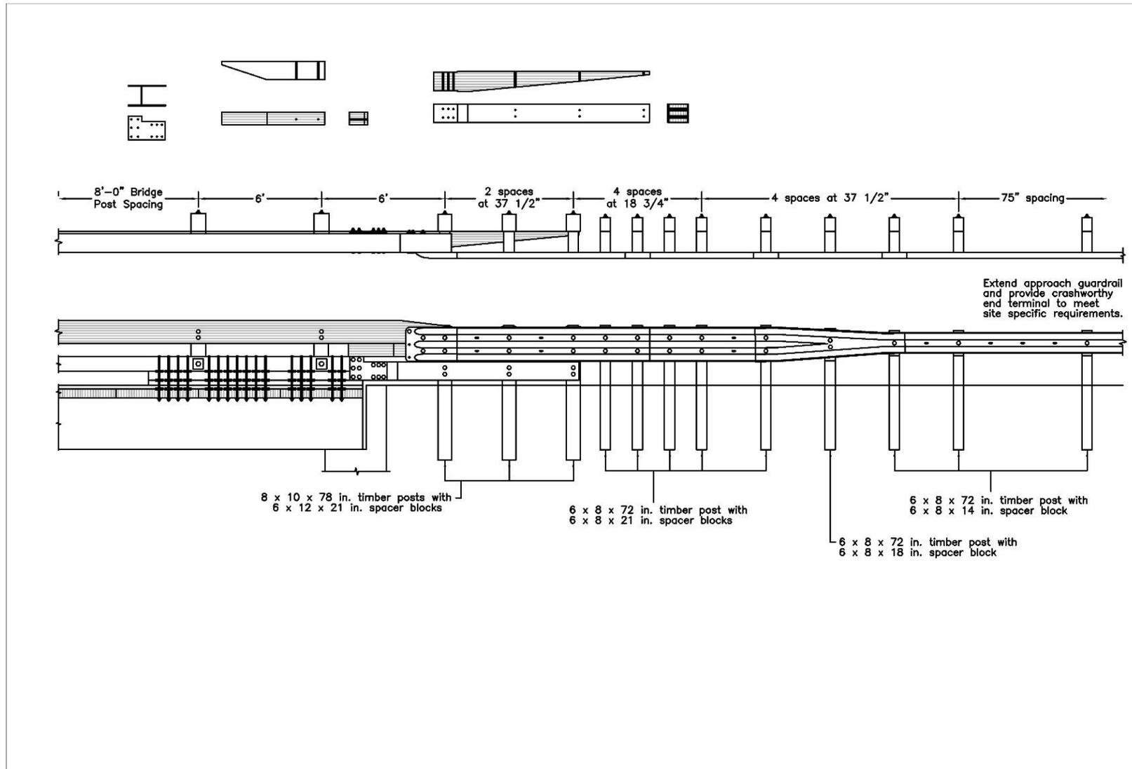
Figure K-15. Option 2.10 – Half-Post Spacing, 6-ft Gap, No Plate, Missing Bolts, Wood Reverse Taper, Stepped Thick Curb Taper
