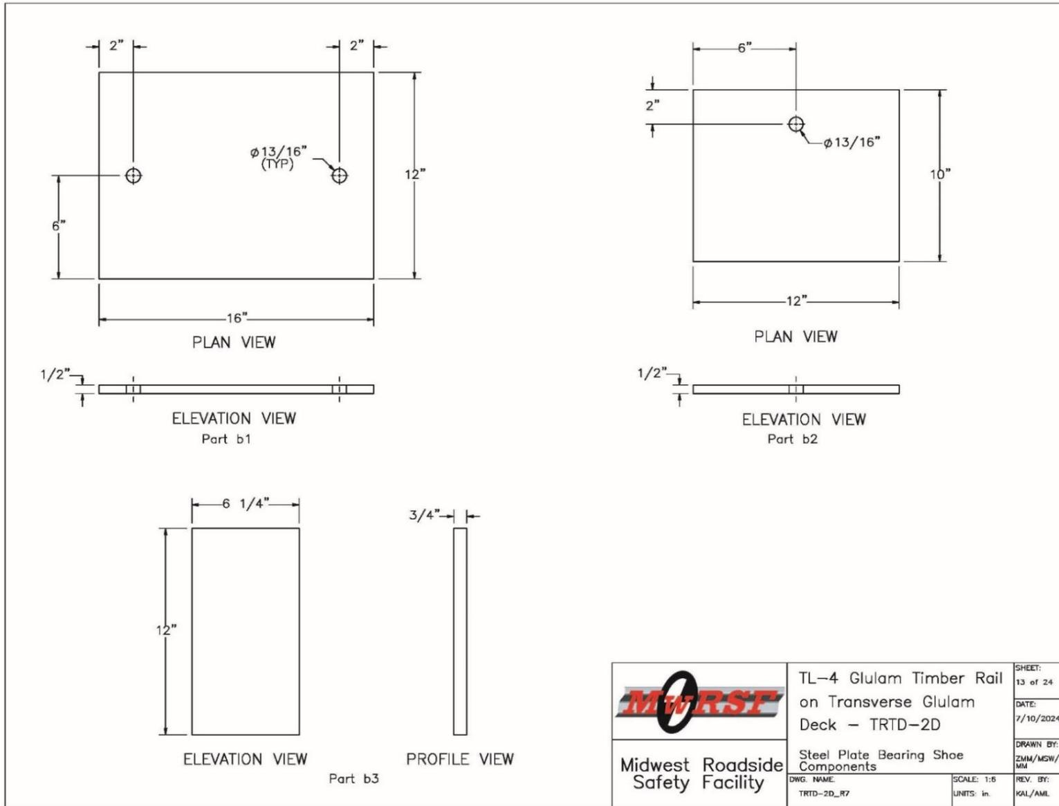
Figure 231. Steel Plate Bearing Assembly Component Details, Test No. TRTD-2
