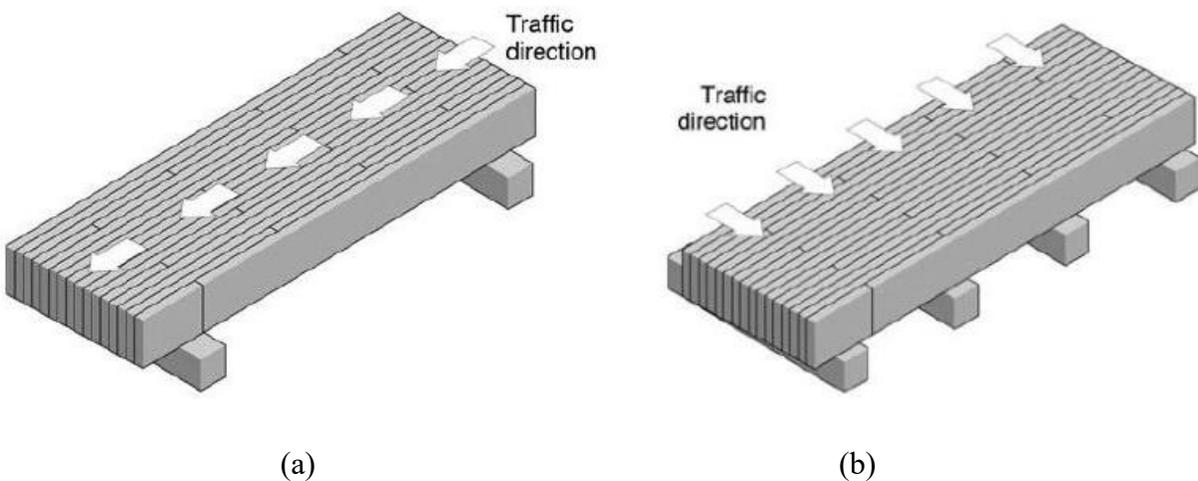
Figure 35. Nail-Laminated Decks: (a) Longitudinal and (b) Transverse [51]
