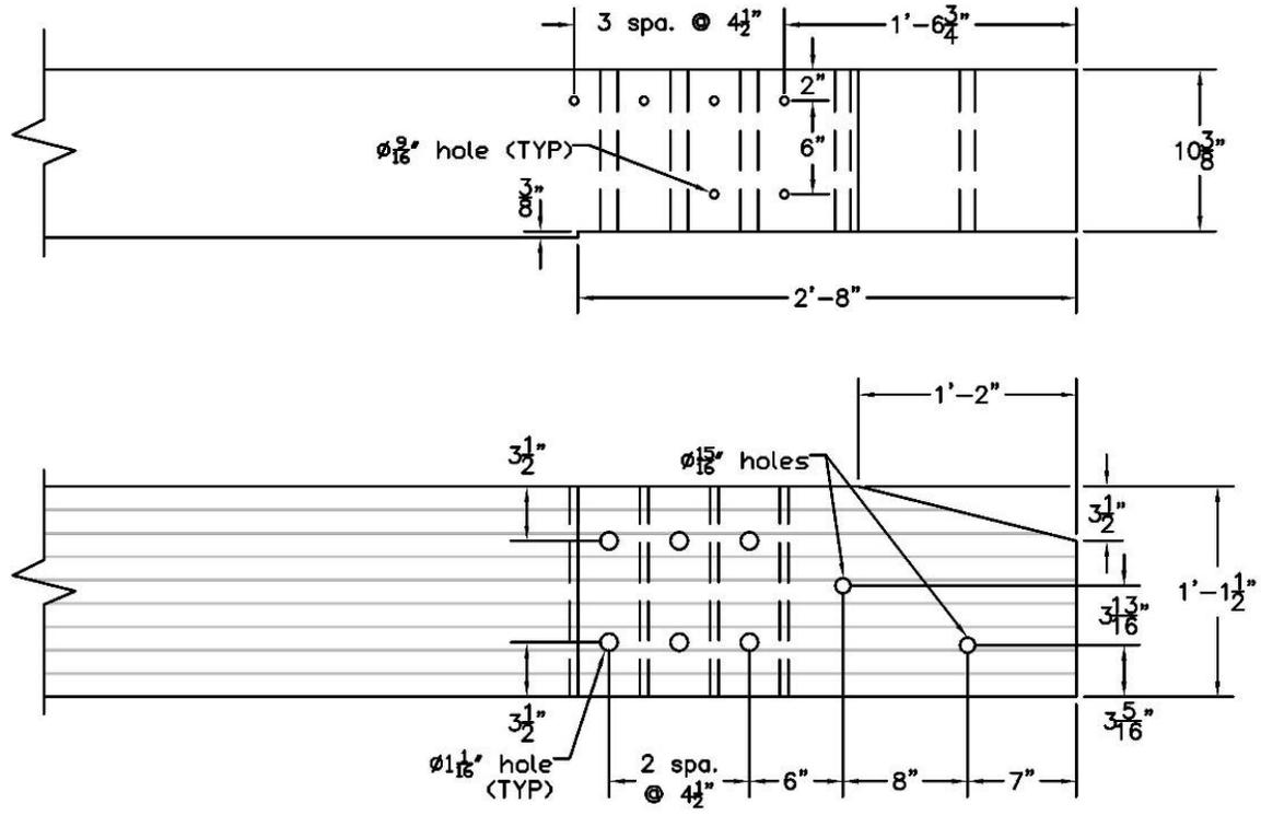
Figure 116. Cuts and Holes Needed in Upper Rail at End for Attachment to Quarter-Post System
