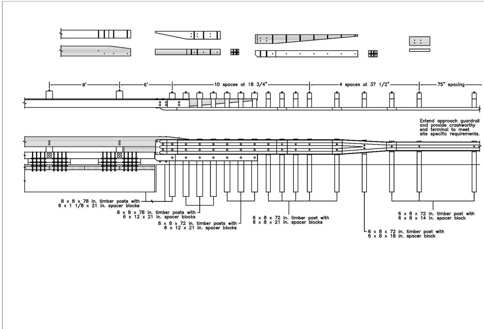
Figure K-7. Option 2.2 – Quarter-Post Spacing, No Plate, Missing Bolts, Removed Blockouts, Wood Reverse Taper, Separated Stepped Curb Taper
