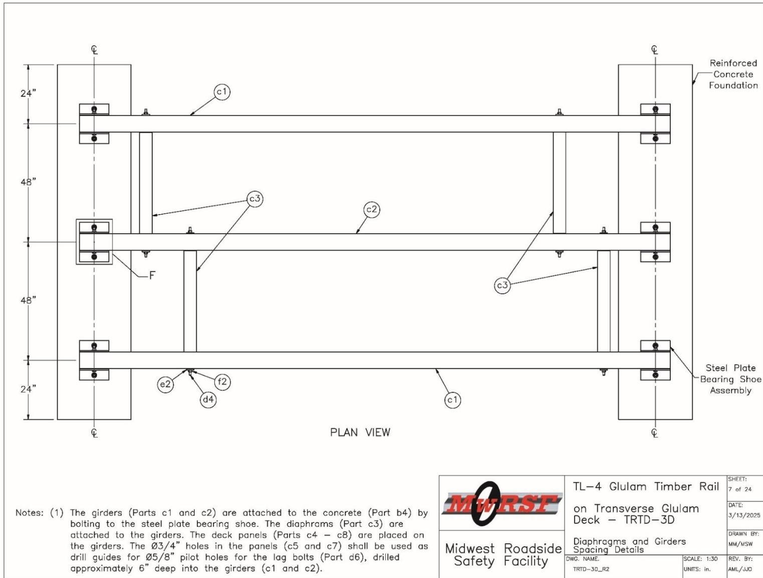
Figure N-7. Test No. TRTD-3 Diaphragms and Girders Spacing Details
