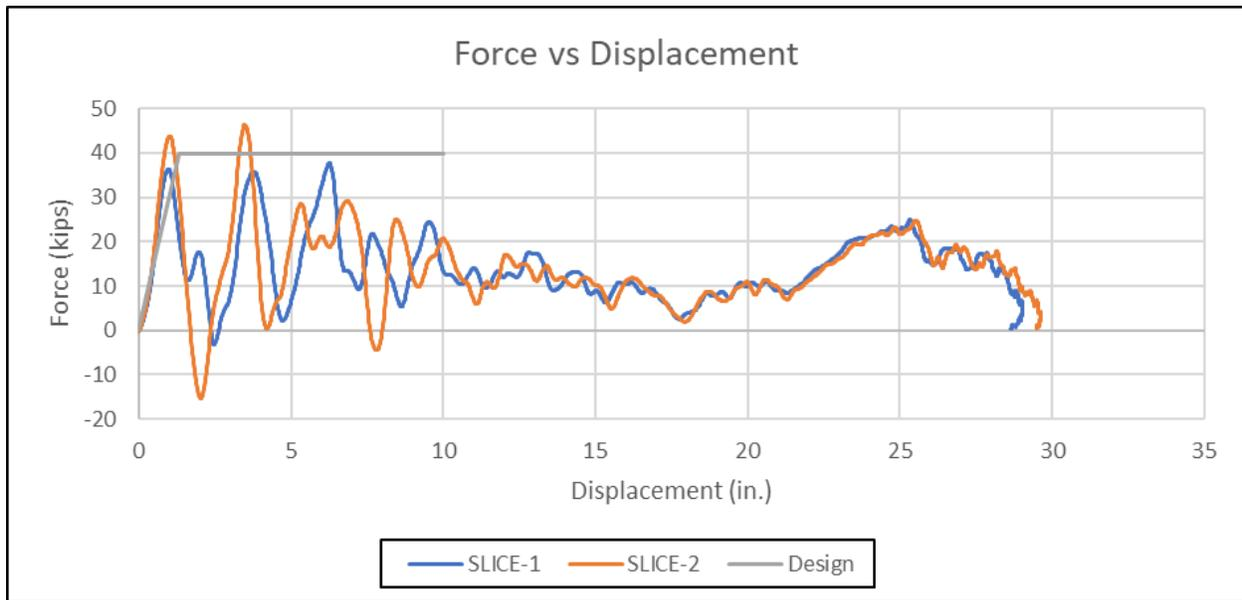
Figure 213. Force vs. Displacement with Design Load, Test No. TRTD-1
