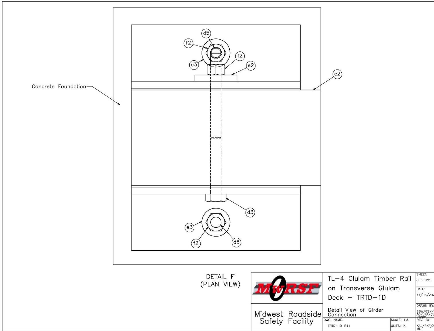
Figure 155. Girder Connection Details, Test No. TRTD-1
