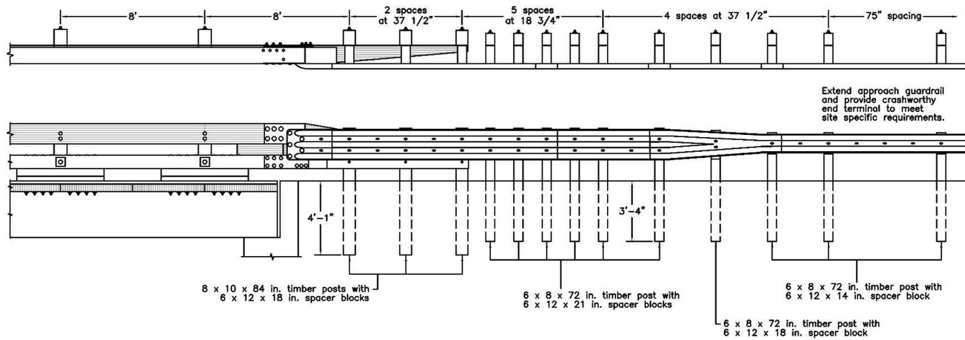
Figure 113. Half-Post MASH 2016 TL-3 AGT between TL-4 Bridge Rail and MGS
