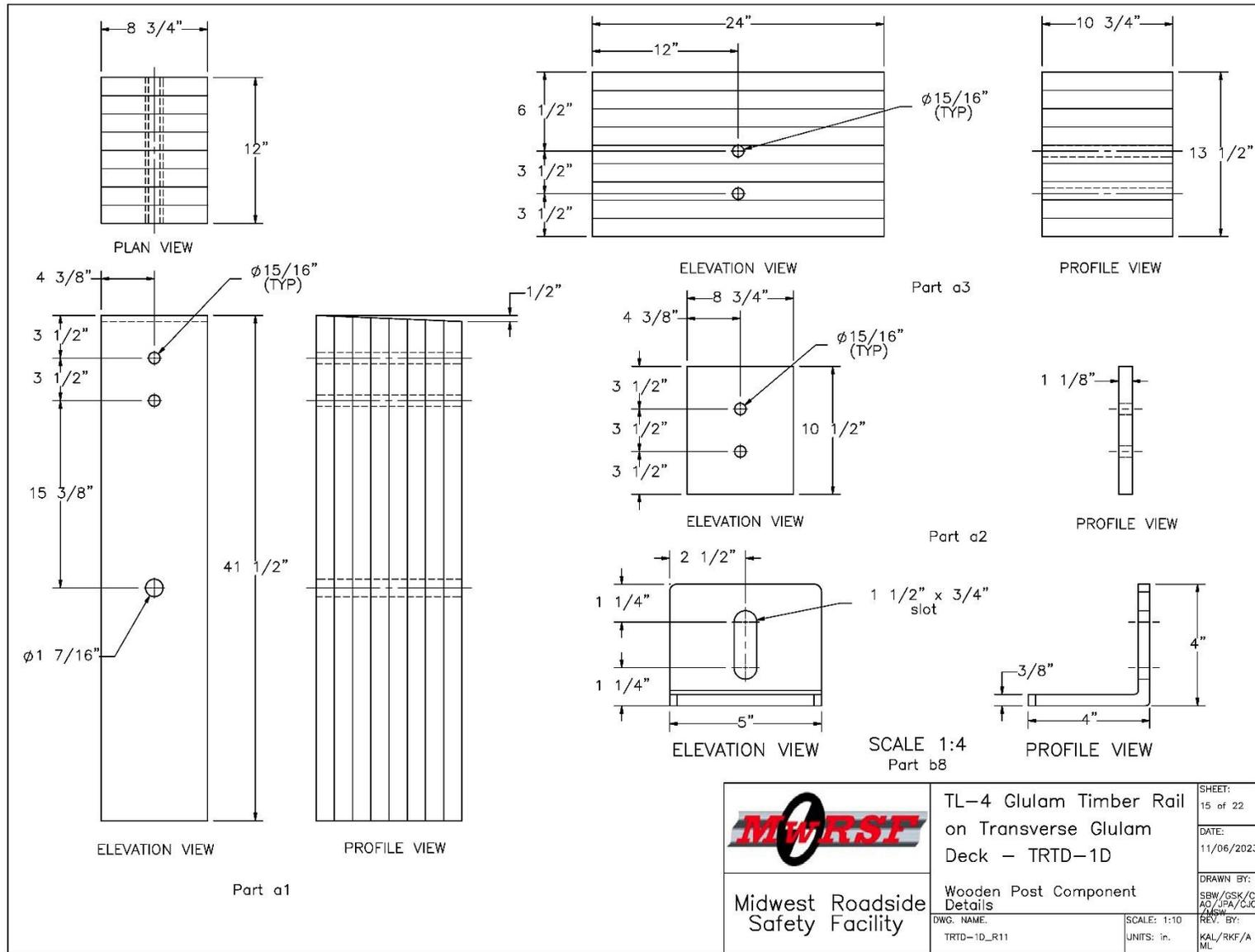
Figure 162. Vertical Post, Upper Rail, Blockout, and Angle Guide Details, Test No. TRTD-1
