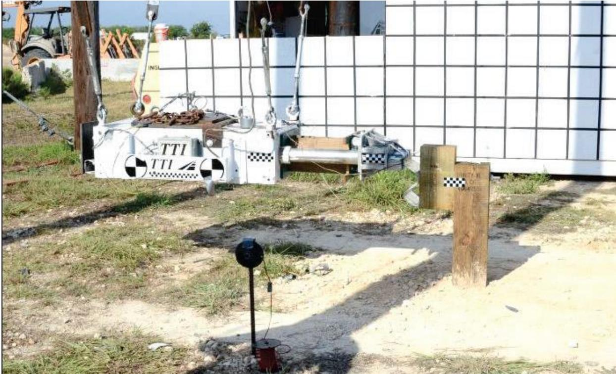
Figure 31. Pendulum Testing Setup on Timber Guardrail Posts [44]
