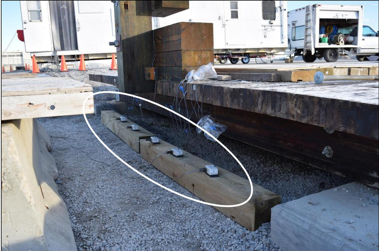
Figure 186. Test No. TRTD-1 String Potentiometers Measuring Deck Deflection
