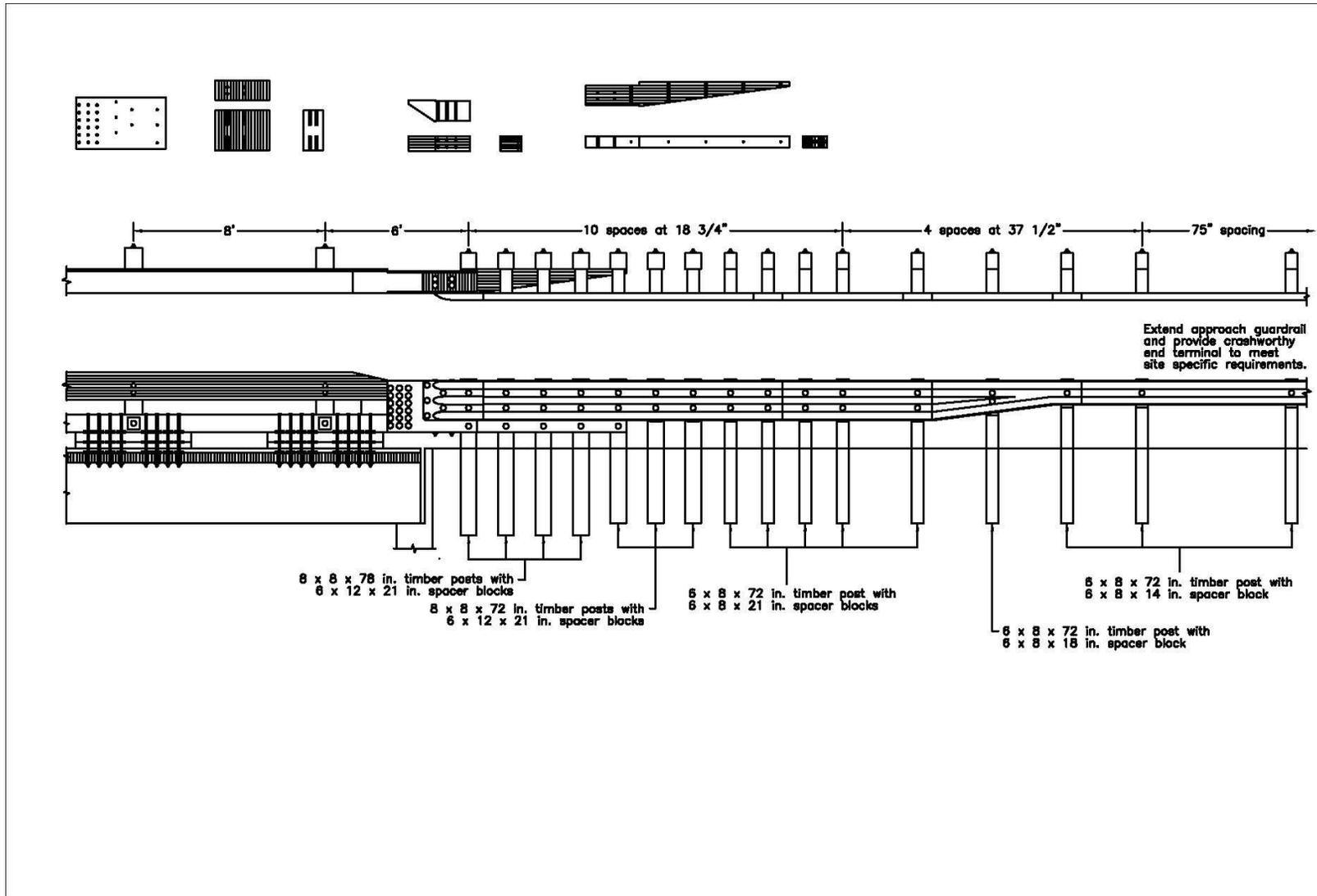
Figure K-3. Option 1.3 – Quarter-Post Spacing, 6-ft Gap, Plate, Separated Block, Removed Blockouts, Wood Reverse Taper, Thin Curb Taper
