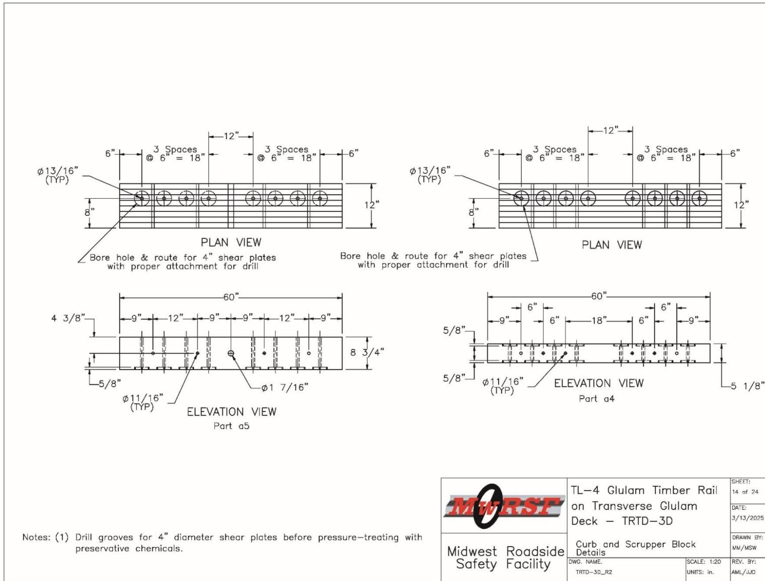
Figure N-14. Test No. TRTD-3 Scupper and Curb Rail Details
