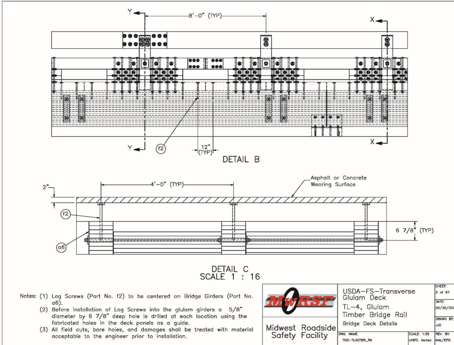
Figure O-3. Full-Scale Bridge System Superstructure Details
