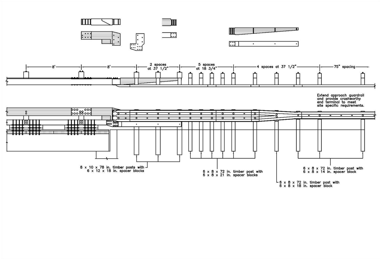
Figure K-29. Option 5.3 – Half-Post Spacing, 8-ft Gap, Custom Glulam Piece, Stepped Curb Taper
