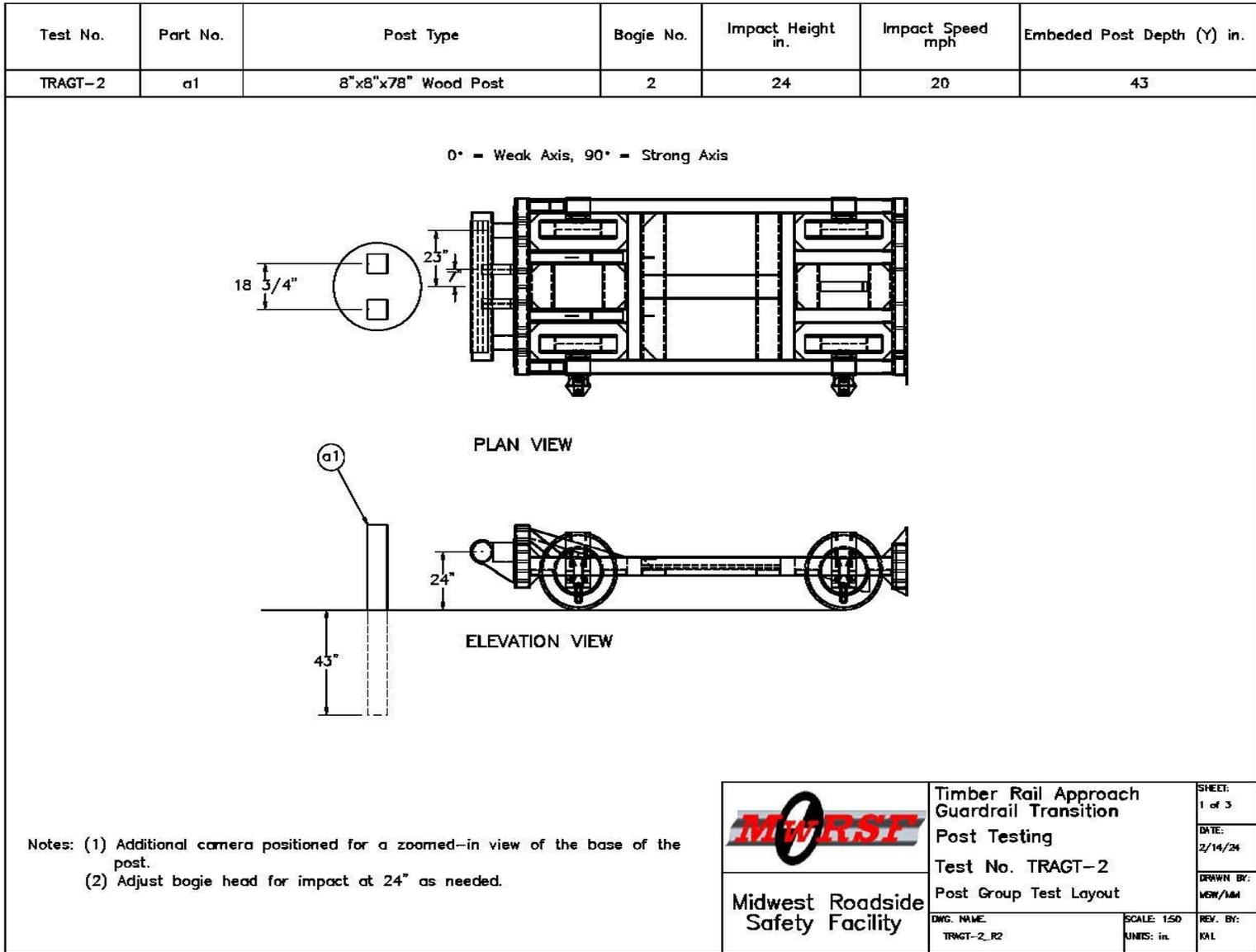
Figure 127. Test Layout, Impact on Single Post, Test No. TRAGT-2
