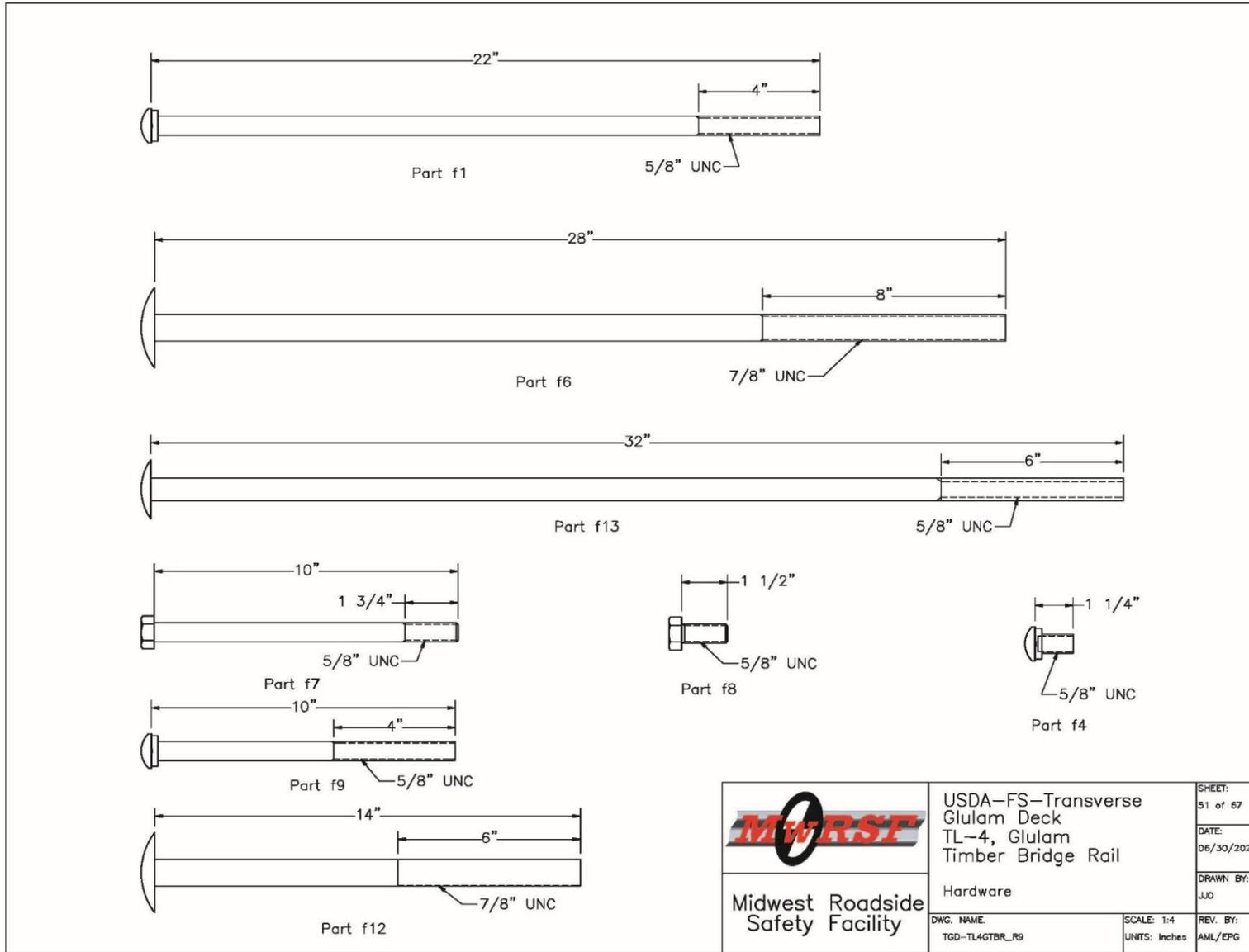
Figure O-51. Bridge Bolt Hardware Details, Page 2
