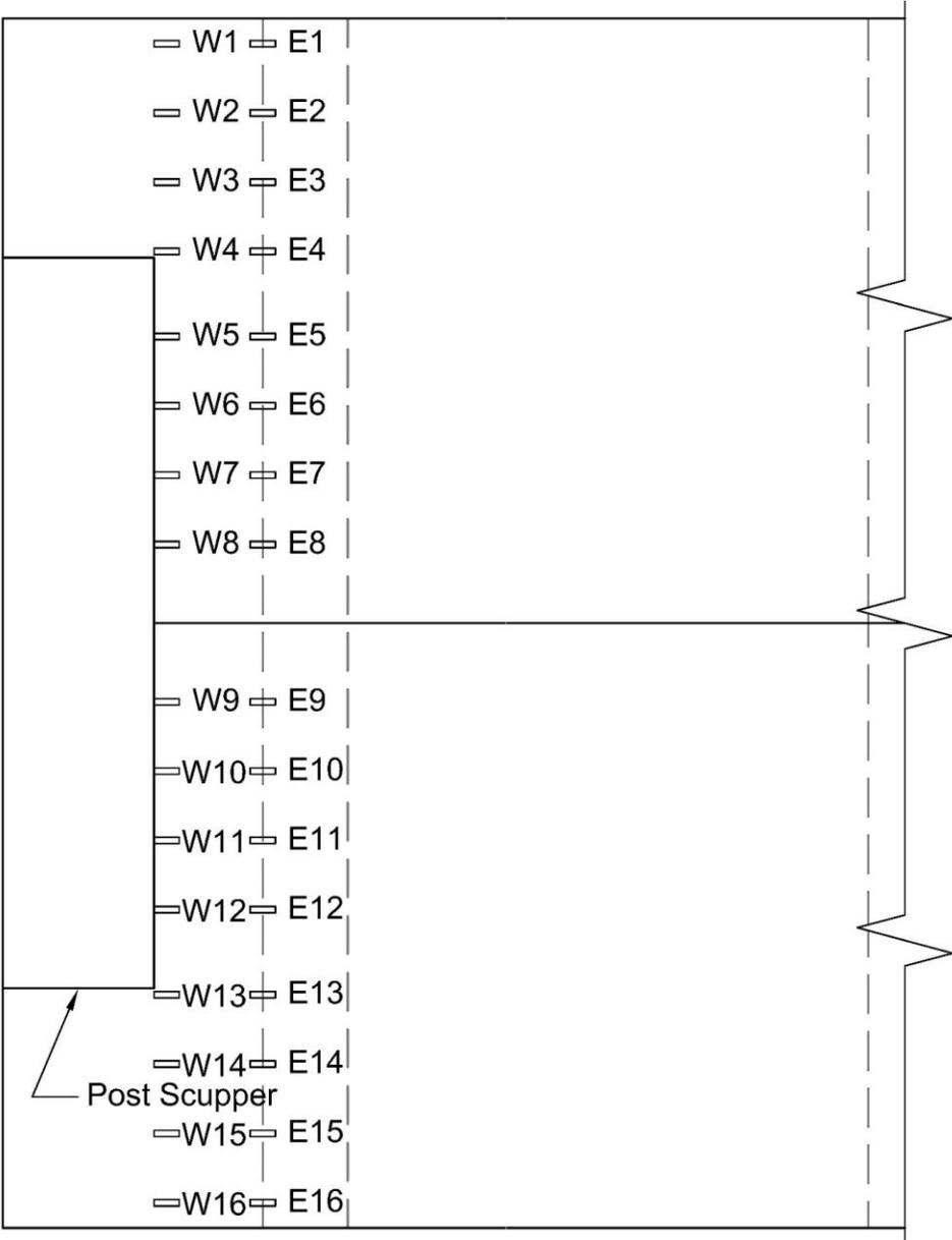
Figure 181. TRTD-1 Deck Surface Strain Gauge Locations (dashed lines denote girder edges)
