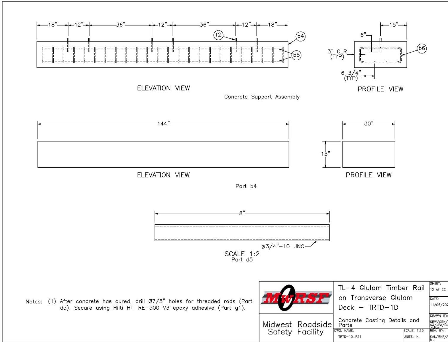
Figure 157. Concrete Casting and Embedded Rod Details, Test No. TRTD-1
