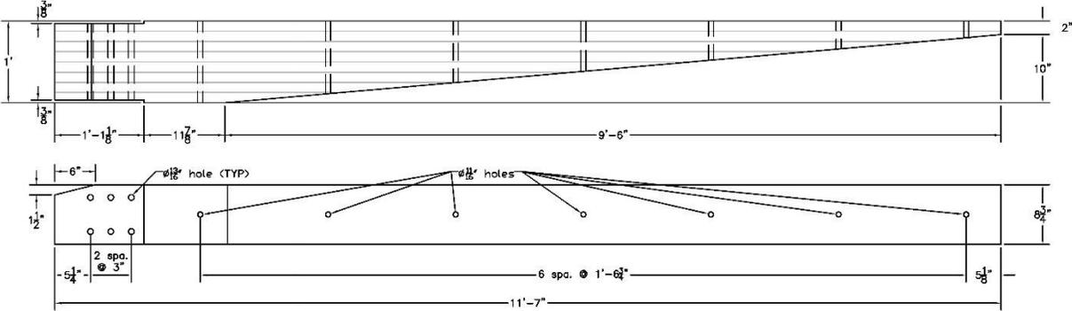
Figure 121. Curb Rail Taper Details for Quarter-Post System
