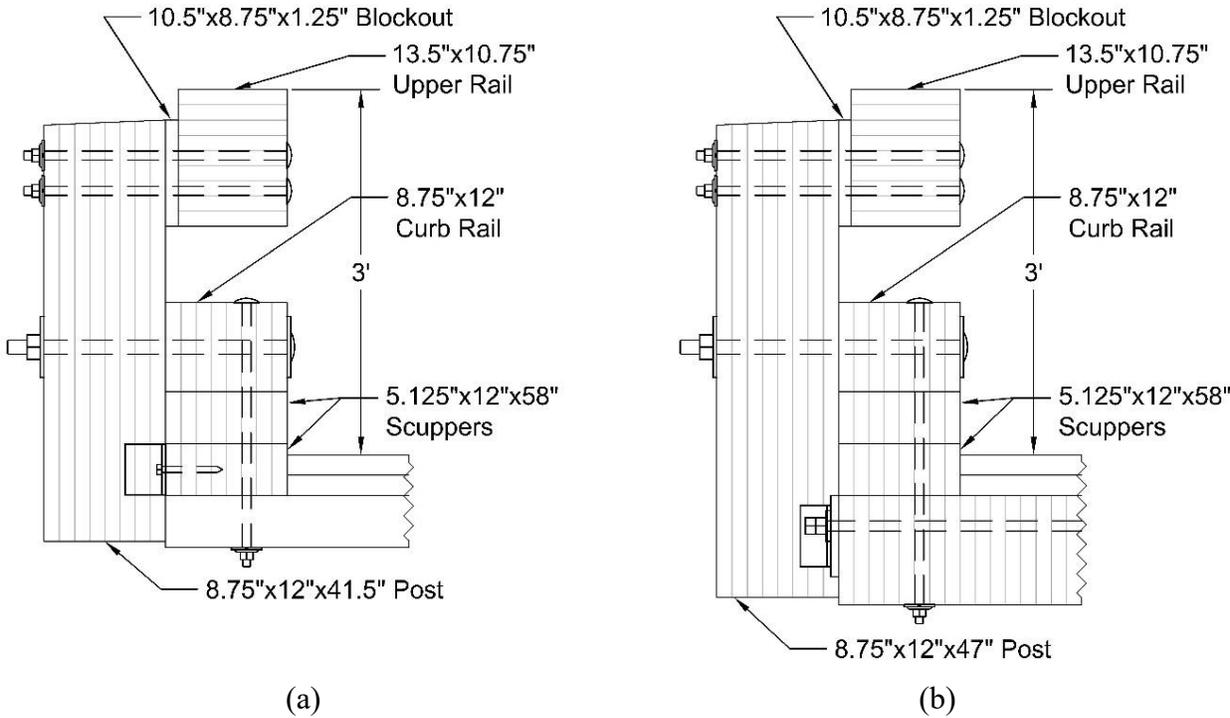
Figure 107. (a) MASH 2016 Bridge Rail Design on Transverse Deck and (b) Longitudinal Deck
