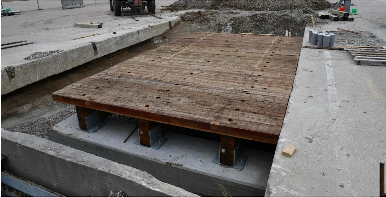
Figure 175. Superstructure Girders with Deck Panels on Top, Test No. TRTD-1
