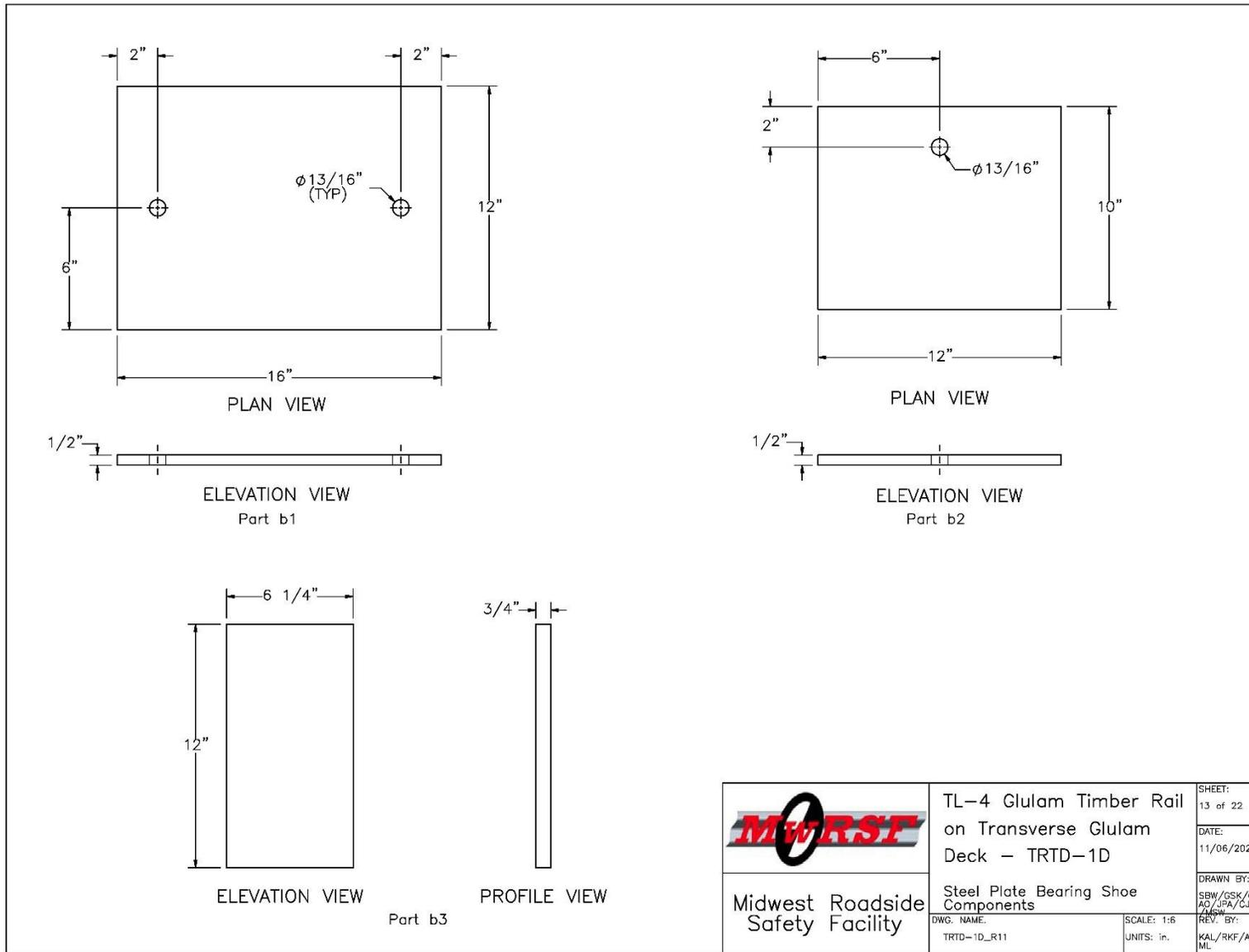
Figure 160. Steel Plate Bearing Assembly Component Details, Test No. TRTD-1
