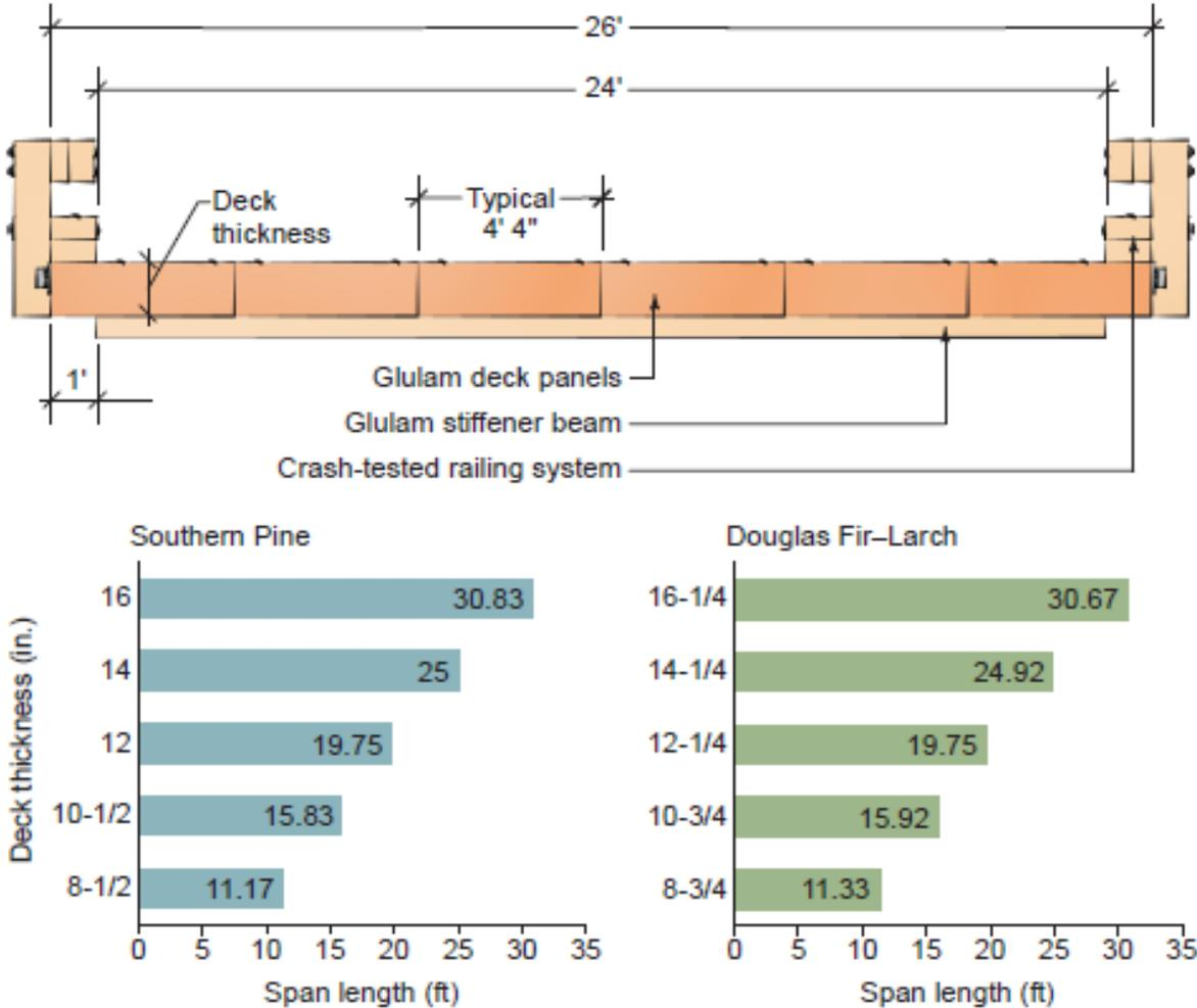
Figure 103. Longitudinal Glulam Deck Cross-Section (Top) and Span Charts for Multilane Bridges (Bottom) [32]
