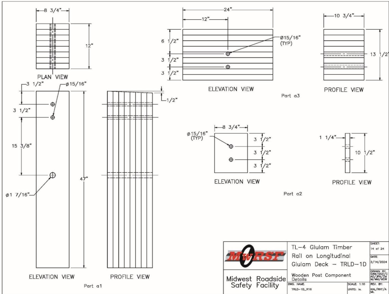
Figure 256. Vertical Post, Upper Rail, Blockout, and Angle Guide Details, Test No. TRLD-1
