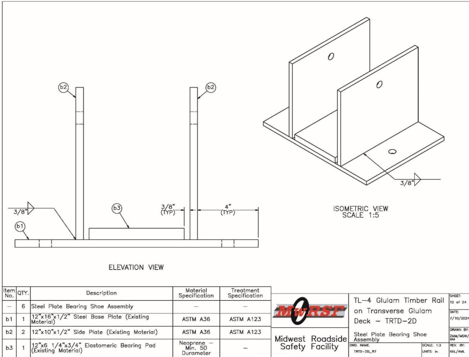
Figure 230. Steel Plate Bearing Assembly Details, Test No. TRTD-2
