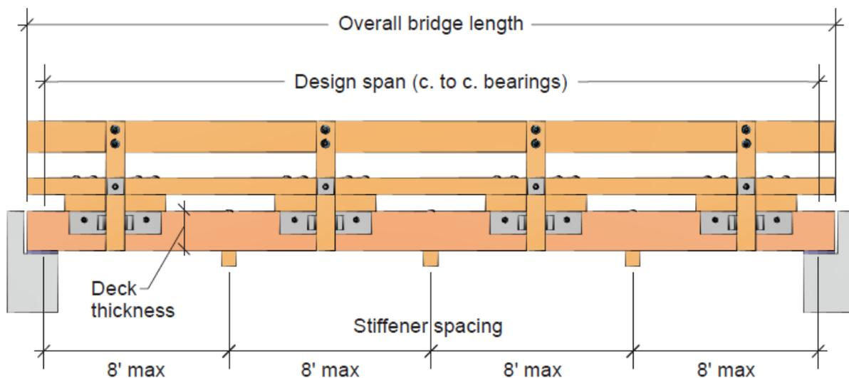
Figure 41. Elevation View of Longitudinal Glulam Bridge Deck with Railing and Spreader Beams [32]
