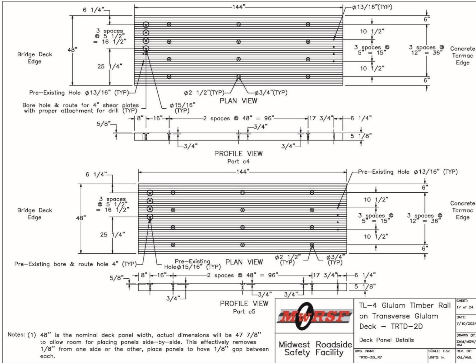
Figure 235. Deck Panel Details, Page 1, Test No. TRTD-2
