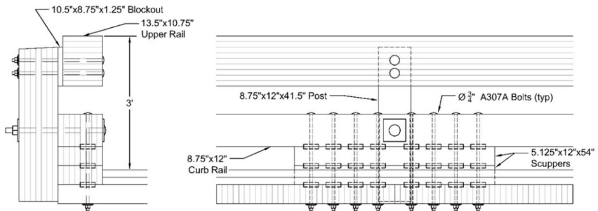
Figure 1. Preliminary Design of MASH TL-4 Glulam Timber Railing with Lower Curb, Phase IIa [10-11]
