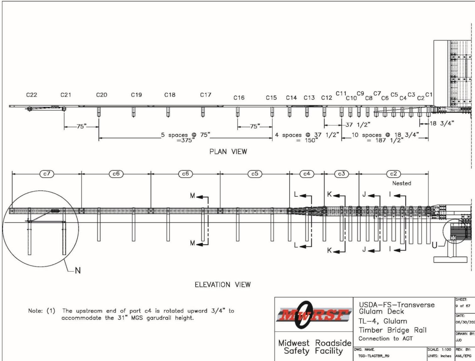
Figure O-9. Plan and Elevation View of AGT
