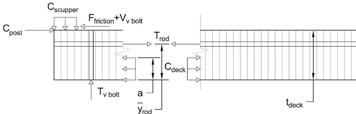
Figure 99. Longitudinal Deck Free-Body-Diagram of External and Internal Forces
