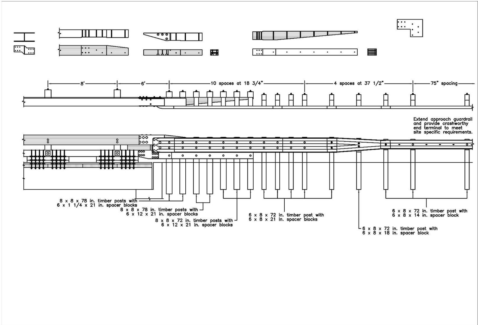
Figure K-25. Option 4.2 – Quarter-Post Spacing, 6-ft Gap, L-Plate, Removed Blockouts, Wood Reverse Taper, Stepped Curb Rail Taper
