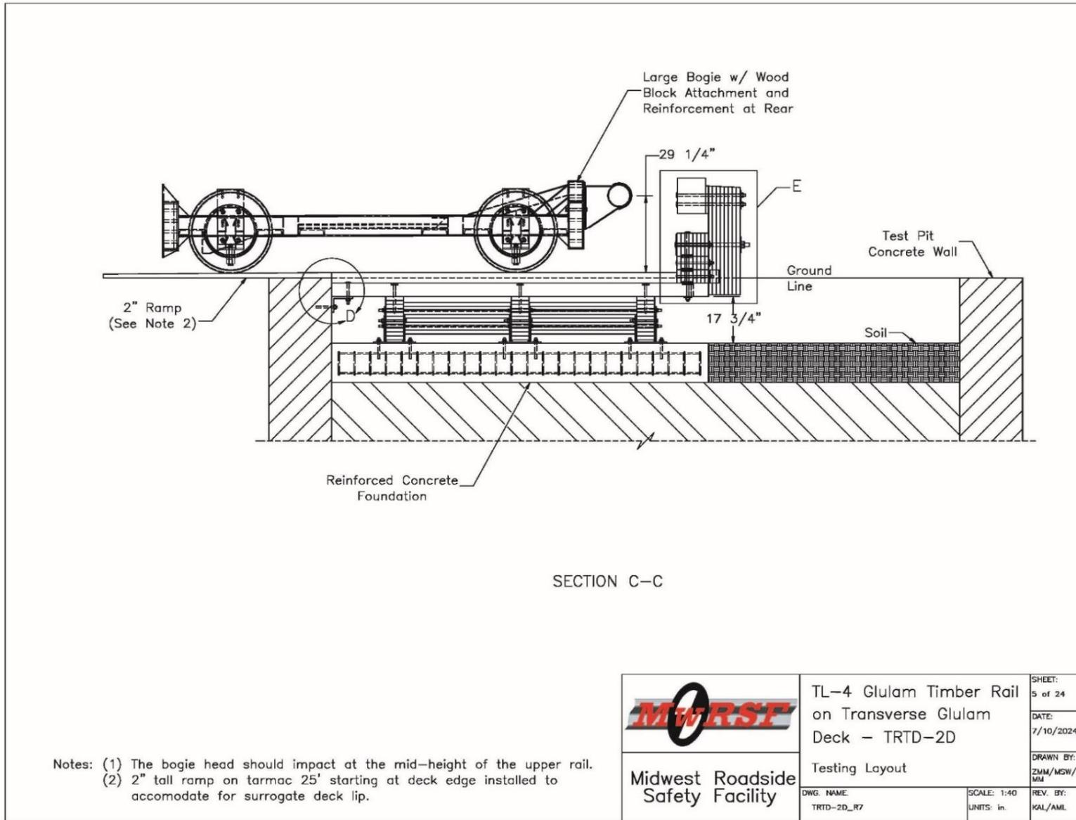
Figure 223. Layout, Elevation View, Test No. TRTD-2
