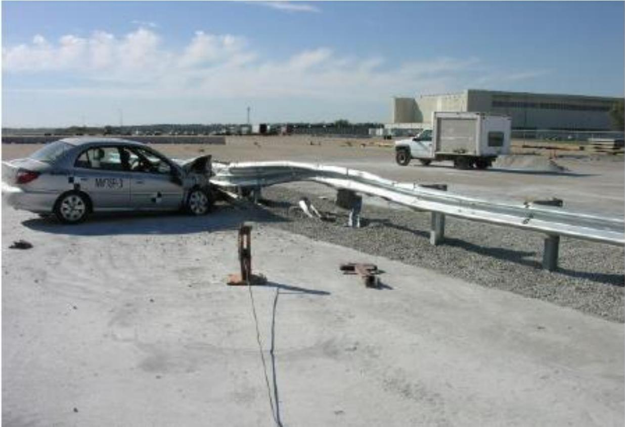
Figure 21. MWTSP-3 Final Location of Small Car after Test with Wheel Snag [36]
