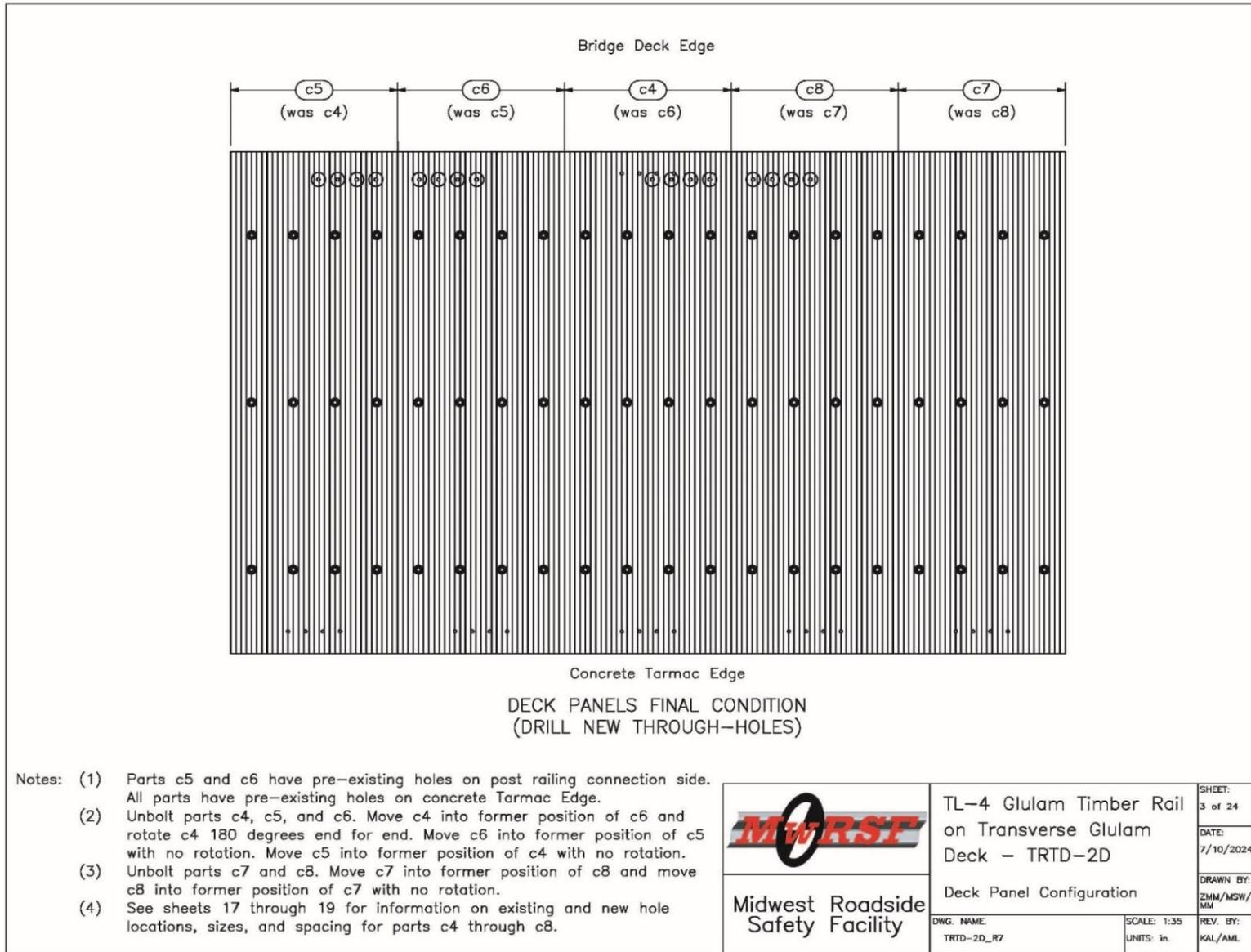
Figure 221. Deck Panel Configuration, Test No. TRTD-2
