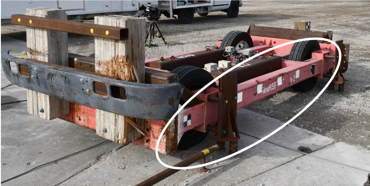
Figure 132. Bogie Railing Guide System, Ends Prior to Impact with Post
