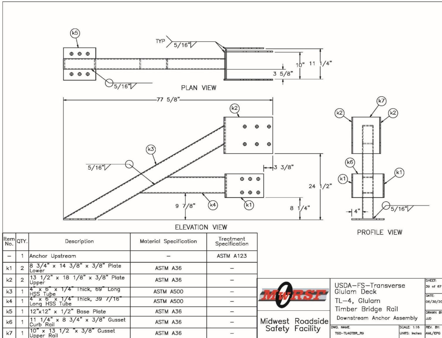
Figure O-39. Bridge Railing End Anchor Component Assembly
