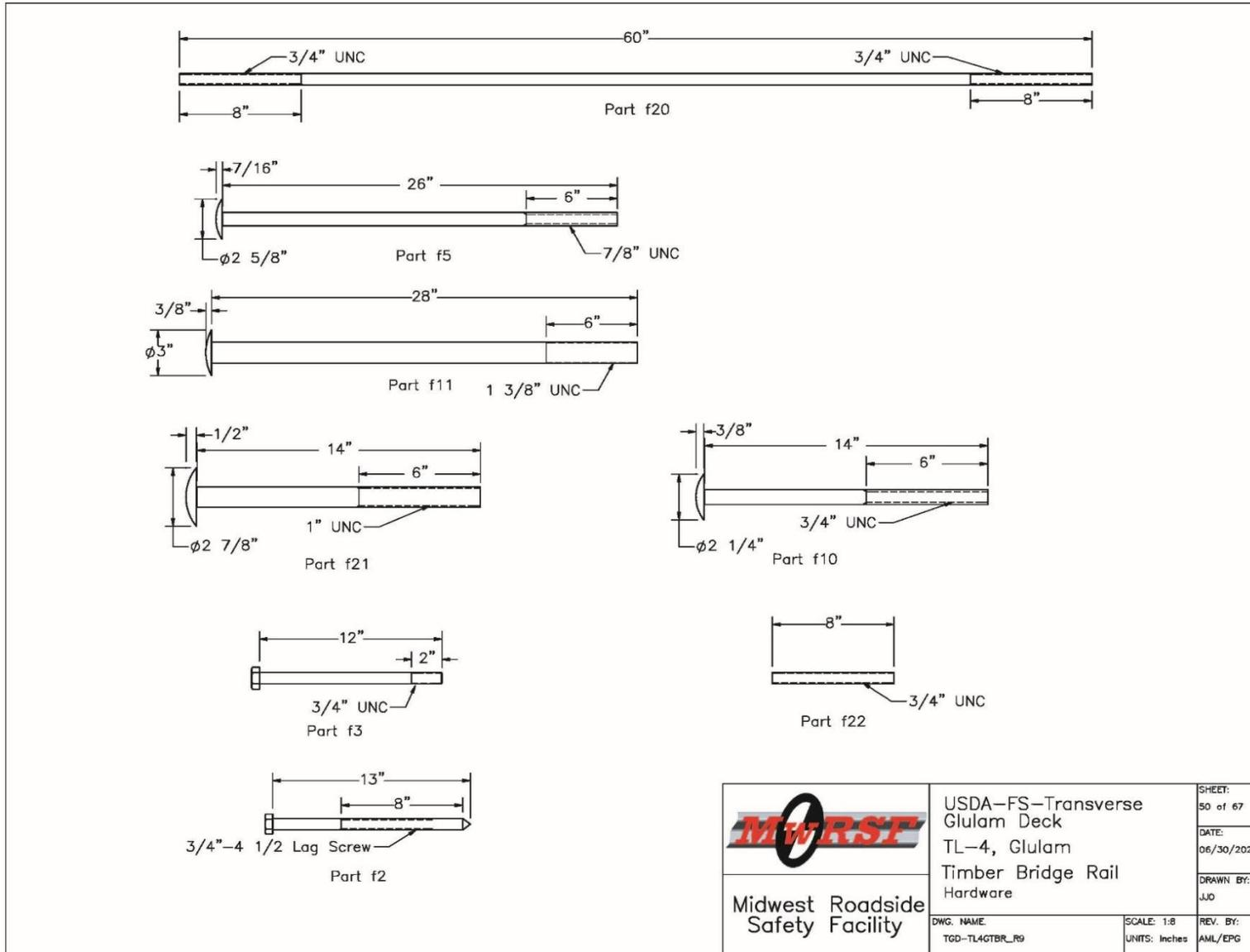
Figure O-50. Bridge Bolt Hardware Details, Page 1
