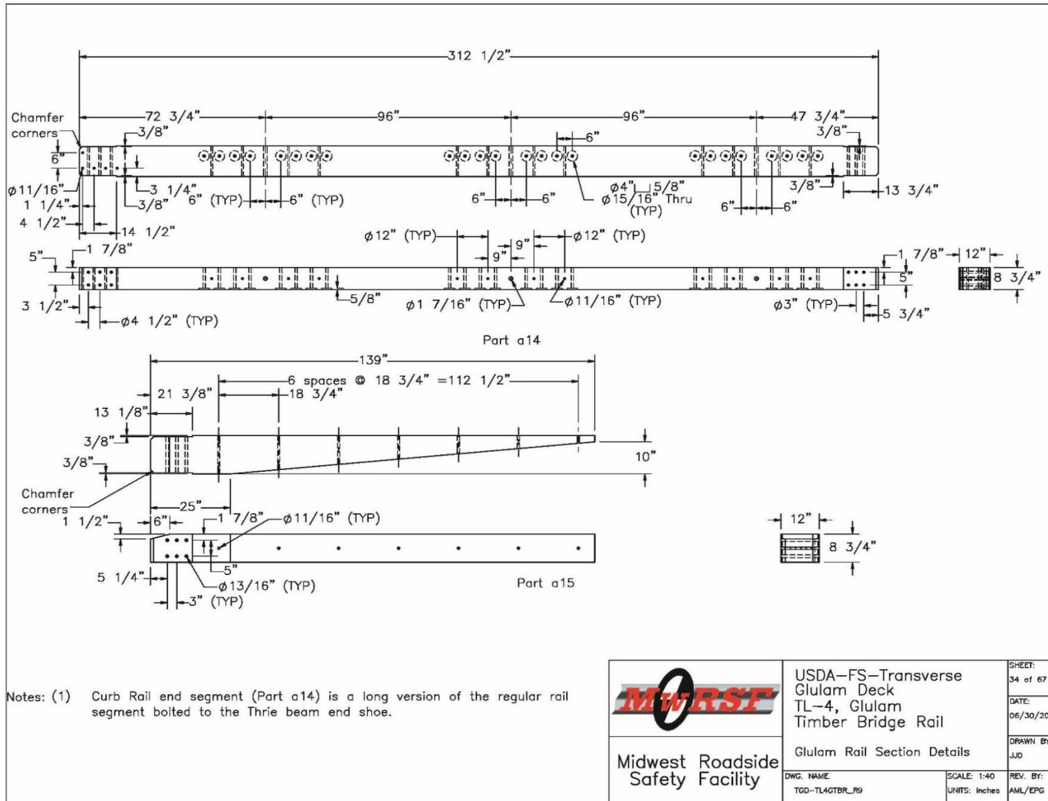
Figure O-34. Bridge Curb Glulam Railing End Pieces
