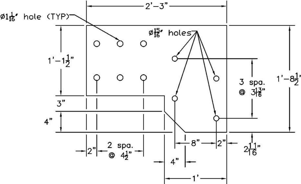
Figure 122. Upper Rail Plate Details for Half-Post System
