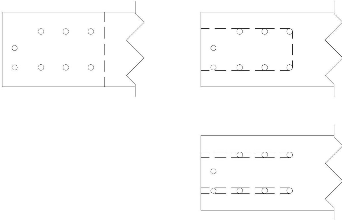
Figure J-2. From top right to bottom left: Net Tensile Failure, Row Tear-out Failure, Group Tear-out Failure.
