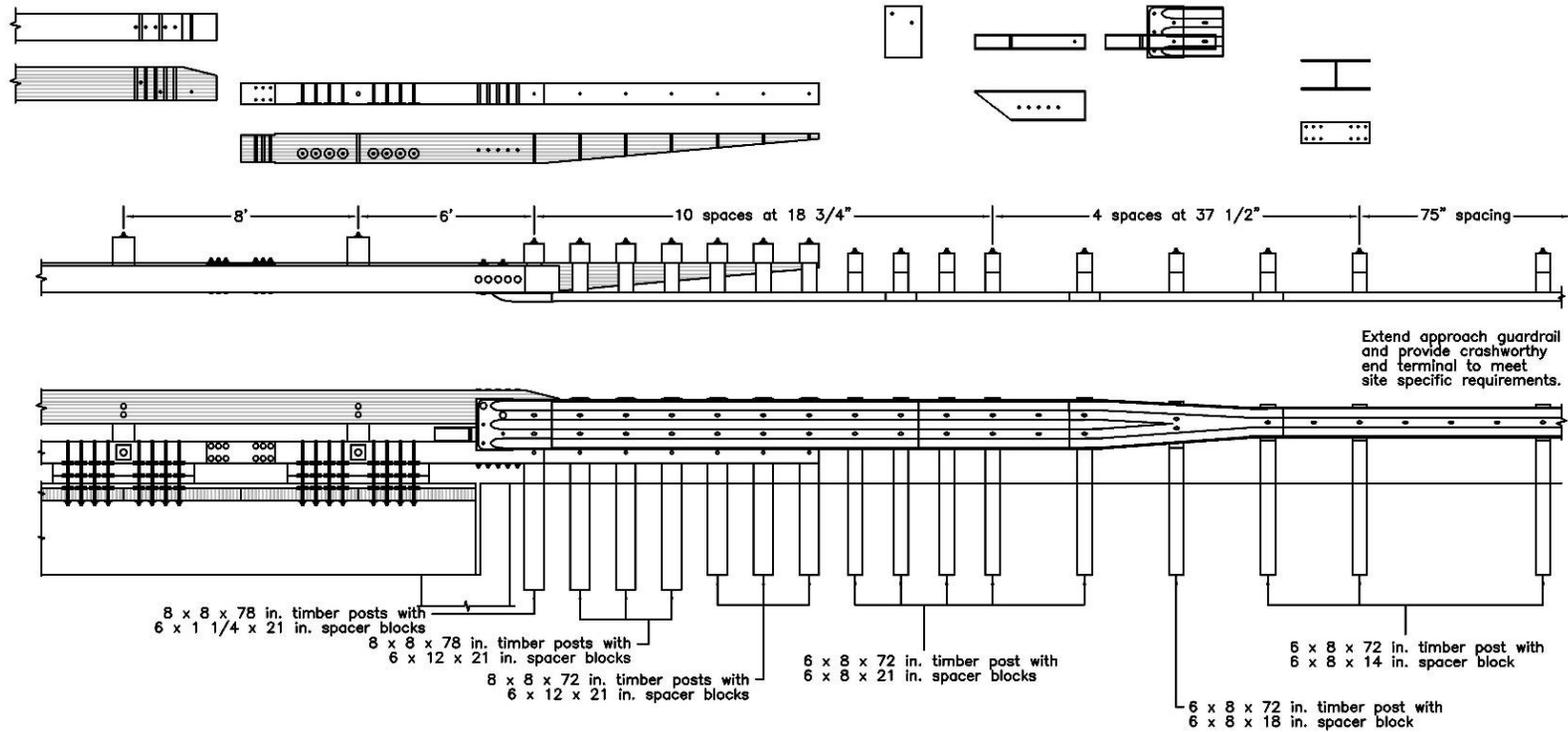
Figure K-47. Option 7.10 – Quarter-Post Spacing, 6-ft Gap, Welded End Shoe to Steel Reverse Taper, Curb Taper Behind Thrie-beam
