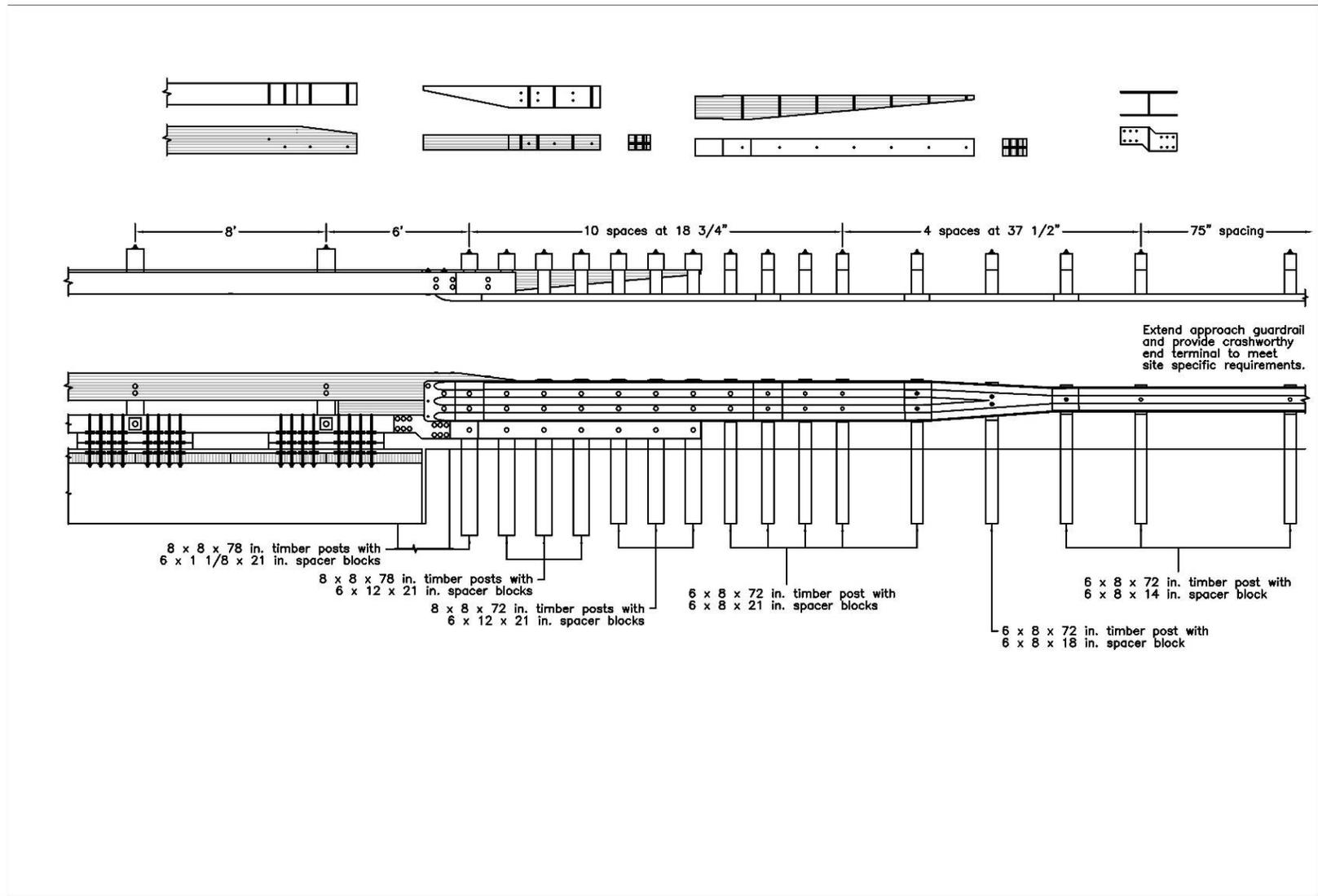
Figure K-8. Option 2.3 – Quarter-Post Spacing, 6-ft Gap, No Plate, Missing Bolts, Removed Blockouts, Wood Reverse Taper, Stepped Curb Taper
