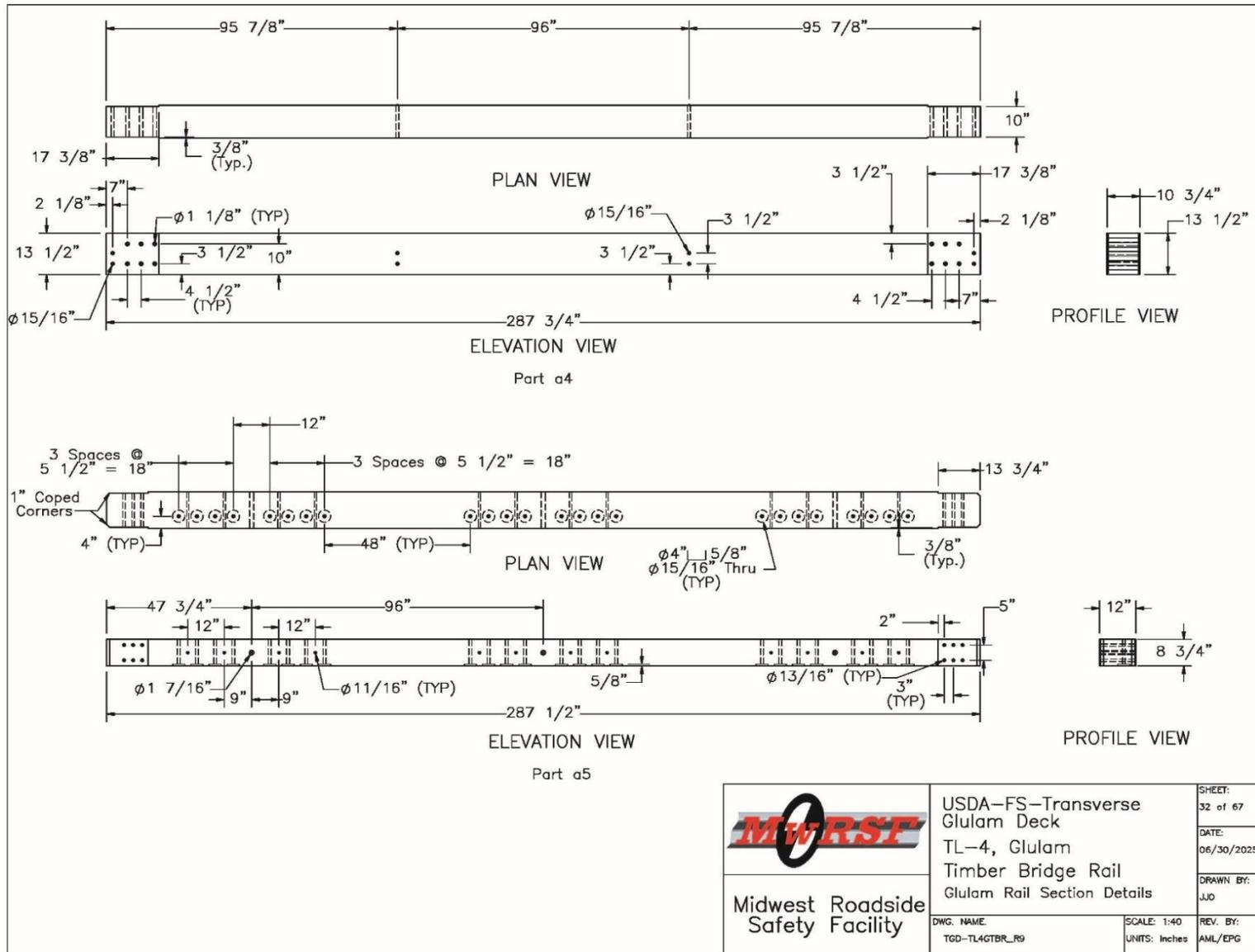
Figure O-32. Bridge Typical Upper and Curb Glulam Railing Pieces
