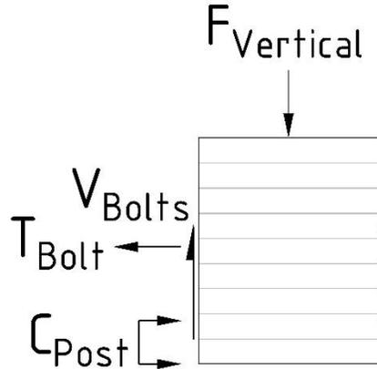
Figure 78. Free-Body-Diagram of Upper Railing Connection to Post Under Vertical Load
