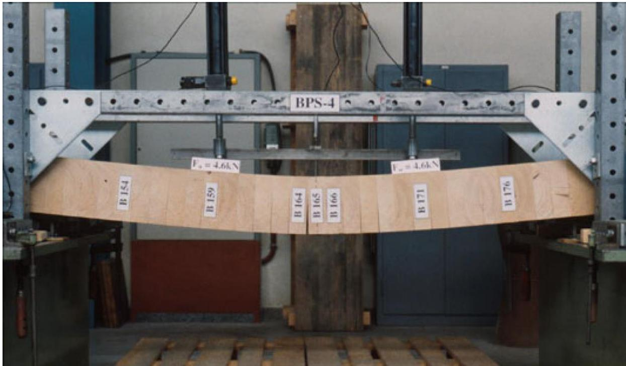
Figure 52. Screw-Laminated Deck Panel Under 4-Point Bending Test [56]
