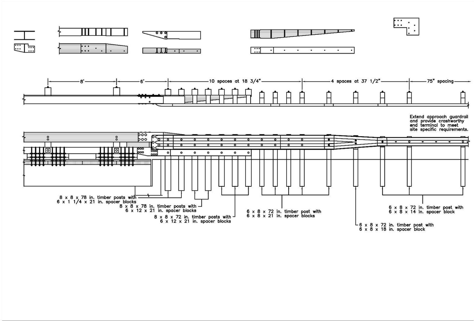
Figure K-34. Option 6.3 – Quarter-Post Spacing, 6-ft Gap, L-Plate, Removed Blockouts, Wood Reverse Taper, Stepped Curb Taper
