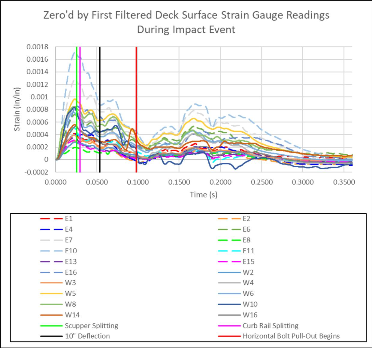
Figure 203. Strain vs. Time Curve for Deck Surface Strain Gauges
