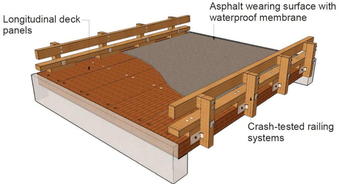
Figure 40. Longitudinal Deck Diagram [32]
