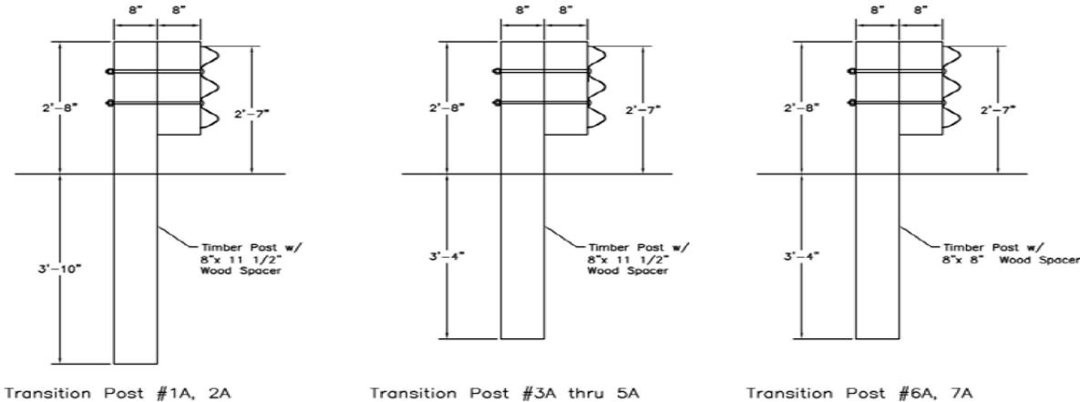
Figure 14. Cross-Section View of AGT Posts Closest to Bridge Railing [16]
