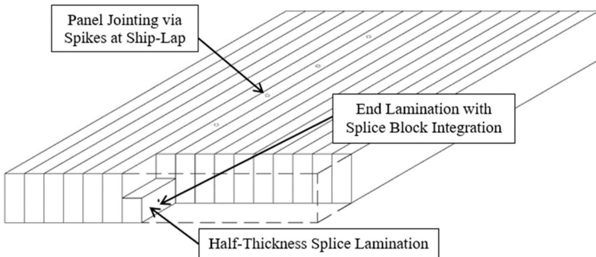
Figure 42. Example of Ship-Lap Joint
