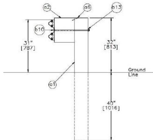
Figure 30. MGS Cross-Section of SYP Grade No. 1 Posts [43]
