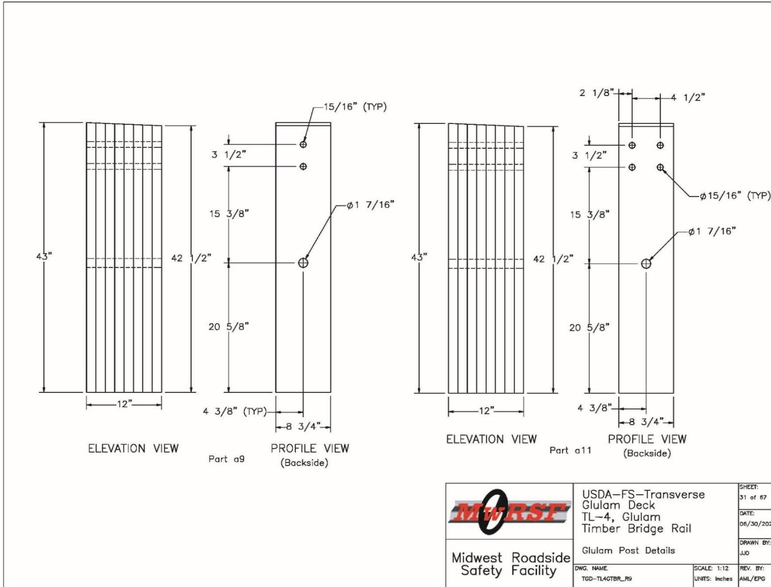
Figure O-31. Bridge Typical and Splice Vertical Post Details
