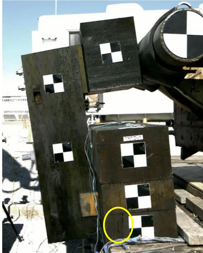
Figure 214. Test No. TRTD-1 Tensile Cracks in Scupper at 0.0260 Seconds after Impact
