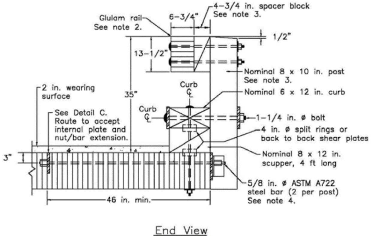
Figure 3. NCHRP 350 TL-4 Bridge Railing Cross-Section on Longitudinal Glulam Deck [16]
