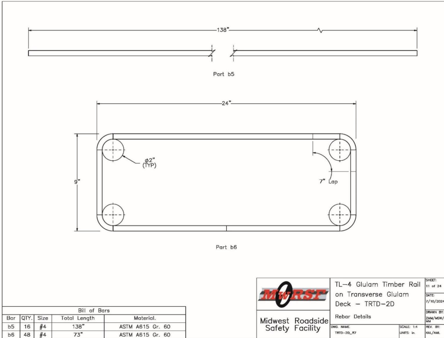
Figure 229. Rebar Details, Test No. TRTD-2
