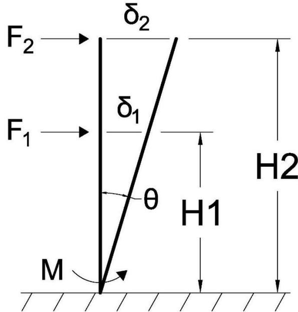
Figure 70. Force and Deflection Diagram for Height Adjustment
