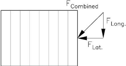
Figure 79. Post Design Case 1 Free-Body-Diagram Combined Shear
