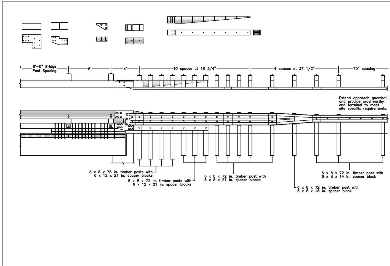
Figure K-19. Option 3.4 – Quarter-Post Spacing, 4-ft and 6-ft Gaps, L-Plate, Removed Blockout, Wood Reverse Taper, Stepped Curb Taper
