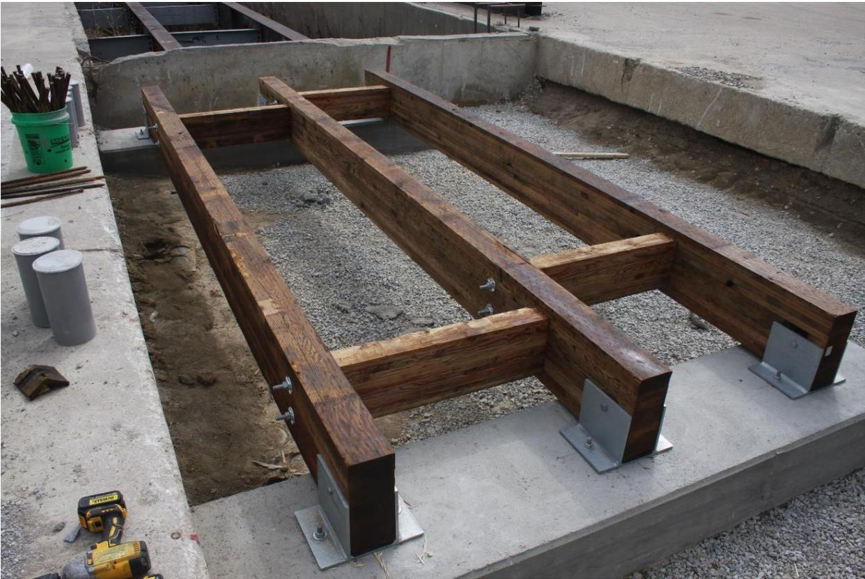
Figure 174. Glulam Girders with Diaphragms Bolted to Supports, Test No. TRTD-1
