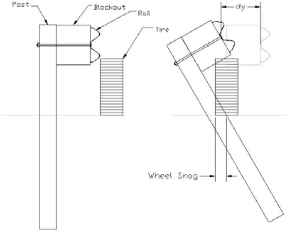
Figure 147. Wheel Snag Diagram [112]
