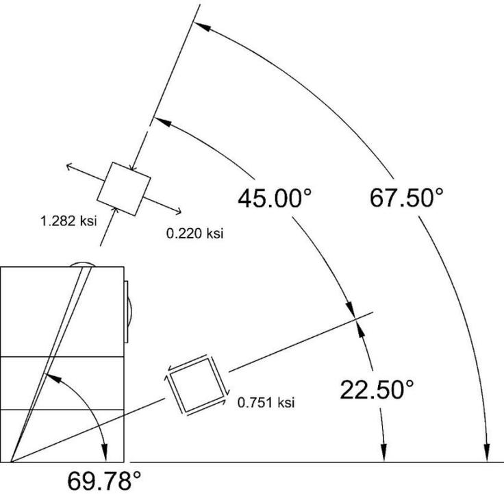
Figure 217. Mohr's Circle of Stresses in Scupper at Compression Block Assuming High Friction Coefficient
