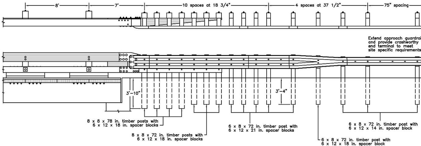
Figure 114. Quarter-Post MASH 2016 TL-3 AGT between TL-4 Bridge Rail and MGS
