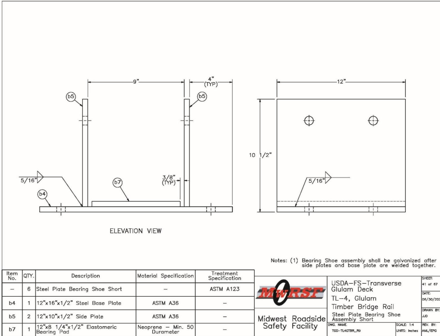
Figure O-41. Bridge Superstructure Abutment Bearing Assembly Details
