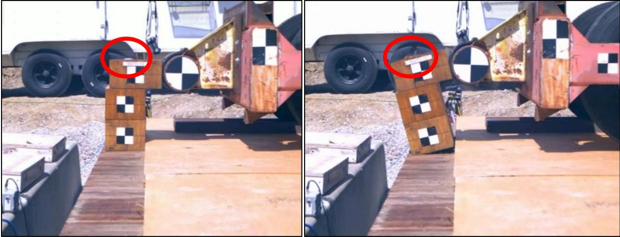
Figure D-2. Left, Post at Start of Impact with Domed Bolt Heads Visible; Right, Domed Bolt Heads No Longer Visible [7]
