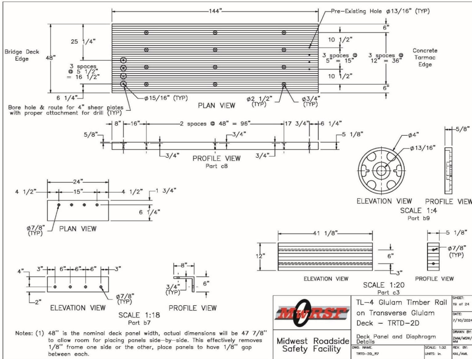
Figure 237. Deck Panel, Tarmac Angle Restraint, Diaphragm, and Shear Plate Details, Test No. TRTD-2
