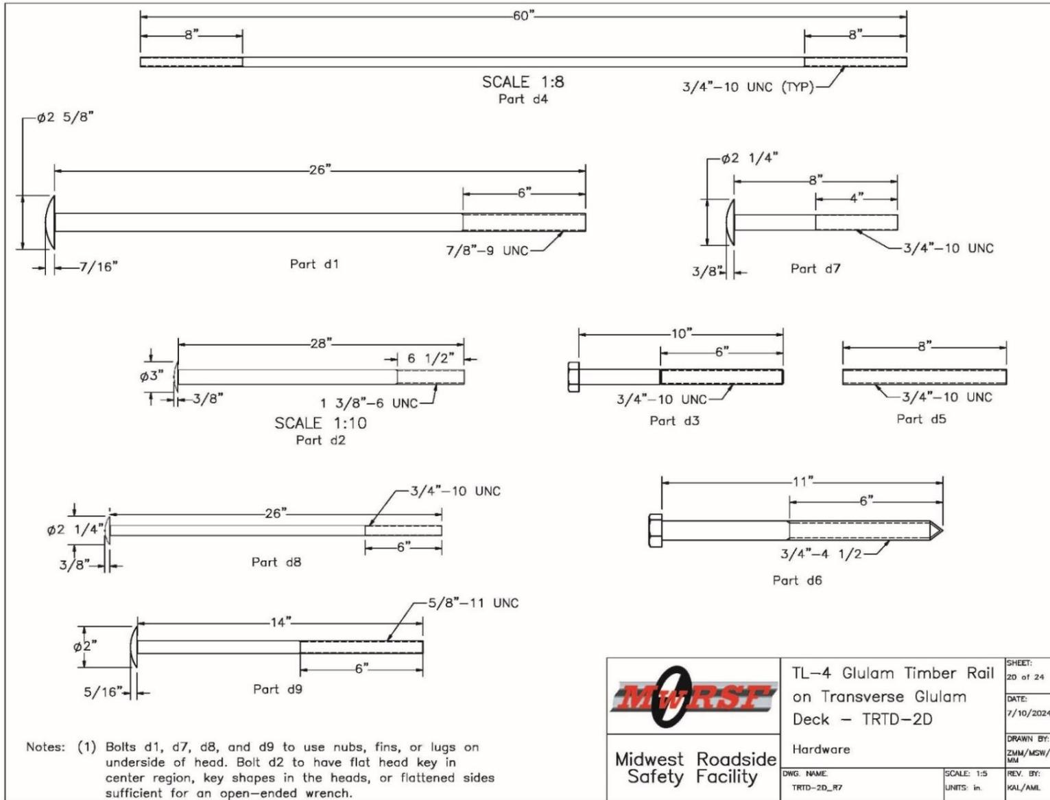
Figure 238. Connection Hardware Details, Page 1, Test No. TRTD-2
