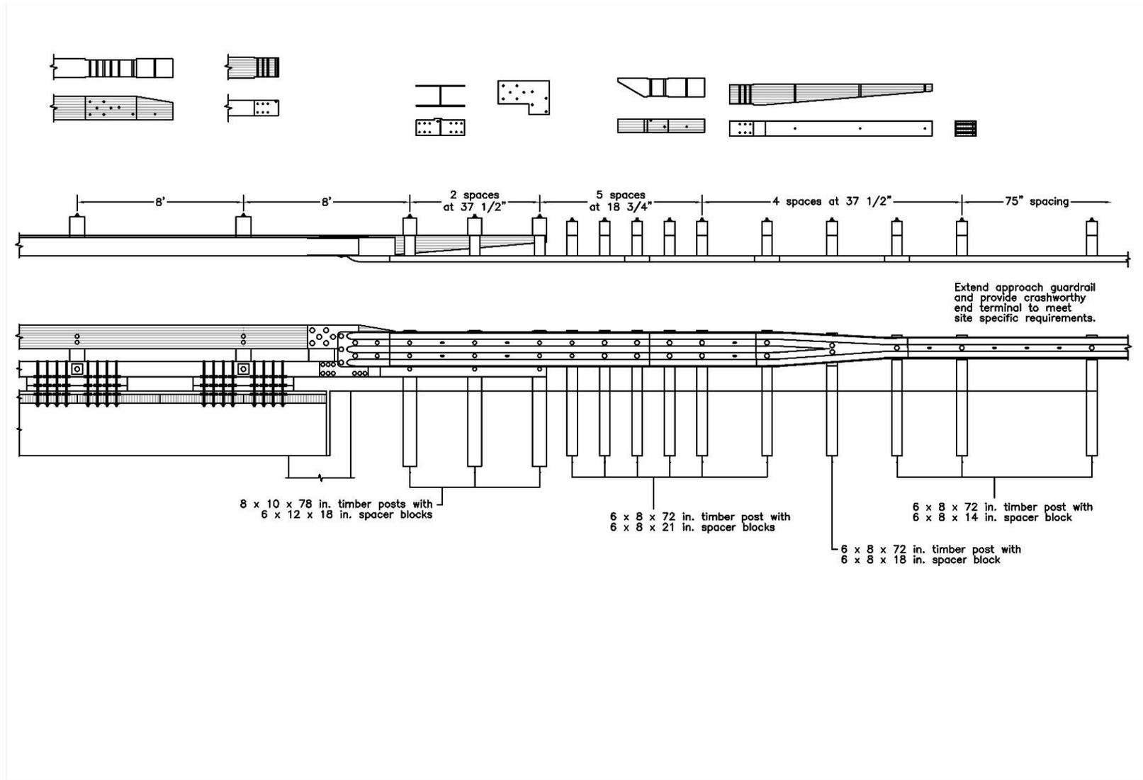
Figure K-26. Option 4.3 – Half-Post Spacing, 8-ft Gap, L-Plate, Wood Reverse Taper, Curb Taper with Bumpout Behind Thrie-Beam
