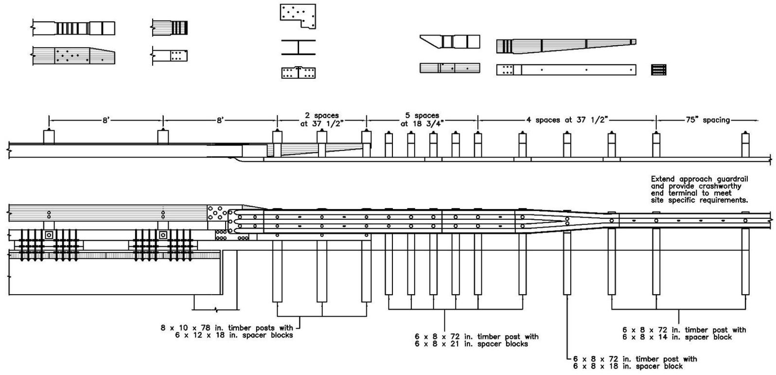
Figure K-27. Option 5.1 – Half-Post Spacing, 8-ft Gap, L-Plate, Wood Reverse Taper, Curb Taper with Bumpout Behind Thrie-beam
