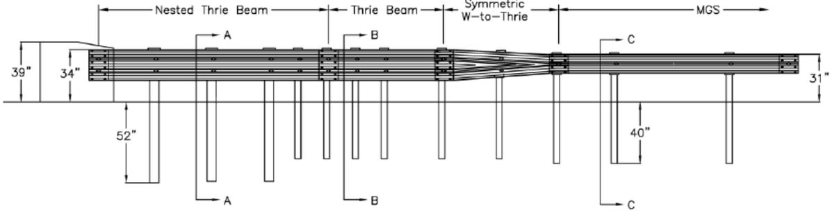
Figure 25. AGT System Configuration before Installation of 3-in. Wearing Surface [38]
