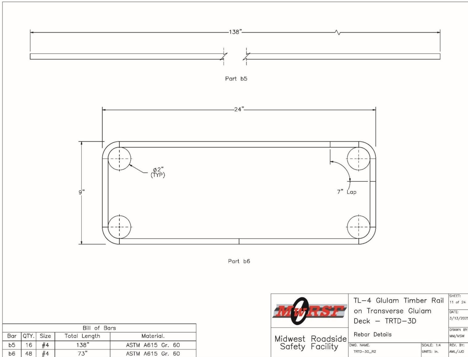
Figure N-11. Test No. TRTD-3 Rebar Details
