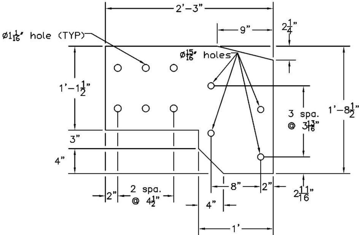
Figure 123. Upper Rail Plate Details for Quarter-Post System
