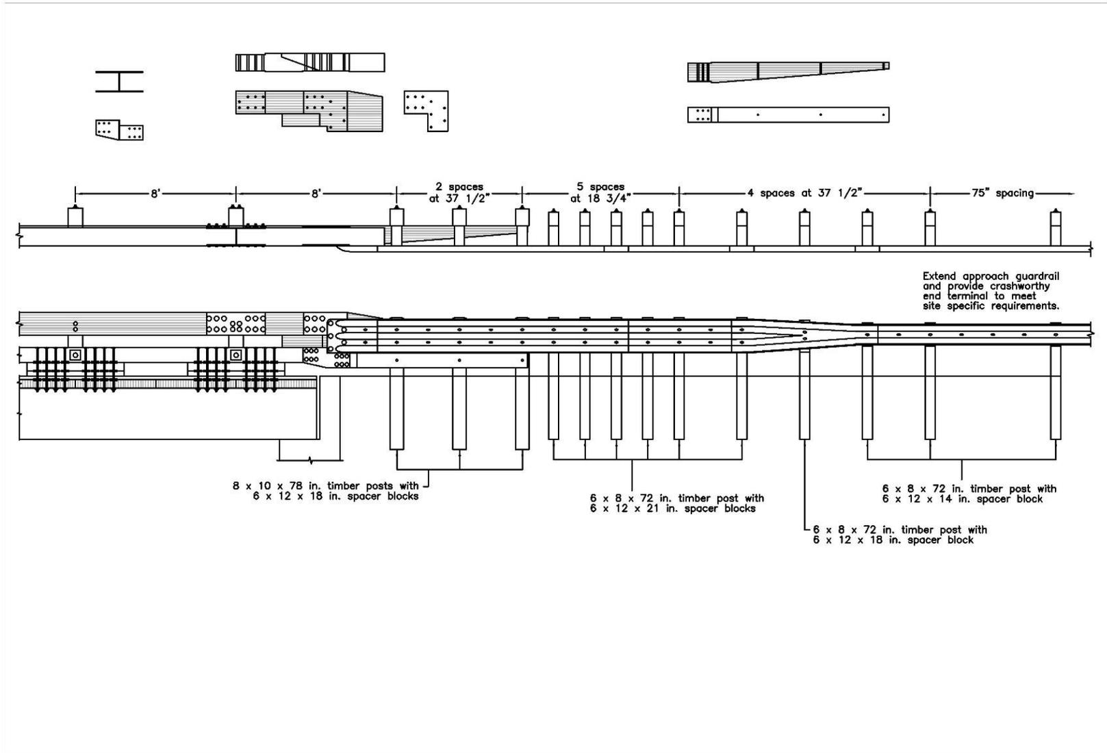
Figure K-43. Option 7.6 – Half-Post Spacing, 8-ft Gap, L-Plate, Custom Glulam Piece, Stepped Curb Taper
