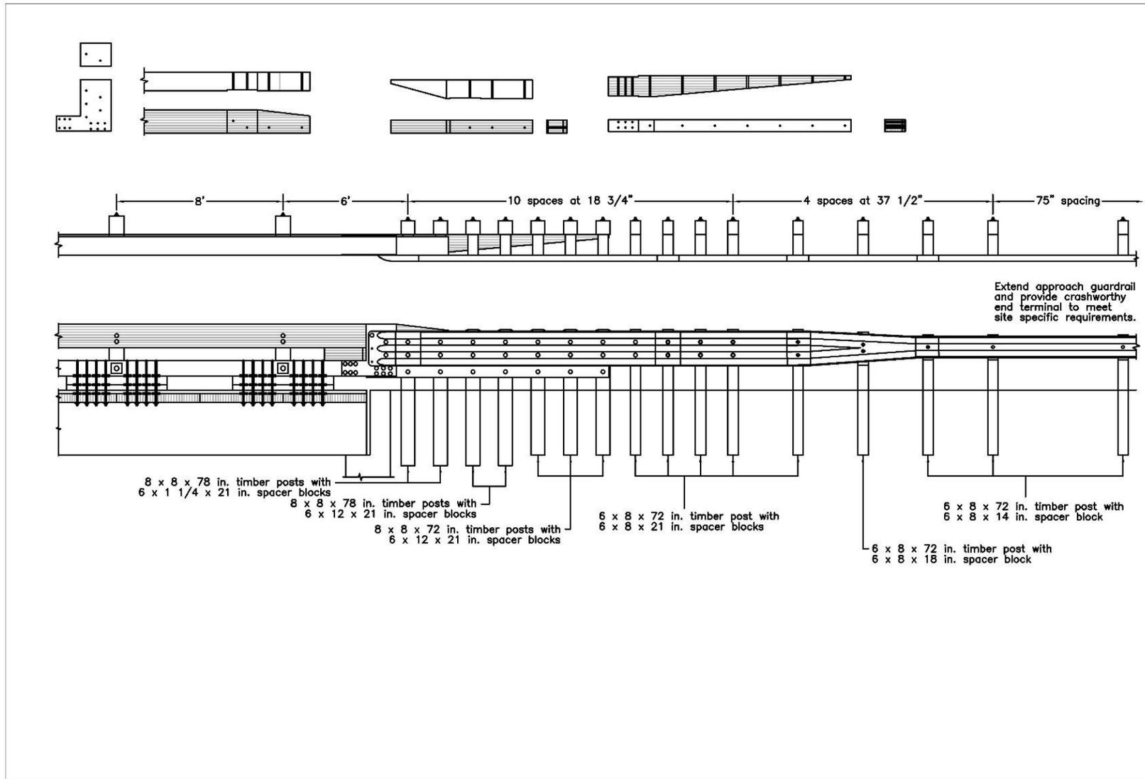
Figure K-6. Option 2.1 – Quarter-Post Spacing, 6-ft Gap, Lower L-Plate, Removed Blockouts, Wood Reverse Taper, Thin Curb Taper
