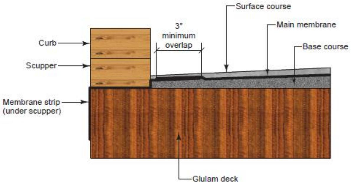
Figure 53. Diagram of Membrane Protecting Bridge Deck Surface, with Timber Railing [32]
