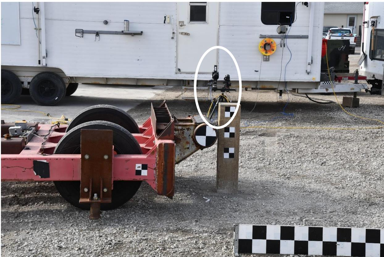
Figure 134. AOS High-Speed Camera
