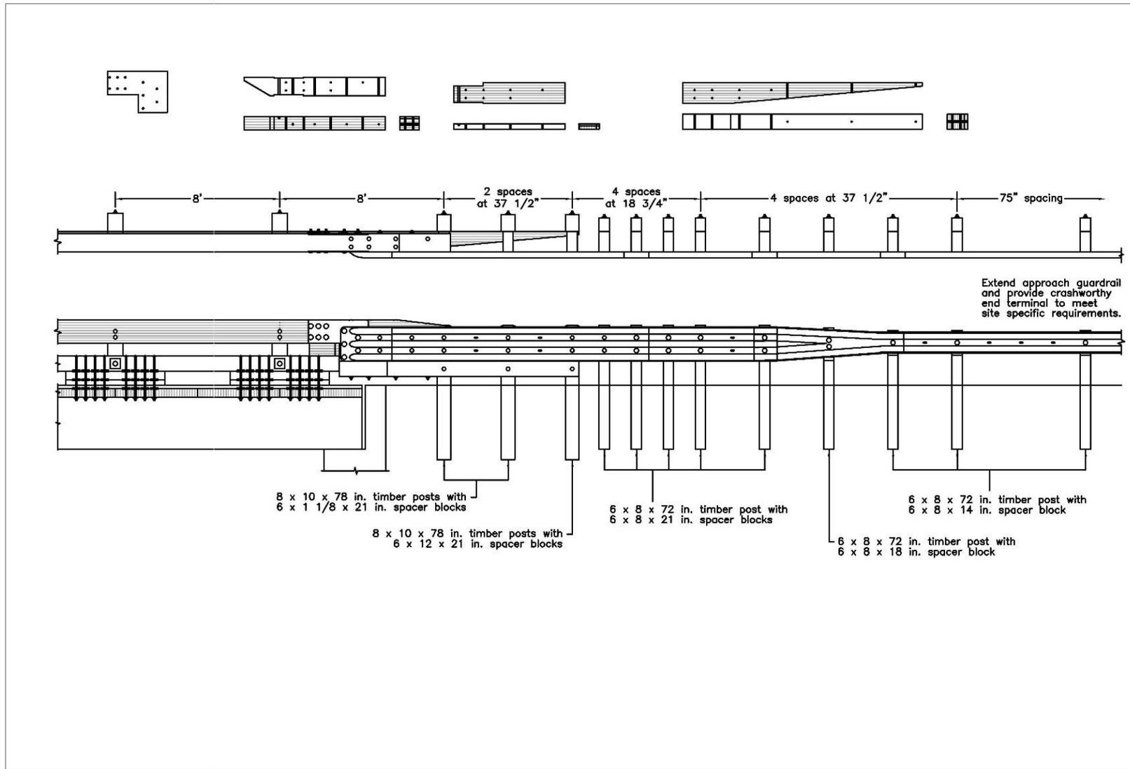
Figure K-18. Option 3.3 – Half-Post Spacing, 8-ft Gap, L-Plate, Removed Blockout, Wood Reverse Taper, Separated Stepped Curb Taper
