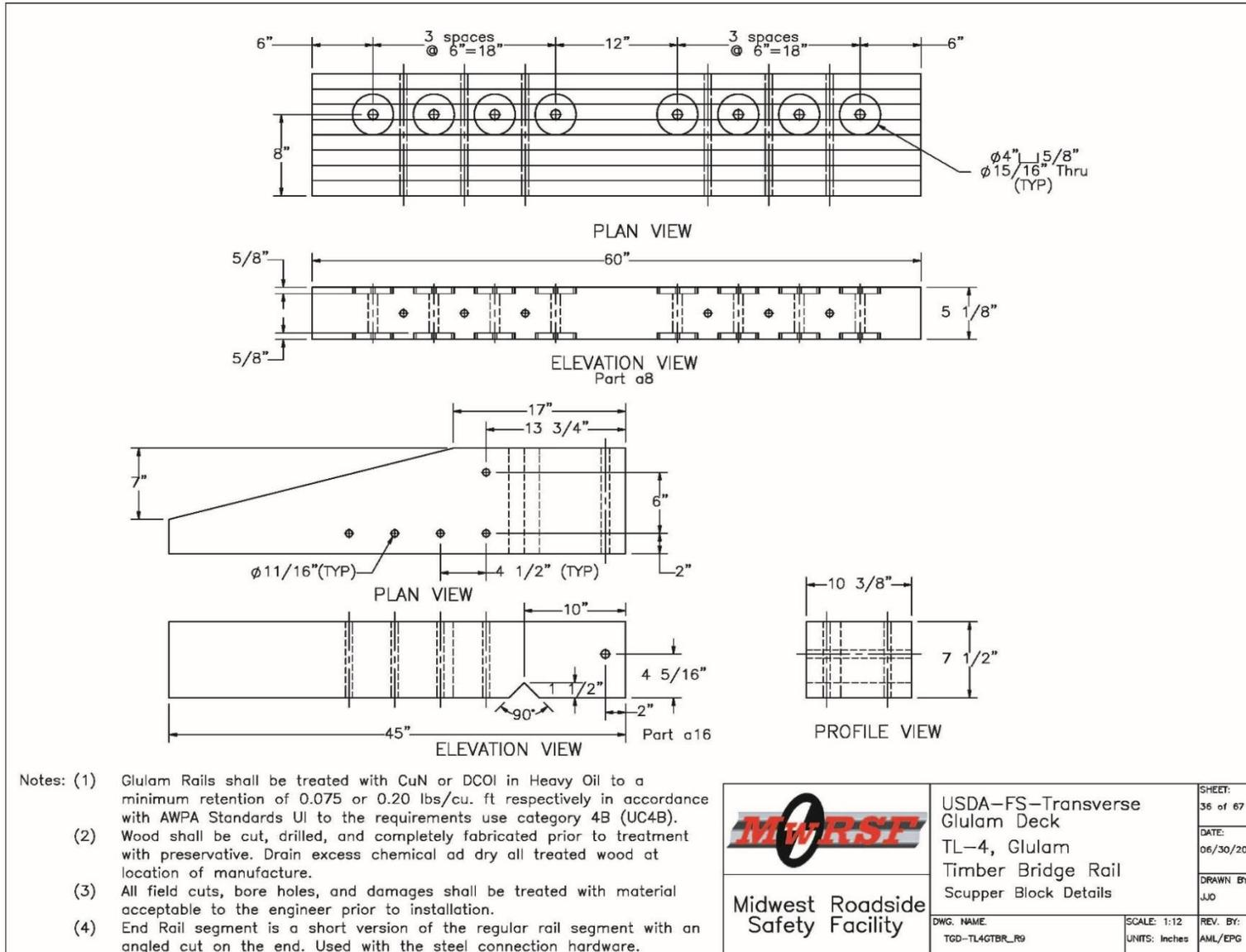
Figure O-36. Bridge Railing Reverse Taper and Scupper Details
