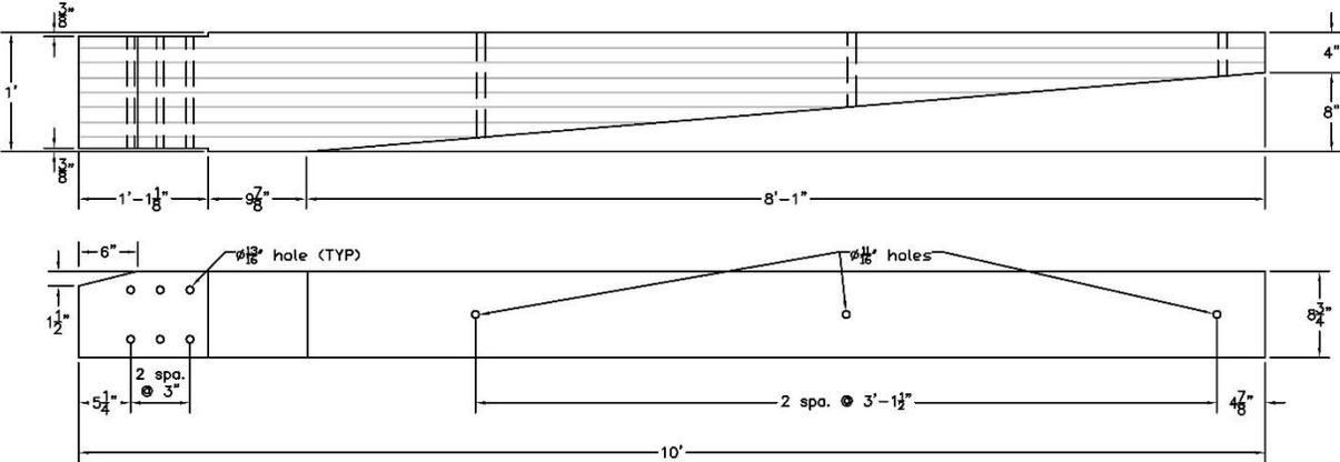
Figure 120. Curb Rail Taper Details for Half-Post System
