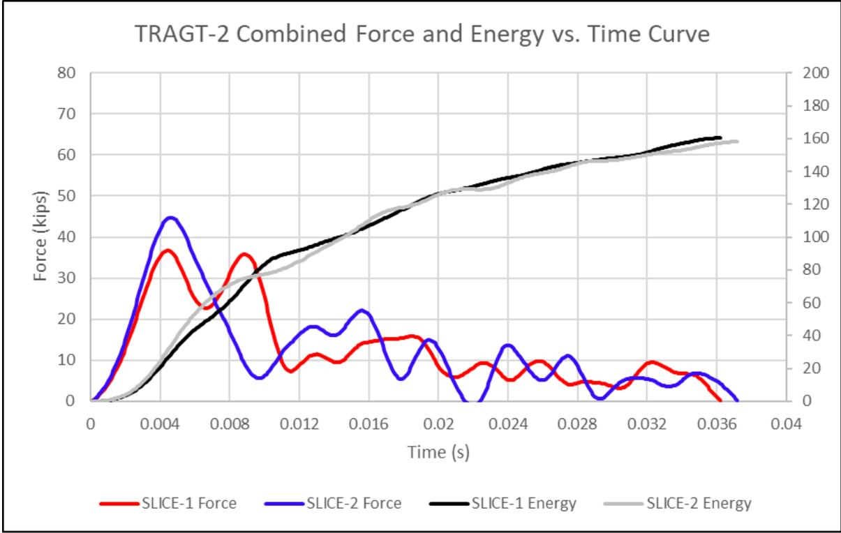
Figure 138. Combined Force and Energy vs. Time Curve, Test No. TRAGT-2
