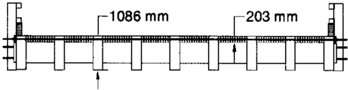
Figure 104. Cross-Section of Stress-Laminated Bridge Deck with Girders in Deck [69]
