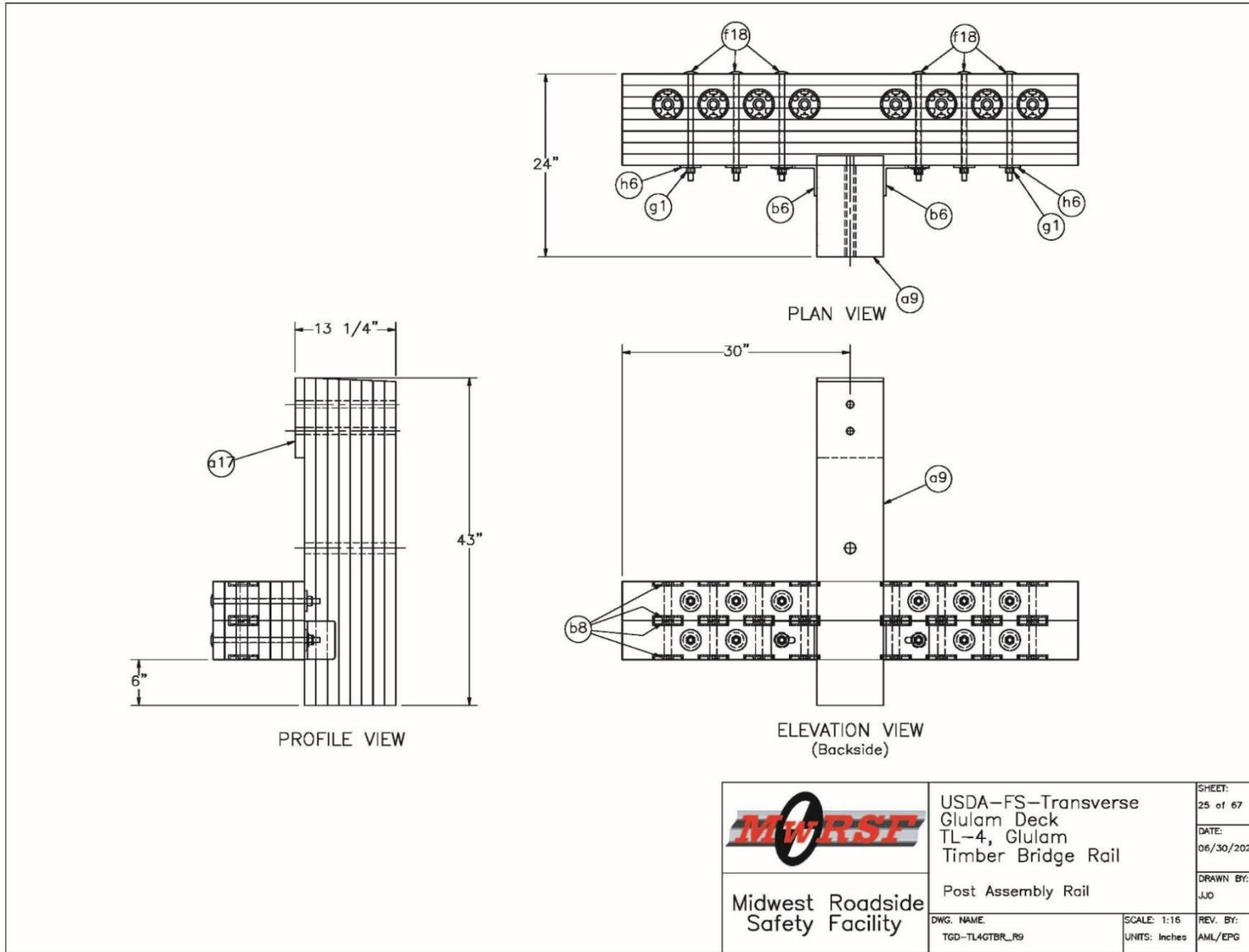
Figure O-25. Bridge Typical Post Assembly Details
