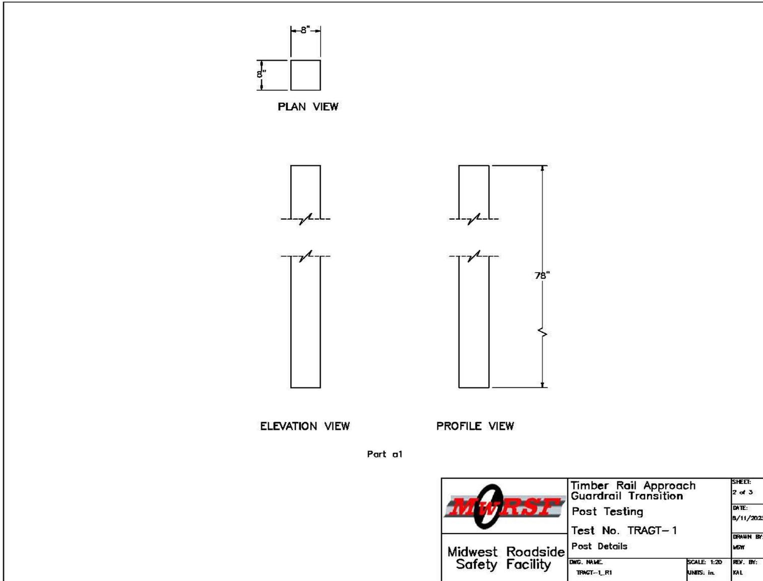
Figure 129. Post Dimensions, Test Nos. TRAGT-1, TRAGT-2, and TRAGT-3
