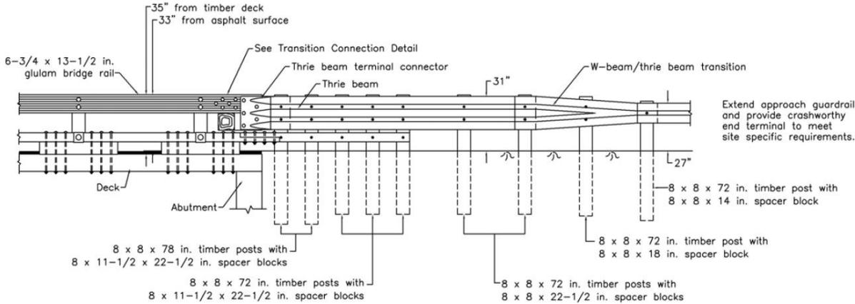
Figure 13. Front View of AGT Developed for GC-8000 [16]
