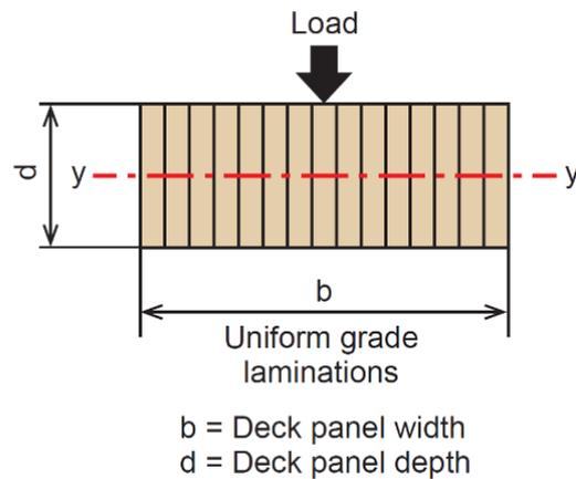
Figure 38. Glulam Deck Panel Loading Diagram [32]
