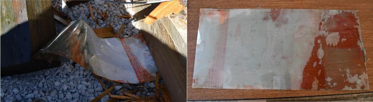
Figure 212. Pressure Film Between Post and Scupper/Deck after Test No. TRTD-1
