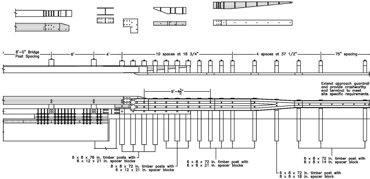
Figure K-21. Option 3.6 – Quarter-Post Spacing, 4-ft and 6-ft Gaps, L-Plate, Removed Blockouts, Missing Bolt, Wood Reverse Taper, Curb Taper Behind Thrie-Beam
