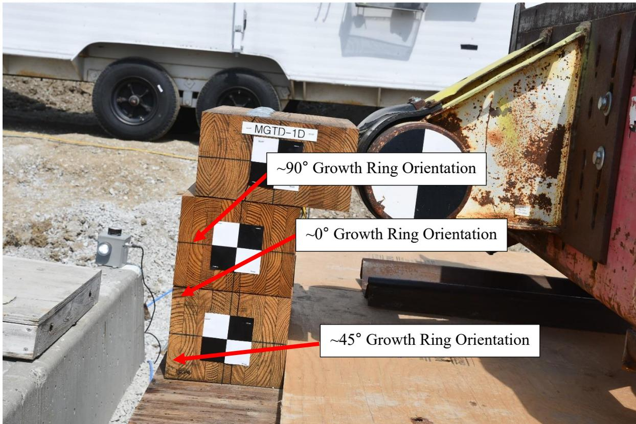
Figure D-4. Growth Ring Orientation in Dynamic Component Test
