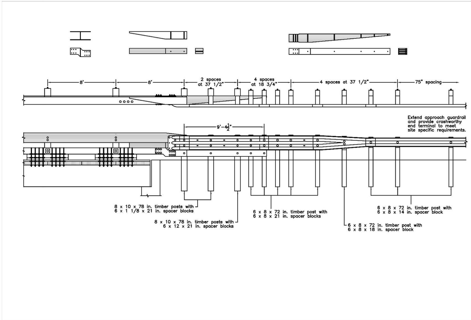
Figure K-14. Option 2.9 – Half-Post Spacing, 8-ft Gap, Shortened Thrie-Beam, No Plate, Missing Bolts, Wood Reverse Taper, Stepped Curb Taper
