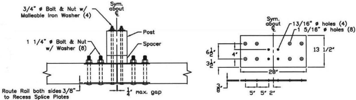
Figure 93. Upper Railing Splice for Glulam Rail and Curb on Transverse Glulam Deck [25]
