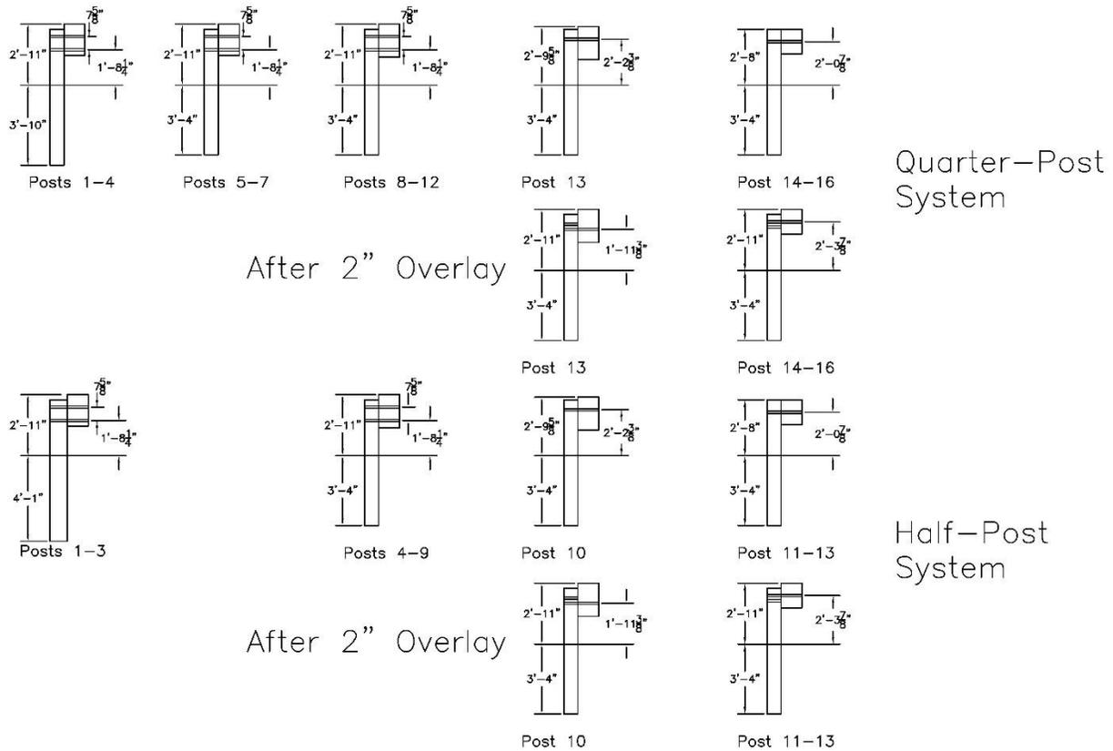
Figure 125. AGT Post Cross-sections for Both Systems
