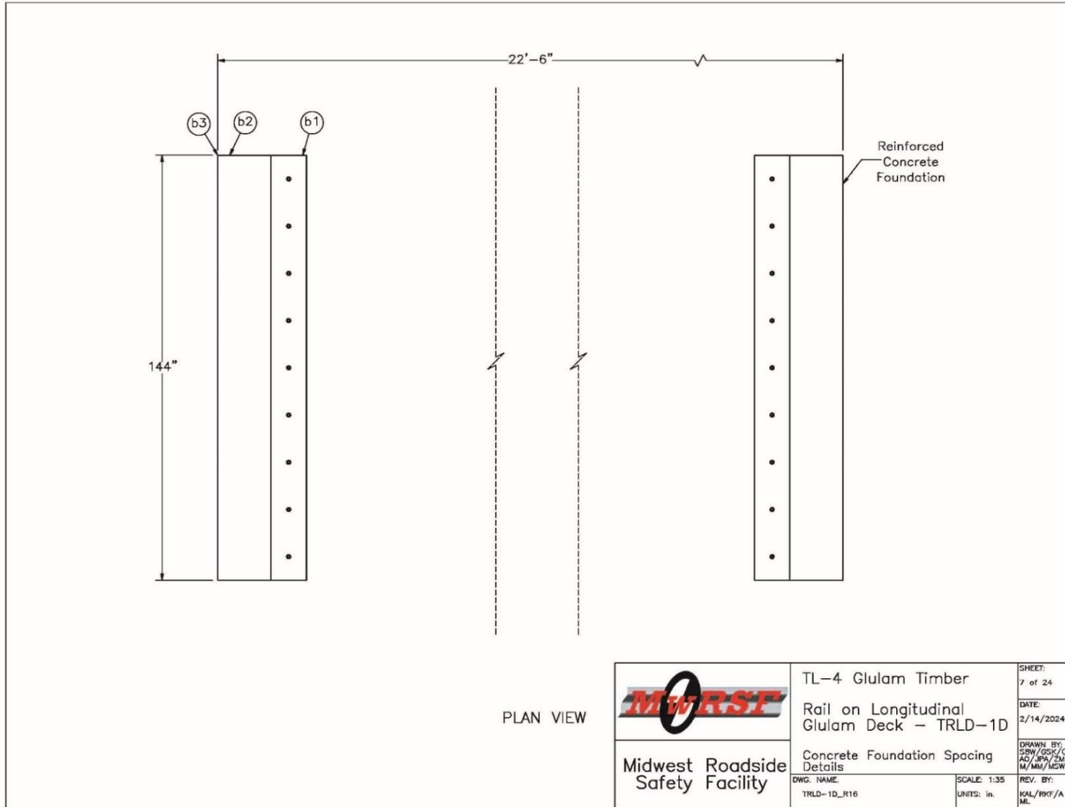
Figure 249. Foundation Layout, Test No. TRLD-1
