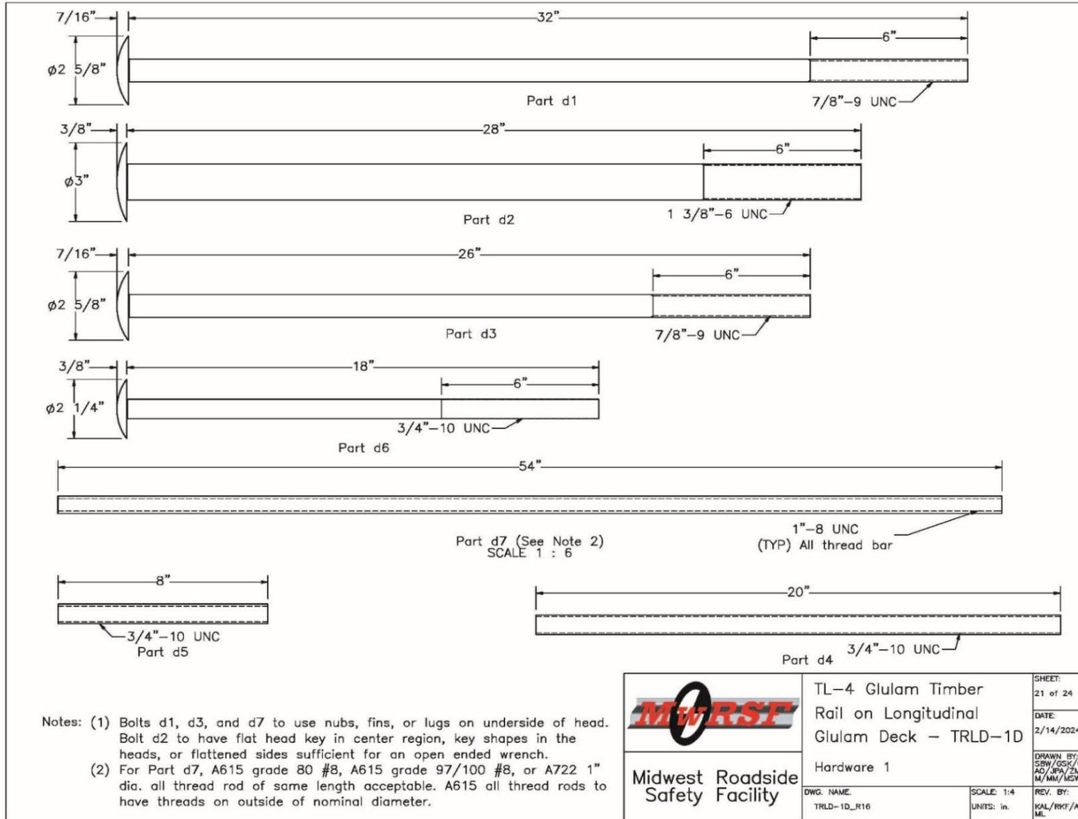
Figure 263. Bolt and Rod Hardware Details, Test No. TRLD-1
