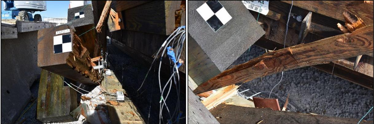
Figure 192. Damaged Curb Rail Attached to Bolts Following Impact
