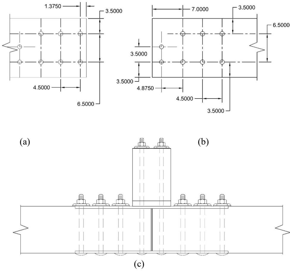
Figure 96. Upper Rail Connection Details: (a) Bolt Spacing Steel Splice Plate; (b) Bolt Spacing in Wood Rail; (c) Plan View of Connection
