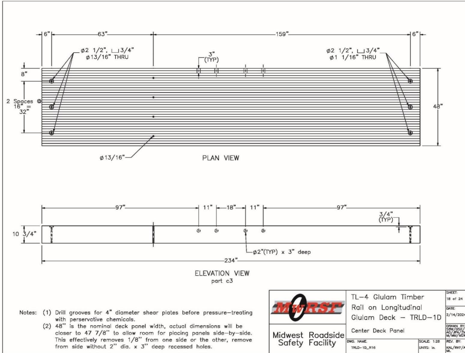
Figure 260. Deck Panel 2 Details, Test No. TRLD-1
