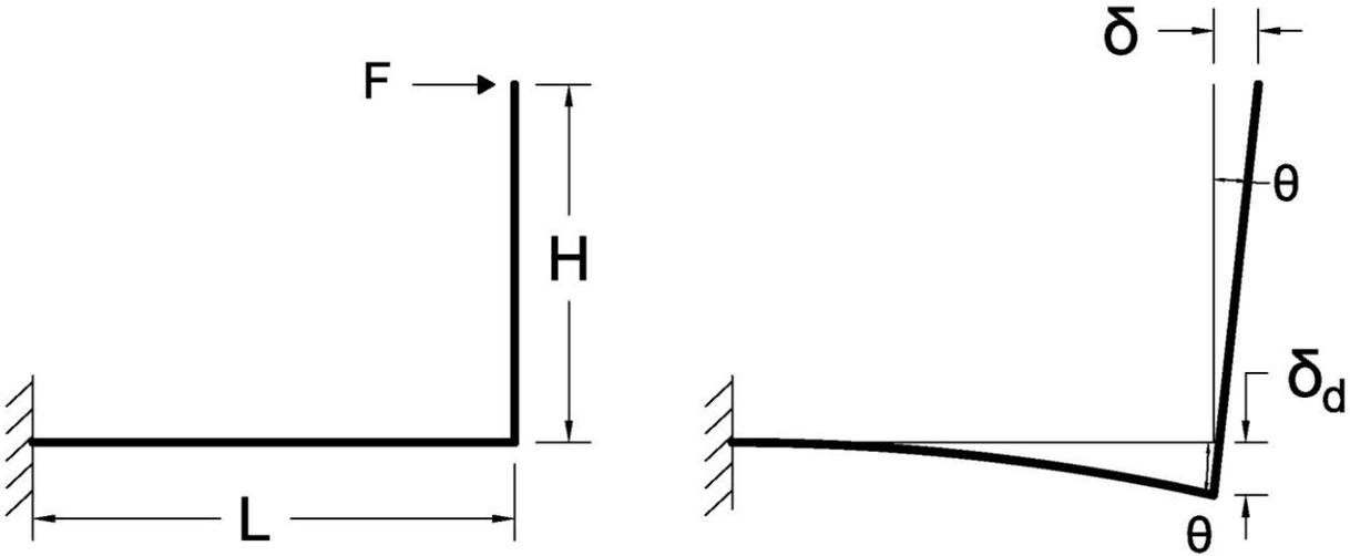
Figure 71. Timber Deck Overhang Deflection Diagram
