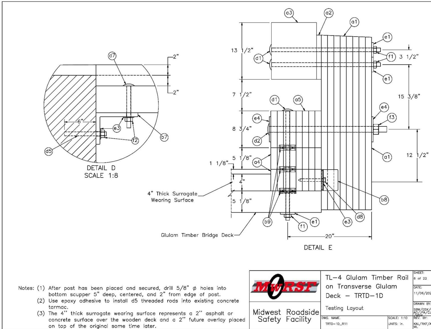
Figure 153. Post and Deck Assembly Details, Section View, Test No. TRTD-1
