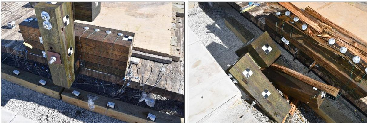
Figure 197. Post Before Test (left) and Post After Test (right)
