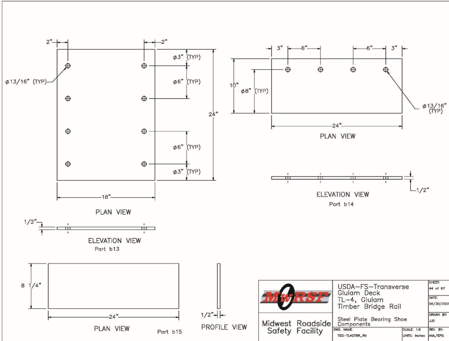
Figure O-44. Bridge Superstructure Pier Bearing Assembly Details
