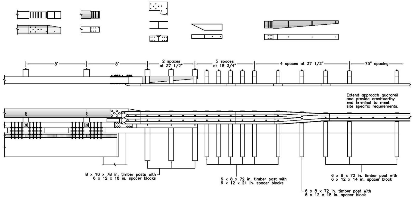
Figure K-40. Option 7.3 – Half-Post Spacing, 8-ft Gap, Cut L-Plate, Steel Reverse Taper, Curb Taper with Bumpout Behind Thrie-beam
