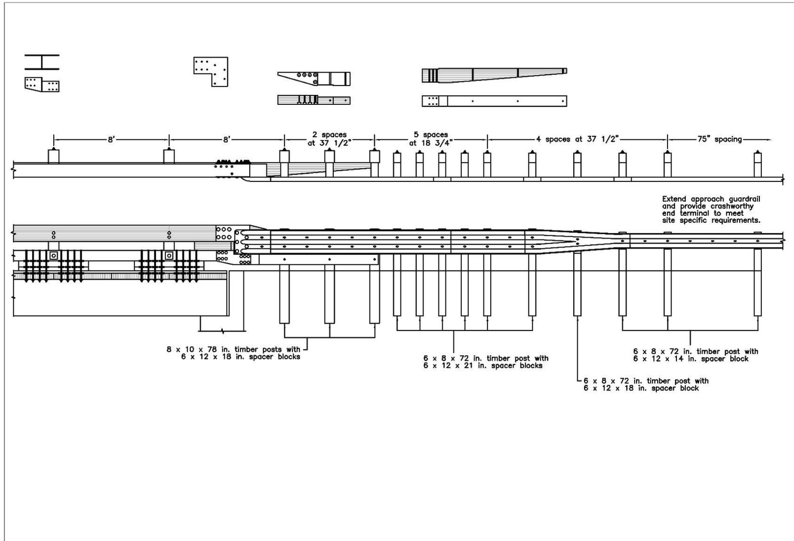
Figure K-38. Option 7.1 – Half-Post Spacing, 8-ft Gap, L-Plate, Wood Reverse Taper, Stepped Curb Taper
