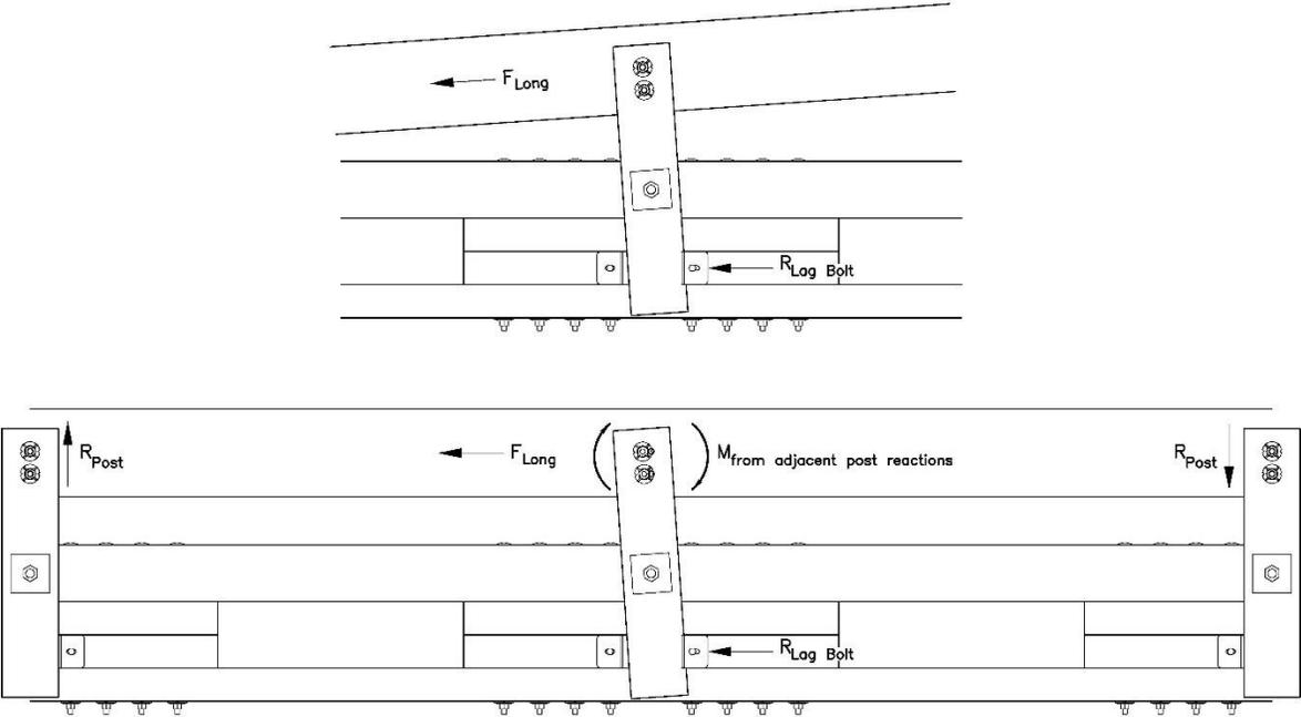
Figure 80. Resistance to Twist without Adjacent Posts (top) and Resistance to Twist with Adjacent Posts (bottom)
