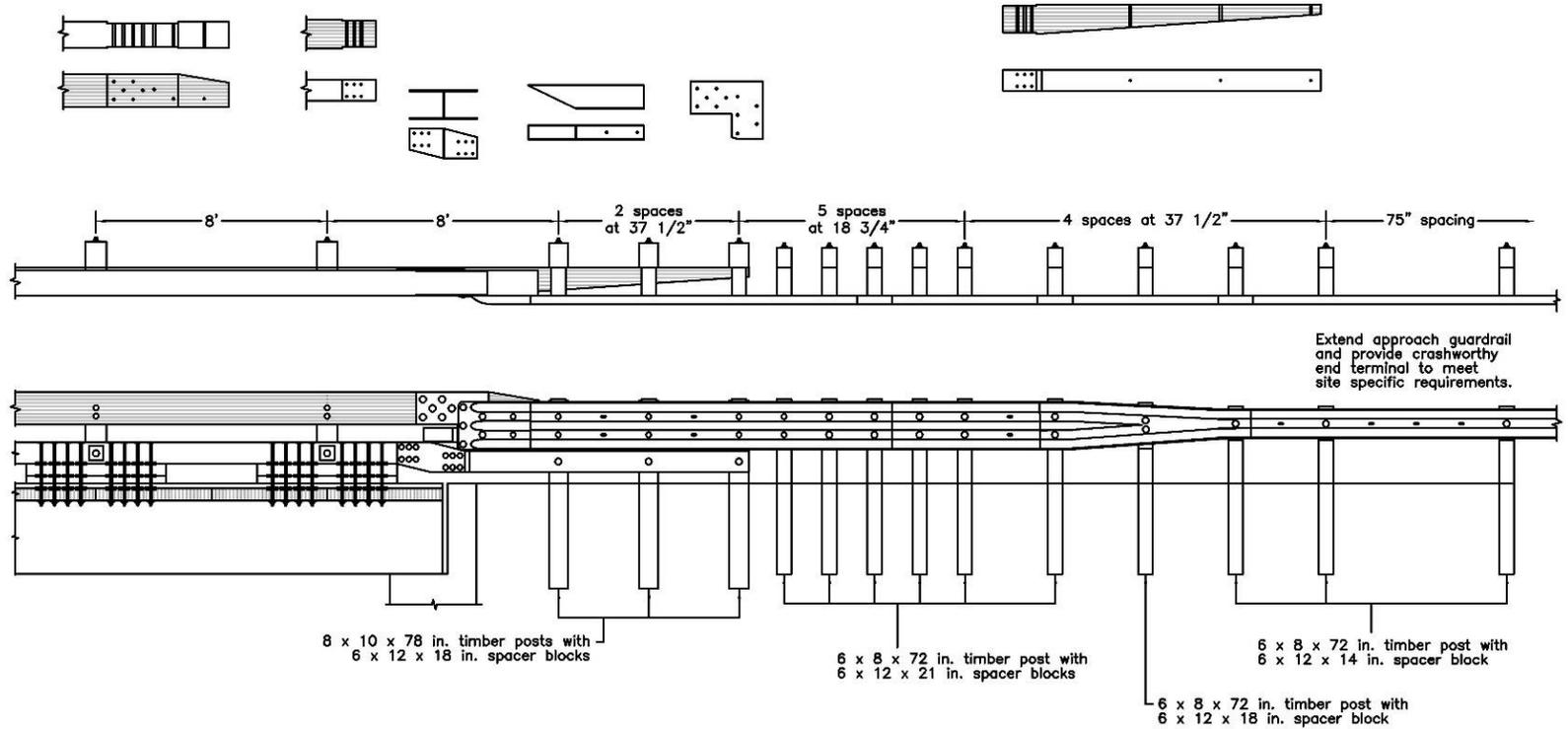
Figure K-33. Option 6.2 – Half-Post Spacing, 8-ft Gap, L-Plate, Steel Reverse Taper, Stepped Curb Taper
