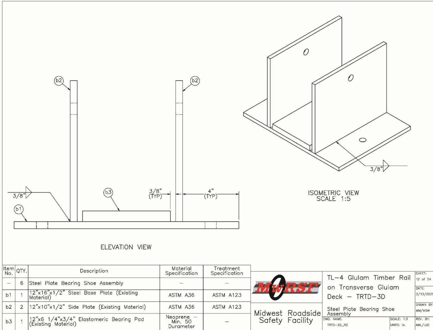
Figure N-12. Test No. TRTD-3 Steel Plate Bearing Assembly Details
