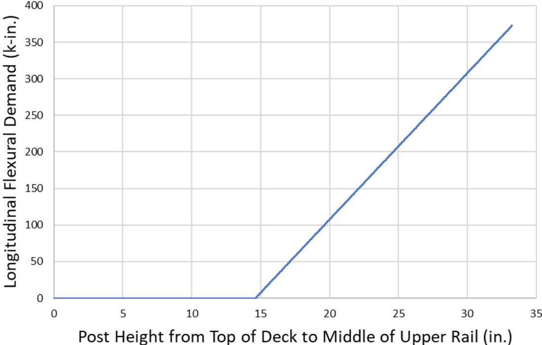
Figure 86. Longitudinal Flexural Demand, Post Diagram
