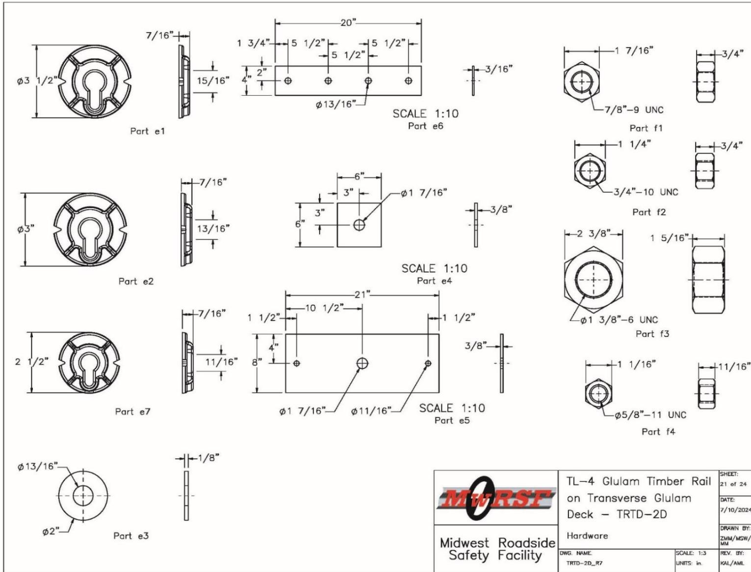
Figure 239. Connection Hardware Details, Page 2, Test No. TRTD-2
