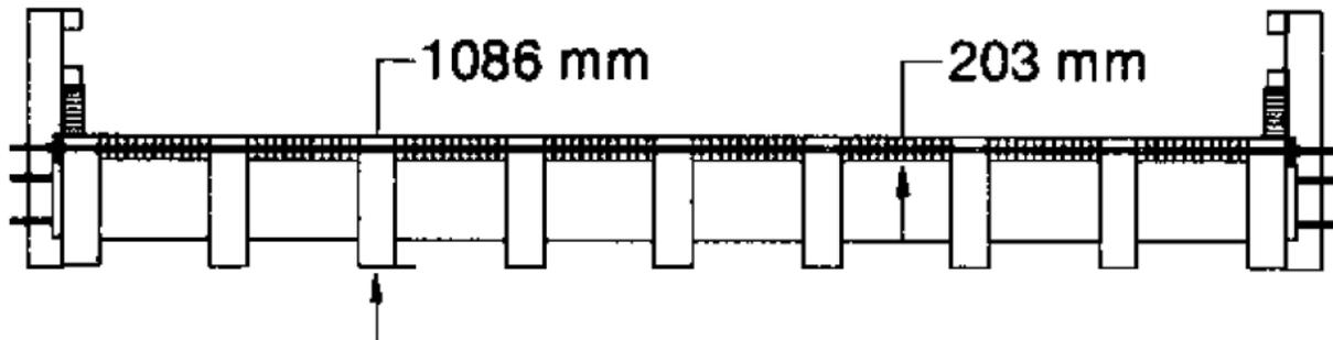
Figure 46. Cross-Section of Humphrey Stress-Laminated T-Beam Timber Bridge Deck [69]
