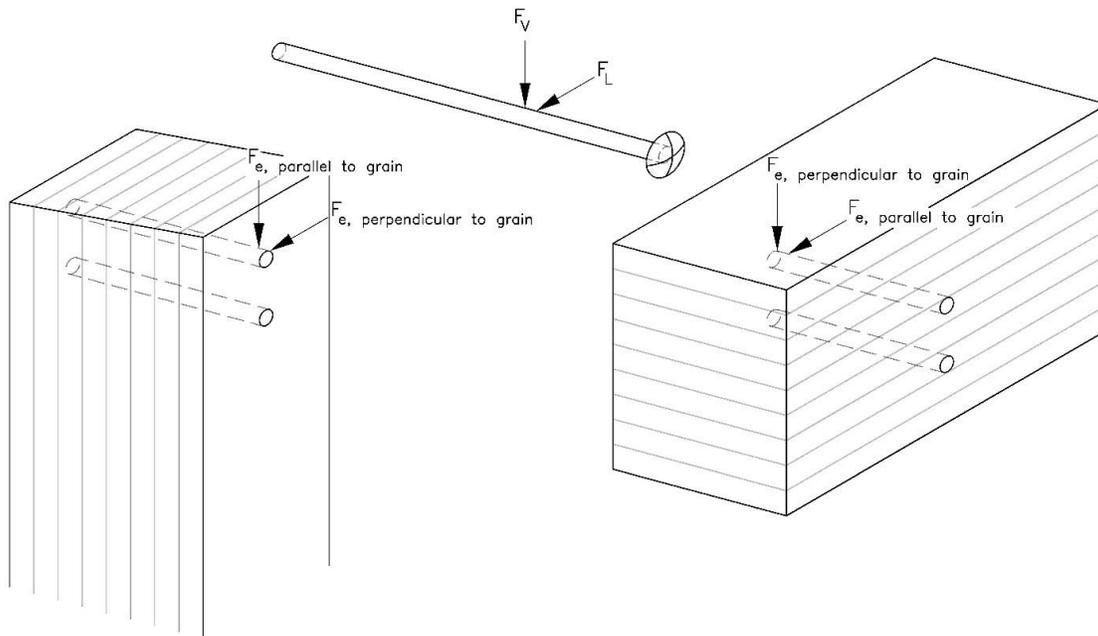
Figure G-1. Dowel Bearing Strength Orientation
