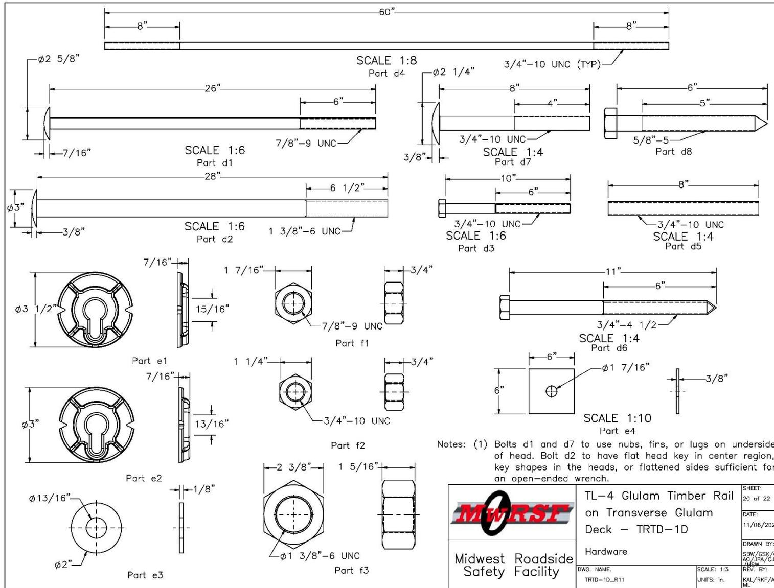
Figure 167. Connection Hardware Details, Test No. TRTD-1
