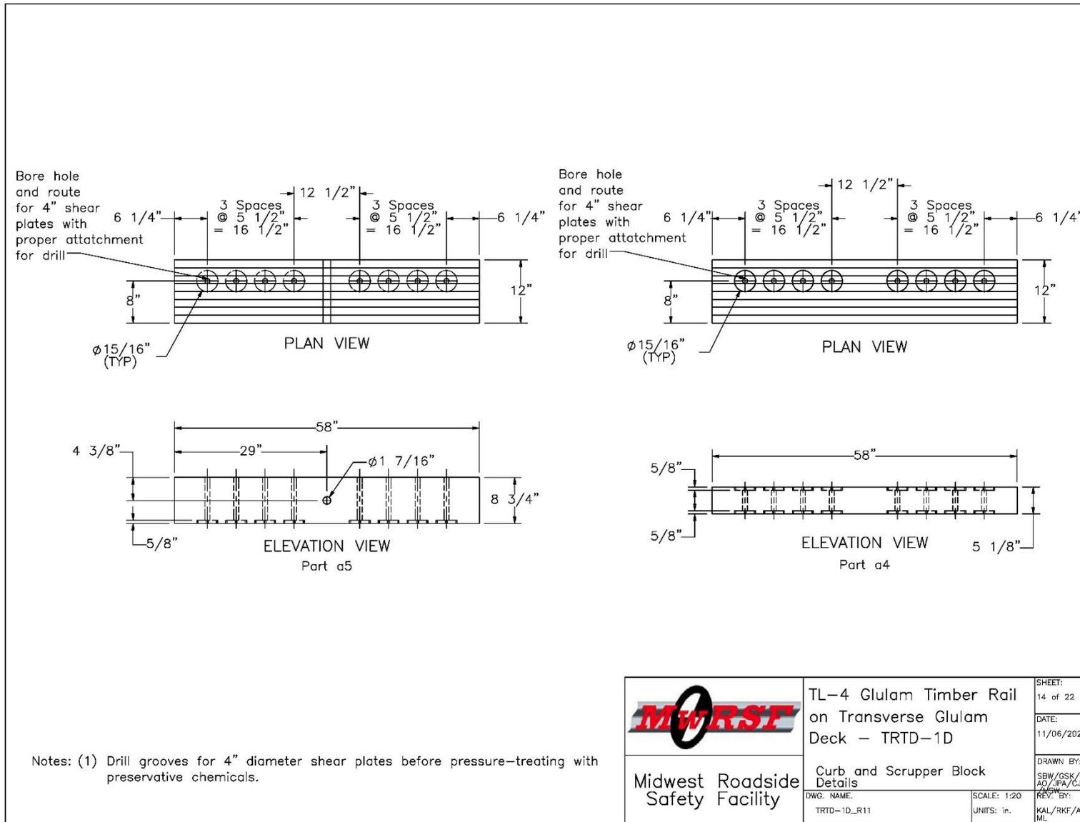
Figure 161. Scupper and Curb Rail Details, Test No. TRTD-1
