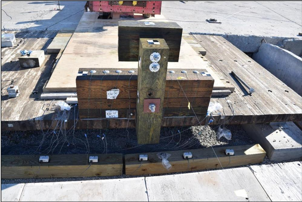
Figure 184. Vertical Bolt Axial Strain Gauges and All String Potentiometers
