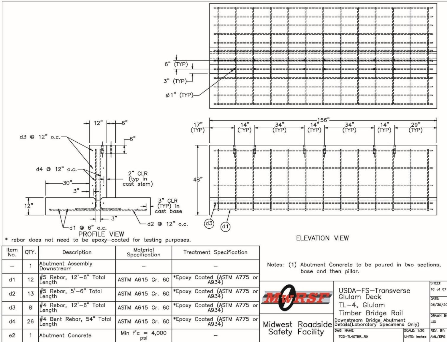
Figure O-18. Bridge Substructure North Abutment Details
