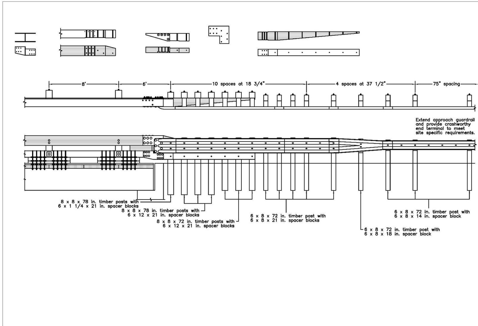
Figure K-44. Option 7.7 – Quarter-Post Spacing, 6-ft Gap, L-Plate, Wood Reverse Taper, Stepped Curb Taper
