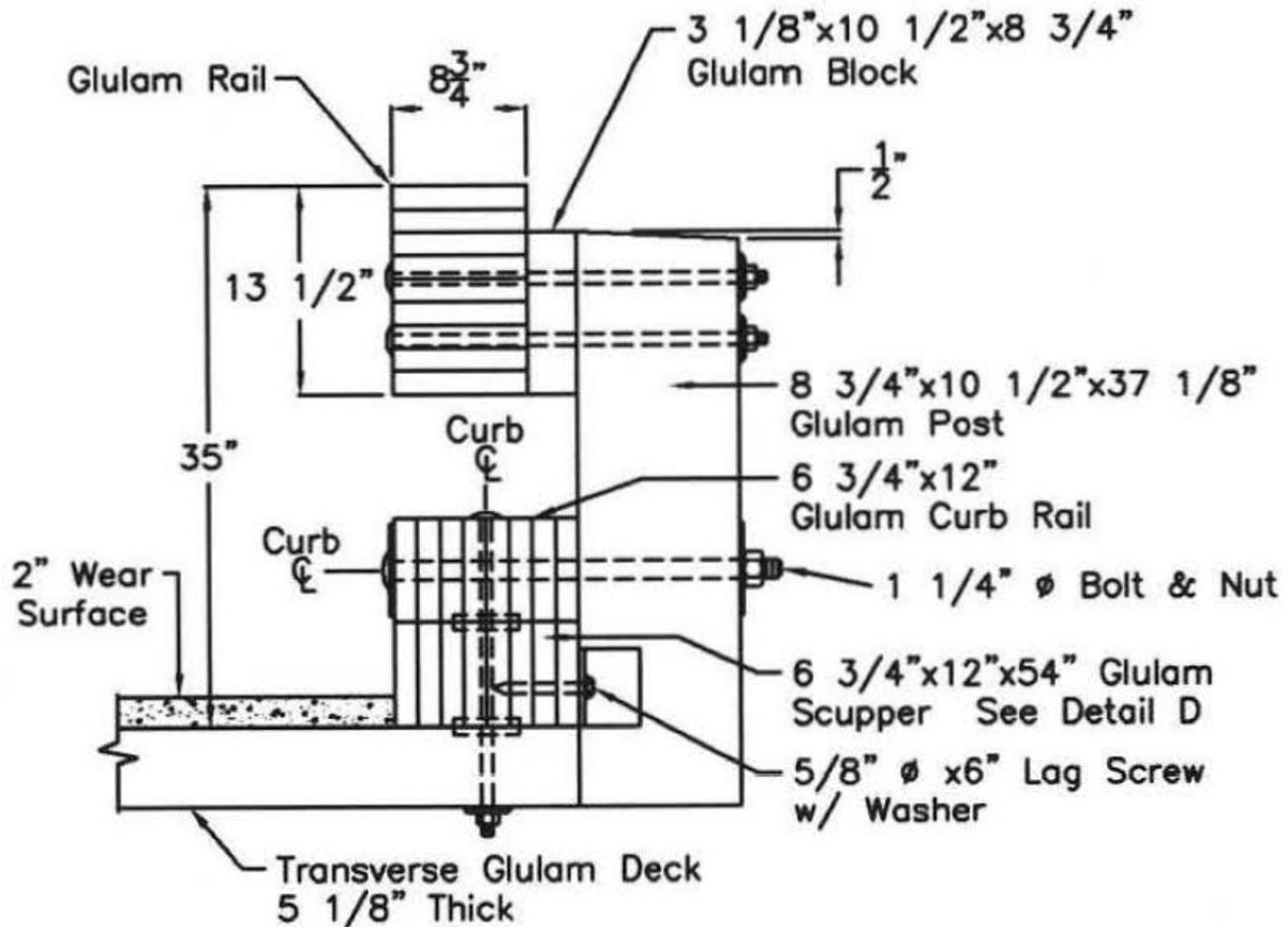
Figure 7. NCHRP 350 TL-4 Bridge Railing Cross-Section on Transverse Glulam Deck [20]
