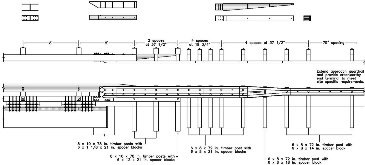
Figure K-17. Option 3.2 – Half-Post Spacing, 8-ft Gap, No Plate, Missing Bolt, Removed Blockout, Wood Reverse Taper, Curb Taper Behind Thrie-Beam
