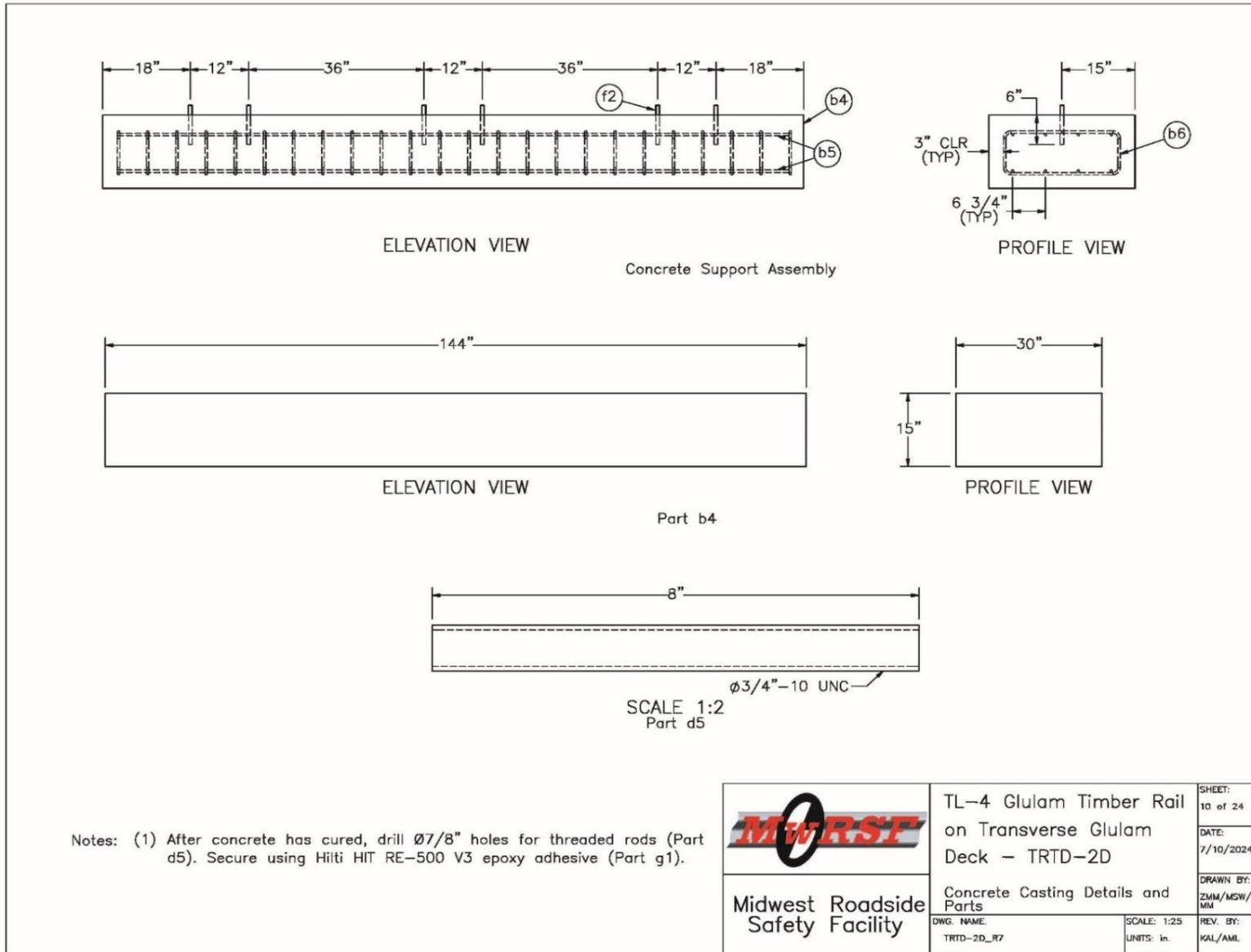
Figure 228. Concrete Casting and Embedded Rod Details, Test No. TRTD-2
