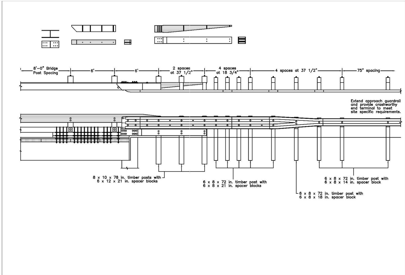
Figure K-12. Option 2.7 – Half-Post Spacing, 6-ft Gap, Removed Blockout, Wood Reverse Taper, Stepped Thick Curb Taper
