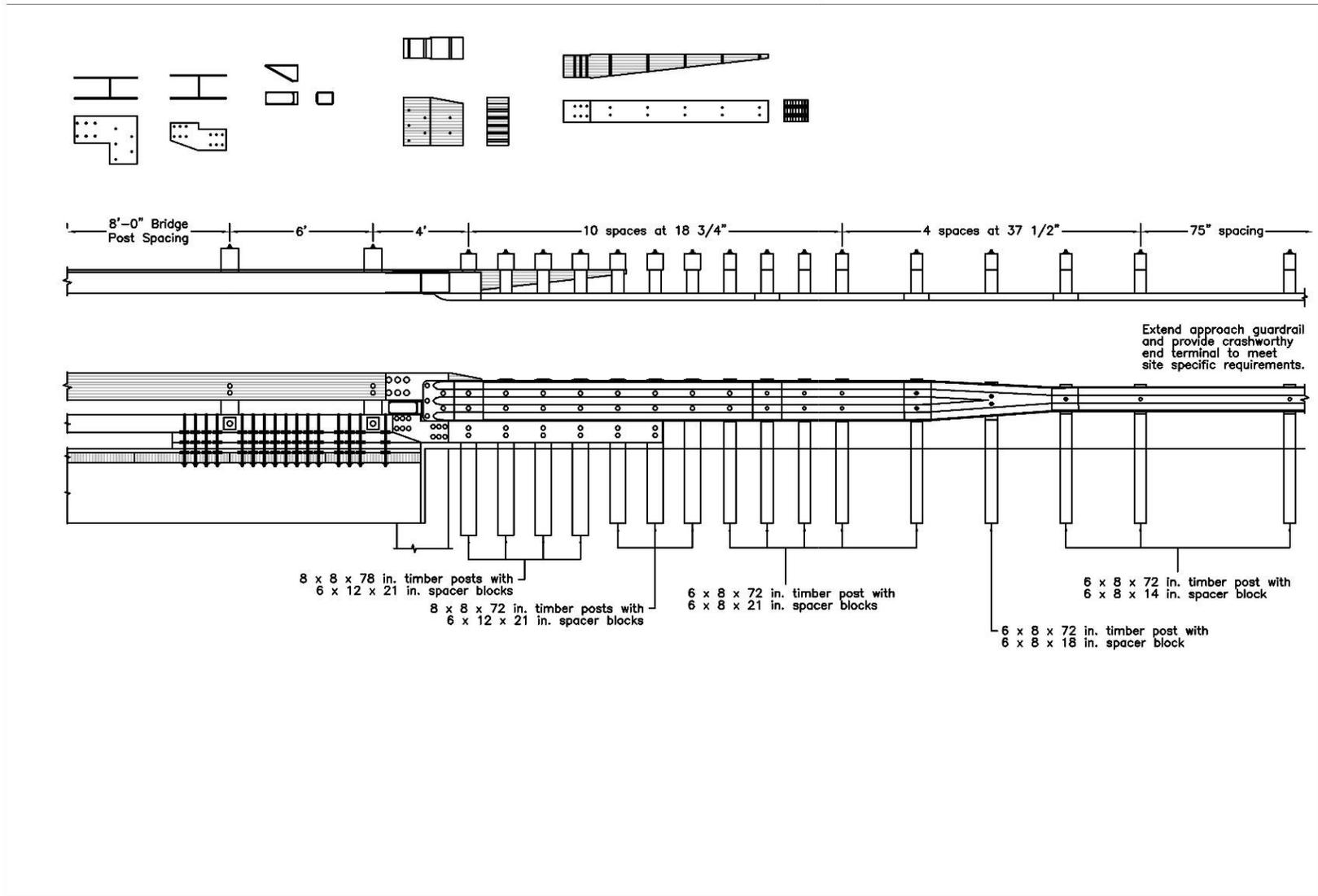
Figure K-9. Option 2.4 – Quarter-Post Spacing, 6-ft Gap, L-Plate, Separated Block, Removed Blockout, Steel Reverse Taper, Thick Stepped Curb Taper
