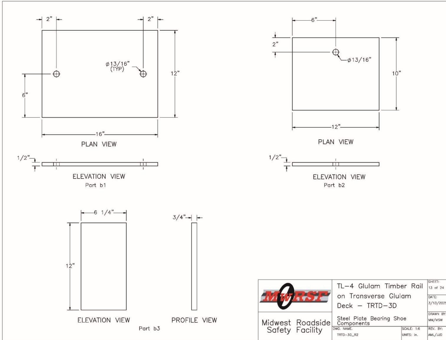
Figure N-13. Test No. TRTD-3 Steel Plate Bearing Assembly Component Details
