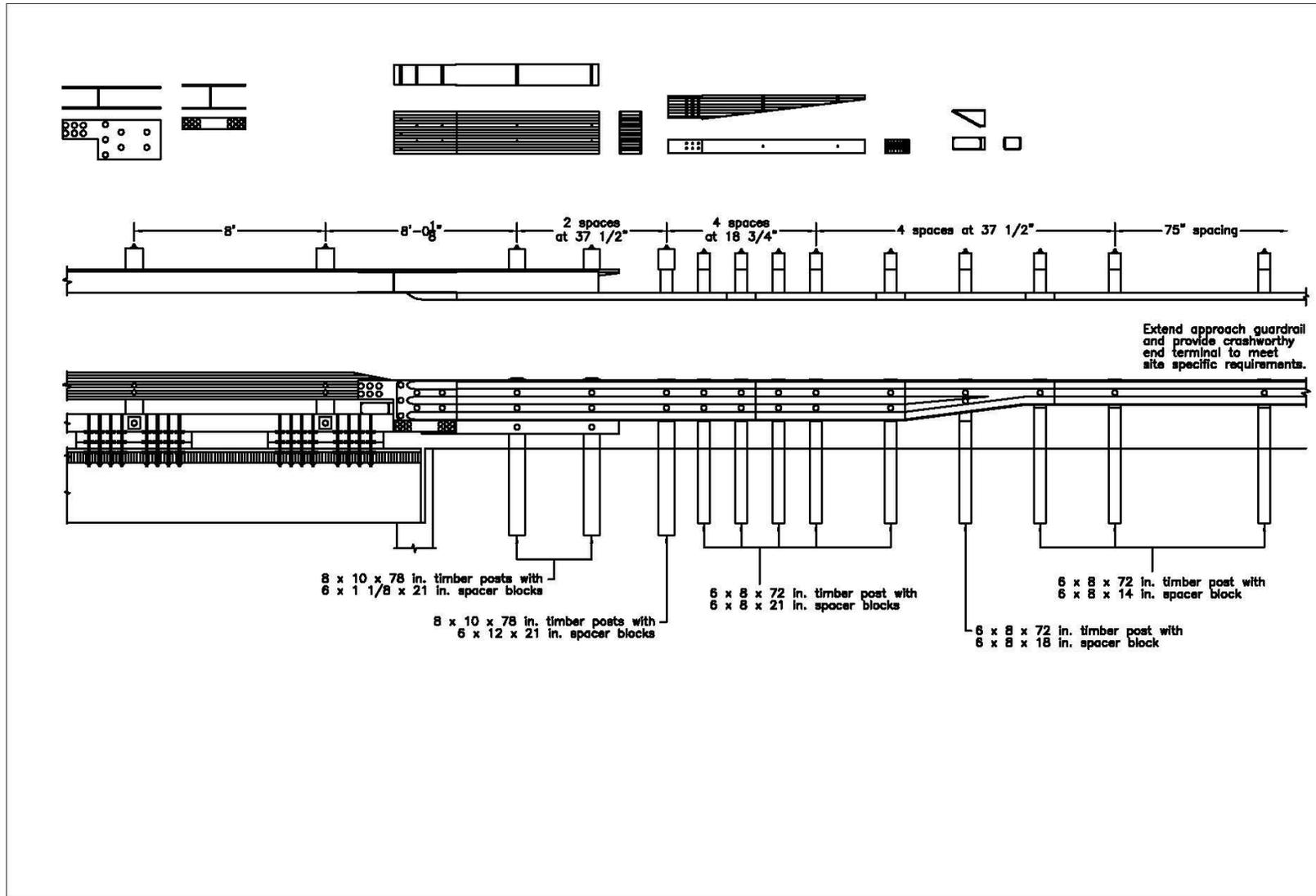
Figure K-5. Option 1.5 – Half-Post Spacing, 8-ft Gap, L-Plate, Separated Block, Removed Blockouts, Steel Reverse Taper, Thin Curb Taper
