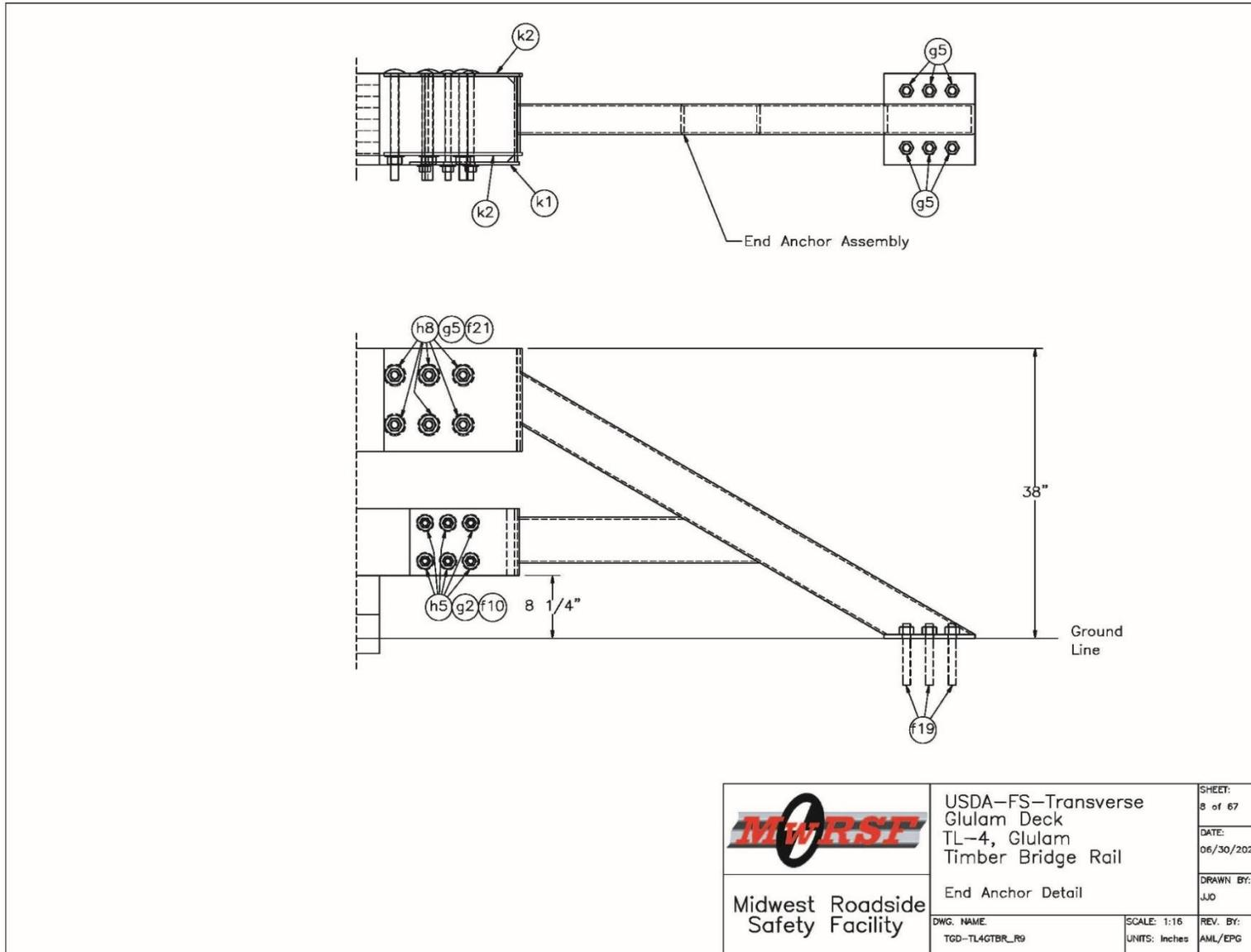
Figure O-8. Bridge Railing End Anchor Detail
