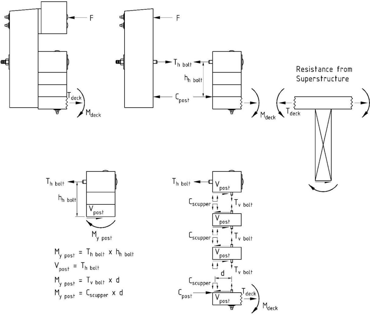
Figure 77. Post Configuration Loading Diagram
