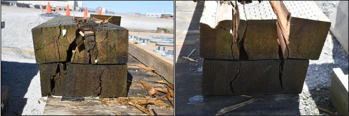
Figure 194. Scupper Ends After Impact on Left End and Right End
