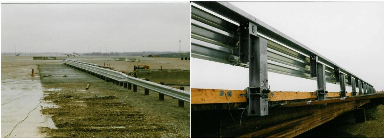
Figure 8. NCHRP 350 TL-4 Steel Thrie-Beam Bridge Railing on Transverse Glulam Deck [25]
