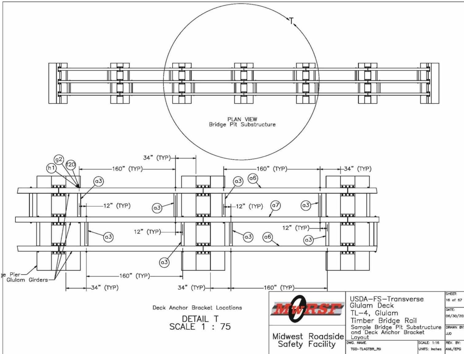
Figure O-16. Bridge Pit Typical Substructure Span Details
