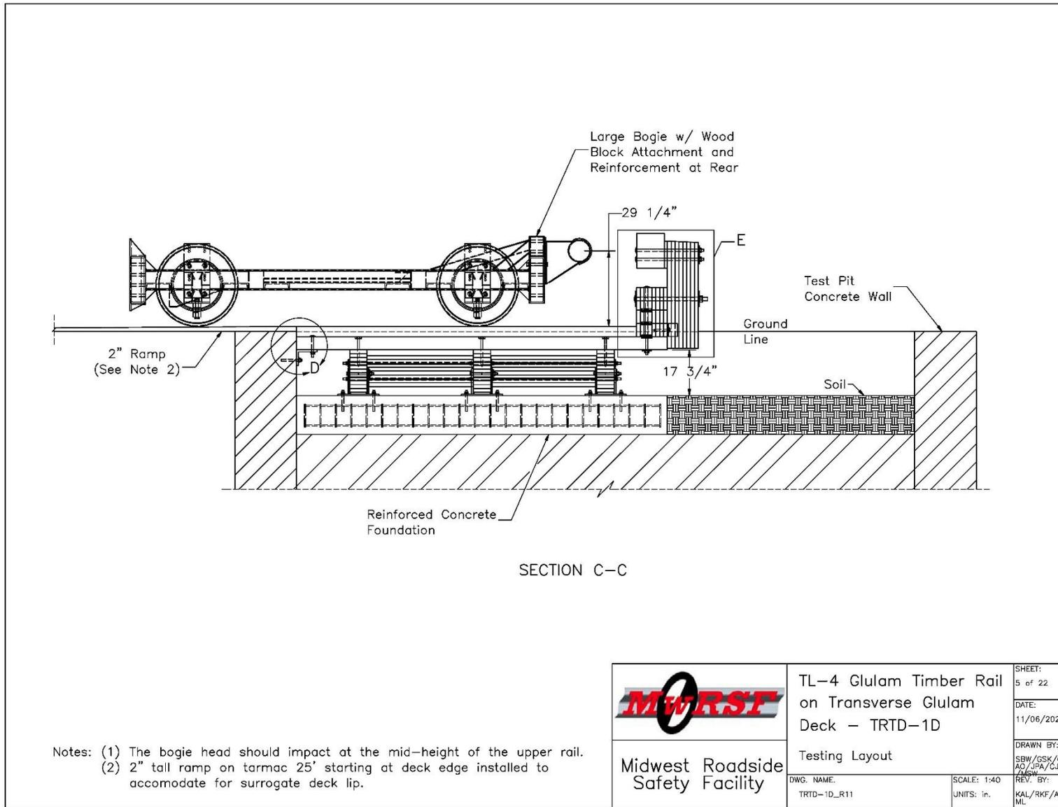
Figure 152. Layout, Elevation View, Test No. TRTD-1
