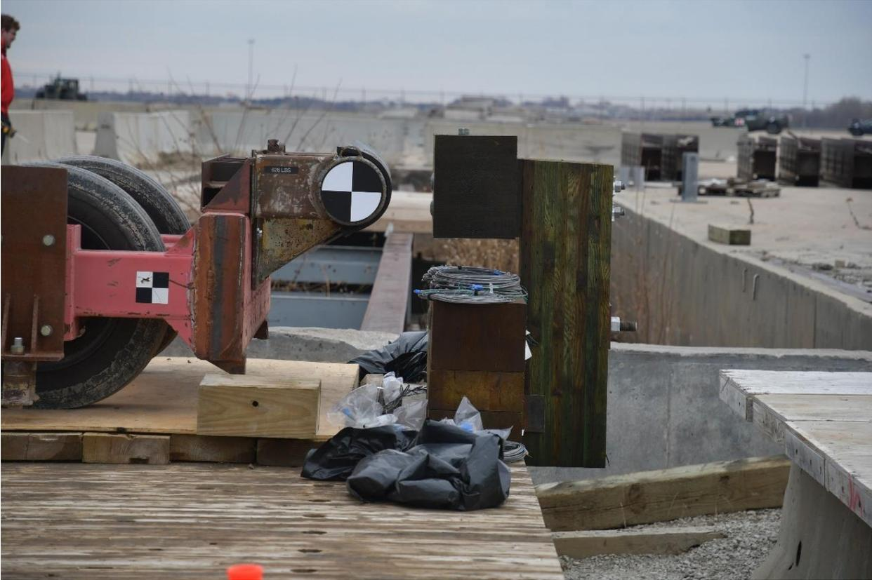
Figure 176. Side View of Assembled Bridge Post and Impact Bogie Vehicle, Test No. TRTD-1
