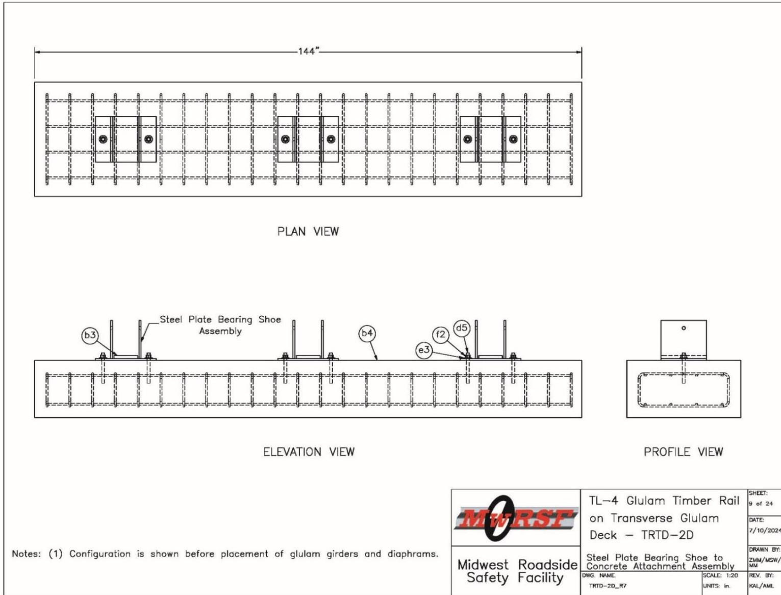
Figure 227. Concrete and Bearing Assembly Details, Test No. TRTD-2
