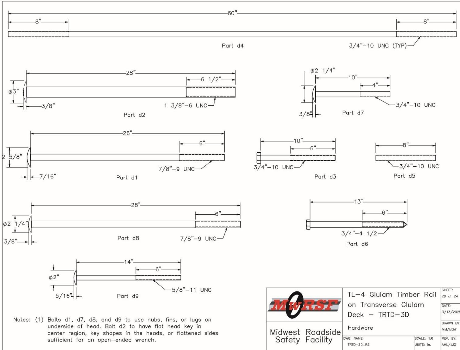
Figure 270: Test No. TRTD-3 Connection Hardware Details, Page 1
