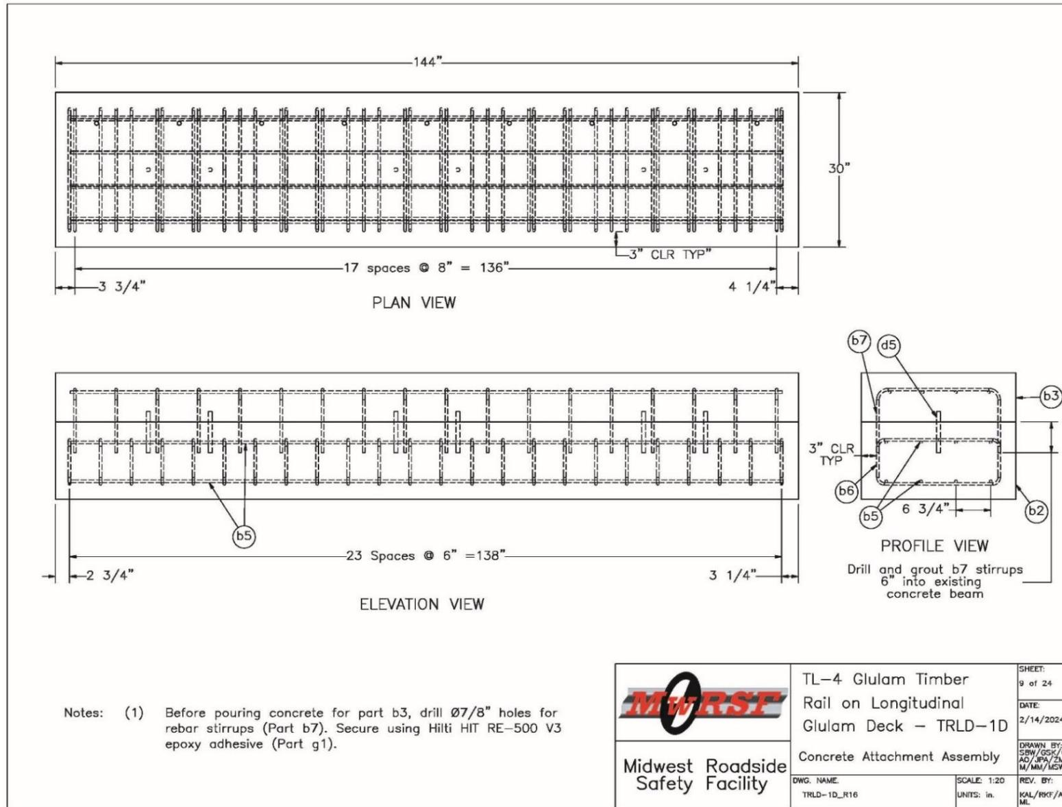
Figure 251. Rebar Layout, Test No. TRLD-1
