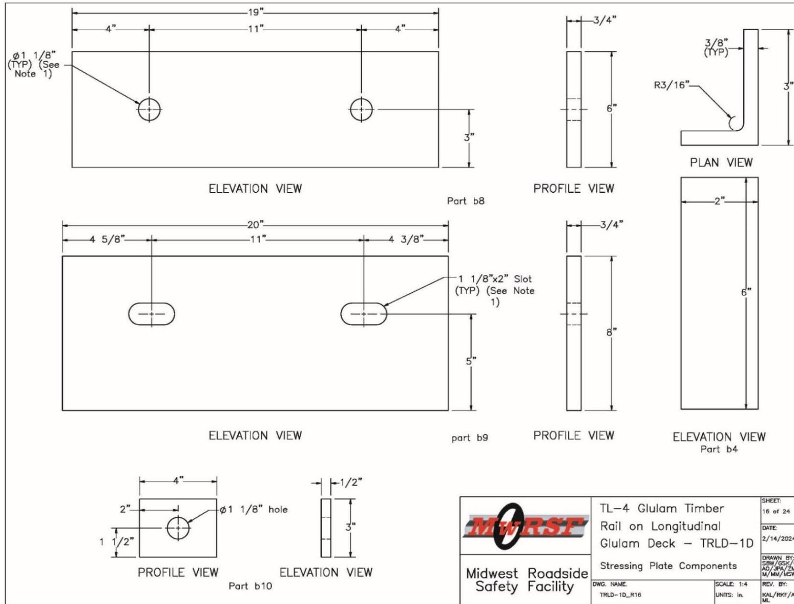
Figure 258. Stressing Plate Assembly Component Details, Test No. TRLD-1
