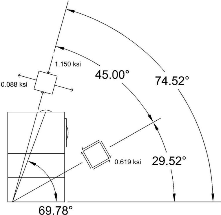
Figure 216. Mohr's Circle of Stresses in Scupper at Compression Block Assuming Low Friction Coefficient
