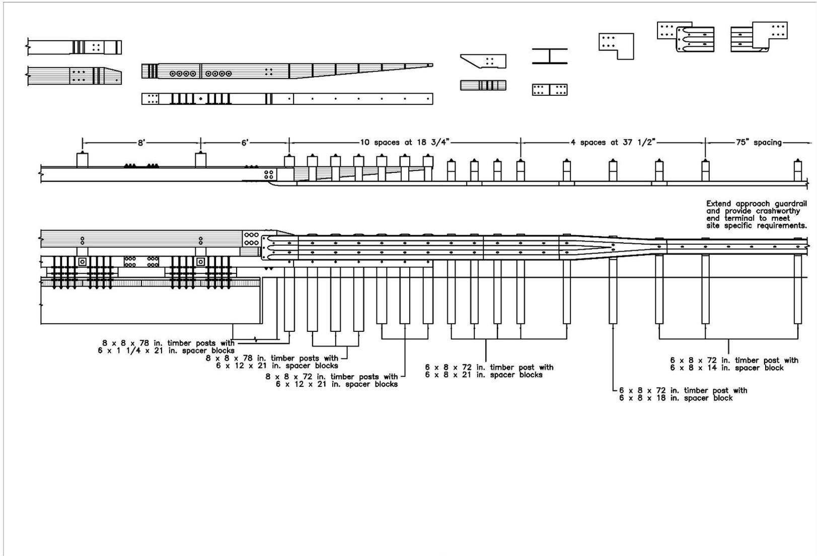
Figure K-48. Option 7.11 – Quarter-Post Spacing, 6-ft Gap, Welded L-Plate to End Shoe, Wood Reverse Taper, Curb Taper Behind Thrie-beam
