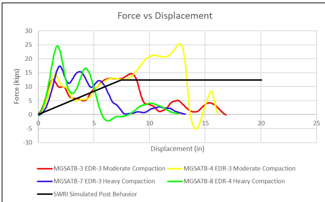
Figure 111. Load-Displacement Behavior of 8x8 Posts from Bogie Testing at MwRSF and Pendulum Testing at SwRI [37, 39]
