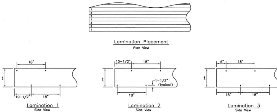
Figure 33. Nail-Laminated Lumber with Staggered Nailing Pattern [48]
