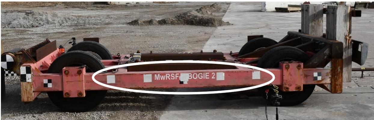
Figure 133. Five Retroreflective Optic Traps on Side of Bogie Vehicle
