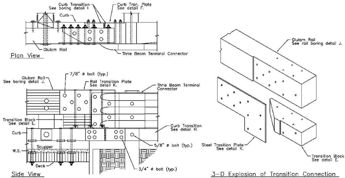
Figure 112. AGT to Bridge Railing Connection Developed for NCHRP-350 TL-4 System [20]
