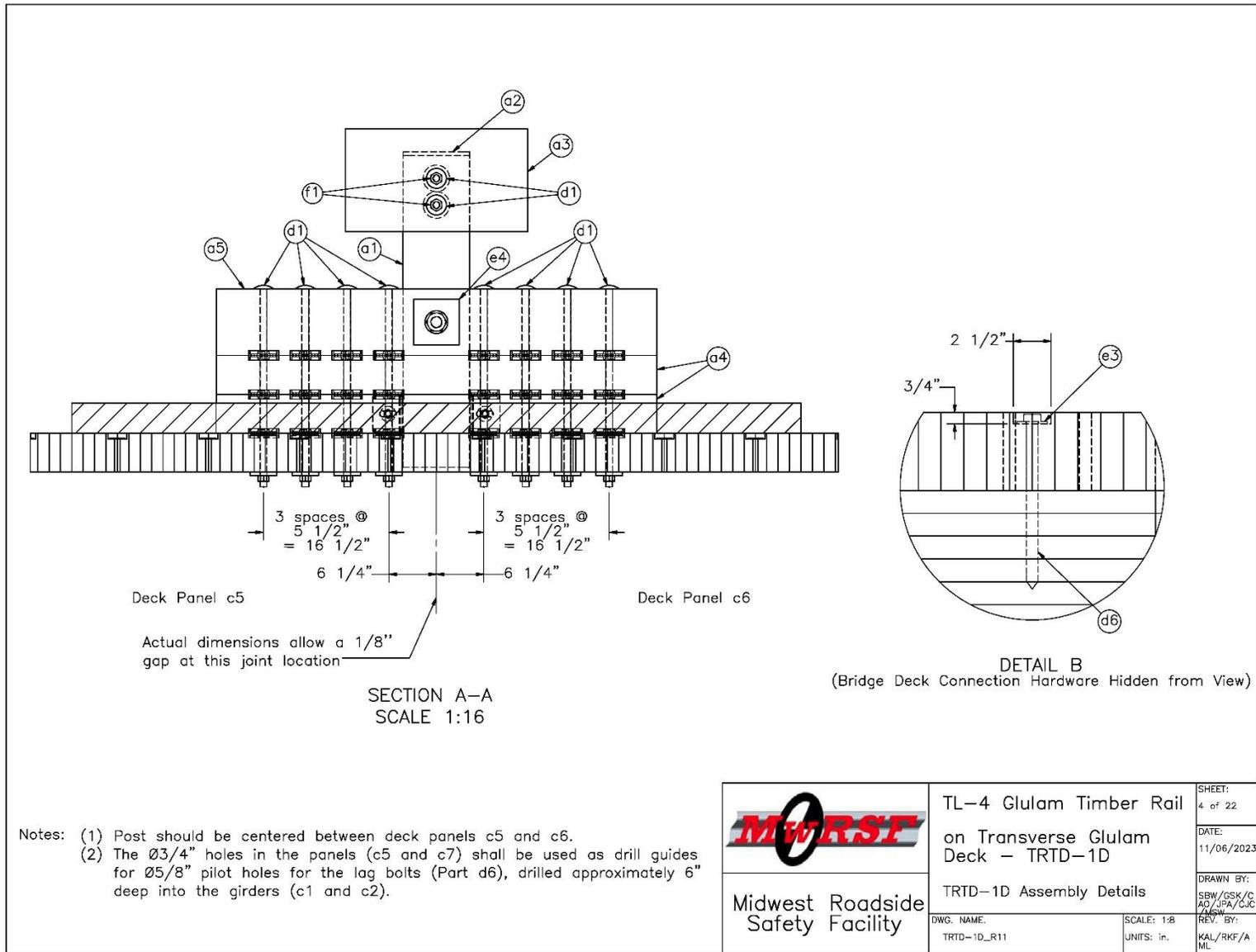
Figure 151. Post and Deck Assembly Details, Test No. TRTD-1
