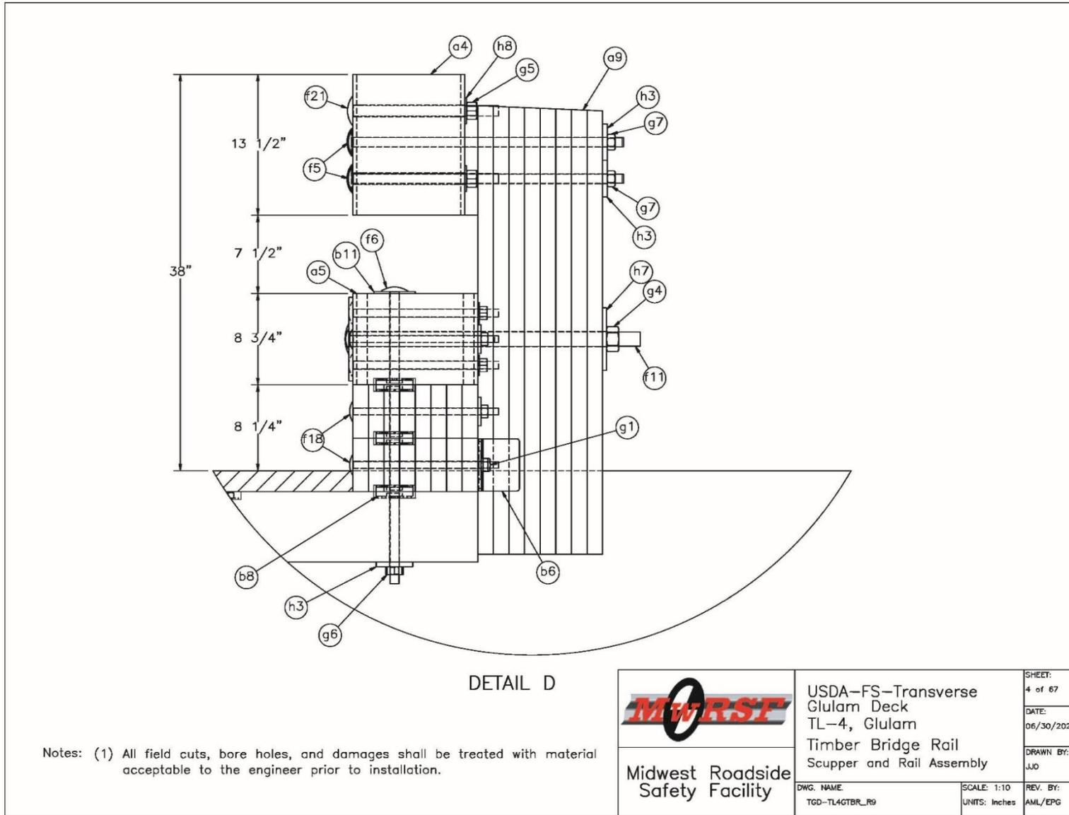
Figure O-4. Bridge Railing Assembly Cross-Section View
