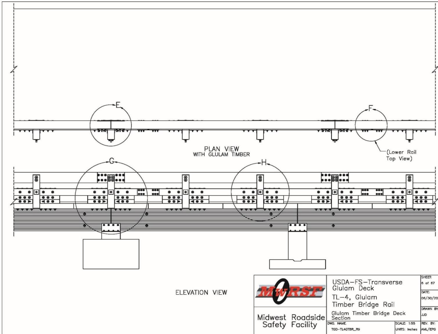
Figure O-6. System Plan and Elevation View of Upper and Curb Rail Splice Locations
