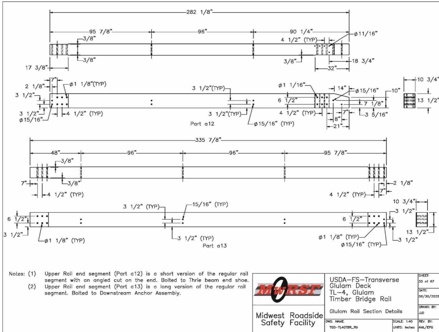
Figure O-33. Bridge Upper Glulam Railing End Pieces
