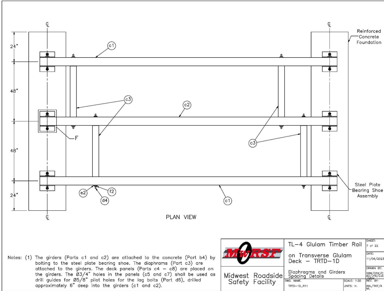
Figure 154. Diaphragm and Girder Spacing Details, Test No. TRTD-1
