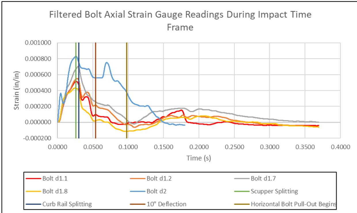
Figure 201. Test No. TRTD-1 Bolt Axial Strain Gauge Strain vs. Time
