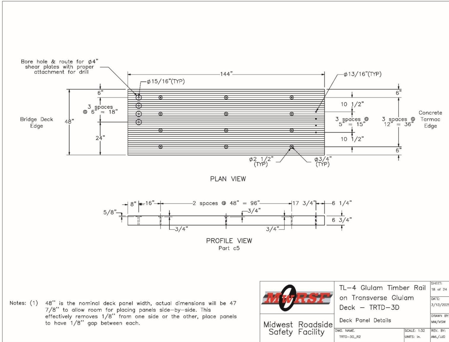
Figure 268: Test No. TRTD-3 Deck Panel Details, Page 2
