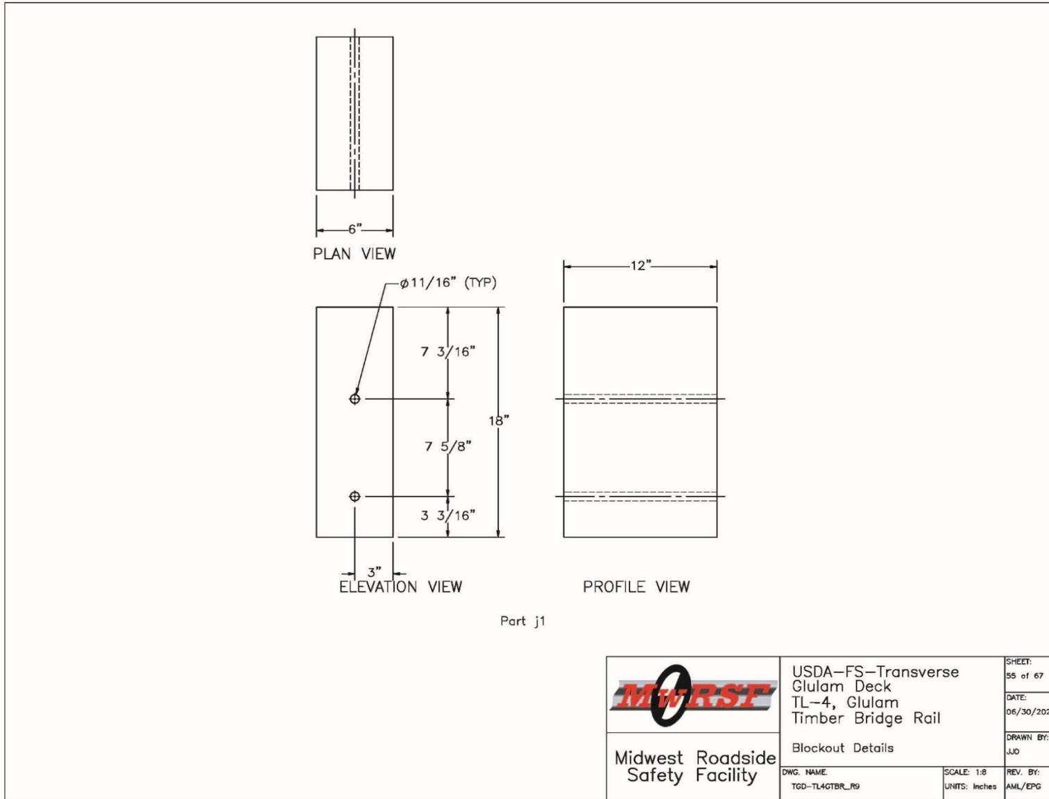
Figure O-55. Bridge AGT Blockout Details, Page 1
