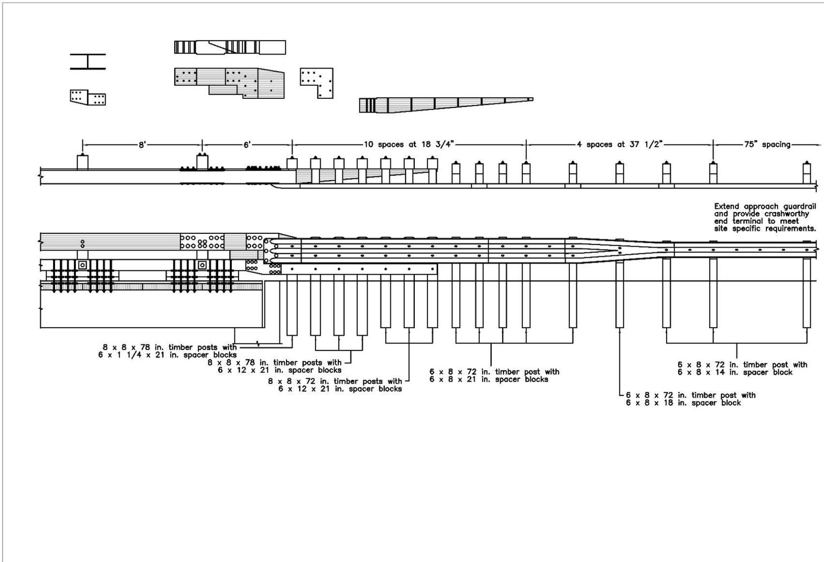
Figure K-49. Option 7.12 – Quarter-Post Spacing, 6-ft Gap, L-Plate, Custom Glulam Piece, Stepped Curb Taper
