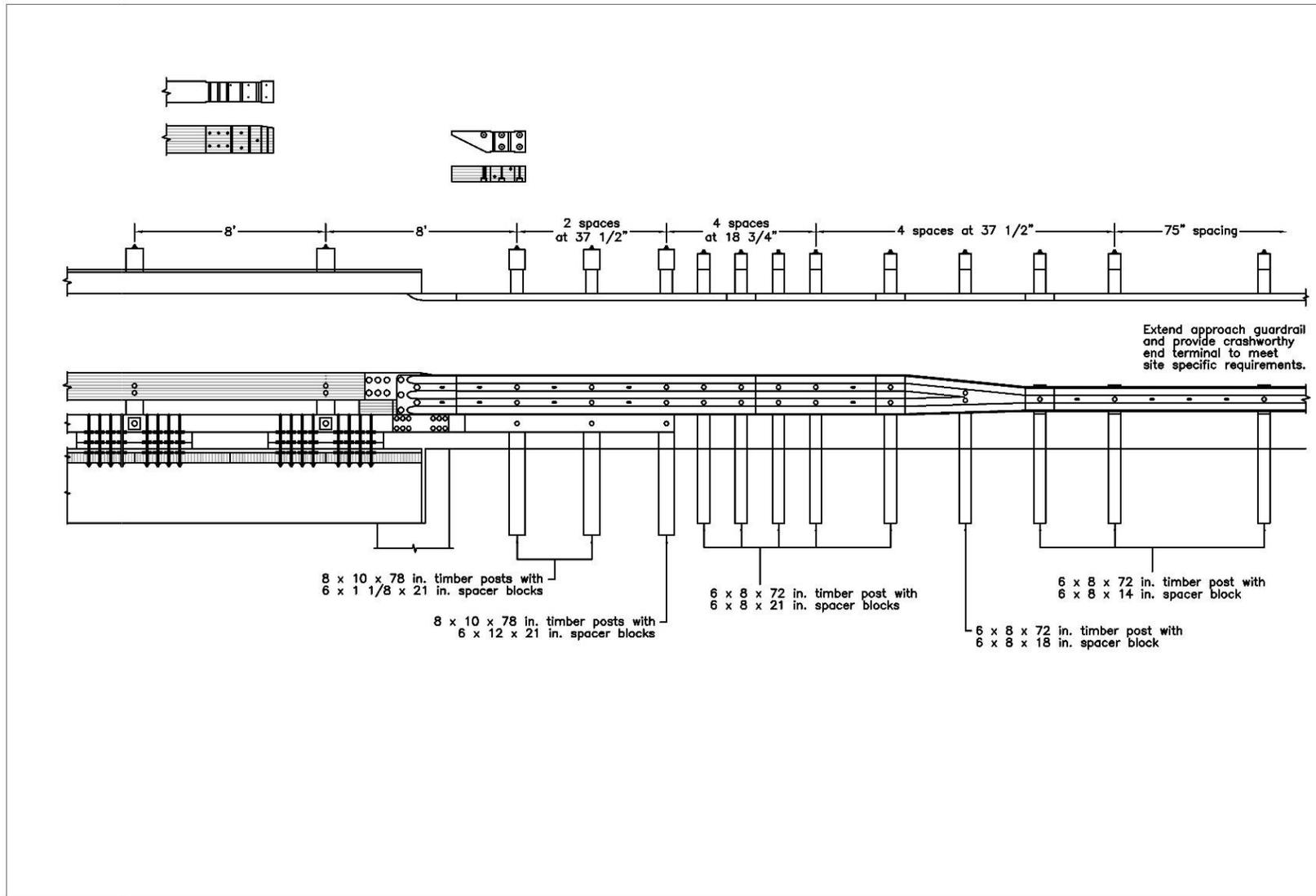
Figure K-23. Option 3.8 – Half-Post Spacing, 8-ft Gap, Custom Thrie-beam to W-beam Transition, L-Plate, Wood Reverse Taper, Curb Taper
