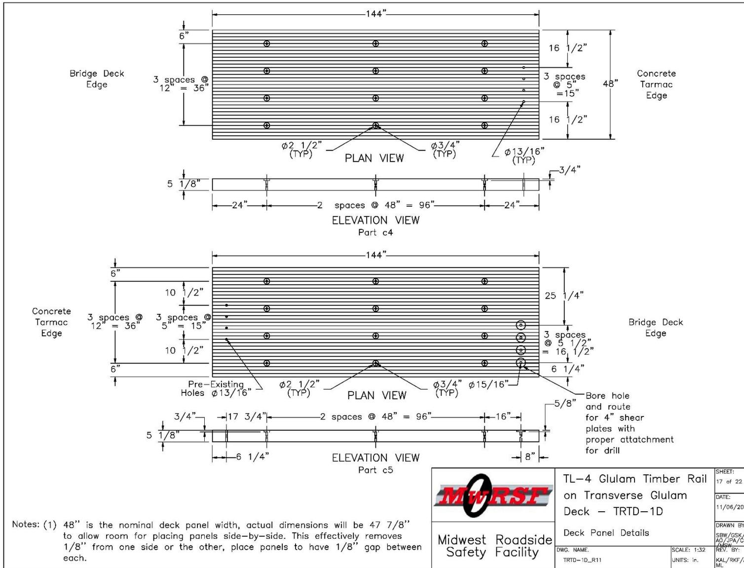
Figure 164. Deck Panel Details, Page 1, Test No. TRTD-1
