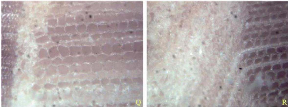
Figure 56. Cell Wall Collapse at Microscopic Level [93]
