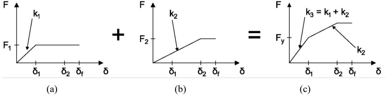
Figure 69. Bilinear Post 1 (a) and Bilinear Post 2 (b) with Linear Stiffness Used to Simulate Trilinear Post (c) Stiffness
