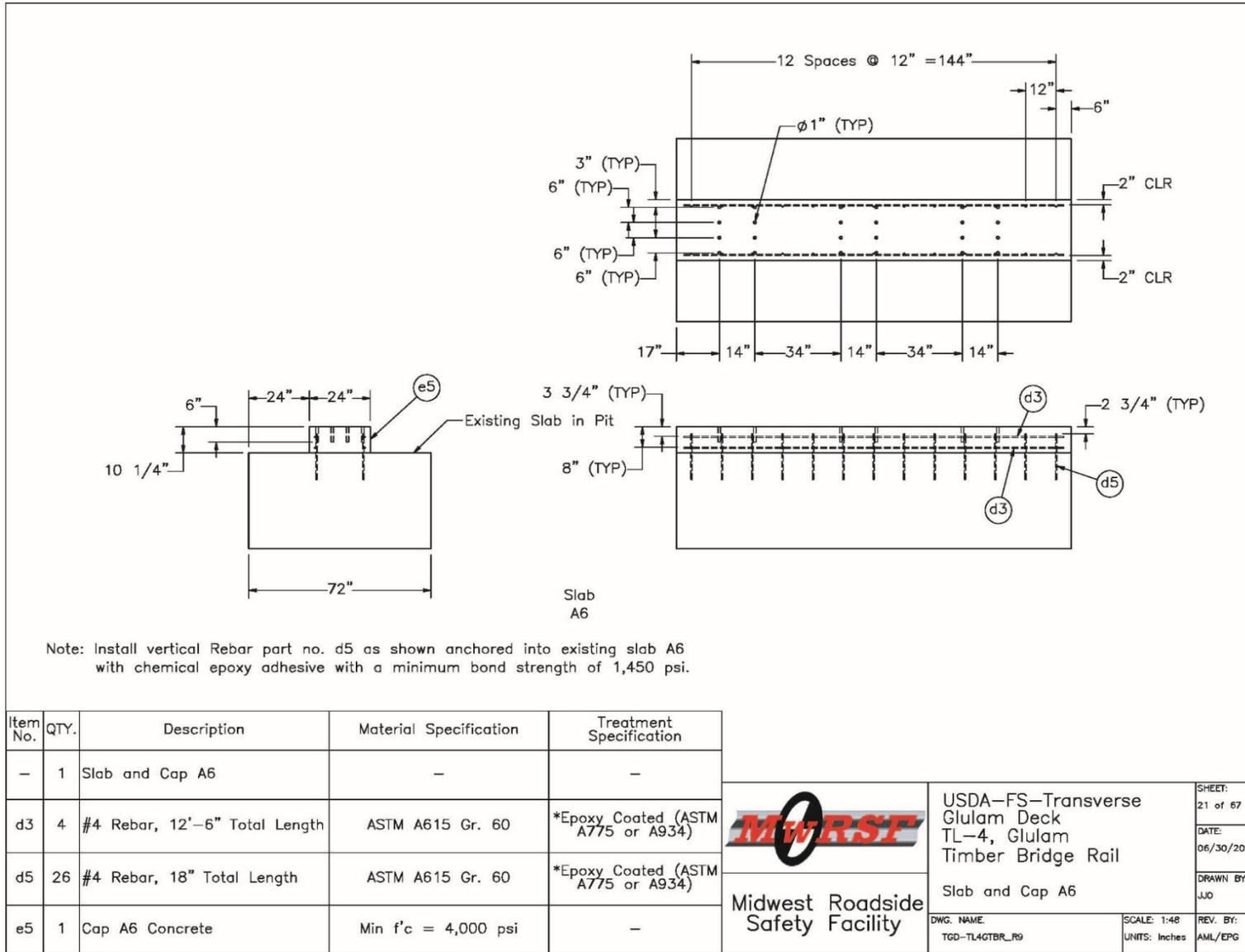
Figure O-21. Bridge Substructure Intermittent Pier A6 Details
