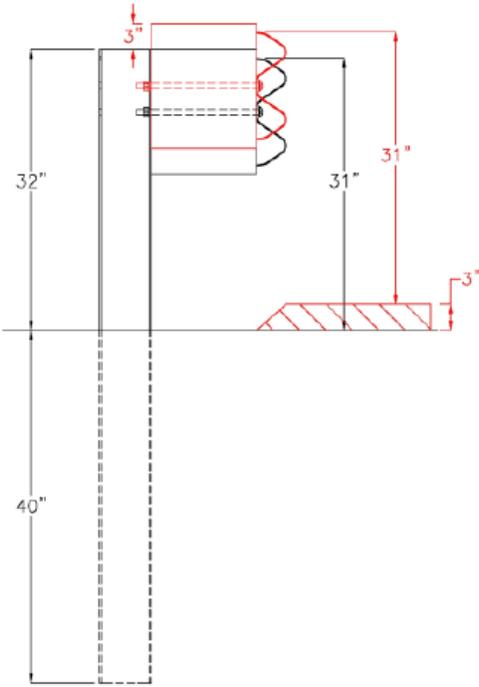
Figure 27. AGT System with Adjustable Height Post Cross-Section for Connecting Guardrail [38]
