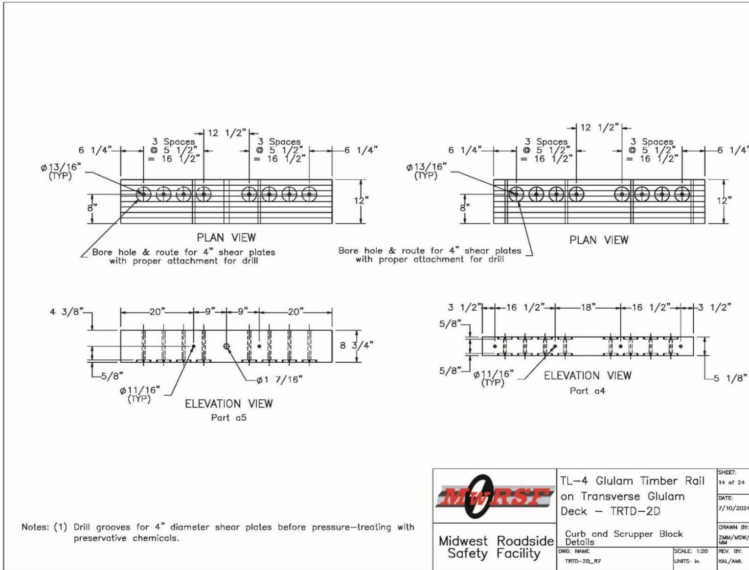
Figure 232. Scupper and Curb Rail Details, Test No. TRTD-2
