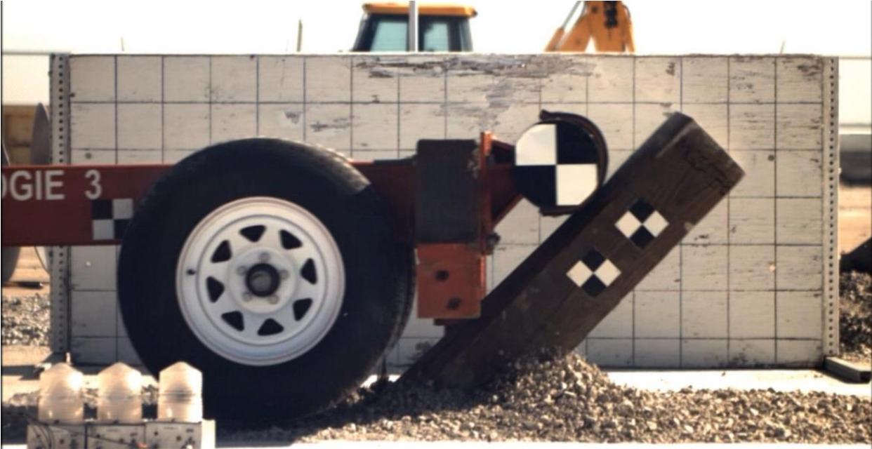
Figure 22. Bogie Test MGSATB-8 on 8-in. x 8-in. Post Embedded 54-in. into Heavily Compacted Soil
