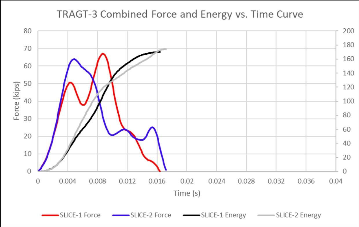
Figure 141. Combined Force and Energy vs. Time Curve, Test No. TRAGT-3
