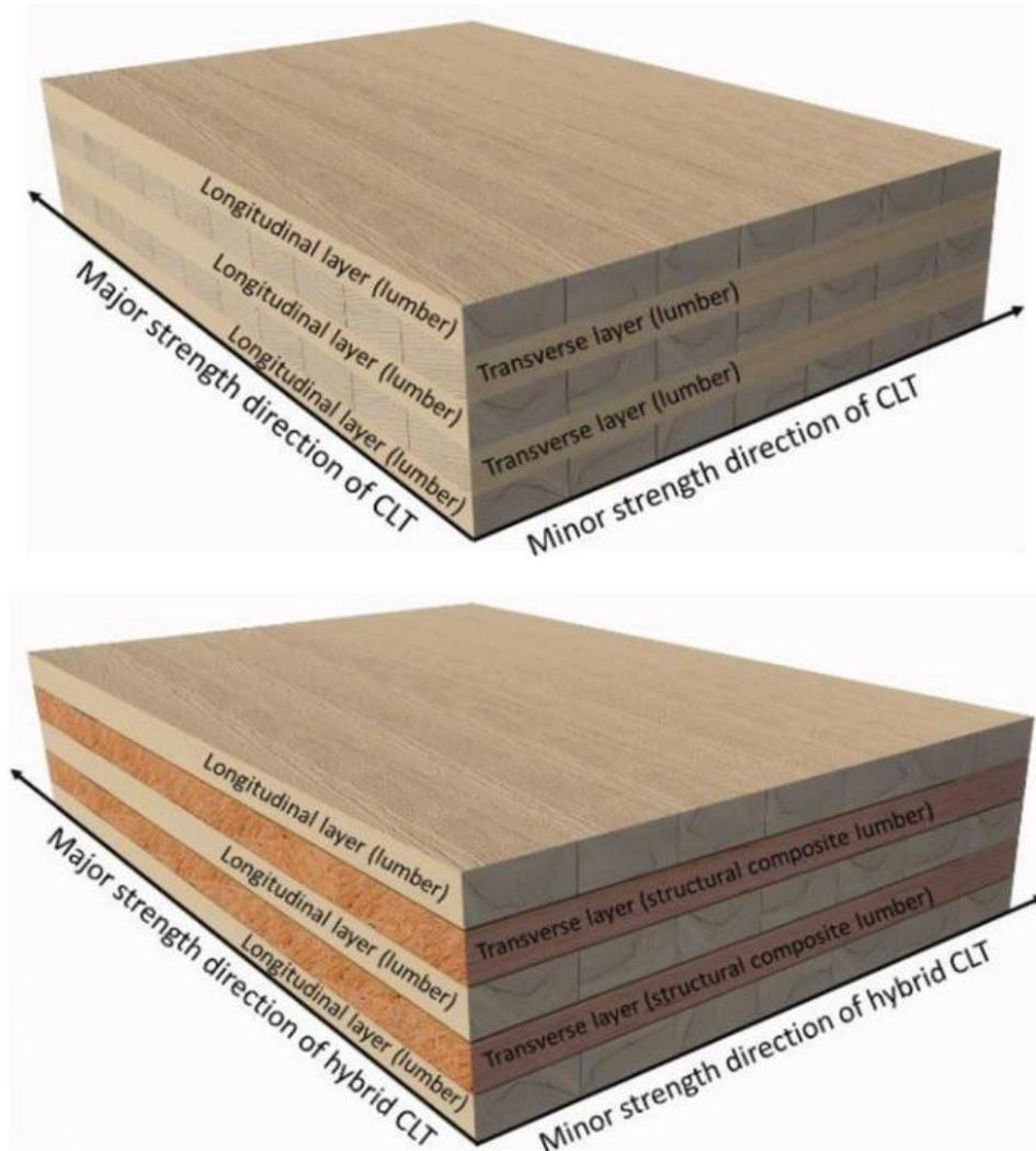
Figure 49. Cross-Laminated Timber [49]
