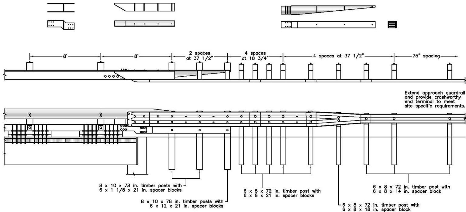
Figure K-11. Option 2.6 – Half-Post Spacing, 8-ft Gap, No Plate, Missing Bolts, Removed Blockout, Wood Reverse Taper, Stepped Curb Taper
