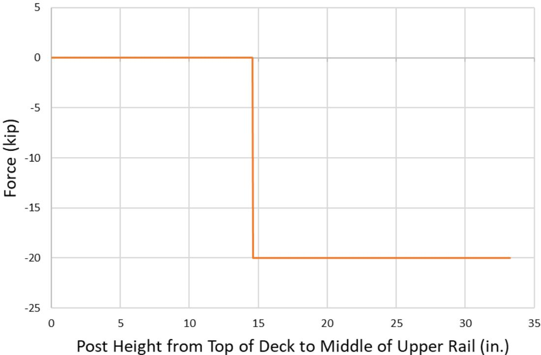
Figure 83. Longitudinal Shear Demand, Post Diagram
