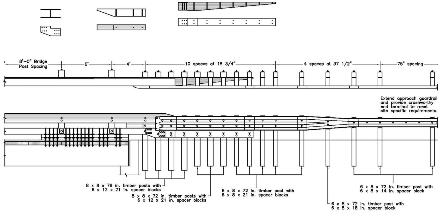
Figure K-10. Option 2.5 – Quarter-Post Spacing, 4-ft and 6-ft Gaps, No Plate, Missing Bolts, Removed Blockouts, Wood Reverse Taper, Stepped Thick Curb Taper
