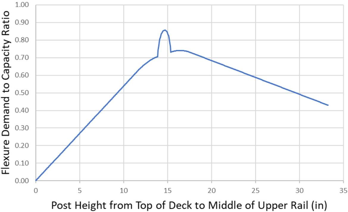
Figure 92. 10.5-in. x 8.75-in. Post Flexural Demand-Capacity Ratio Across Post Height
