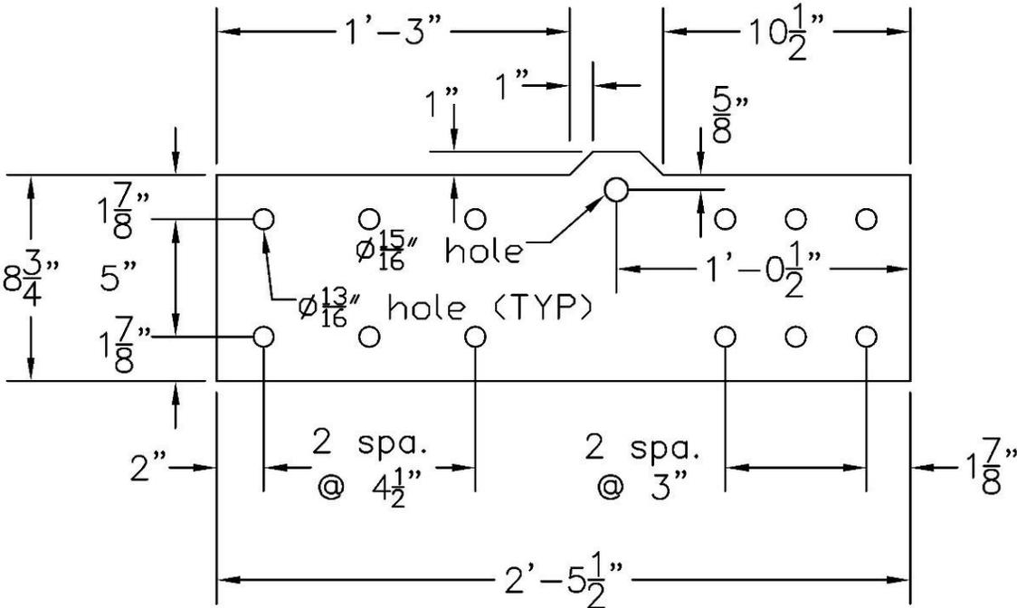
Figure 124. Curb Rail Plate Details for Both Systems
