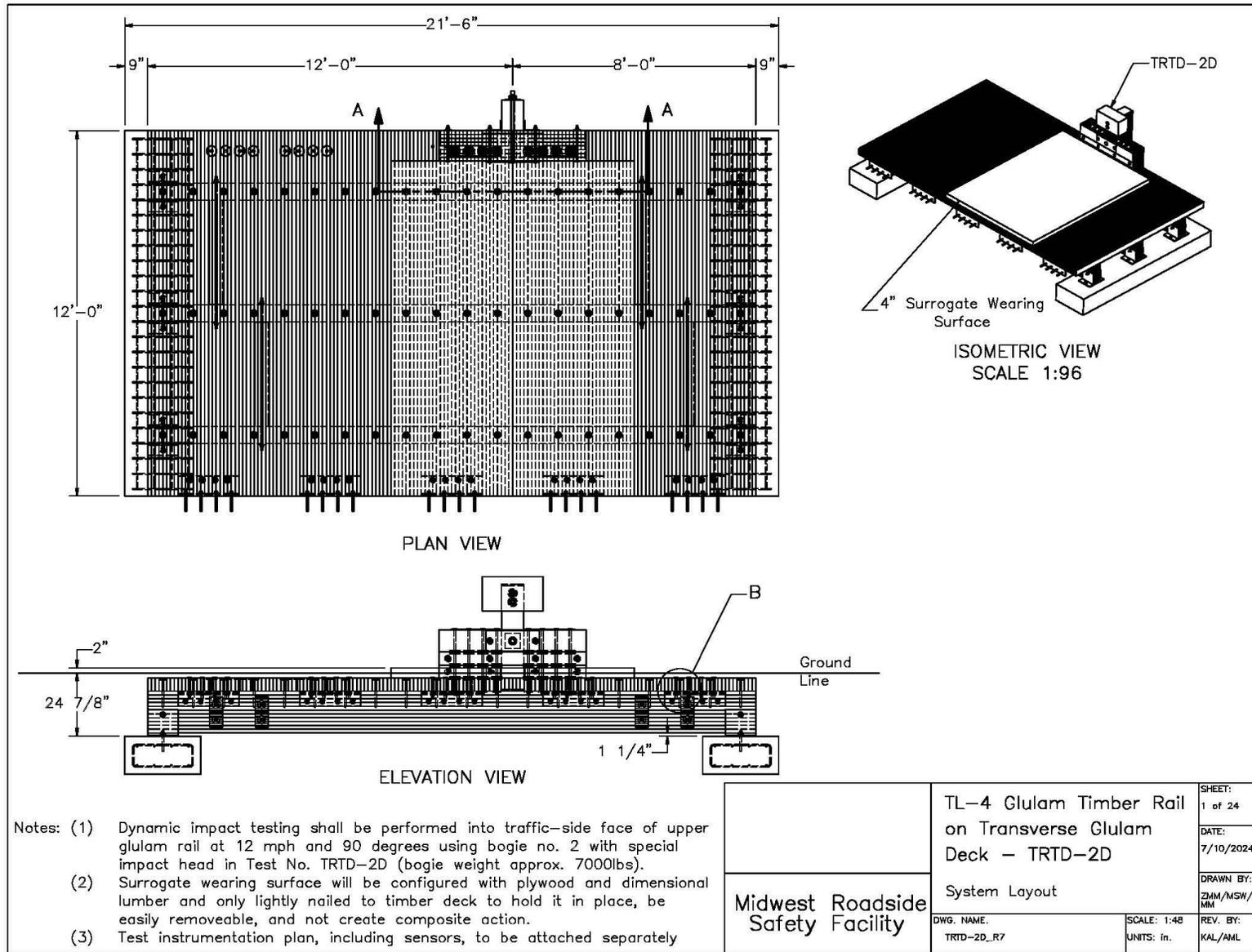
Figure 219. System Layout, Test No. TRTD-2
