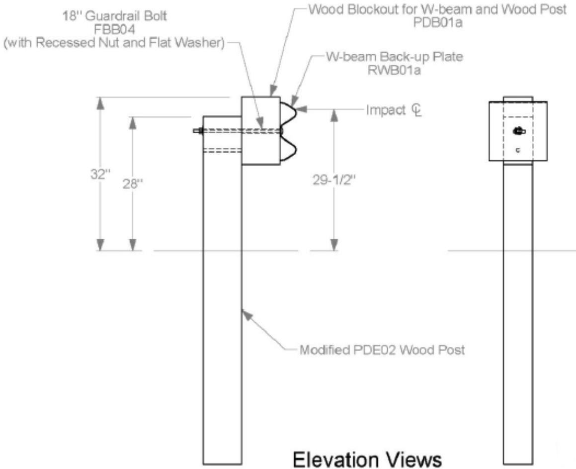
Figure 32. Test Configuration for Pendulum Impact Tests on Posts with Raised Timber Blockouts [44]
