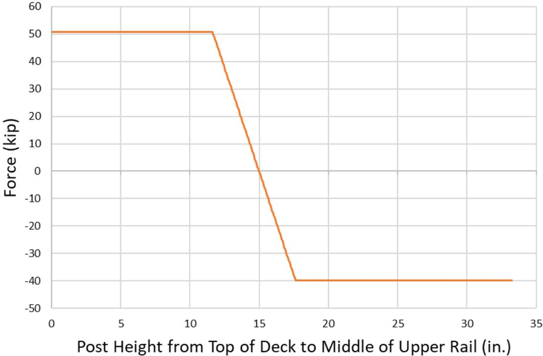
Figure 84. Lateral Shear Demand, Post Diagram
