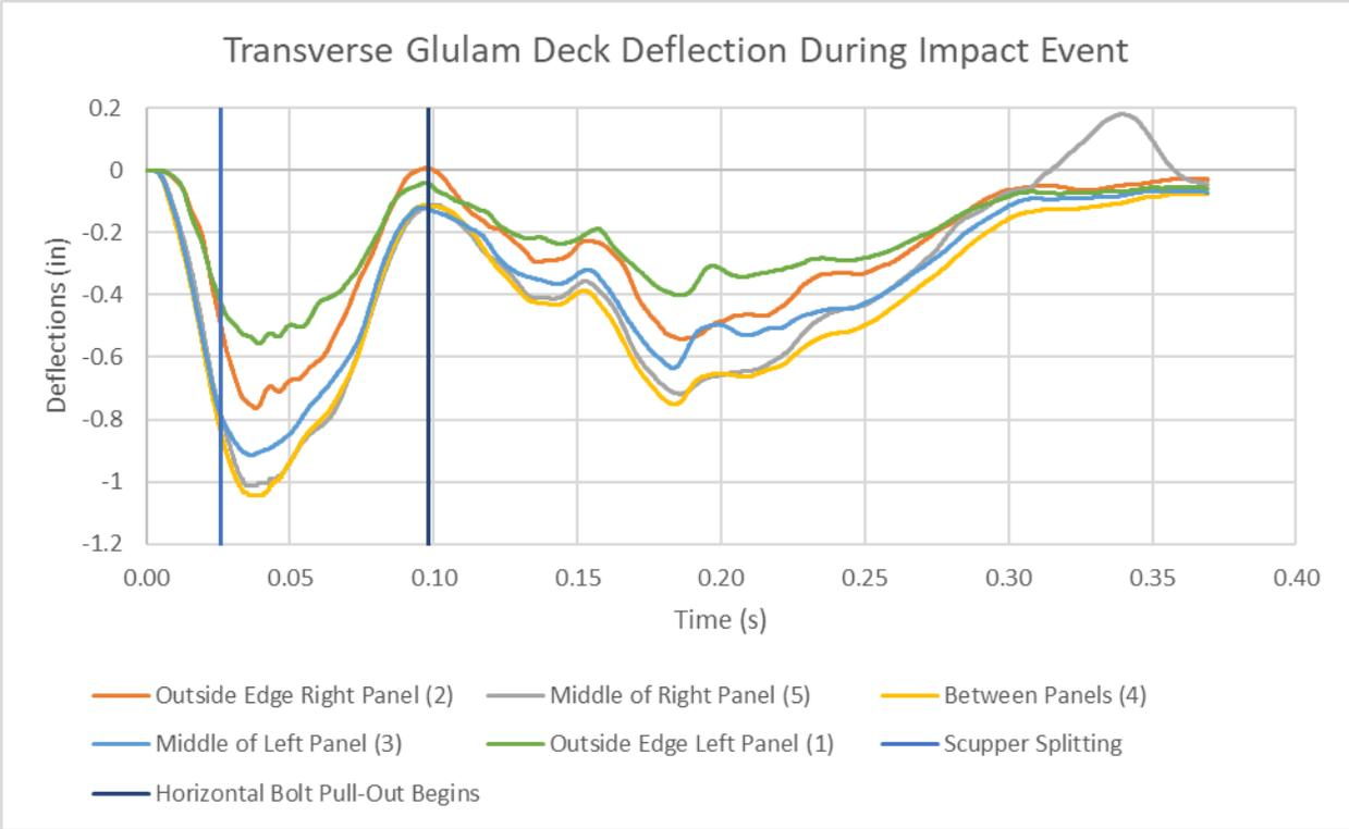
Figure 208. Test No. TRTD-1 Strain vs. Time Graph for Deck Deflections from String Potentiometers
