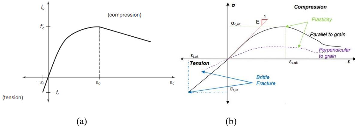
Figure 67. Typical Stress-Strain Curve for: (a) Concrete [114] and (b) Timber [115]
