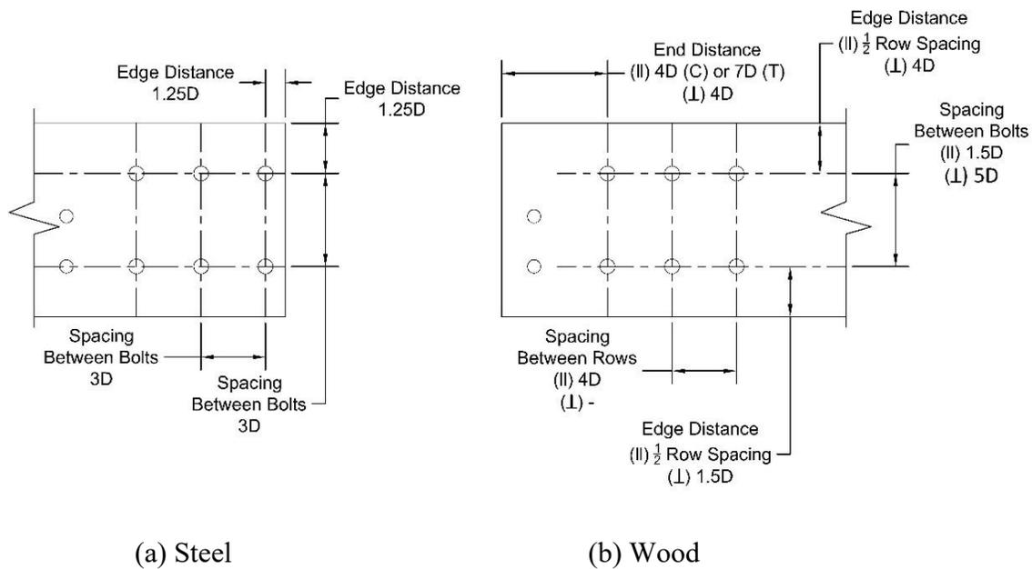
Figure 95. Bolt Spacing Requirements for (a) Steel and (b) Wood
