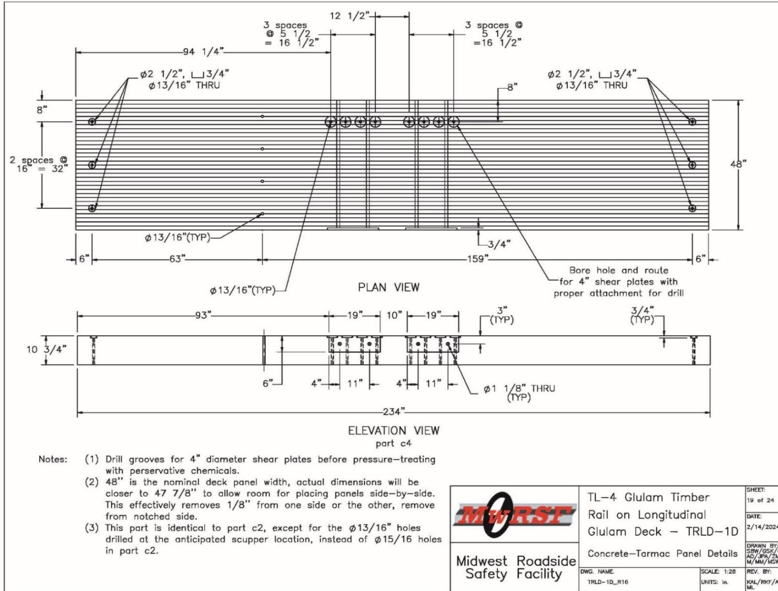
Figure 261. Deck Panel 1 Details, Test No. TRLD-1
