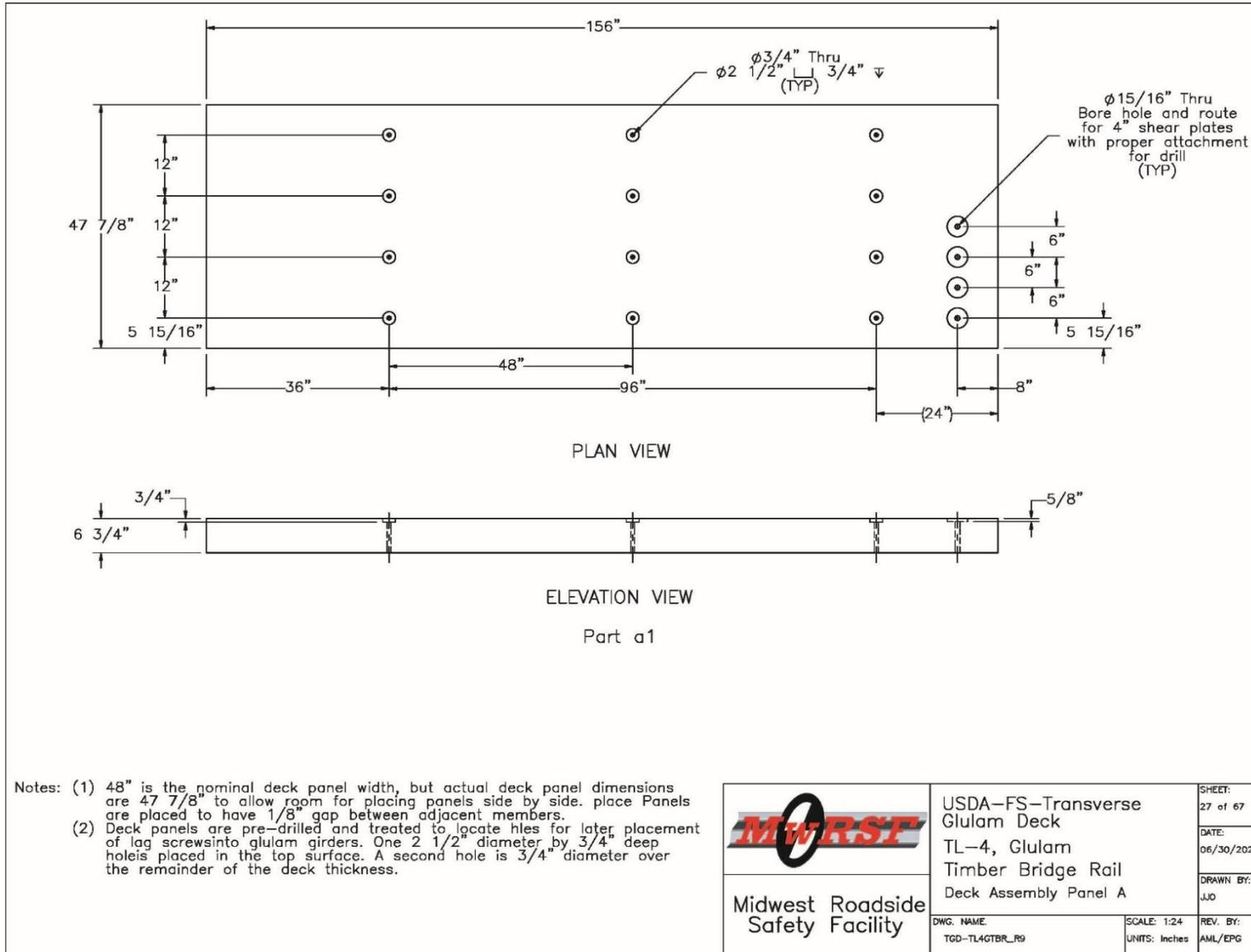
Figure O-27. Deck Assembly Panel Type A Details
