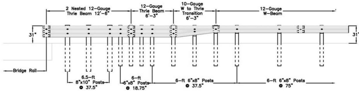
Figure 24. Proposed AGT Design Utilizing Half-Post Spacing [37]
