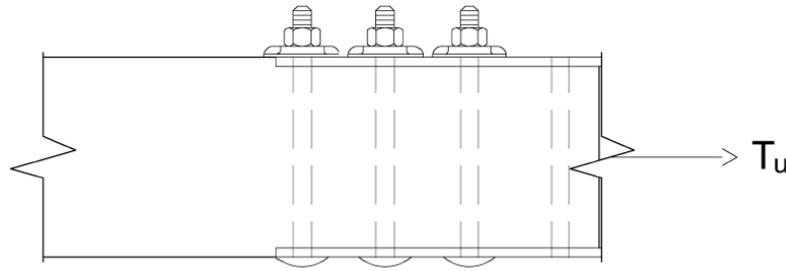
Figure 88. Upper Rail Splice Section with Tensile Demand
