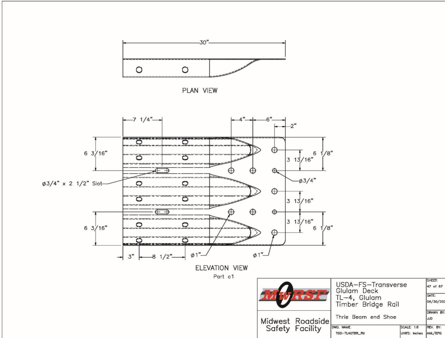
Figure O-47. Bridge AGT Thrie Beam End Shoe Details
