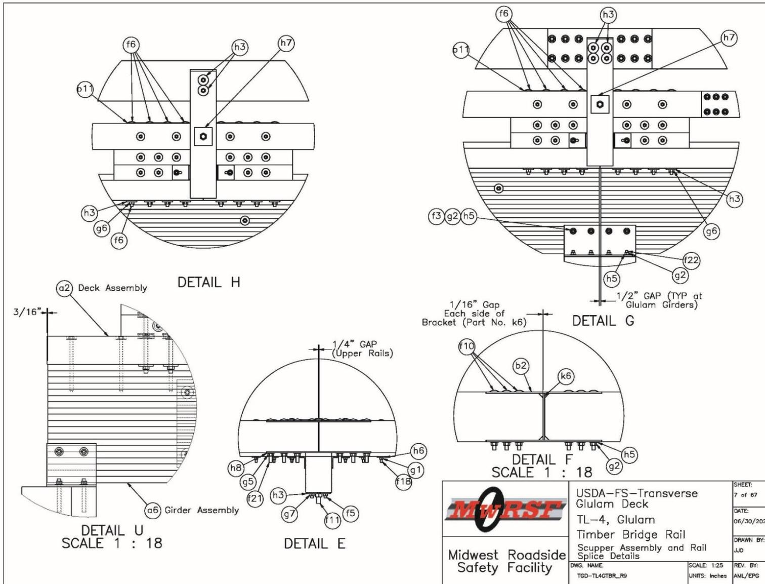
Figure O-7. System Details for Scupper and Rail Splice Assemblies
