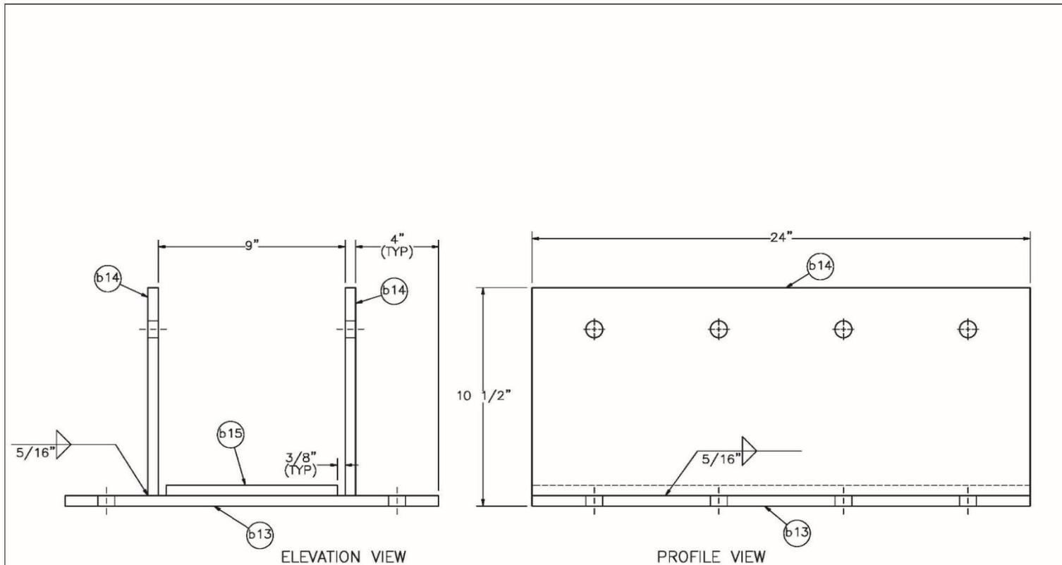
Notes: Bearing Shoe assembly shall be galvanized after side plates and base plate are welded together.
