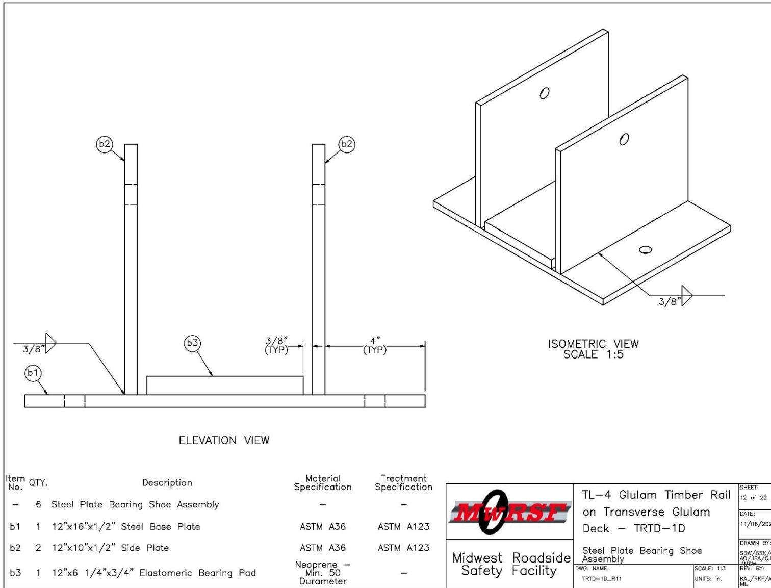
Figure 159. Steel Plate Bearing Assembly Details, Test No. TRTD-1
