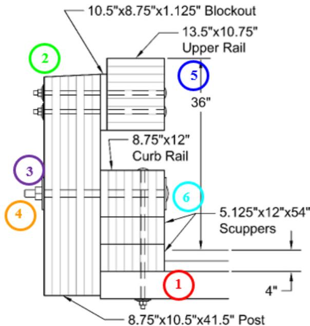
Figure 76. Phase IIa Post Configuration Connections to Design
