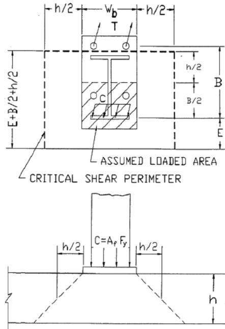
Figure 102. AASHTO Punching Shear Failure for Concrete Decks [15]
