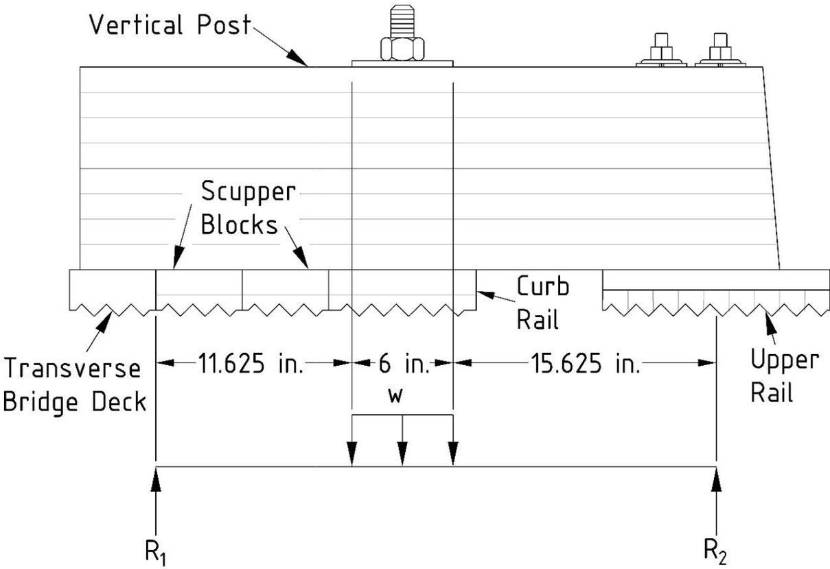
Figure 82. Free-Body-Diagram for Post Flexure from Lateral Loads
