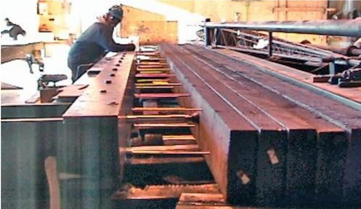
Figure 43. Spikes Being Driven Through Lumber for Spike-Laminated Deck Panel [63]
