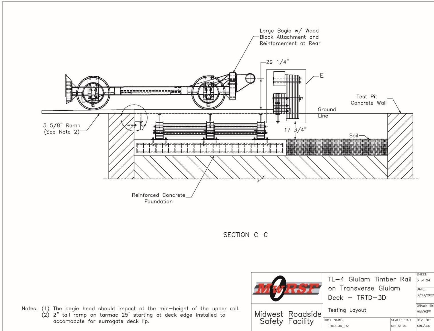
Figure N-5. Test No. TRTD-3 Layout, Elevation View
