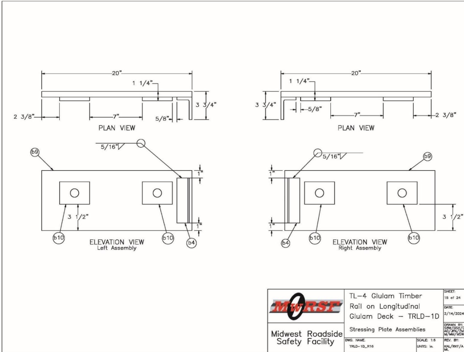
Figure 257. Stressing Plate Assembly Details, Test No. TRLD-1
