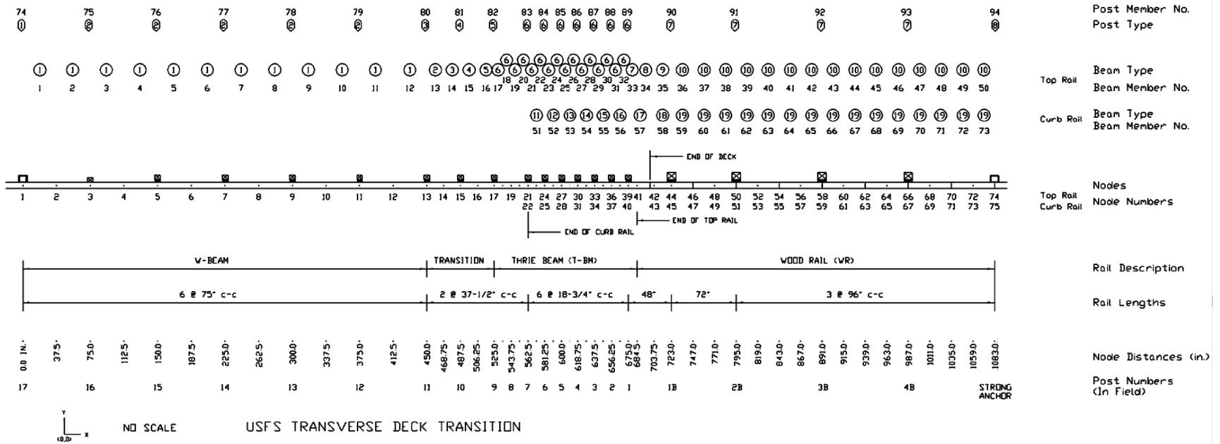
Figure 108. BARRIER VII Model Developed for Design of AGT Connection Glulam Timber Bridge Railing with Curb Rail and Strong W-Beam Guardrail [25]
