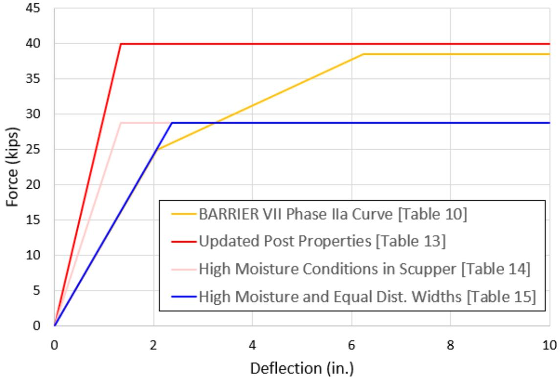
Figure 74. Adjusted Surrogate TL-4 Post Force-Deflection Curves for High Moisture and Equal Distribution Widths
