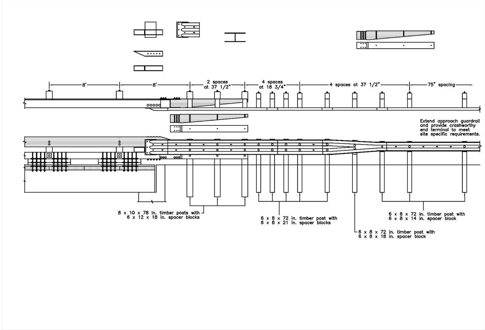
Figure K-30. Option 5.4 – Half-Post Spacing, 8-ft Gap, Welded End Shoe, Steel Reverse Taper, Curb Taper Behind Thrie-beam
