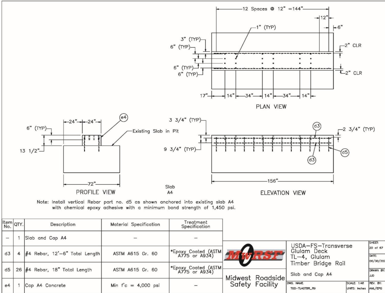
Figure O-20. Bridge Substructure Intermittent Pier A4 Details
