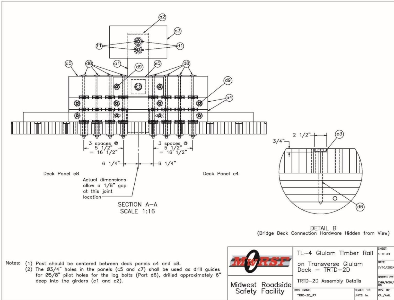
Figure 222. Post and Deck Assembly Details, Test No. TRTD-2
