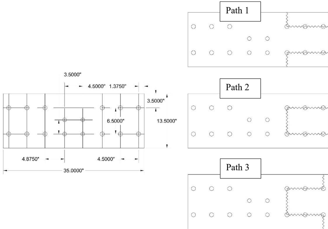
Figure J-1. Upper Rail Splice Block Shear Failure Paths
