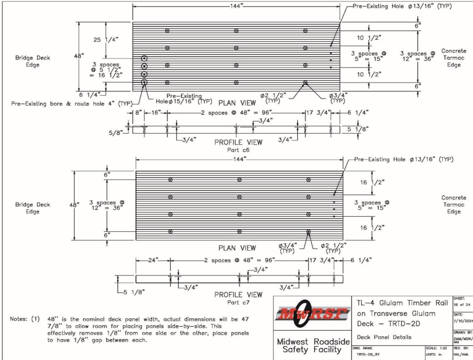
Figure 236. Deck Panel Details, Page 2, Test No. TRTD-2
