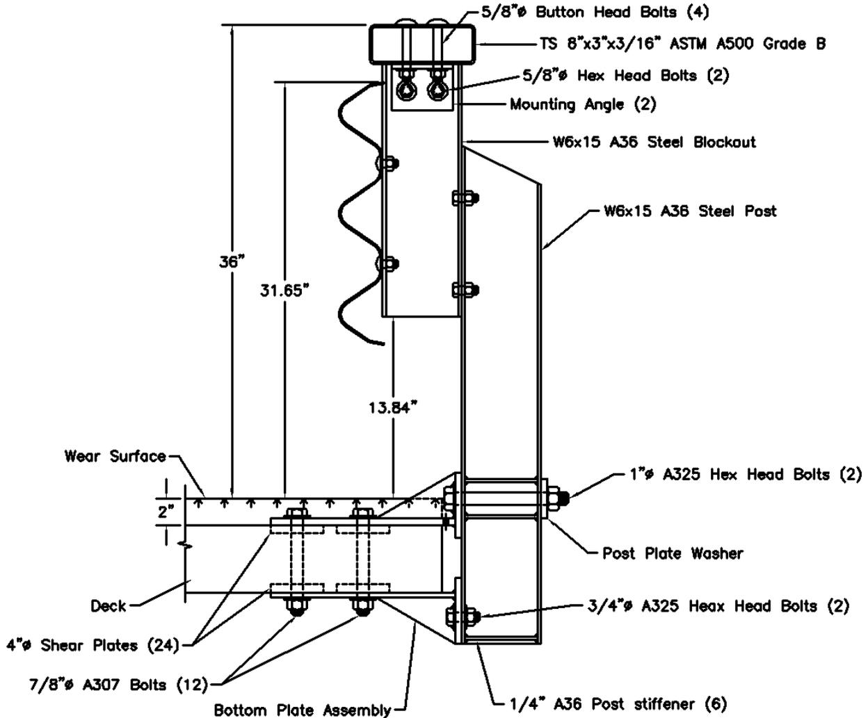
Figure 9. Steel Thrie-Beam Railing for NCHRP-350 TL-4 on Transverse Glulam Deck [25]
