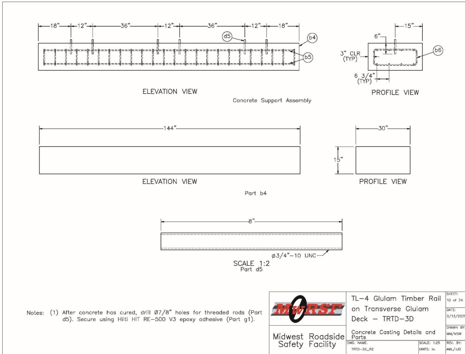
Figure N-10. Test No. TRTD-3 Concrete Casting and Embedded Rod Details
