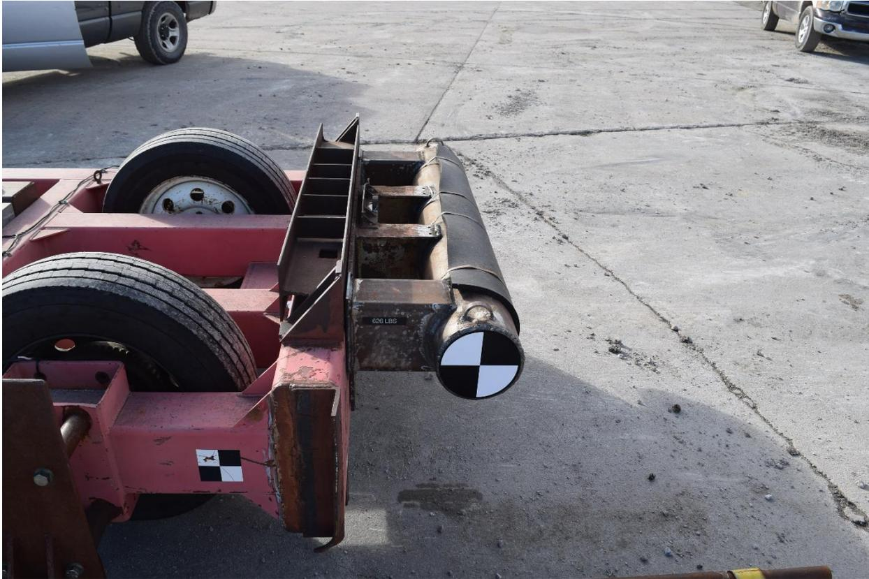
Figure 131. Bogie Impact Head, Test Nos. TRAGT-2 and TRAGT-3
