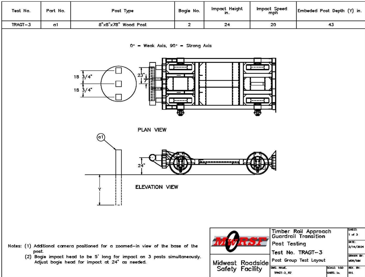
Figure 128. Test Layout, Impact on Single Post, Test No. TRAGT-3
