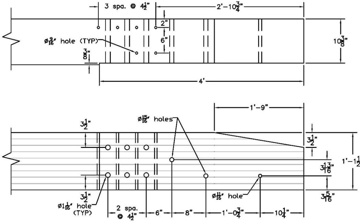
Figure 115. Cuts and Holes Needed in Upper Rail at End for Attachment to Half-Post System
