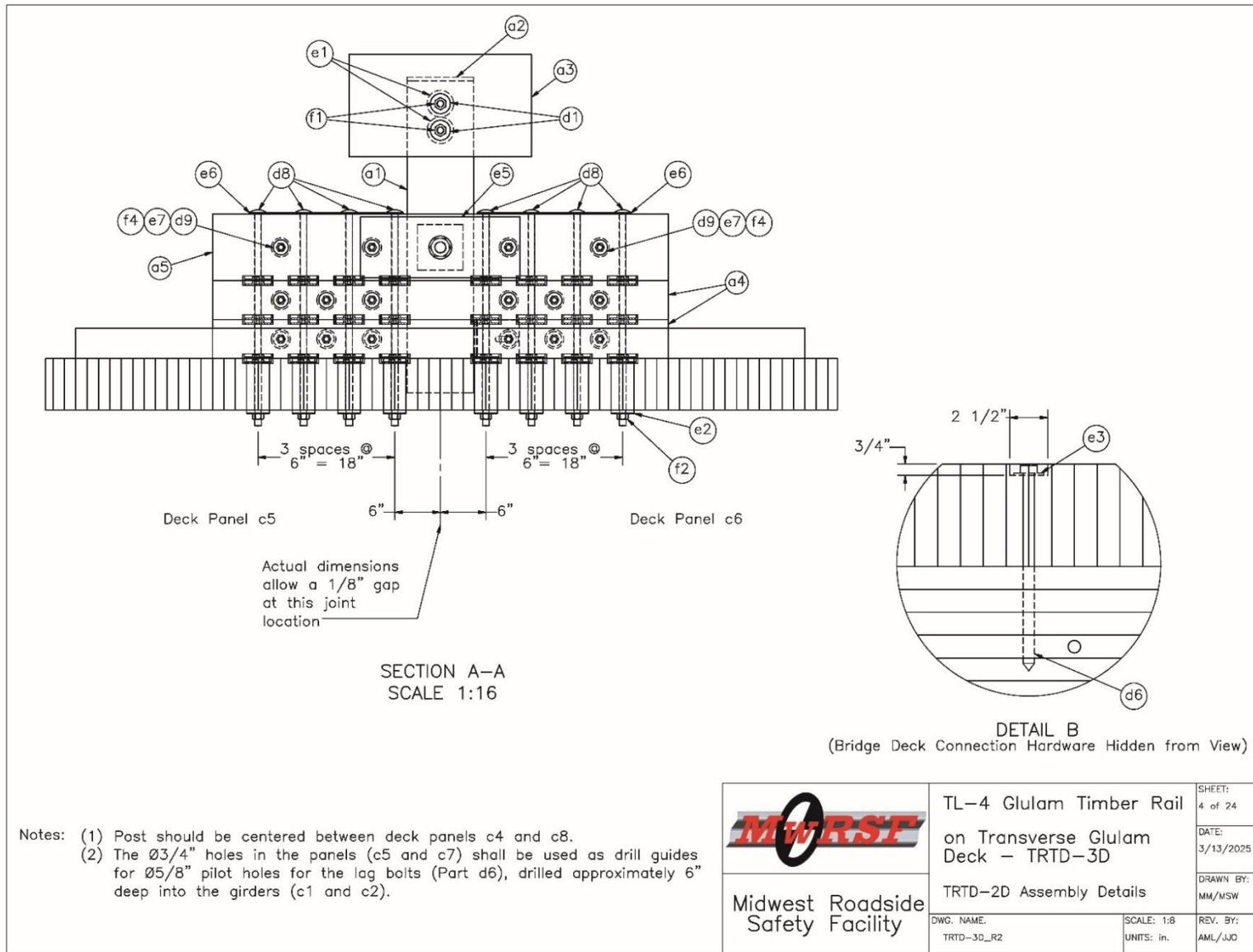
Figure N-4. Test No. TRTD-3 Post and Deck Assembly Details
