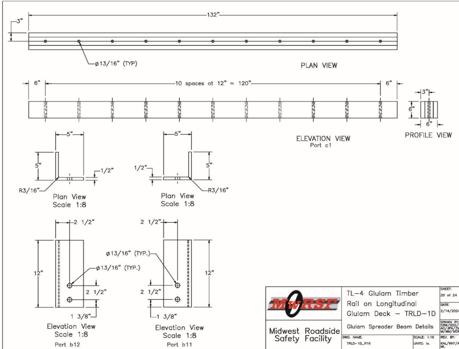
Figure 262. Spreader Beam and Deck Panel Edge Hardware Details, Test No. TRLD-1
