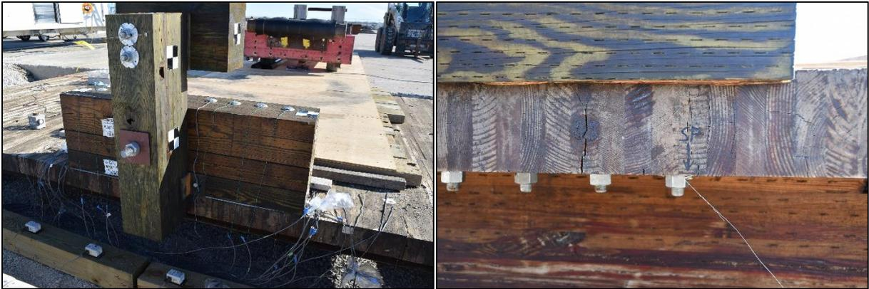
Figure 209. South Deck Panel Laminations Before (left) and After (right) Test
