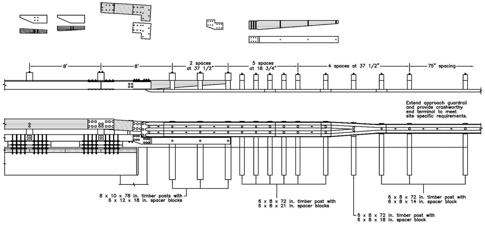
Figure K-31. Option 5.5 – Half-Post Spacing, 8-ft Gap, Rotated Custom Glulam Piece, Wood Reverse Taper, Stepped Curb Taper
