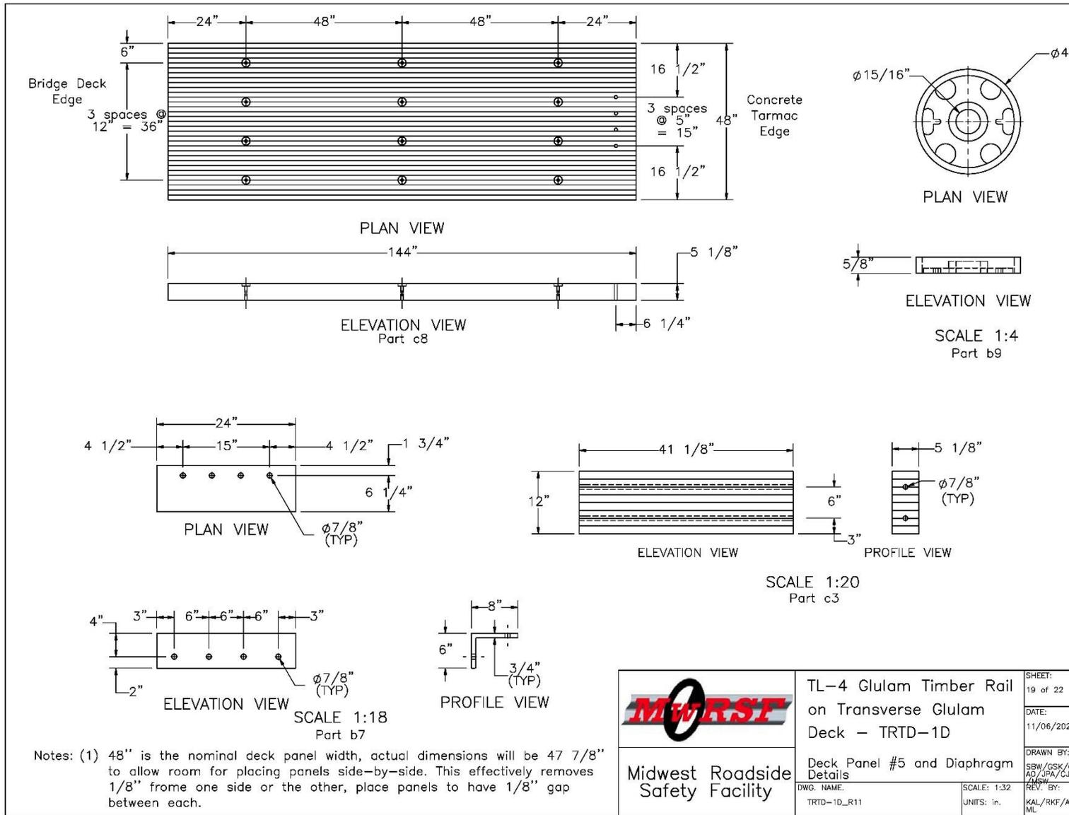
Figure 166. Deck Panel, Tarmac Angle Restraint, Diaphragm, and Shear Plate Details, Test No. TRTD-1
