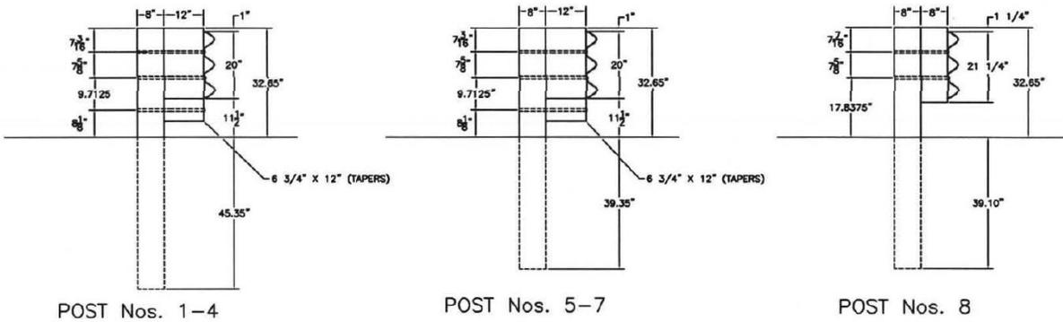
Figure 17. Cross-Section View of AGT Posts Closest to Bridge Railing [25]
