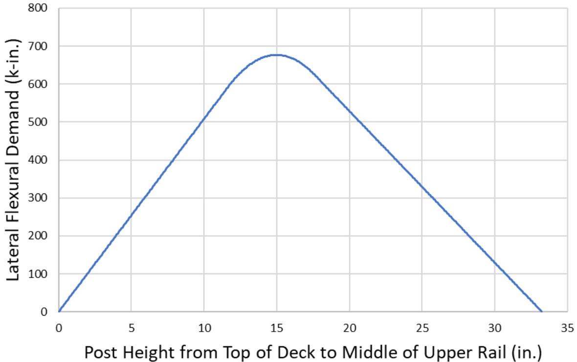
Figure 87. Lateral Flexural Demand, Post Diagram
