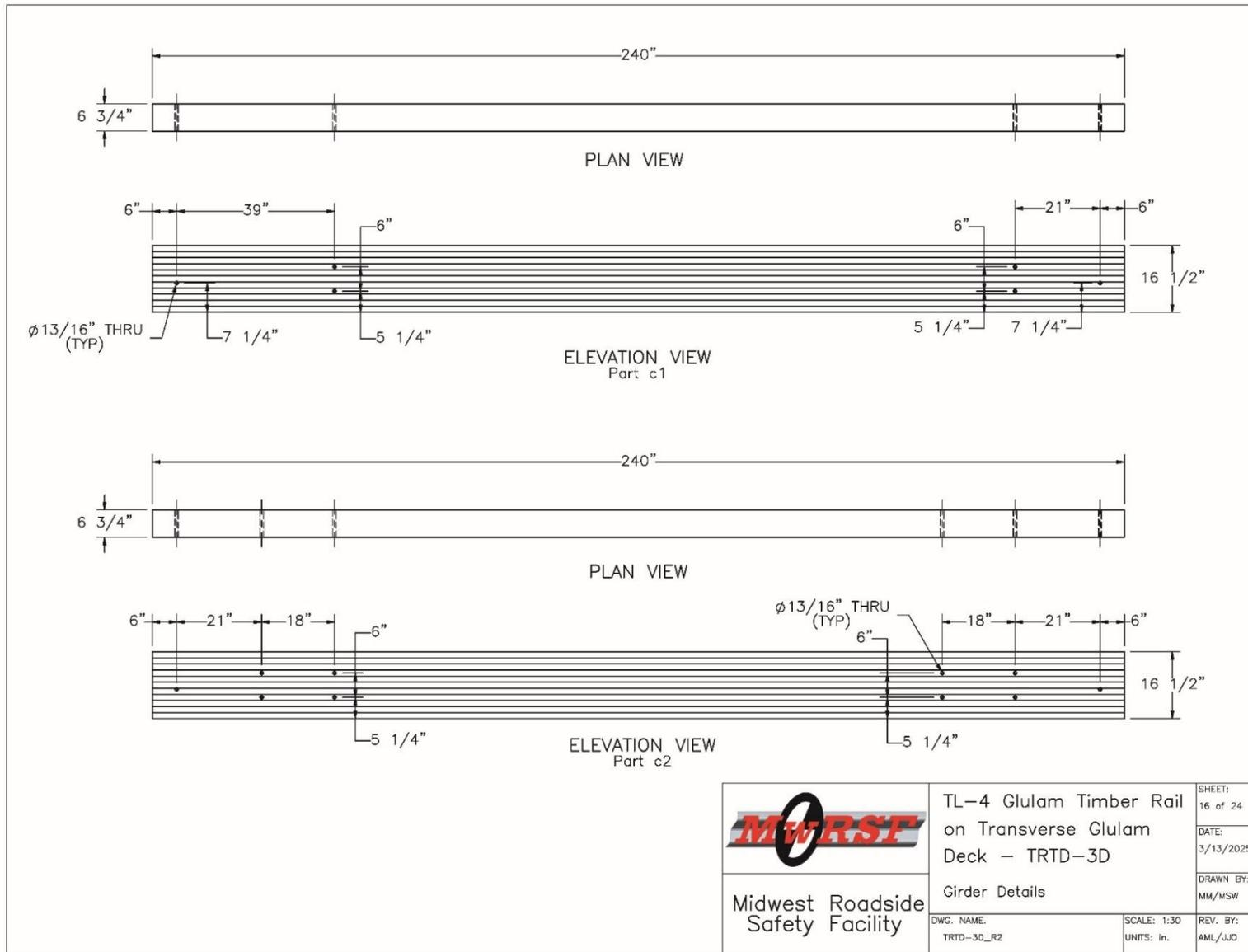
Figure N-16. Test No. TRTD-3 Girder Details
