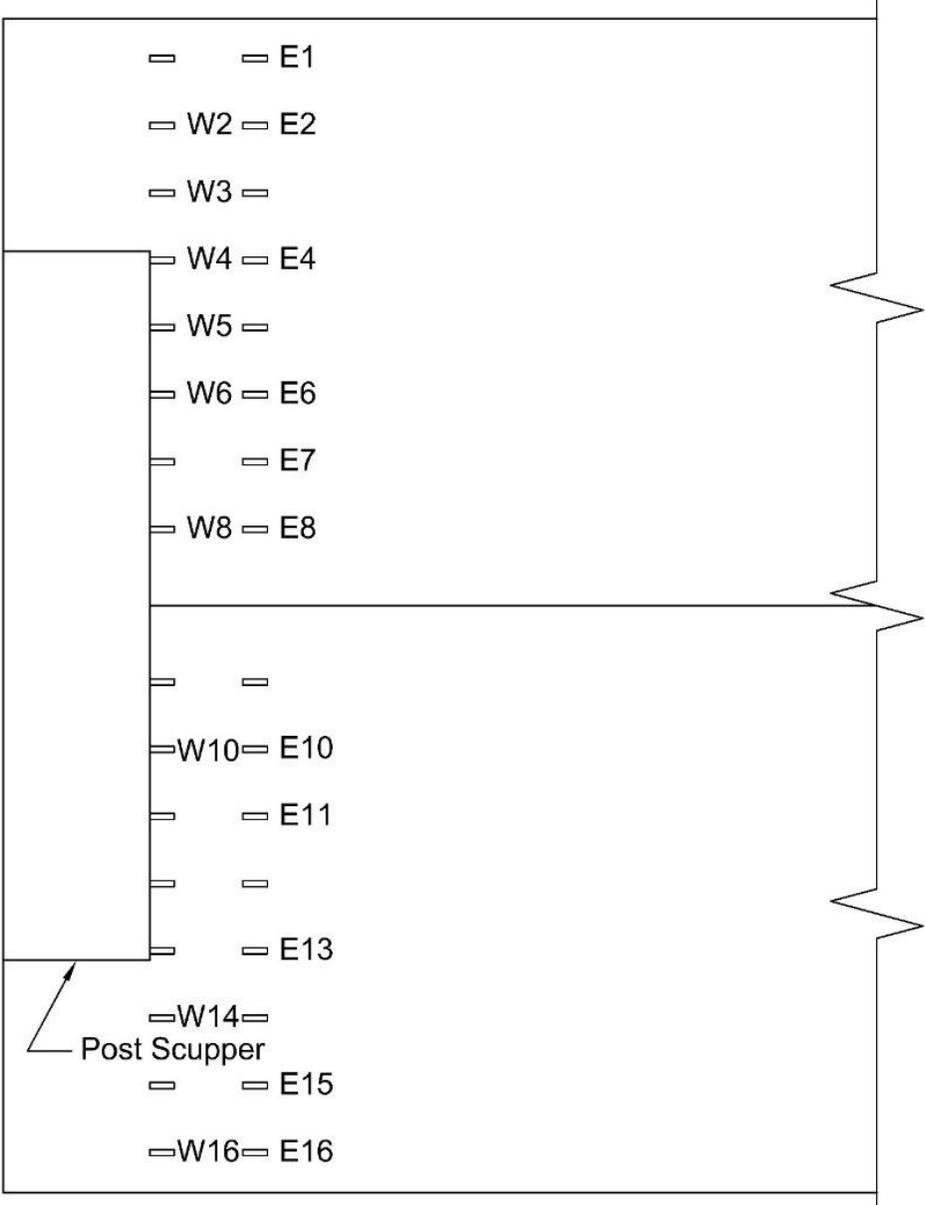
Figure 202. Deck Surface Strain Gauge Locations
