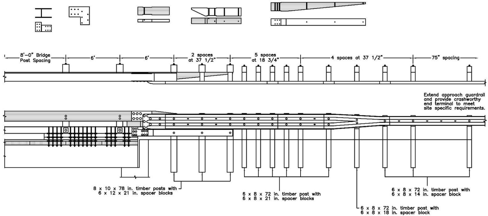
Figure K-20. Option 3.5 – Half-Post Spacing, 6-ft Gap, L-Plate, Removed Blockout, Wood Reverse Taper, Stepped Curb Taper
