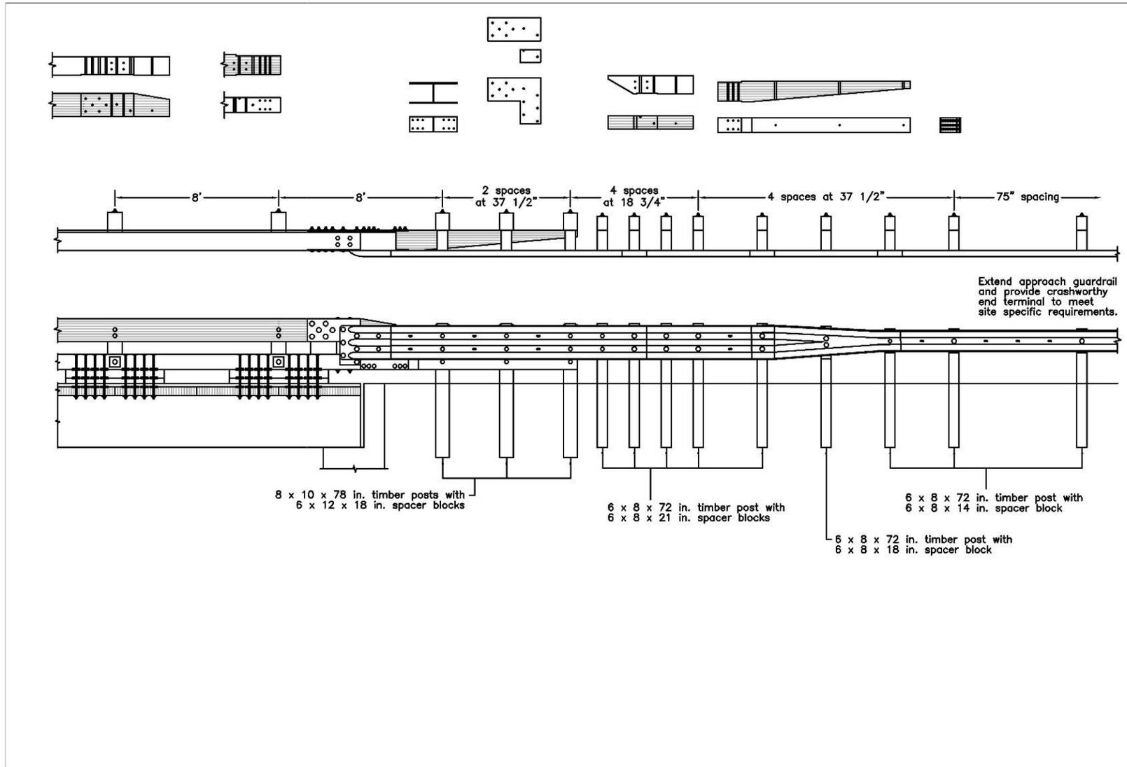
Figure K-24. Option 4.1 – Half-Post Spacing, 8-ft Gap, L-Plate, Wood Reverse Taper, Curb Taper Behind Thrie-beam
