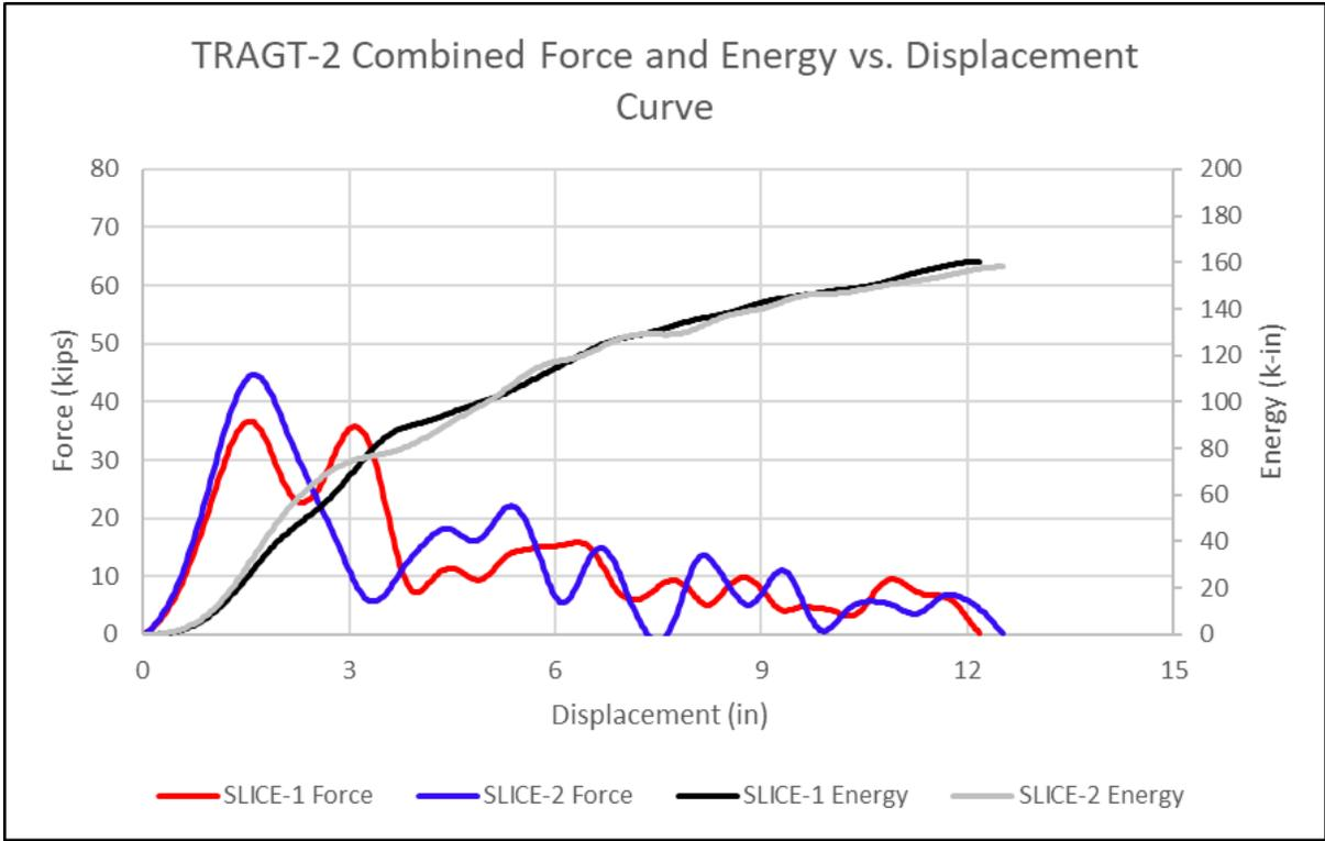
Figure 139. Combined Force and Energy vs. Displacement Curve, Test No. TRAGT-2
