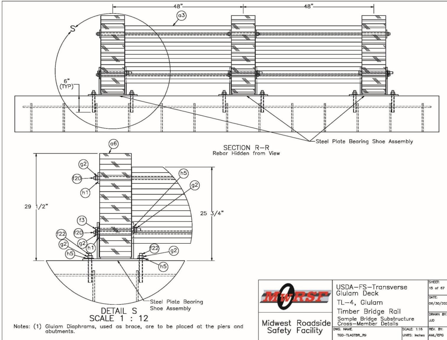
Figure O-15. Bridge Superstructure and Bearing Connection Details
