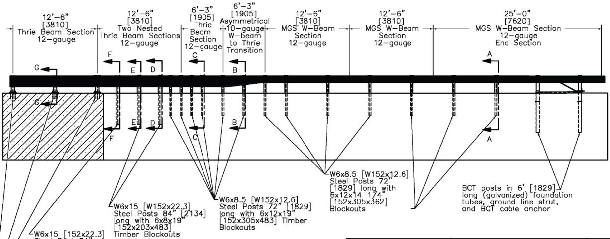
Figure 20. Elevation View of AGT Built with Two Standard Post Sizes [36]
