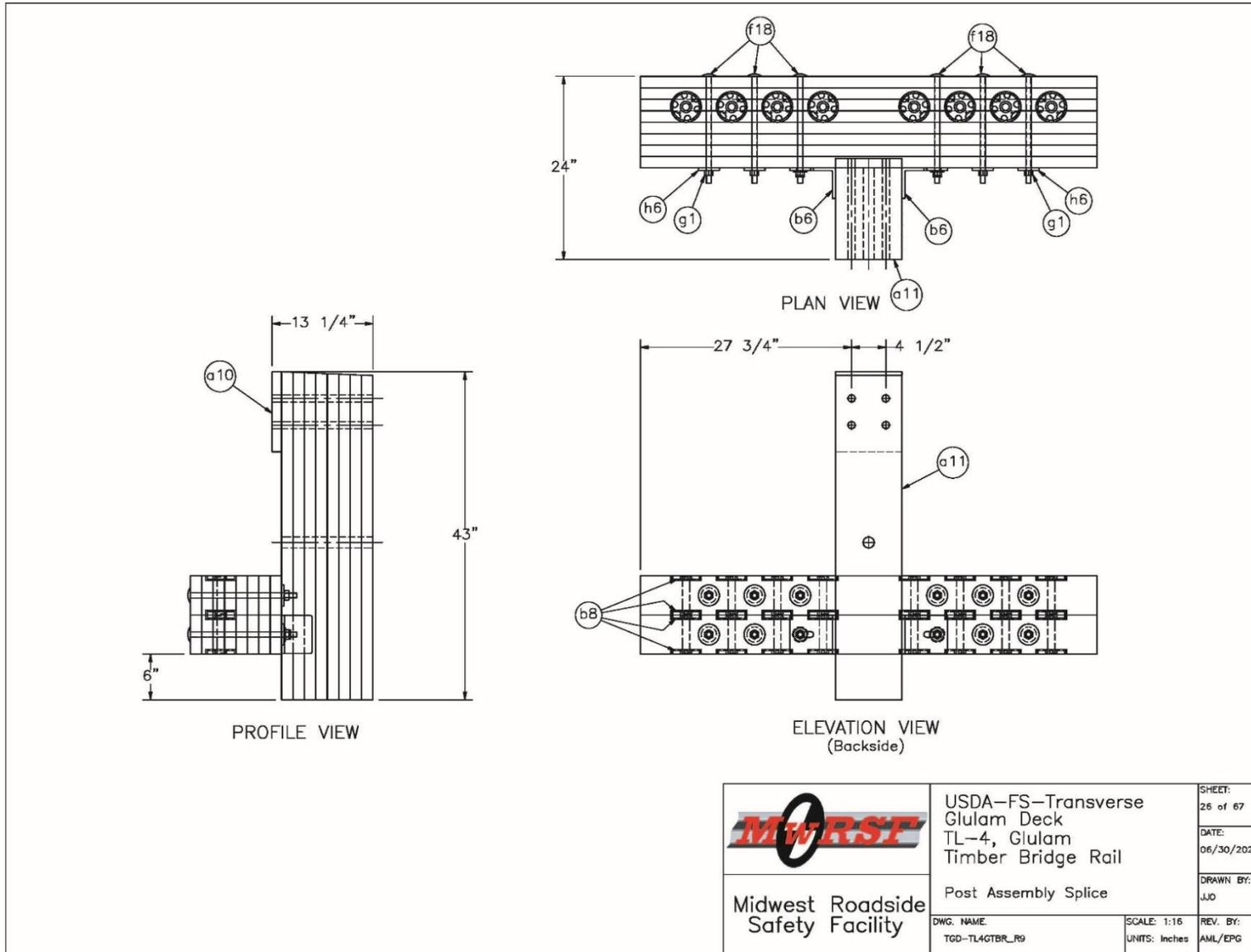
Figure O-26. Bridge Splice Post Assembly Details
