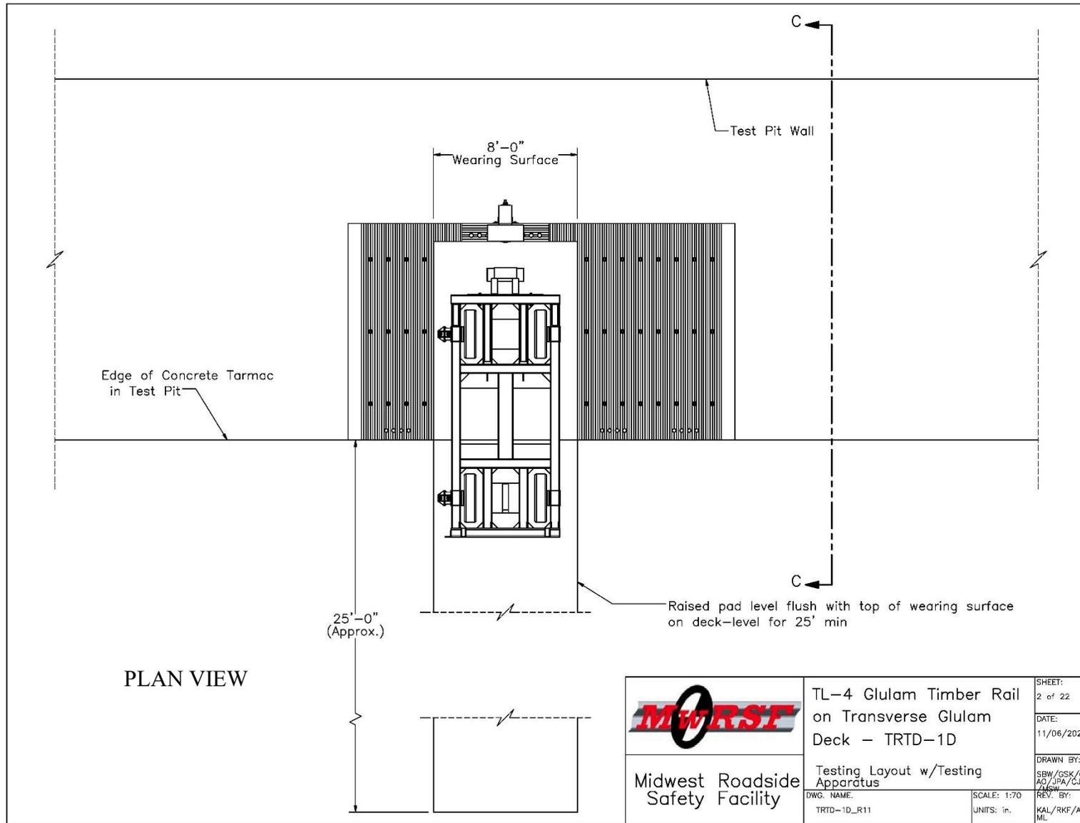
Figure 149. Layout with Bogie, Test No. TRTD-1
