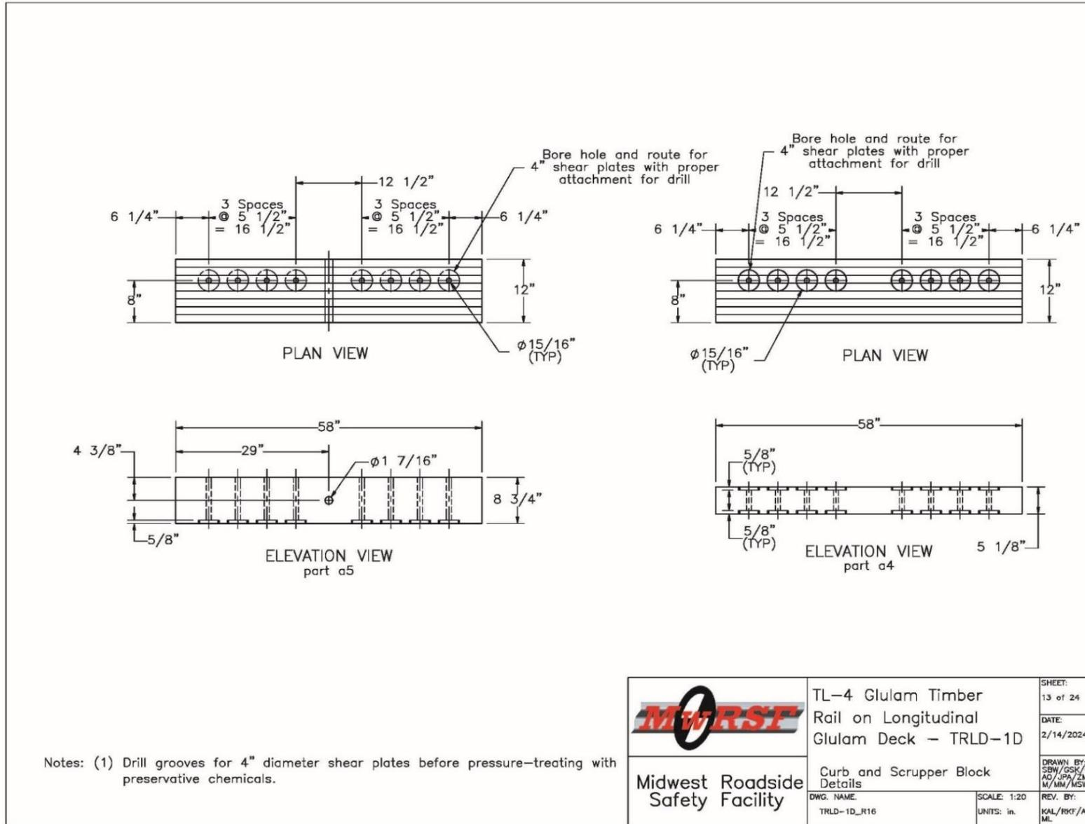
Figure 255. Scupper and Curb Rail Details, Test No. TRLD-1
