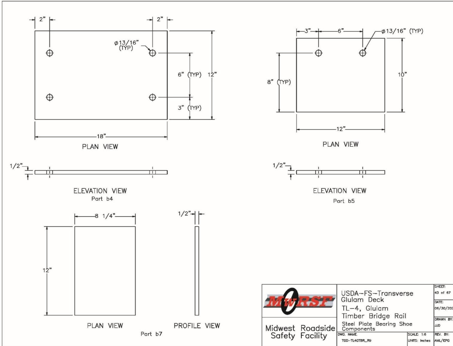
Figure O-43. Bridge Superstructure Abutment Bearing Component Details
