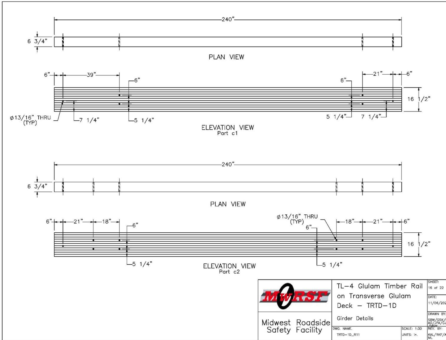
Figure 163. Girder Details, Test No. TRTD-1
