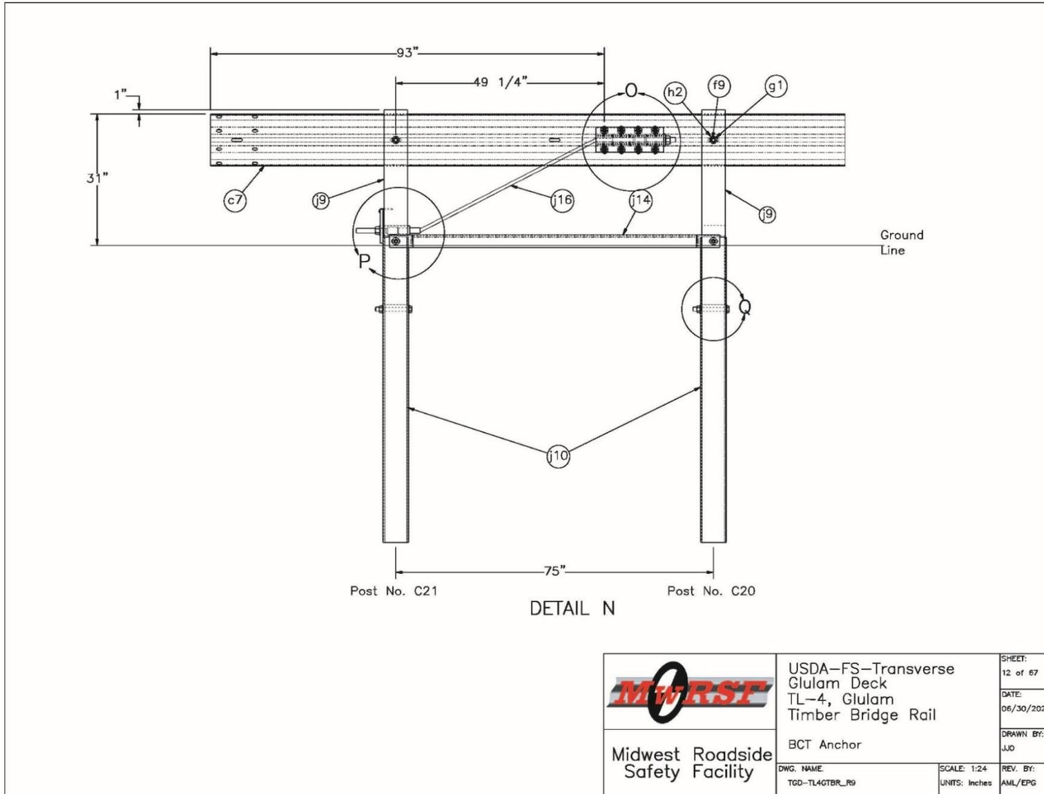
Figure O-12. AGT BCT End Anchor Elevation View
