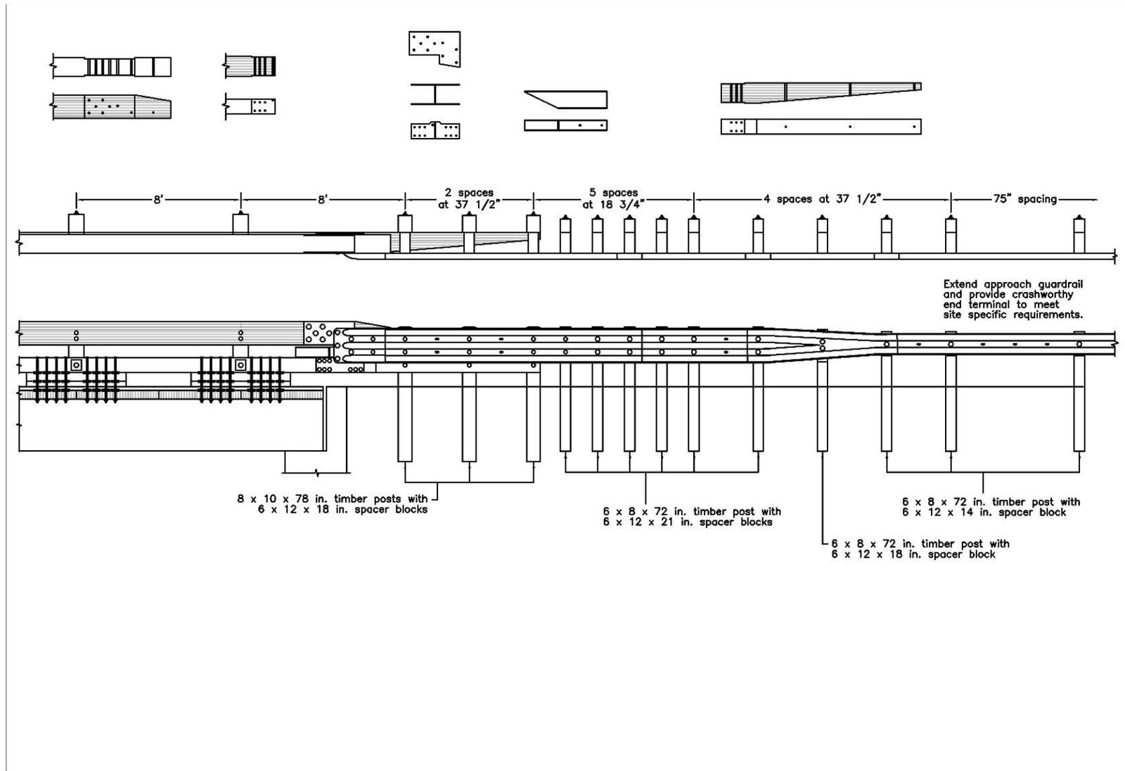
Figure K-35. Option 6.4 – Half-Post Spacing, 8-ft Gap, L-Plate, Steel Reverse Taper, Curb Taper Behind Thrie-beam
