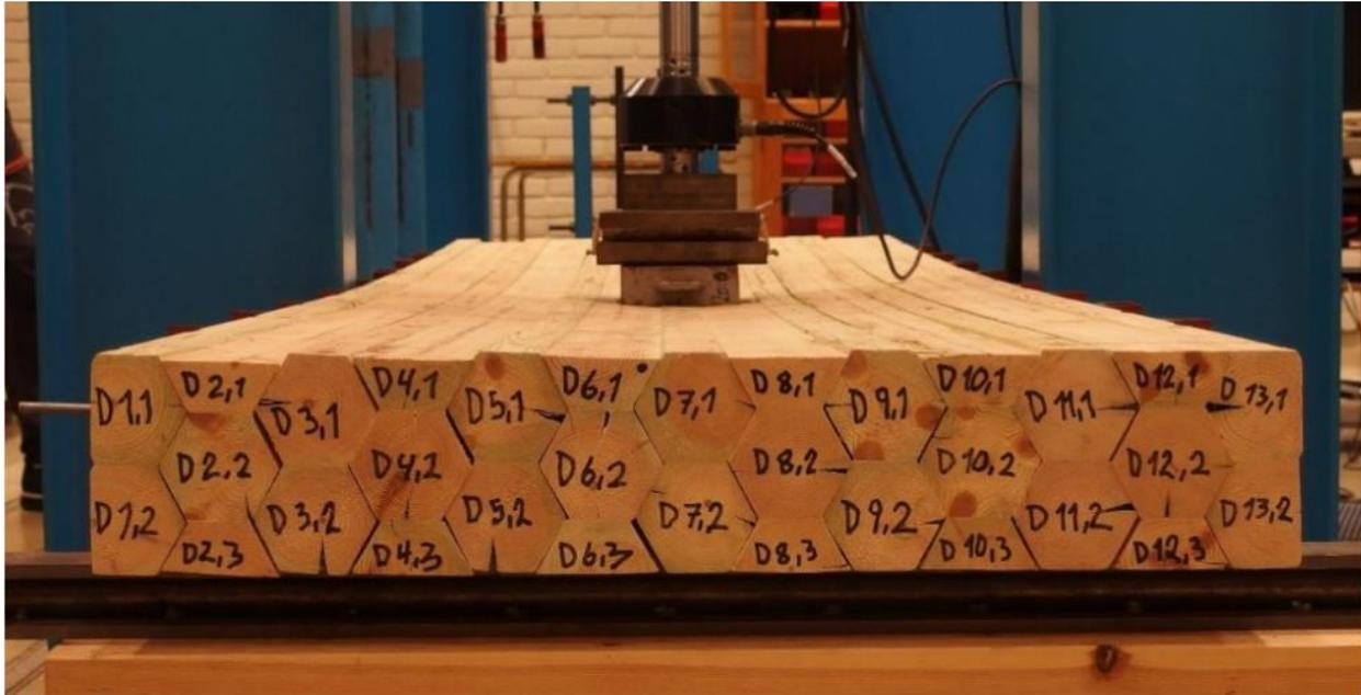
Figure 51. Testing of Oblique Interlocked Laminated Timber Deck [79]
