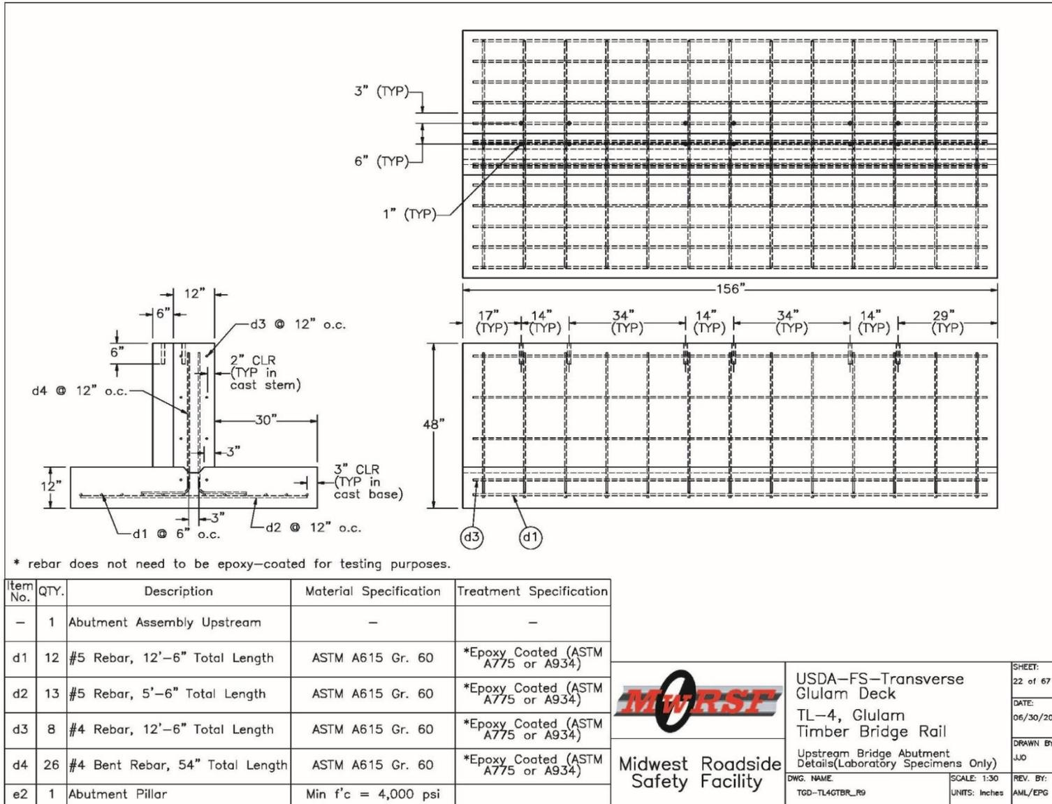
Figure O-22. Bridge Substructure South Abutment Details
