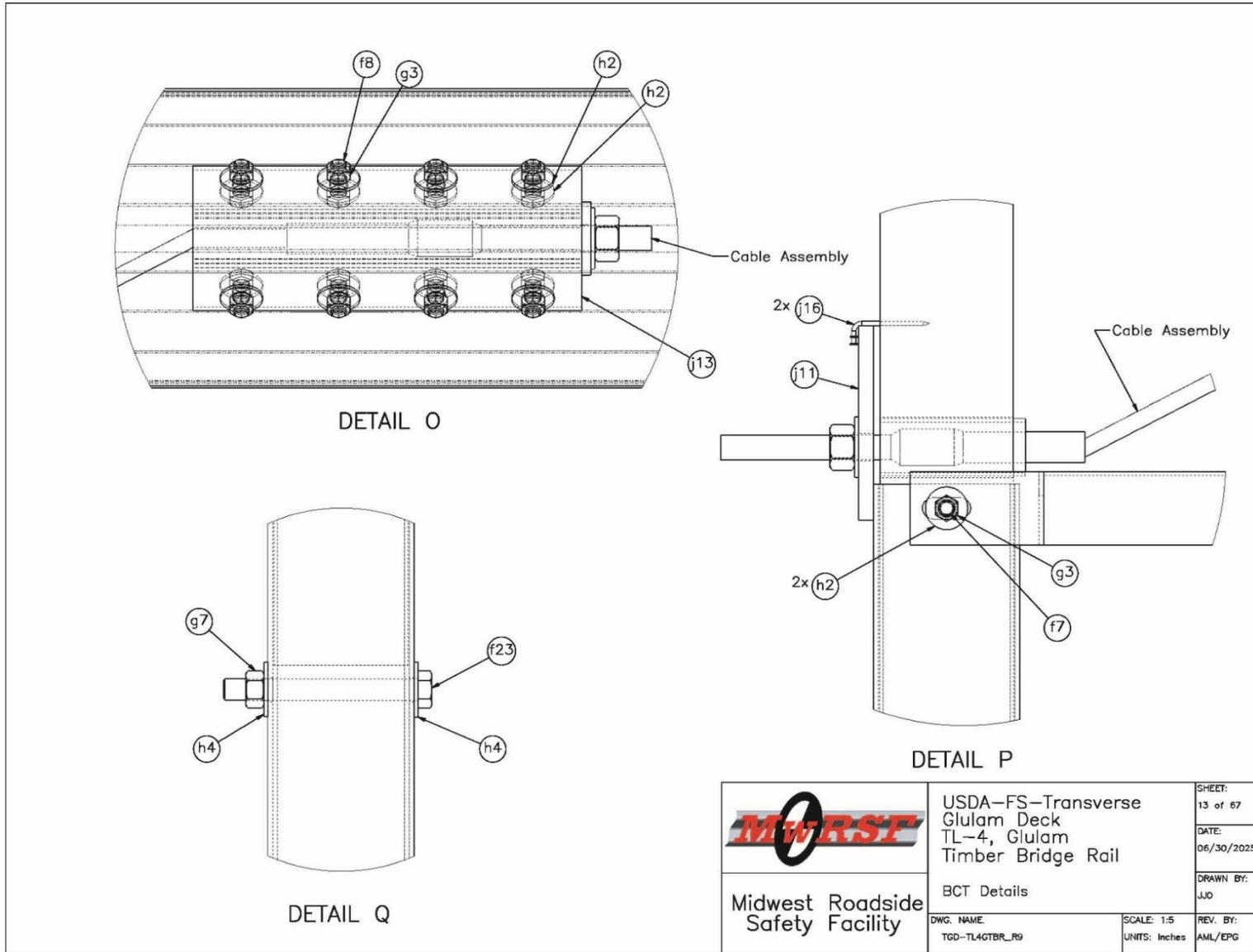
Figure O-13. AGT BCT End Anchor Component Details
