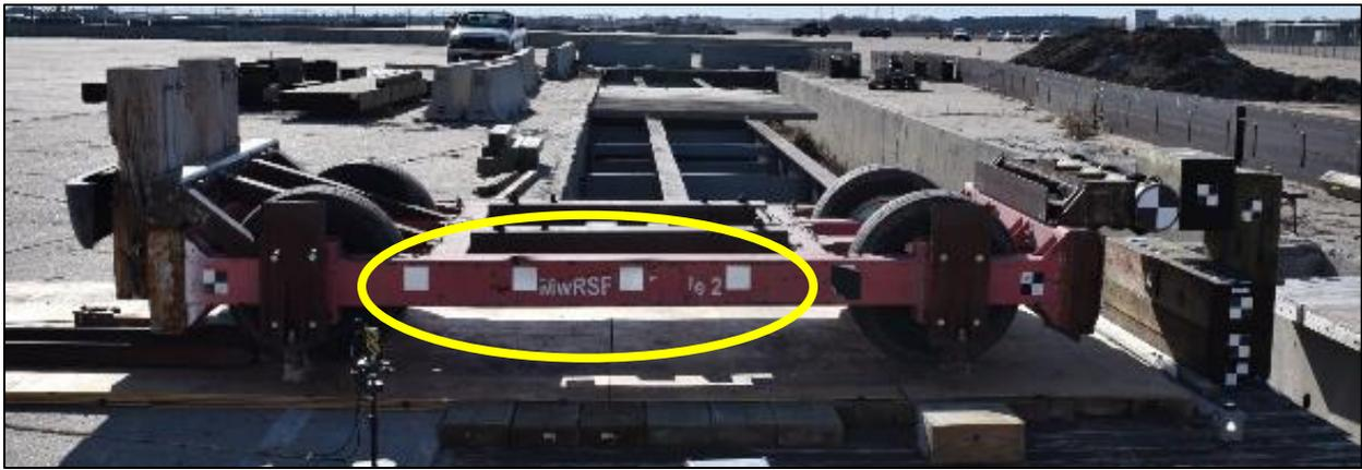
Figure 180. Retroreflective Optic Tape on Side of Bogie Vehicle
