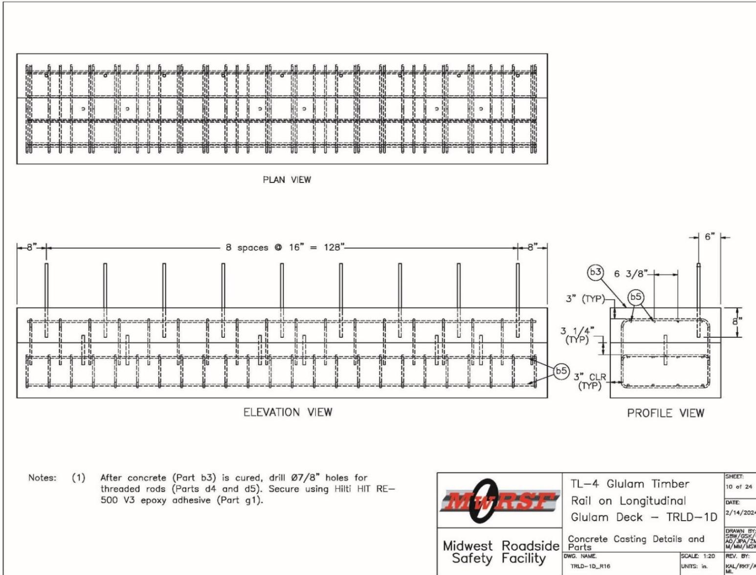
Figure 252. Rebar Layout with Embedded Rods, Test No. TRLD-1
