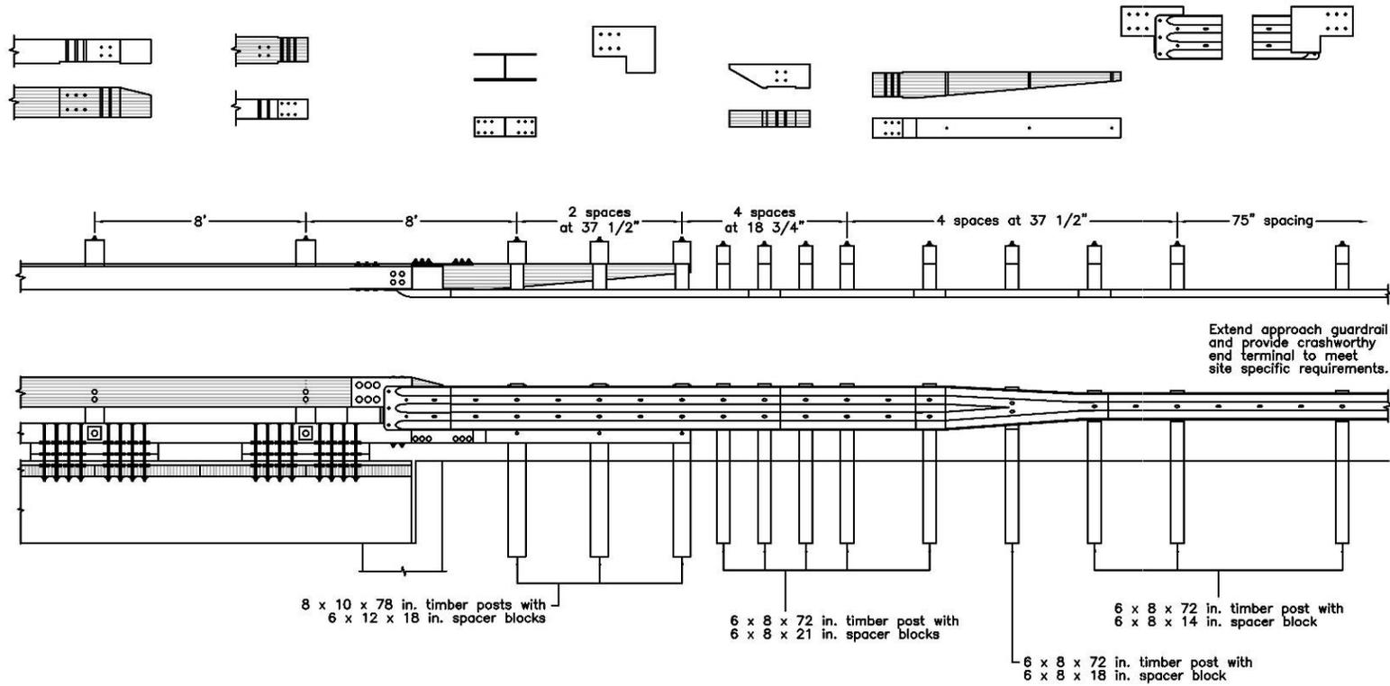
Figure K-42. Option 7.5 – Half-Post Spacing, 8-ft Gap, Welded L-Plate to End Shoe, Wood Reverse Taper, Curb Taper Behind Thrie-beam
