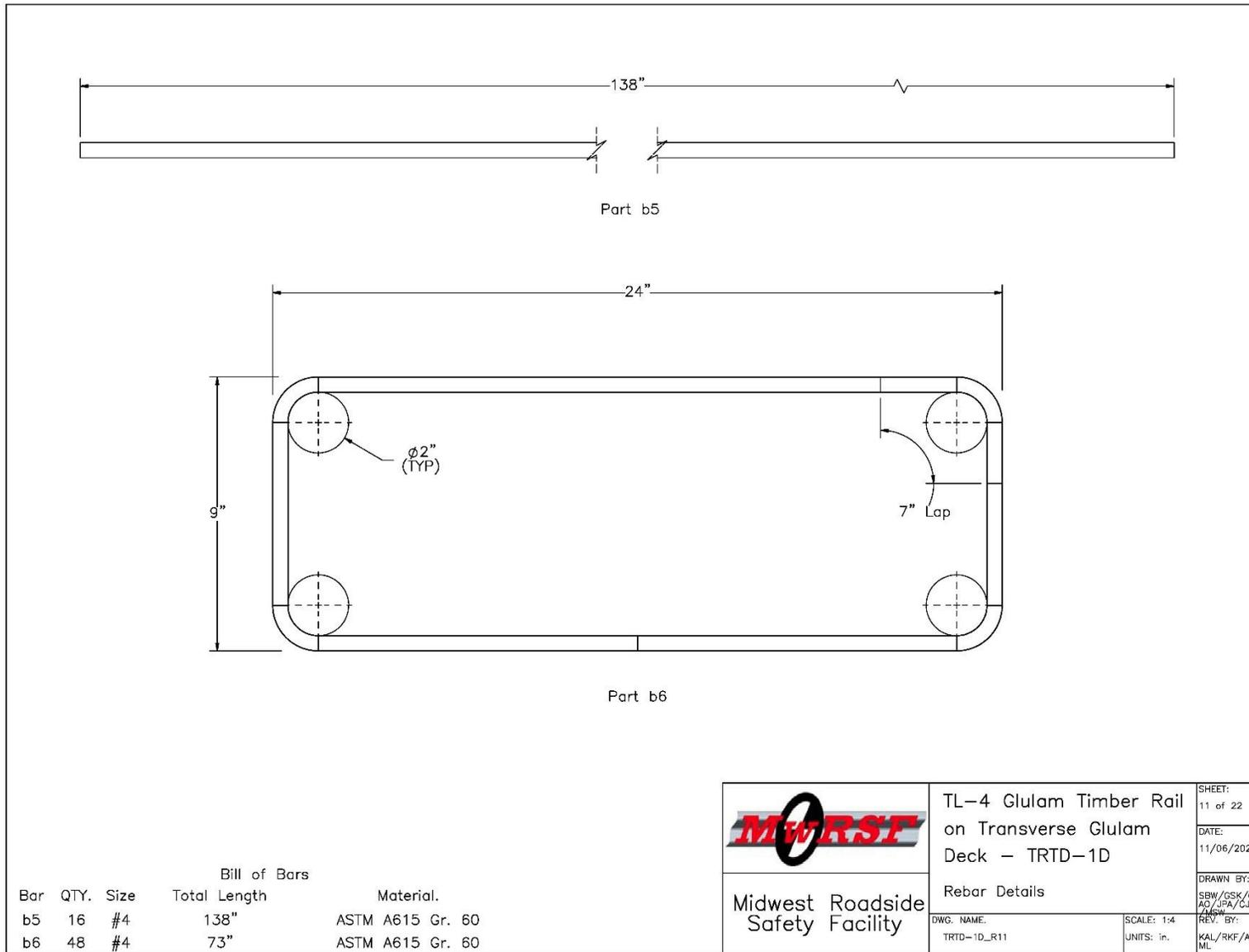
Figure 158. Rebar Details, Test No. TRTD-1
