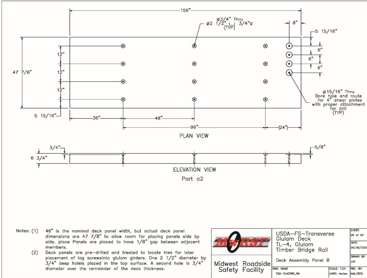
Figure O-28. Deck Assembly Panel Type B Details
