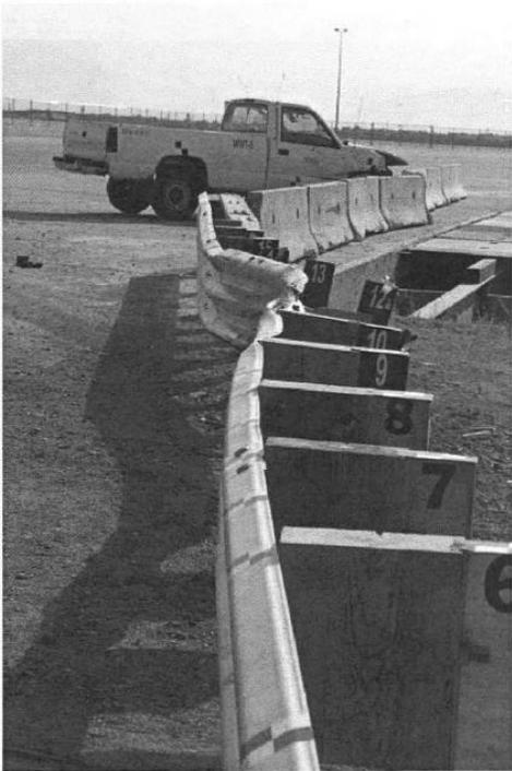
Figure 19. Post-Test Photograph of Successful Crash-Test MWT-5 on Upstream Transition [35]
