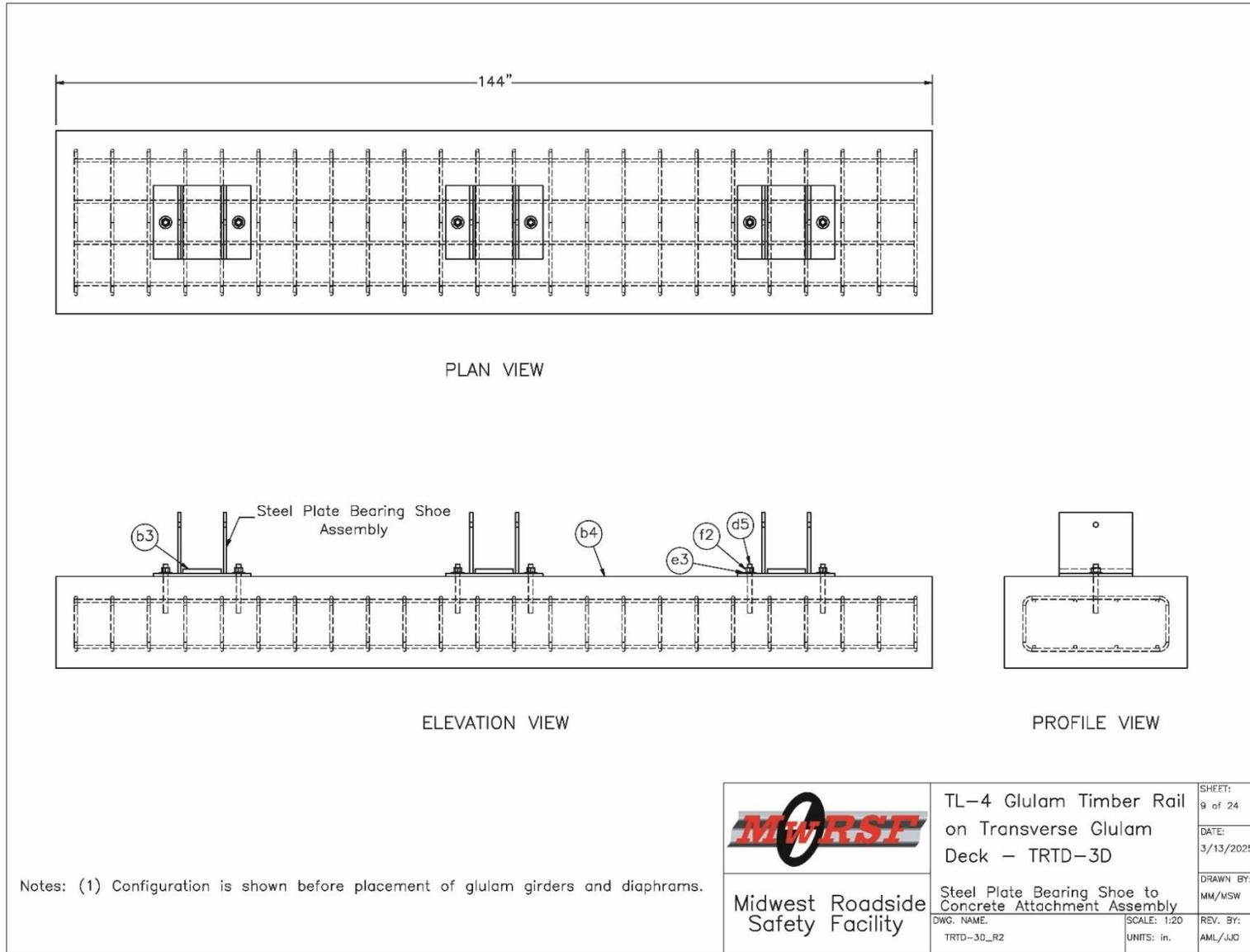
Figure N-9. Test No. TRTD-3 Concrete and Bearing Assembly Details
