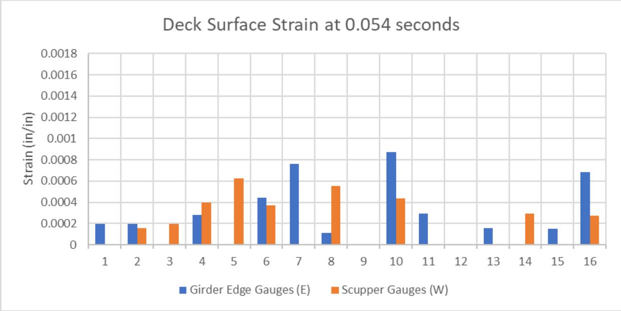
Figure 206. Deck Strain Gauges Across Both Deck Panels at 0.054 Seconds After Impact
