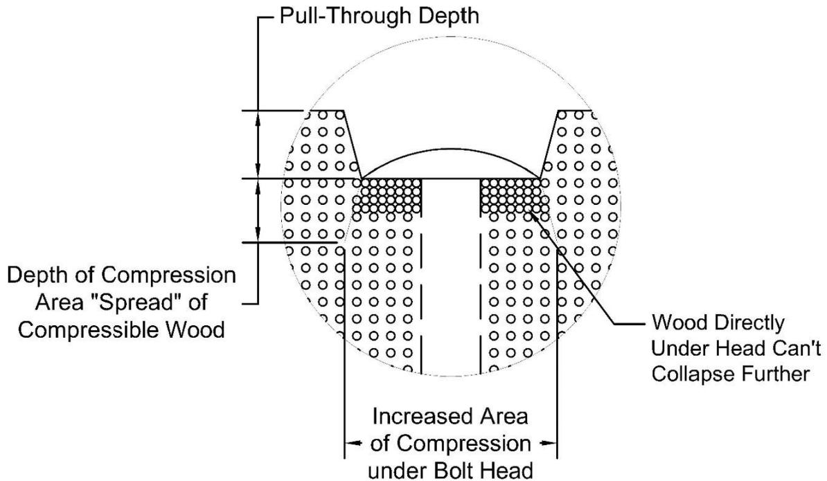
Figure D-5. Bolt Head Pull-Through Model
