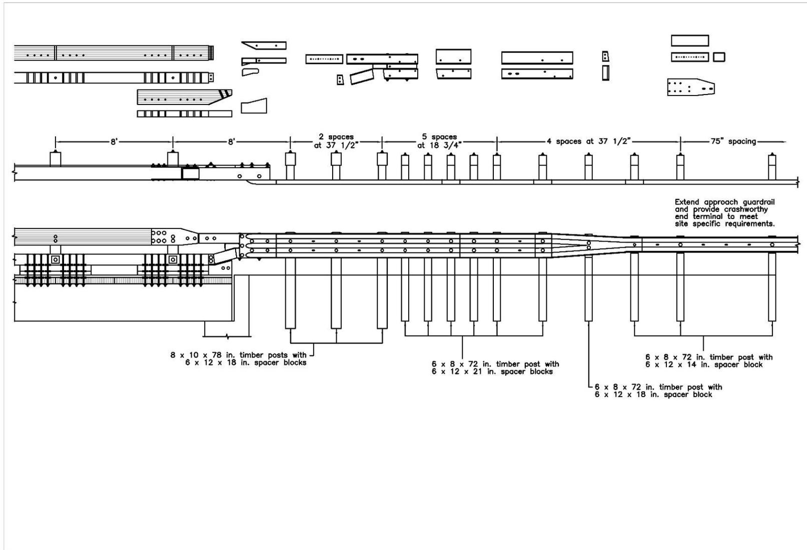
Figure K-37. Option 6.6 – Half-Post Spacing, 8-ft Gap, Steel Components, Steel Reverse Taper, Steel Flap Curb Taper
