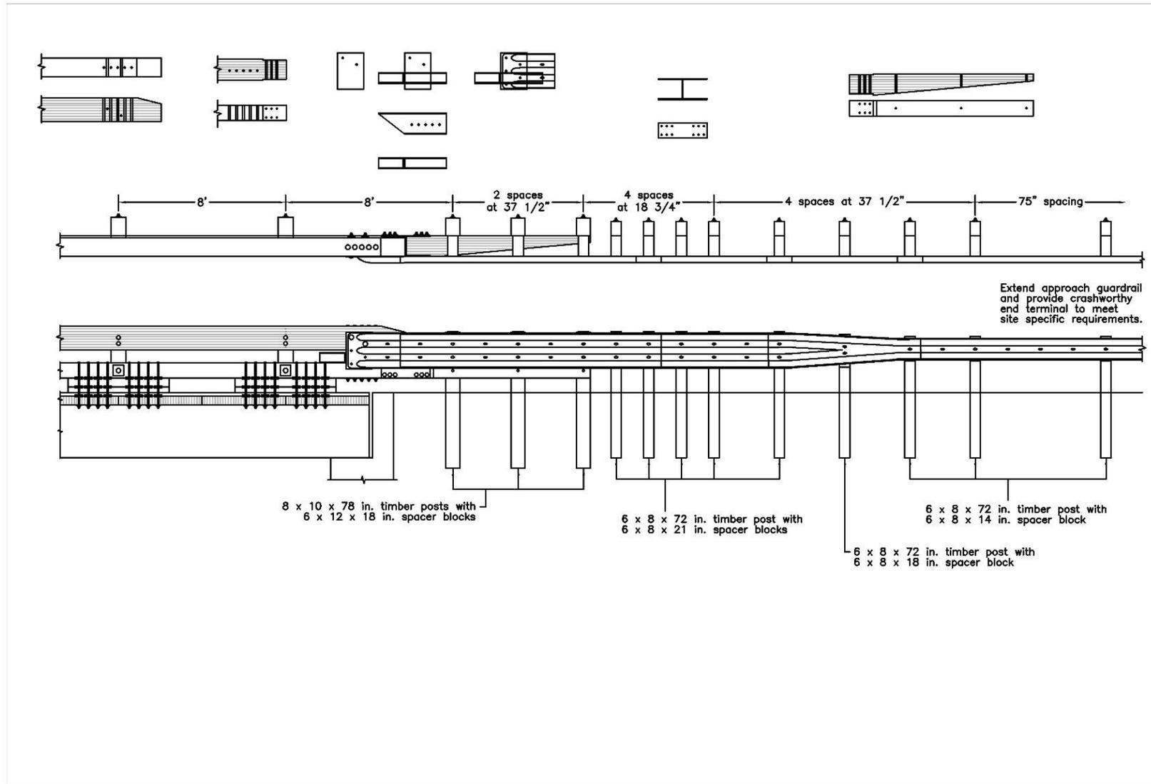
Figure K-41. Option 7.4 – Half-Post Spacing, 8-ft Gap, Welded End Shoe to Steel Reverse Taper, Curb Taper Behind Thrie-beam
