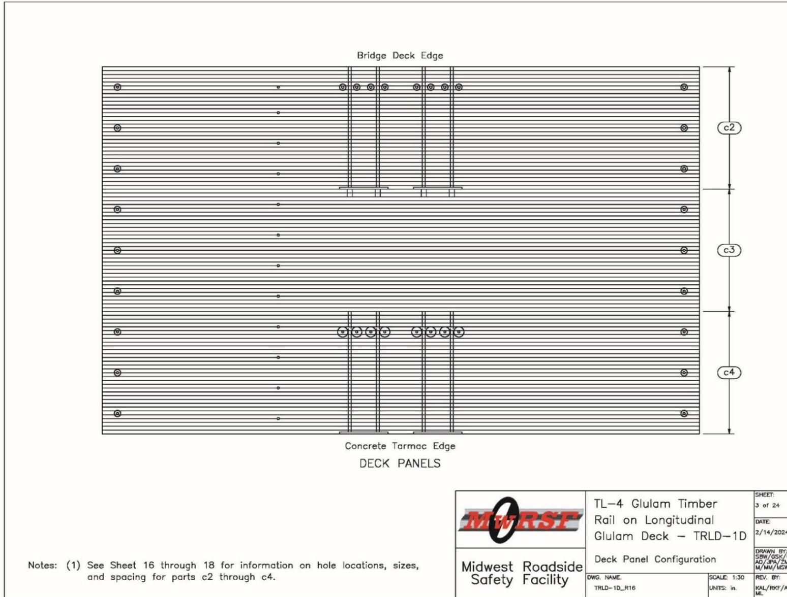
Figure 245. Deck Panel Configuration, Test No. TRLD-1
