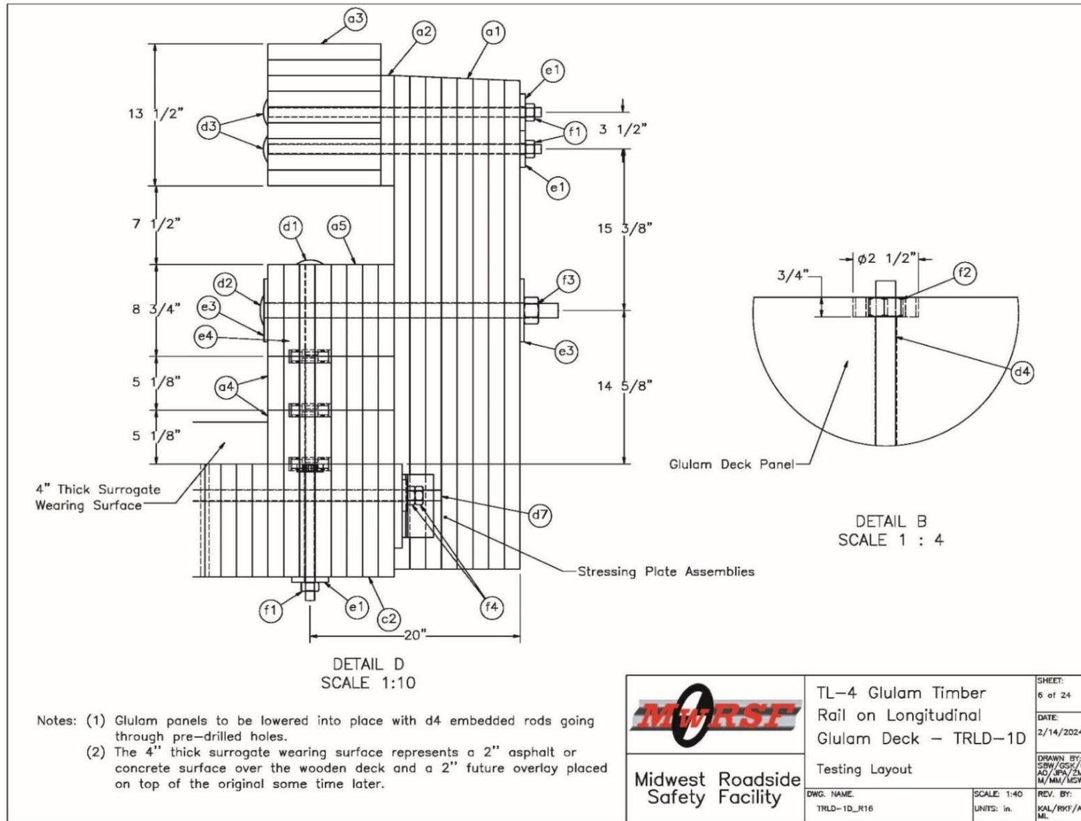
Figure 248. Post and Deck Assembly Details, Section View, Test No. TRLD-1
