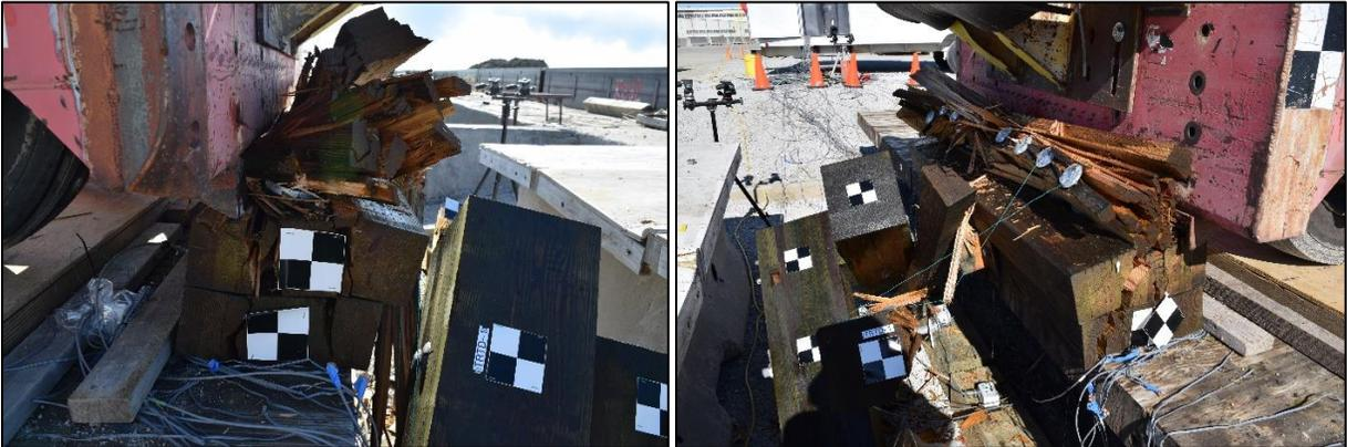
Figure 191. Damaged Curb Rail Attached to Bolts Following Impact
