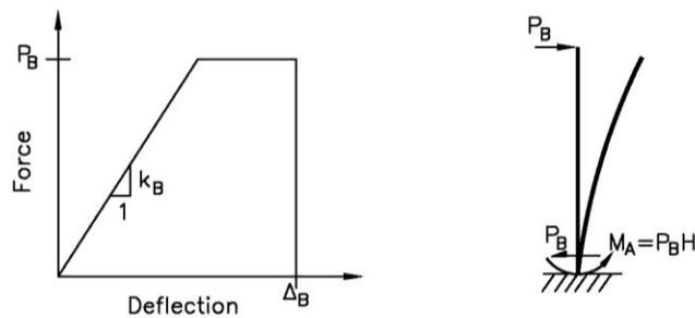
Figure 64. BARRIER VII Post Load-Deflection Curve when Limited by Deflection [11]
