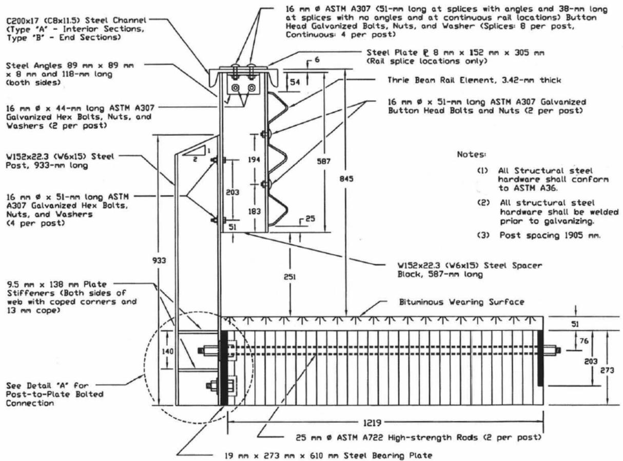
Figure 4. AASHTO PL-2 Bridge Railing Cross-Section on Longitudinal Glulam Deck [19]
