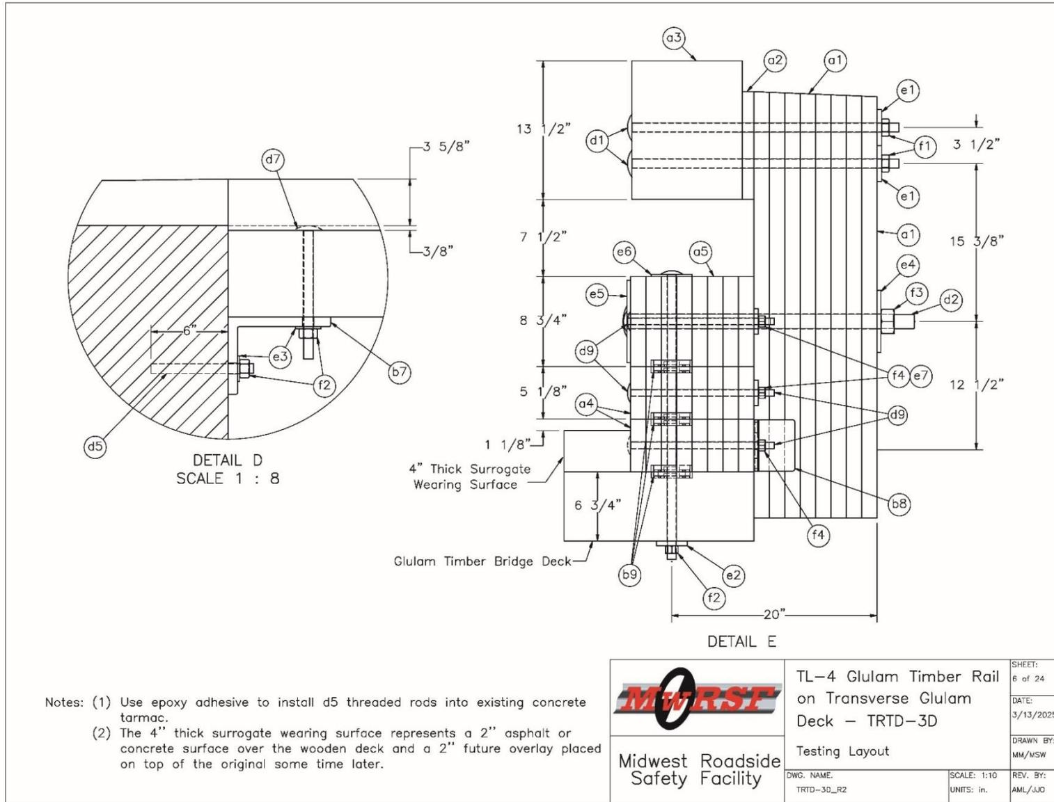
Figure N-6. Test No. TRTD-3 Post and Deck Assembly Details, Section View
