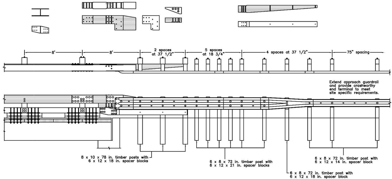
Figure K-36. Option 6.5 – Half-Post Spacing, 8-ft Gap, Notched L-Plate, Custom Glulam Piece, Wood Reverse Taper, Stepped Curb Taper
