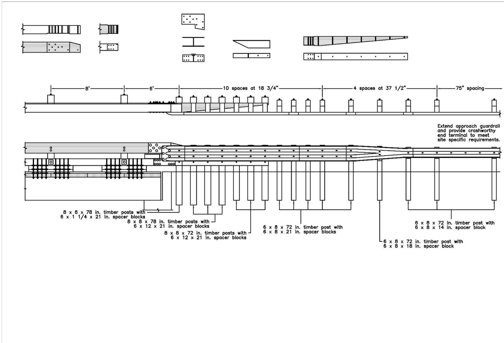
Figure K-46. Option 7.9 – Quarter-Post Spacing, 6-ft Gap, Cut L-Plate, Steel Reverse Taper, Curb Taper with Bumpout Behind Thrie-beam
