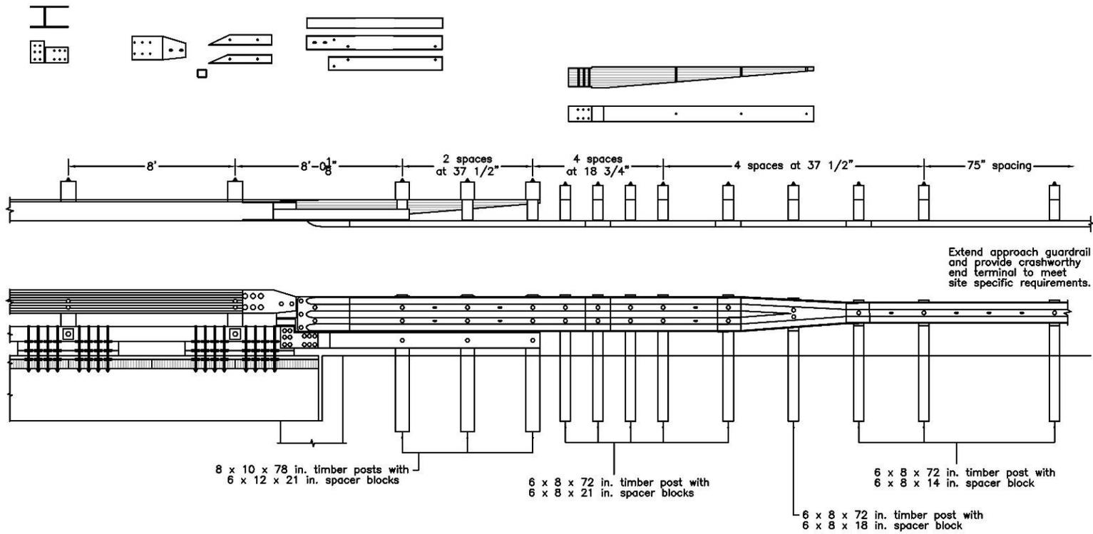
Figure K-13. Option 2.8 – Half-Post Spacing, 8-ft Gap, Steel Components, Partially Removed Blockout, Steel Reverse Taper, Stepped Thick Curb Taper
