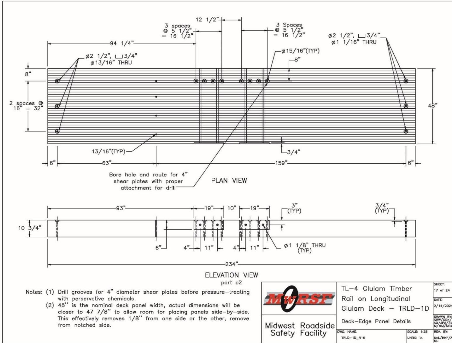
Figure 259. Deck Panel 1 Details, Test No. TRLD-1
