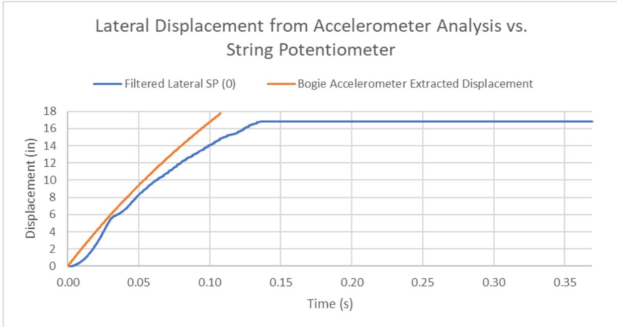
Figure 207. Test No. TRTD-1 Bogie Accelerometer vs. String Potentiometer Lateral Post Deflections
