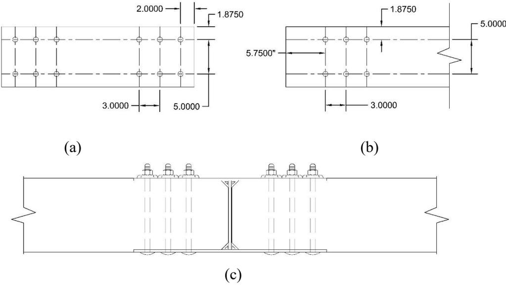
Figure 97. Lower Curb Rail Connection Details: (a) Bolt Spacing in Steel Plate; (b) Bolt Spacing in Wood Rail; (c) Plan View of Connection
