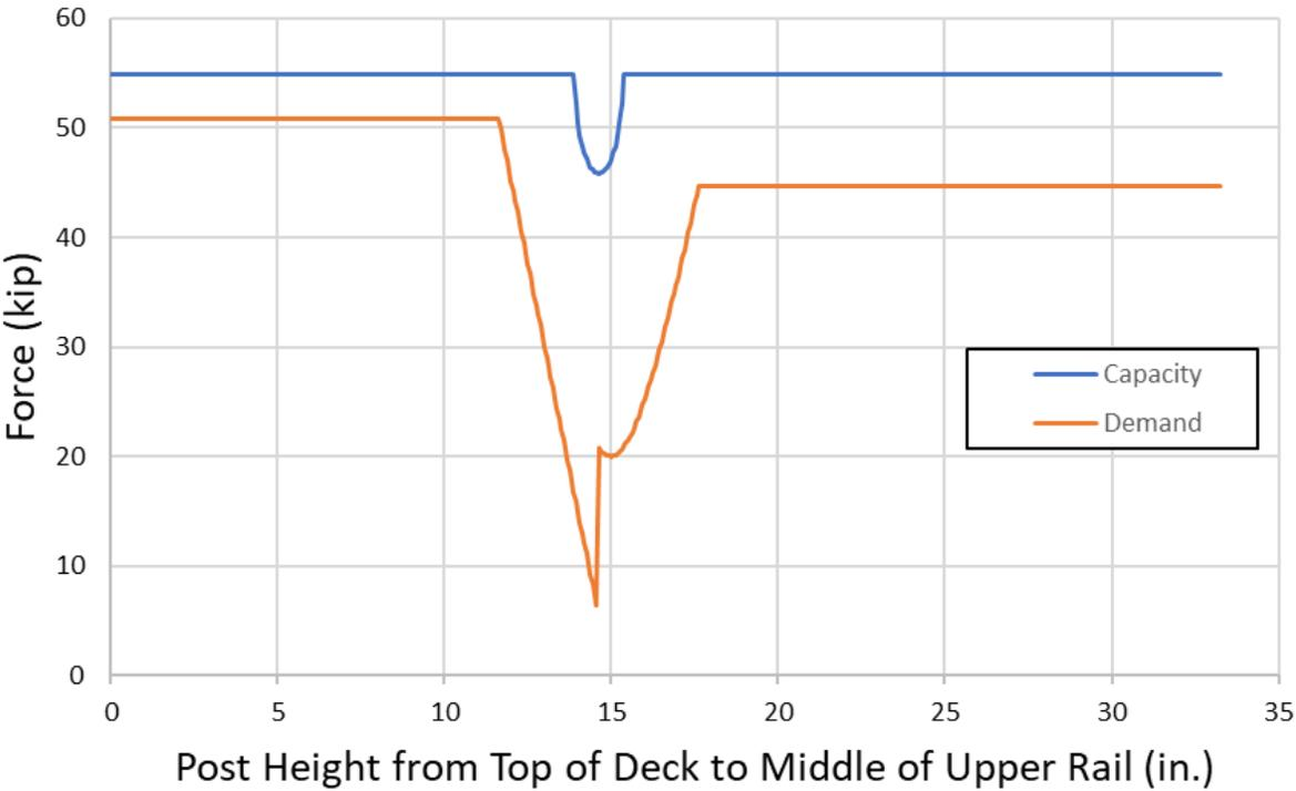
Figure 91. 10.5-in. x 8.75-in. Post Shear Capacity to Demand Comparison
