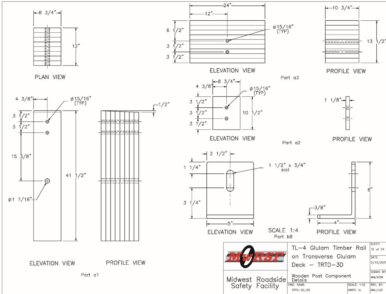
Figure N-15. Test No. TRTD-3 Vertical Post, Upper Rail, Blockout, and Angle Guide Details
