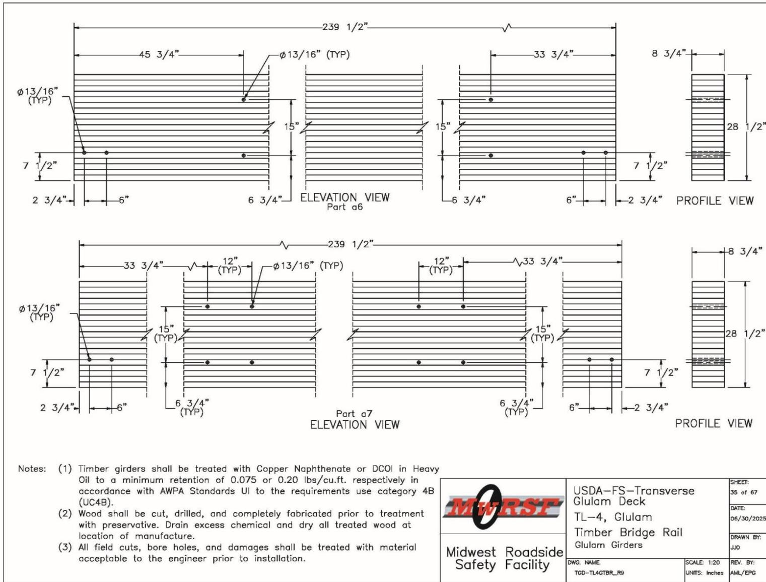
Figure O-35. Bridge Superstructure Girder Details
