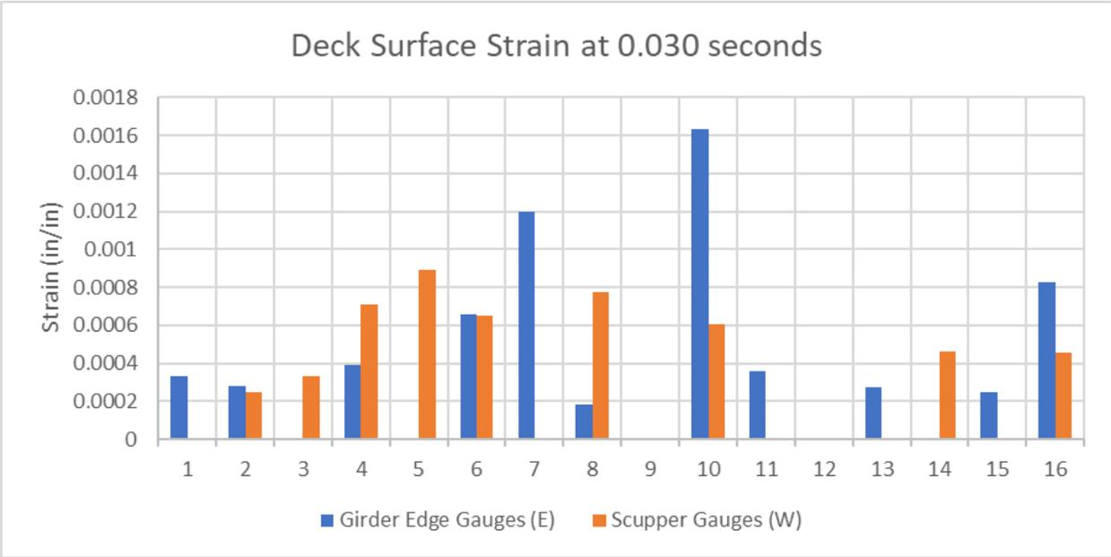
Figure 205. Deck Strain Gauges Across Both Deck Panels at 0.030 Seconds After Impact
