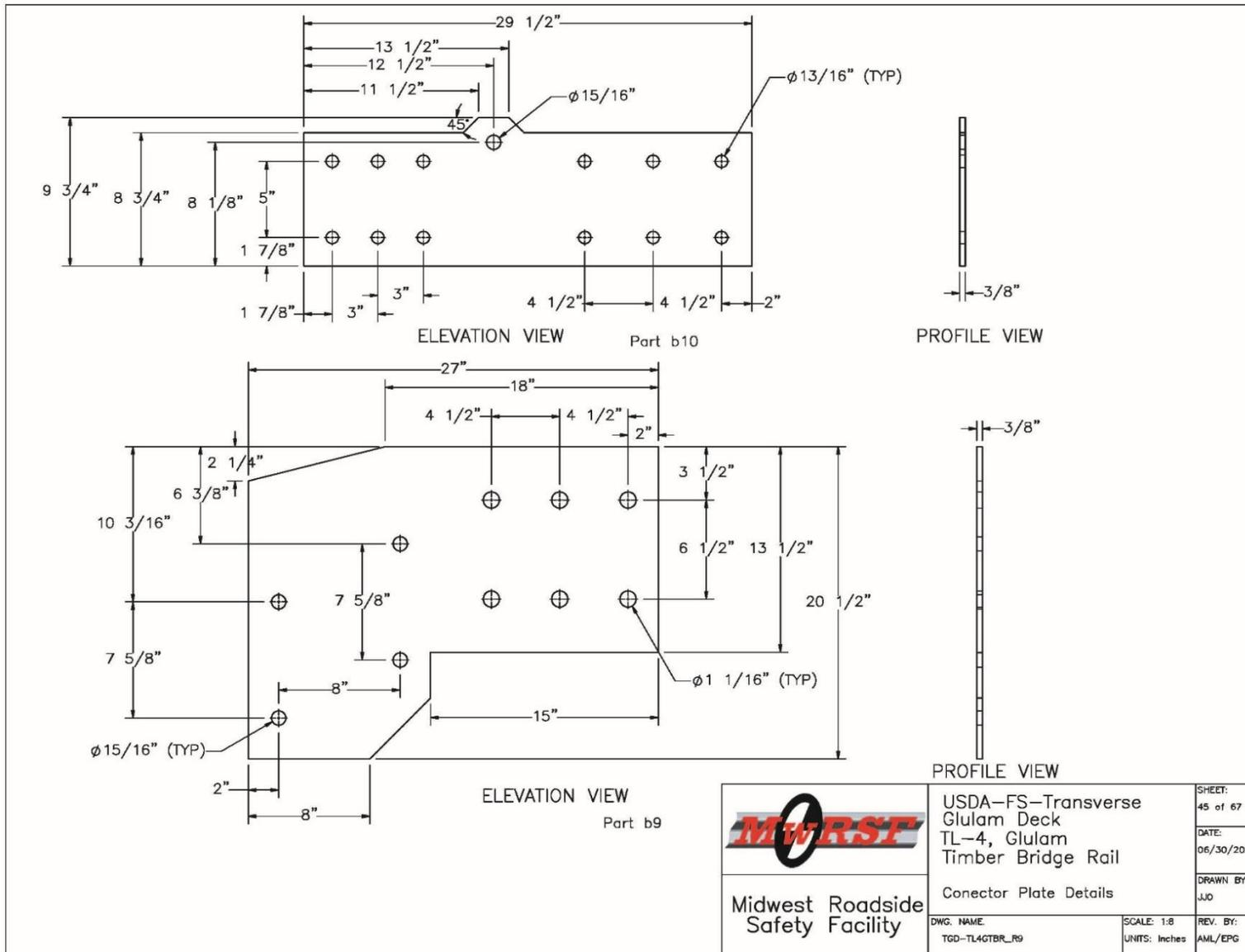
Figure O-45. Bridge Railing to AGT Steel Plate Connection Details
