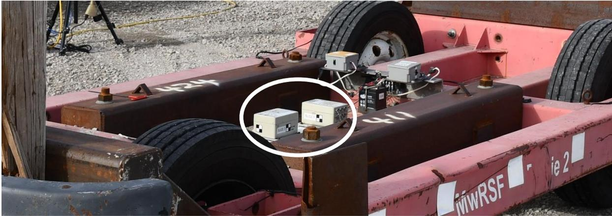
Figure 130. Accelerometers on Bogie Vehicle, SLICE-1 on Left and SLICE-2 on Right
