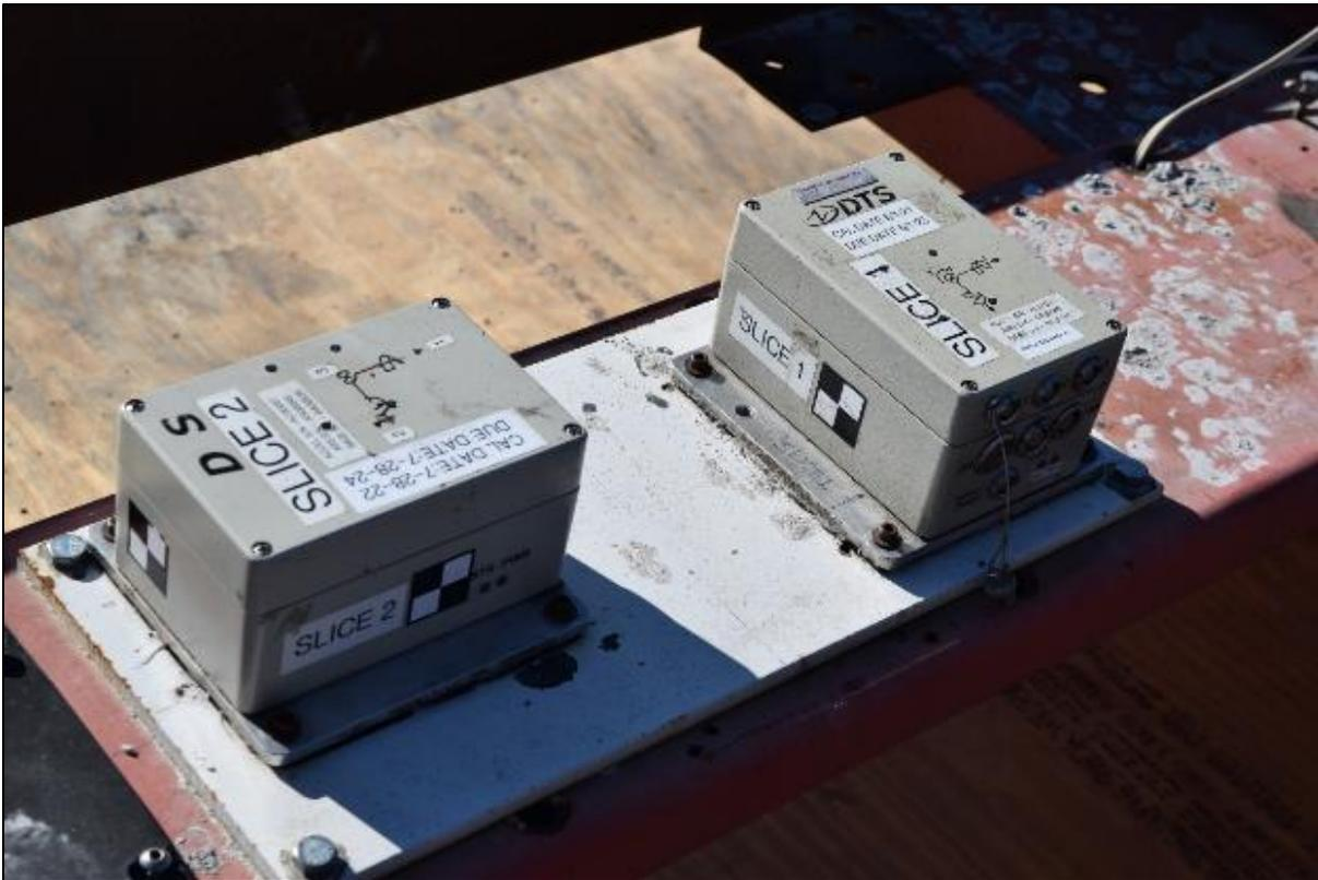
Figure 179. Accelerometer and Rate Transducer Systems on Bogie Vehicle
