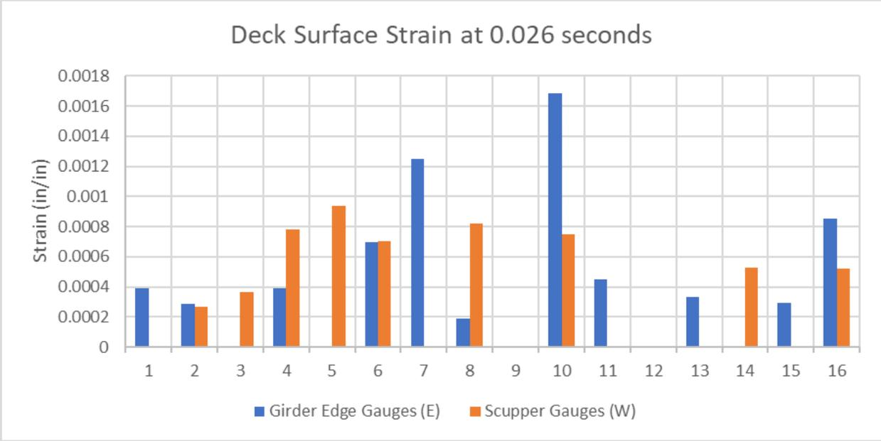
Figure 204. Deck Strain Gauges Across Both Deck Panels at 0.026 Seconds After Impact
