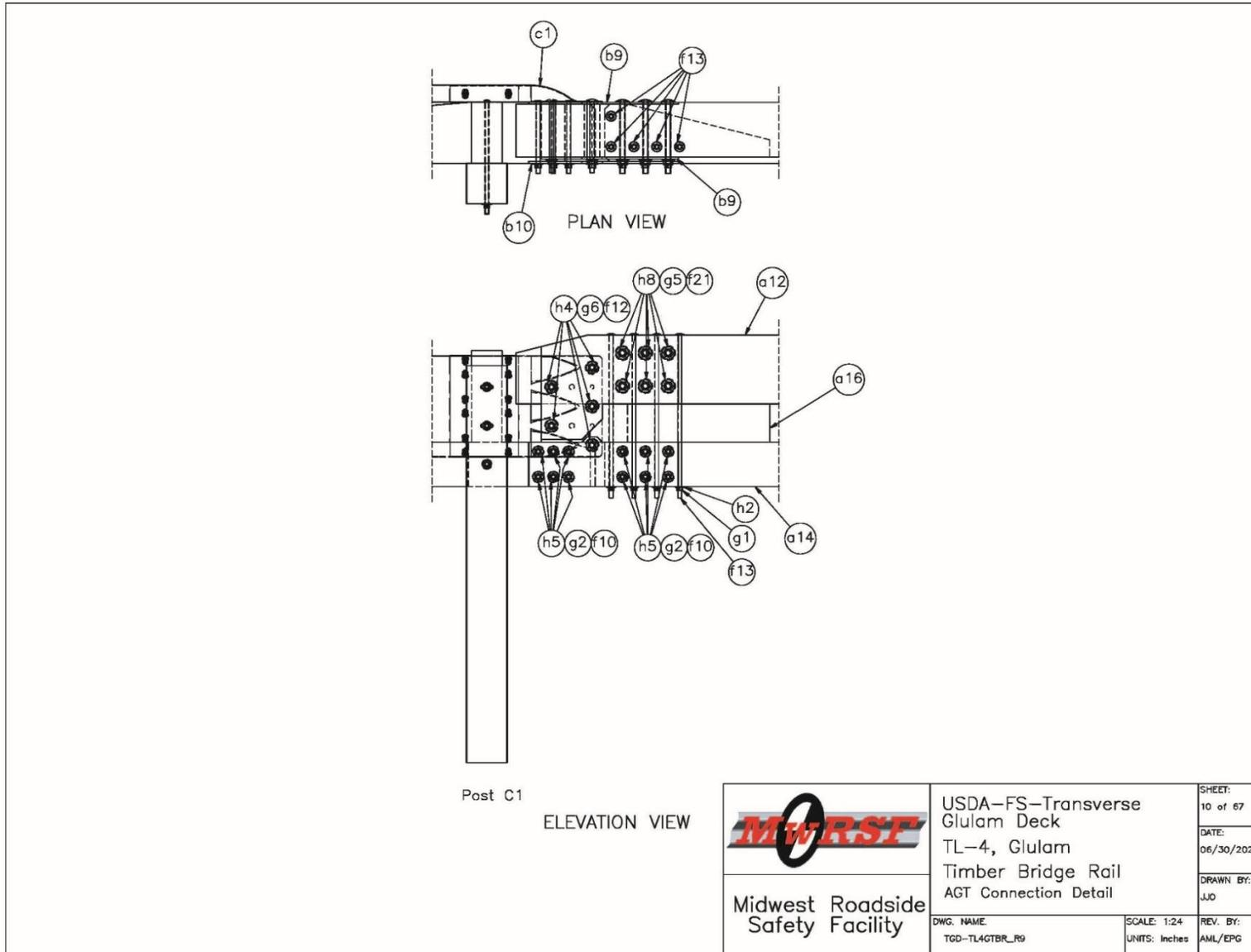
Figure O-10. AGT System Connection to Bridge Railing Detail
