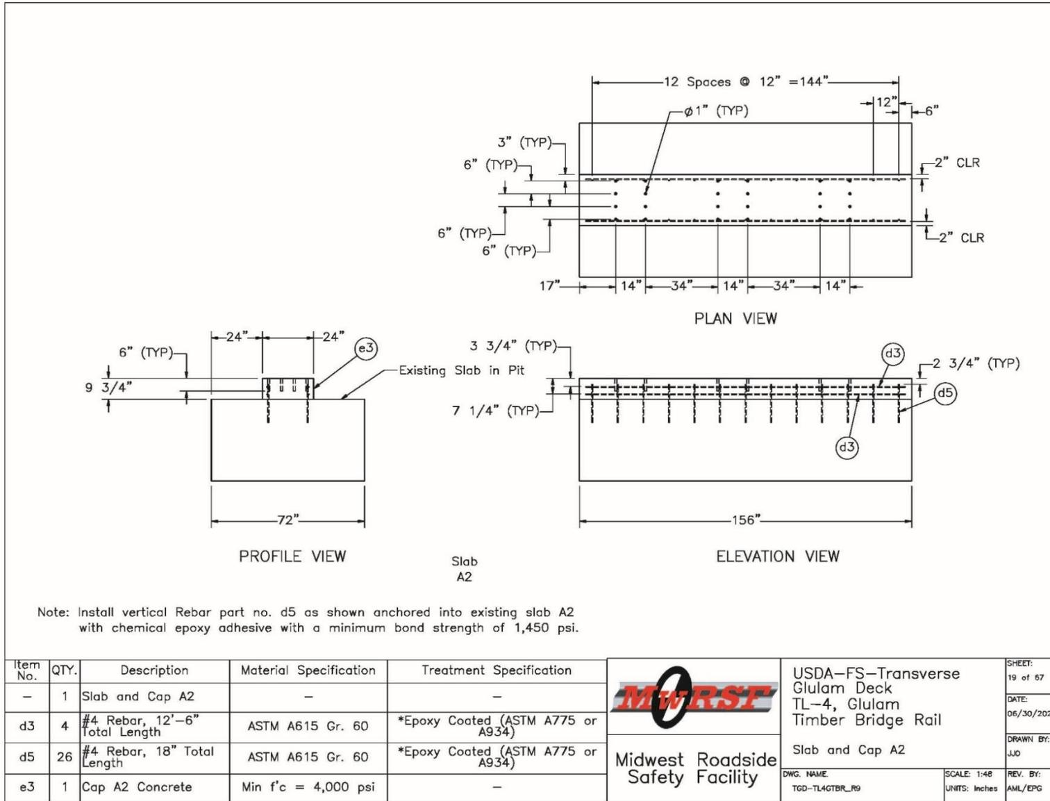
Figure O-19. Bridge Substructure Intermittent Pier A2 Details
