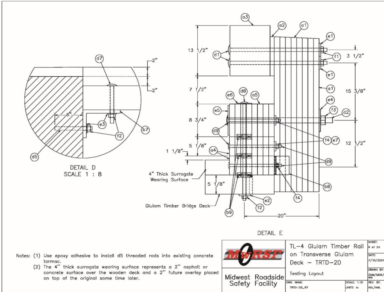
Figure 224. Post and Deck Assembly Details, Section View, Test No. TRTD-2
