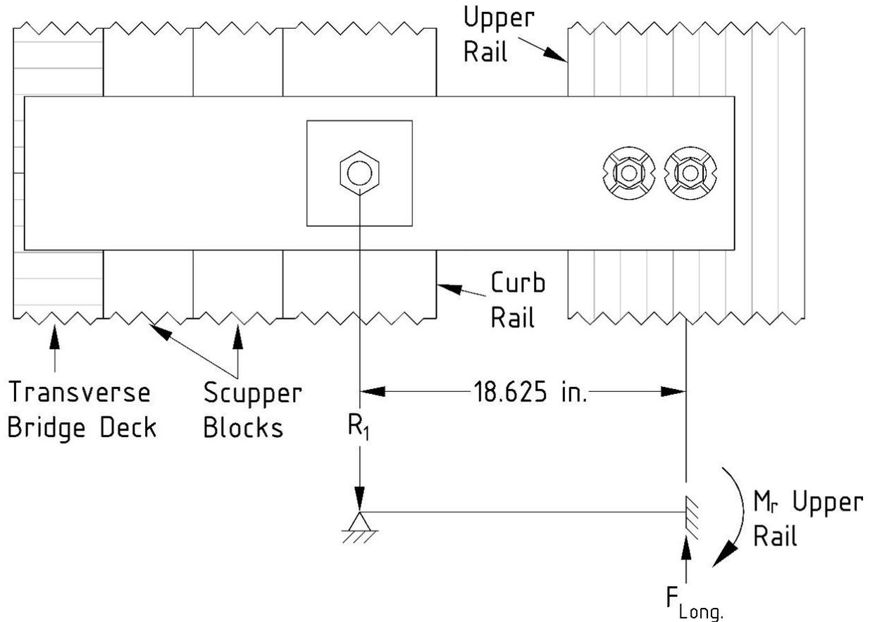
Figure 81. Free-Body-Diagram for Post Flexure from Longitudinal Loads
