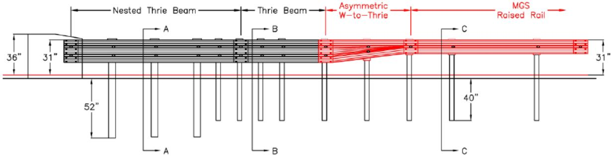
Figure 26. AGT System Configuration after Installation of 3-in. Wearing Surface [38]
