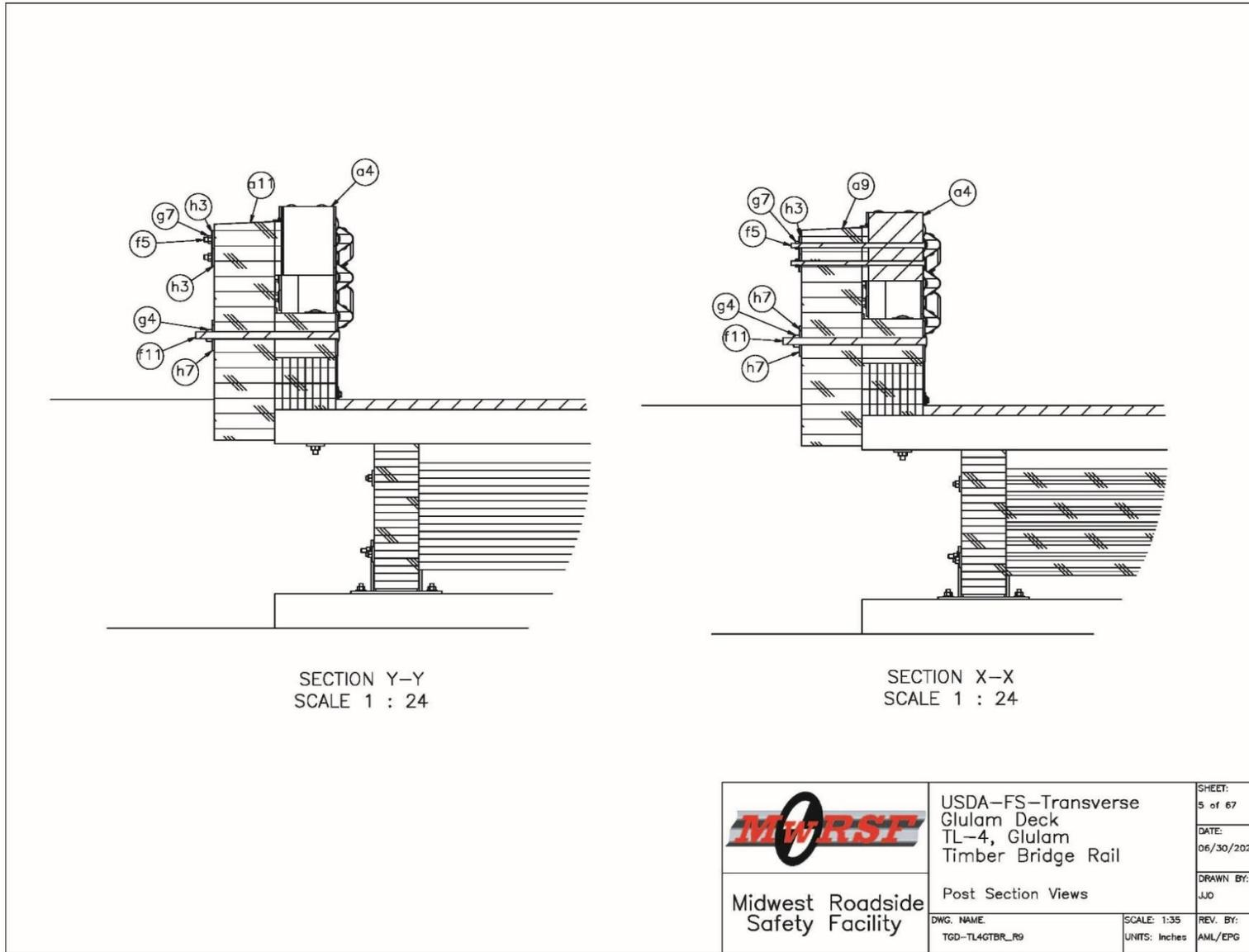
Figure O-5. Post Cross-Section View at Upper Railing Splice and at Typical Post Locations
