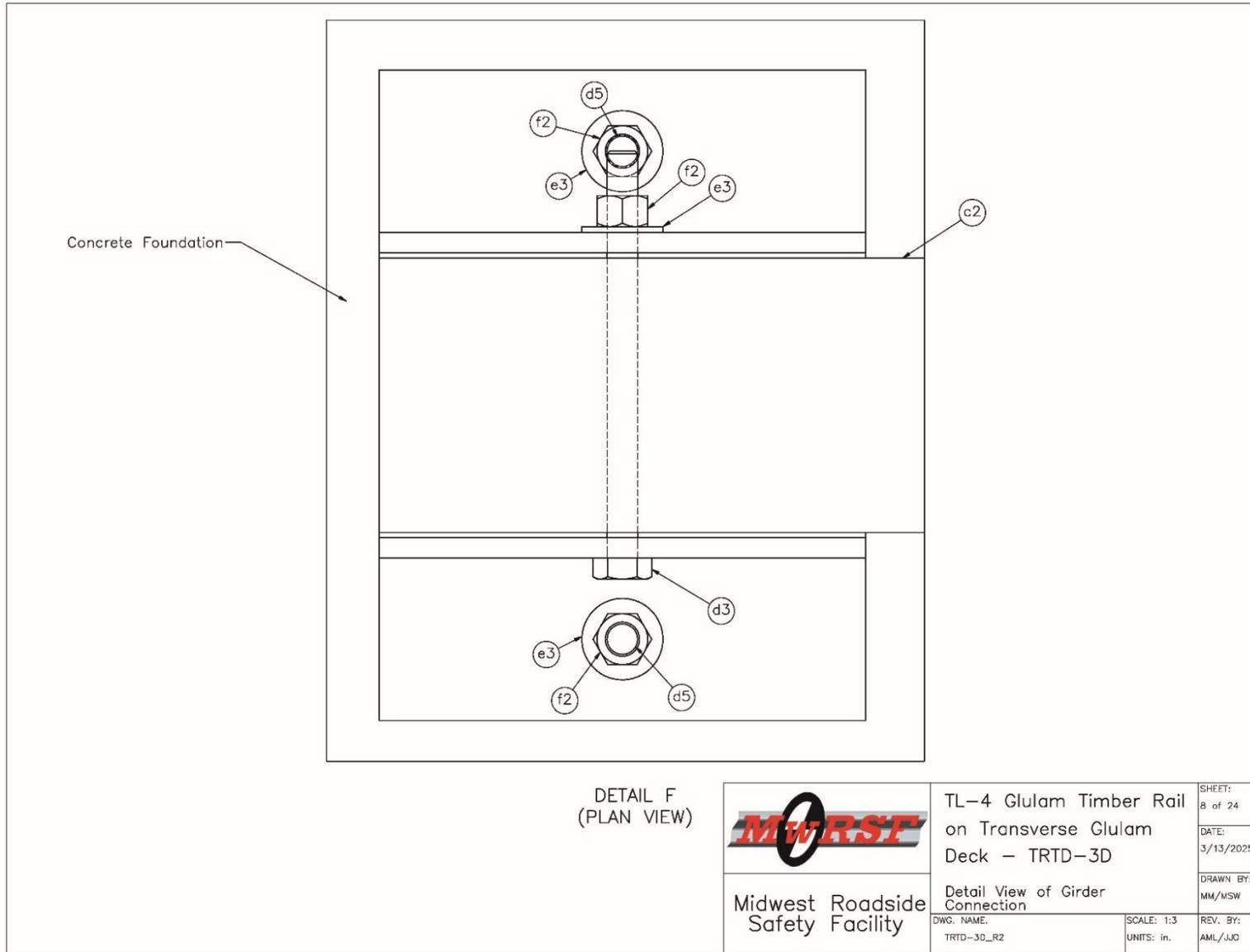
Figure N-8. Test No. TRTD-3 Girder Connection Details
