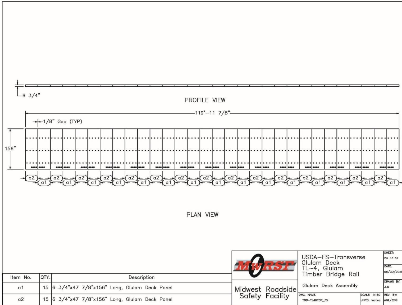
Figure O-24. Bridge Superstructure Deck Panel Layout
