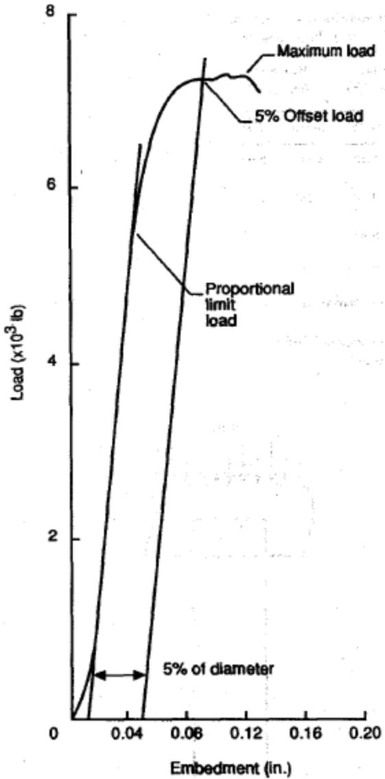
Figure 90. Typical Load-Displacement Curve for 3/4-in. Diameter Bolt Bearing Capacity on Southern Pine Wood Block [125]
