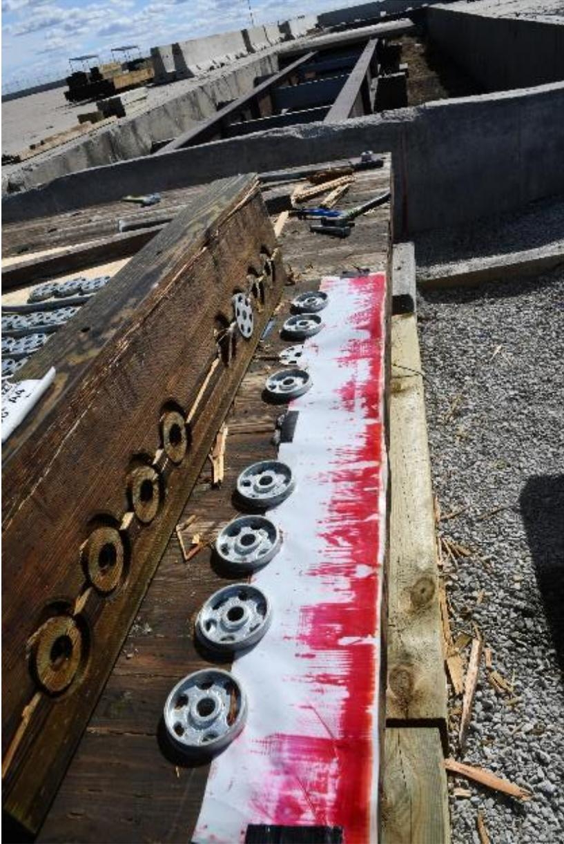
Figure 211. Pressure Film Underneath Bottom Scupper after Test No. TRTD-1
