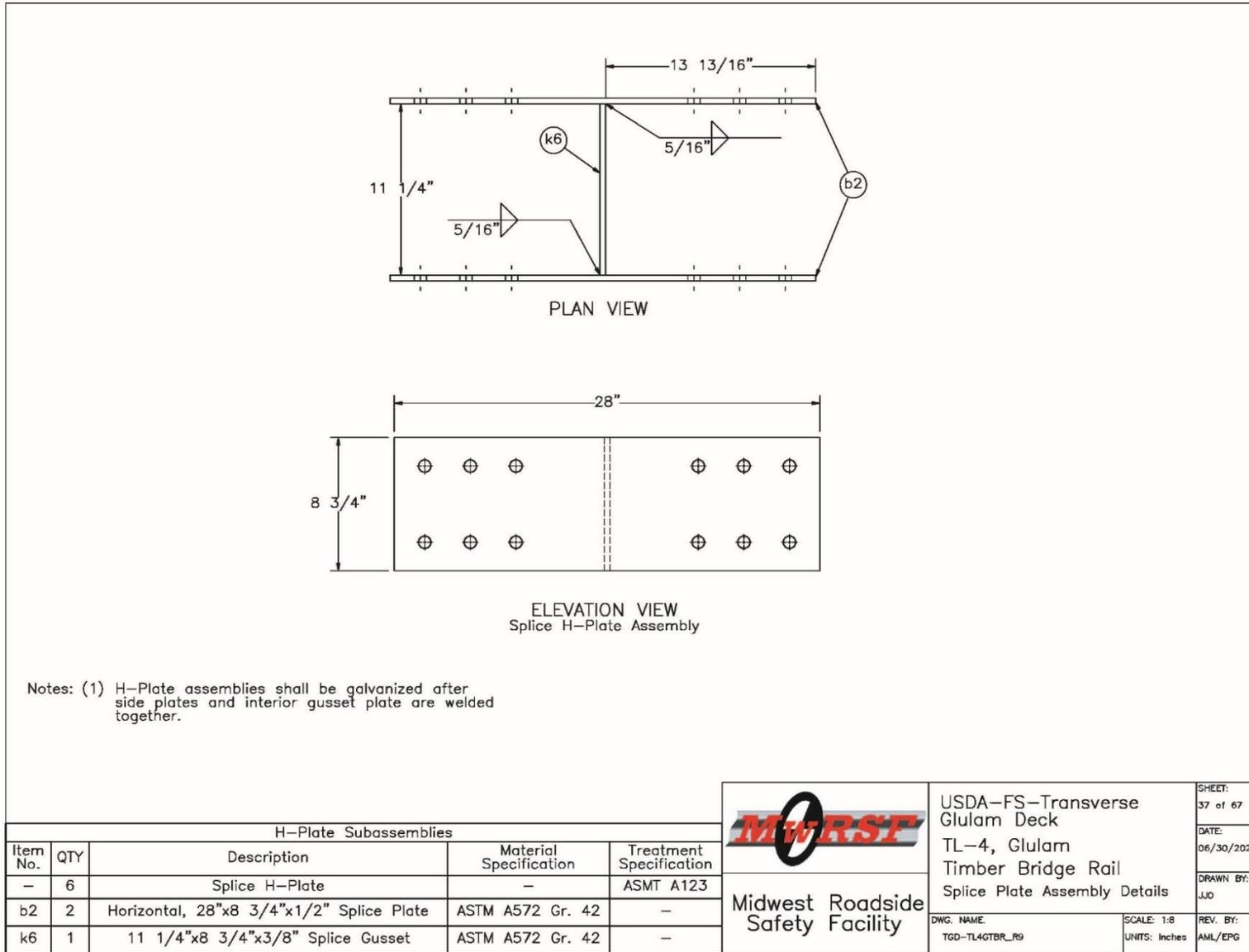
Figure O-37. Bridge Curb Railing Splice Plate Assembly Details
