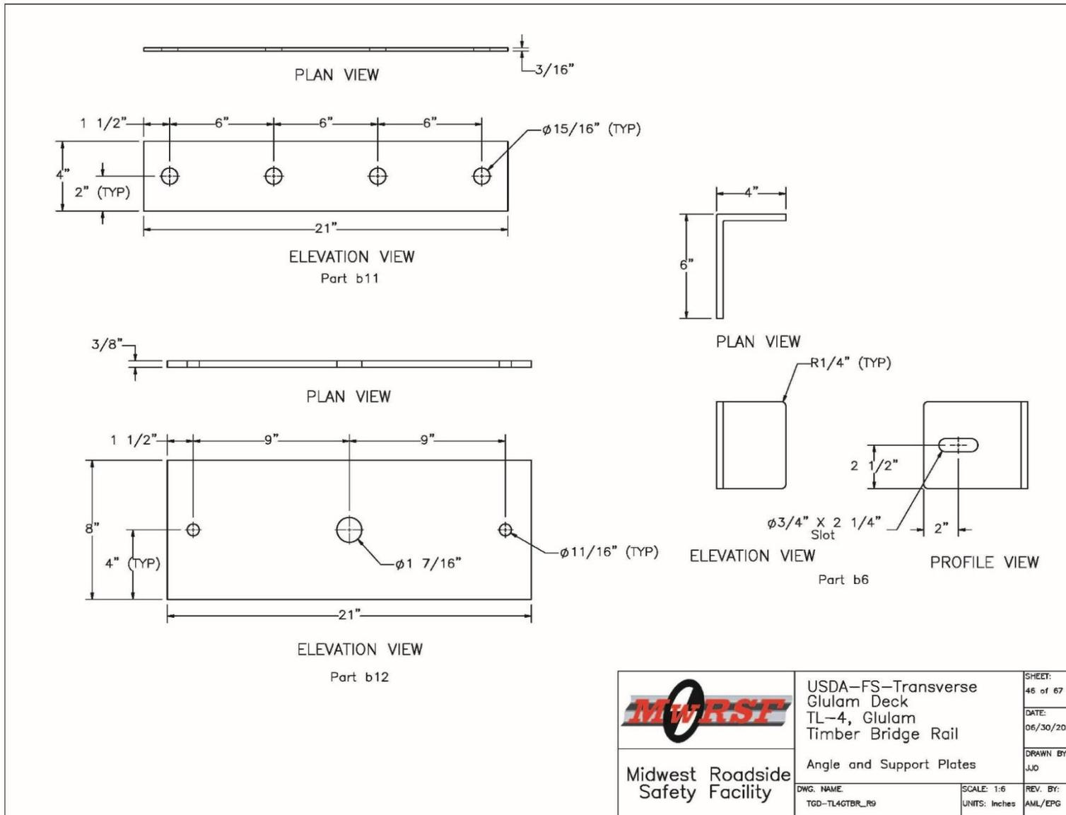
Figure O-46. Bridge Post Connection Hardware Details
