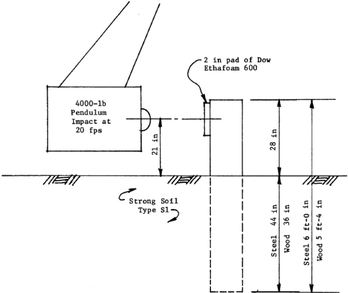
Figure 28. Diagram of Dynamic Component Test Setup by SwRI [39]
