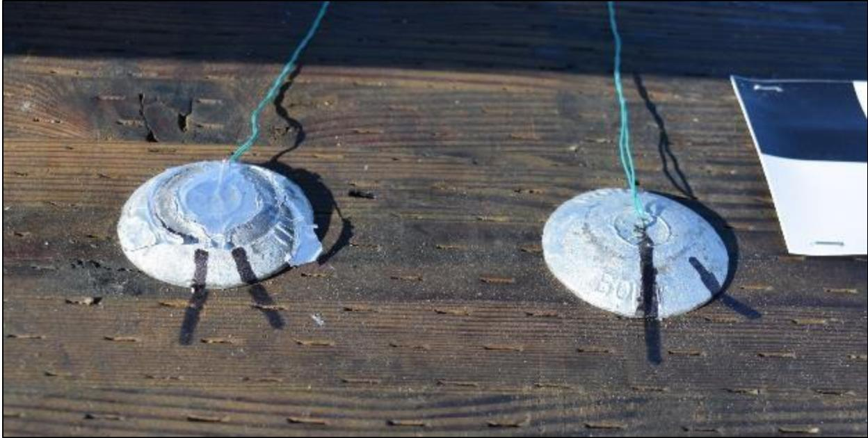
Figure 185. Bolt Axial Strain Gauges on Bolts d1.1 (right) and d1.2 (left) in test no. TRTD-1
