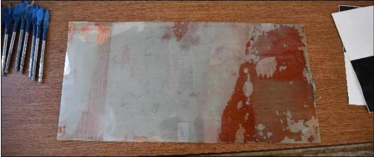
Figure 187. Pressure Film Between Back of Vertical Post and Back of Transverse Glulam Deck or Scupper Blocks, After Test No. TRTD-1
