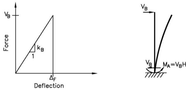
Figure 65. BARRIER VII Post Load-Deflection Curve when Limited by Shear [11]
