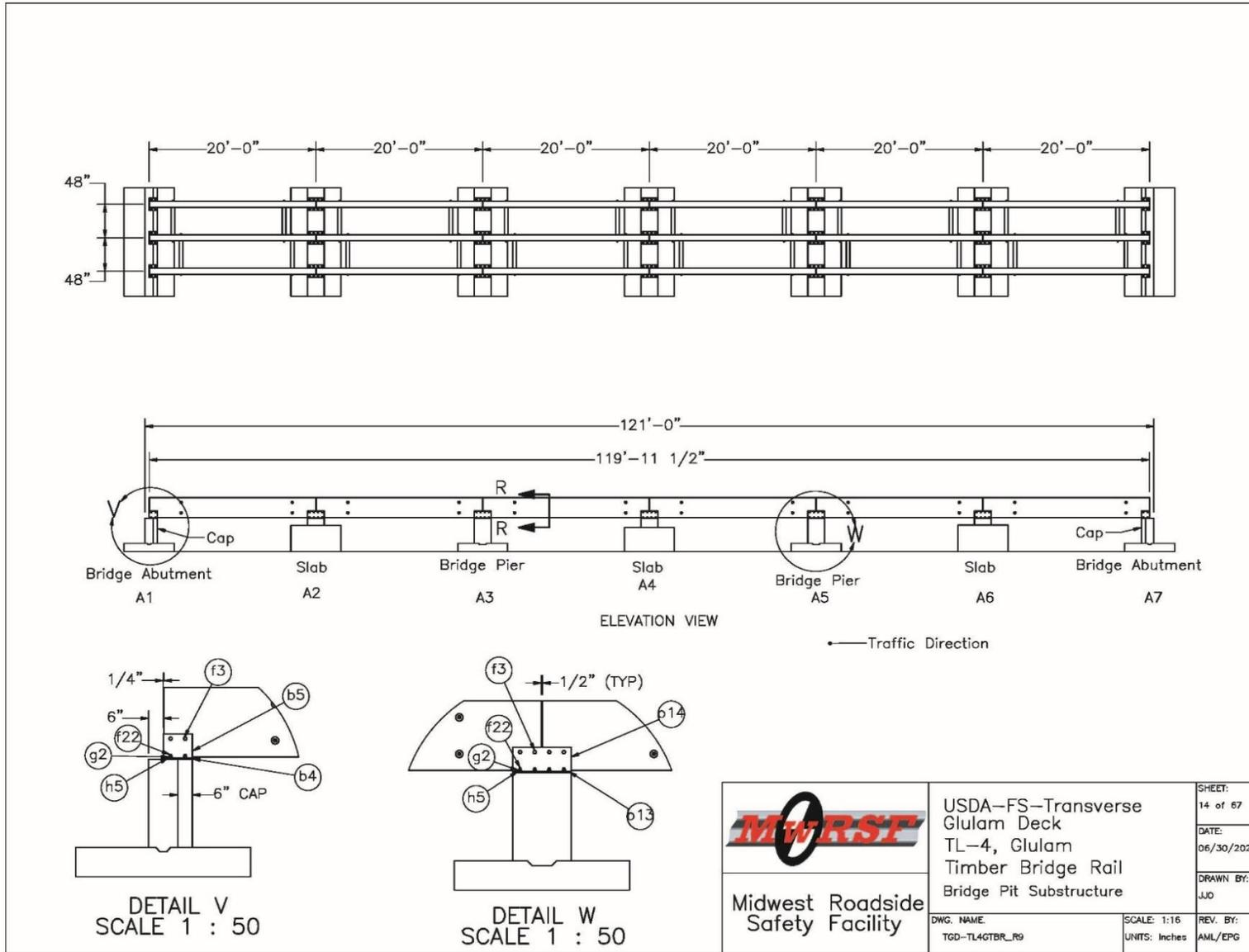
Figure O-14. Bridge Pit Substructure Plan and Elevation Views and Details
