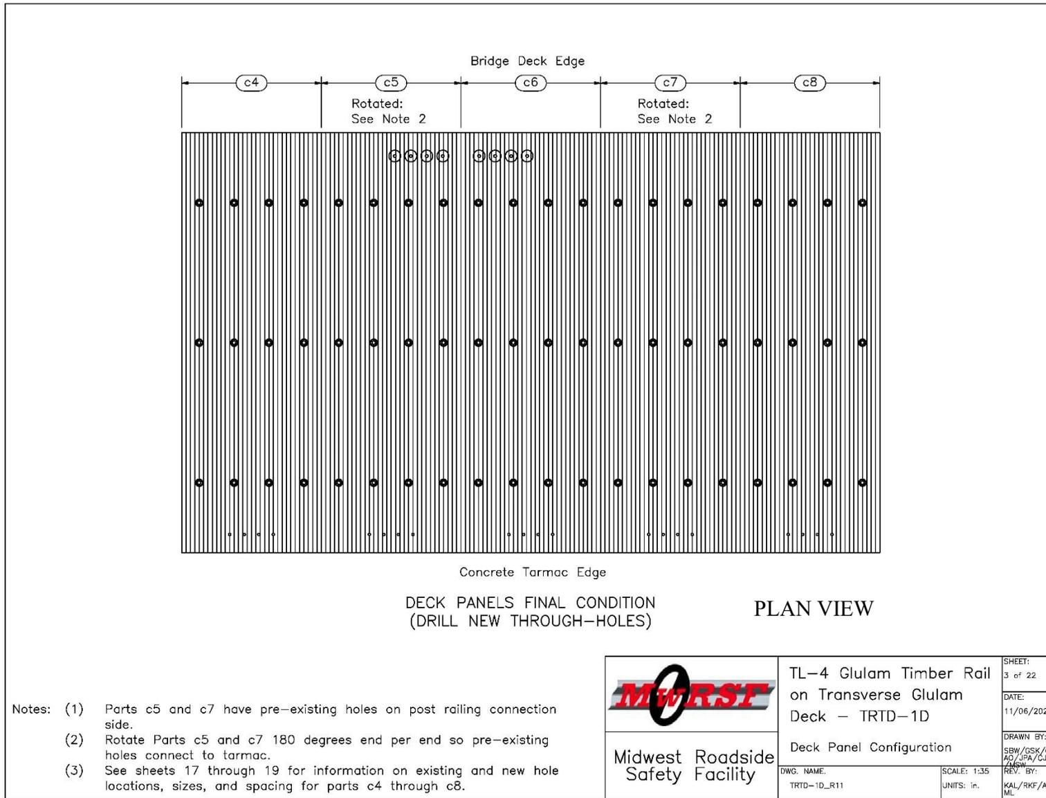
Figure 150. Deck Panel Configuration, Test No. TRTD-1
