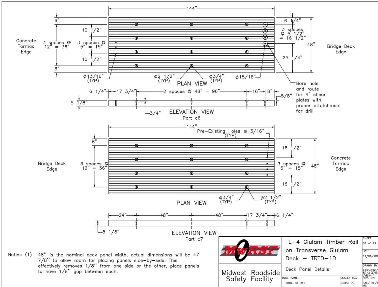
Figure 165. Deck Panel Details, Page 2, Test No. TRTD-1
