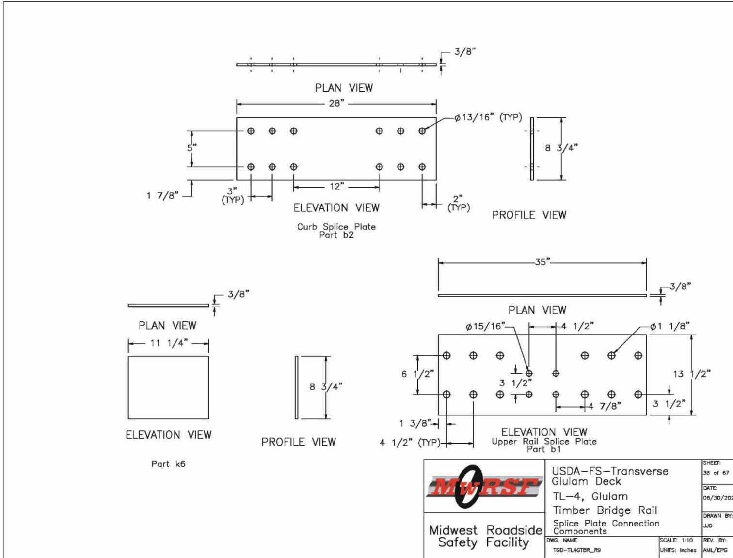
Figure O-38. Bridge Upper and Curb Railing Splice Pieces Details
