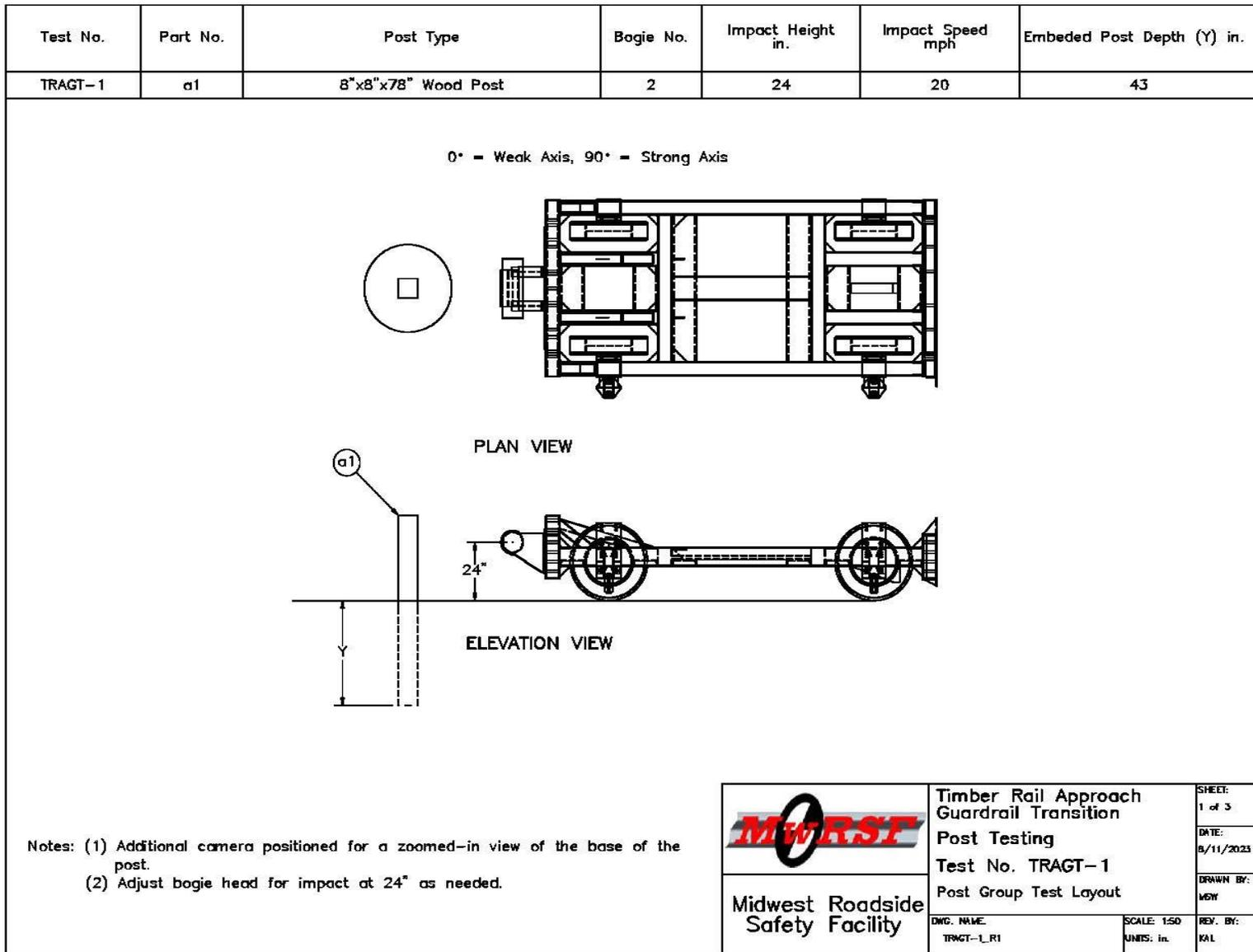
Figure 126. Test Layout, Impact on Single Post, Test No. TRAGT-1
