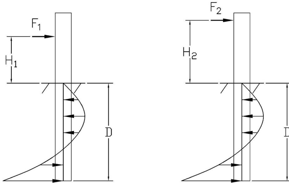
Soil Flexural Resistance Constant,  $F_1H_1 = F_2H_2$
