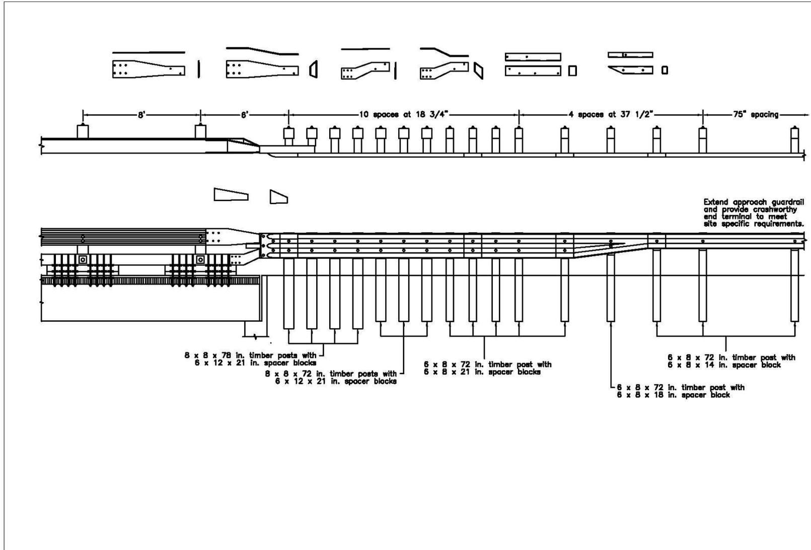
Figure K-2. Option 1.2 – Quarter-Post Spacing, 6-ft Gap, Steel Components, Partial Removal of Blockouts, Steel Reverse Taper, No Curb Taper
