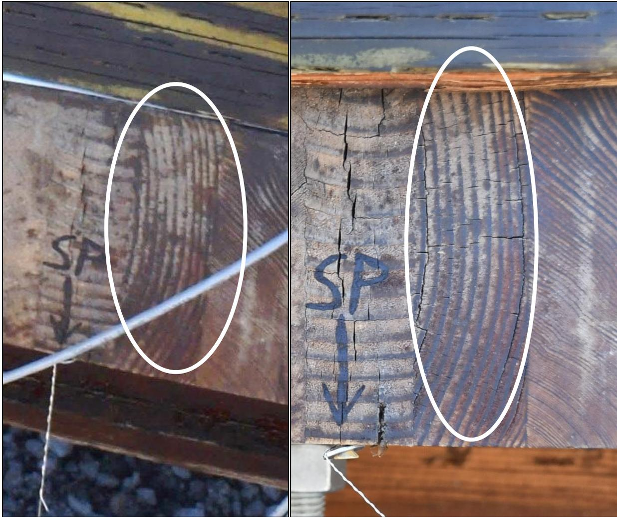
Figure 210. End Laminations of Left Deck Panel Before (left) and After (right) Component Testing
