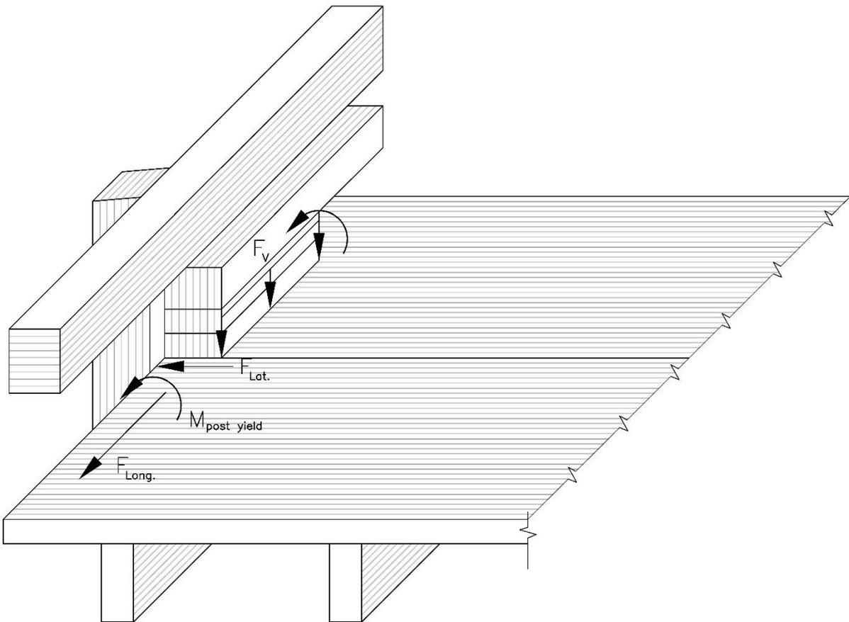
Figure 105. Transverse Deck External Force Diagram
