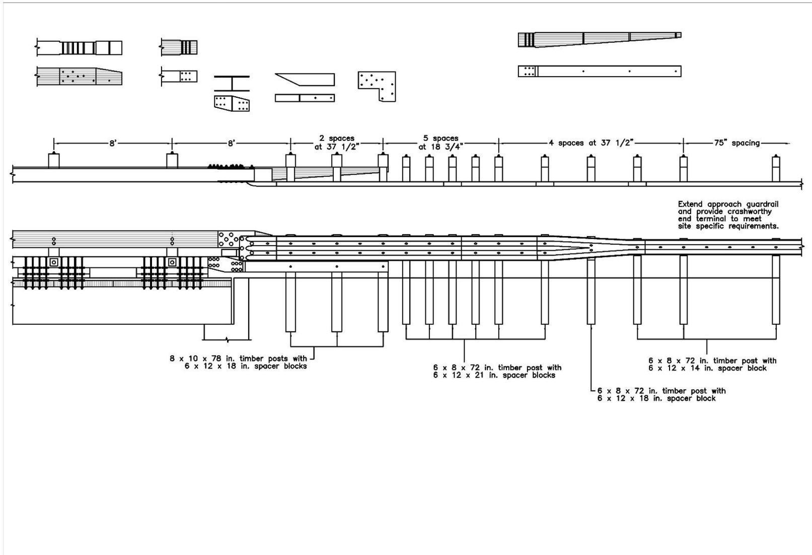
Figure K-39. Option 7.2 – Half-Post Spacing, 8-ft Gap, Notched L-Plate, Steel Reverse Taper, Stepped Curb Taper
