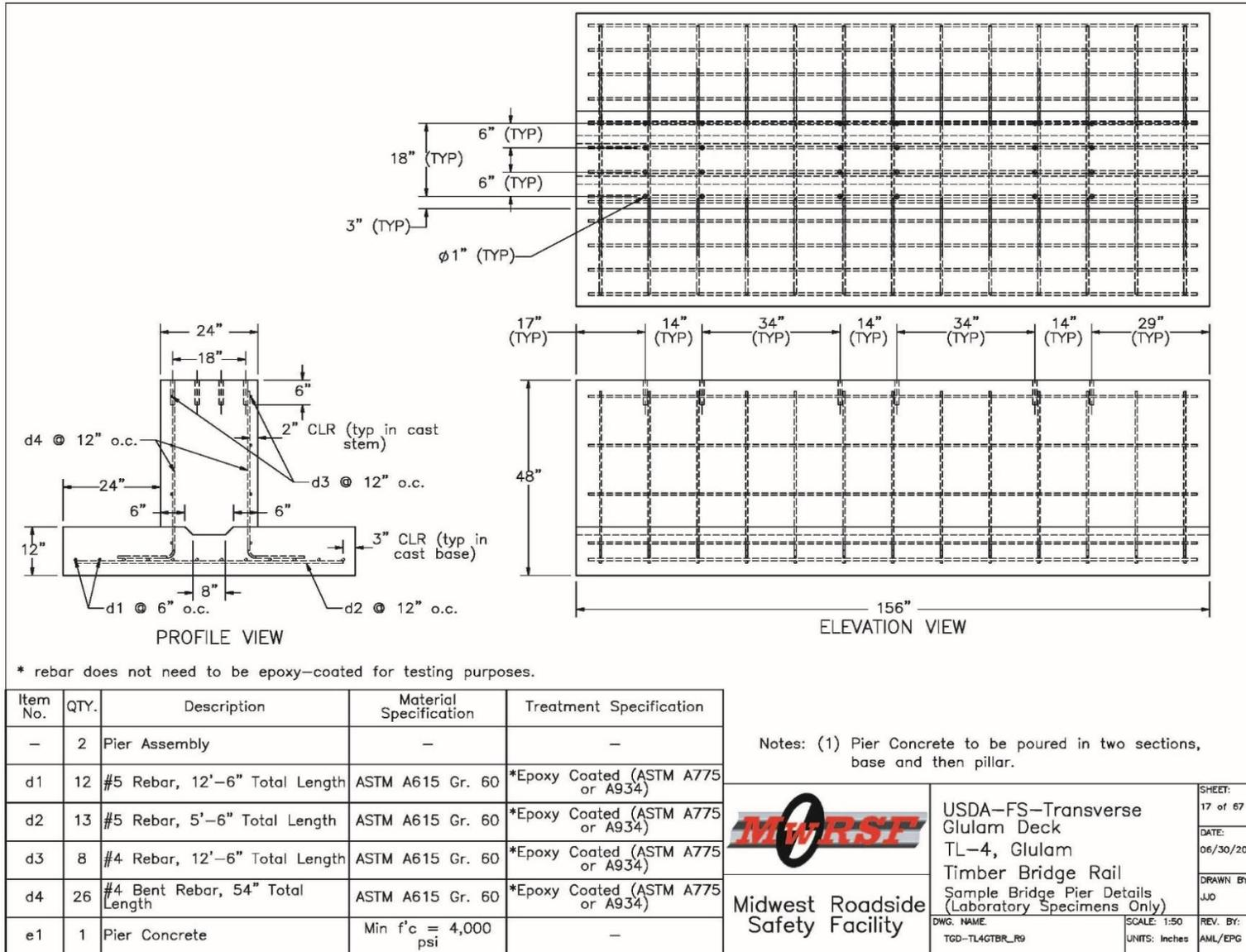
Figure O-17. Bridge Substructure Typical Pier Details
