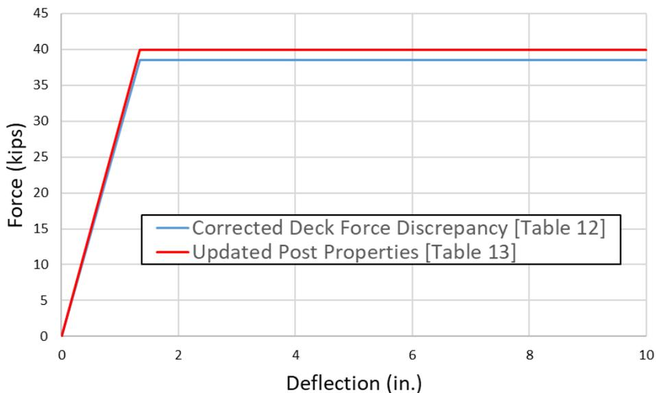
Figure 73. Adjusted Surrogate TL-4 Post Force-Deflection Curves for Flexural Capacity
