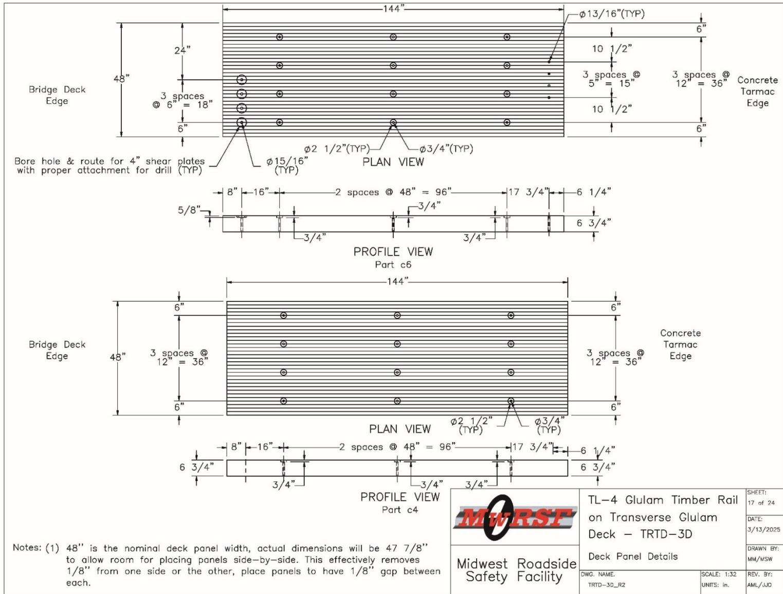
Figure 267: Test No. TRTD-3 Deck Panel Details, Page 1
