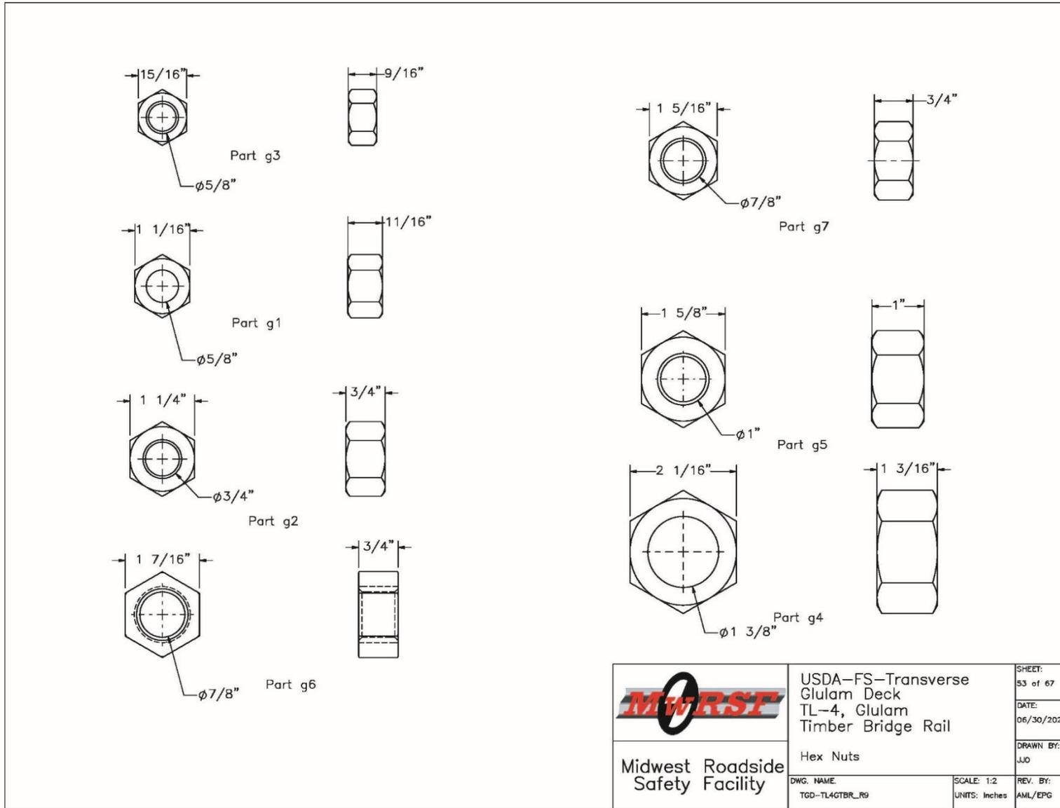
Figure O-53. Bridge Nut Hardware Details
