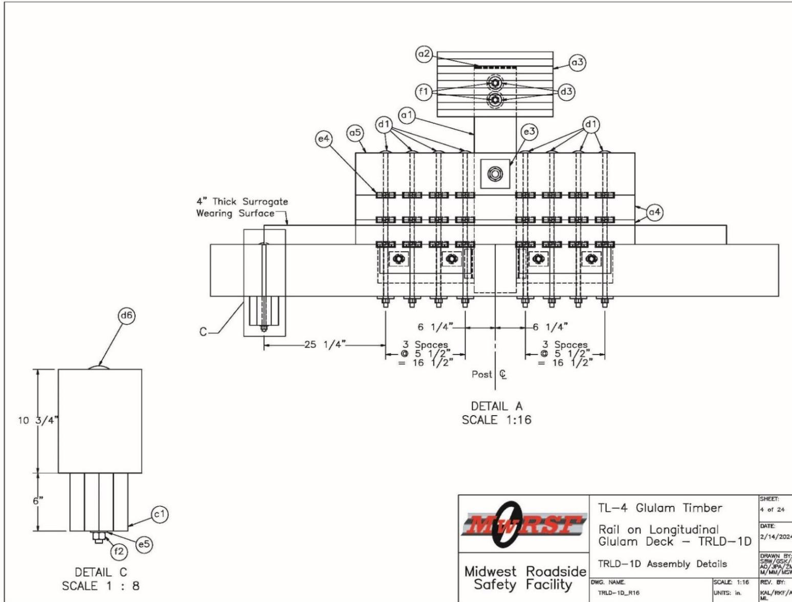
Figure 246. Post and Deck Assembly Details, Test No. TRLD-1
