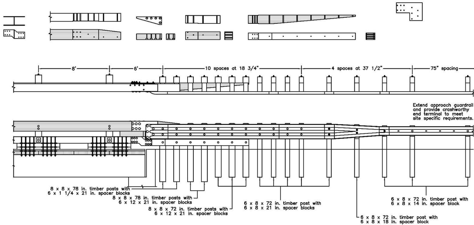
Figure K-16. Option 3.1 – Quarter-Post Spacing, 6-ft Gap L-Plate, Removed Blockouts, Wood Reverse Taper, Stepped Curb Taper
