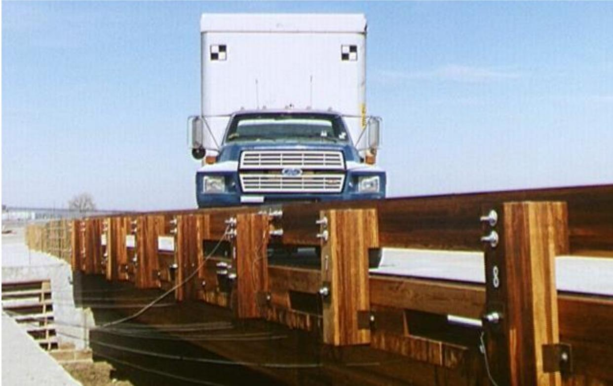
Figure 106. MwRSF NCHRP-350 TL-4 Tested Timber Bridge Railing [20]
