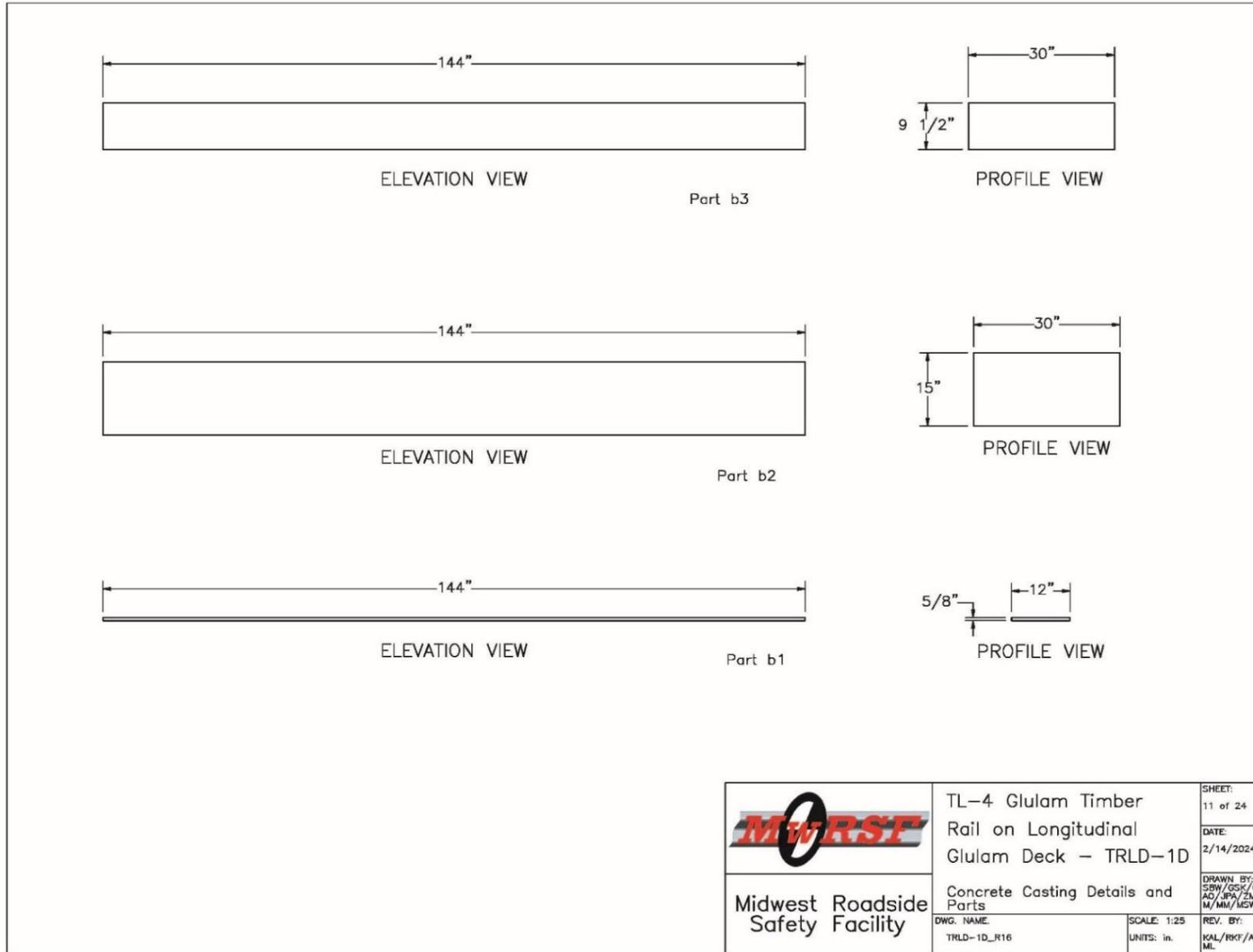
Figure 253. Concrete Details, Test No. TRLD-1
