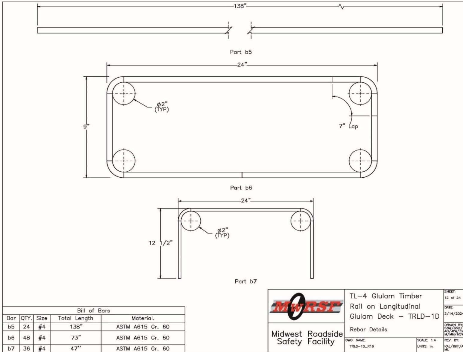
Figure 254. Rebar Details, Test No. TRLD-1
