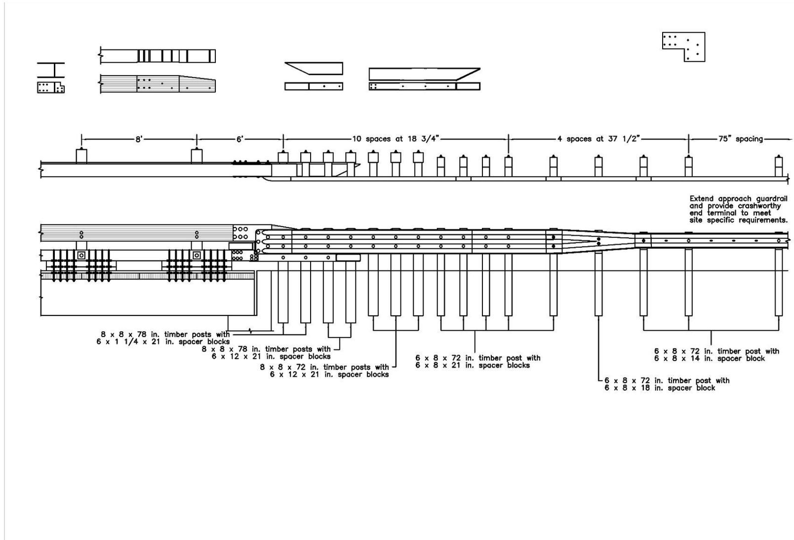
Figure K-32. Option 6.1 – Quarter-Post Spacing, 6-ft Gap, L-Plate, Removed Blockout, Steel Reverse Taper, Steel Curb Taper
