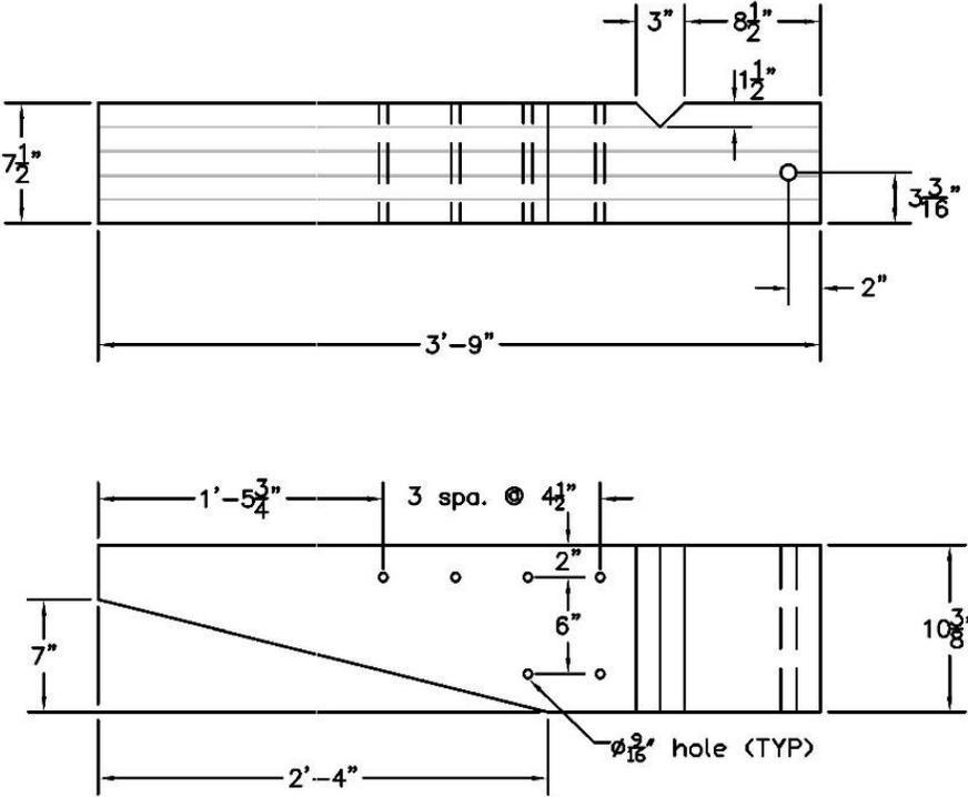
Figure 118. Reverse Taper Details for Quarter-Post System
