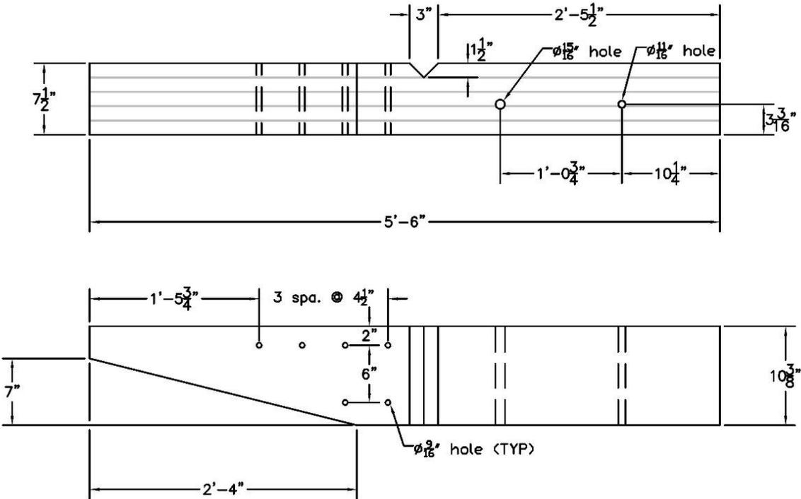
Figure 117. Reverse Taper Details for Half-Post System
