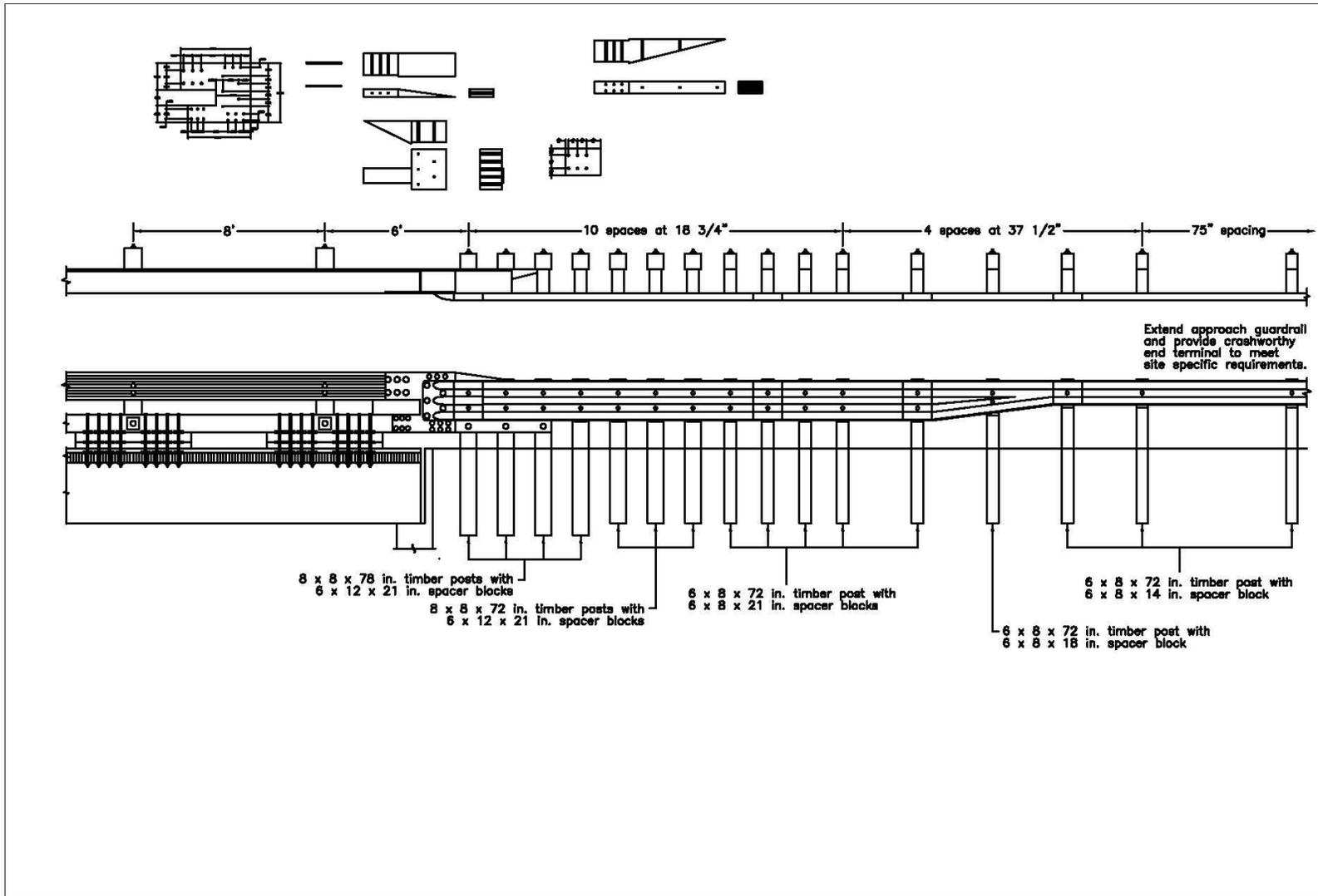
Figure K-1. Option 1.1 – Quarter-Post Spacing, 6-ft Gap, U-Plate, Removed Blockouts, Wood Reverse Taper, Thin Curb Taper
