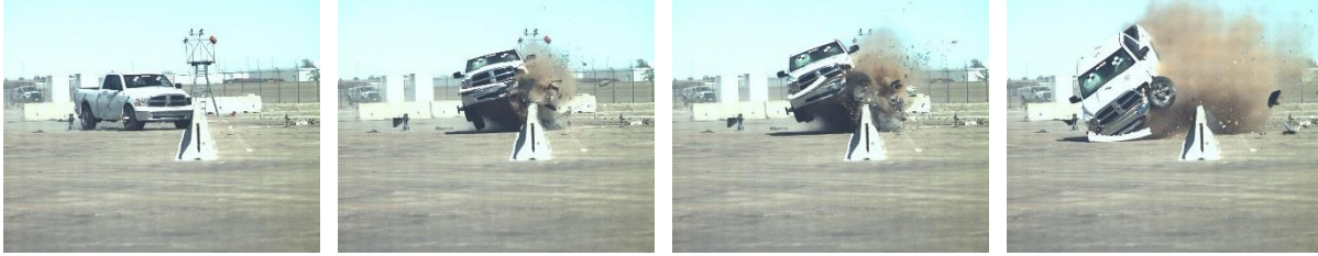
Figure 1. Vehicle Climb, Roll, and Pitch Motions with Safety-Shape Portable Concrete Barrier
