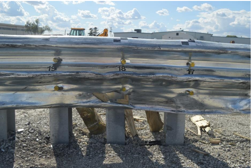
Figure 47. Thrie-Beam Damage, Test No. FLAGT-2
