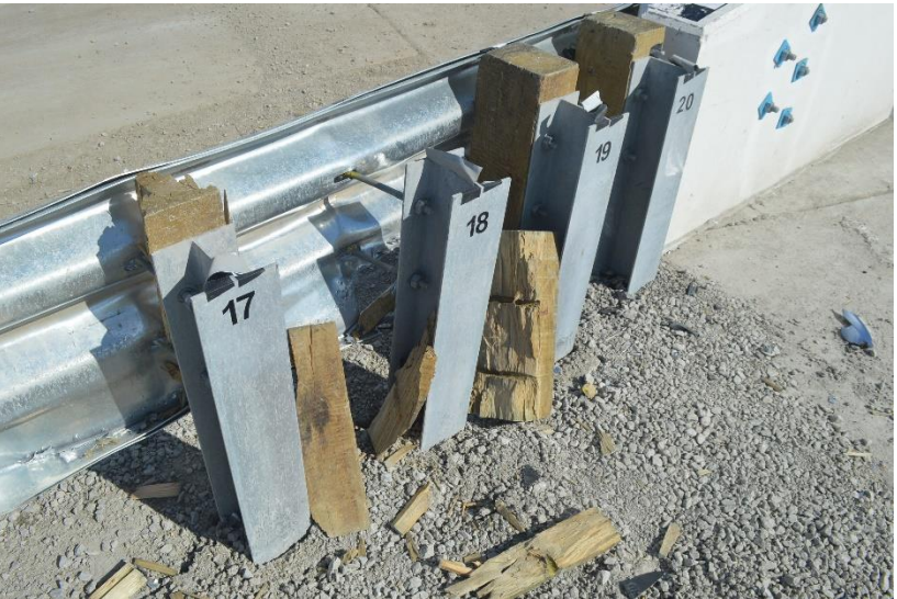
Figure 48. Post and Blockout Damage, Test No. FLAGT-2
