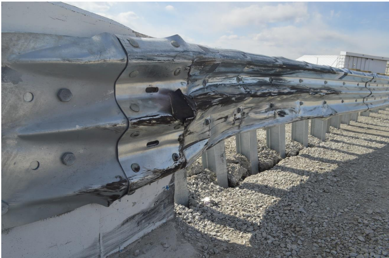
Figure 2. System Damage, Test No. FLAGT-1
