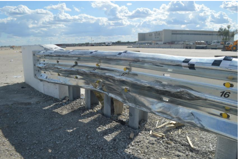
Figure 45. Overall System Damage, Test No. FLAGT-2
