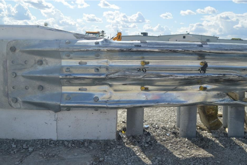
Figure 46. Concrete and Thrie-Beam Damage, Test No. FLAGT-2
