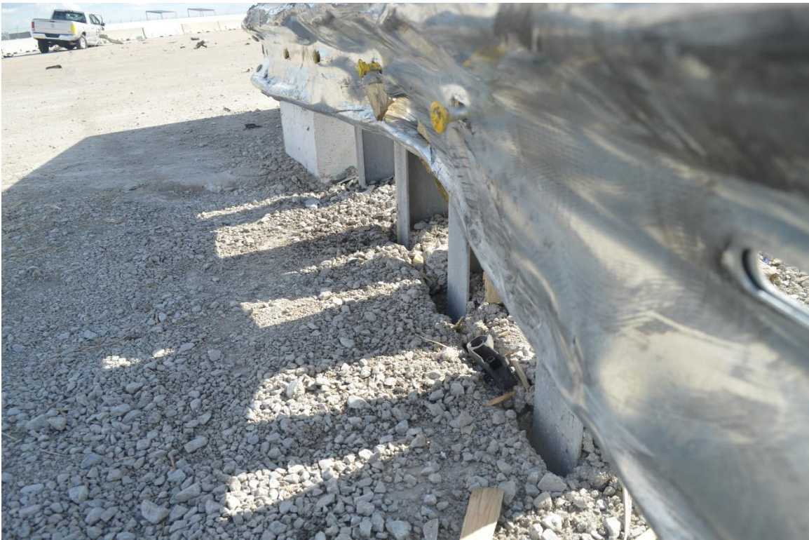
Figure 49. Soil Disturbance, Test No. FLAGT-2
