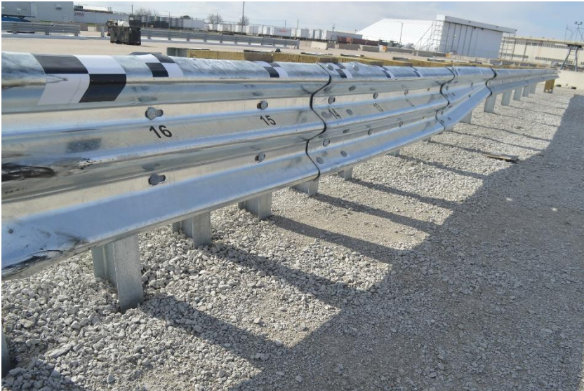
Figure 53. Post Nos. 15 through 17 Damage, Test No. FLAGT-1
