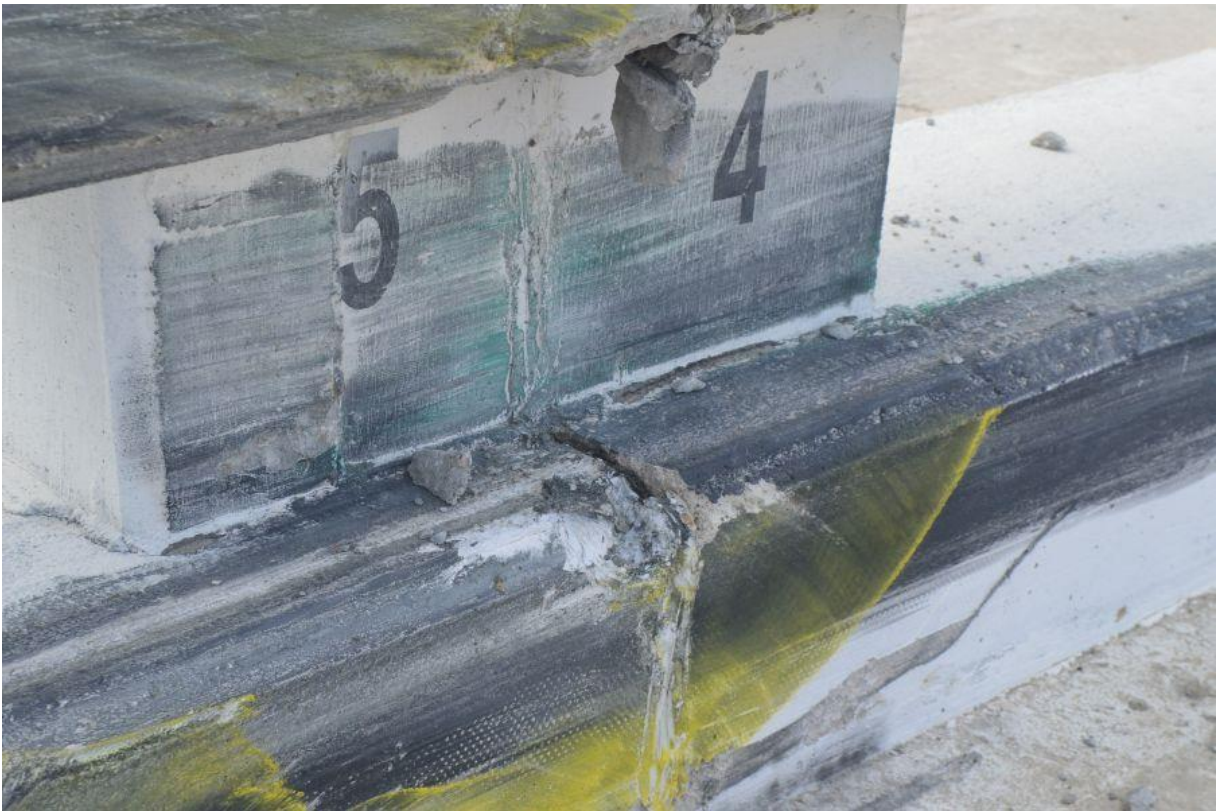
Figure 43. Curb and Concrete Rail Damage, Test No. HNTBR-2
