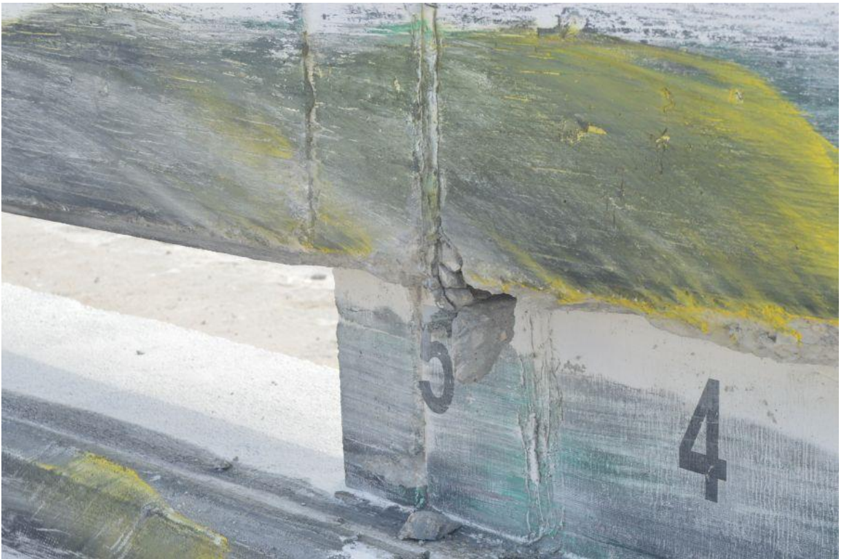
Figure 42. Curb and Concrete Rail Damage, Test No. HNTBR-2
