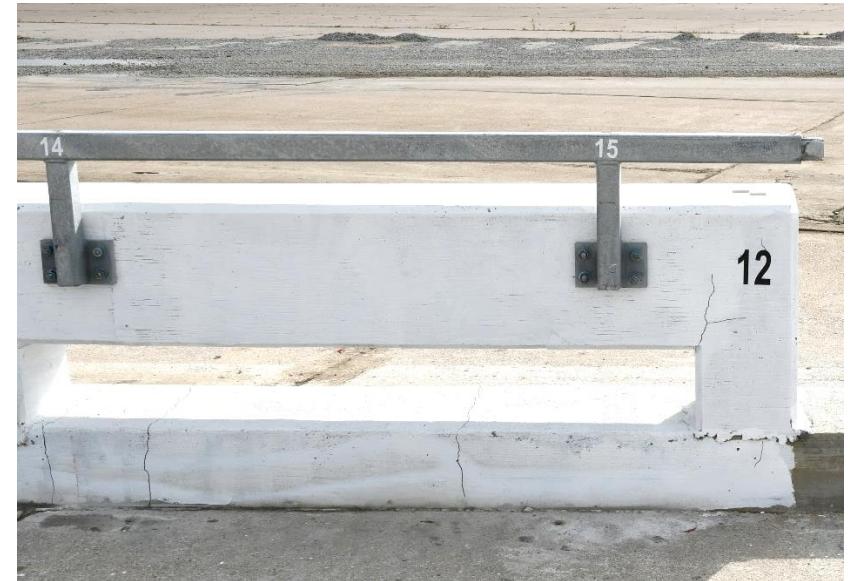
Figure 25. Test Installation Photographs, Handrail Assembly, Test Nos. HNTBR-2 and HNTBR-3
