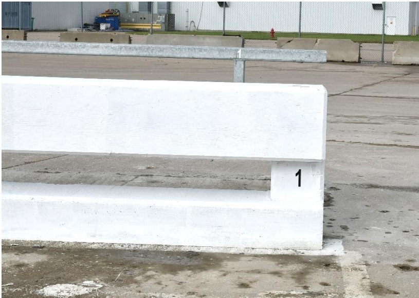
Figure 25. Test Installation Photographs, Handrail Assembly, Test Nos. HNTBR-2 and HNTBR-3
