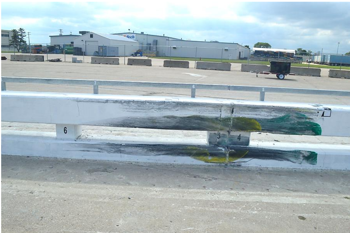
Figure 41. System Damage, Test No. HNTBR-2
