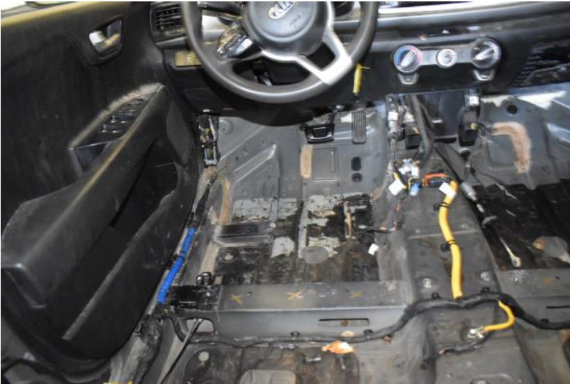
Figure 62. Vehicle's Interior Compartment Damage, Test No. HNTBR-3
