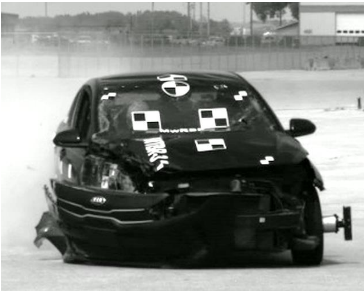
Figure 60. Vehicle Damage before Secondary Impact, Test No. HNTBR-3
