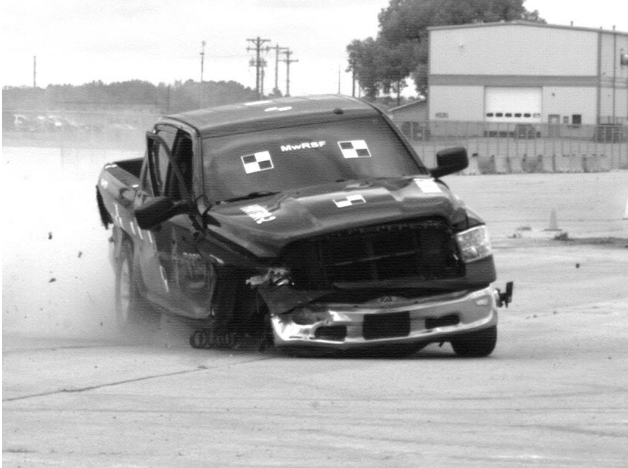
Figure 45. Vehicle Damage before Secondary Impact, Test No. HNTBR-2
