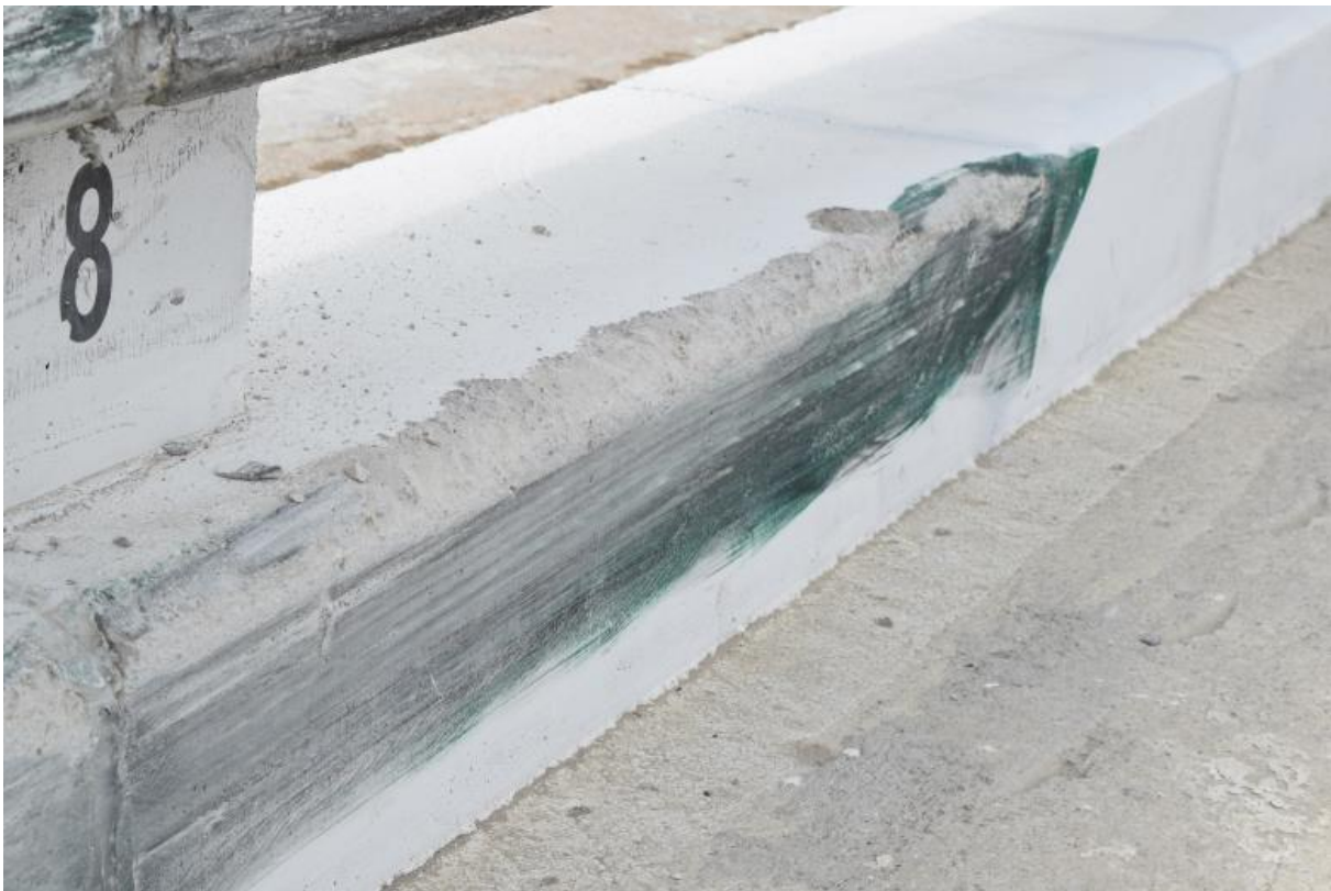
Figure 58. Curb and Concrete Rail Damage, Test No. HNTBR-3
