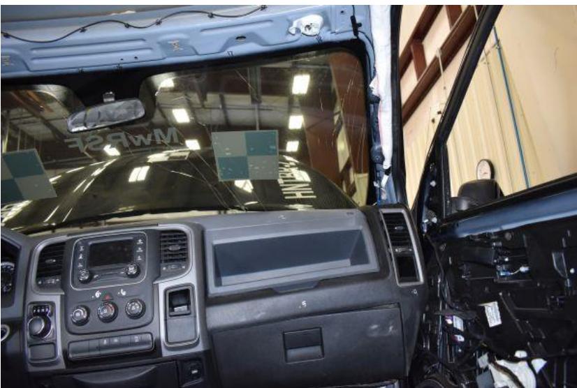
Figure 48. Vehicle's Floor Pan and Interior Compartment Damage, Test No. HNTBR-2
