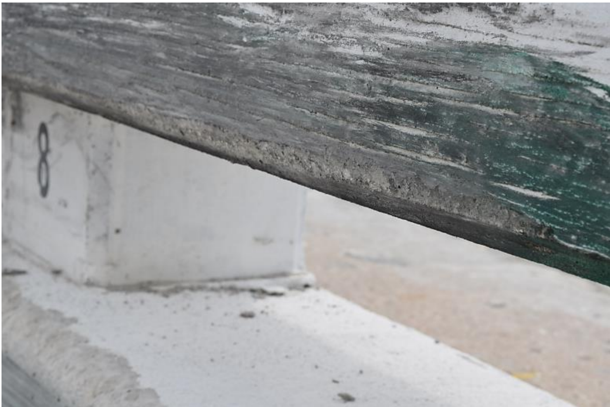
Figure 57. Curb and Concrete Rail Damage, Test No. HNTBR-3
