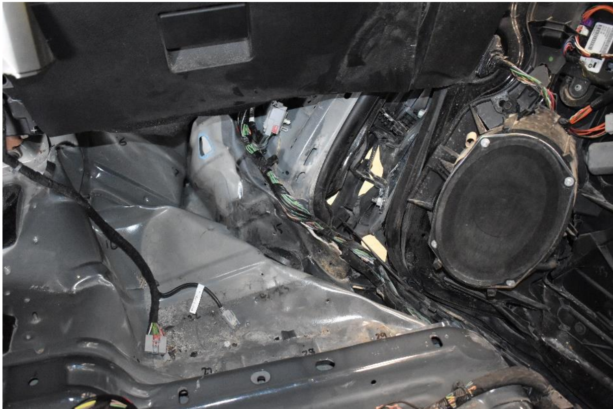
Figure 5. Vehicle Damage and Excessive Wheel and Toe Pan Intrusion – Test No. HNTBR-1
