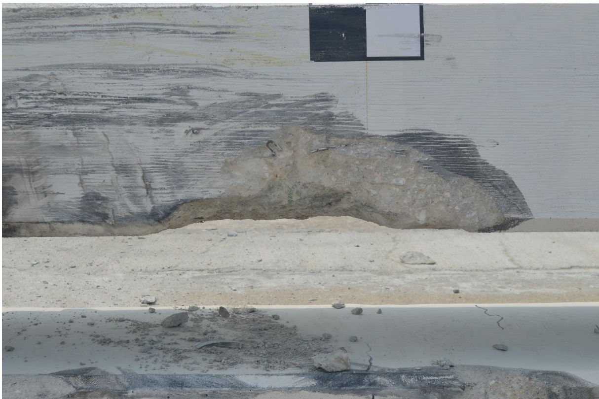
Figure 28. Curb and Concrete Rail Damage, Test No. HNTBR-1
