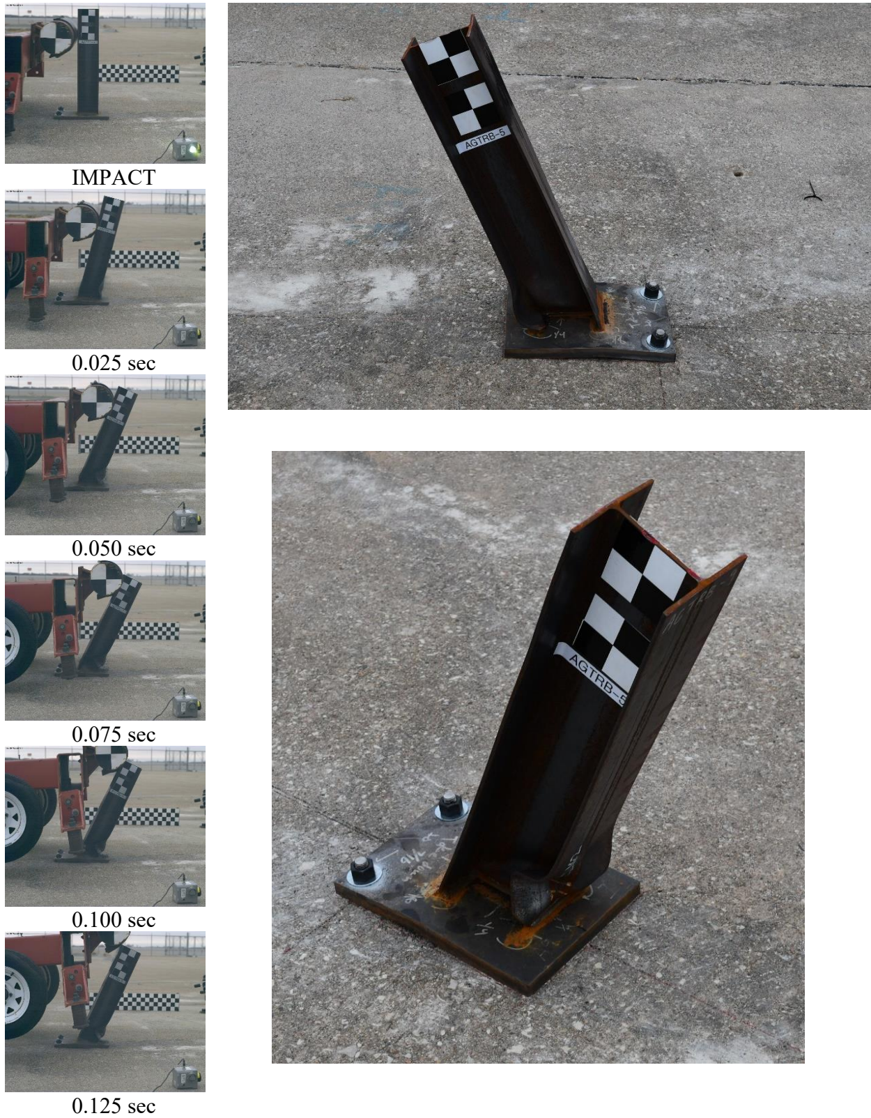
Figure 32. Time-Sequential and Post-Impact Photographs, Test No. AGTRB-5
