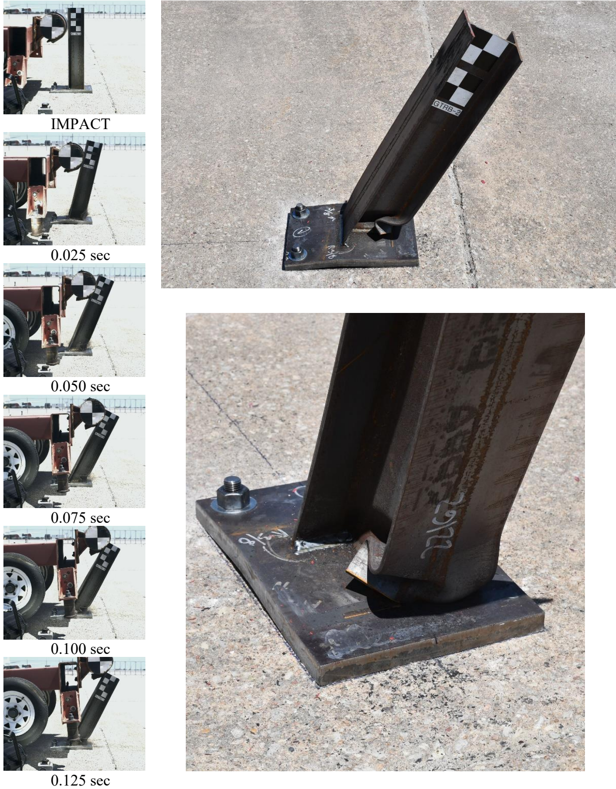
Figure 26. Time-Sequential and Post-Impact Photographs, Test No. AGTRB-2
