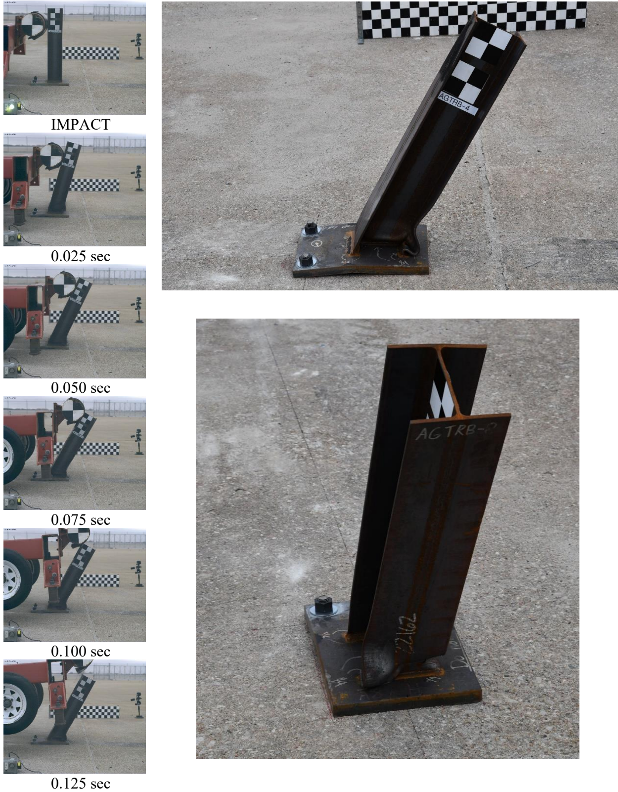
Figure 30. Time-Sequential and Post-Impact Photographs, Test No. AGTRB-4
