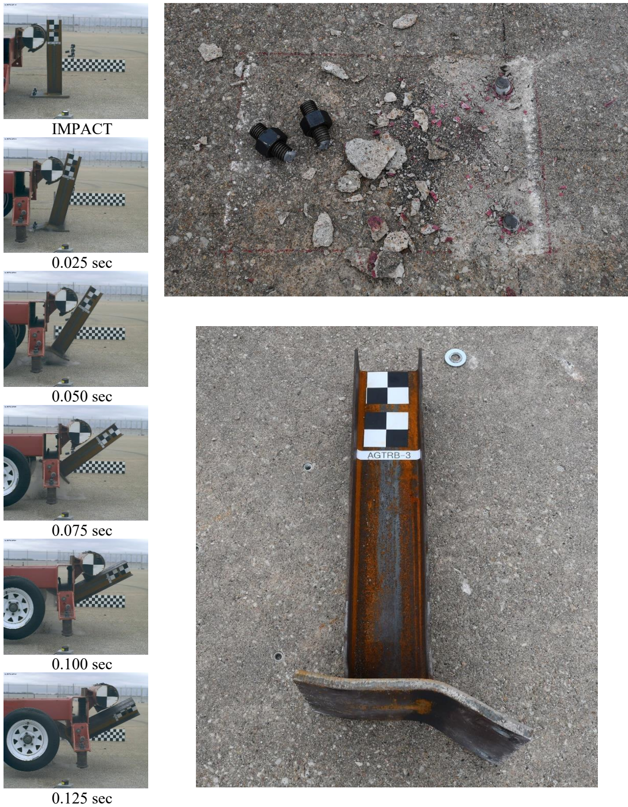
Figure 28. Time-Sequential and Post-Impact Photographs, Test No. AGTRB-3
