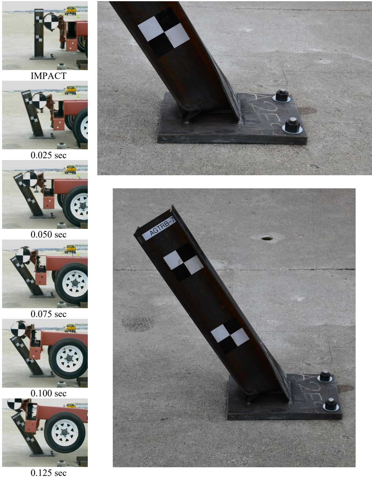
Figure 48. Time-Sequential and Post-Impact Photographs, Test No. AGTRB-7
