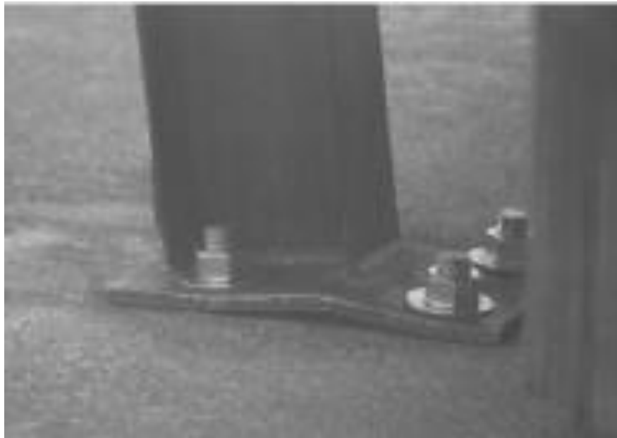
Figure 8. Base Plate Bending Allowing Post Rotation
