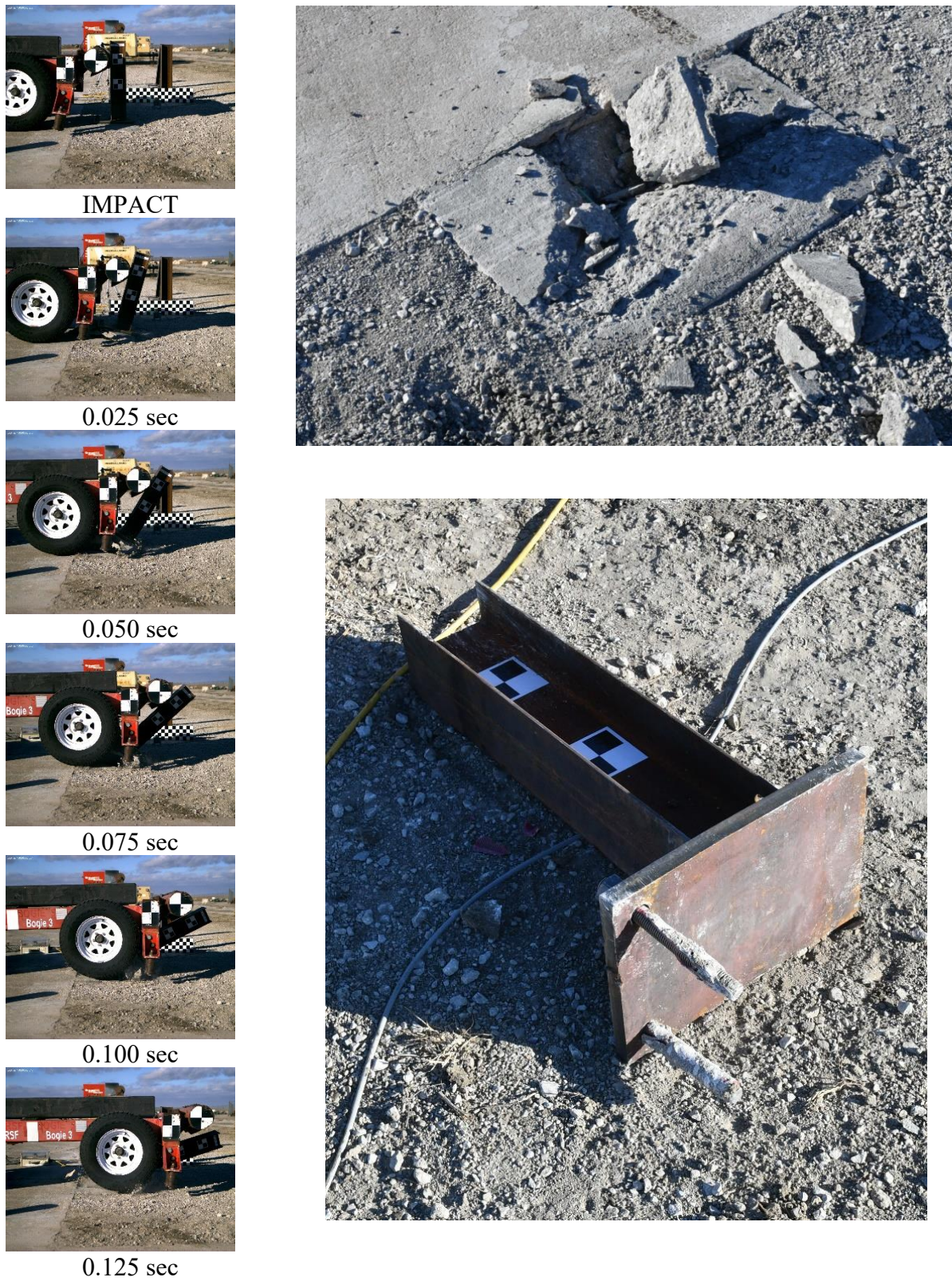
Figure 60. Time-Sequential and Post-Impact Photographs, Test No. AGTRB-8
