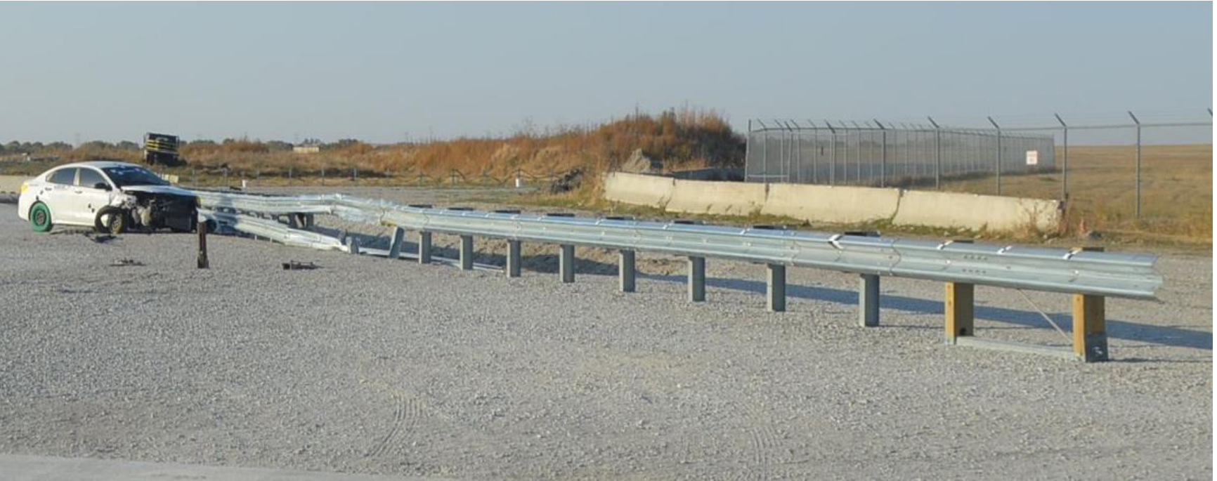
Figure 97. Overall System Damage Test No. HBIB-7
