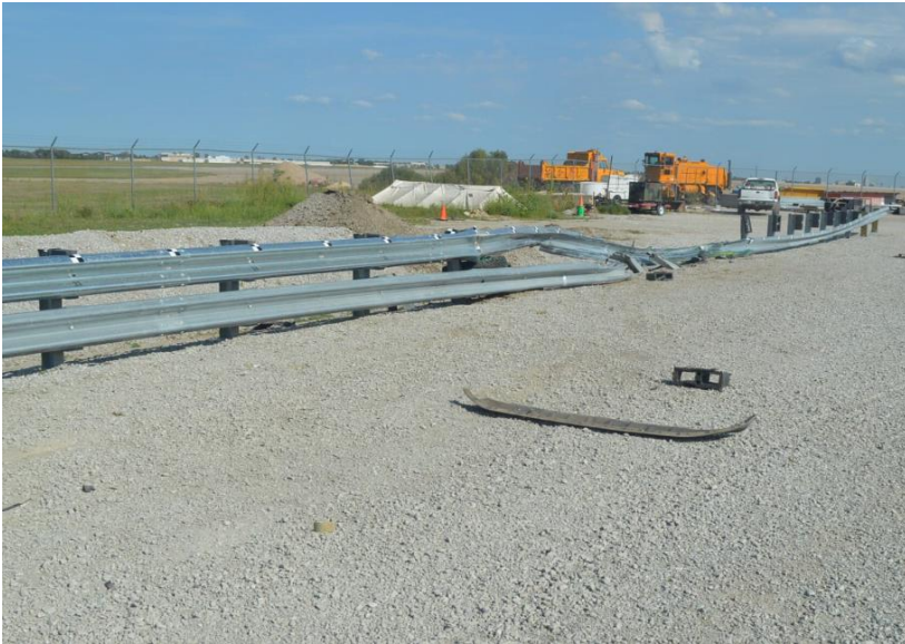
Figure 82. System Damage, Test No. HBIB-6
