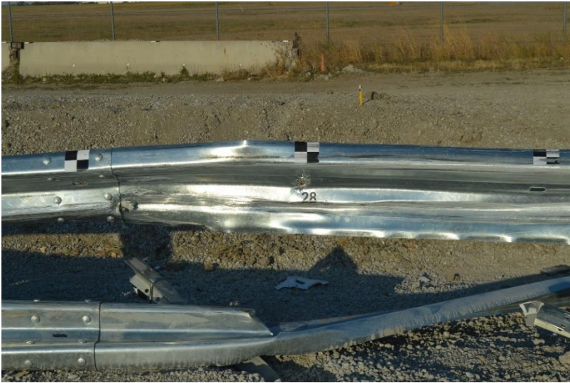
Figure 99. Upper Rail and Rubrail Damage Test No. HBIB-7
