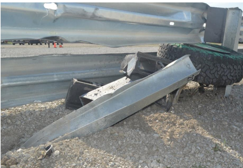
Figure 85. Post Damage, Post Nos. 26 (top left), 27 (bottom left), 28 (top right), and 29 (bottom right), Test No. HBIB-6
