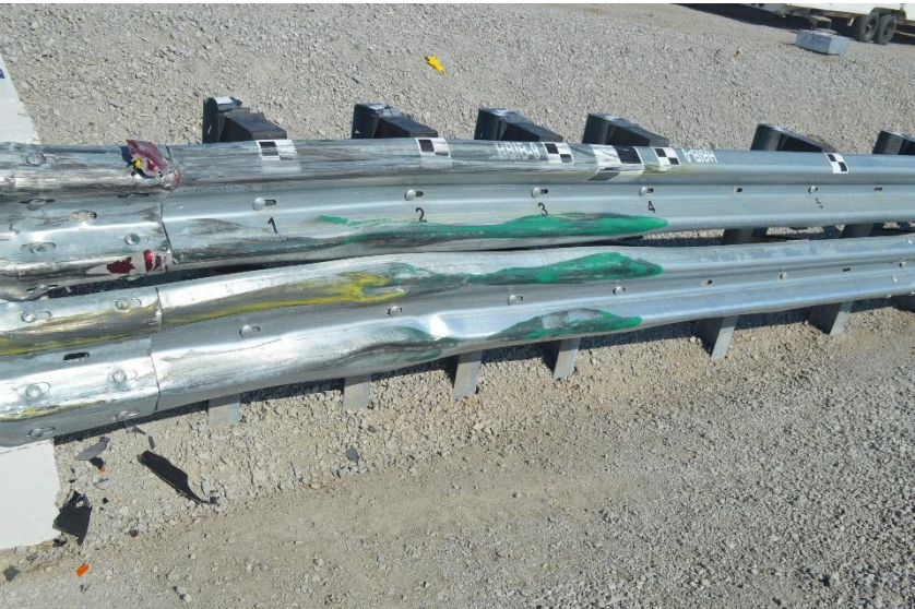
Figure 178. Upper Rail and Rub Rail Damage, Test No. HBIB-9
