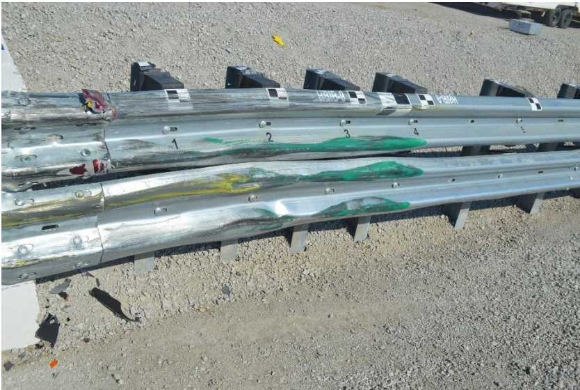
Figure 111. Upper Rail and Rub rail Damage, Test No. HBIB-8
