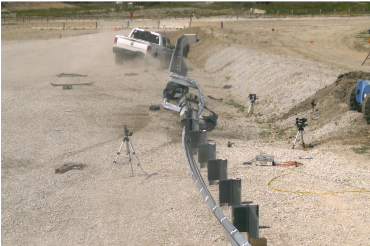
Figure 80. Vehicle Final Position and Trajectory Marks, Test No. HBIB-6
