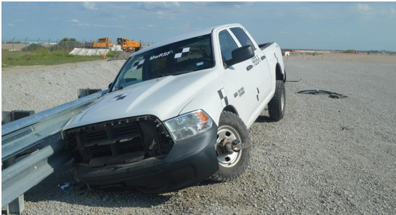
Figure 88. Vehicle Damage, Test No. HBIB-6
