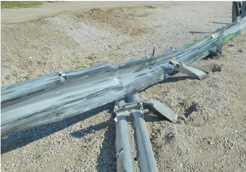
Figure 84. Post Damage Test No. HBIB-6
