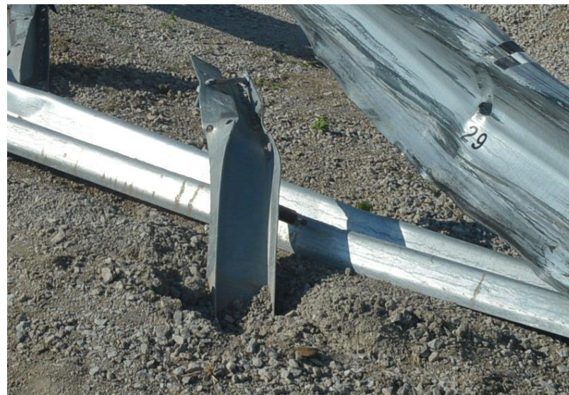
Figure 85. Post Damage, Post Nos. 26 (top left), 27 (bottom left), 28 (top right), and 29 (bottom right), Test No. HBIB-6
