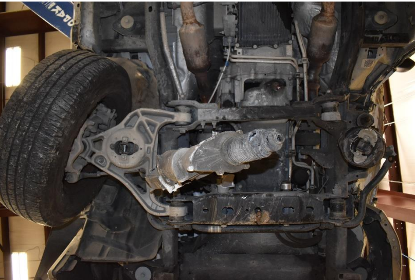
Figure 116. Test Vehicle's Interior Floorboards and Undercarriage Damage, Test No. HBIB-8
