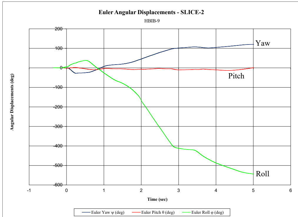
Figure K-15. Vehicle Angular Displacements (SLICE-2), Test No. HBIB-9
