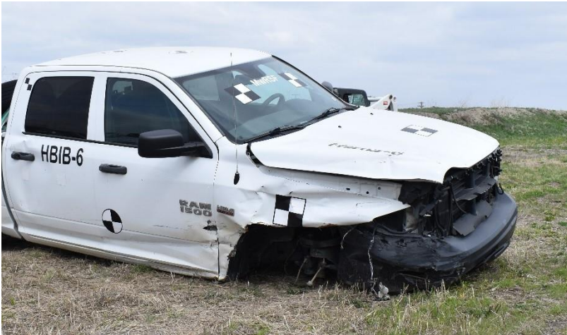
Figure 89. Vehicle Damage, Test No. HBIB-6
