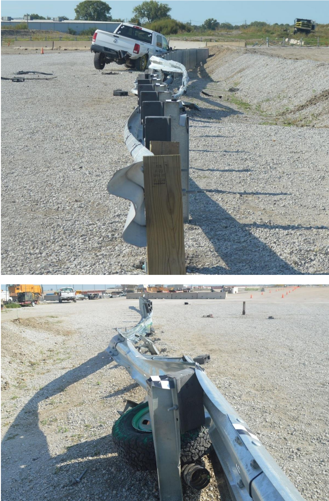
Figure 81. System Damage, Test No. HBIB-6
