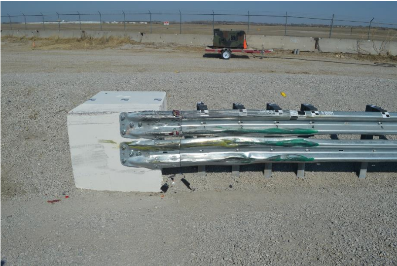
Figure 110. System Damage, Test No. HBIB-8
