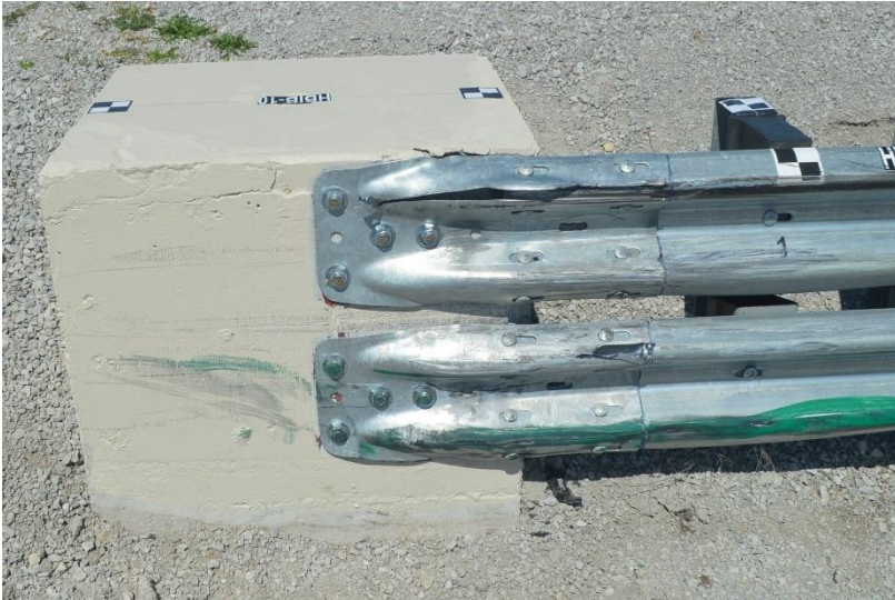
Figure 125. System Damage, Test No. HBIB-10
