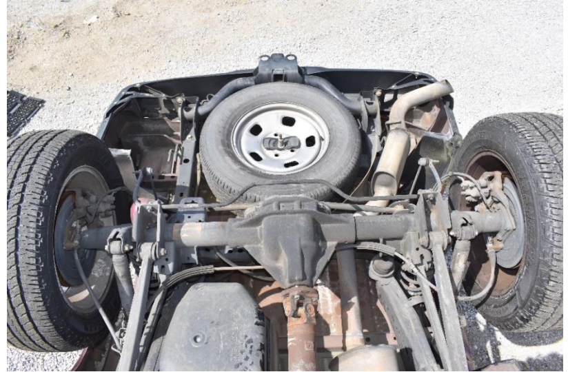
Figure 182. Test Vehicle's Interior Floorboards and Undercarriage Damage, Test No. HBIB-9
