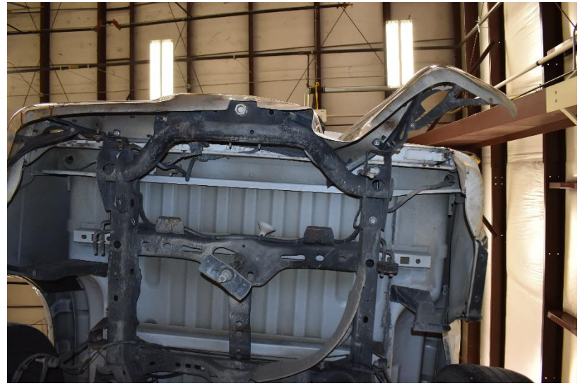
Figure 116. Test Vehicle's Interior Floorboards and Undercarriage Damage, Test No. HBIB-8
