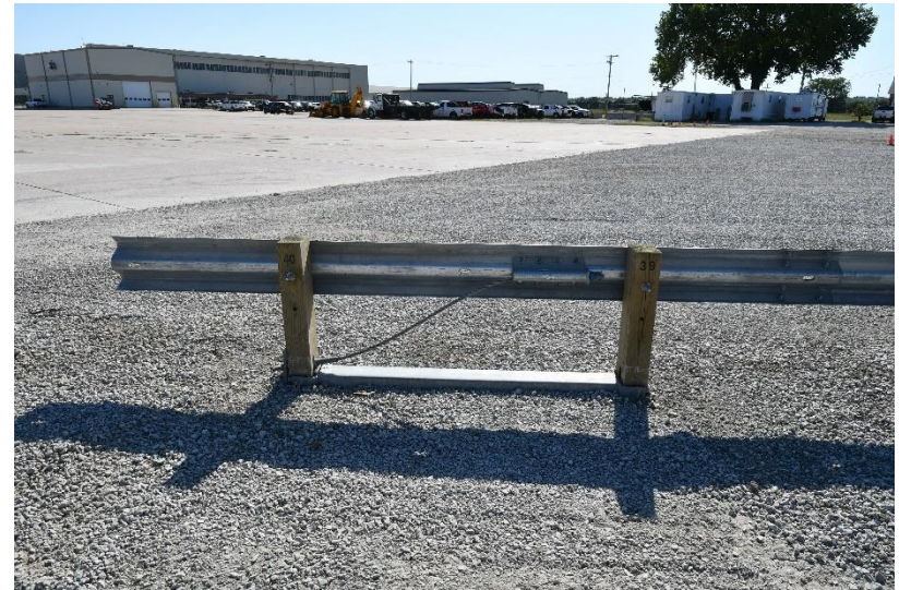
Figure 169. Test Installation Photographs, Rubrail Termination and System Anchorage, Test No. HBIB-9
