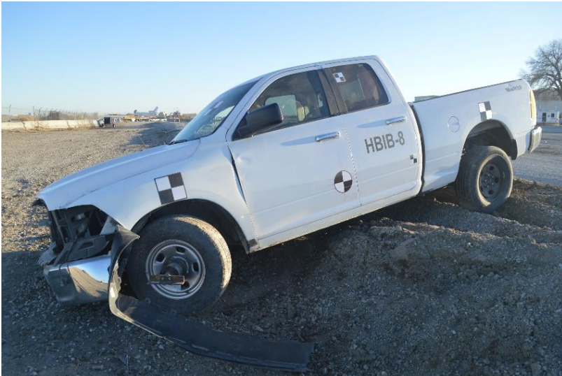
Figure 113. Vehicle Damage, Test No. HBIB-8
