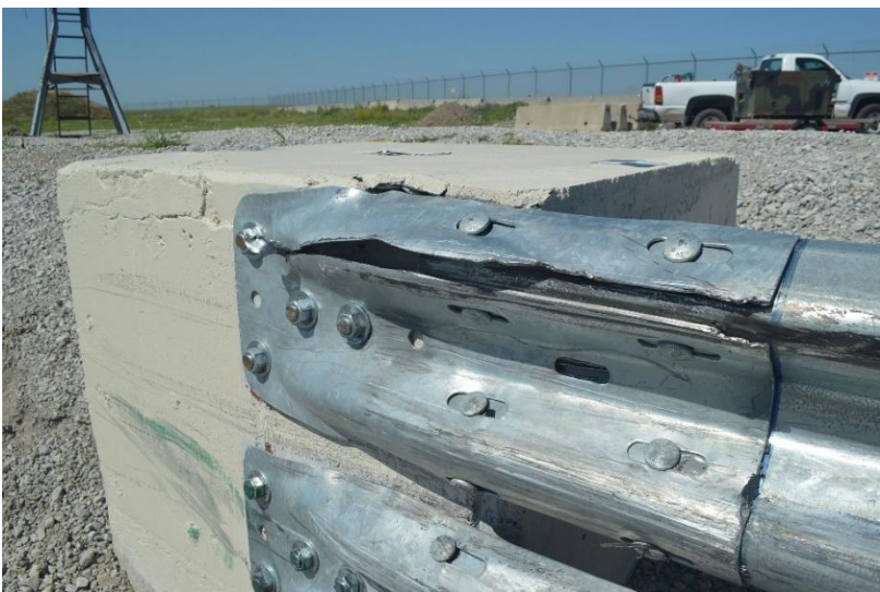
Figure 126. Upper Rail and Rub Rail Damage, Test No. HBIB-10
