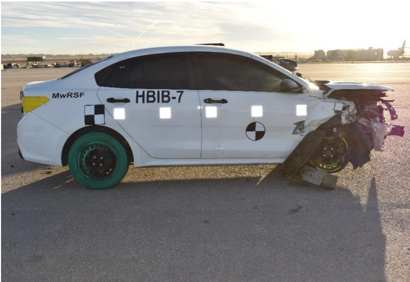
Figure 102. Vehicle Damage, Test No. HBIB-7
