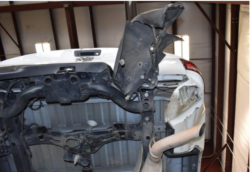
Figure 90. Test Vehicle's Interior Floorboards and Undercarriage Damage, Test No. HBIB-6
