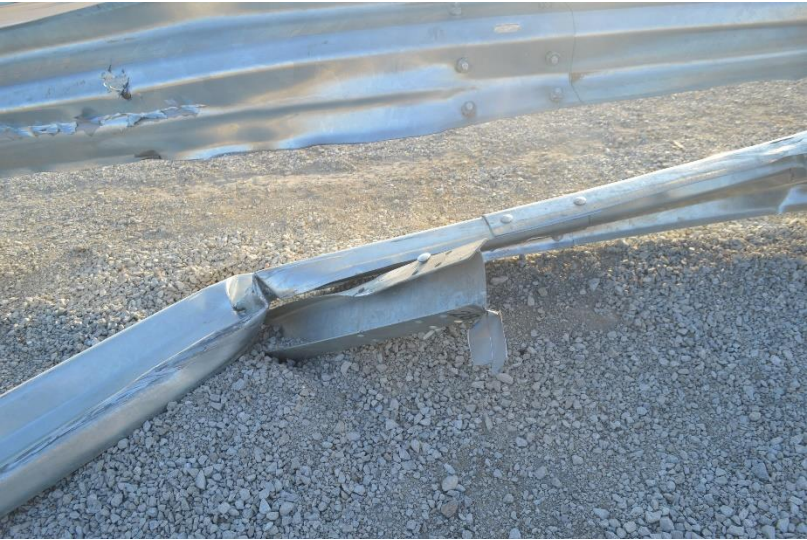
Figure 100. Post Damage, Post Nos. 27 through 30, Test No. HBIB-7
