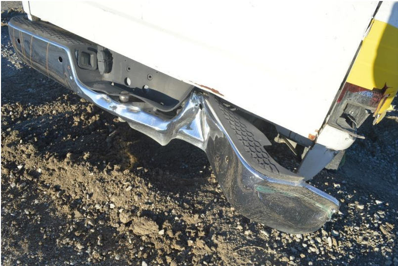
Figure 115. Vehicle Damage, Test No. HBIB-8
