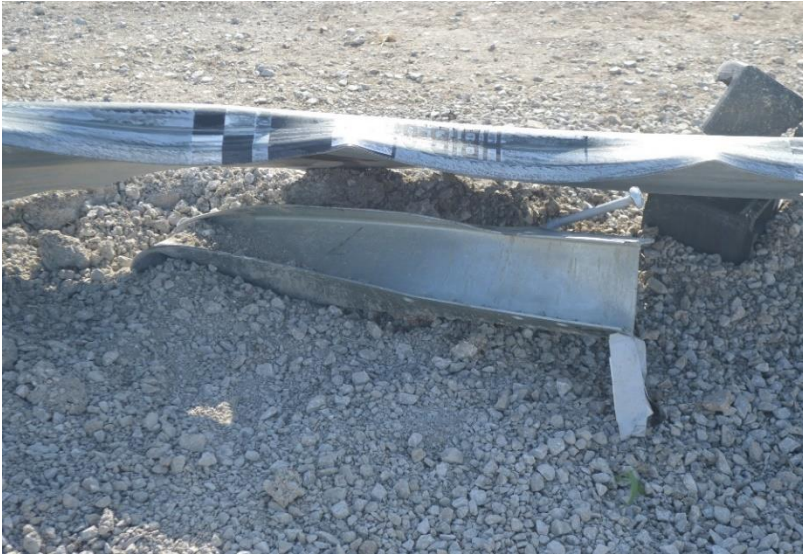
Figure 86. Post Damage, Post Nos. 30 through 33, Test No. HBIB-6
