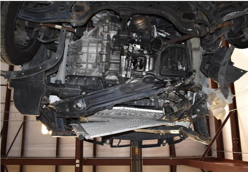
Figure 103. Test Vehicle's Interior Floorboards and Undercarriage Damage, Test No. HBIB-7
