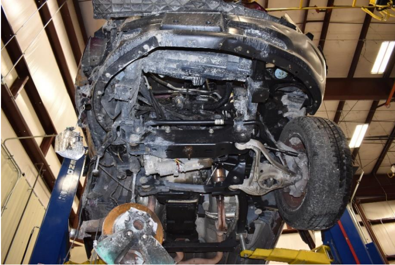
Figure 182. Test Vehicle's Interior Floorboards and Undercarriage Damage, Test No. HBIB-9
