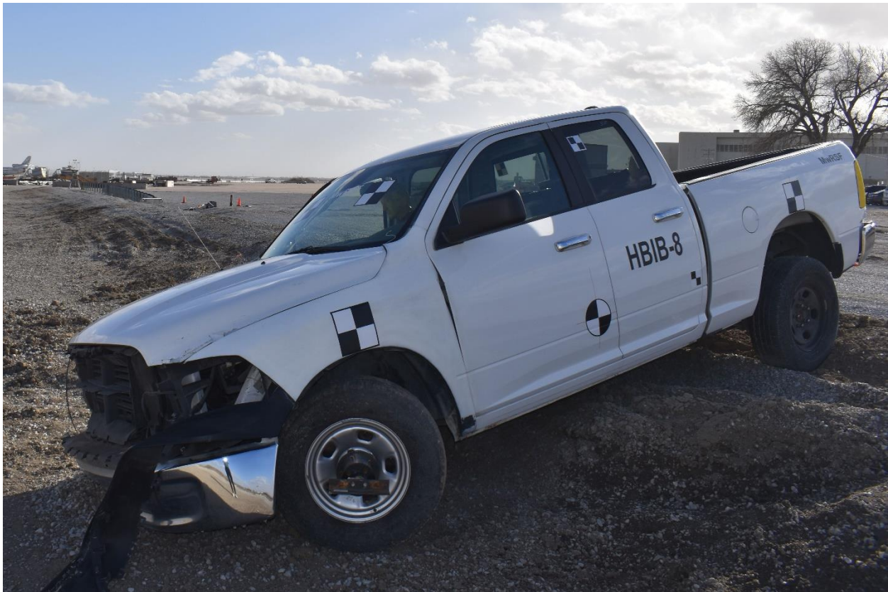
Figure 109. Vehicle Final Position and Trajectory Marks, Test No. HBIB-8
