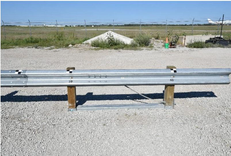
Figure 169. Test Installation Photographs, Rubrail Termination and System Anchorage, Test No. HBIB-9
