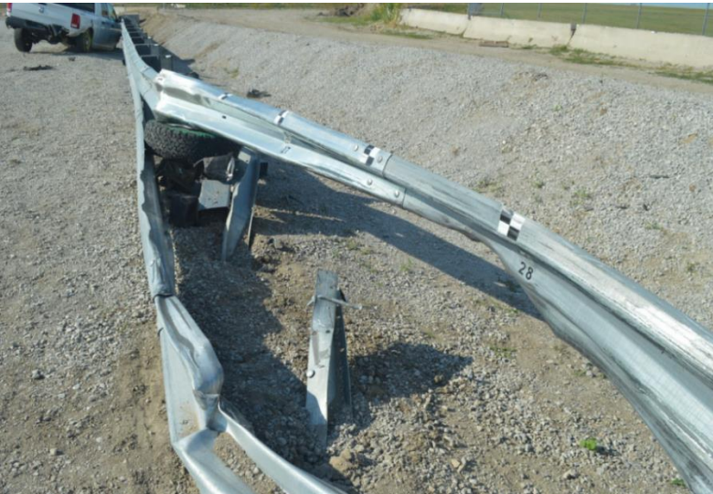
Figure 83. Upper Rail and Rubrail Damage Test No. HBIB-6
