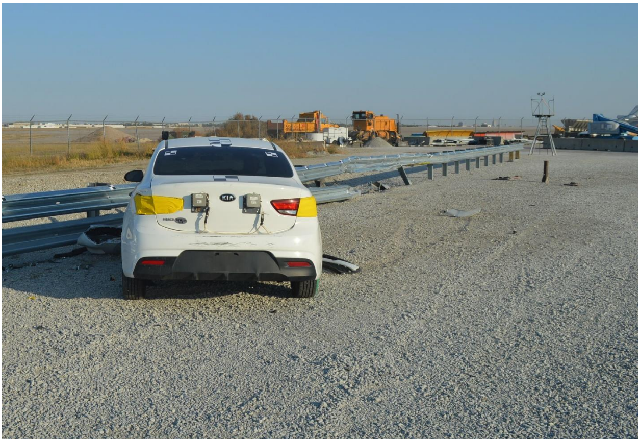
Figure 96. Vehicle Final Position and Trajectory Marks, Test No. HBIB-7
