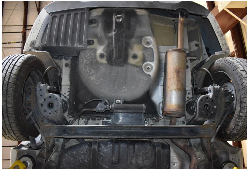
Figure 103. Test Vehicle's Interior Floorboards and Undercarriage Damage, Test No. HBIB-7
