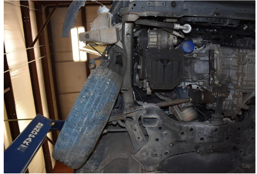
Figure 130. Test Vehicle's Interior Floorboards and Undercarriage Damage, Test No. HBIB-10
