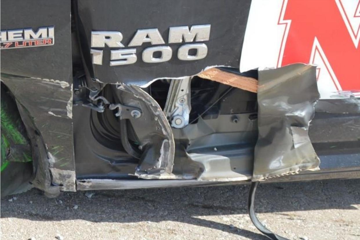
Figure 77. Left-Front Door Snag, Test No. WITD-4
