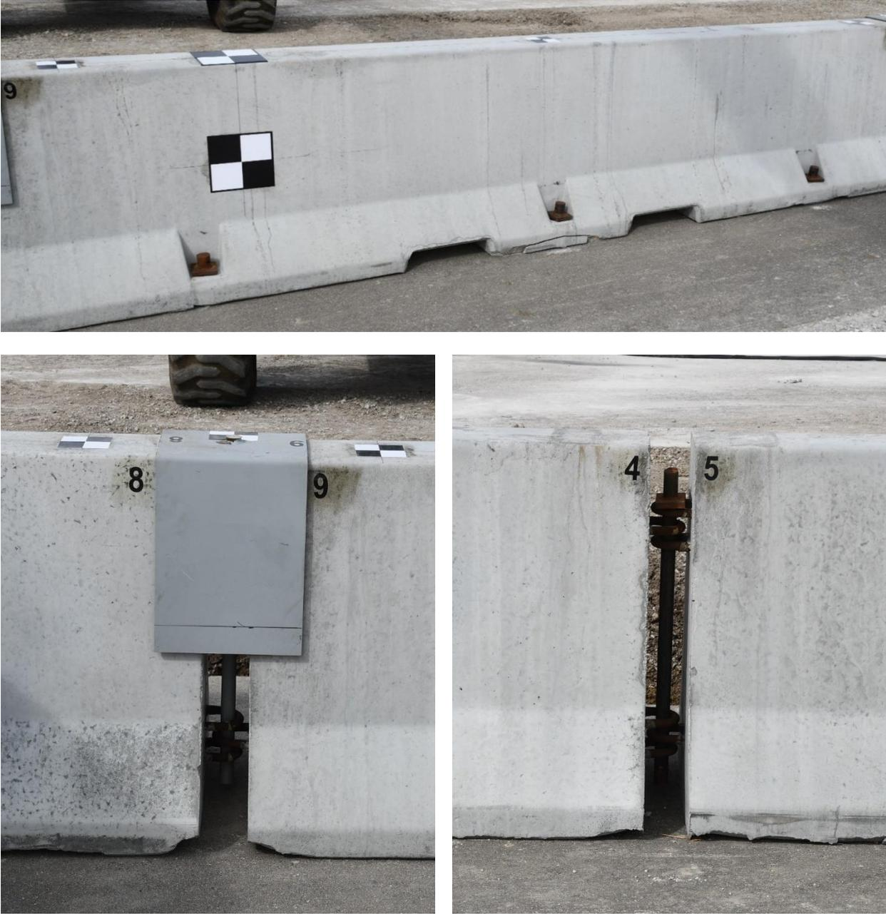
Figure 61. Test Installation Photographs: Anchor (top), Saddle Cap (bottom left) and Connection Pin (bottom right) Details, Test No. WITD-4
