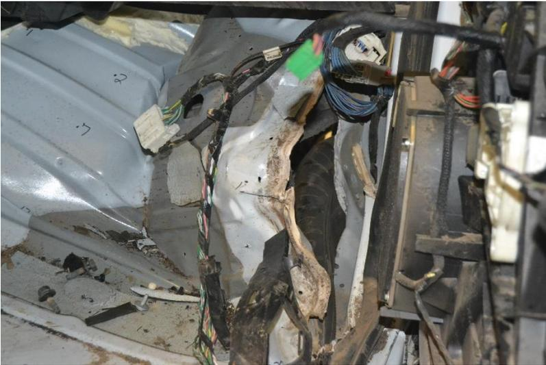
Figure 5. Occupant Compartment Damage, Test No. WITD-3
