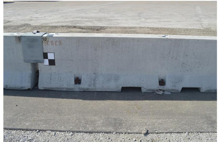
Figure 70. System Damage, Barrier Nos. 9 and 10, Test No. WITD-4
