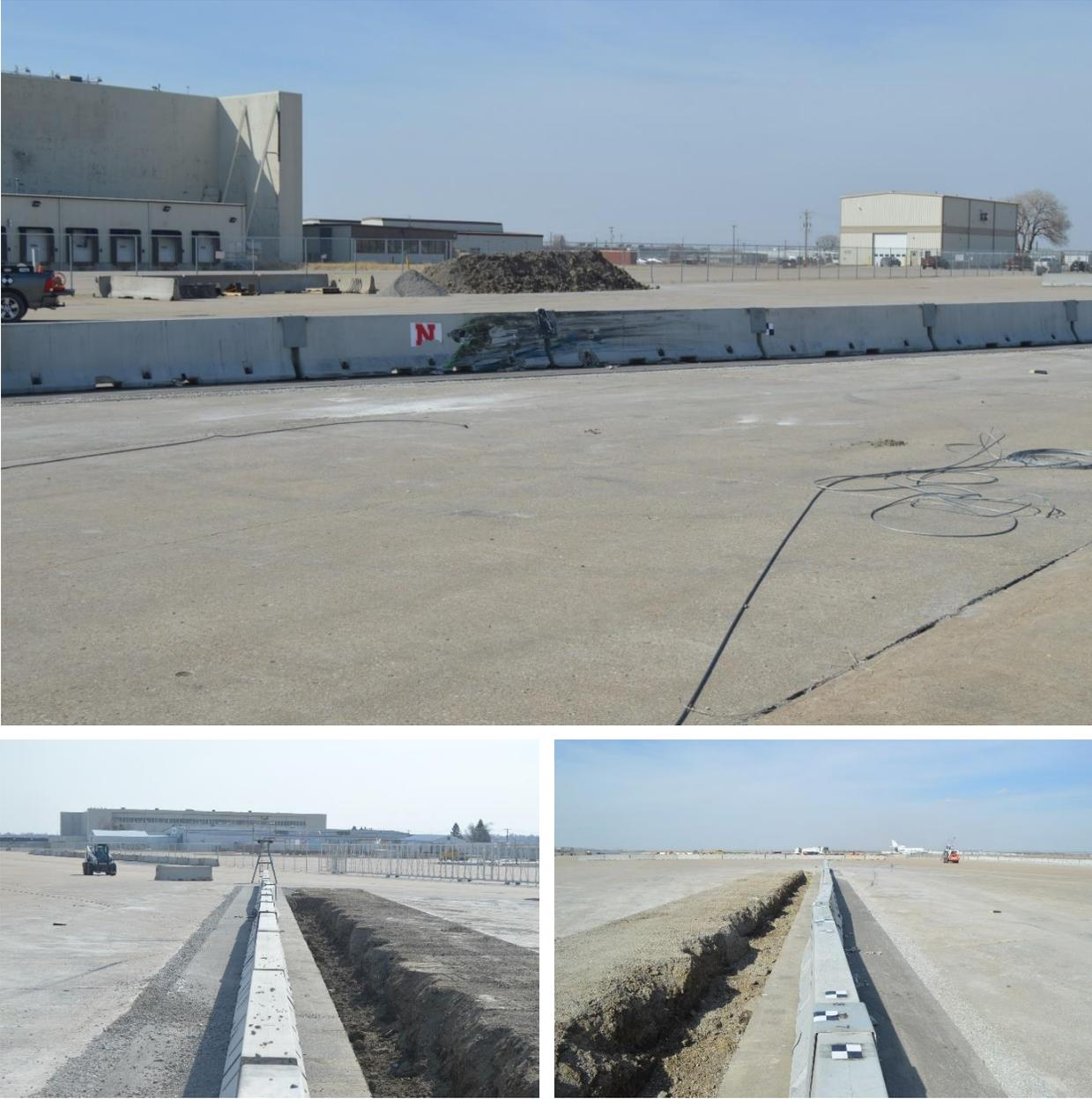
Figure 68. Overall System Damage, Test No. WITD-4
