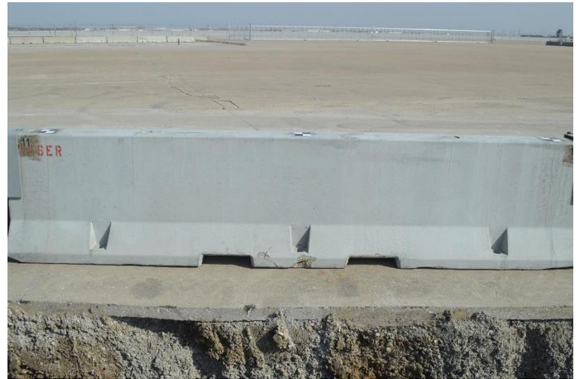
Figure 71. System Damage, Non-Traffic Side, Barrier Nos. 7 through 11, Test No. WITD-4
