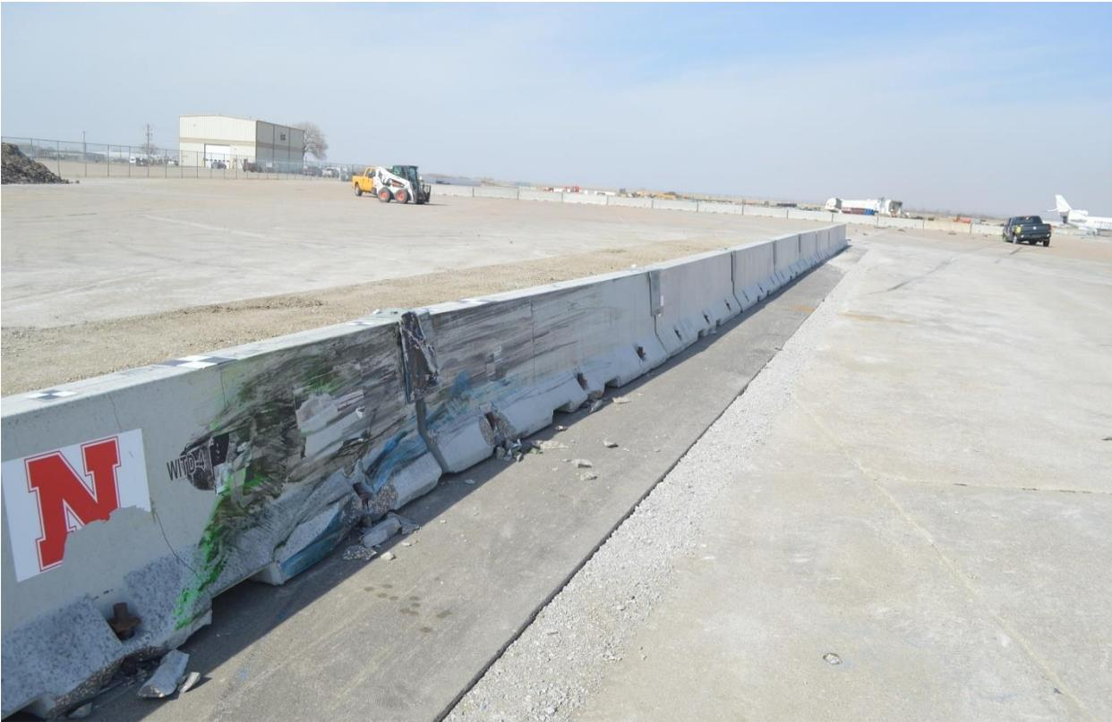
Figure 67. Vehicle Final Position and Trajectory Marks, Test No. WITD-4
