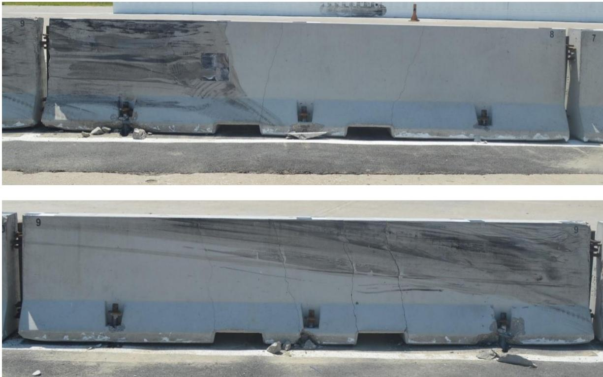
Figure 27. Barrier Nos. 8 and 9 Damage, Test No. WITD-3
