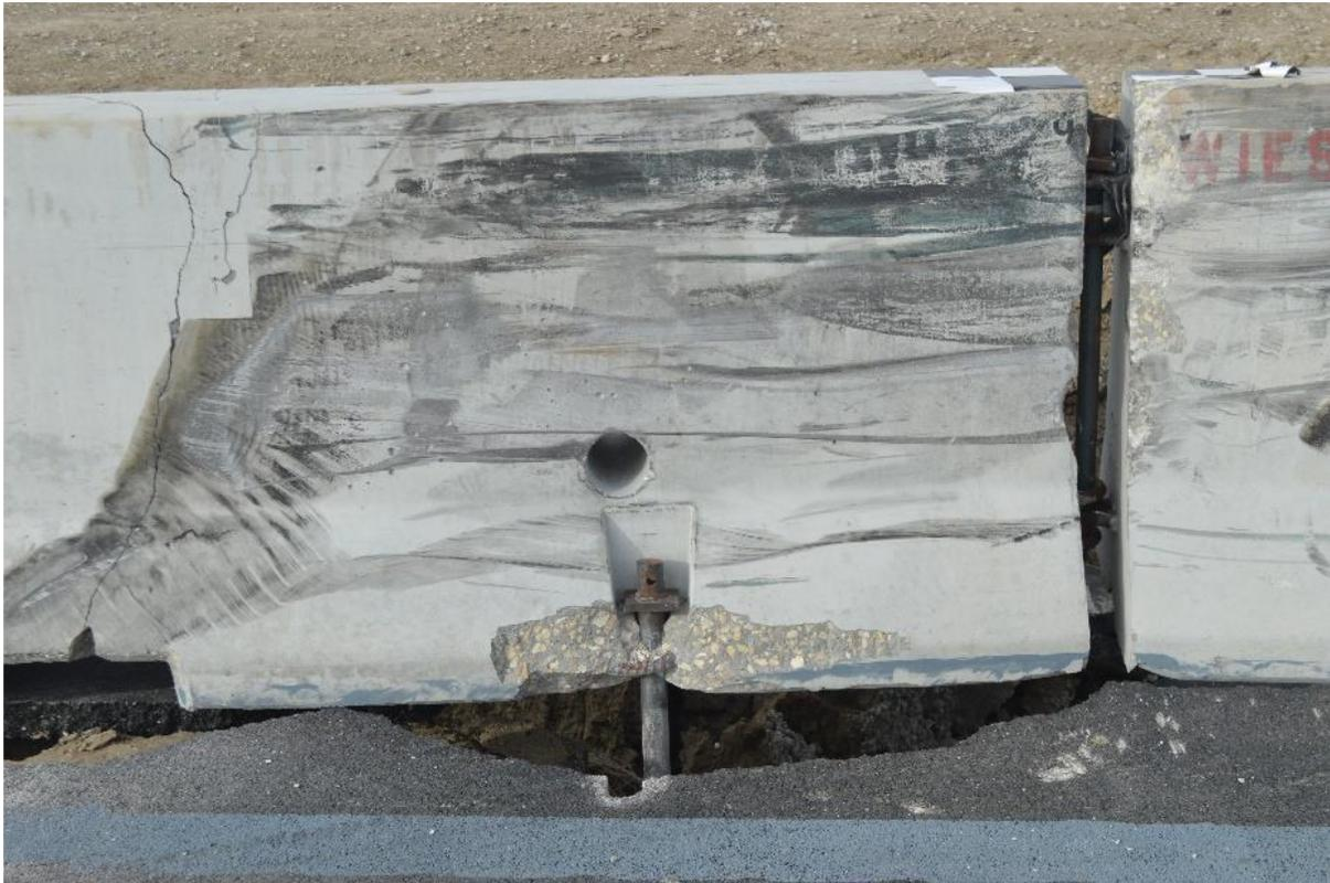
Figure 2. Barrier Joint Snag, Test No. WITD-3
