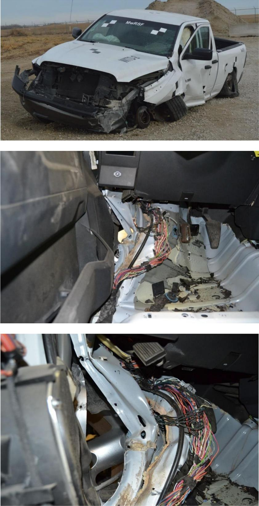
Figure 3. Occupant Compartment Damage, Test No. WITD-2
