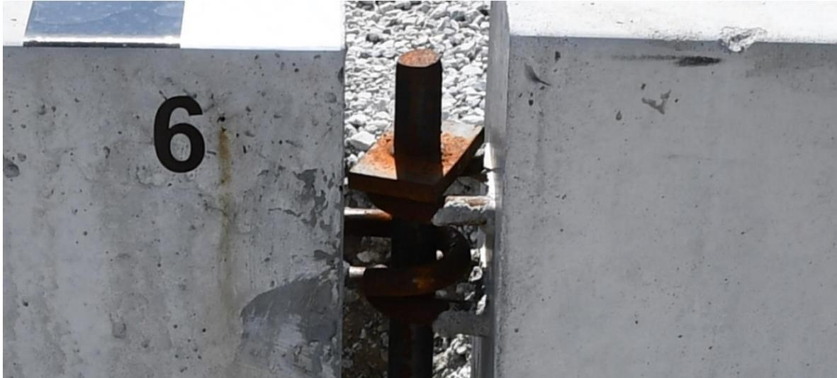
Figure 28. Gap Between Connection Loop and Pin, Test No. WITD-3
