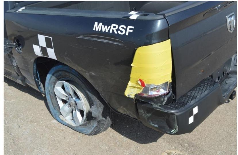
Figure 74. Vehicle Damage, Test No. WITD-4
