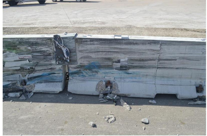
Figure 69. System Damage at Impact Location, Barrier Nos. 8 and 9, Test No. WITD-4
