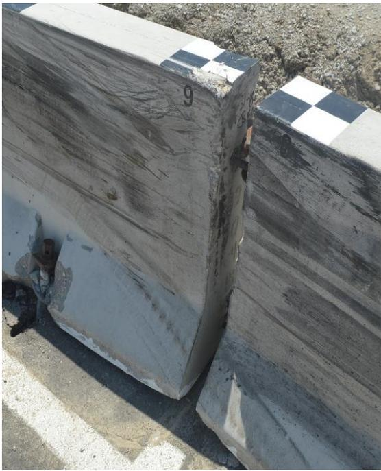
Figure 4. Barrier Joint Snag, Test No. WITD-3
