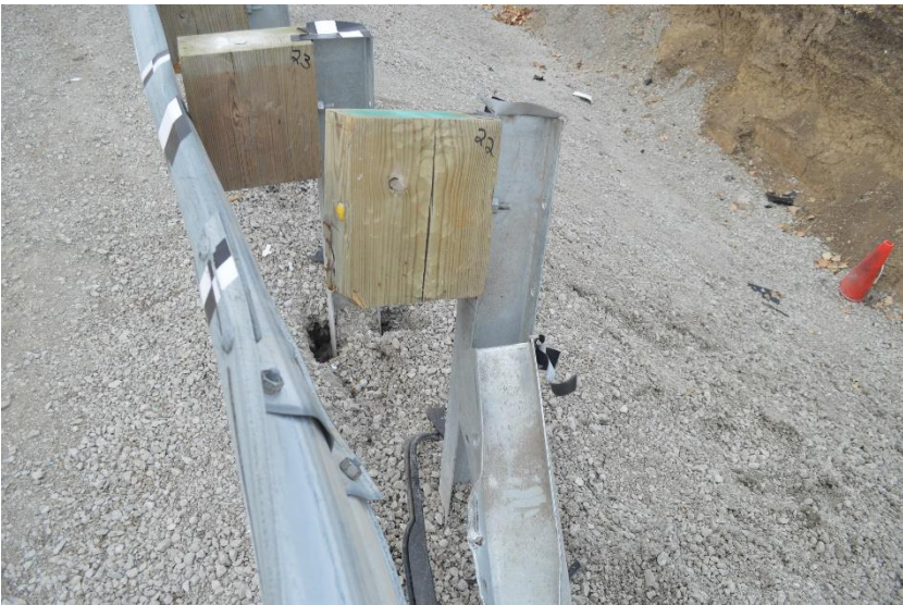
Figure 38. Damage to Post Nos. 21 and 22, Test No. MGS7S-1
