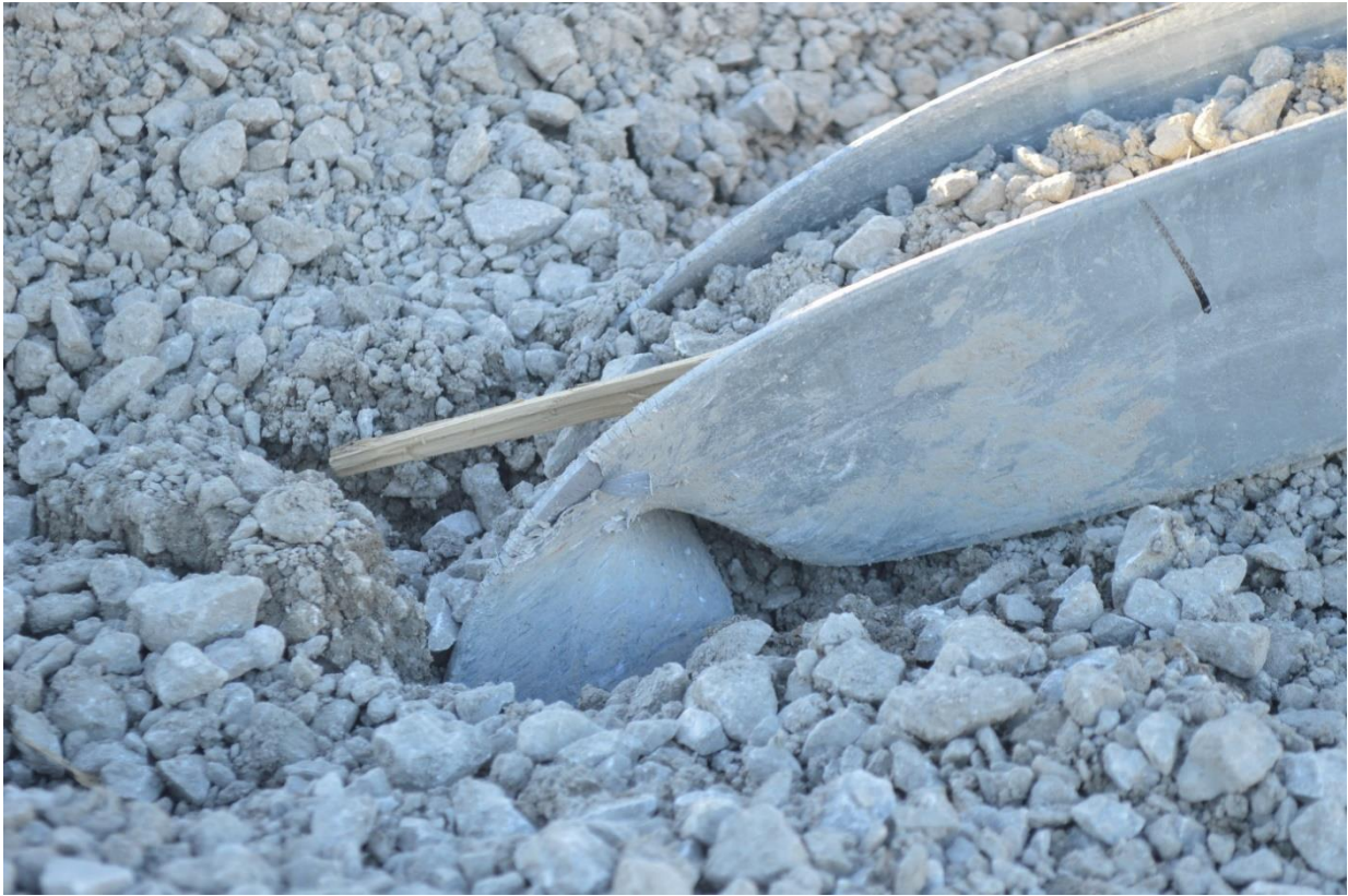
Figure 57. Blockout Damage and Post Buckling, Test No. MGS7S-2
