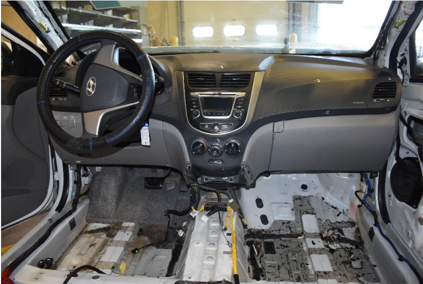
Figure 44. Vehicle Undercarriage and Occupant Compartment Damage, Test No. MGS7S-1
