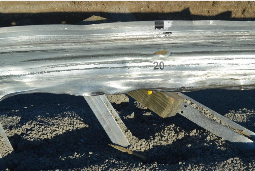
Figure 54. Damage to Post Nos. 19 and 20, Test No. MGS7S-2
