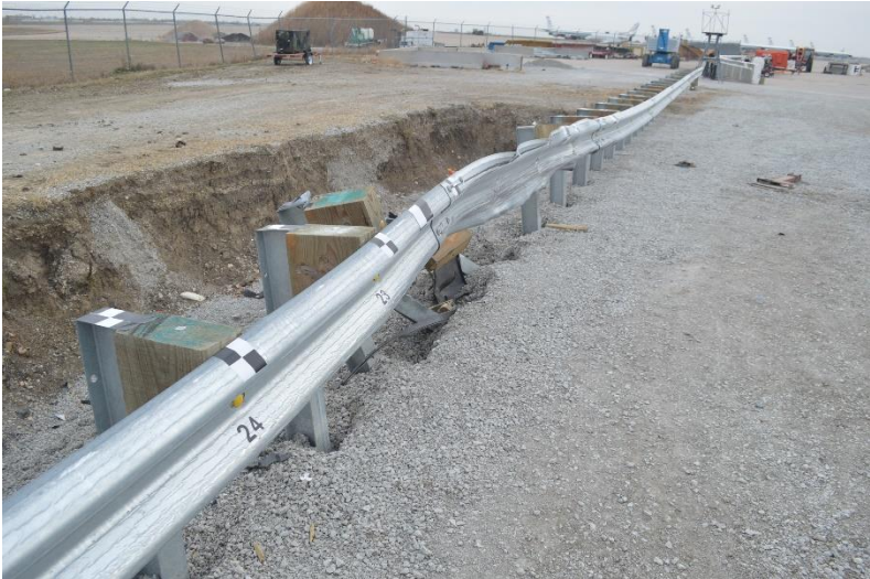
Figure 36. System Damage, Test No. MGS7S-1
