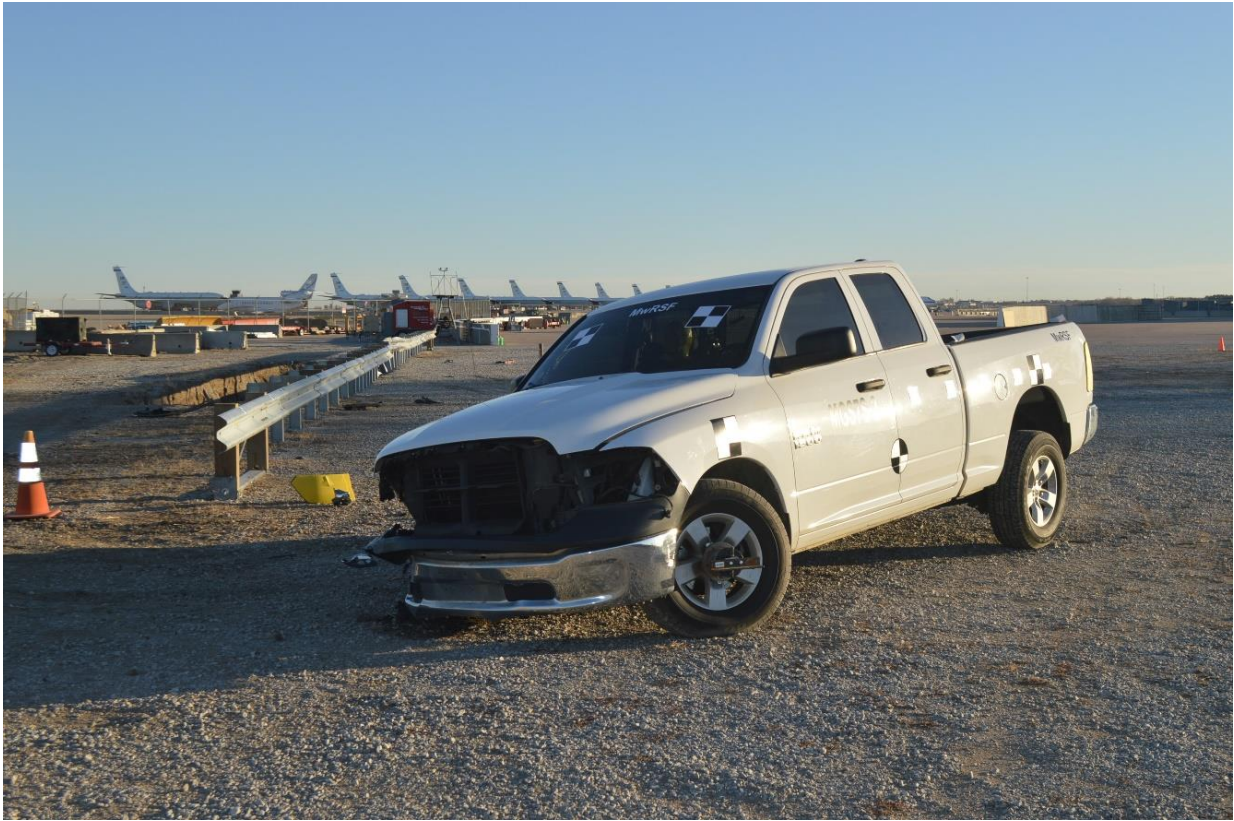
Figure 51. Vehicle Final Position and Trajectory Marks, Test No. MGS7S-2
