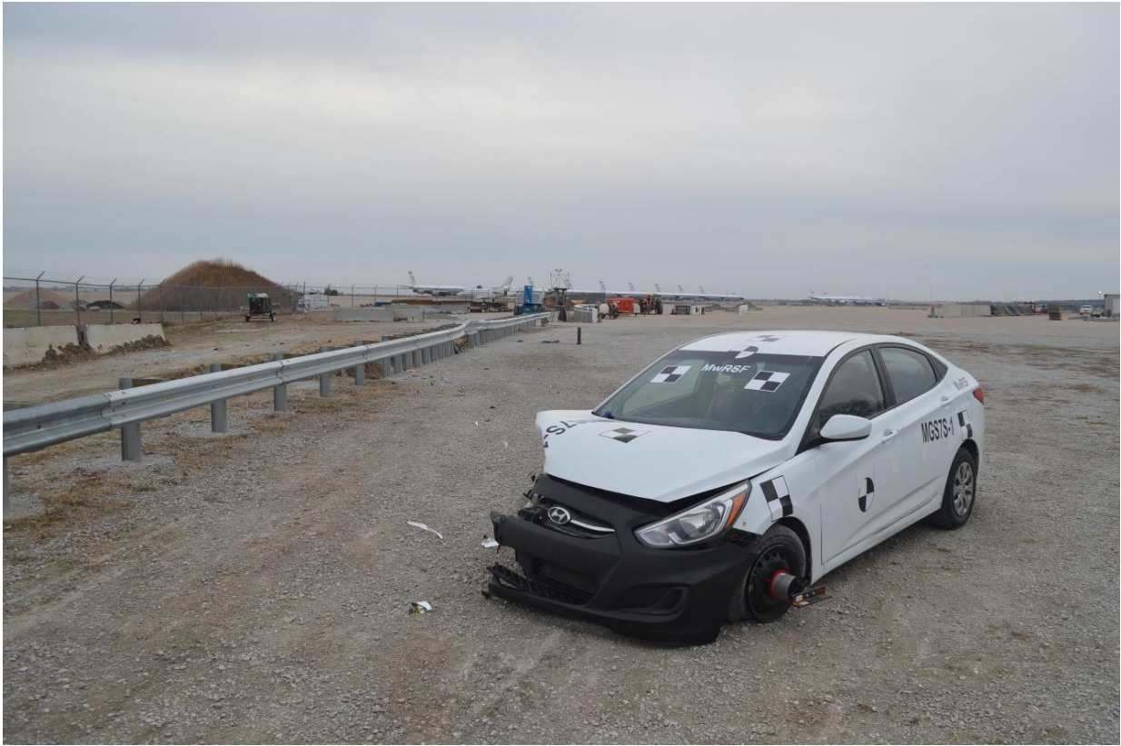
Figure 34. Vehicle Final Position and Trajectory Marks, Test No. MGS7S-1
