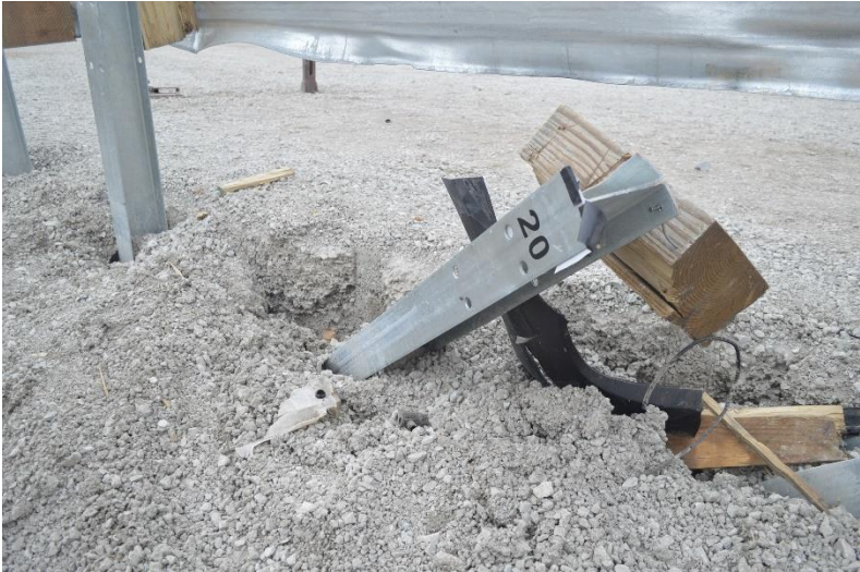
Figure 39. Post and Flange Damage, Test No. MGS7S-1
