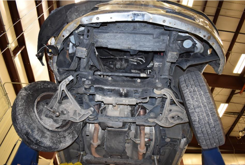
Figure 60. Vehicle Undercarriage and Occupant Compartment Damage, Test No. MGS7S-2
