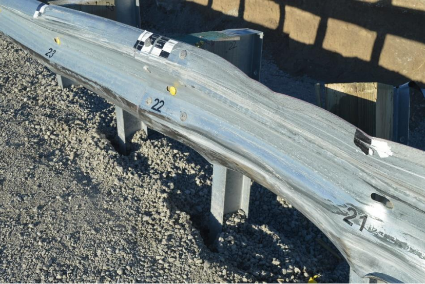
Figure 55. Damage to Post Nos. 21 and 22, Test No. MGS7S-2 Description
