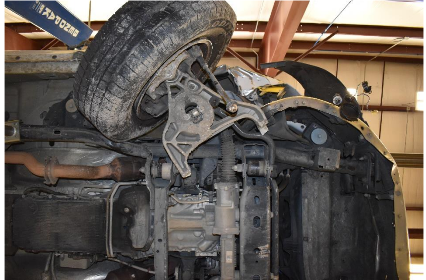
Figure 60. Vehicle Undercarriage and Occupant Compartment Damage, Test No. MGS7S-2
