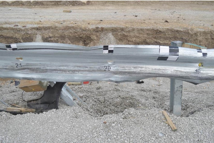
Figure 37. Damage to Post Nos. 19 and 20, Test No. MGS7S-1
