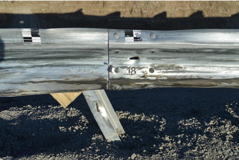
Figure 53. Damage to Post Nos. 17 and 18, Test No. MGS7S-2
