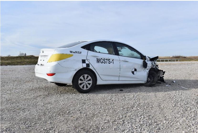
Figure 43. Vehicle Damage. Test No. MGS7S-1
