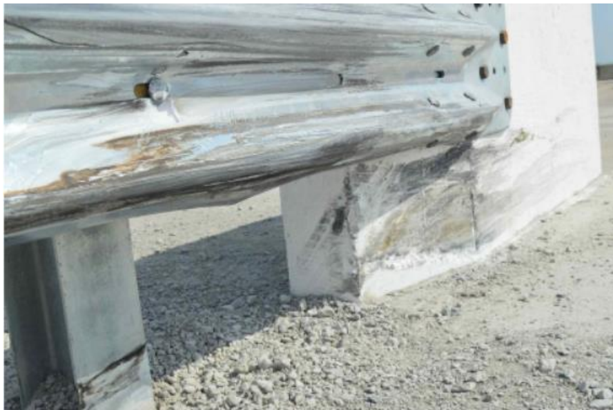
Figure 20. Wheel Snag on 34-in. AGT during MASH Crash Testing [2]
