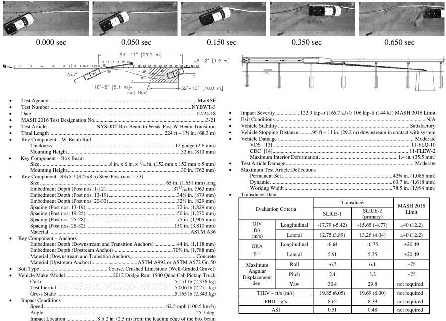
Figure 101. Summary of Test Results and Sequential Photographs, Test No. NYBWT-3
