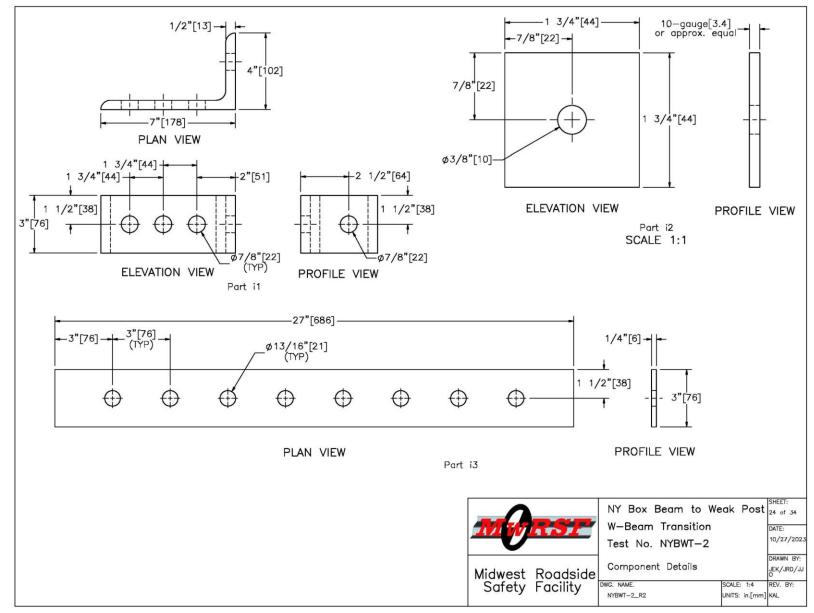
Figure 24. Components Details, Test No. NYBWT-2
