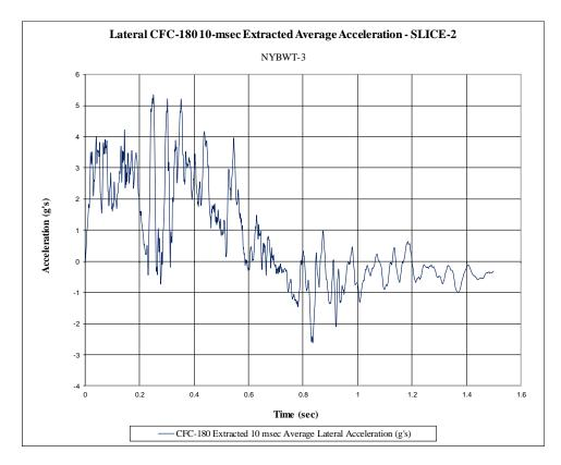
Figure H-12. 10-ms Average Lateral Deceleration (SLICE-2), Test No. NYBWT-3
