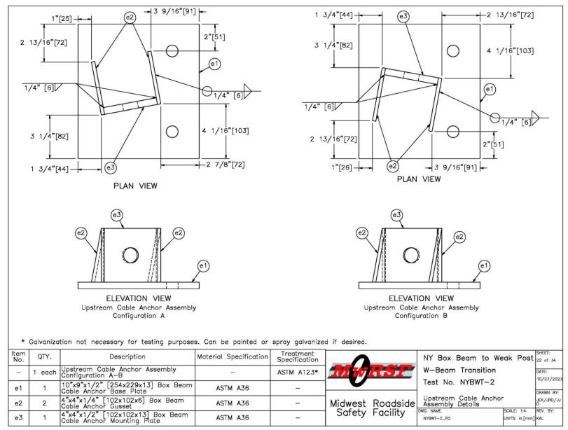
Figure 22. Upstream Cable Anchor Assembly Details Test No. NYBWT-2
