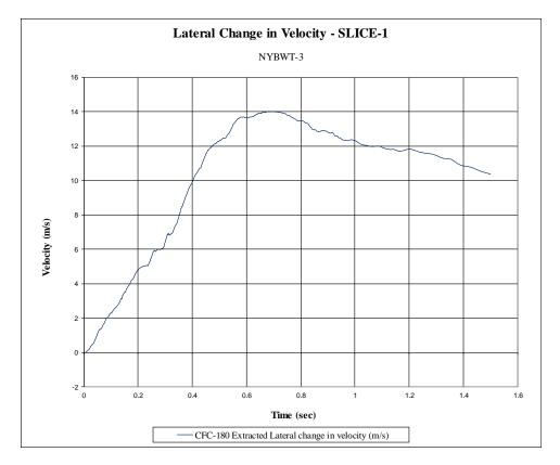
Figure H-5. Lateral Occupant Impact Velocity (SLICE-1), Test No. NYBWT-3
