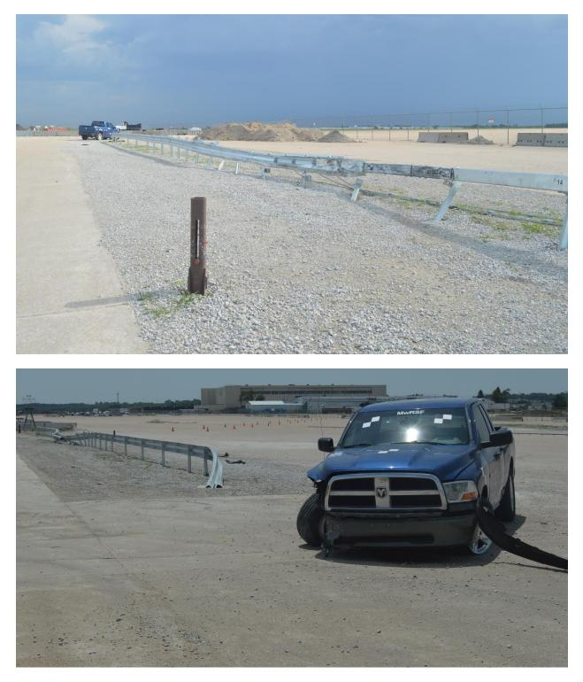
Figure 64. Vehicle Trajectory Marks and Final Position, Test No. NYBWT-2
