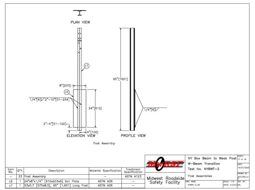
Figure 17. Post Assemblies, Test No. NYBWT-2
