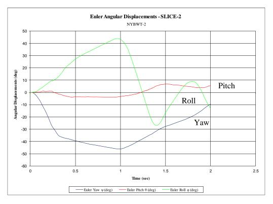
Figure G-15. Vehicle Angular Displacements (SLICE-2), Test No. NYBWT-2
