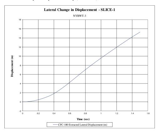
Figure H-6. Lateral Occupant Displacement (SLICE-1), Test No. NYBWT-3
