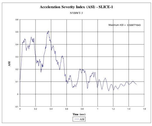
Figure H-8. Acceleration Severity Index (SLICE-1), Test No. NYBWT-3
