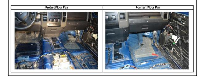
Figure F-2. Floor Pan Deformation Data – Set 2, Test No. NYBWT-2
