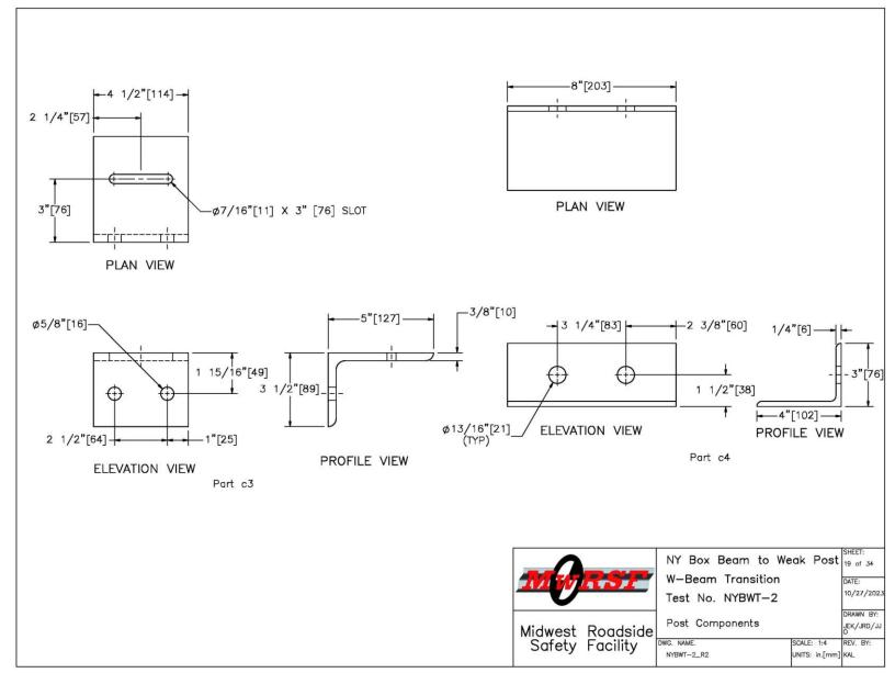
Figure 19. Post Components, Rail Support Bracket and Post Collar, Test No. NYBWT-2
