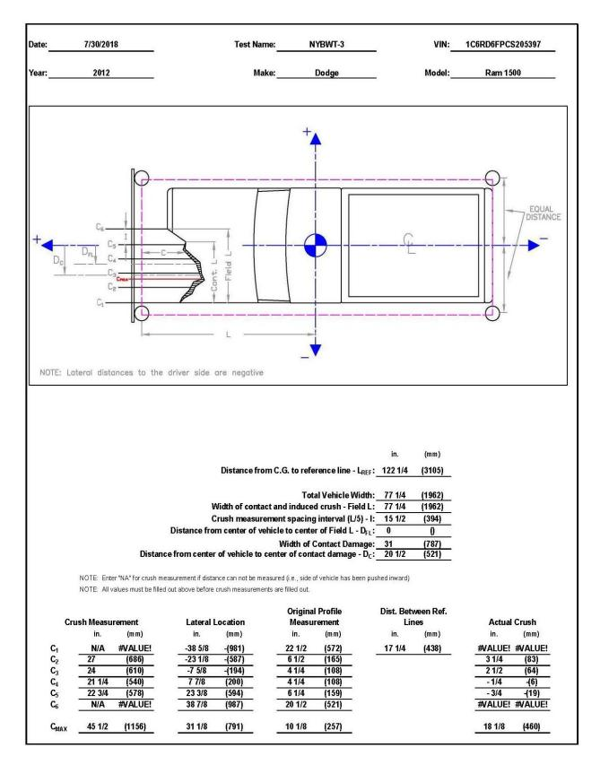
Figure F-11. Exterior Vehicle Crush (NASS) - Front, Test No. NYBWT-3
