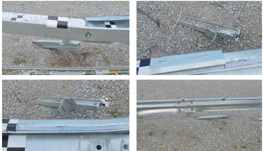
Figure 72. Backside Rail and Post Damage, Post Nos. 16 through 19, Test No. NYBWT-2
