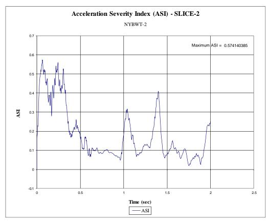
Figure G-16. Acceleration Severity Index (SLICE-2), Test No. NYBWT-2
