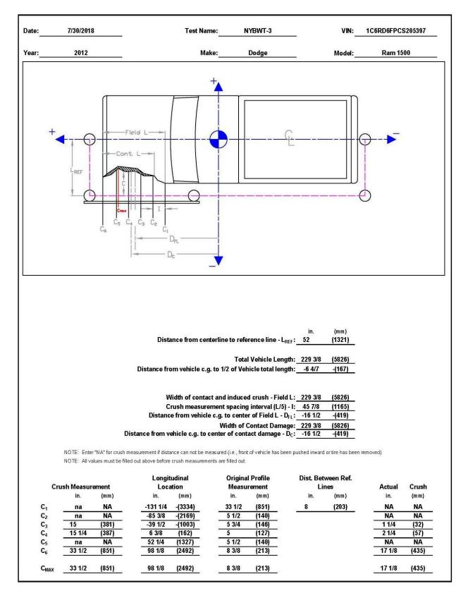
Figure F-12. Exterior Vehicle Crush (NASS) - Side, Test No. NYBWT-3
