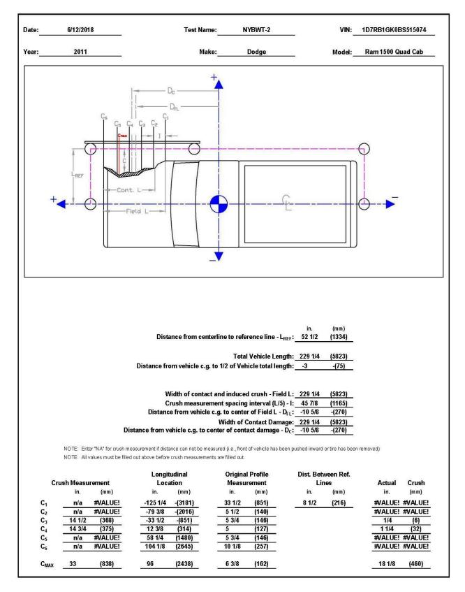
Figure F-6. Exterior Vehicle Crush (NASS) - Side, Test No. NYBWT-2
