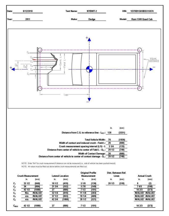
Figure F-5. Exterior Vehicle Crush (NASS) - Front, Test No. NYBWT-2
