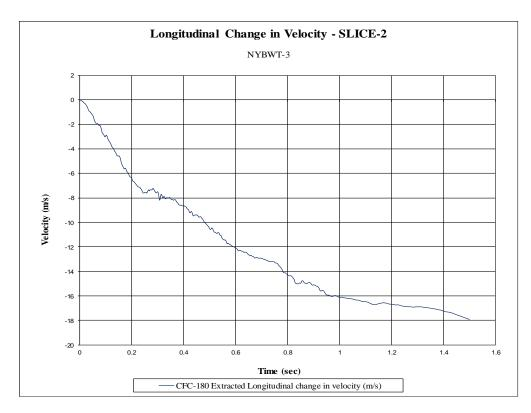
Figure H-10. Longitudinal Occupant Impact Velocity (SLICE-2), Test No. NYBWT-3
