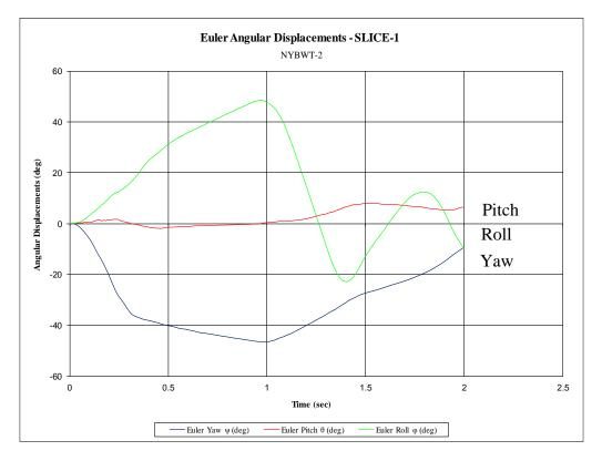
Figure G-7. Vehicle Angular Displacements (SLICE-1), Test No. NYBWT-2
