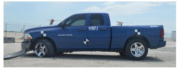
Figure 76. Vehicle Damage, Test No. NYBWT-2
