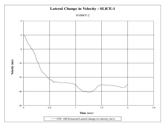
Figure G-5. Lateral Occupant Impact Velocity (SLICE-1), Test No. NYBWT-2
