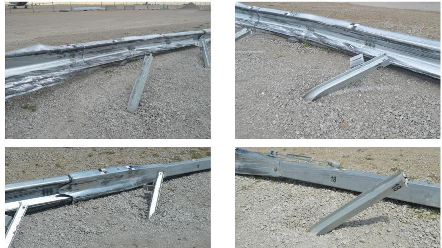
Figure 92. Damage to Post Nos. 15 through 18, Test No. NYBWT-3
