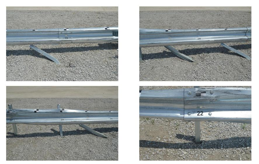
Figure 71. Rail and Post Damage, Post Nos. 19 through 22, Test No. NYBWT-2
