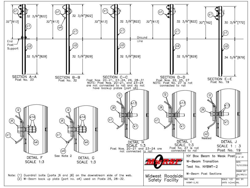
Figure 2. W-Beam Post Section, Test No. NYBWT-2
