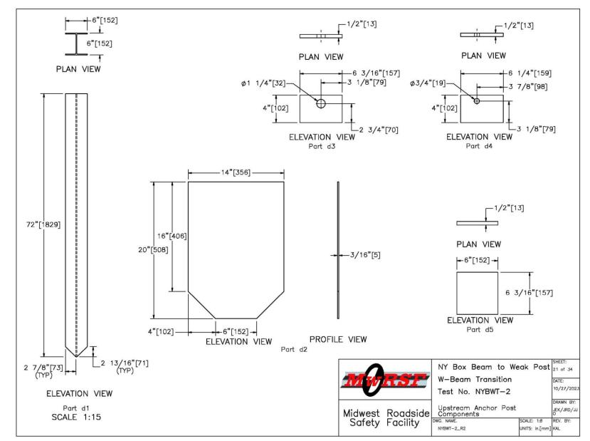
Figure 21. HFT Anchor Assembly Components, Test No. NYBWT-2
