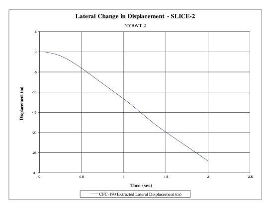
Figure G-14. Lateral Occupant Displacement (SLICE-2), Test No. NYBWT-2
