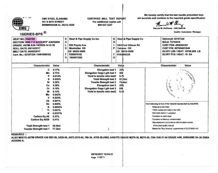
Figure B-31. 7 x 4 x <sup>1</sup>/<sub>2</sub>-in. (178 x 102 x 13-mm), 3-in. (76-mm) Long L-Brackets, Test Nos. NYBWT-2 and NYBWT-3 (Item No. i1)
