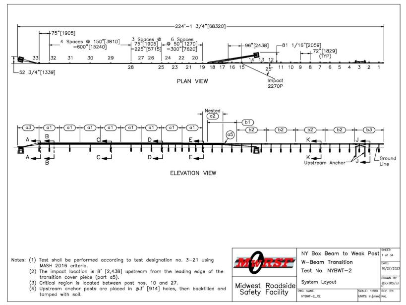
Figure 1. System Layout, Test No. NYBWT-2
