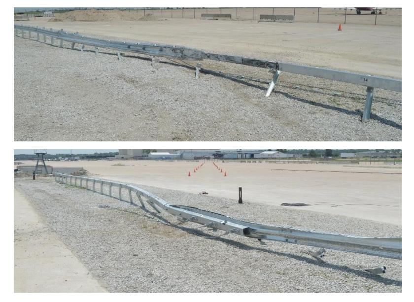
Figure 66. Overall System Damage, Test No. NYBWT-2
