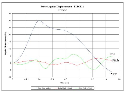
Figure H-15. Vehicle Angular Displacements (SLICE-2), Test No. NYBWT-3
