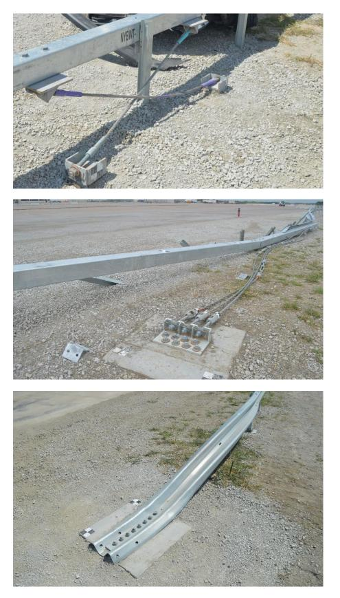
Figure 95. Anchor Damage, Test No. NYBWT-3
