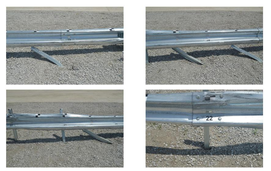
Figure 69. Rail and Post Damage, Post Nos. 19 through 22, Test No. NYBWT-2
