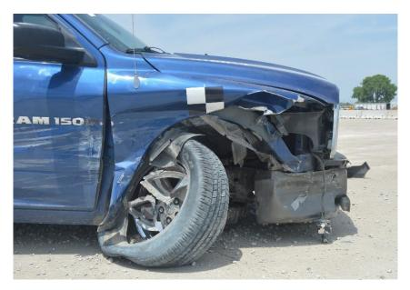
Figure 77. Vehicle Damage, Test No. NYBWT-2
