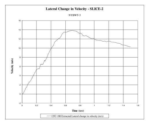
Figure H-13. Lateral Occupant Impact Velocity (SLICE-2), Test No. NYBWT-3
