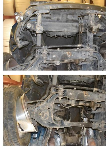
Figure 79. Undercarriage Vehicle Damage, Test No. NYBWT-2
