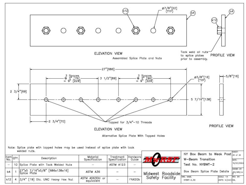
Figure 30. Box Beam Splice Plate Details, Test No. NYBWT-2
