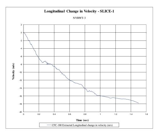
Figure H-2. Longitudinal Occupant Impact Velocity (SLICE-1), Test No. NYBWT-3
