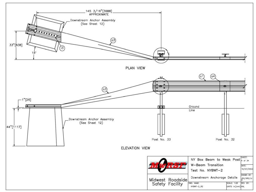
Figure 4. Downstream Anchorage Details, Test No. NYBWT-2
