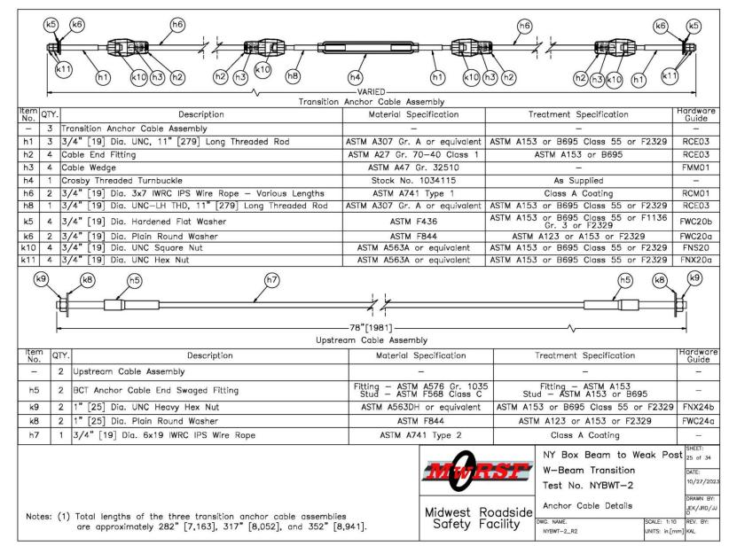
Figure 25. Anchor Cable Details, Test No. NYBWT-2
