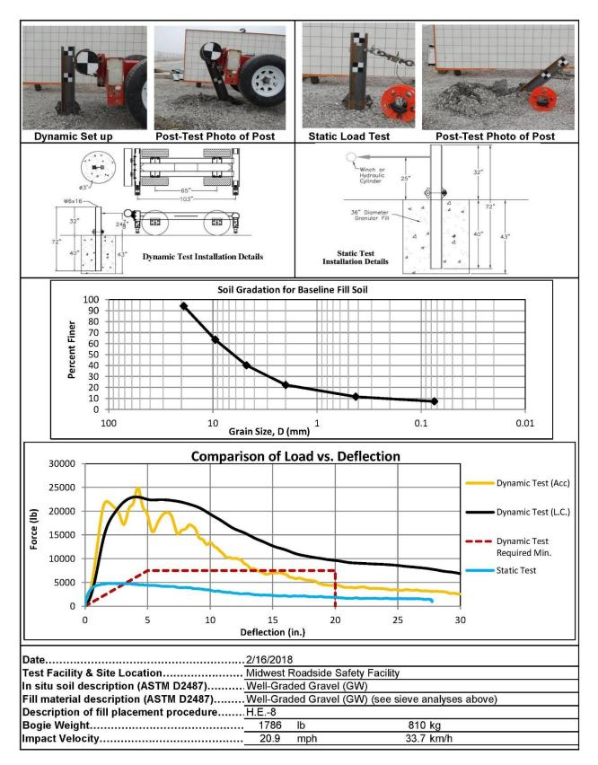
Figure C-1. Soil Strength, Initial Calibration Tests, Nos. NYBWT-2 and NYBWT-3
