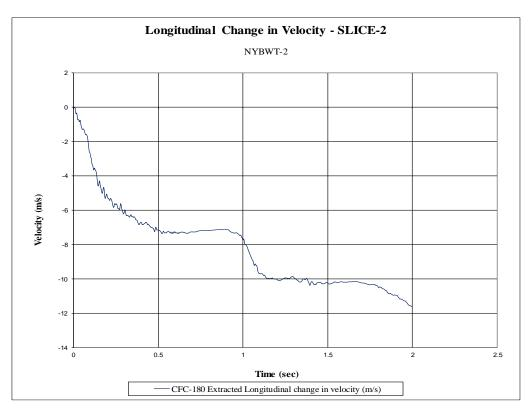
Figure G-10. Longitudinal Occupant Impact Velocity (SLICE-2), Test No. NYBWT-2
