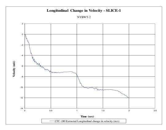
Figure G-2. Longitudinal Occupant Impact Velocity (SLICE-1), Test No. NYBWT-2
