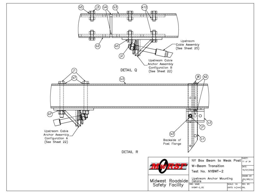
Figure 10. Upstream Anchorage Details, Test No. NYBWT-2
