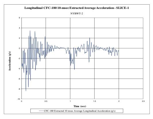
Figure G-1. 10-ms Average Longitudinal Deceleration (SLICE-1), Test No. NYBWT-2
