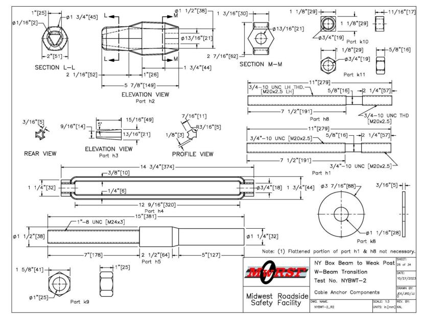
Figure 26. Cable Anchor Components, Test No. NYBWT-2
