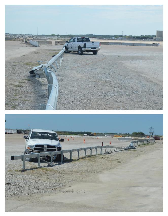
Figure 88. Vehicle Trajectory Marks and Final Position, Test No. NYBWT-3
