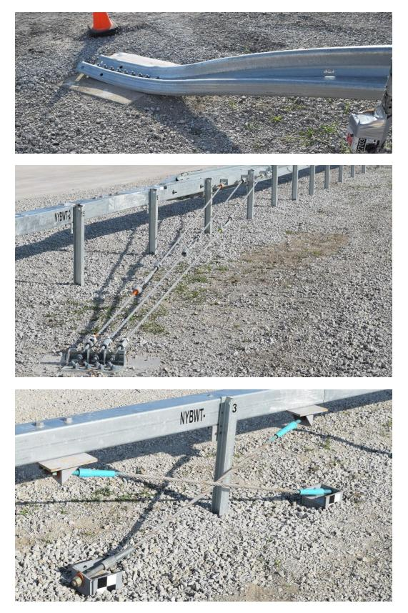
Figure 39. Anchors, Test No. NYBWT-2
