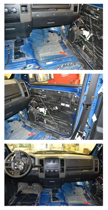
Figure 78. Occupant Compartment Vehicle Damage, Test No. NYBWT-2
