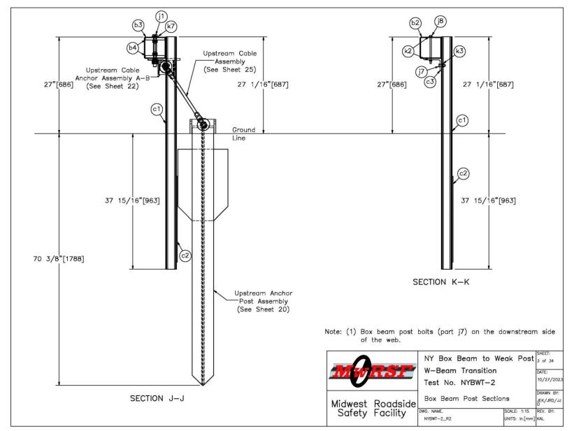
Figure 3. Box Beam Post Section, Test No. NYBWT-2
