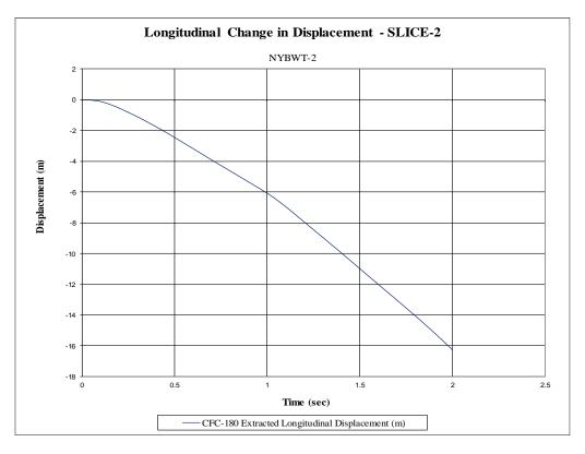
Figure G-11. Longitudinal Occupant Displacement (SLICE-2), Test No. NYBWT-2
