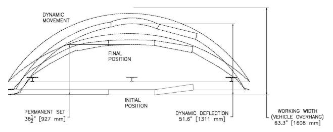
Figure 75. Permanent Set, Dynamic Deflection, and Working Width, Test No. NYBWT-2
