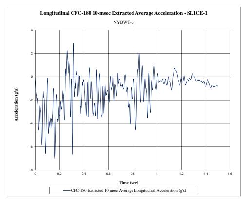
Figure H-1. 10-ms Average Longitudinal Deceleration (SLICE-1), Test No. NYBWT-3
