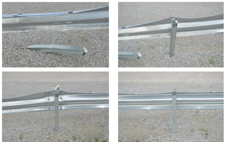
Figure 73. Backside Rail and Post Damage, Post Nos. 20 through 23, Test No. NYBWT-2
