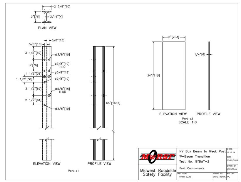
Figure 18. Post Components, Test No. NYBWT-2
