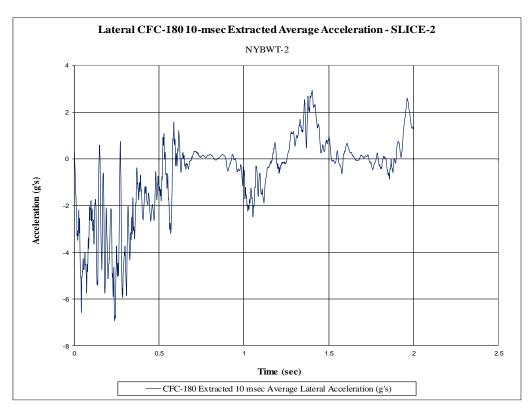
Figure G-12. 10-ms Average Lateral Deceleration (SLICE-2), Test No. NYBWT-2
