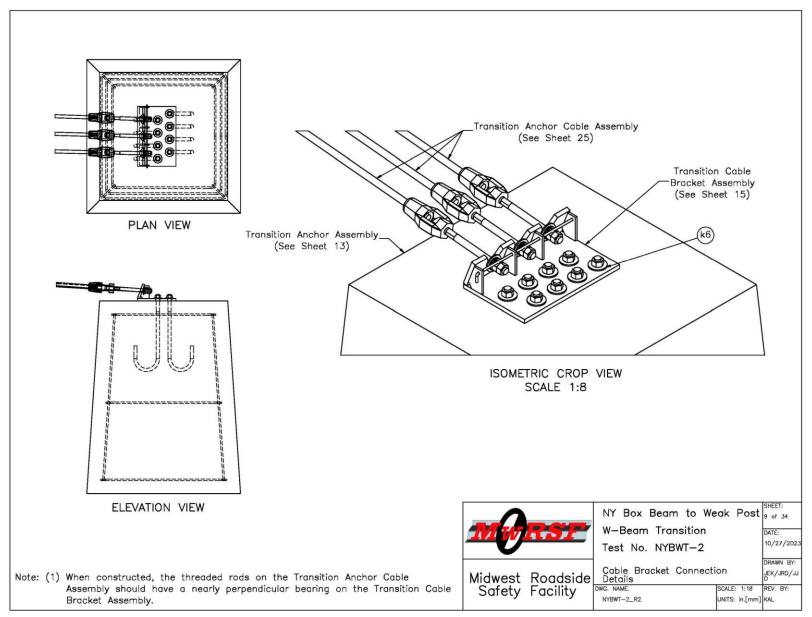
Figure 9. Cable Bracket Connection Details, Test No. NYBWT-2
