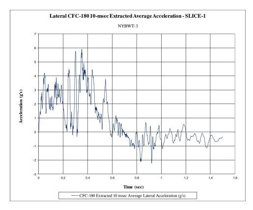
Figure H-4. 10-ms Average Lateral Deceleration (SLICE-1), Test No. NYBWT-3
