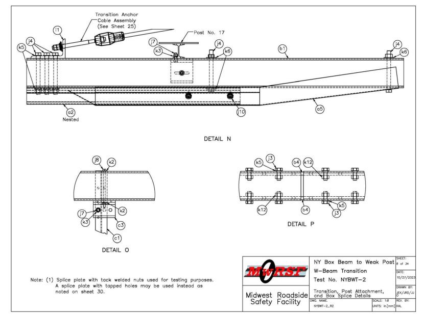
Figure 8. Transition, Post Attachment, and Box Splice Details, Test No. NYBWT-2
