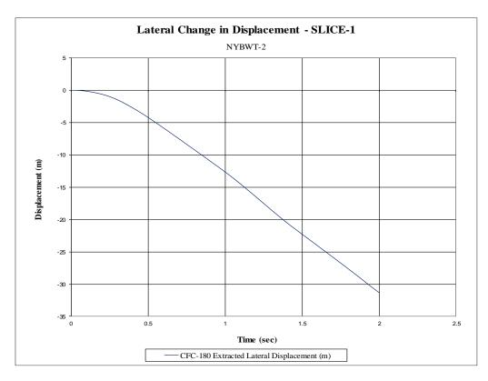
Figure G-6. Lateral Occupant Displacement (SLICE-1), Test No. NYBWT-2
