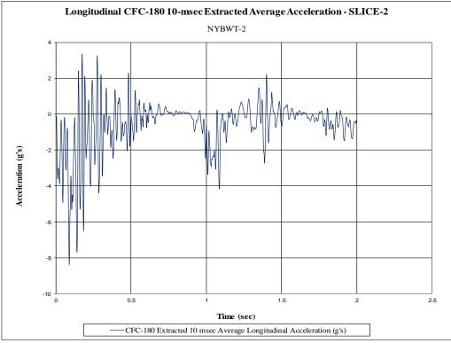
Figure G-9. 10-ms Average Longitudinal Deceleration (SLICE-2), Test No. NYBWT-2
