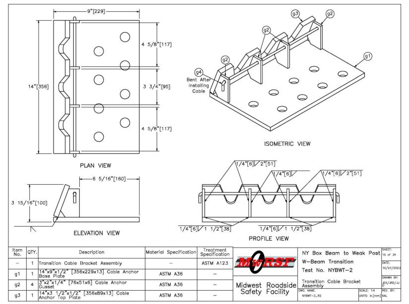
Figure 15. Transition Cable Bracket Assembly, Test No. NYBWT-2
