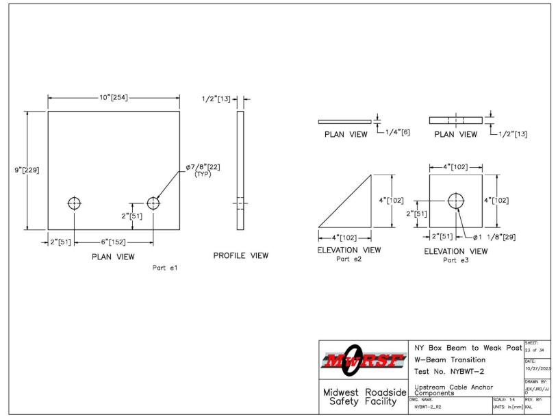
Figure 23. Upstream Cable Anchor Components, Test No. NYBWT-2
