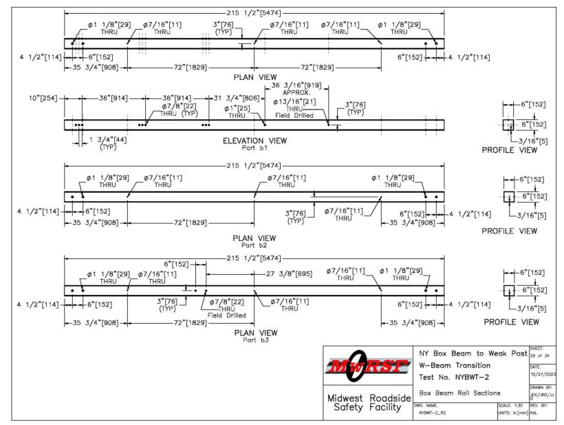
Figure 29. Box Beam Rail Section, Test No. NYBWT-2
