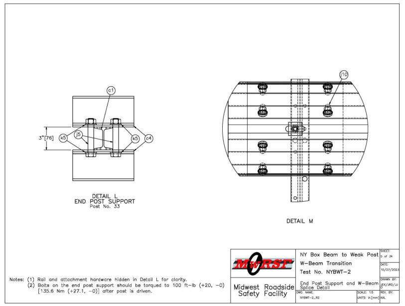
Figure 5. End Post Support and W-beam Splice Detail, Test No. NYBWT-2
