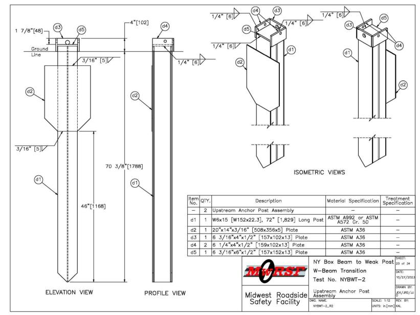
Figure 20. HFT Anchor Assembly, Test No. NYBWT-2
