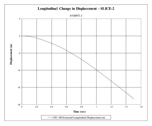
Figure H-11. Longitudinal Occupant Displacement (SLICE-2), Test No. NYBWT-3
