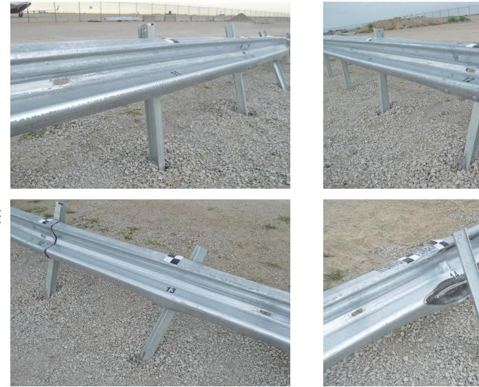
Figure 91. Damage to Post Nos. 11 through 14, Test No. NYBWT-3
