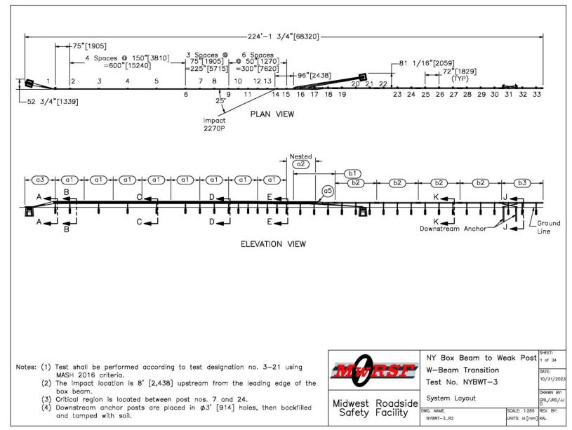
Figure 35. System Layout, Test No. NYBWT-3
