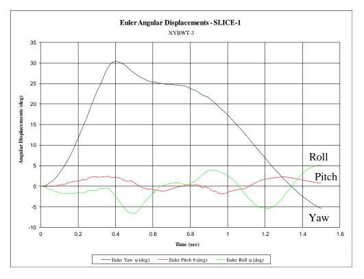
Figure H-7. Vehicle Angular Displacements (SLICE-1), Test No. NYBWT-3
