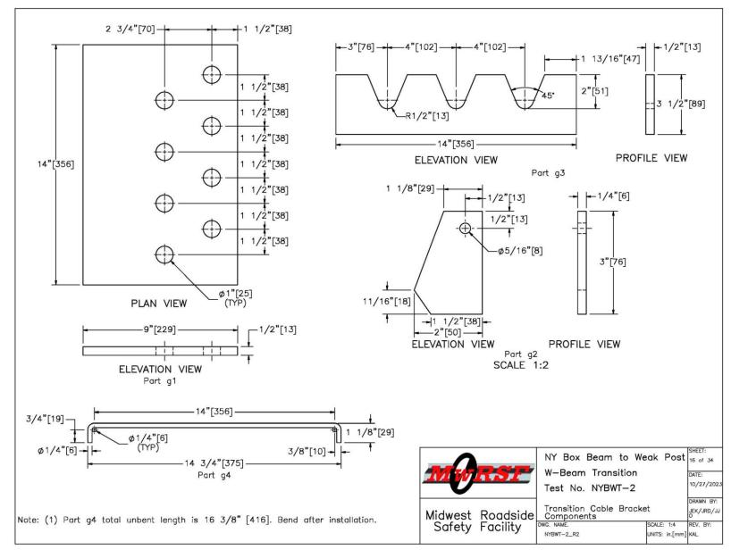
Figure 16. Transition Cable Bracket Components, Test No. NYBWT-2
