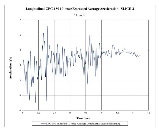
Figure H-9. 10-ms Average Longitudinal Deceleration (SLICE-2), Test No. NYBWT-3
