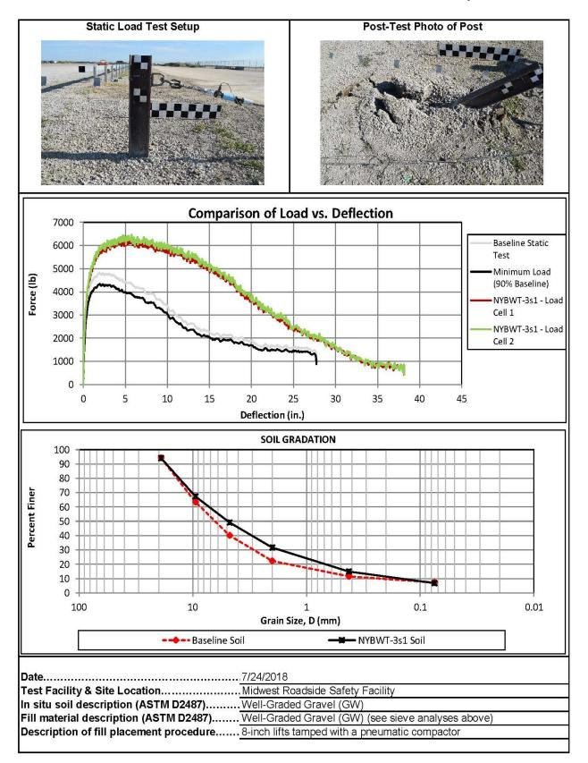
Figure C-3. Static Soil Test, Test No. NYBWT-3
