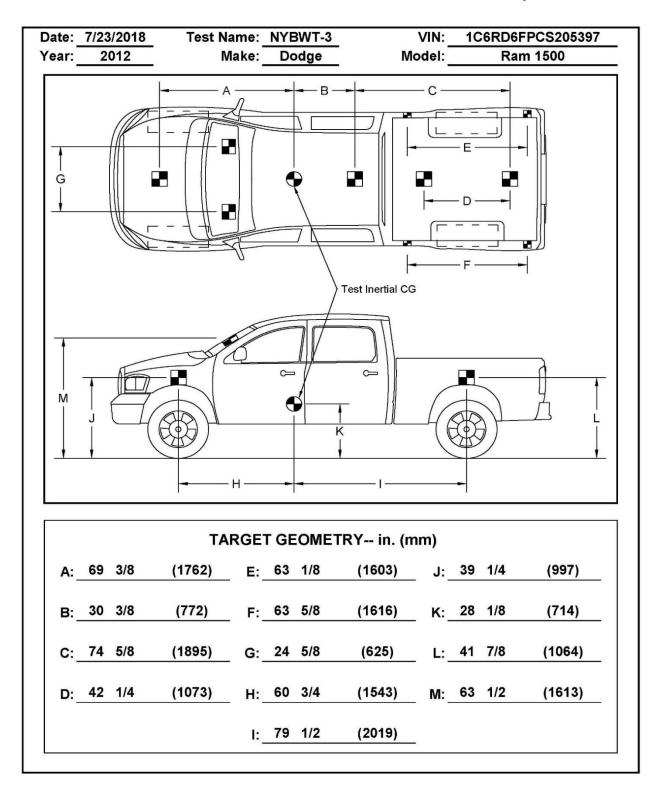
Figure 51. Target Geometry, Test No. NYBWT-3
