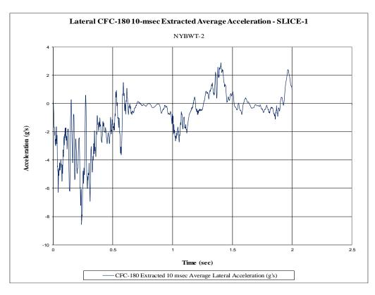
Figure G-4. 10-ms Average Lateral Deceleration (SLICE-1), Test No. NYBWT-2
