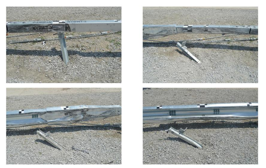
Figure 68. Rail and Post Damage, Post Nos. 15 through 18, Test No. NYBWT-2
