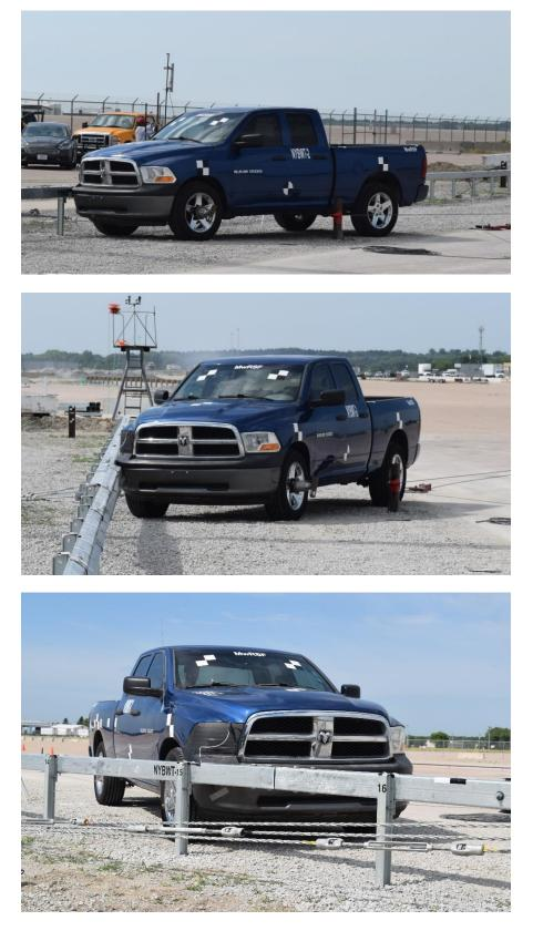
Figure 54. Impact Location, Test No. NYBWT-2
