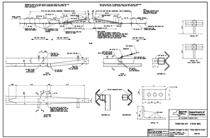
Figure A-1. New York Standard Sheet for Box Beam to Weak-Post W-Beam Transition, Test No. NYBWT-2 [15]
