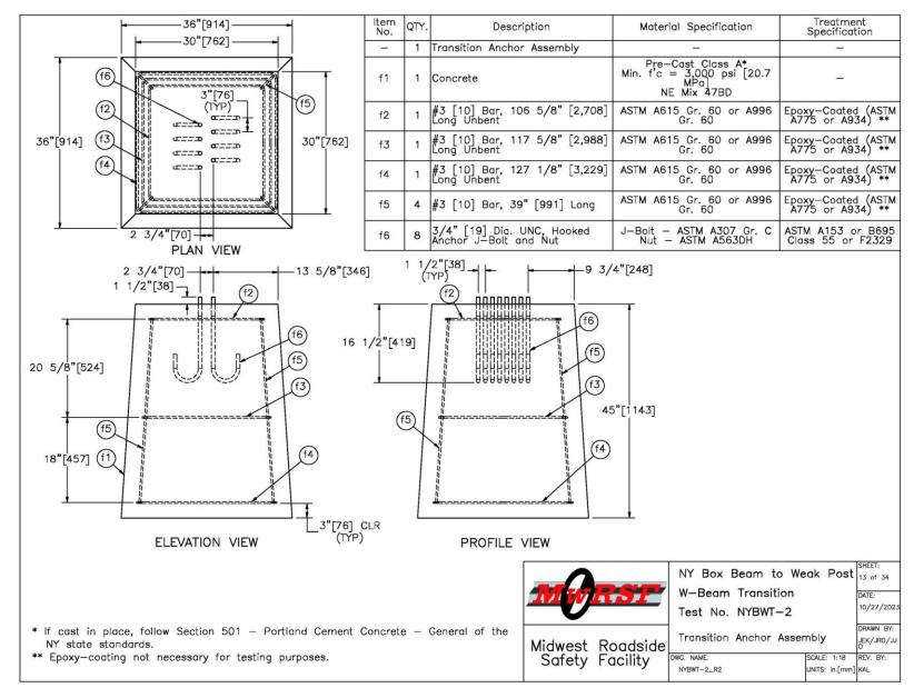
Figure 13. Transition Anchor Assembly, Test No. NYBWT-2
