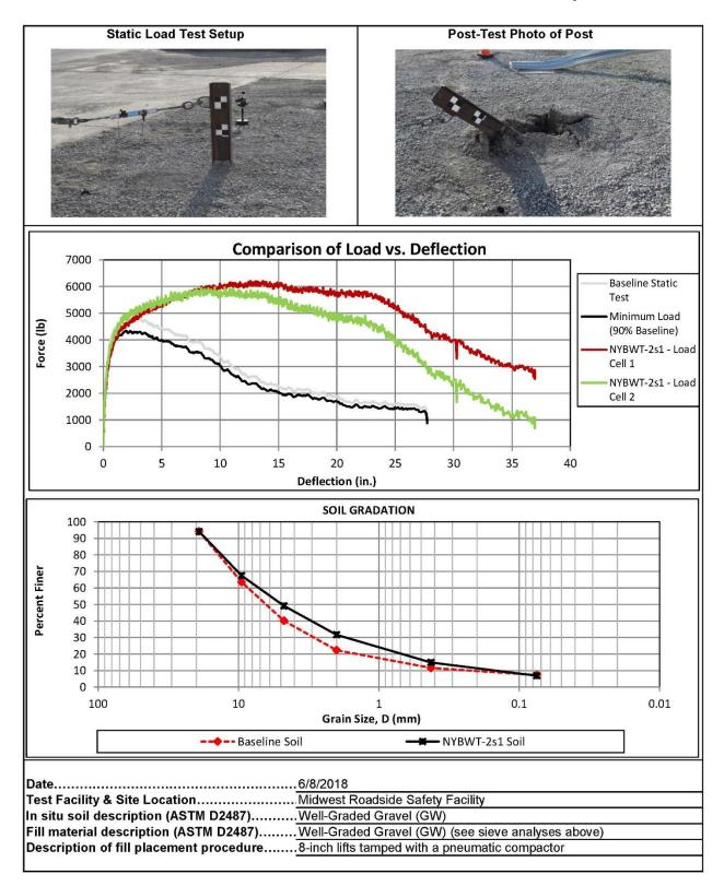
Figure C-2. Static Soil Test, Test No. NYBWT-2
