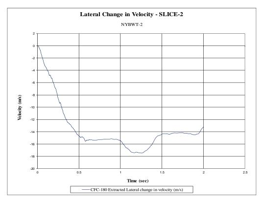
Figure G-13. Lateral Occupant Impact Velocity (SLICE-2), Test No. NYBWT-2
