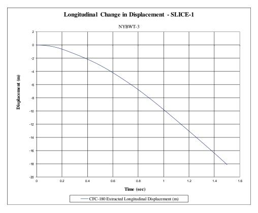
Figure H-3. Longitudinal Occupant Displacement (SLICE-1), Test No. NYBWT-3
