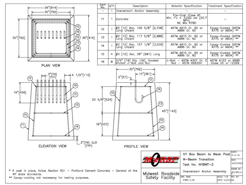
Figure 12. Downstream Anchor Assembly, Test No. NYBWT-2
