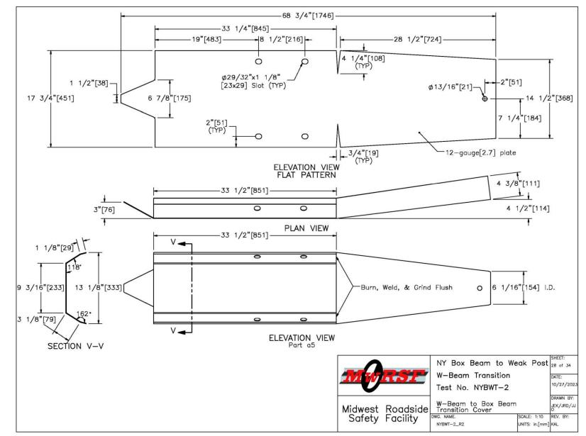
Figure 28. Box Beam to W-Beam Transition Cover, Test No. NYBWT-2
