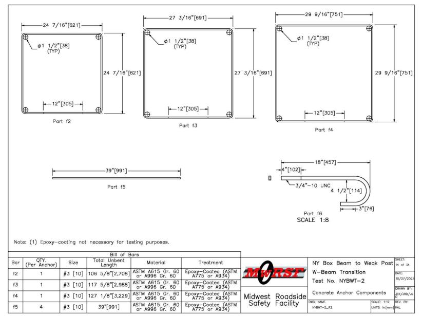
Figure 14. Concrete Anchor Components, Test No. NYBWT-2
