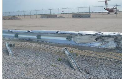
Figure 67. System Damage, Test No. NYBWT-2
