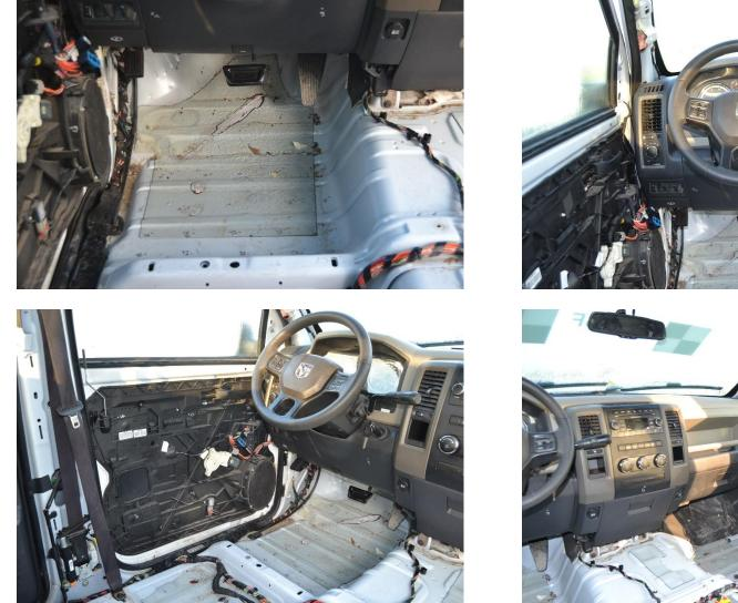
Figure 100. Occupant Compartment Damage, Test No. NYBWT-3
