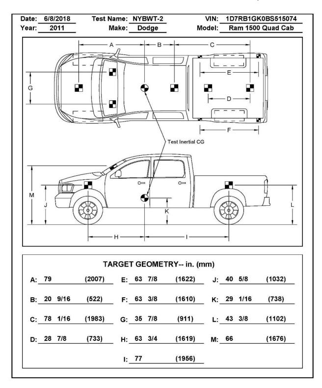
Figure 50. Target Geometry, Test No. NYBWT-2
