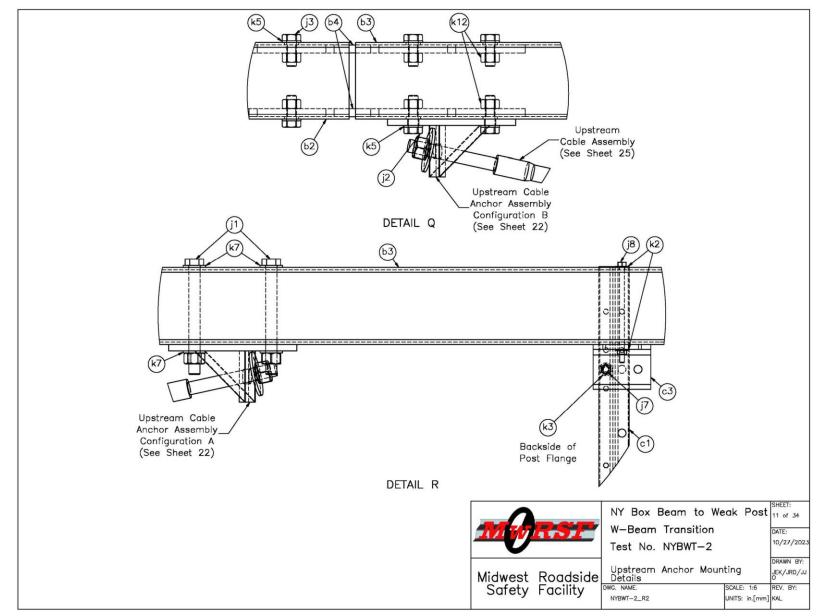
Figure 11. Upstream Anchor Mounting Details, Test No. NYBWT-2
