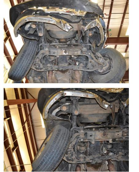
Figure 99. Undercarriage Vehicle Damage, Test No. NYBWT-3
