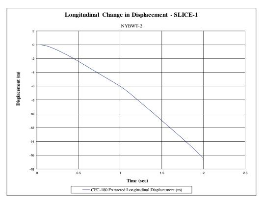
Figure G-3. Longitudinal Occupant Displacement (SLICE-1), Test No. NYBWT-2
