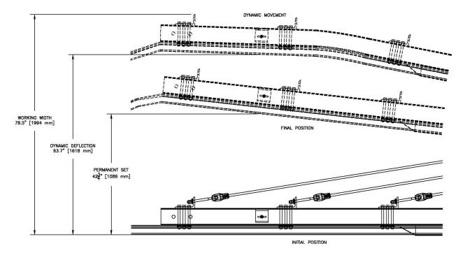
Figure 96. Permanent Set, Dynamic Deflection, and Working Width, Test No. NYBWT-3
