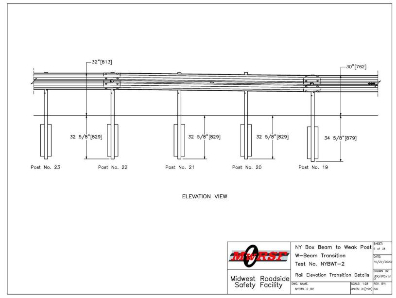
Figure 6. Rail Elevation Transition Details, Test No. NYBWT-2
