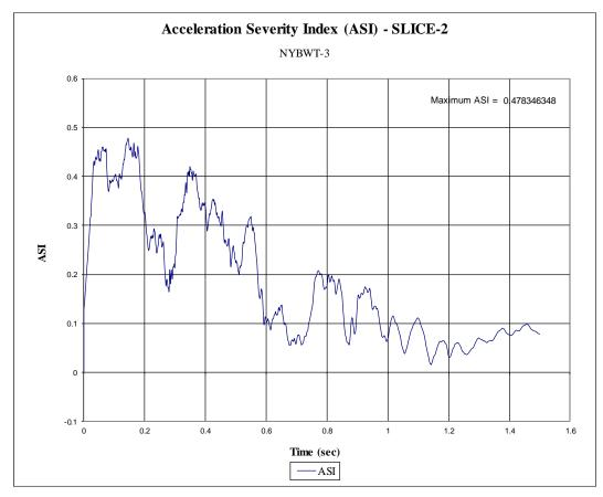
Figure H-16. Acceleration Severity Index (SLICE-2), Test No. NYBWT-3
