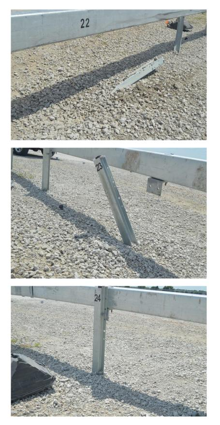
Figure 94. Damage to System at Post Nos. 22 through 24 117
