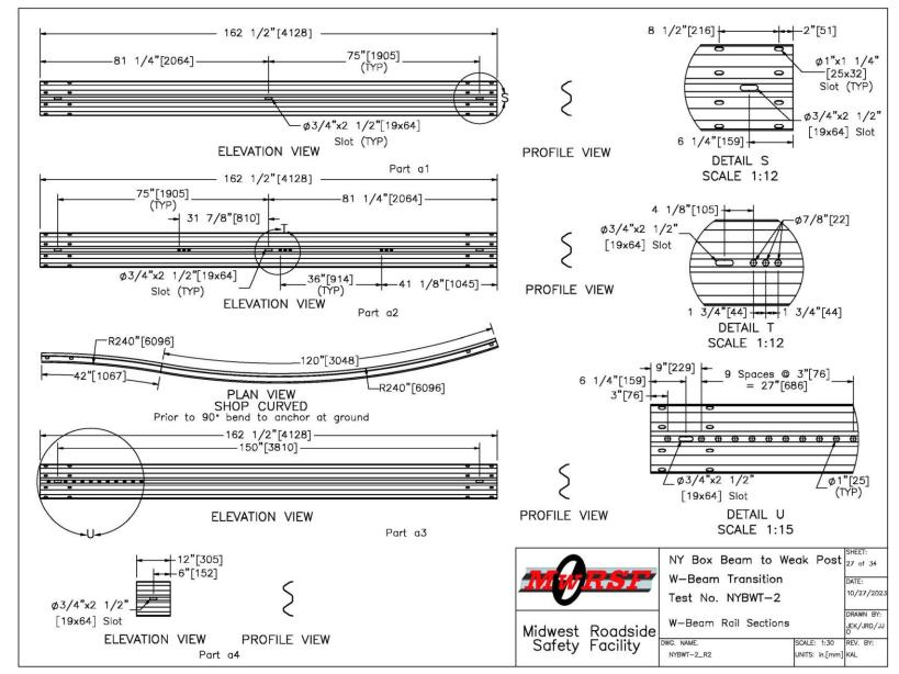
Figure 27. W-Beam Rail Section, Test No. NYBWT-2
