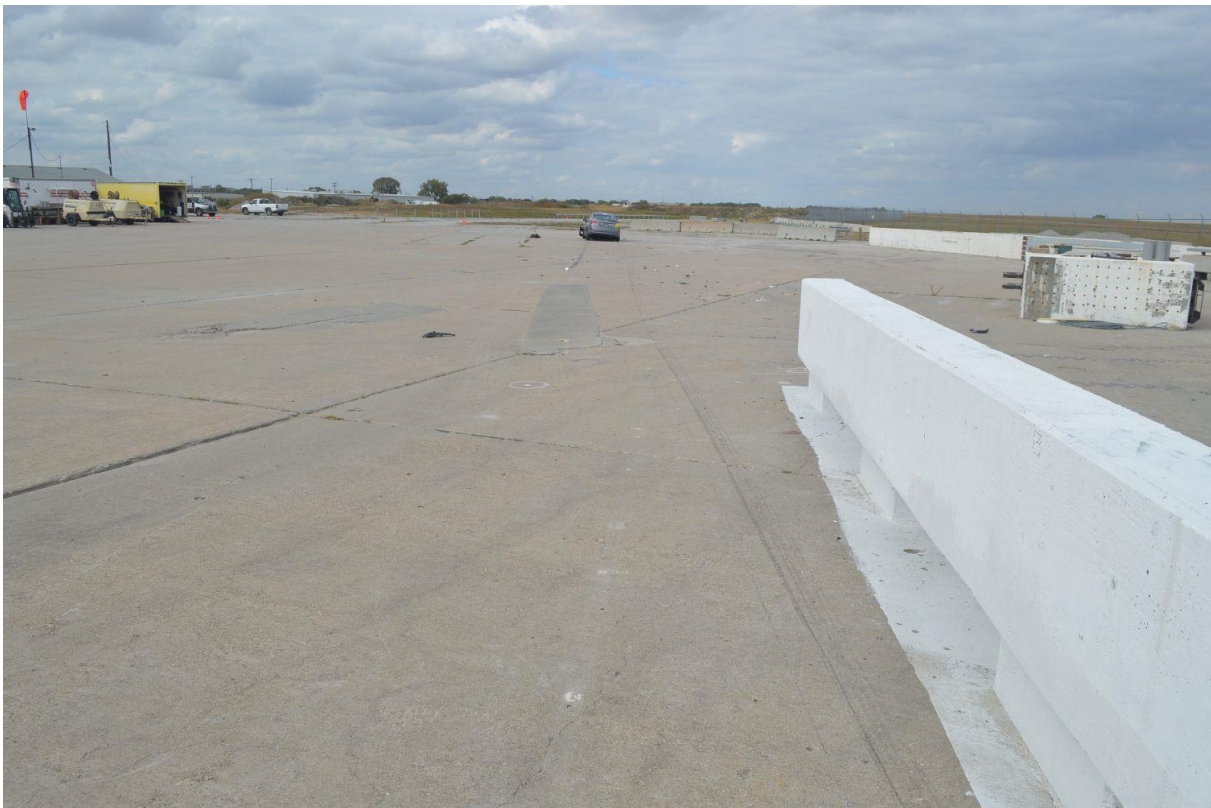
Figure 50. Vehicle Final Position and Trajectory Marks, Test No. OCBR-1
