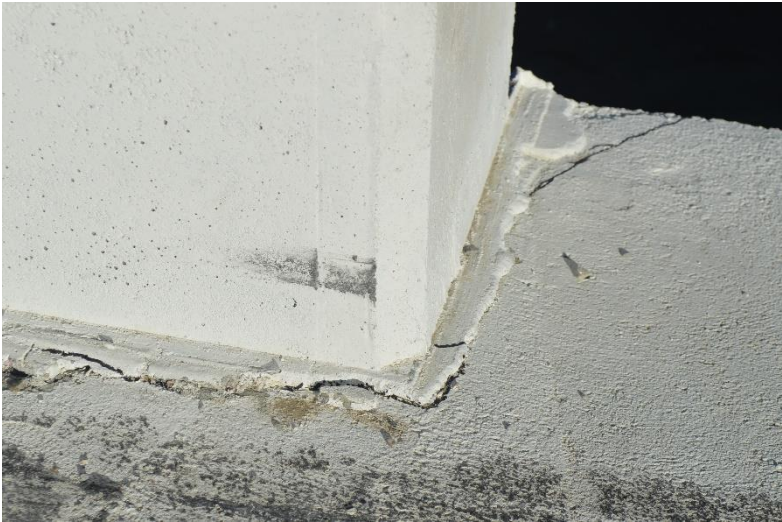
Figure 67. Post Nos. 7 and 8 Damage, Test No. OCBR-2
