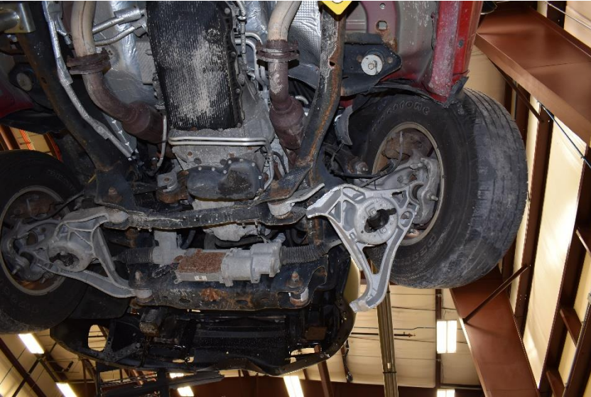
Figure 70. Interior and Undercarriage Damage, Test No. OCBR-2
