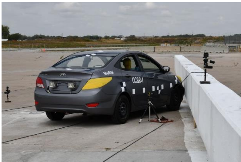
Figure 46. Target Impact Location, Test No. OCBR-1
