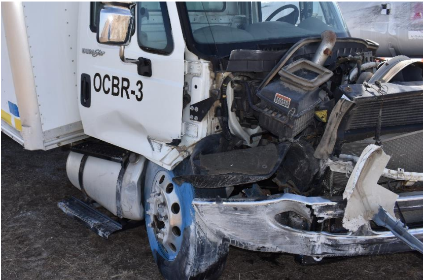
Figure 84. Vehicle Damage, Test No. OCBR-3
