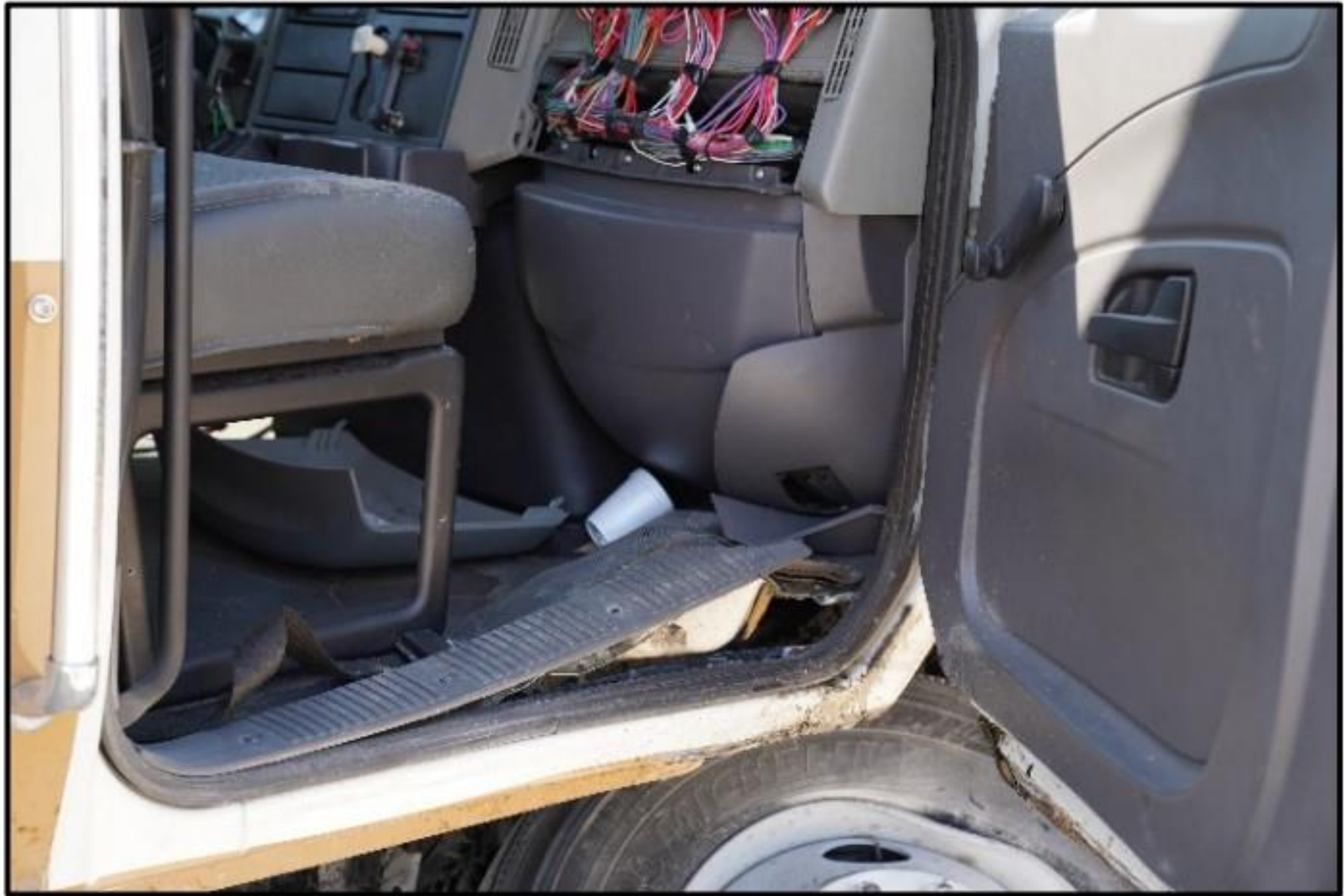
Figure 86. Vehicle Floor Pan Separation, MASH TL-4 Flared Concrete Barrier, Test No. 611901-05-1 [18]
