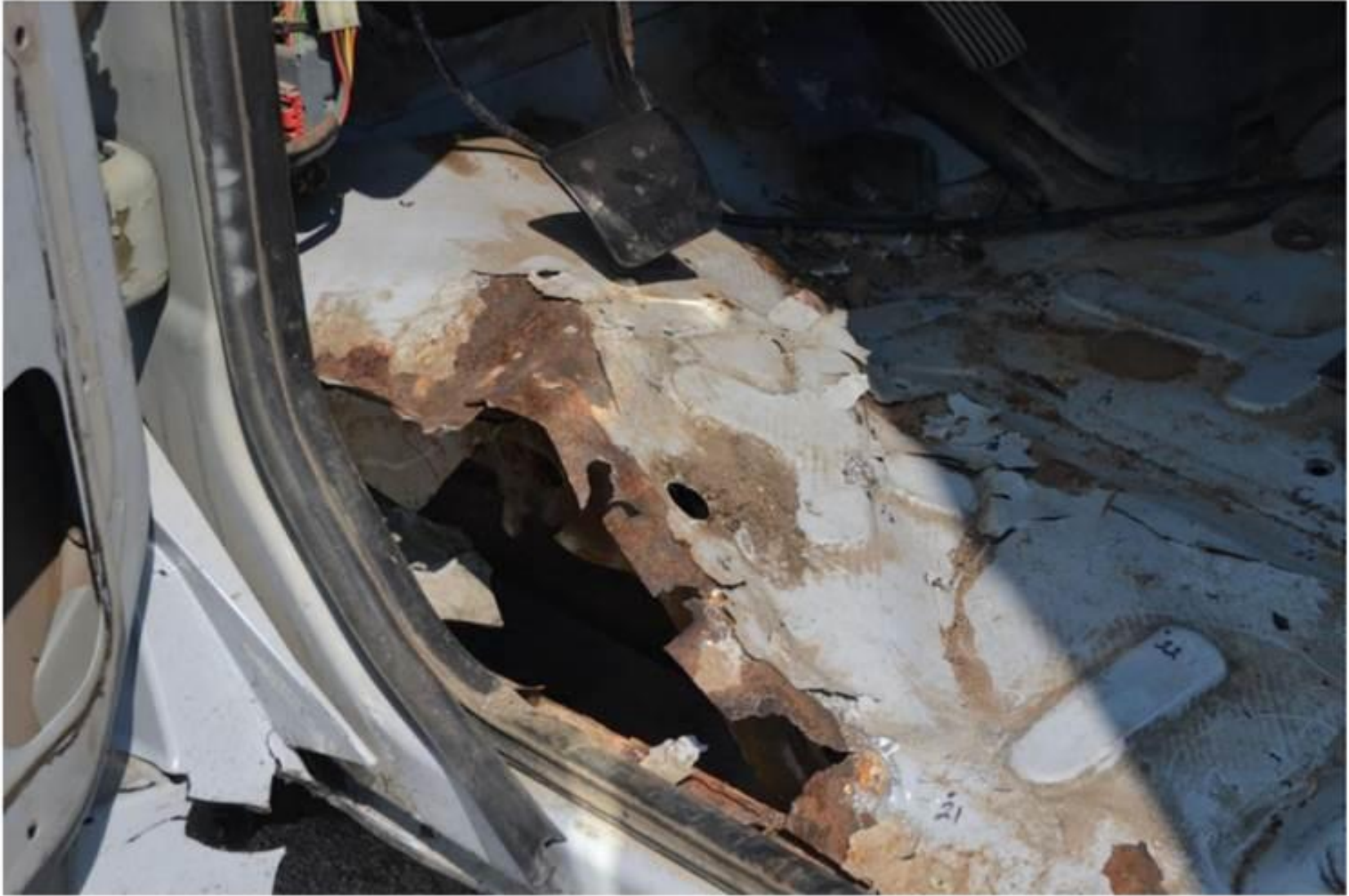
Figure 91. Vehicle Floor Pan Separation, Optimized TL-4 Concrete Bridge Rail, Test No. 4CBR-1 [23]
