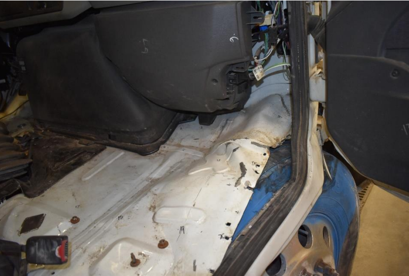
Figure 85. Vehicle Damage, Occupant Compartment Deformation Test No. OCBR-3
