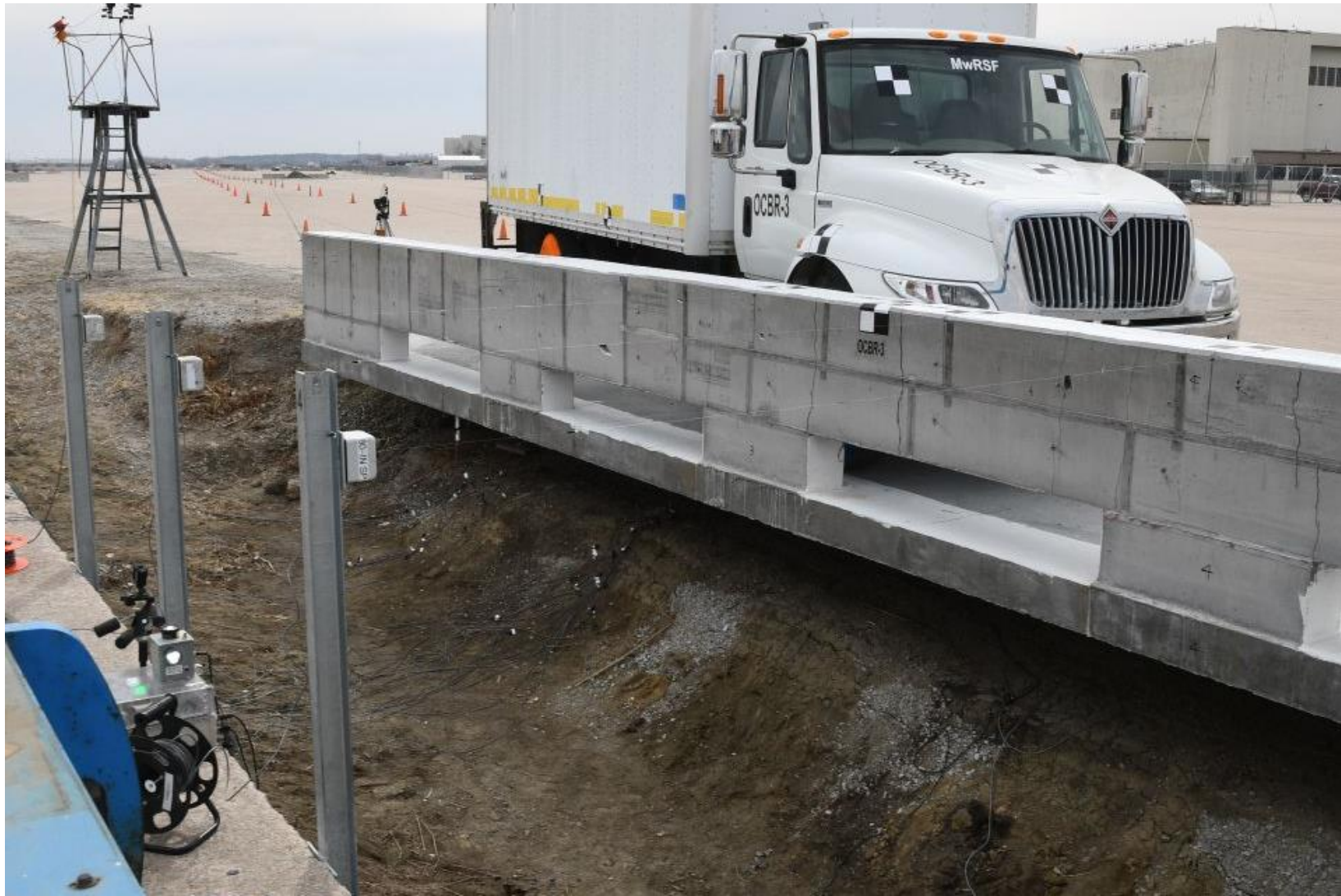
Figure 42. Location of String Potentiometers, Test No. OCBR-3
