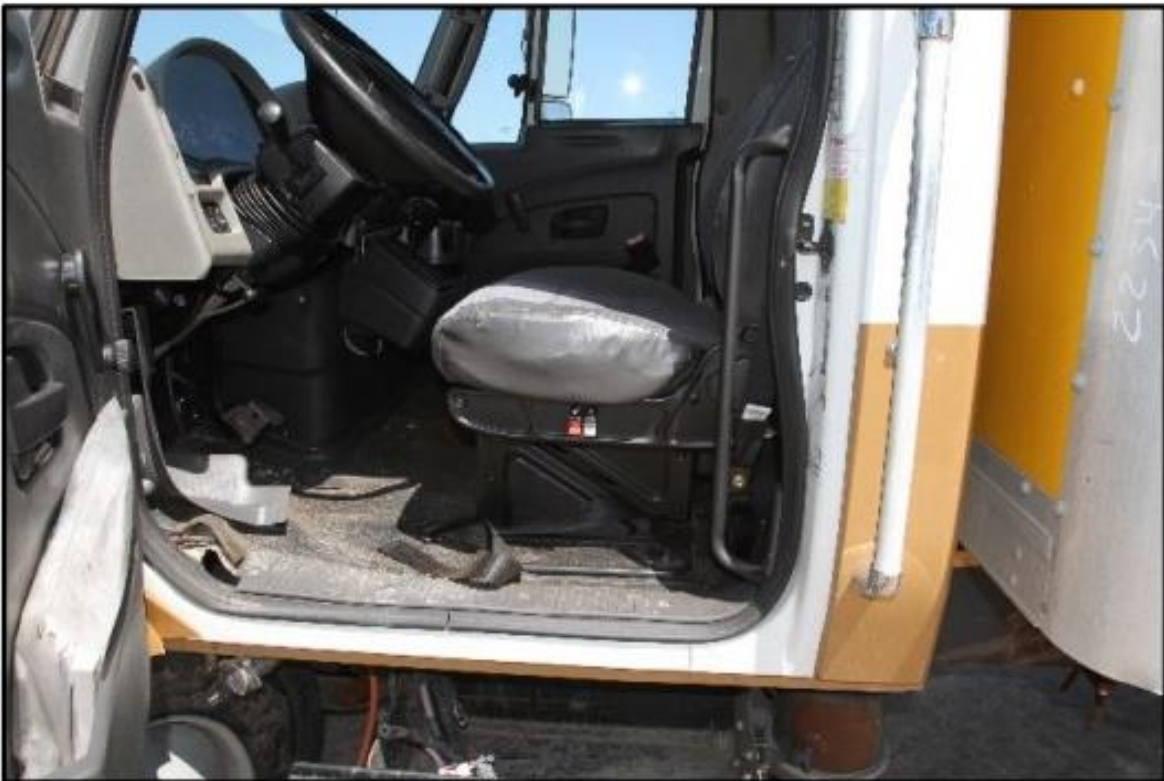
Figure 87. Vehicle Floor Pan Separation, C1W Bridge Rail, Test No. 469469-1 [19]
