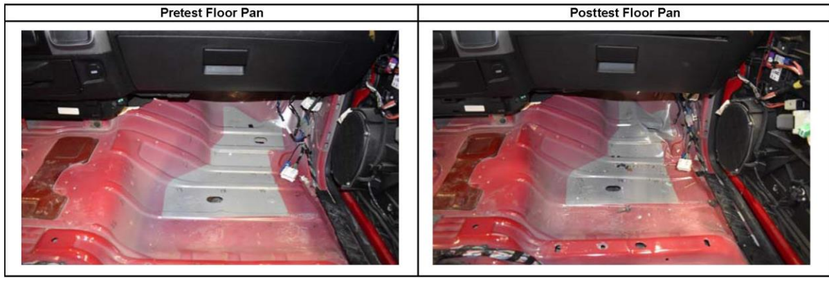
Figure C-6. Floor Pan Deformation Data – Set 1, Test No. OCBR-2
