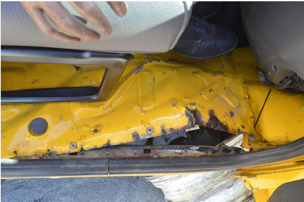
Figure 90. Vehicle Floor Pan Separation, Minnesota Combination Bridge Rail, Test No. MNCBR-1 [22]
