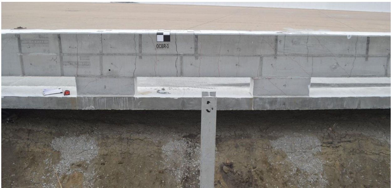
Figure 77. Overall System Damage, Test No. OCBR-3
