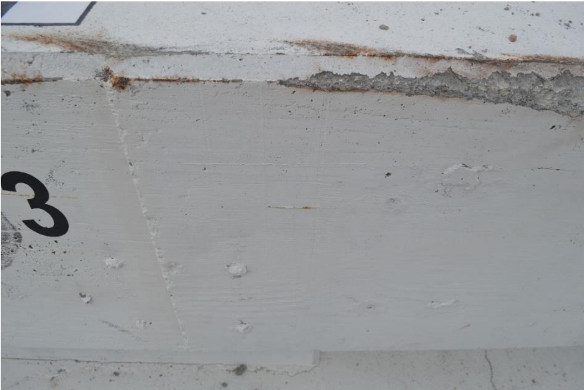
Figure 78. Concrete Beam and Deck Damage, Test No. OCBR-3
