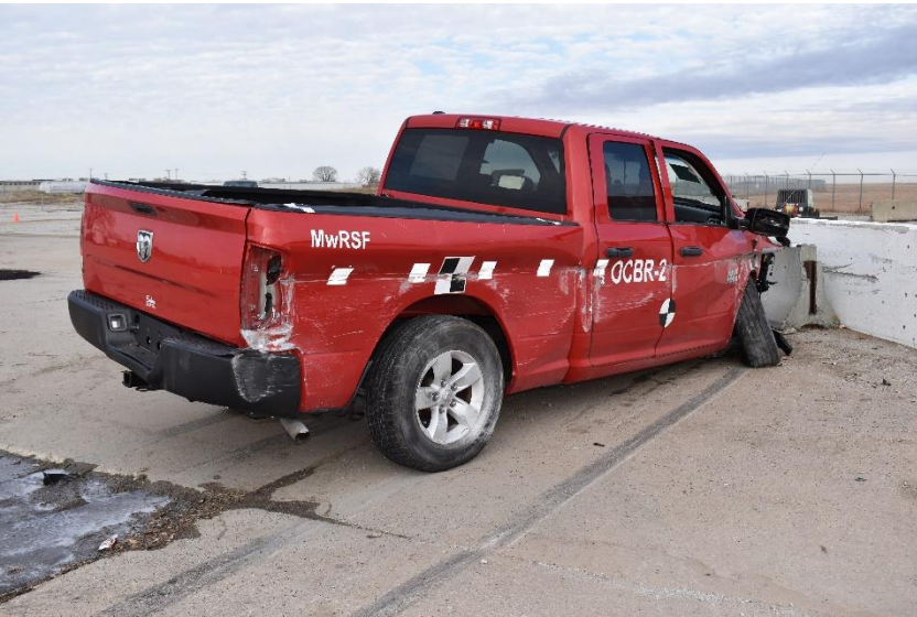
Figure 69. Vehicle Damage, Test No. OCBR-2
