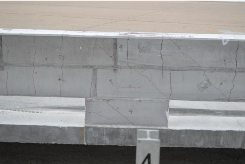
Figure 79. Concrete Beam and Post Damage, Post Nos. 3 and 4, Test No. OCBR-3
