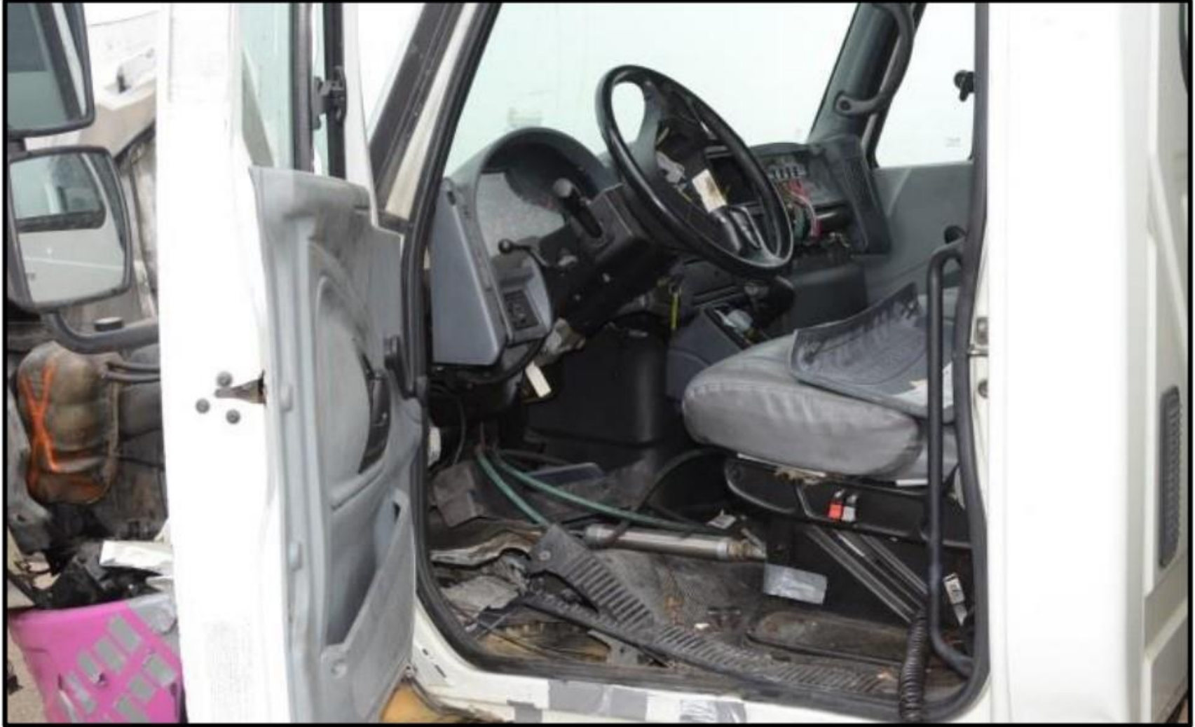
Figure 89. Vehicle Floor Pan Separation, 42-in. Tall Single Slope Barrier, Test No. 469467-1 [21]
