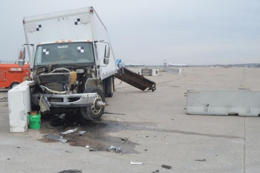
Figure 83. Vehicle Damage, Test No. OCBR-3
