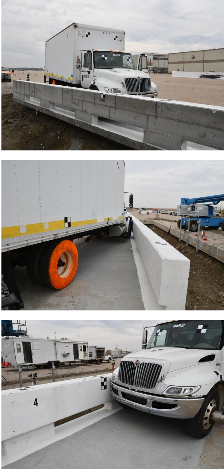
Figure 72. Target Impact Location, Test No. OCBR-3
