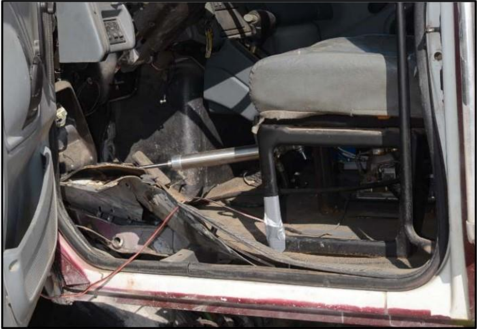
Figure 88. Vehicle Floor Pan Separation, TL-4 Barrier on Rubber Posts, Test No. 468958-3 [20]
