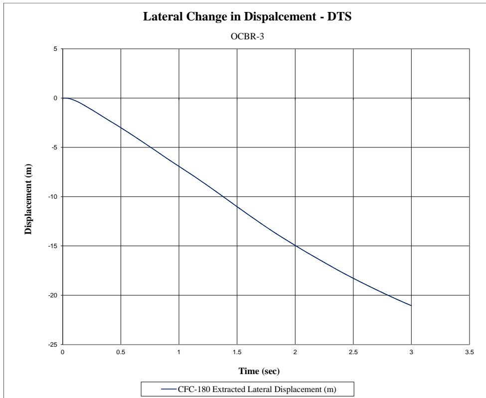
Figure F-22. Lateral Occupant Displacement (DTS), Test No. OCBR-3
