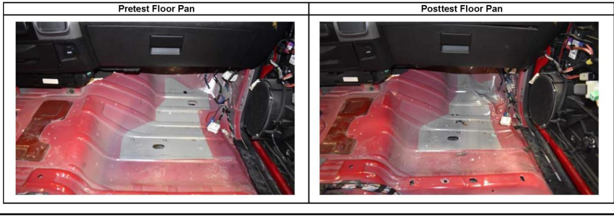
Figure C-7. Floor Pan Deformation Data – Set 2, Test No. OCBR-2
