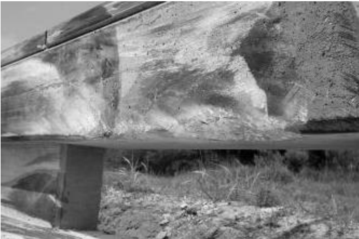
Figure 36. Lateral Extent of the 2000P Vehicle on the 30-in. Tall T203 Barrier [23]
