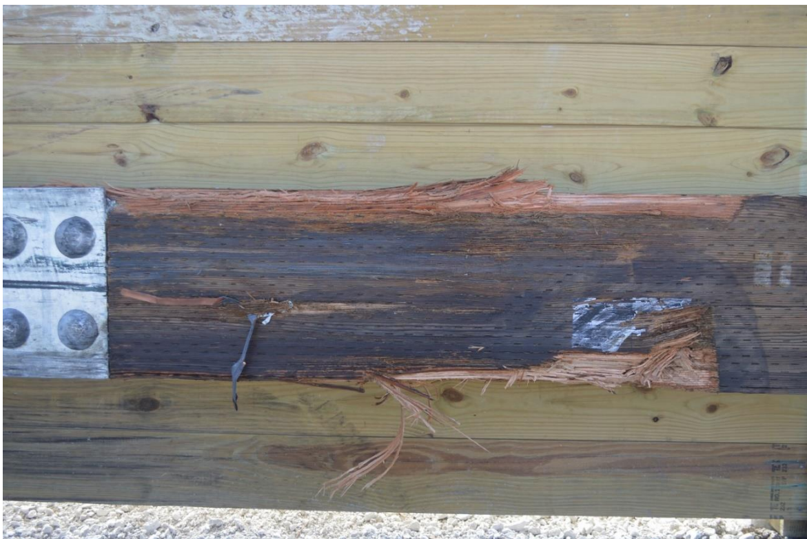
Figure 67. Lateral Extent of the 2270P Vehicle in. Test No. MNNW-3 on the Minnesota Noise Wall [33]
