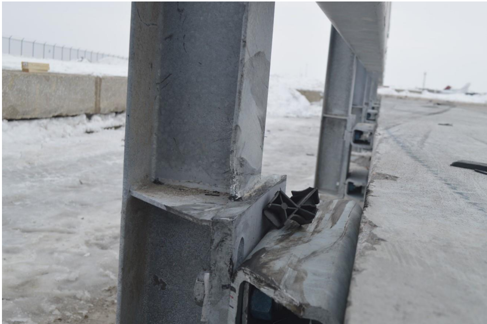
Figure 57. Lateral Extent of the 1100C Vehicle on the 39-in. Tall Illinois-Ohio Steel Bridge Rail [29-32]
