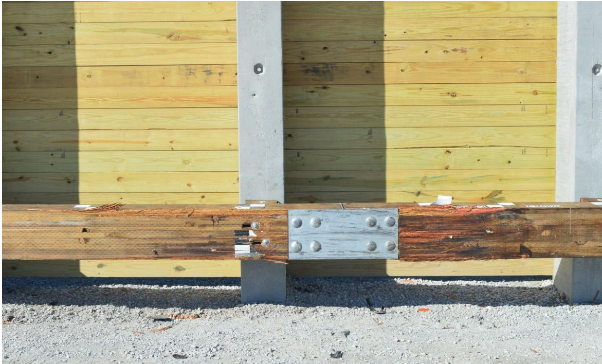
Figure 66. Lateral Extent of the 1100C Vehicle in. Test No. MNNW-2 on the Minnesota Noise Wall [33]
