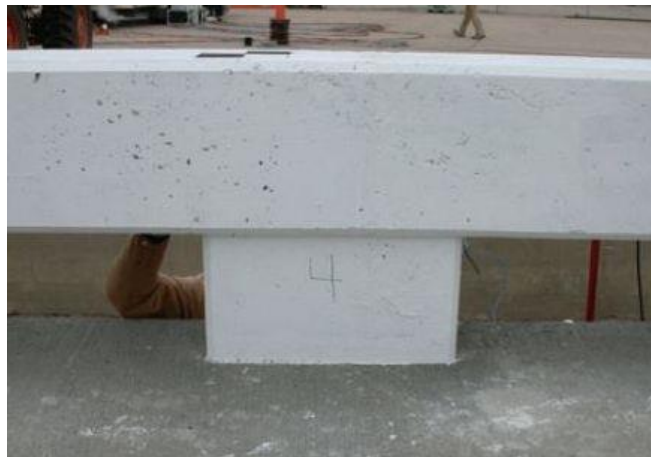
Figure 1. Rectangular Open Concrete Rail Posts [1]
