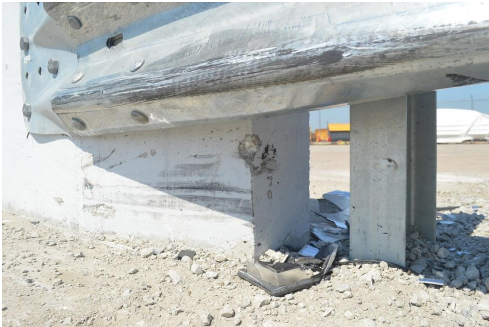
Figure 76. Lateral Extent of the Second 2270P Vehicle on the Standardized AGT Buttress, Test No. AGTB-2 [35]
