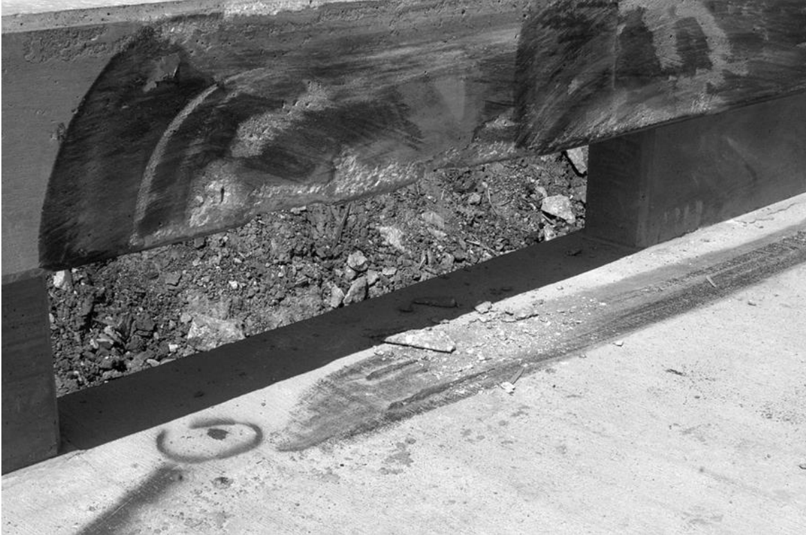
Figure 35. Lateral Extent of the 2000P Vehicle on the 27-in. Tall T203 Barrier [23]
