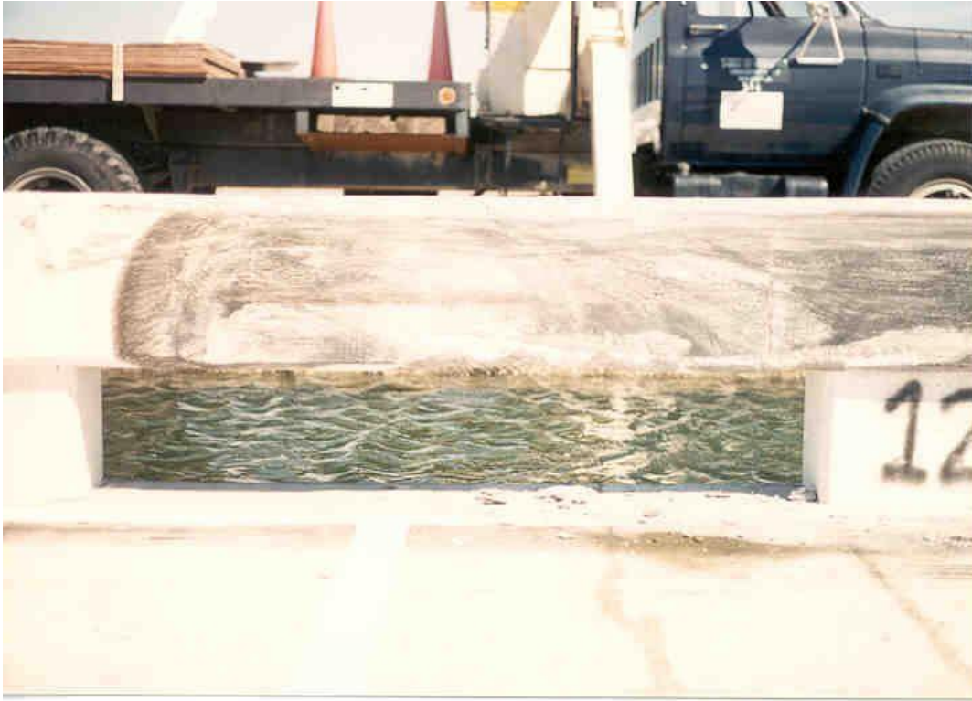
Figure 27. Lateral Extent of the 5,399-lb Pickup Truck on the Nebraska Open Concrete Rail [22]
