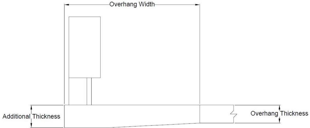
Figure 95. Overhang Width, Thickness, and Additional Thickness
