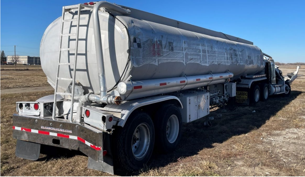
Figure 6.25 Trailer Damage After Uprighting, Test No. MTL6-1
