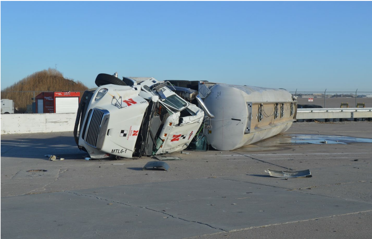
Figure 6.9 Vehicle Final Position and Trajectory Marks, Test No. MTL6-1
