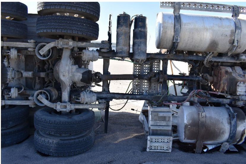
Figure 6.20 Tractor Undercarriage Chassis Damage, Test No. MTL6-1
