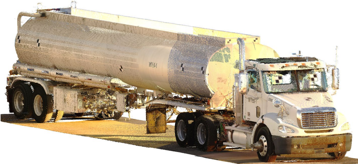
Figure 5.12 Images of 3D Point Clouds of Test Vehicle, Test No. MTL6-1
