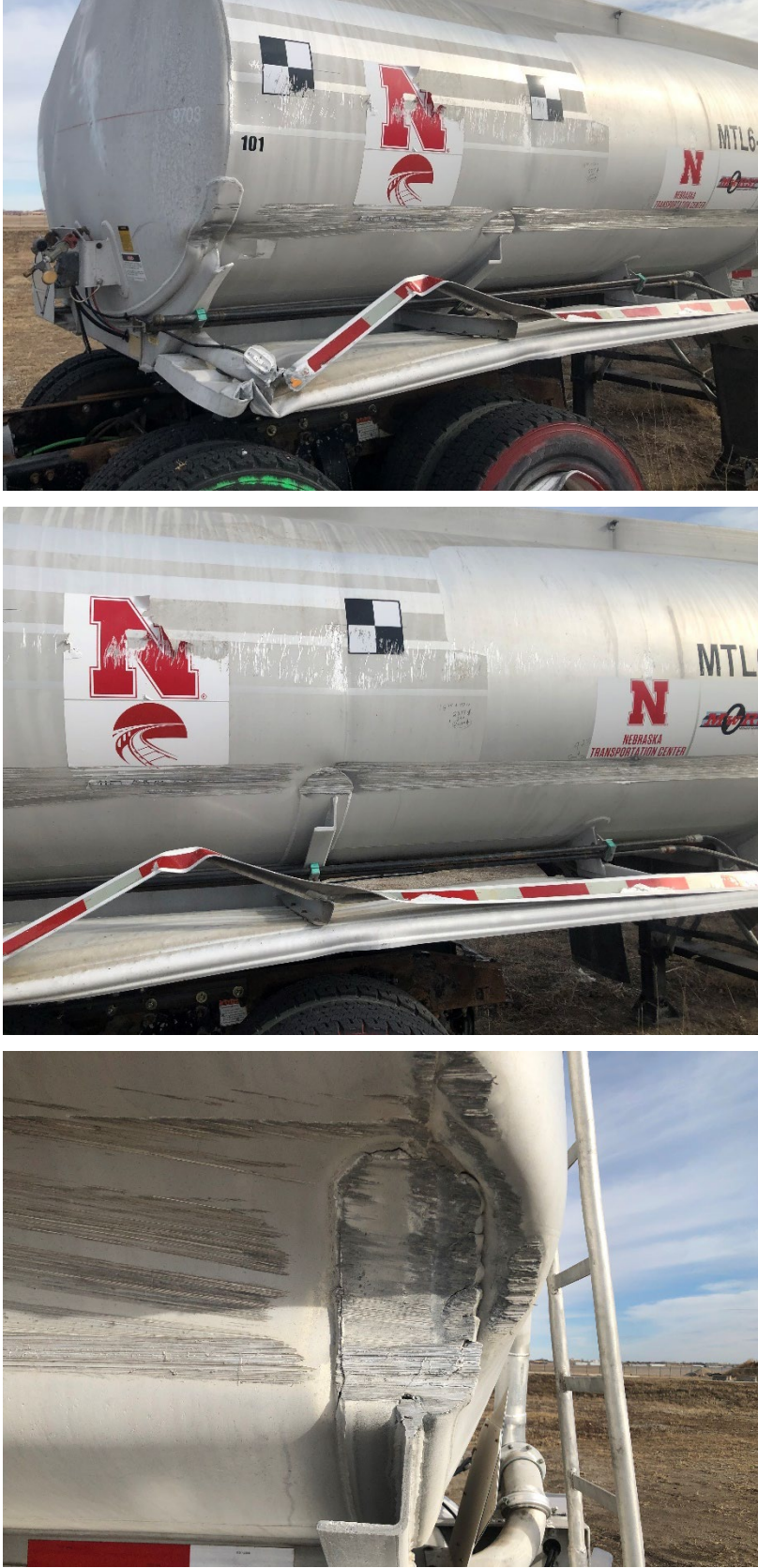
Figure 6.27 Trailer Damage on Impact Side After Being Uprighted, Test No. MTL6-1
