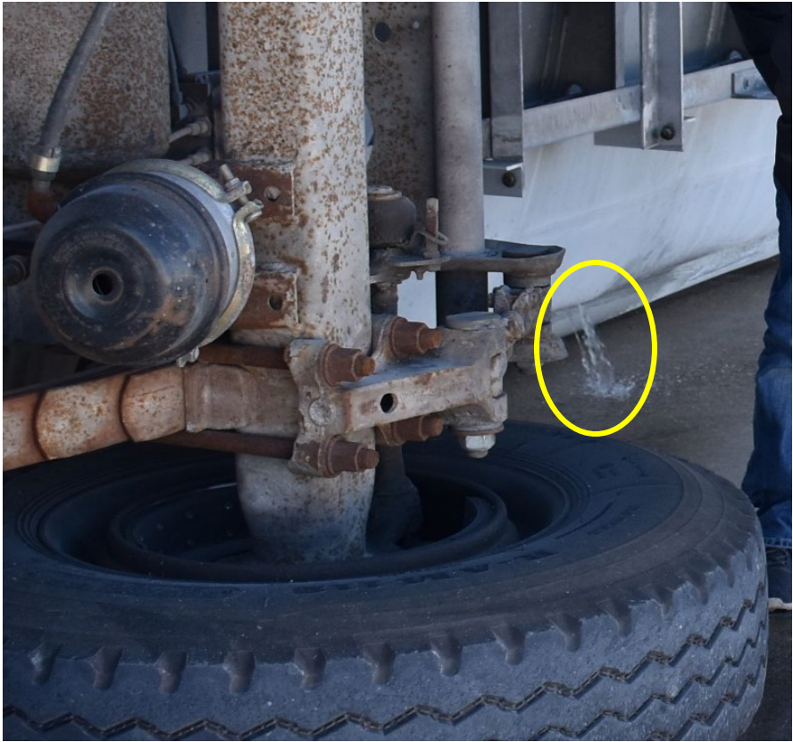
Figure 6.24 Locations of Trailer Leaks, Test No. MTL6-1
