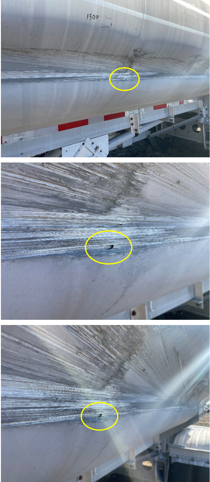
Figure 6.26 Pinhole Damage in Trailer After Being Uprighted, Test No. MTL6-1
