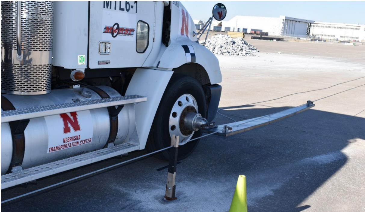
Figure 5.2 Test Vehicle Guidance System, Test No. MTL6-1
