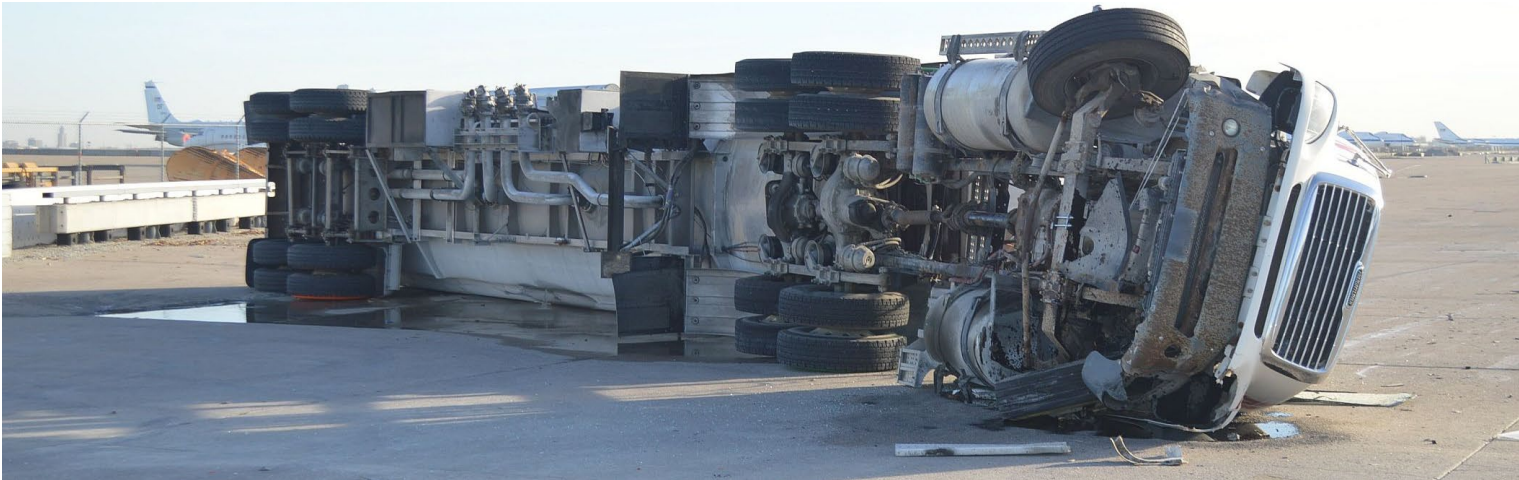
Figure 6.17 Vehicle Damage and Final Rest, Test No. MTL6-1
