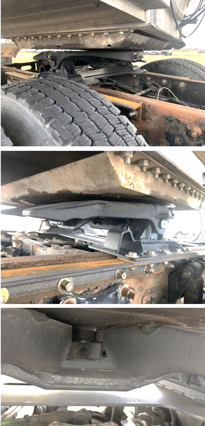
Figure 6.30 Fifth Wheel Damage, Test No. MTL6-1
