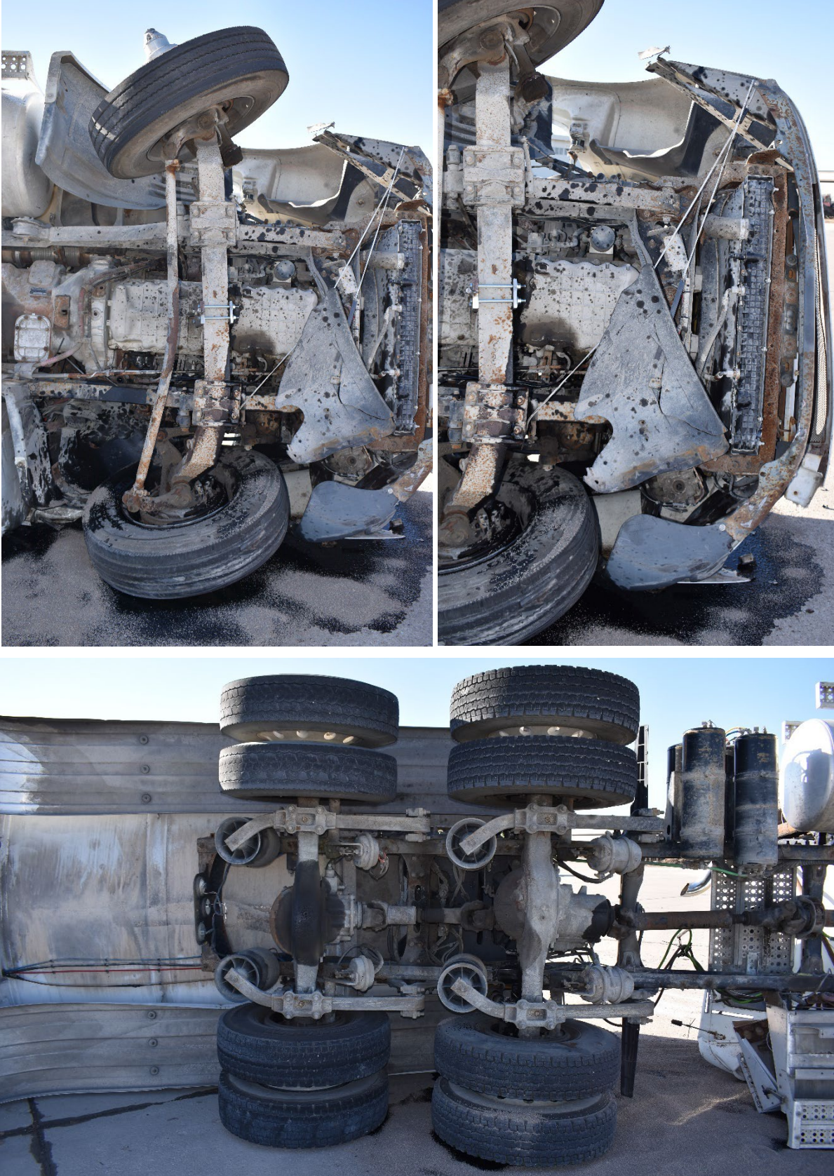
Figure 6.21 Tractor Suspension Damage, Test No. MTL6-1 101
