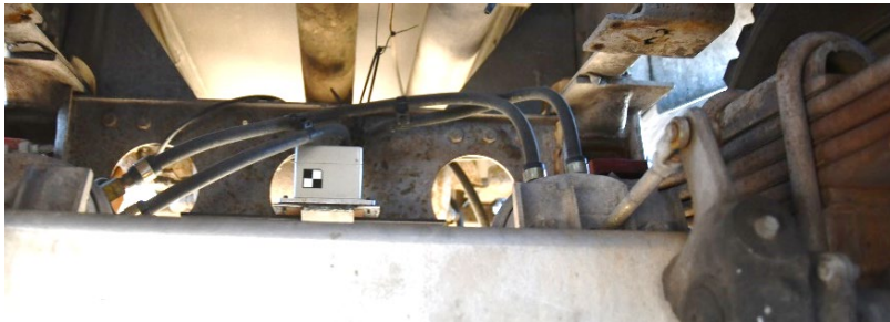
Figure 5.15 Accelerometer Mounting Locations, Test No. MTL6-1
