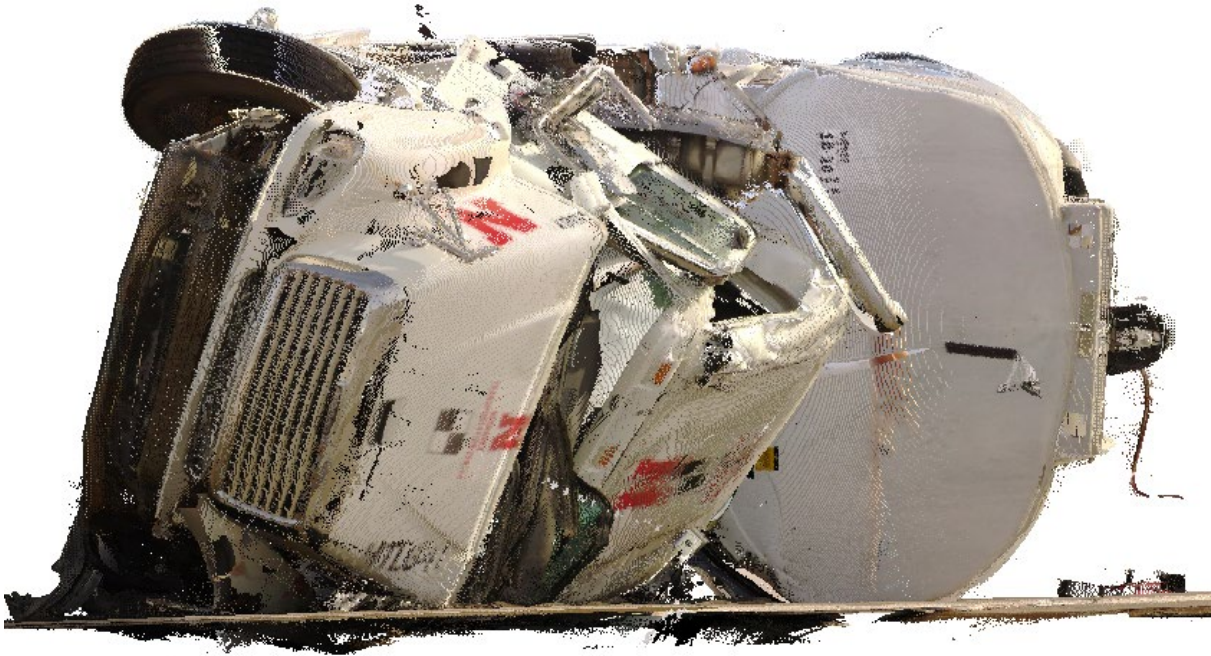
Figure 6.32 Vehicle Scan Results, Tractor Damage, Test No. MTL6-1
