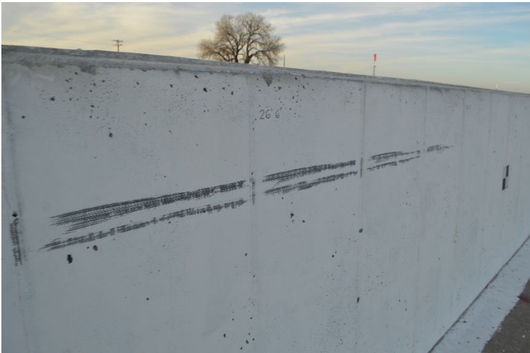
Figure 6.15 Scraping Damage along Top Impact-Side Edge of Barrier, Test No. MTL6-1
