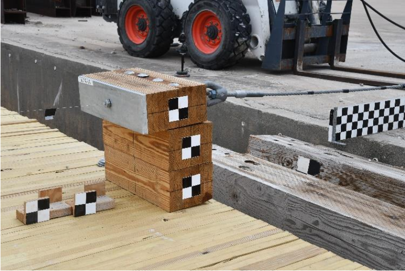
(a) Damage Sustained to Rail and Scupper Blocks
