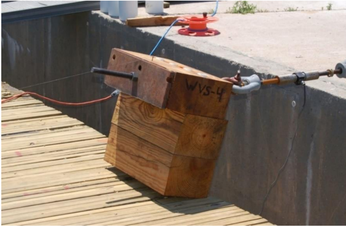
Figure 19. Deflected State in Static Test No. WVS-4 on WVDOT TL-1 Low-Height, Curb-Type, Glulam Bridge Railing [5-6]
