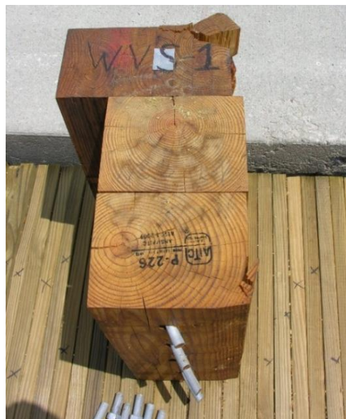
Figure 18. Test No. WVS-1 Scupper Block and Bolt Deformation [5-6]
