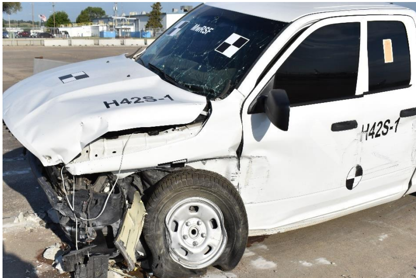
Figure 56. Vehicle Damage, Test No. H42S-1
