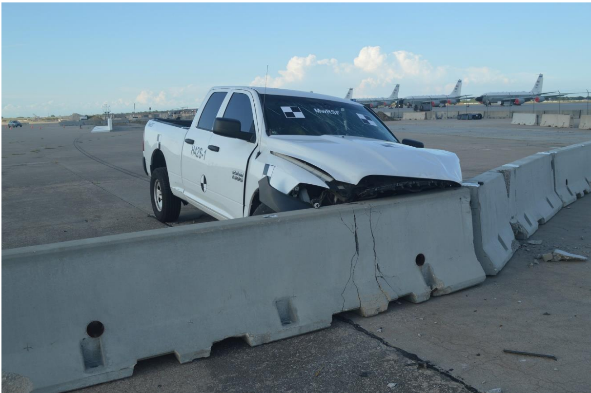
Figure 46. Vehicle Final Position and Trajectory Marks, Test No. H42S-1
