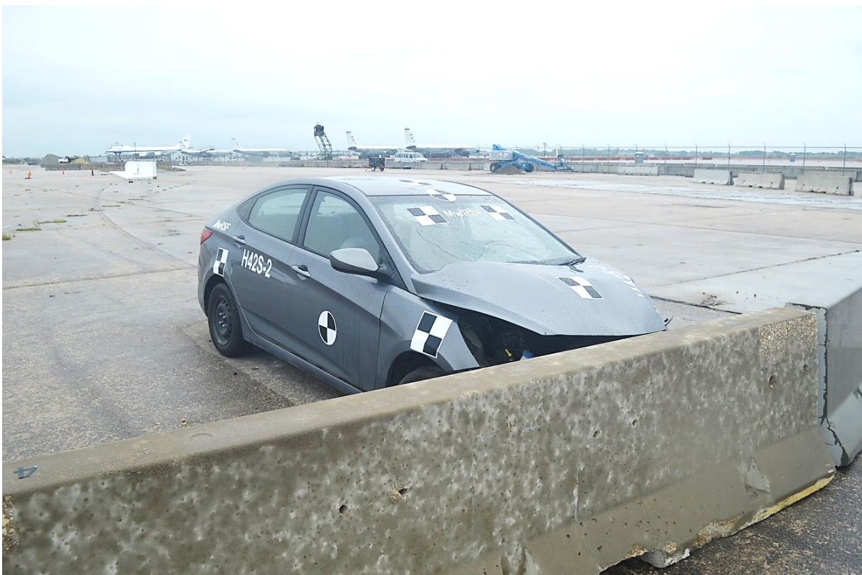
Figure 65. Vehicle Final Position and Trajectory Marks, Test No. H42S-2
