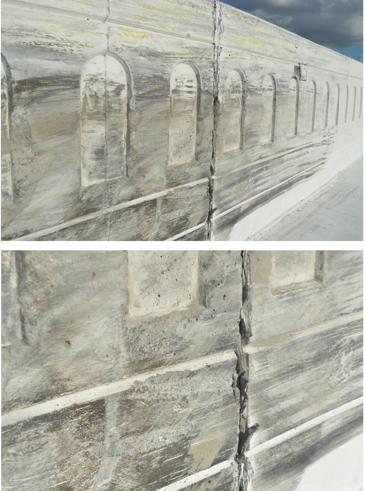
Figure 52. System Damage Due to Wheel Contact, Test No. H42S-1
