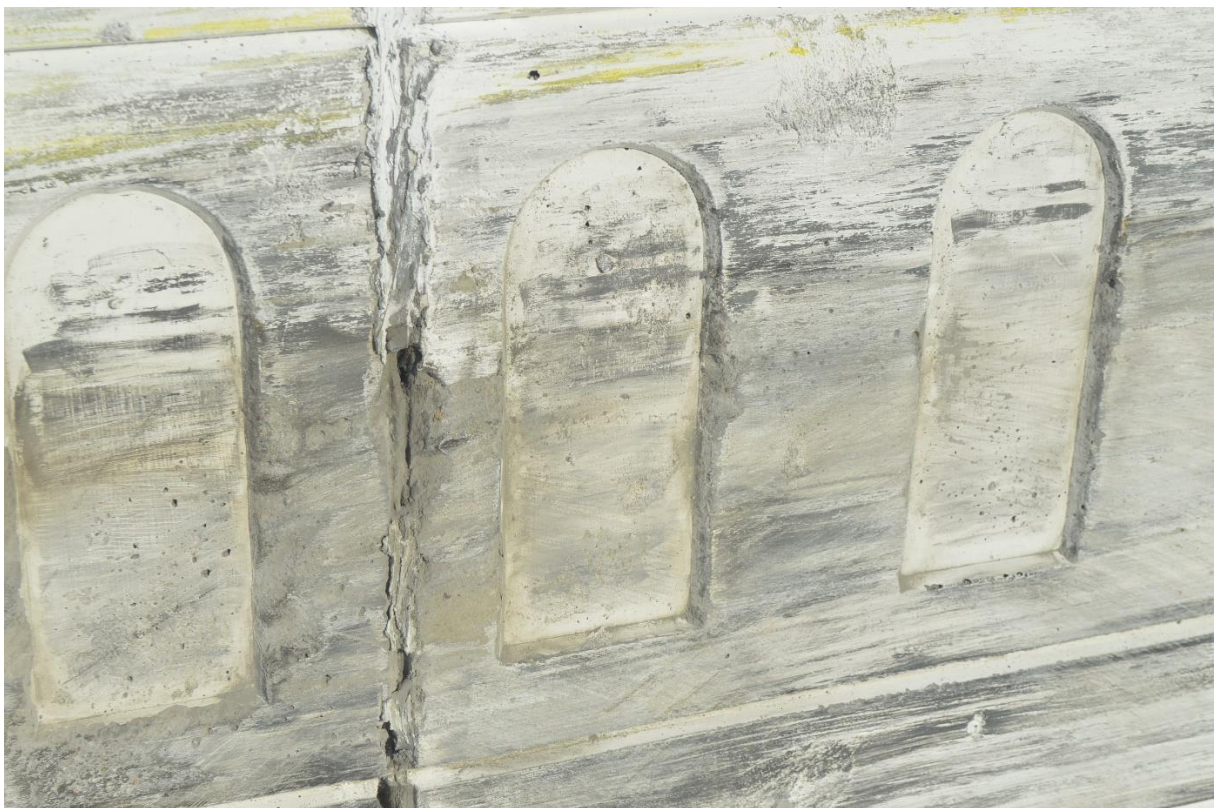
Figure 53. System Damage at Expansion Joint No. 1, Test No. H42S-1
