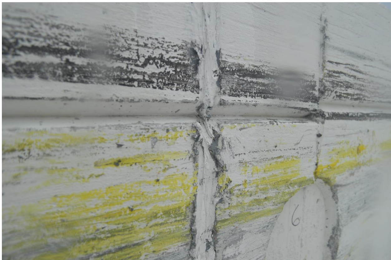
Figure 72. System Damage at Expansion Joint No. 2, Test No. H42S-2
