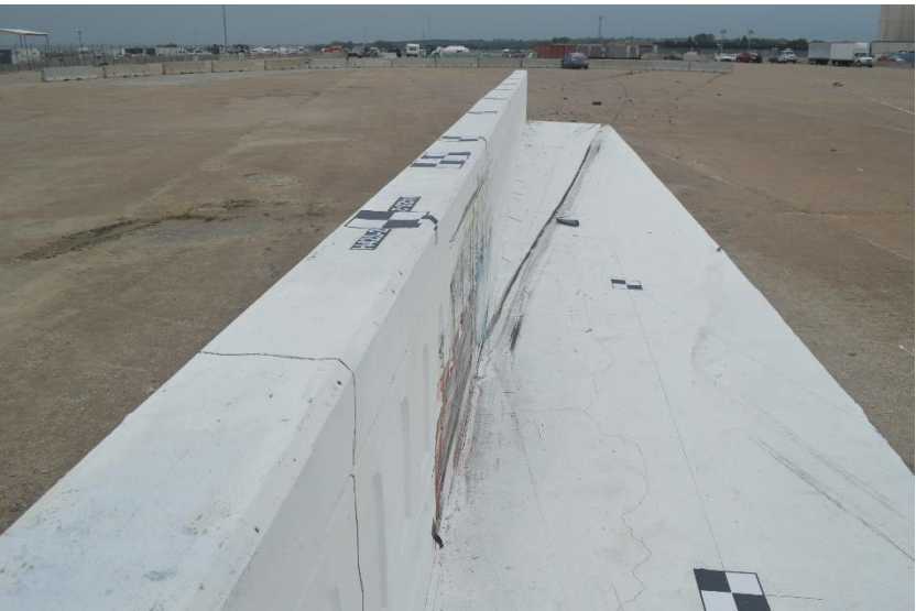
Figure 67. System Damage, Sidewalk, Test No. H42S-2
