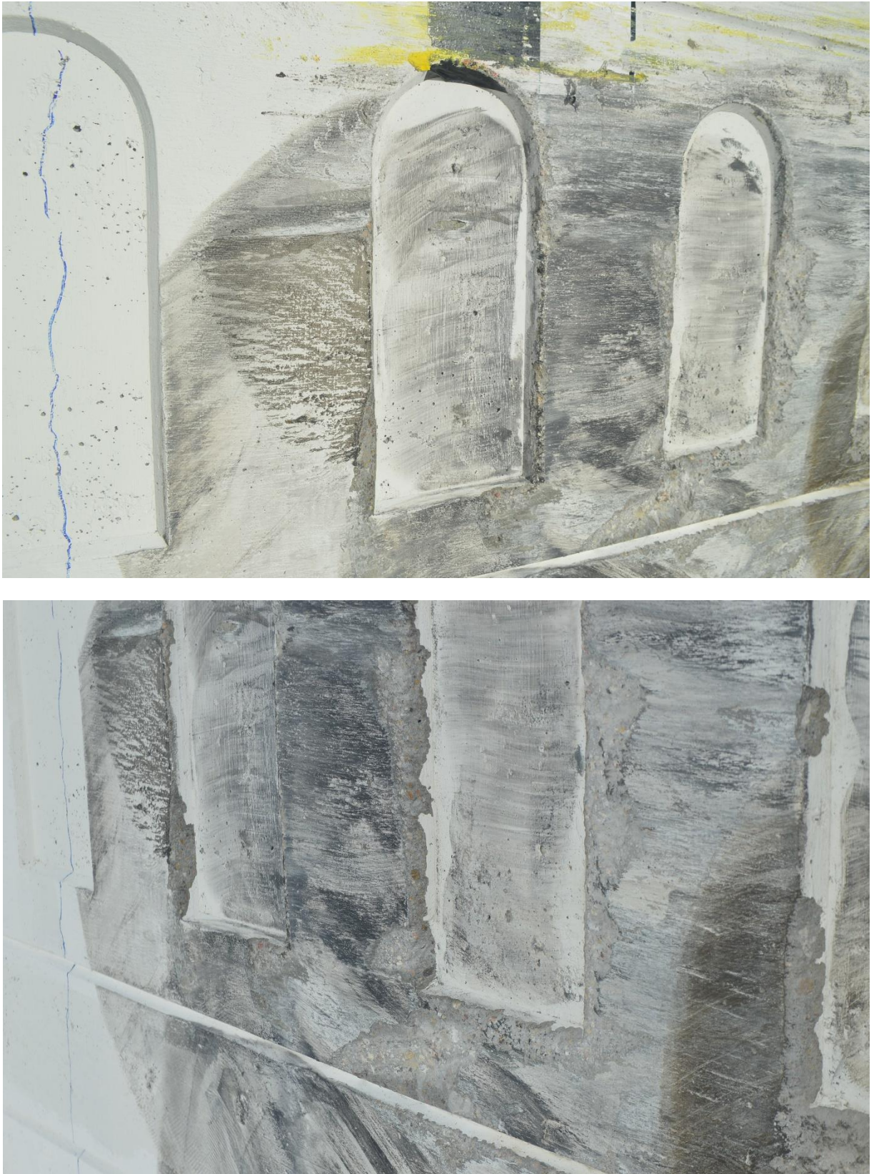
Figure 51. System Damage due to Wheel Contact, Test No. H42S-1
