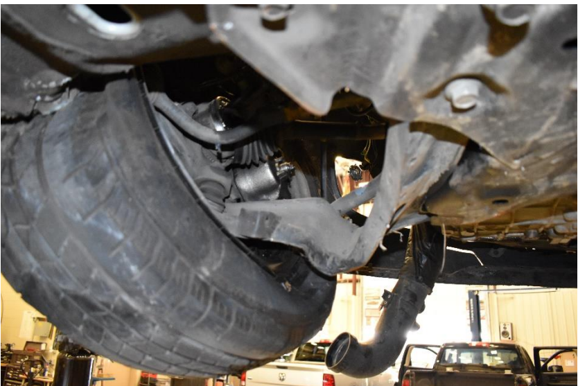
Figure 77. Vehicle Undercarriage Damage, Test No. H42S-2
