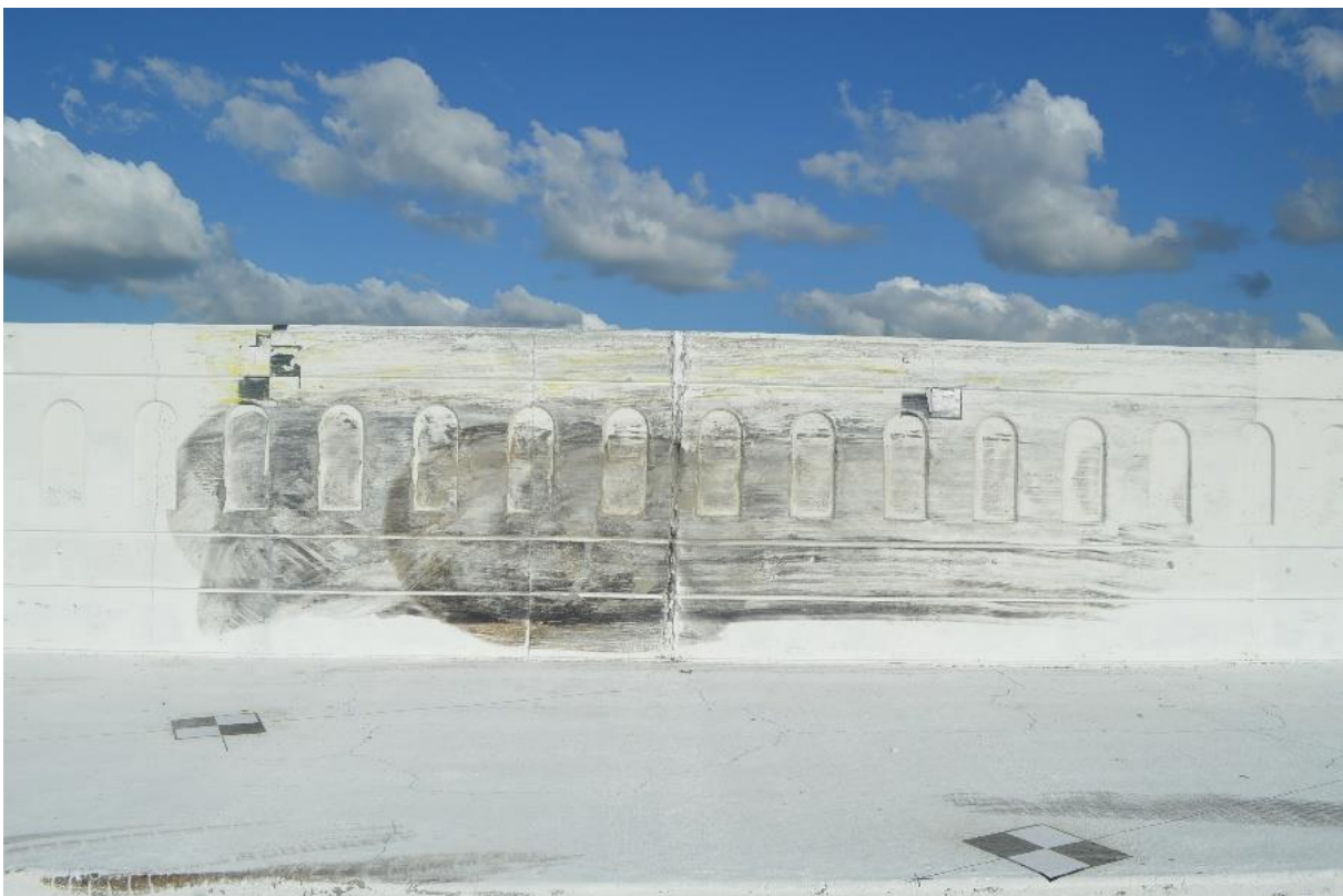
Figure 49. System Damage, Test No. H42S-1
