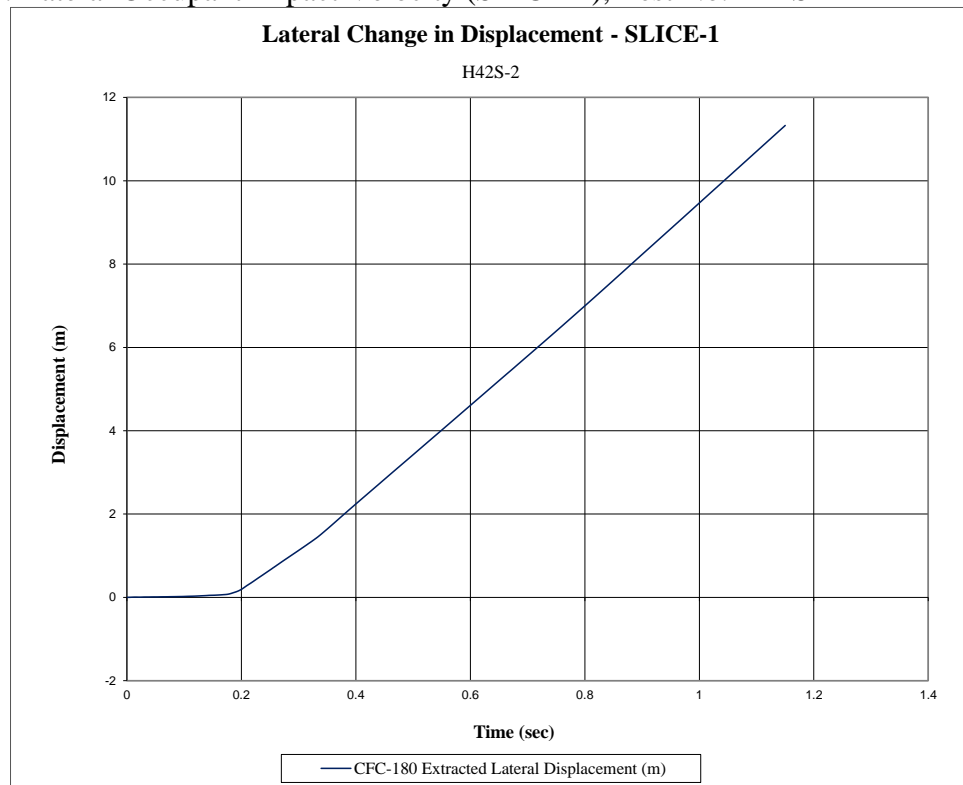
Figure E-6. Lateral Occupant Displacement (SLICE-1), Test No. H42S-2
