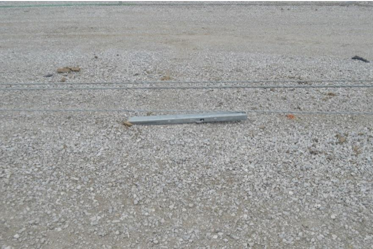
Figure 65. Post Nos. 51 (Left) and 52 (Right) Damage, Test No. MTP-1
