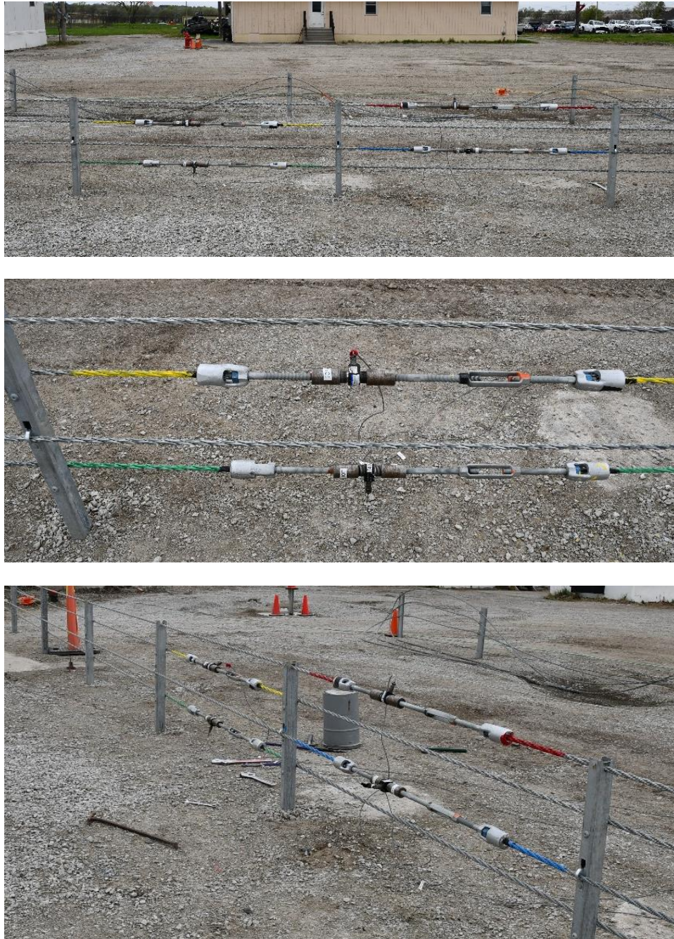
Figure 9. Location and Setup of Load Cells, Test No. MTP-1
