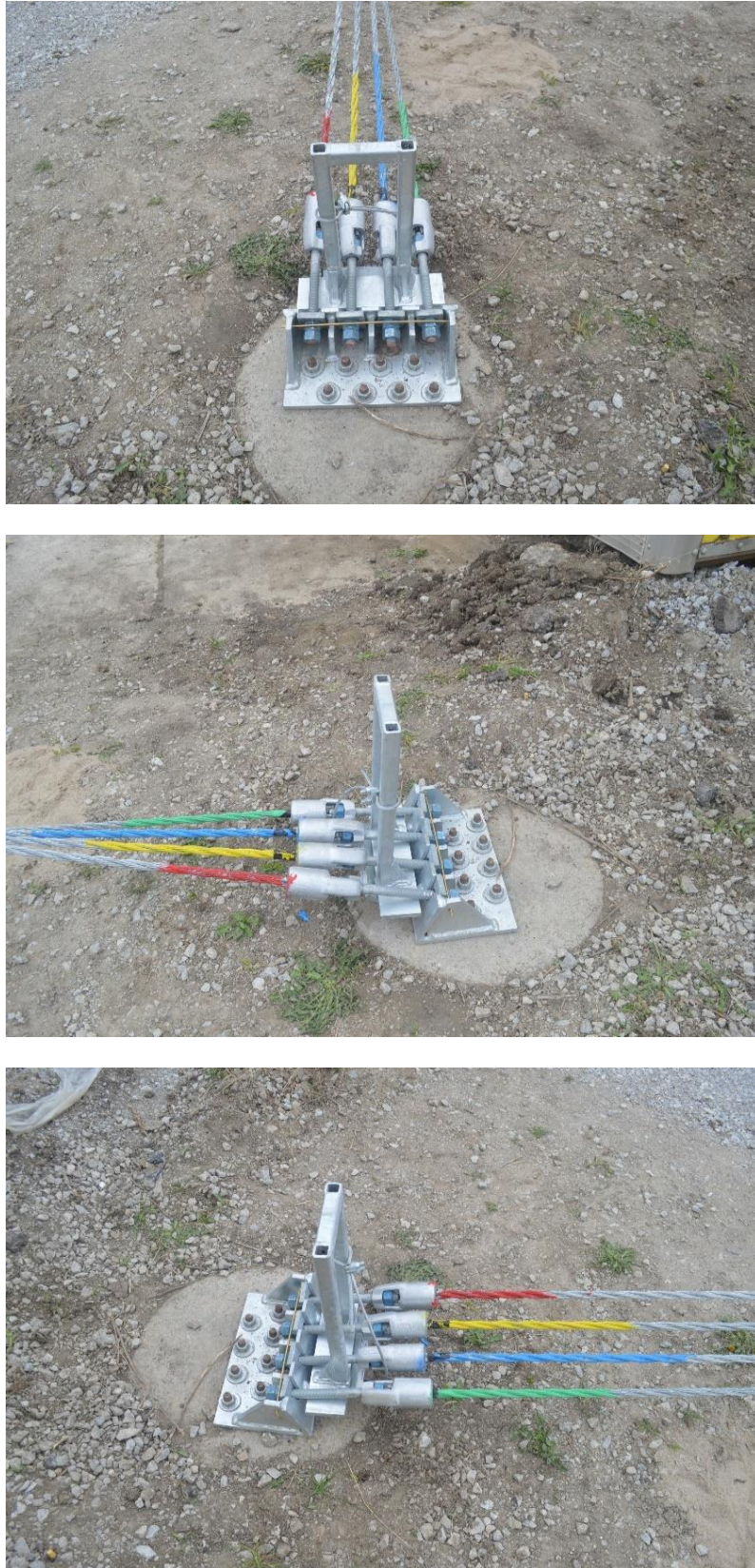
Figure 75. Post-Test Upstream Anchorage, Test No. MTP-1
