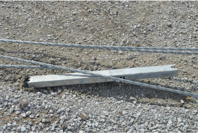
Figure 68. Post Nos. 57 (Left) and 58 (Right) Damage, Test No. MTP-1
