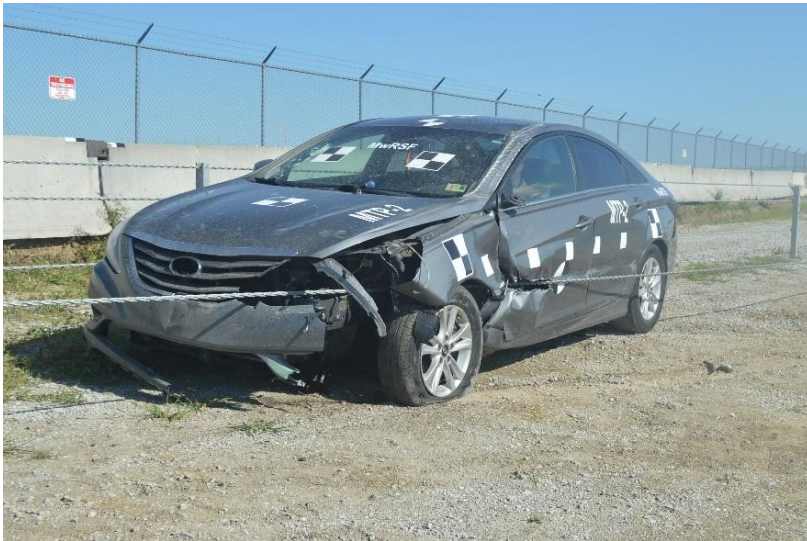
Figure 139. Vehicle Damage, Test No. MTP-2
