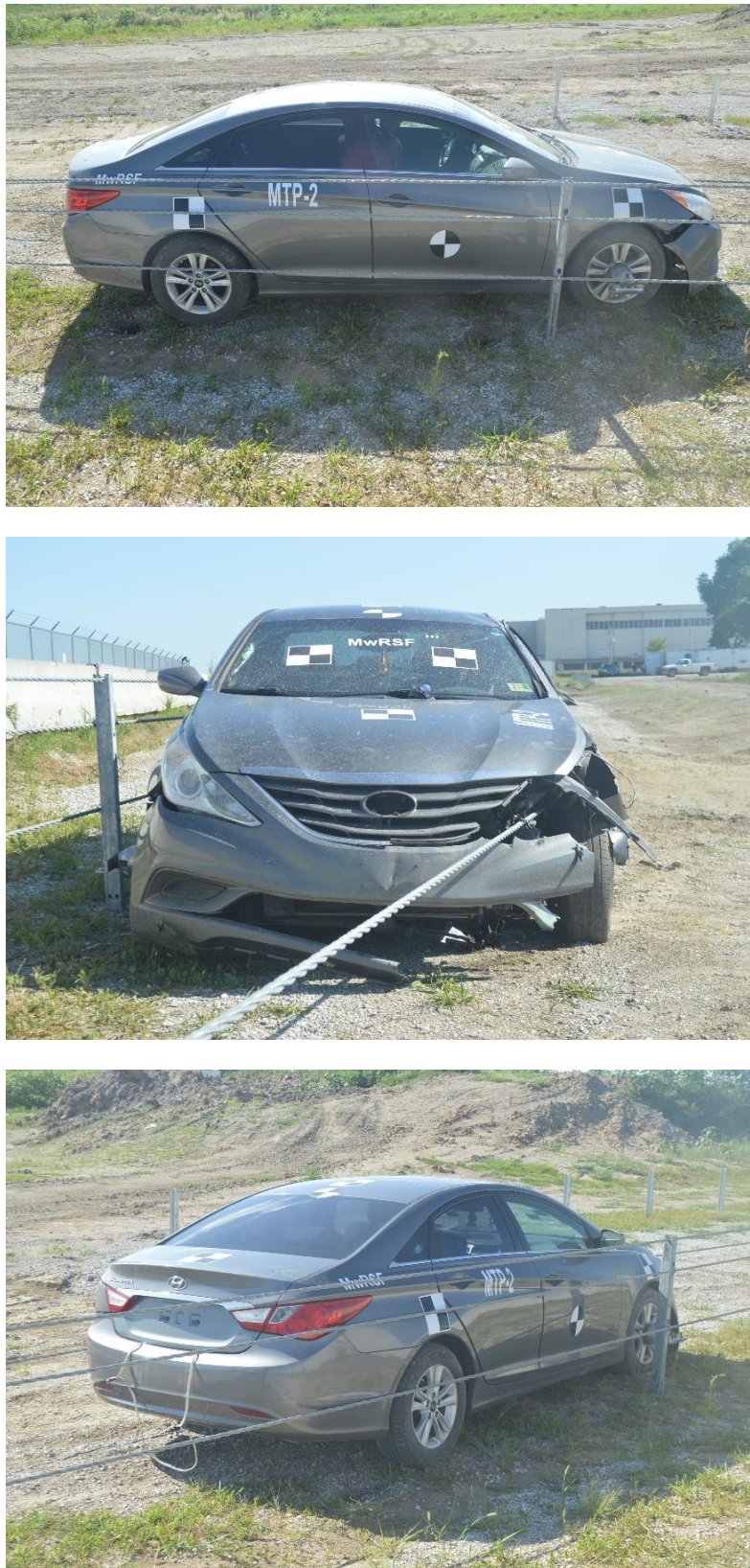
Figure 140. Additional Vehicle Damage, Test No. MTP-2
