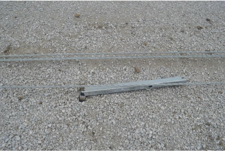
Figure 64. Post Nos. 49 (Left) and 50 (Right) Damage, Test No. MTP-1
