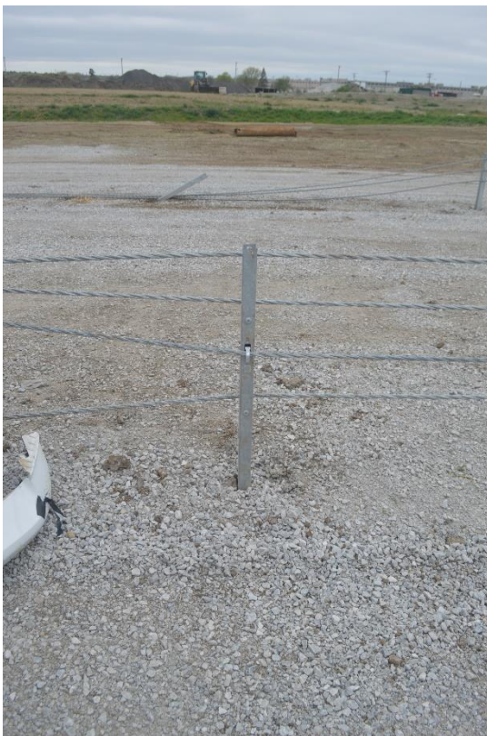
Figure 70. Post Nos. 59 (Left) and 60 (Right) Damage, Test No. MTP-1
