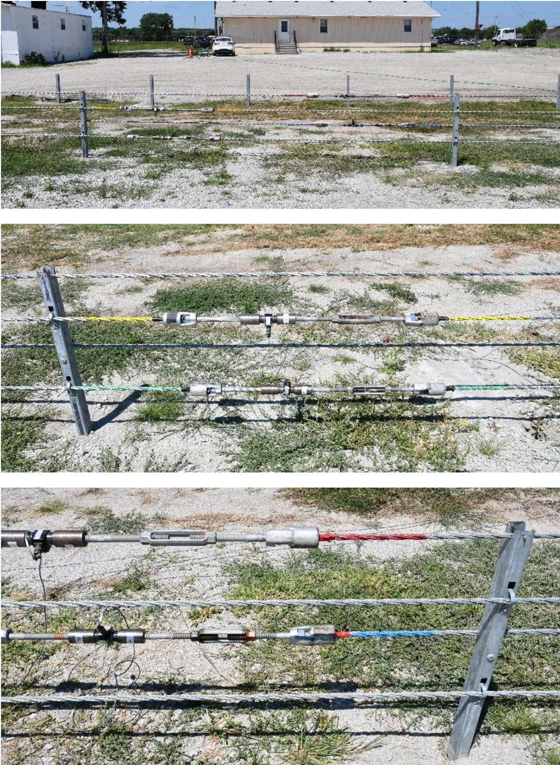
Figure 10. Location and Setup of Load Cells, Test No. MTP-2
