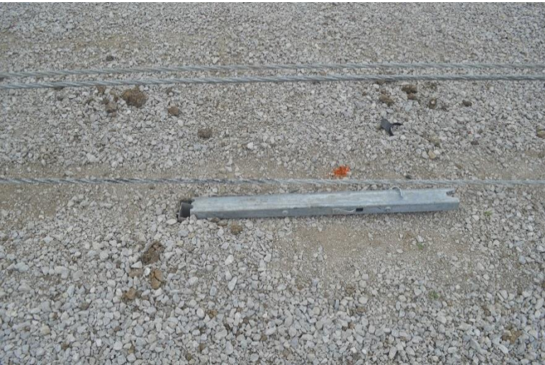
Figure 66. Post Nos. 53 (Left) and 54 (Right) Damage, Test No. MTP-1
