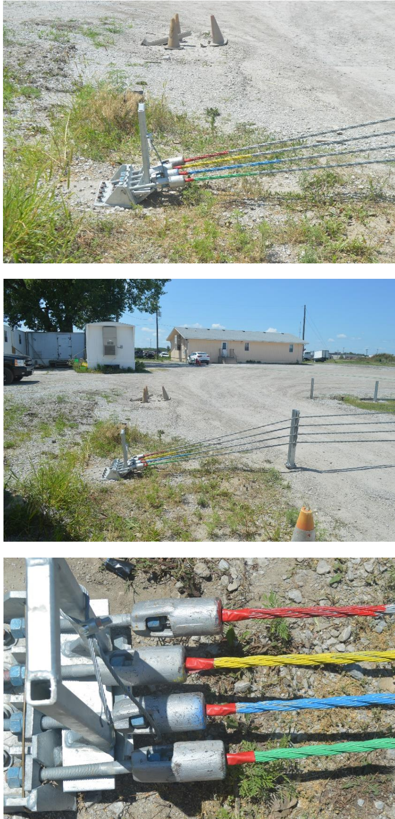
Figure 137. Post-Test Upstream Anchor, Test No. MTP-2
