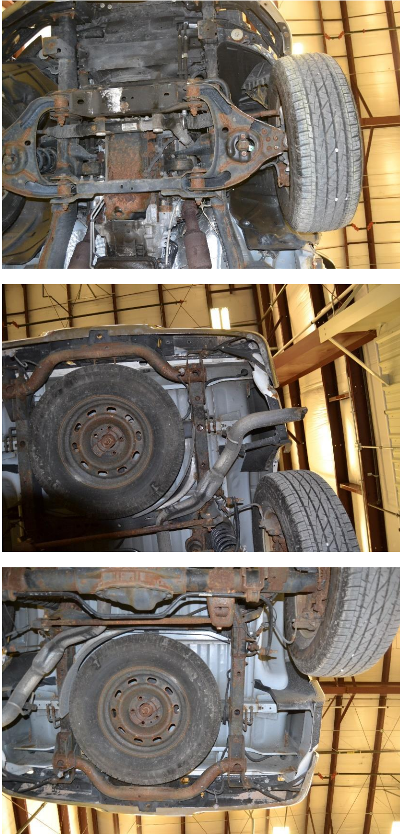
Figure 80. Vehicle Undercarriage Damage, Test No. MTP-1
