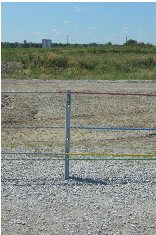
Figure 124. Post Nos. 14 (Left) and 15 (Right) Damage, Test No. MTP-2
