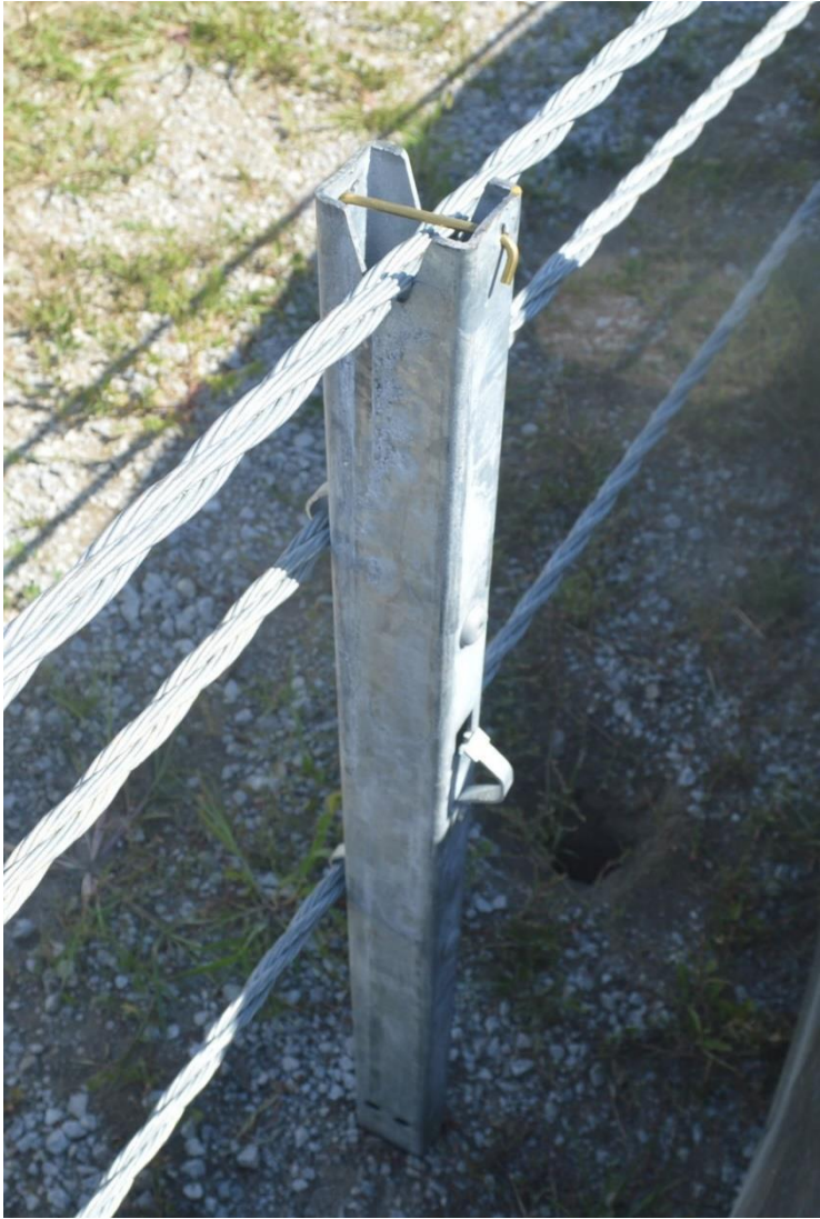
Figure 134. Post No. 33 Damage with Vehicle, Test No. MTP-2
