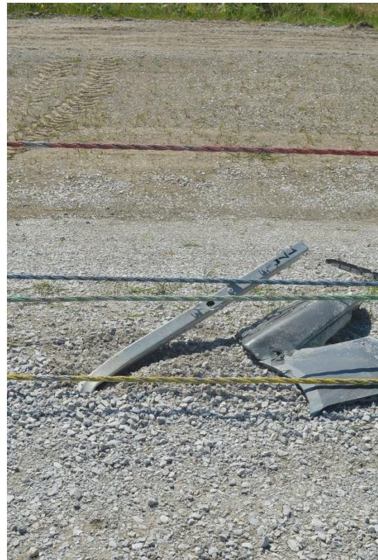
Figure 125. Post Nos. 16 (Left) and 17 (Right) Damage, Test No. MTP-2
