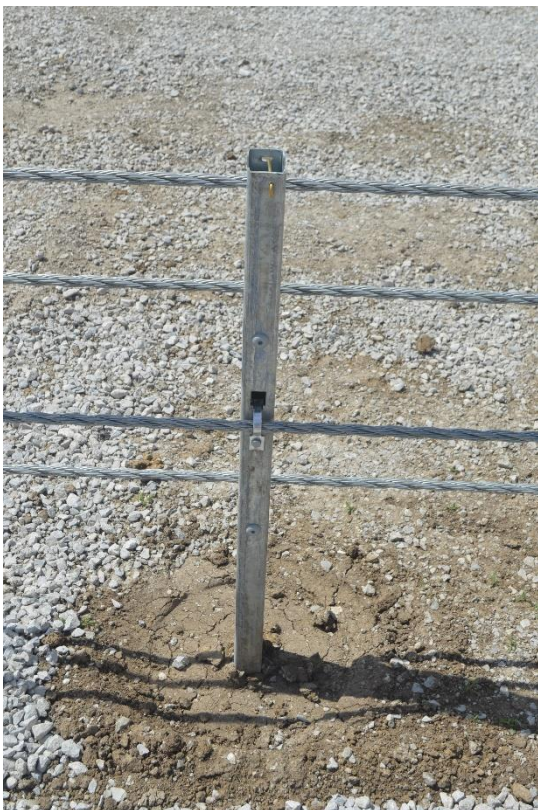
Figure 71. Post Nos. 61 (Left) and 62 (Right) Damage, Test No. MTP-1
