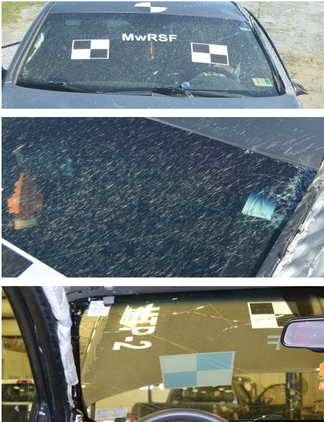
Figure 143. Vehicle Windshield Damage, Test No. MTP-2
