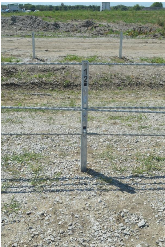
Figure 123. Post Nos. 12 (Left) and 13 (Right) Damage, Test No. MTP-2
