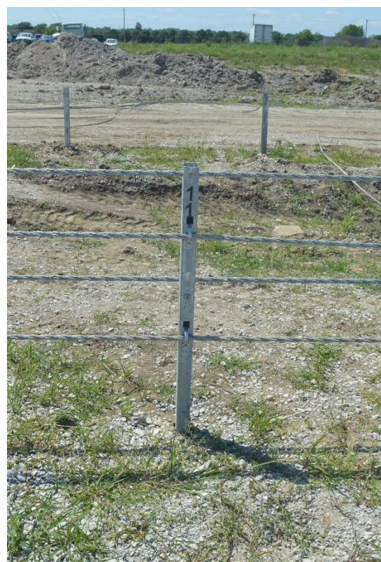
Figure 122. Post Nos. 10 (Left) and 11 (Right) Damage, Test No. MTP-2
