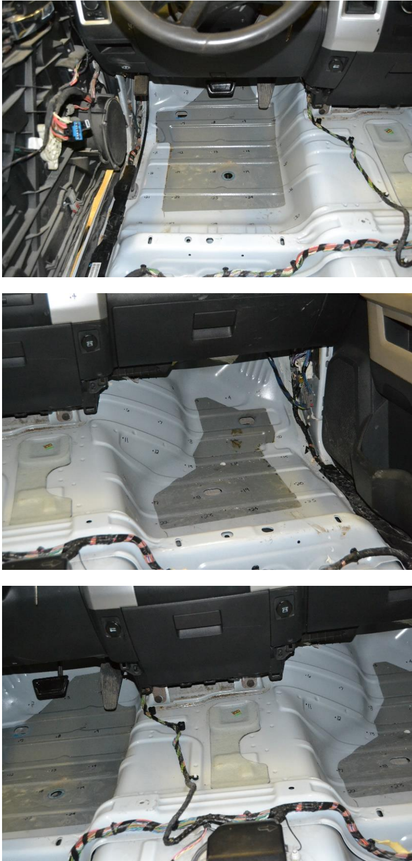
Figure 79. Occupant Compartment Damage, Test No. MTP-1
