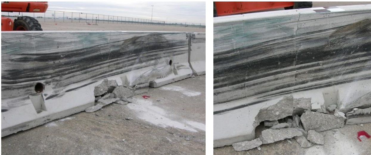
Figure 1. F-Shape PCB Deflection and Damage in MASH Testing with 2270P Vehicle [6]
