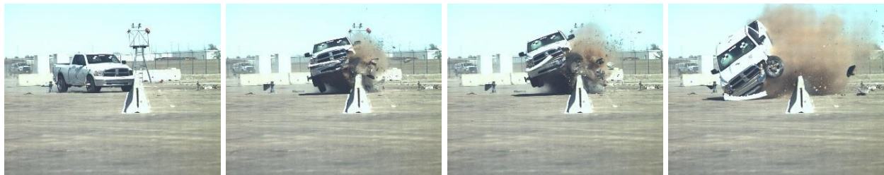
Figure 2. Vehicle Climb, Roll, and Pitch Motions with Safety Shape PCB [8]
