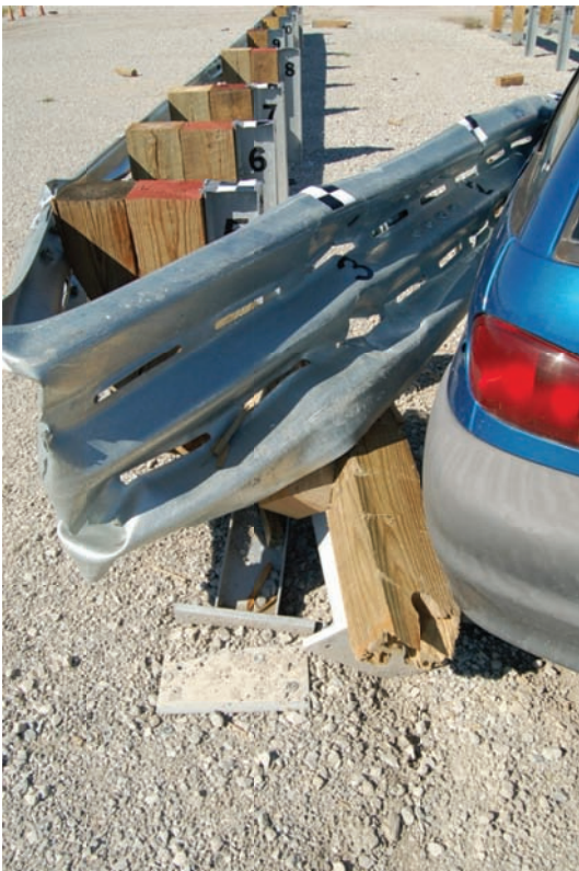
Figure 40. System Damage, Test No. USPBN-3
