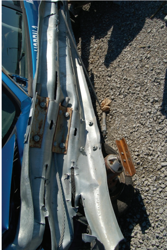
Figure 42. System Damage, Test No. USPN-3
