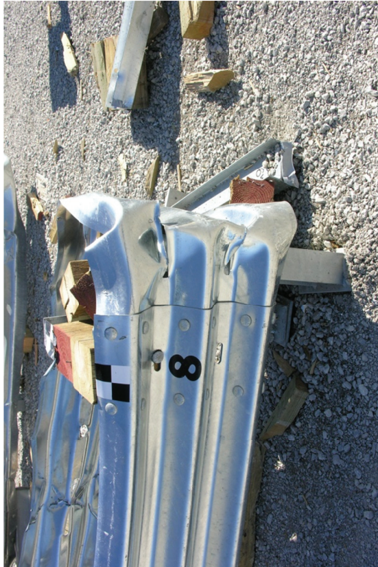
Figure 52. System Damage, Test No. USPBN-4
