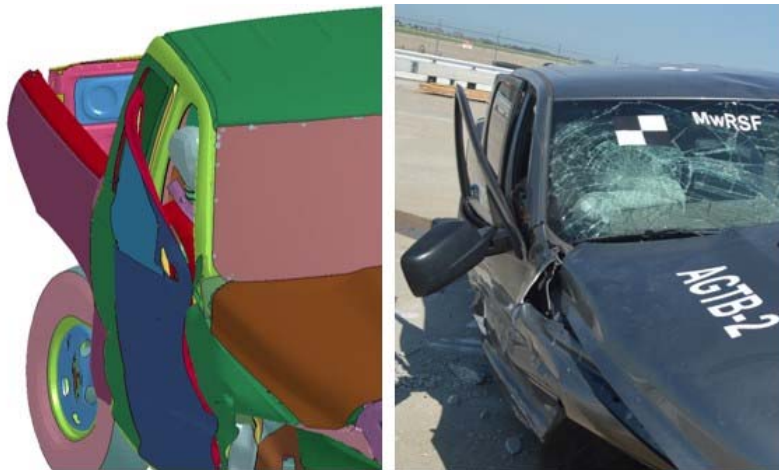
Figure 26. Right-Front Door Deformation with ATD, Simulation No. agt-v18--Ram and Test No. AGTB-2
