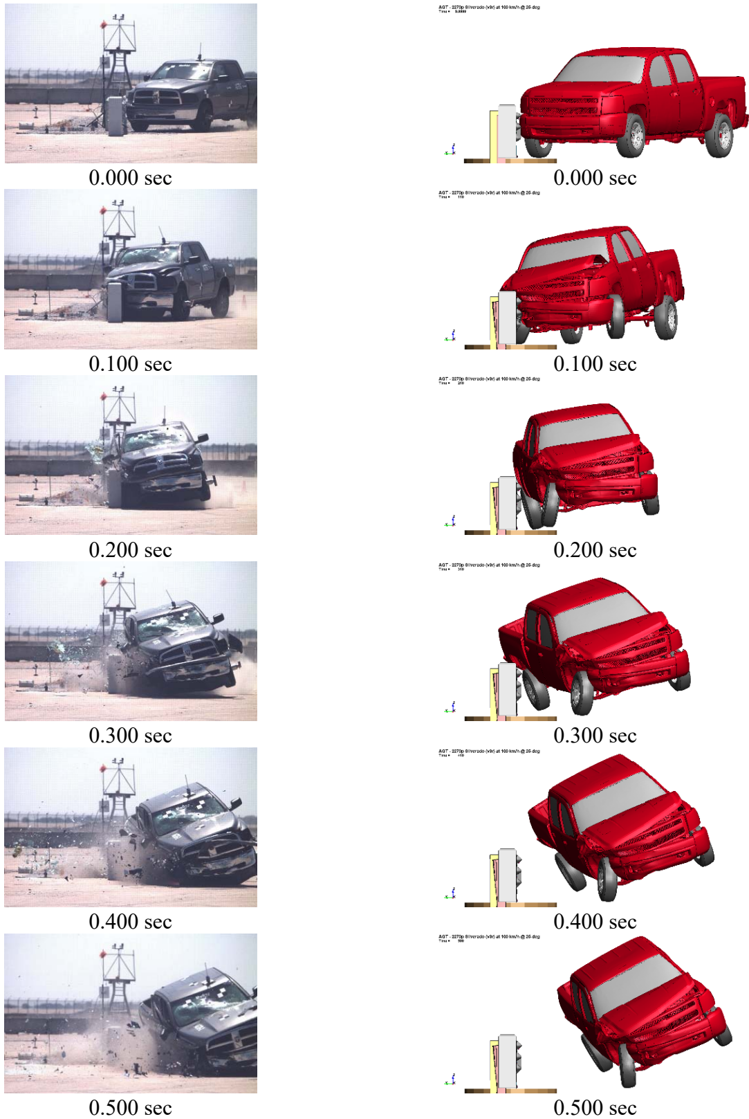
Figure 30. Sequential Images, Test No. AGTB-2 (Left) vs. Simulation No. agt-v3r-v15-single-thrie (Right)
