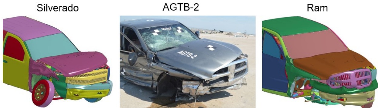
Figure 20. Right-Front Vehicle Deformation Comparison
