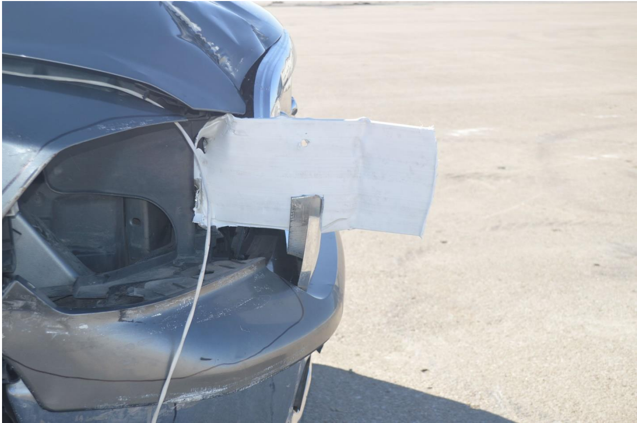
Figure 30. Vehicle Damage Details, Test No. WZNP-2
