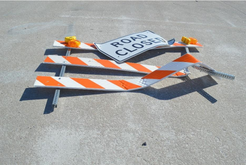
Figure 26. Additional System A Damage, Test No. WZNP-2
