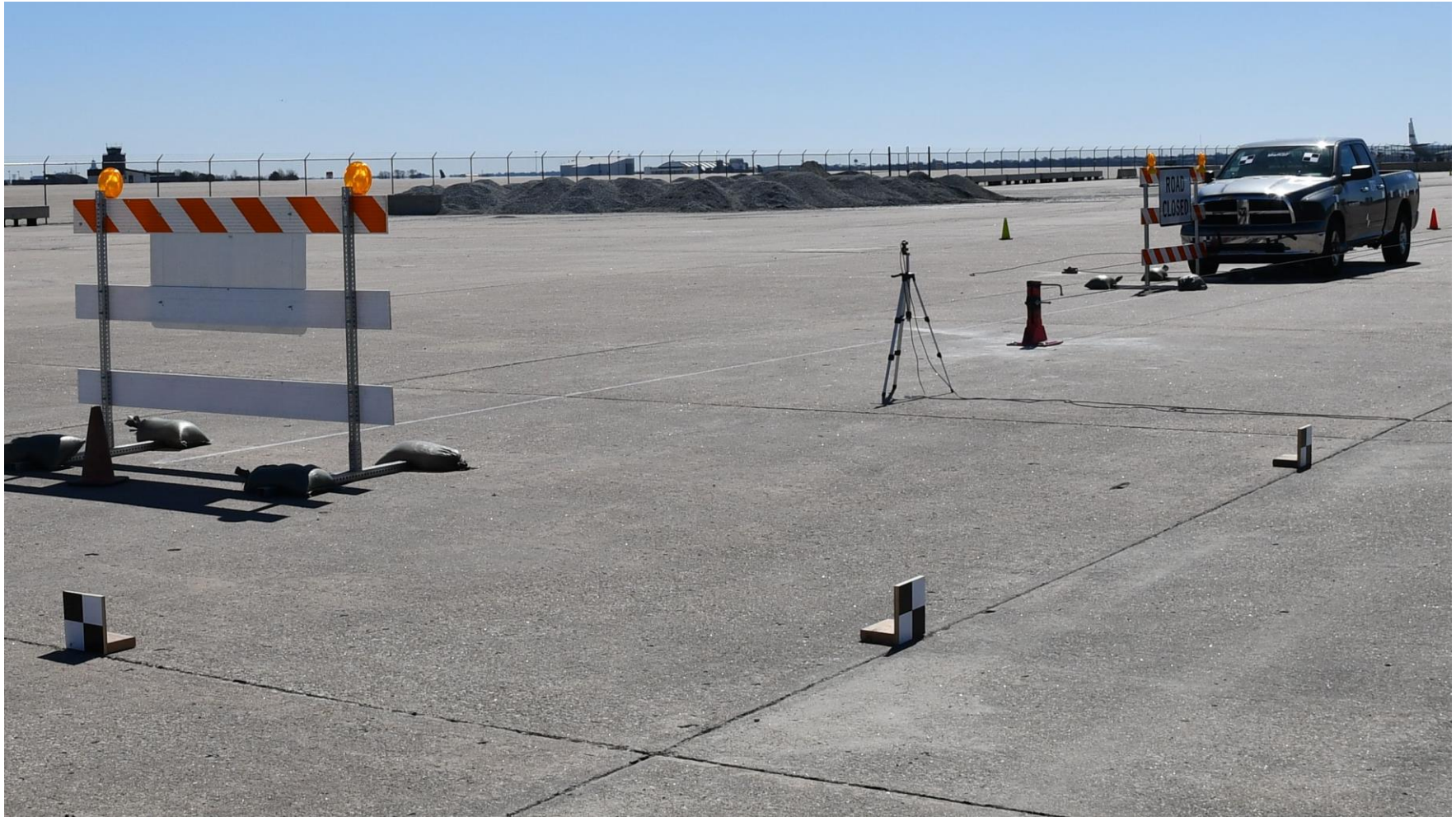
Figure 11. Test Impact Point, Test No. WZNP-2
