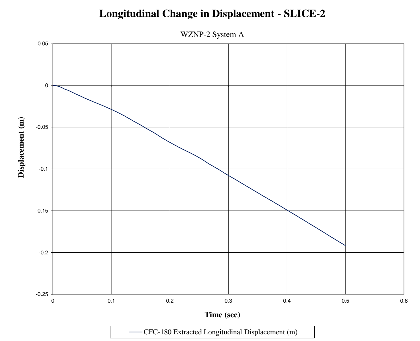
Figure D-11. Longitudinal Occupant Displacement System A (SLICE-2), Test No. WZNP-2
