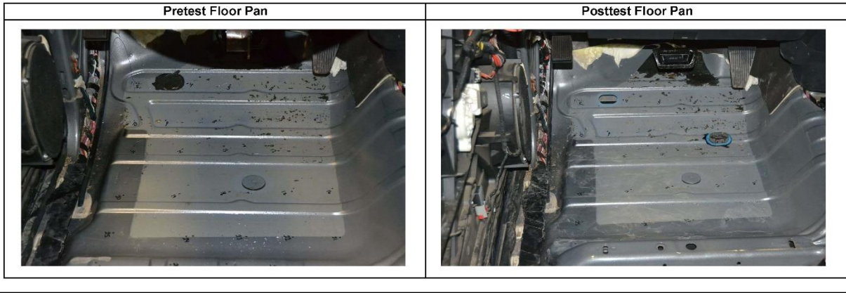
Figure C-1. Left Floor Pan Deformation Data – Set 1, Test No. WZNP-2
