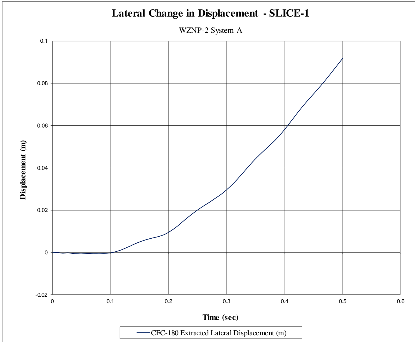
Figure D-6. Lateral Occupant Displacement System A (SLICE-1), Test No. WZNP-2
