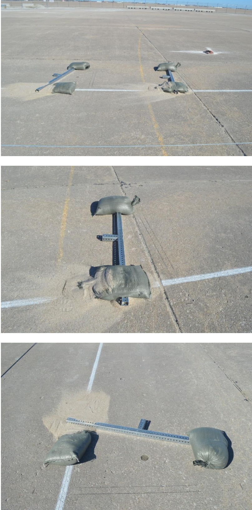
Figure 25. System A Damage, Test No. WZNP-2
