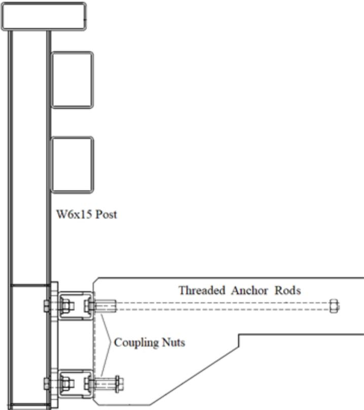
Figure 6. Anchorage Hardware Shown within Bridge Deck
