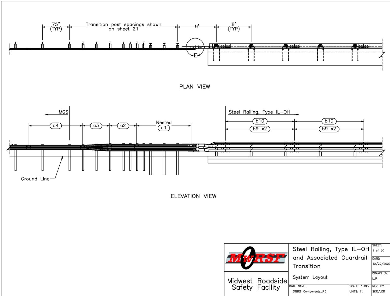
Figure A-1. Steel Railing, Type IL-OH and Associated Guardrail Transition
