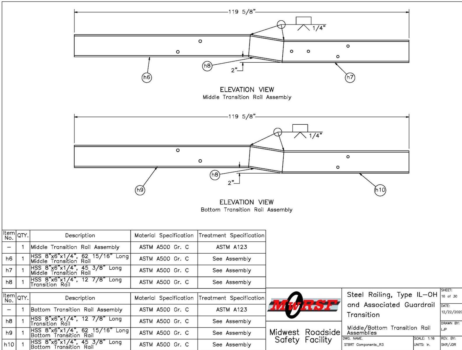
Figure A-16. Steel Railing, Type IL-OH, Middle and Bottom Transition Tube Rails
