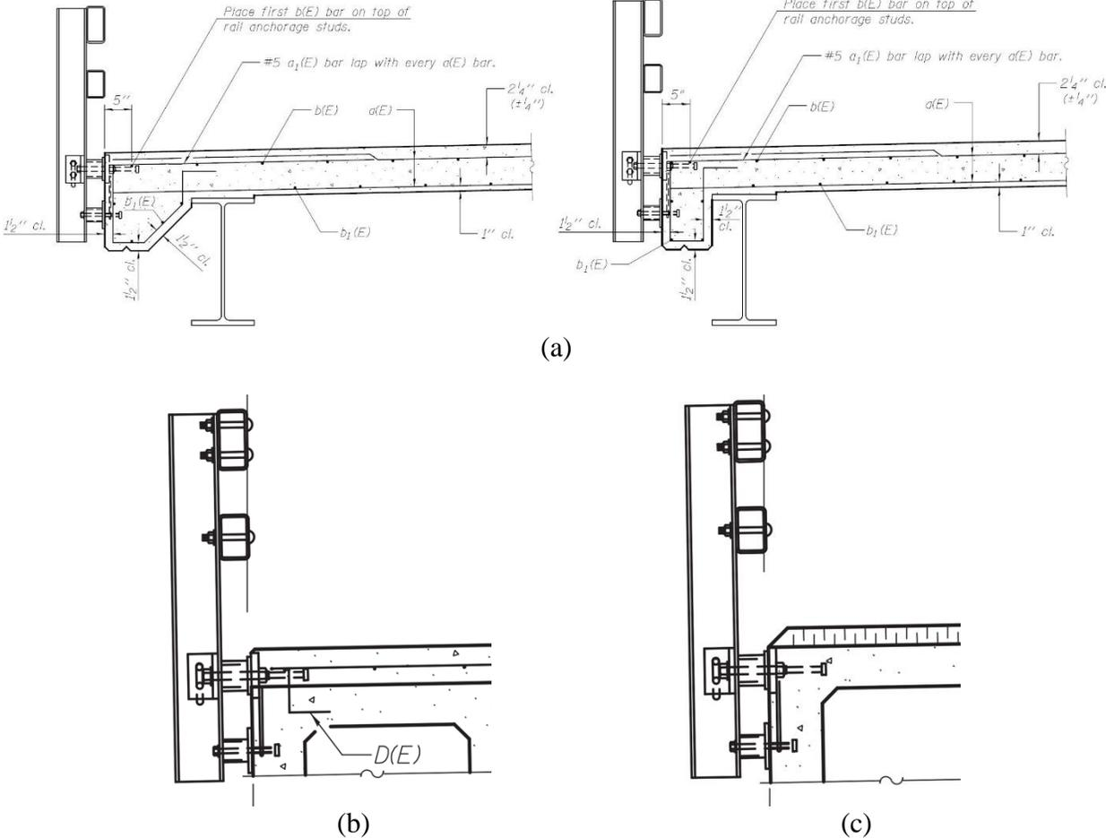
Figure 3. Illinois DOT (a) Bridge Slab, (b) Box Girder with Concrete Wearing Surface, and (c) Box Girder with Asphalt Wearing Surface [4]
