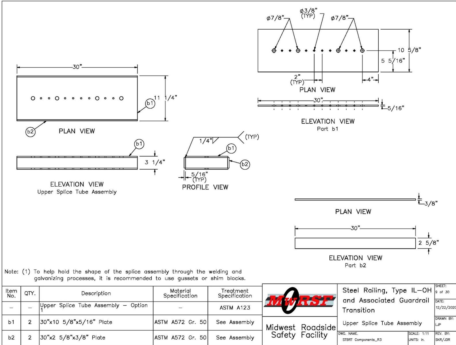
Figure A-9. Steel Railing, Type IL-OH, Upper Splice Tube Assembly
