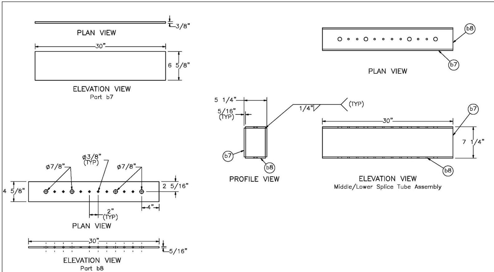
Note: (1) To help hold the shape of the splice assembly through the welding and galvanizing processes, it is recommended to use gussets or shim blocks.
