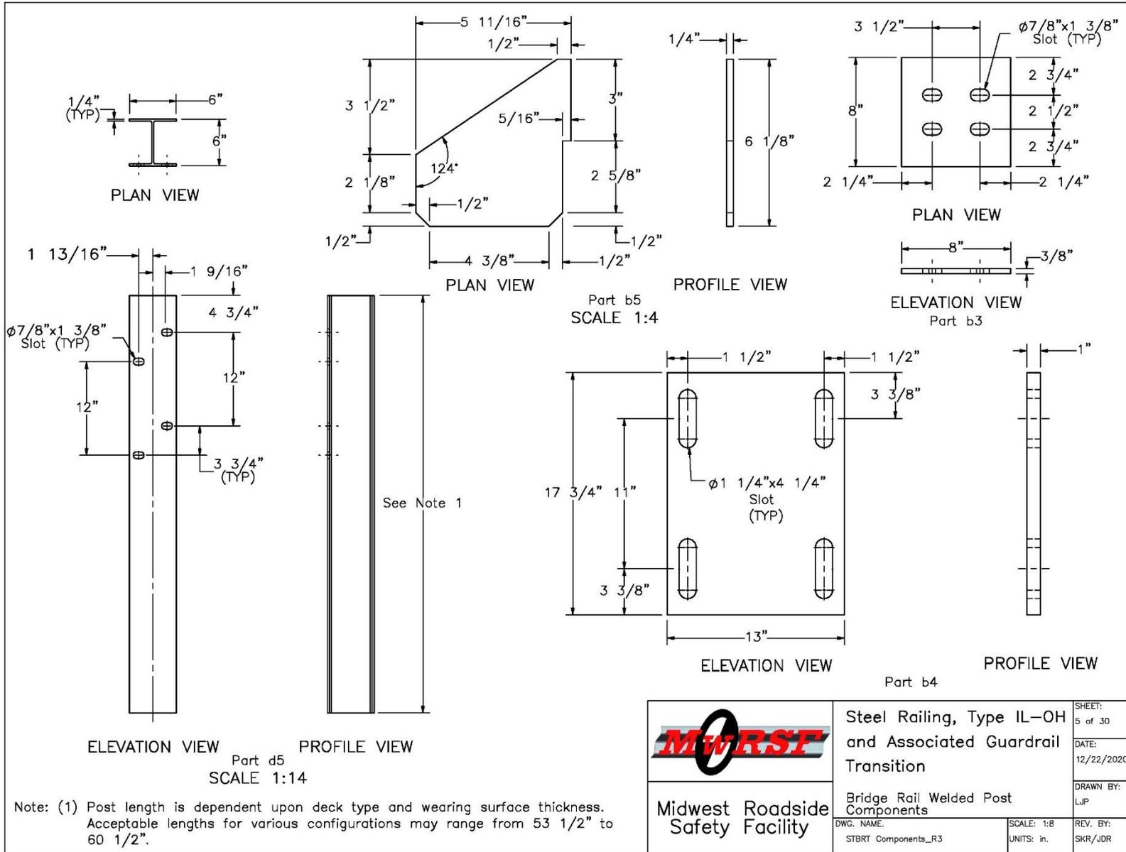
Figure A-5. Steel Railing, Type IL-OH, Post Assembly Components
