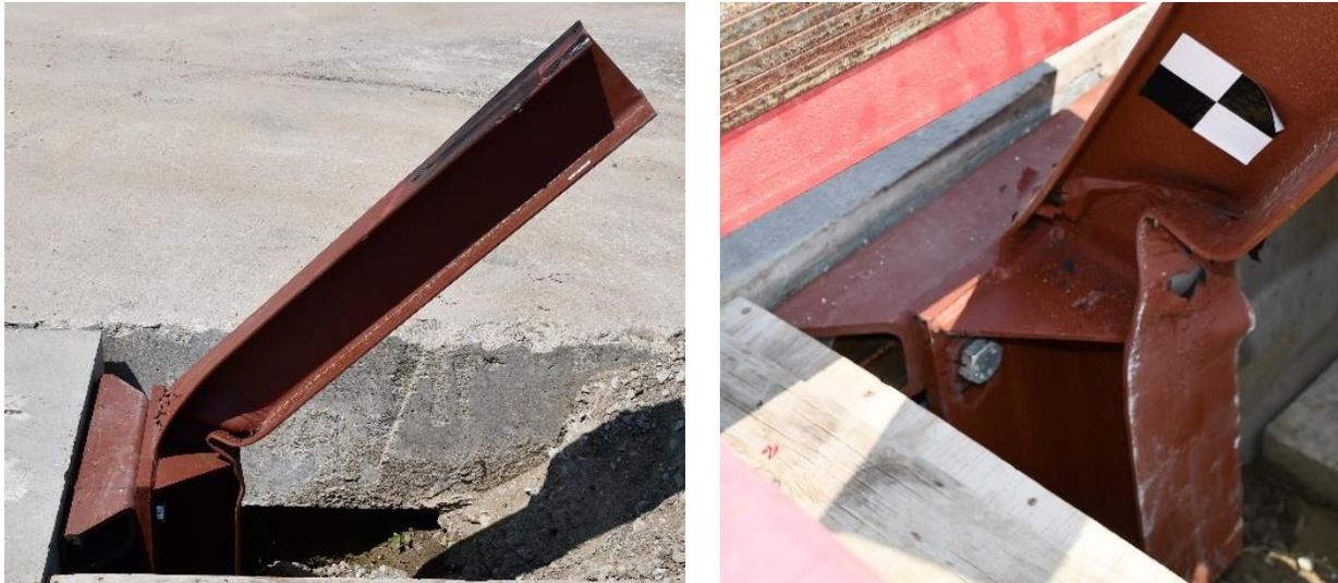
Figure 11. Post-Test Photographs of Selected Post-to-Deck Connection
