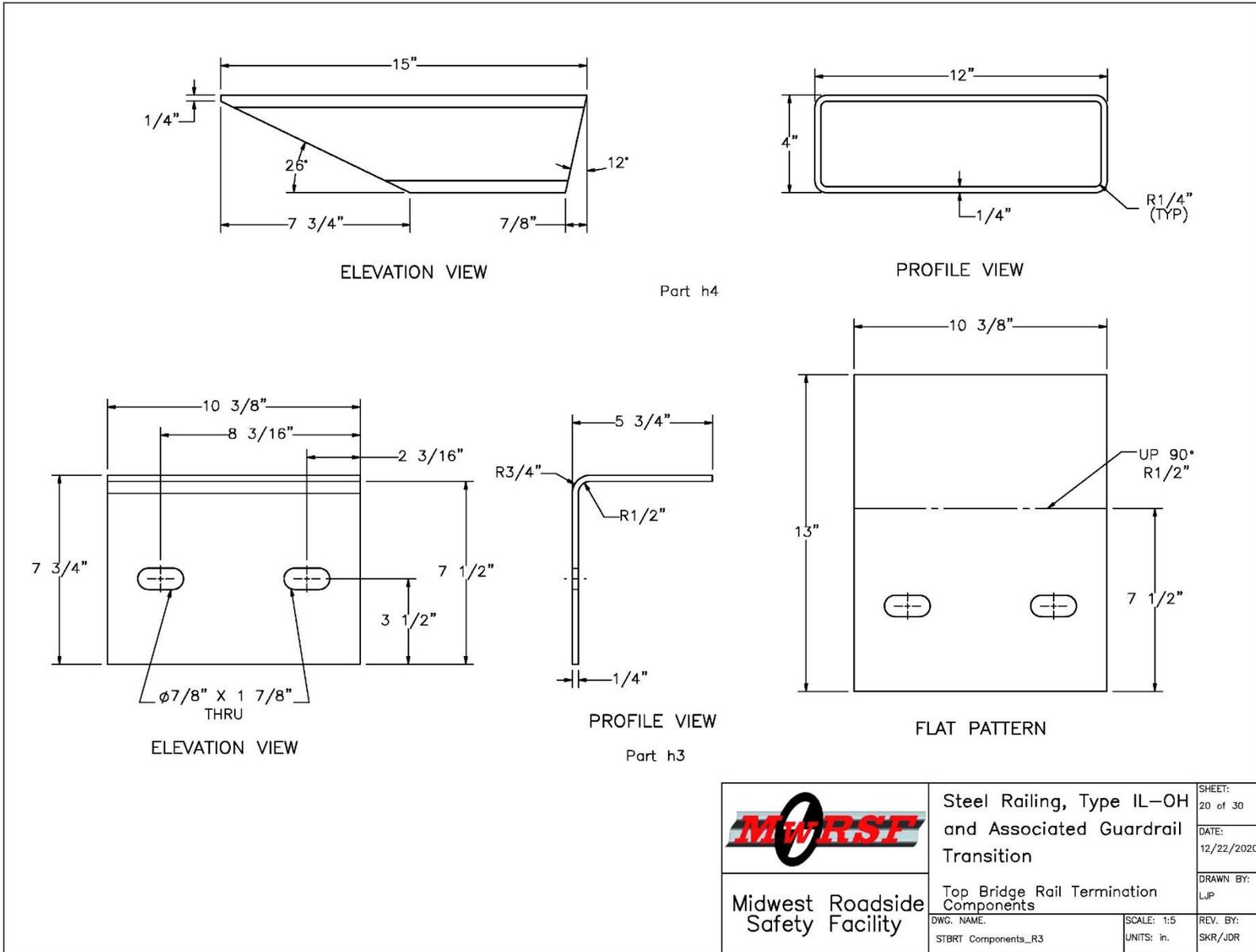
Figure A-20. Steel Railing, Type IL-OH, Top Transition Tube Rail Components
