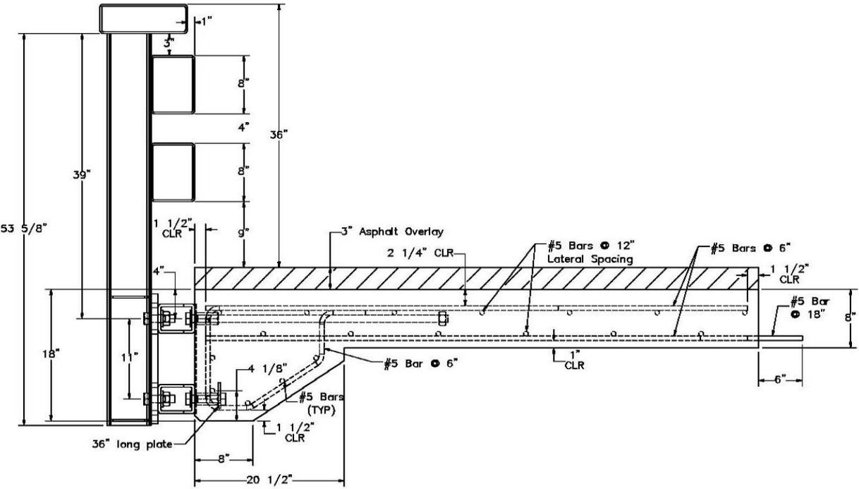
Note: (1) The Bridge Deck shown is the Illinois Wide Overhang design and is compatible with the Illinois Narrow Overhand and the Ohio Deck Slab.
