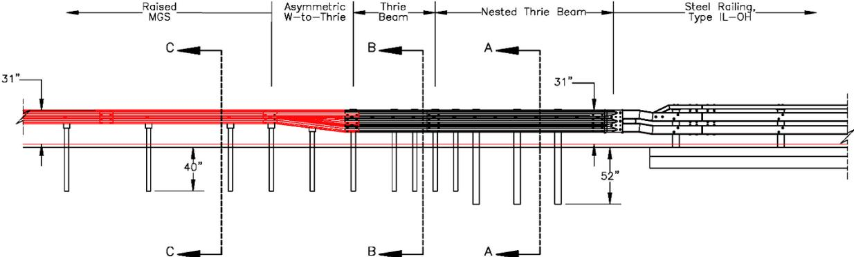
Figure 35. AGT Configuration After a 3-in. Roadway Overlay
