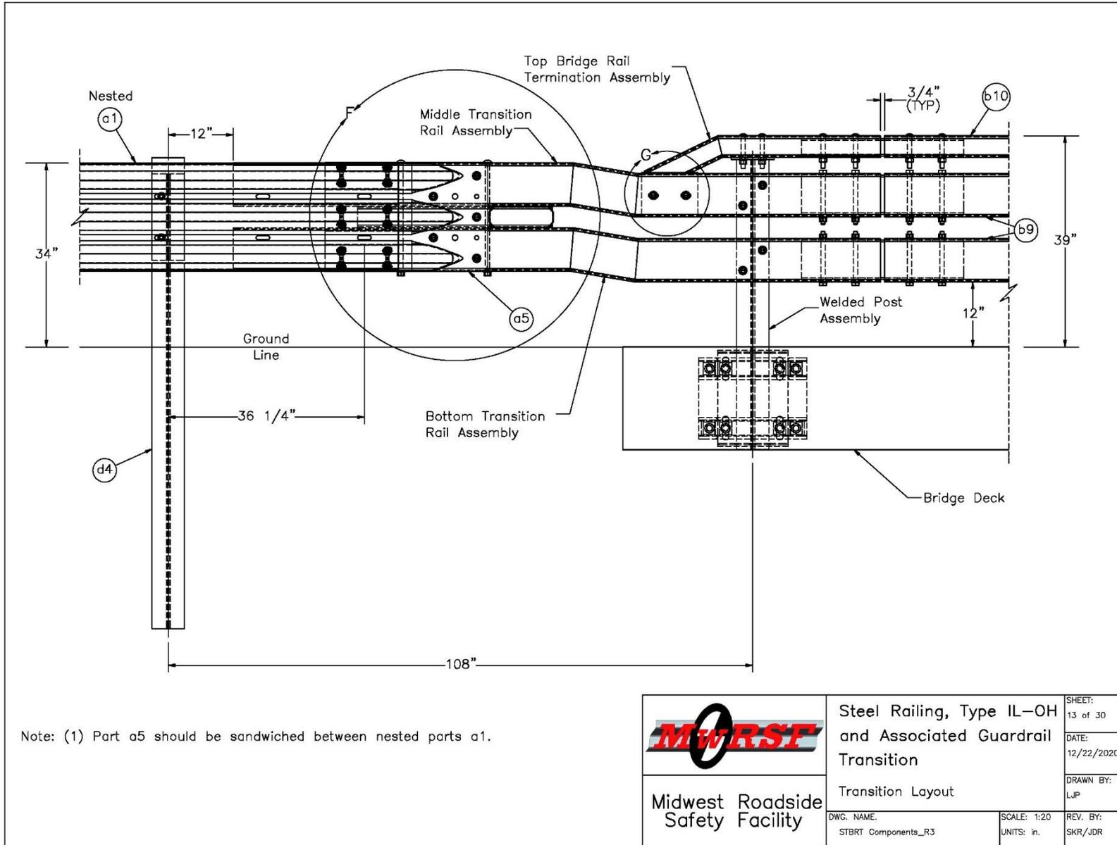
Figure A-13. Steel Railing, Type IL-OH, Connection to Guardrail Transition
