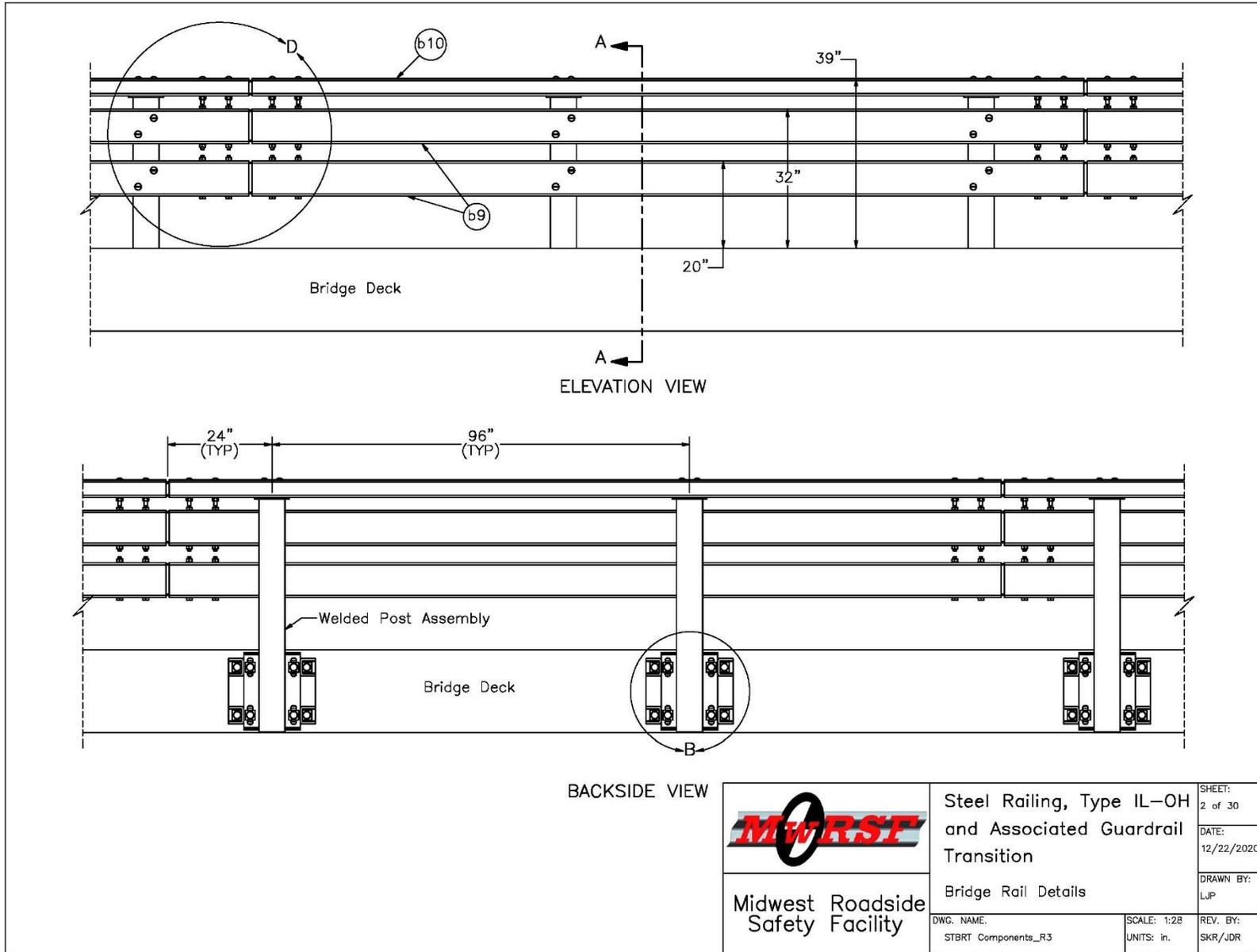
Figure A-2. Steel Railing, Type IL-OH, Elevation View
