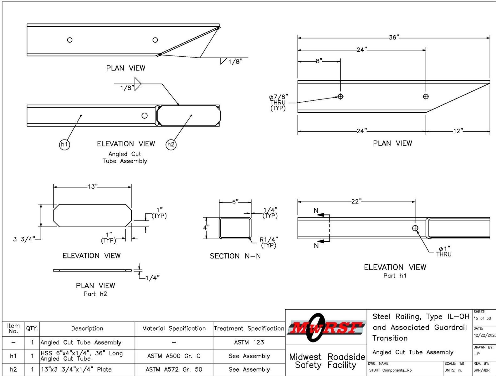
Figure A-15. Steel Railing, Type IL-OH, Angled Cut Tube Assembly
