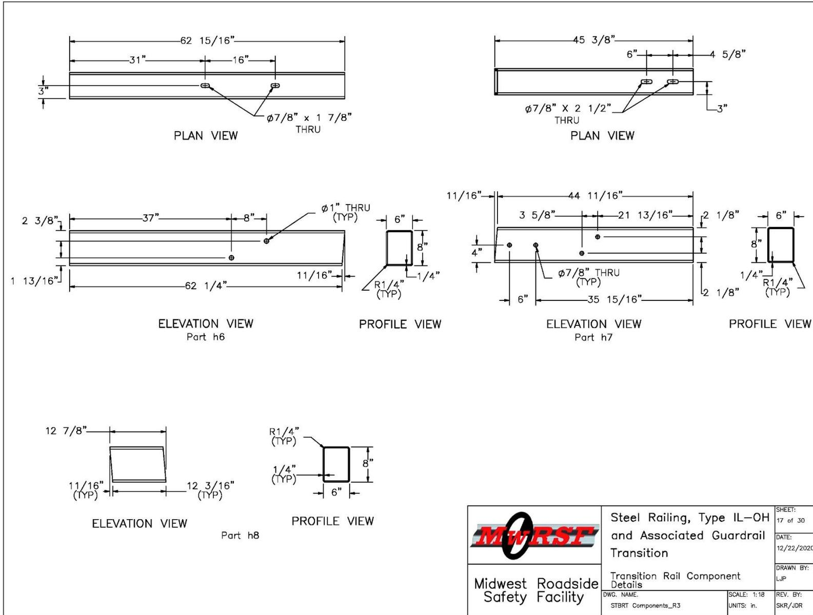
Figure A-17. Steel Railing, Type IL-OH, Transition Tube Rail Components
