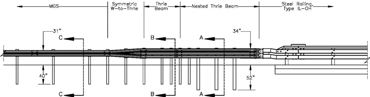
Figure 34. AGT Configuration at Time of Initial Installation, No Overlay
