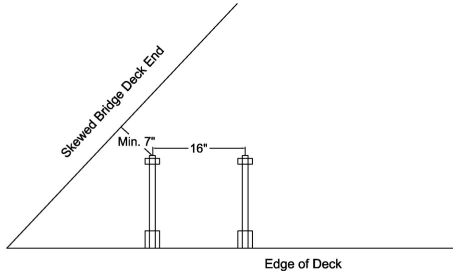
Figure 33. Minimum Distance for Anchor Placement near Skewed Deck Ends
