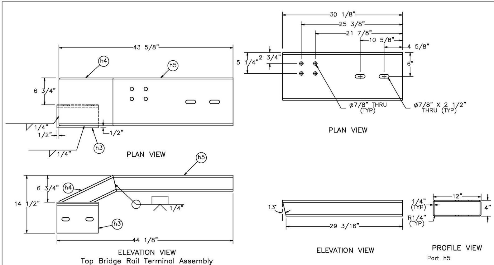
Note: Top bridge rail terminal assembly must be mirrored to use on other end of bridge.
