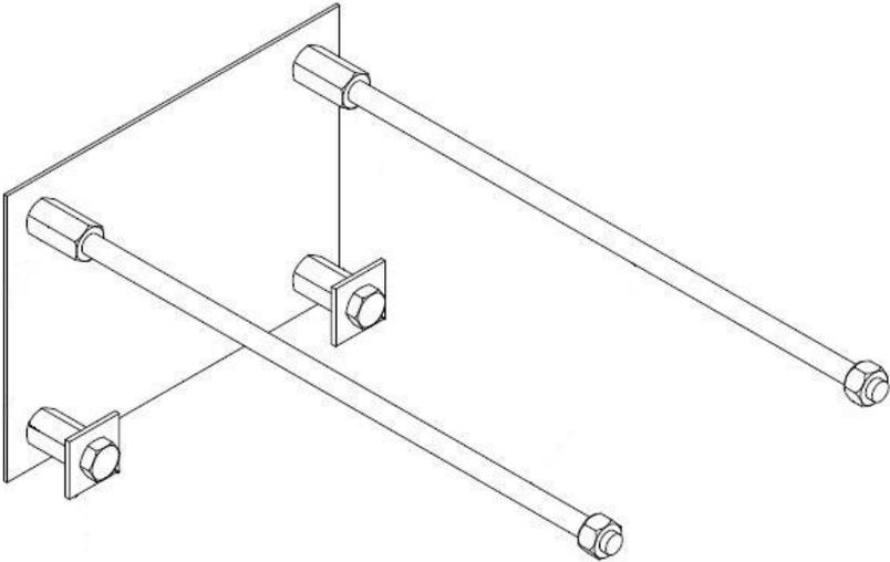
Figure 7. Isometric View of Post-to-Deck Anchorage Hardware
