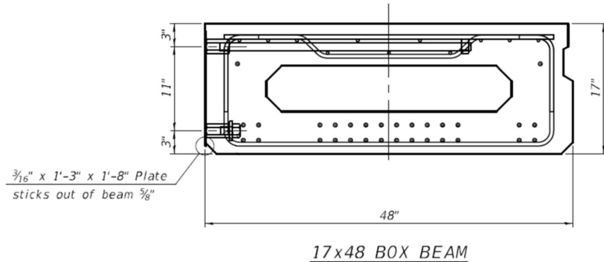
Figure 31. Edge Plate Extending from Face of 17-in. Box Beam
