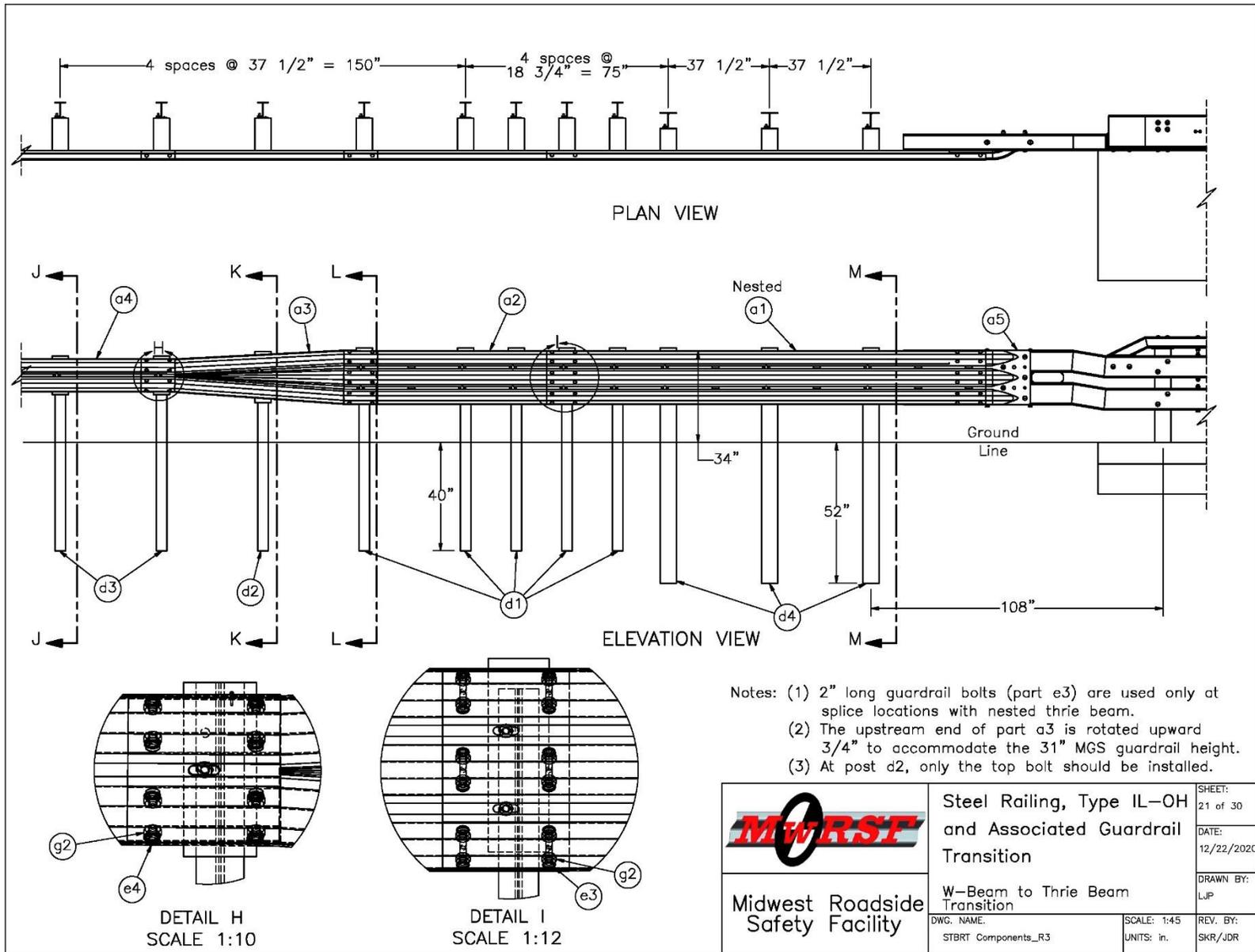
Figure A-21. Steel Railing, Type IL-OH, Approach Guardrail Transition Layout
