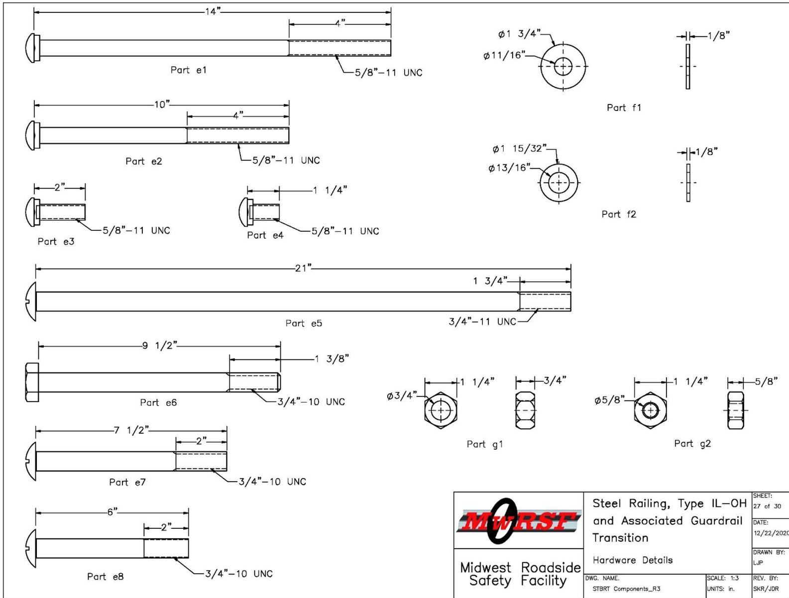
Figure A-27. Steel Railing, Type IL-OH, Hardware Details
