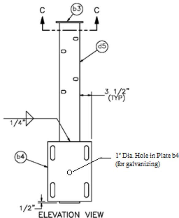
Figure 26. Example of Hole in Mounting Plate for Galvanization Purposes
