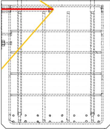
(a) Box Beam Deck, Solid End Section
