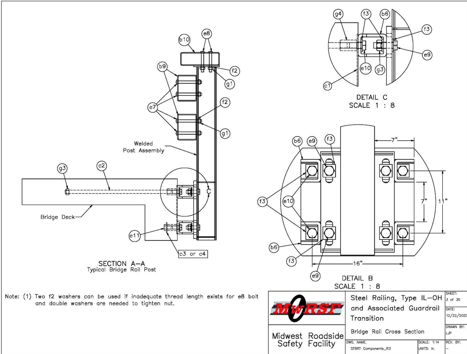
Figure A-3. Steel Railing, Type IL-OH, Cross Section and Attachment Details
