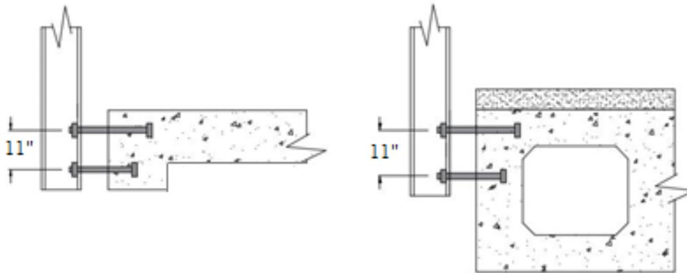
Figure 8. Same Anchorage Configuration for CIP and Prestressed Box Beam Decks
