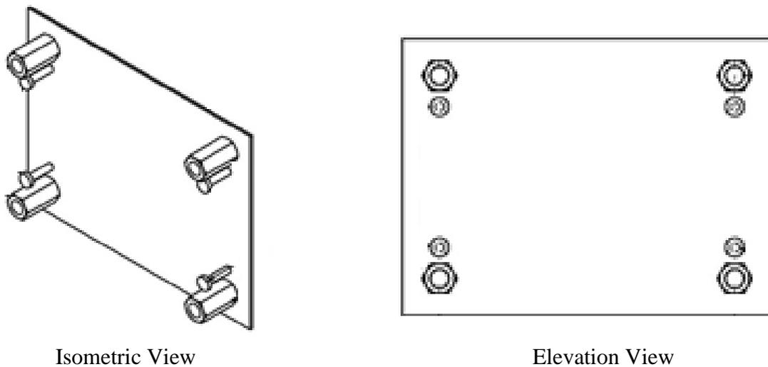
Figure 30. Example of Shear Studs Applied to Inner Face of the Embedded Edge Plate
