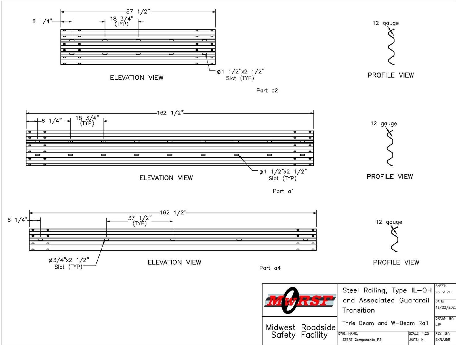
Figure A-25. Steel Railing, Type IL-OH, AGT Rail Segments
