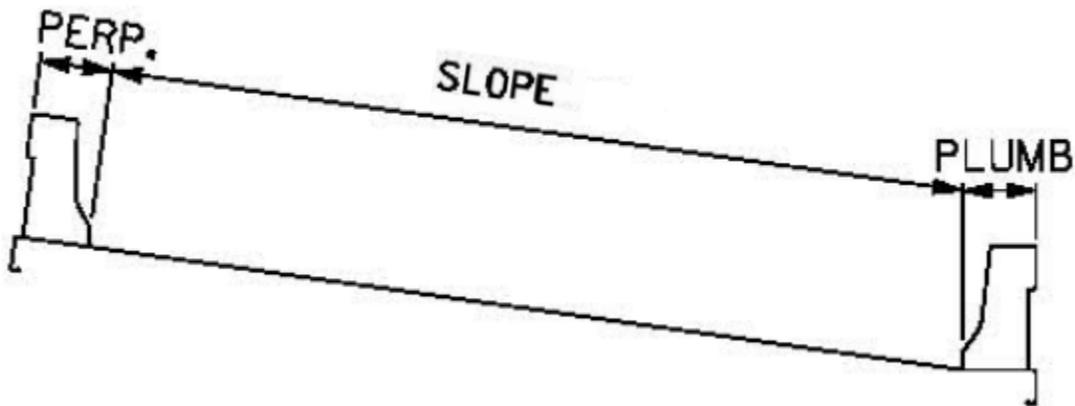
Figure 28. Plumb vs. Perpendicular Barrier Installations on Superelevated Roadways
