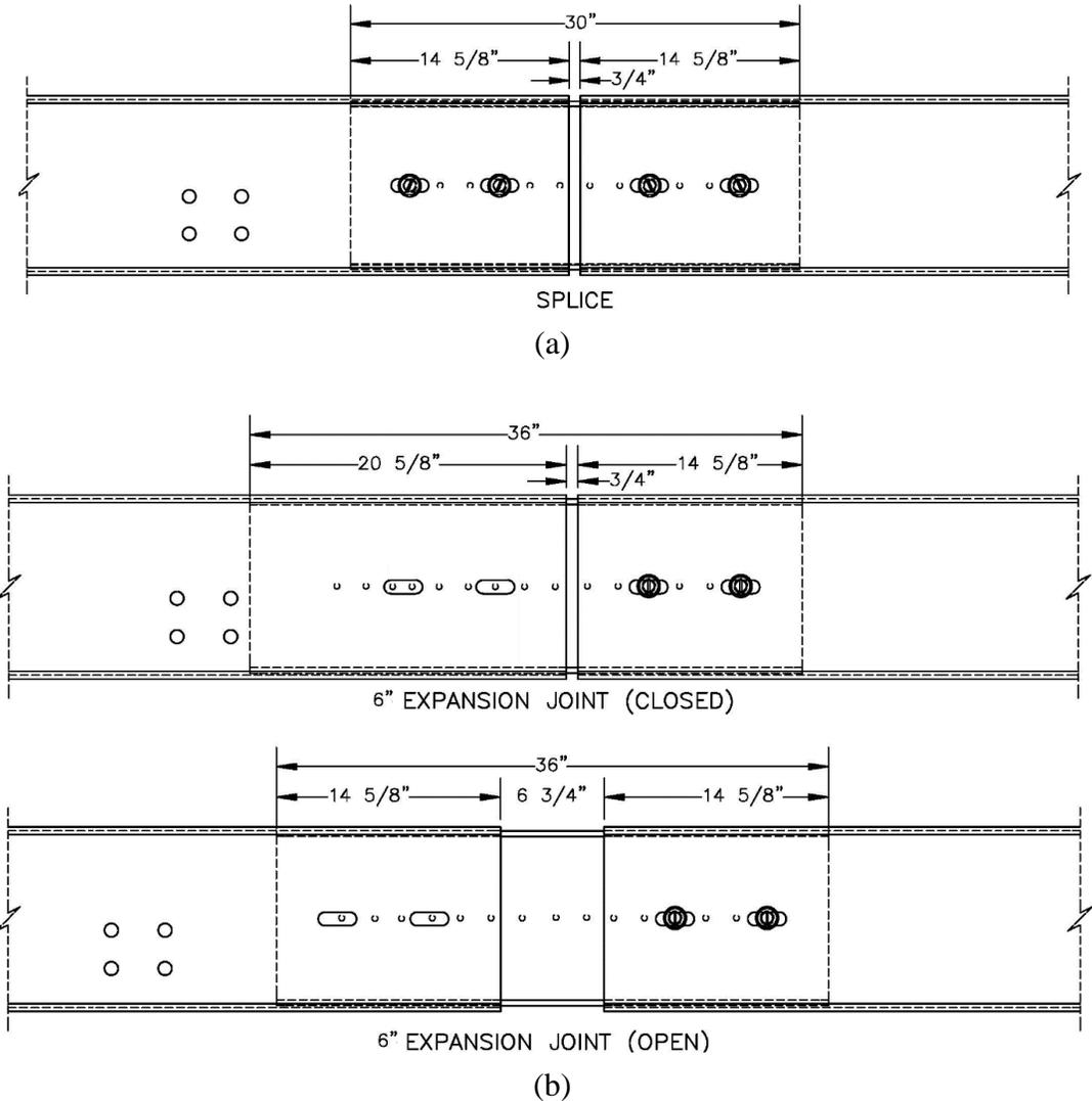
Figure 27. Top HSS Tube Rail Connections at (a) Typical Splice Joints and (b) a 6-in. Expansion/Contraction Joint
