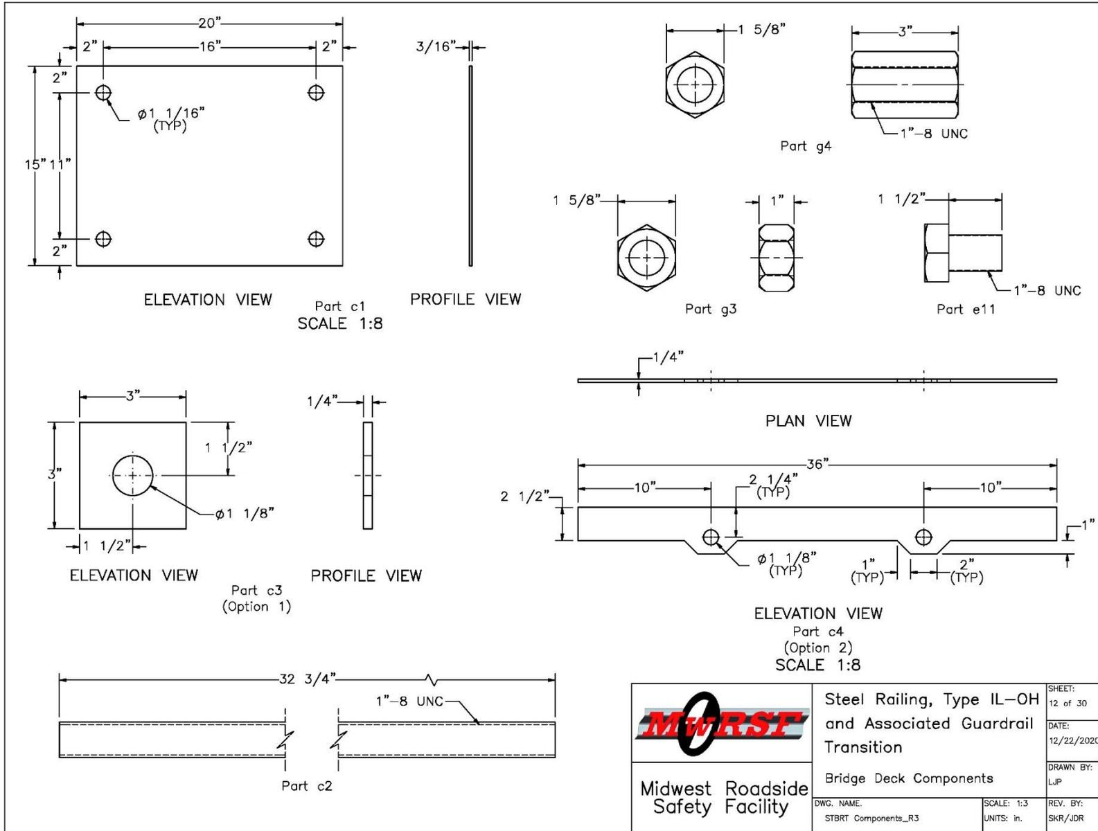
Figure A-12. Steel Railing, Type IL-OH, Embedded Attachment Hardware
