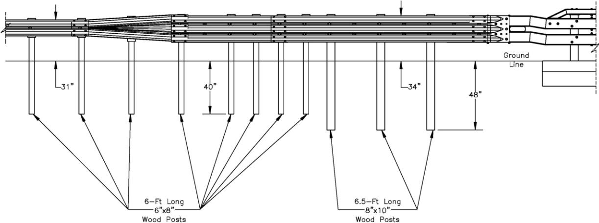
Figure 37. Wood Post Alternative Approach Guardrail Transition
