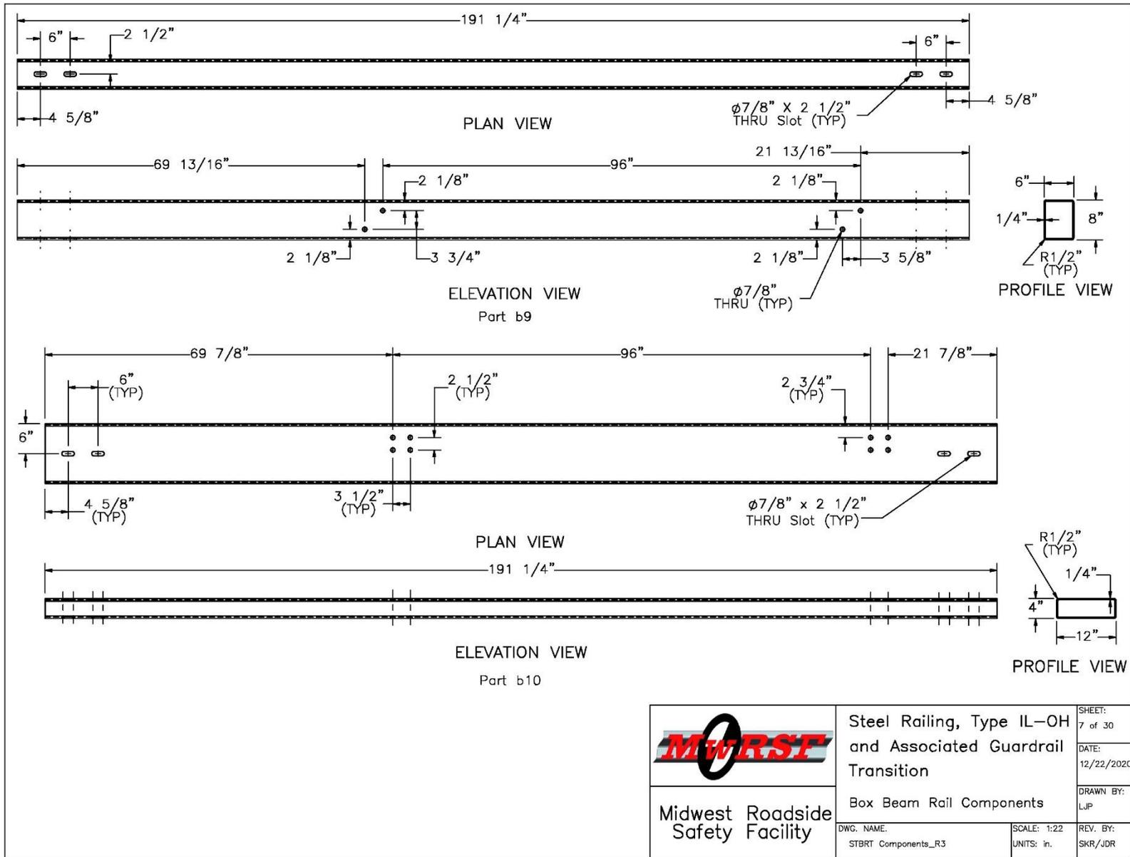
Figure A-7. Steel Railing, Type IL-OH, Rail Components
