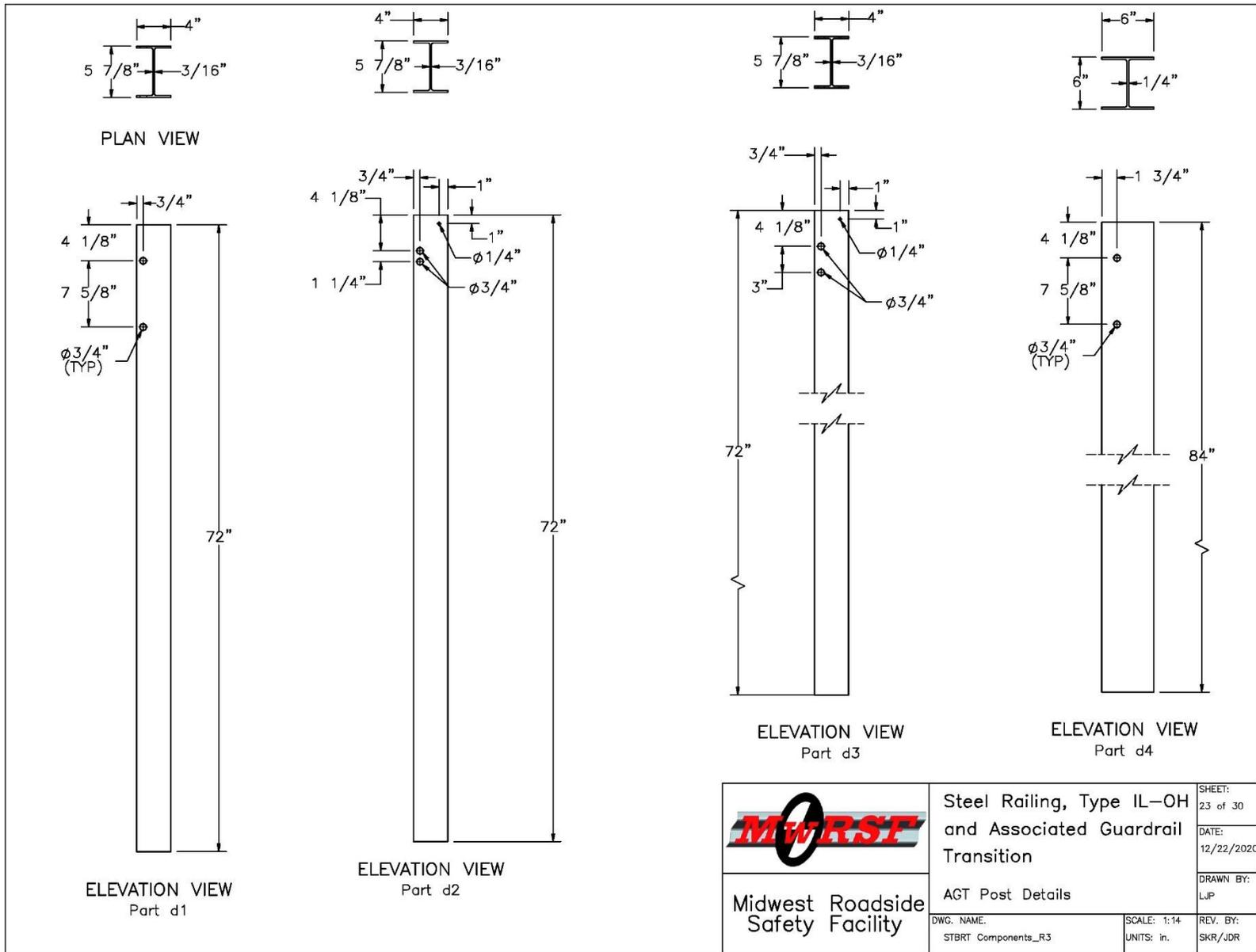
Figure A-23. Steel Railing, Type IL-OH, AGT Post Details
