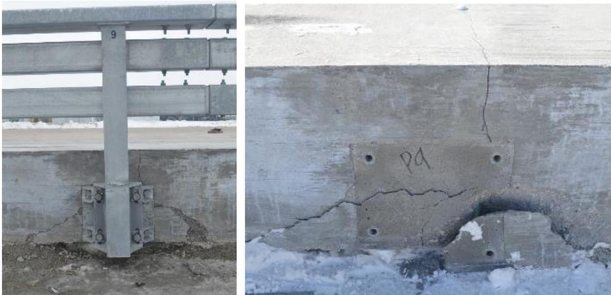
Figure 29. Concrete Damage Observed during Test No. STBR-2
