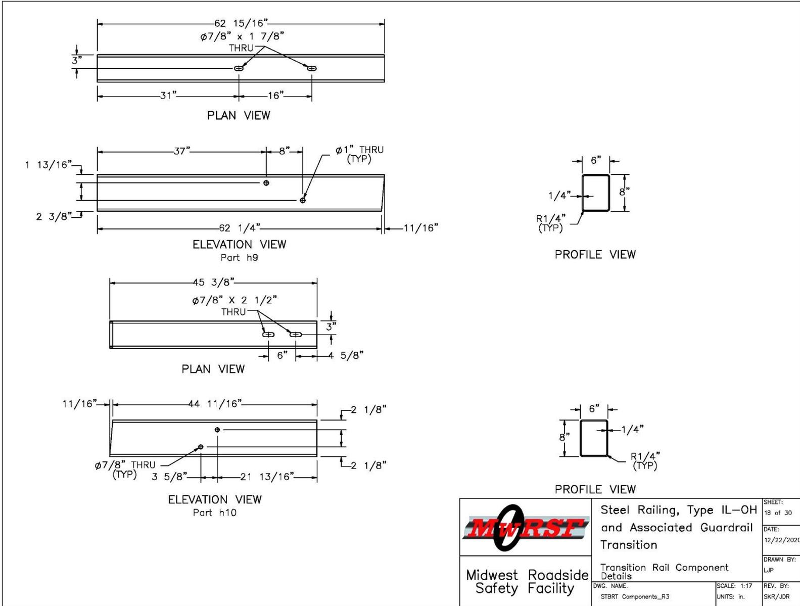
Figure A-18. Steel Railing, Type IL-OH, Transition Tube Rail Components
