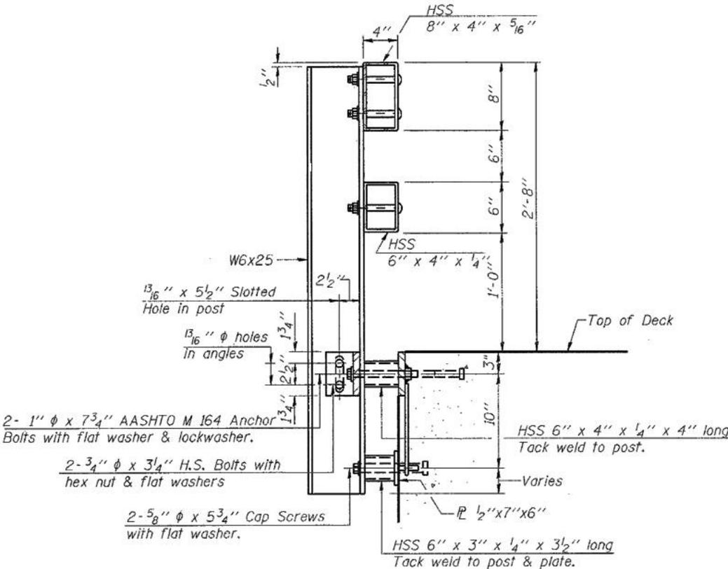
Figure 1. Illinois Side-Mounted Bridge Railing [2-4]
