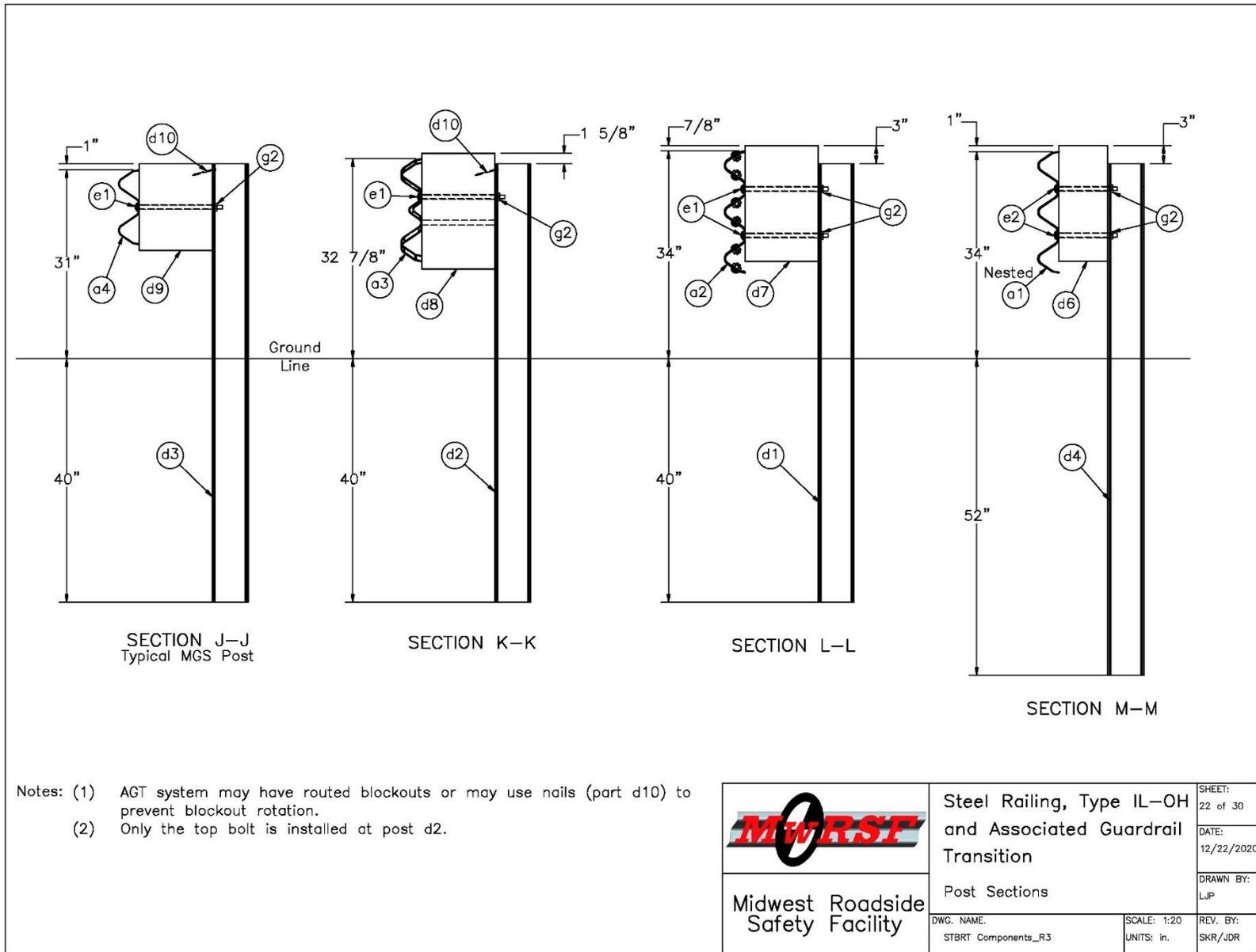
Figure A-22. Steel Railing, Type IL-OH, AGT Cross-Sections
