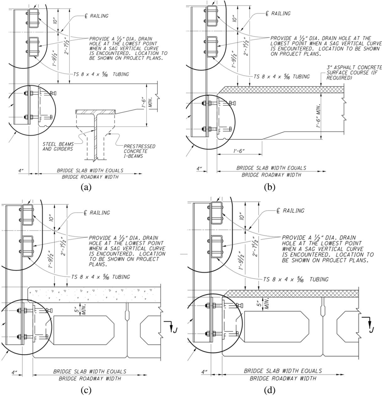
Figure 4. Ohio DOT (a) Bridge Slab, (b) Bridge Slab with Asphalt Wearing Surface, (c) Box Girder with Concrete Wearing Surface, and (d) Box Girder with Asphalt Wearing Surface [5]
