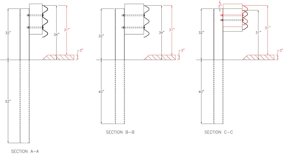
Figure 36. System Cross-Sections Before and After a 3-in. Overlay
