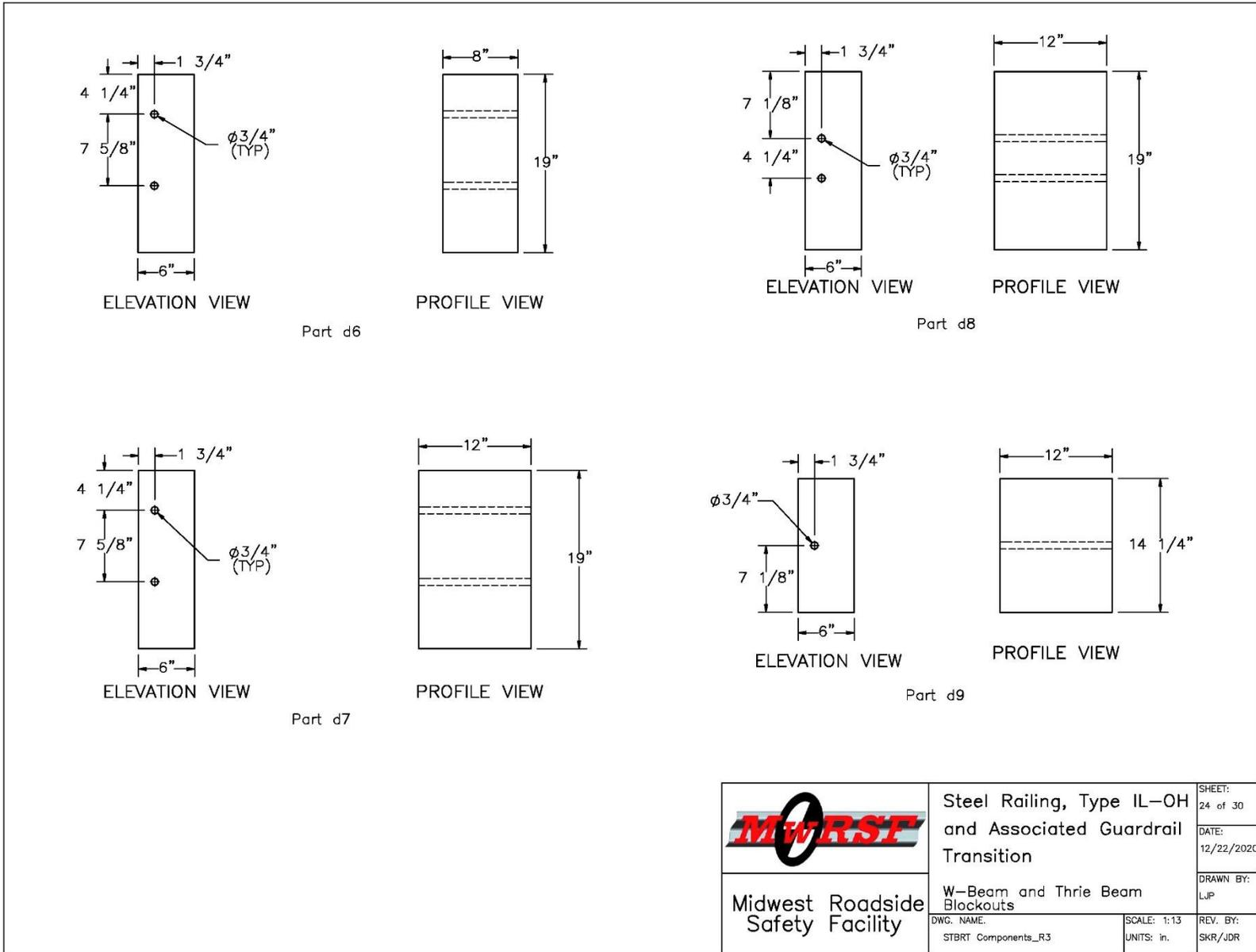
Figure A-24. Steel Railing, Type IL-OH, AGT Blockouts
