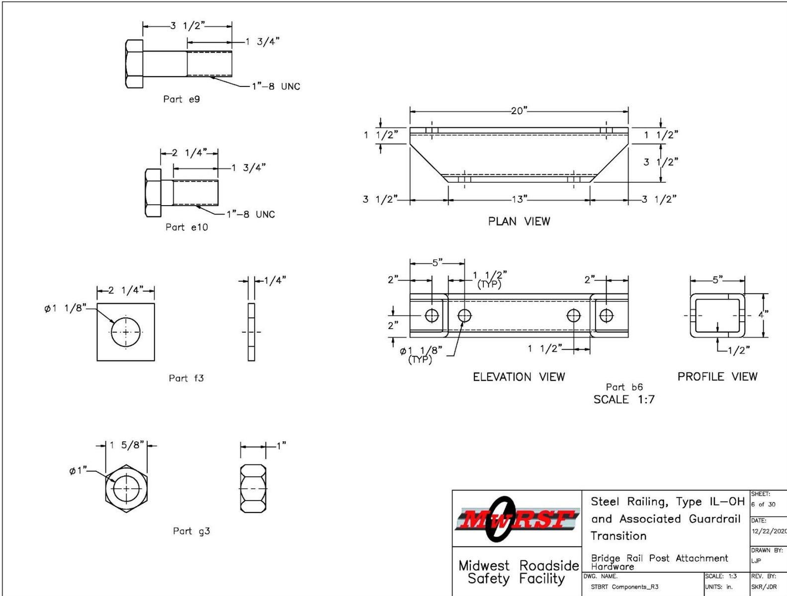
Figure A-6. Steel Railing, Type IL-OH, Post Attachment Hardware
