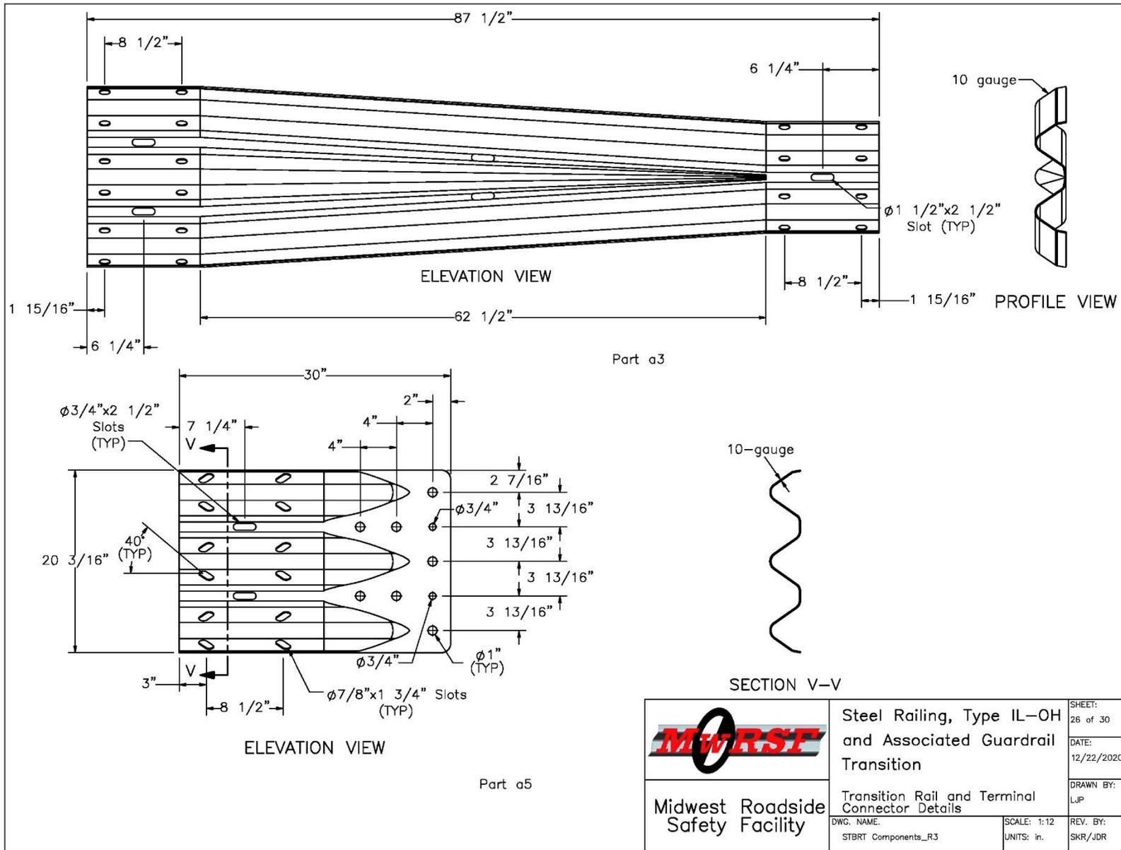
Figure A-26. Steel Railing, Type IL-OH, Transition Rail and Terminal Connector
