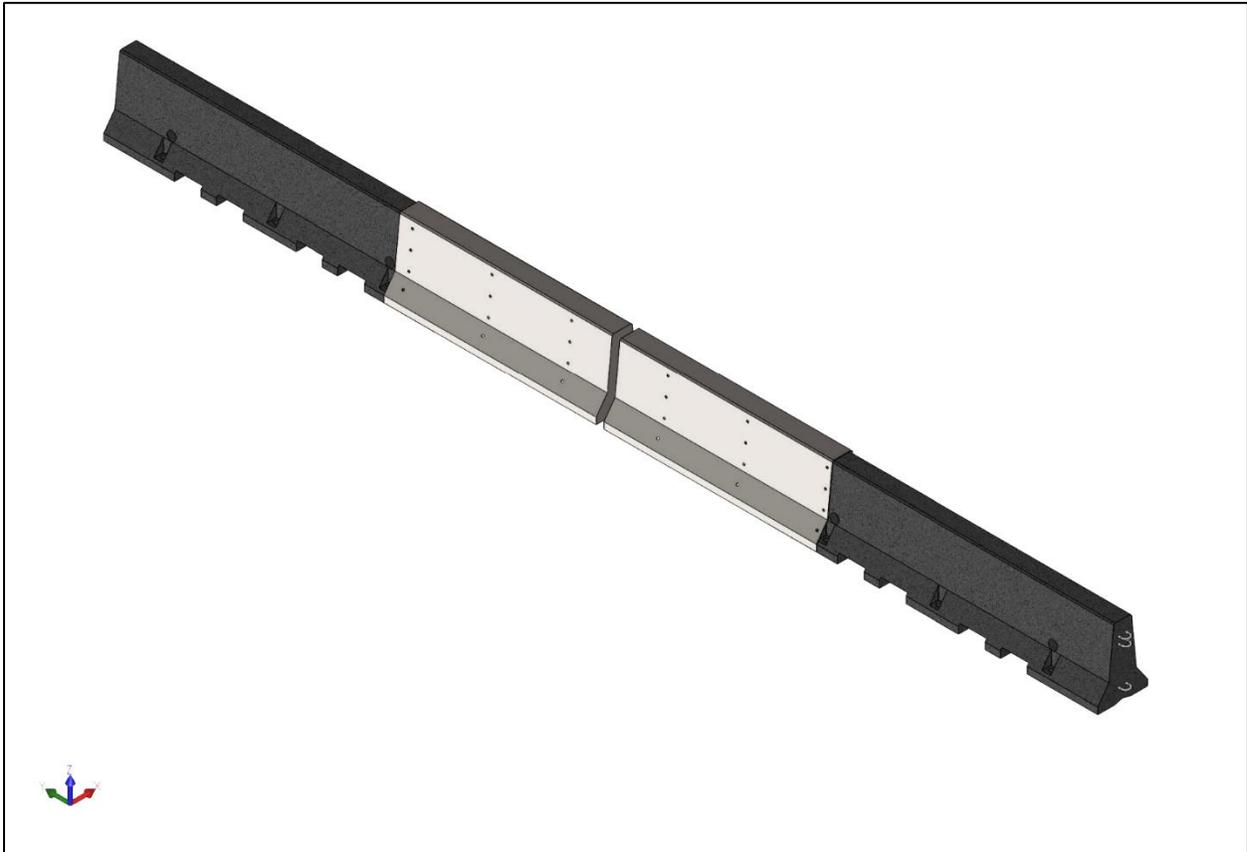
Figure 32. Concept No. 7 – Two-Piece Cover Plate
