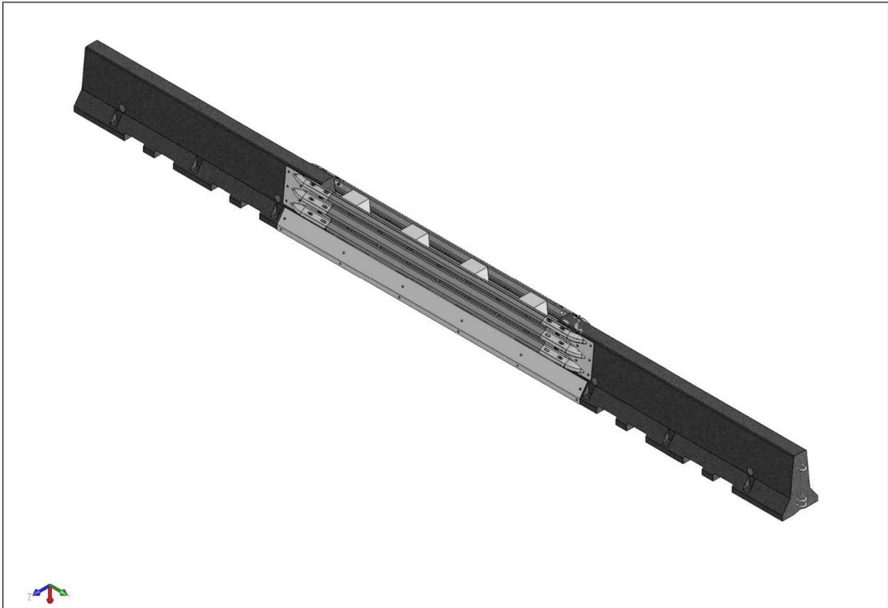
Figure 26. Concept No. 4 – Thrie Beam and Toe Plate
