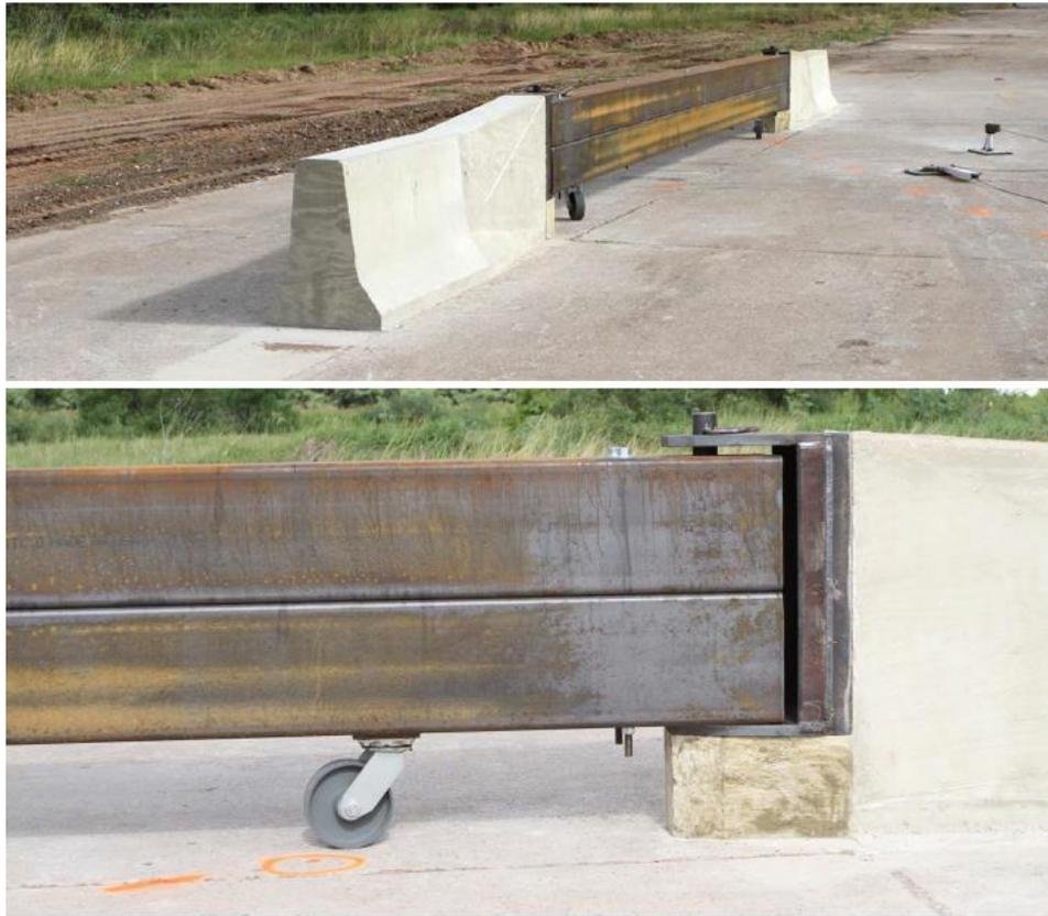
Figure 7. TxDOT Median Barrier Gate [14]
