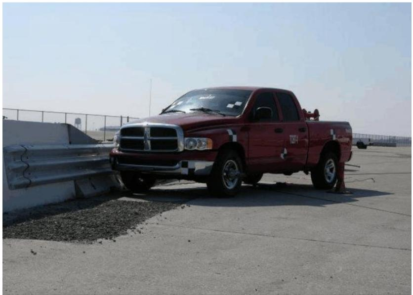
Figure 73. Free-Standing PCB Transition to Permanent Concrete Median Barrier, Test No. TCBT-1
