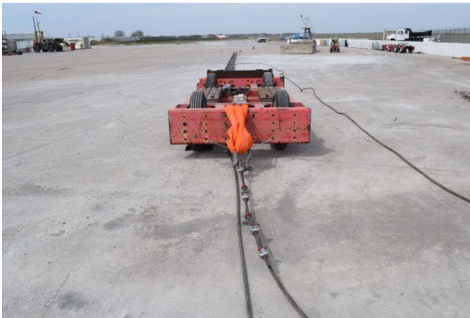
Figure 61. Rigid-Frame Bogie Vehicle, Test Nos. SPDA-1 through SPDA-5
