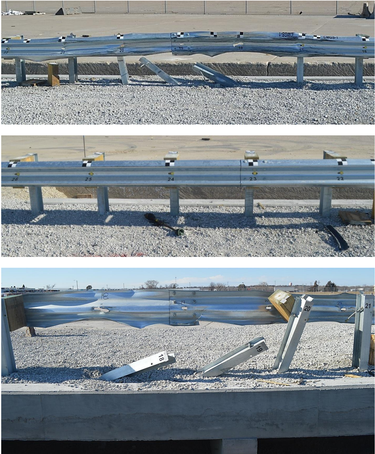
Figure 60. System Damage, Test No. CMGS-1
