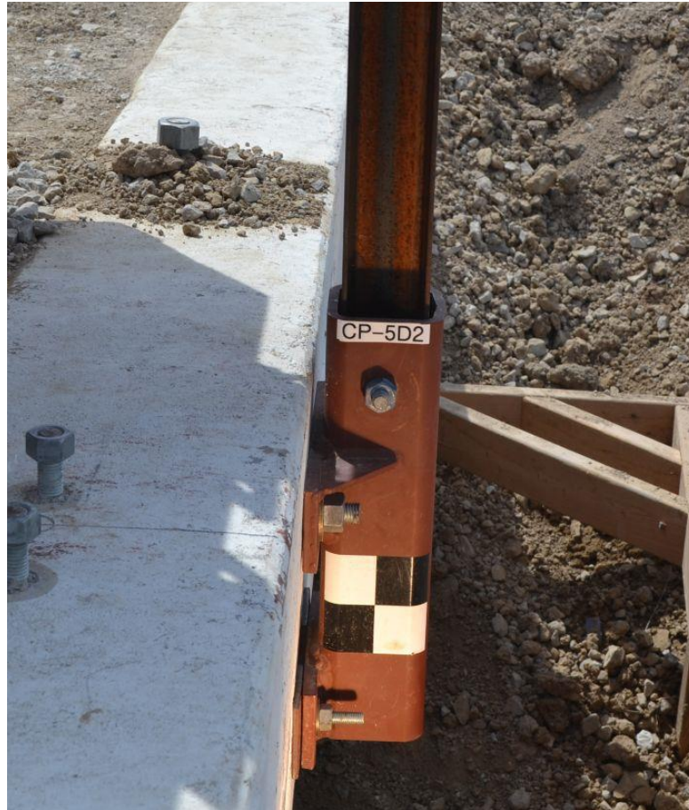
Figure 1. Side-Mounted Configuration for Guardrail on Culvert Headwalls [4]
