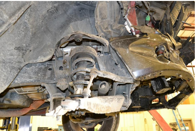
Figure 95. Vehicle Undercarriage Damage, Test No. CMGS-2
