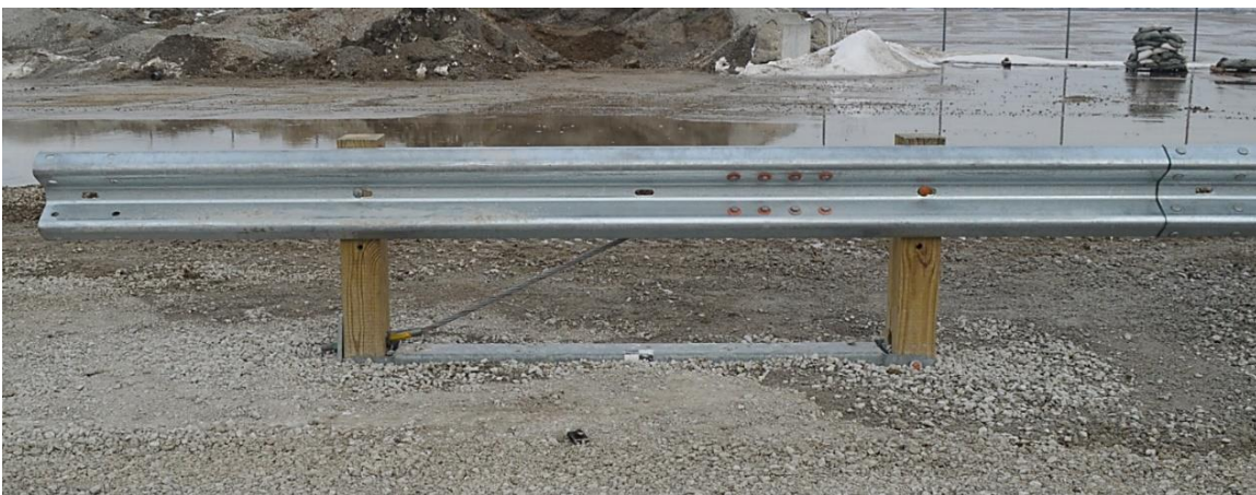
Figure 88. Culvert Deck after Removal of Soil Fill and Posts and Downstream Anchorage System Deformation, Test No. CMGS-2
