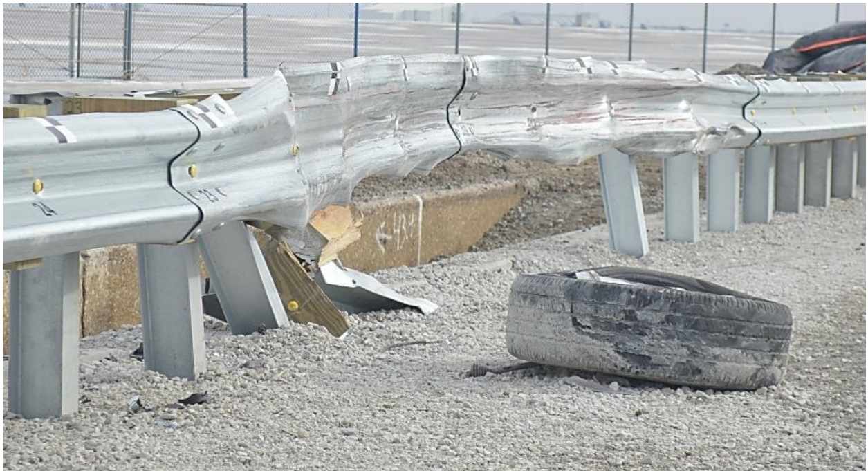
Figure 80. System Damage, Test No. CMGS-2
