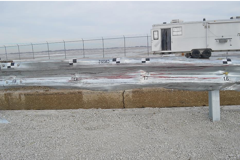
Figure 81. Damage to Post Nos. 15 through 21, Test No. CMGS-2
