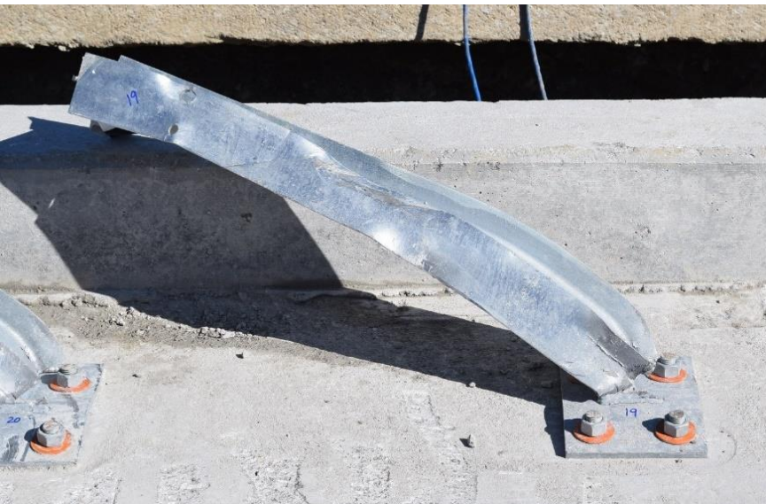
Figure 87. Damage to Post Nos. 17 through 22 Damage – After Soil Removal, Test No. CMGS-2
