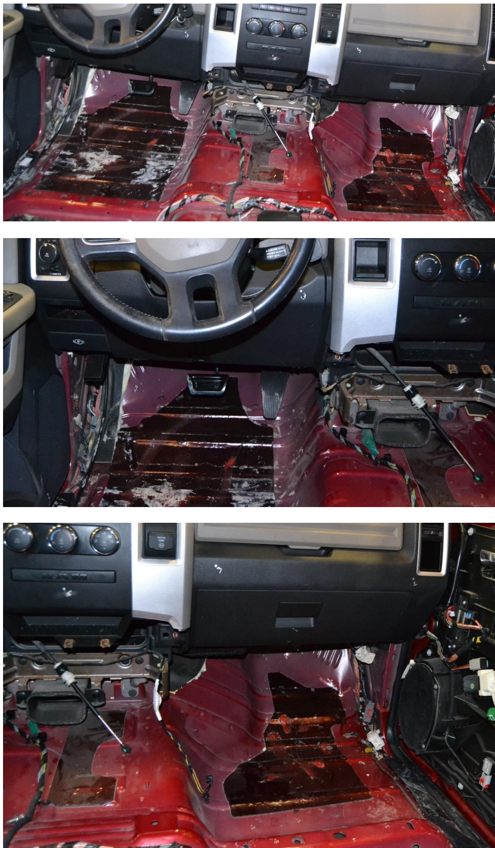
Figure 94. Vehicle Occupant Compartment Damage, Test No. CMGS-2
