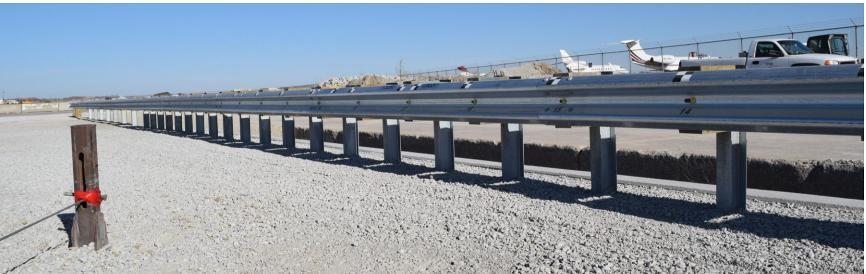
Figure 41. System Installation, Test Nos. CMGS-1 and CMGS-2
