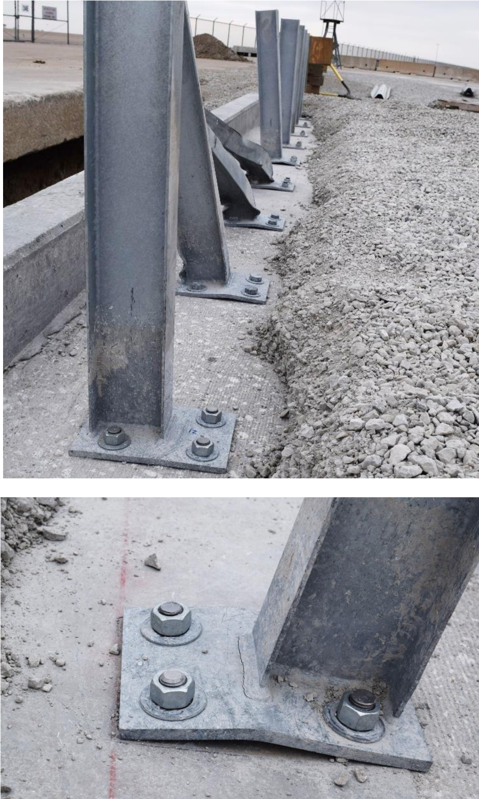
Figure 62. Damage to Post and Base Plate Nos. 17 through 21 (After Removal of Soil Fill Post and Base), Test No. CMGS-1
