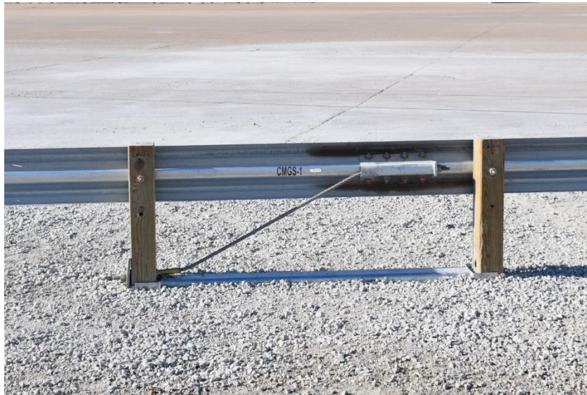
Figure 43. Bottom-Side Steel Post Connection Details and End Anchorage Systems, Test Nos. CMGS-1 and CMGS-2
