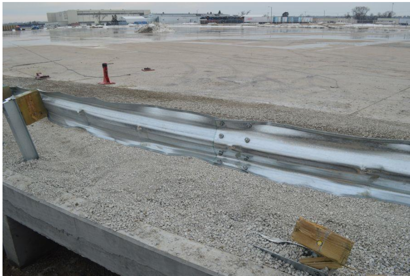
Figure 83. Guardrail Damage, Post Nos. 15 through 22, Test No. CMGS-2
