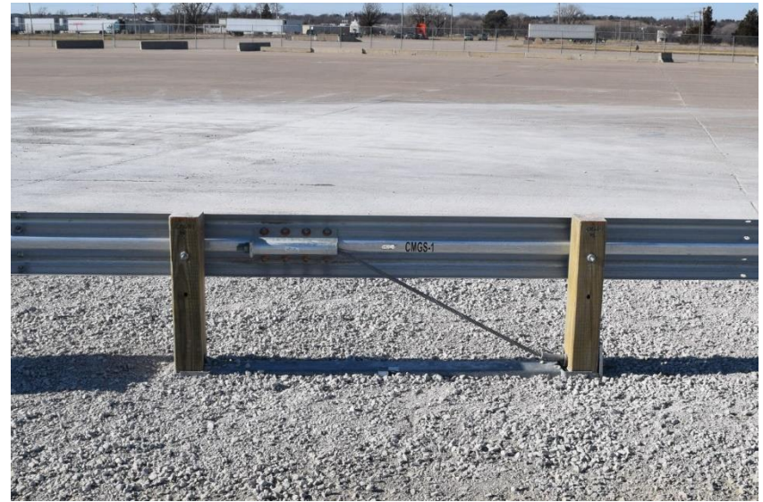
Figure 43. Bottom-Side Steel Post Connection Details and End Anchorage Systems, Test Nos. CMGS-1 and CMGS-2
