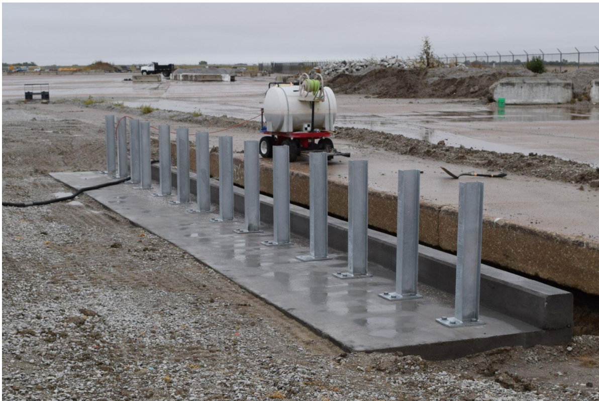
Figure 21. Concrete Culvert Superstructure, Top Slab, Headwall, and Vertical Supports, Test Nos. CMGS-1 and CMGS-2
