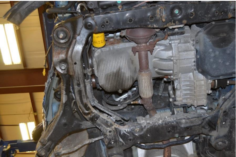
Figure 72. Vehicle Undercarriage Damage, Test No. CMGS-1
