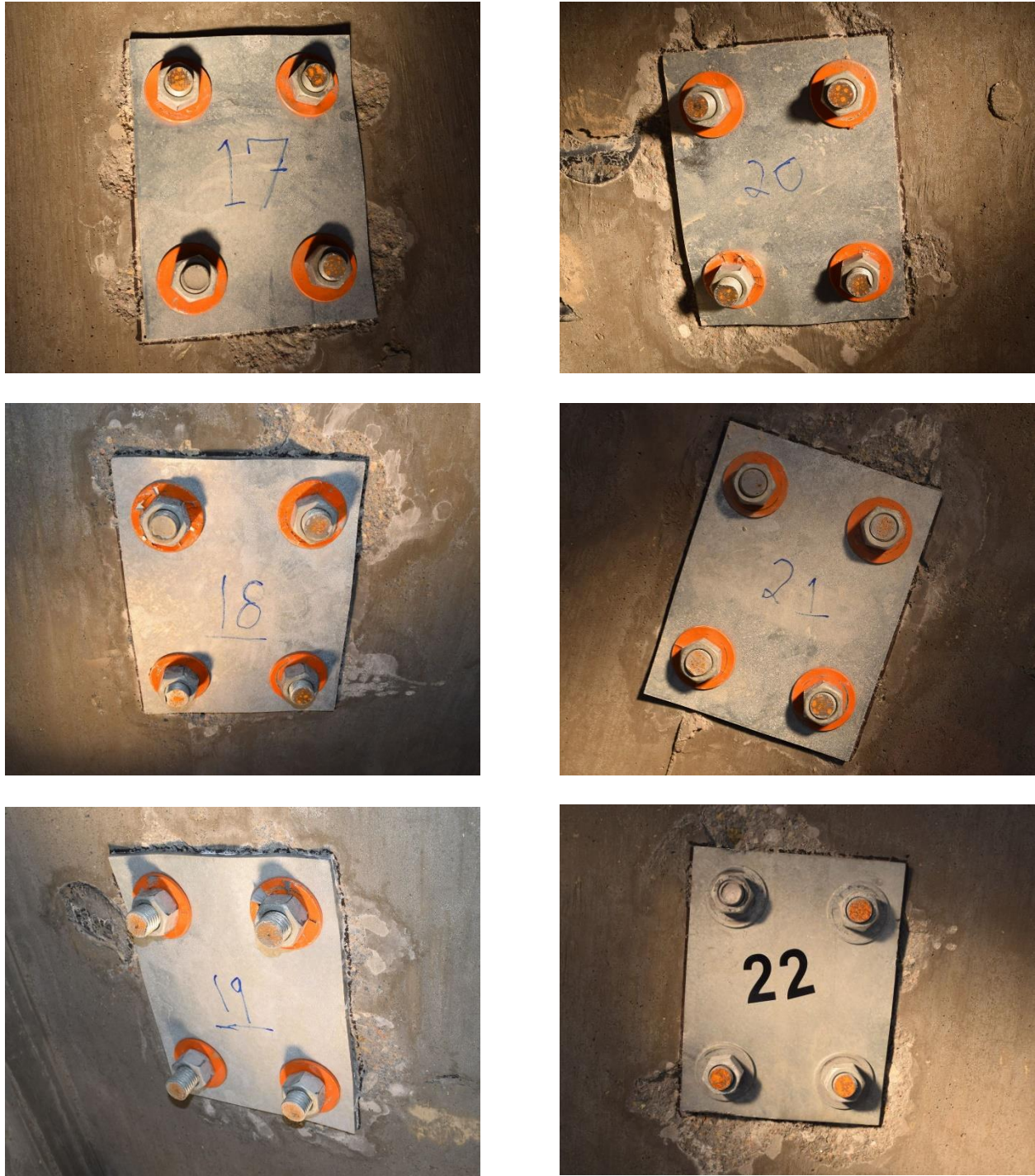
Figure 85. Damage to Base Plates of Post Nos. 17 through 22, Test No. CMGS-2
