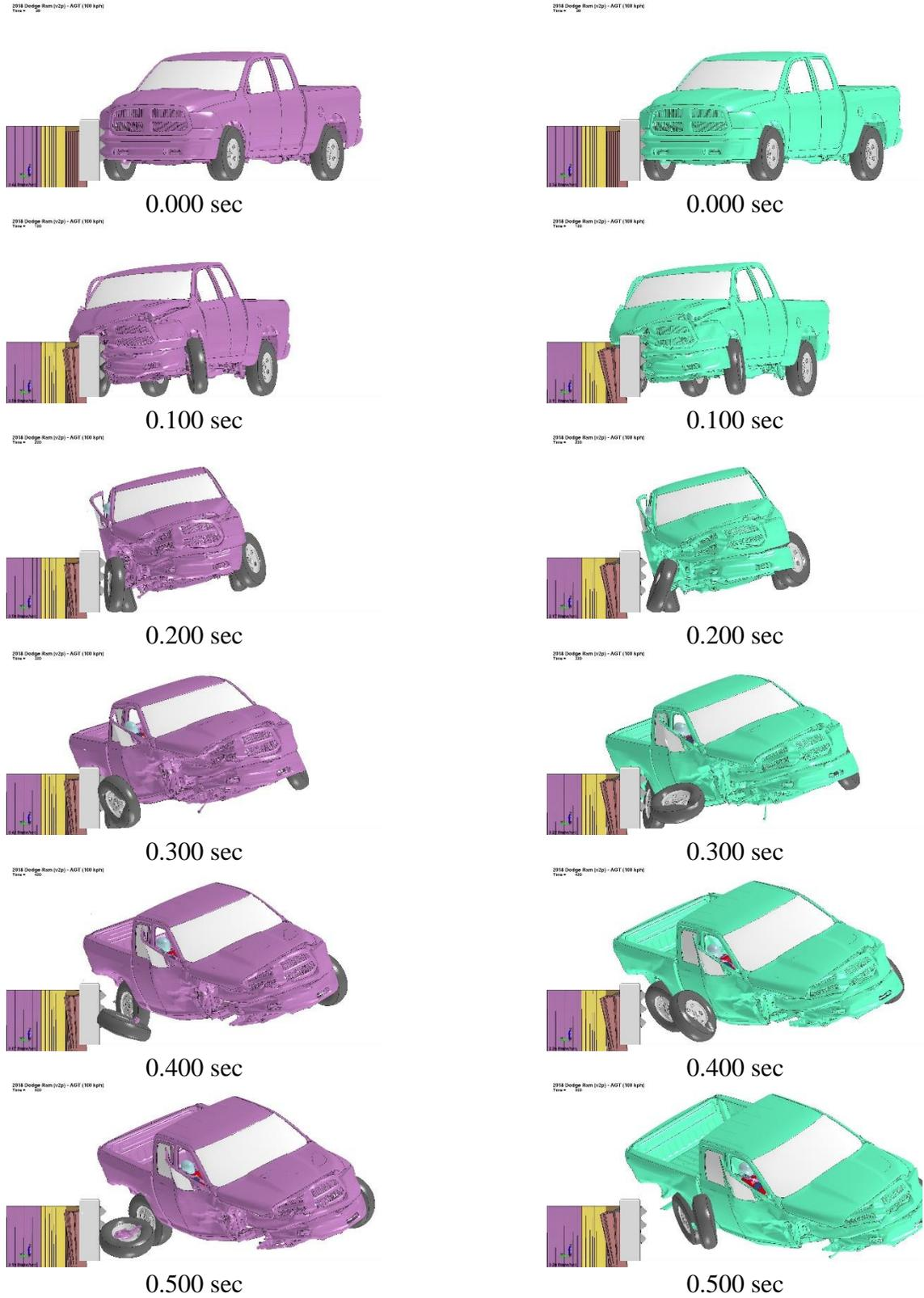
Figure D-3. 15:1 X Simulation (Left) vs. 15:1 US1 Simulation (Right) Sequential Images
