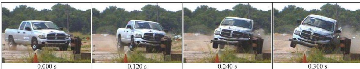
Figure 34. Sequential Photographs for Test No. 490022-8 [16]
