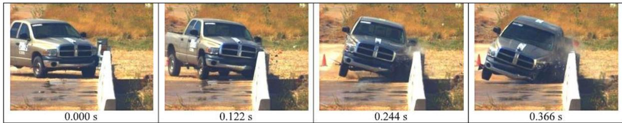
Figure 7. Sequential Photographs for Test No. 420021-4 [10]
