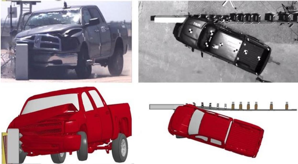
Figure 57. Full-Scale Crash Test No. AGTB-2 (Top) and Silverado Simulation (Bottom) [22]
