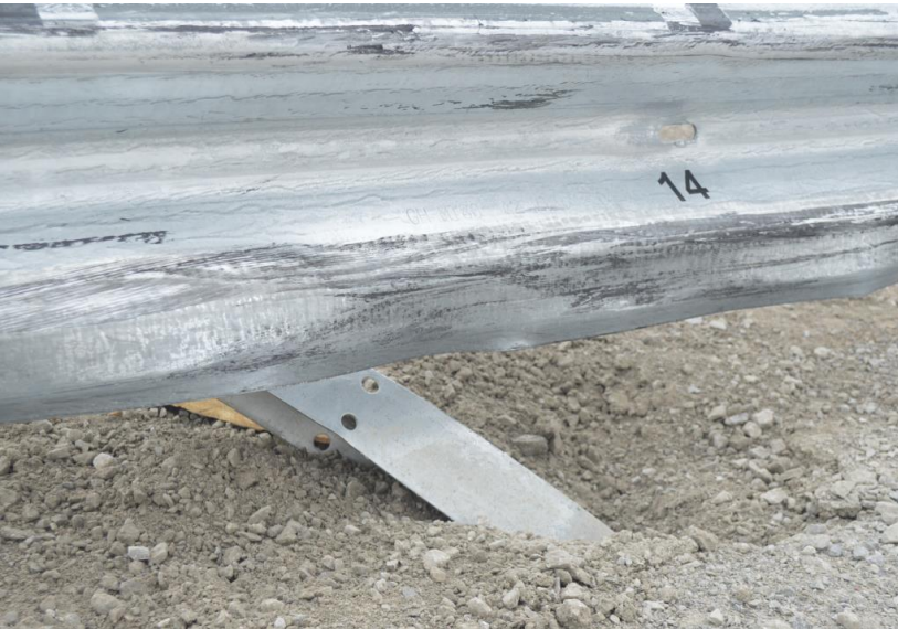
Figure 33. System Damage, Post Nos. 14 and 15, Test No. MGSCO-4
