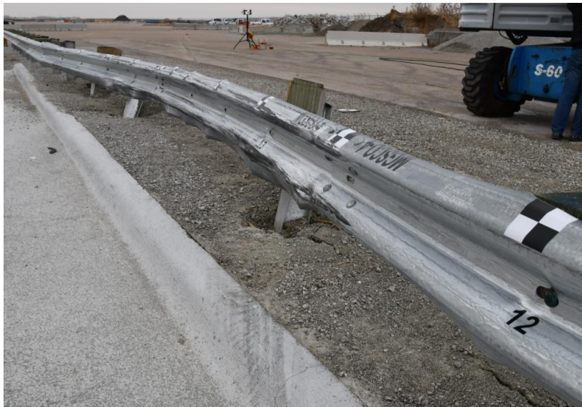
Figure 31. System Damage, Test No. MGSCO-4
