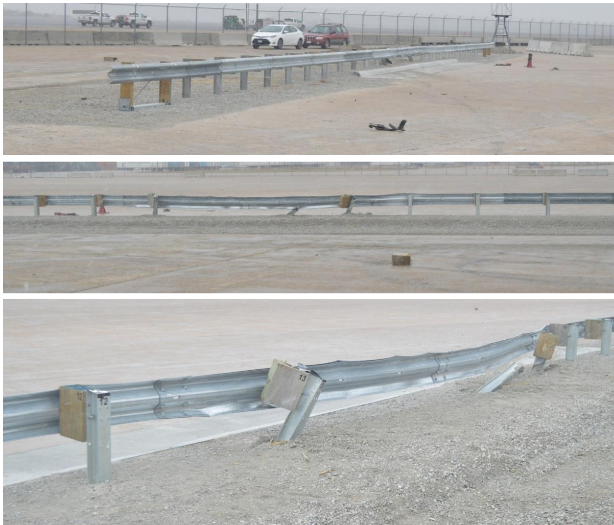
Figure 29. System Damage, Test No. MGSCO-4
