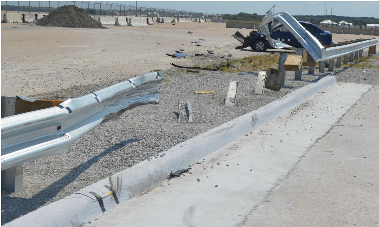
Figure 2. Rail Rupture Resulting from Test No. MGSCO-1
