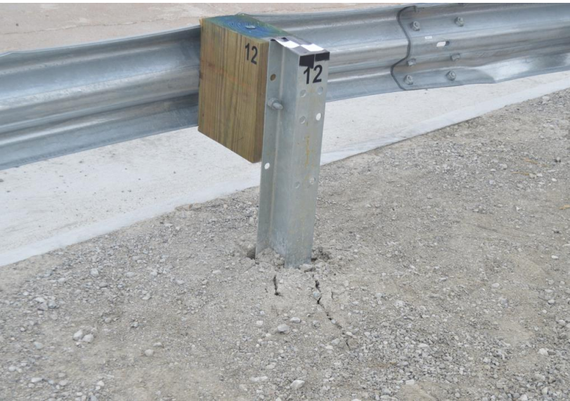
Figure 32. System Damage, Post Nos. 12 and 13, Test No. MGSCO-4
