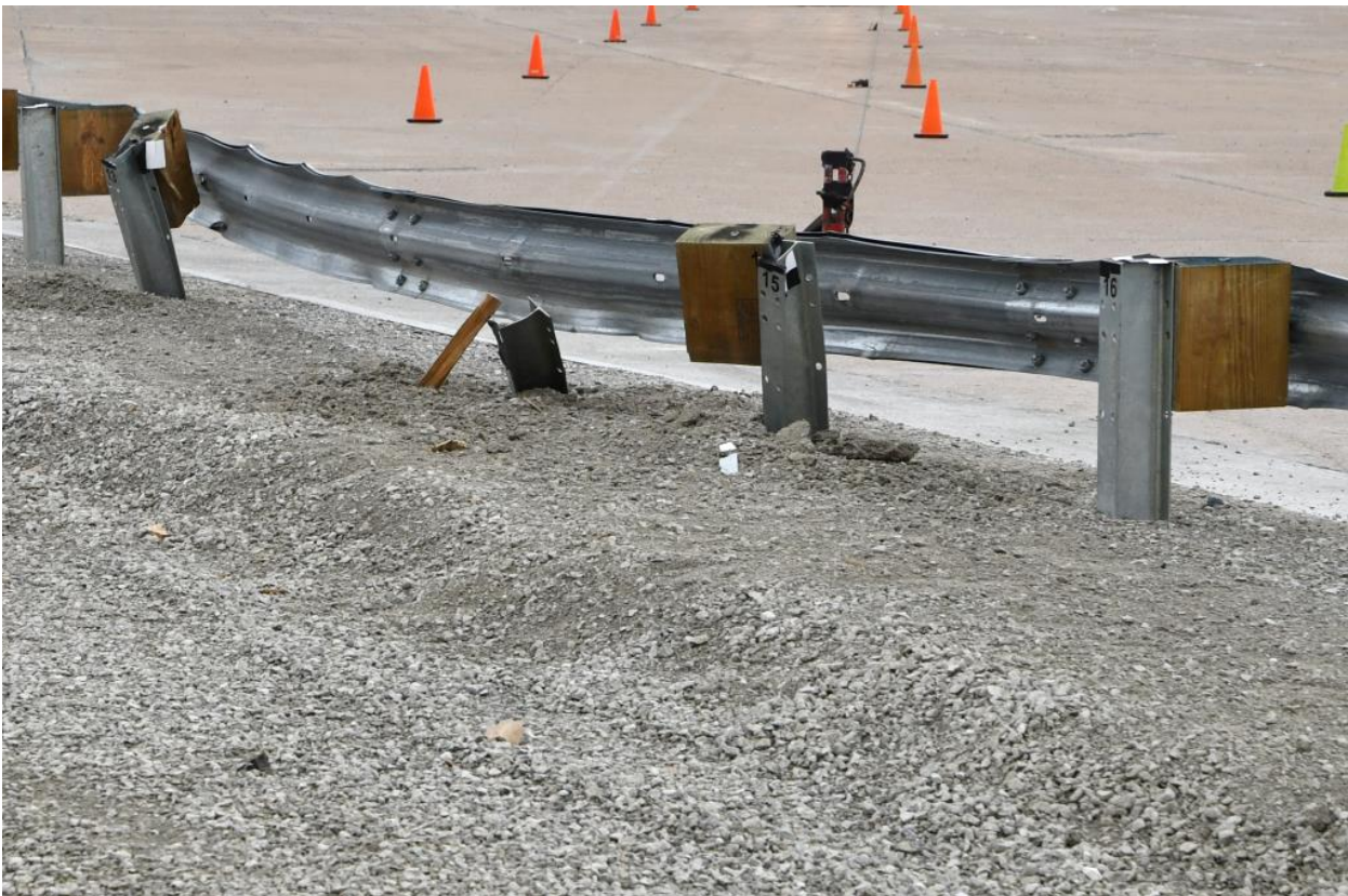
Figure 30. System Damage, Test No. MGSCO-4
