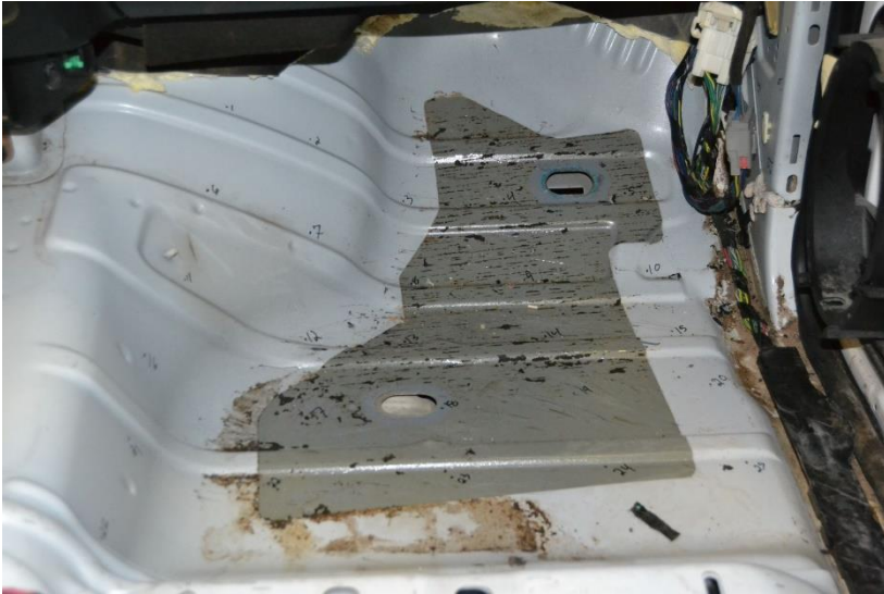
Figure 37. Occupant Compartment and Undercarriage Damage, Test No. MGSCO-4
