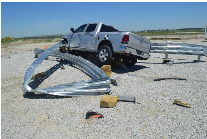
Figure 176. Damage to Rail at Post Nos. B5 through B8, Test No. MSPBN-7
