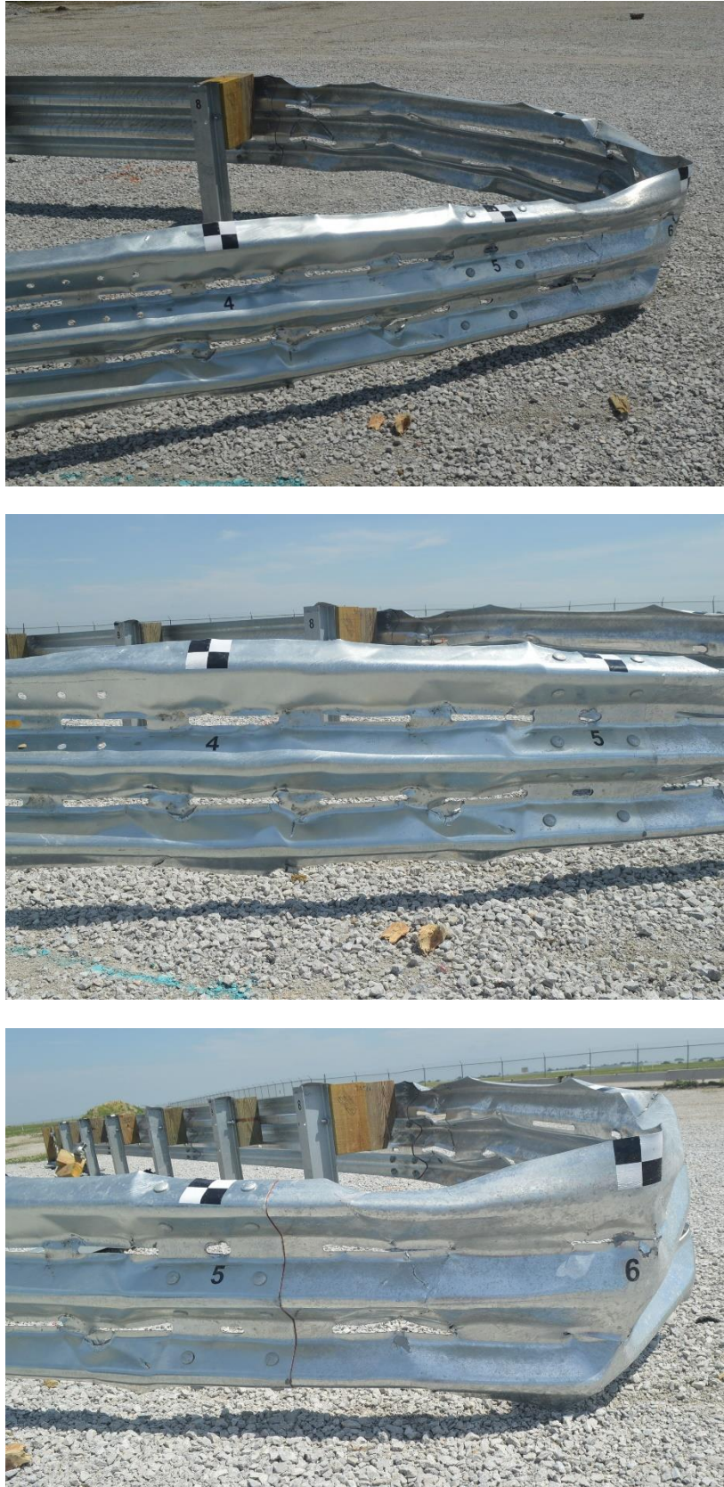
Figure 172. Damage to Rail at Post Nos. A4 through A6, Test No. MSPBN-7
