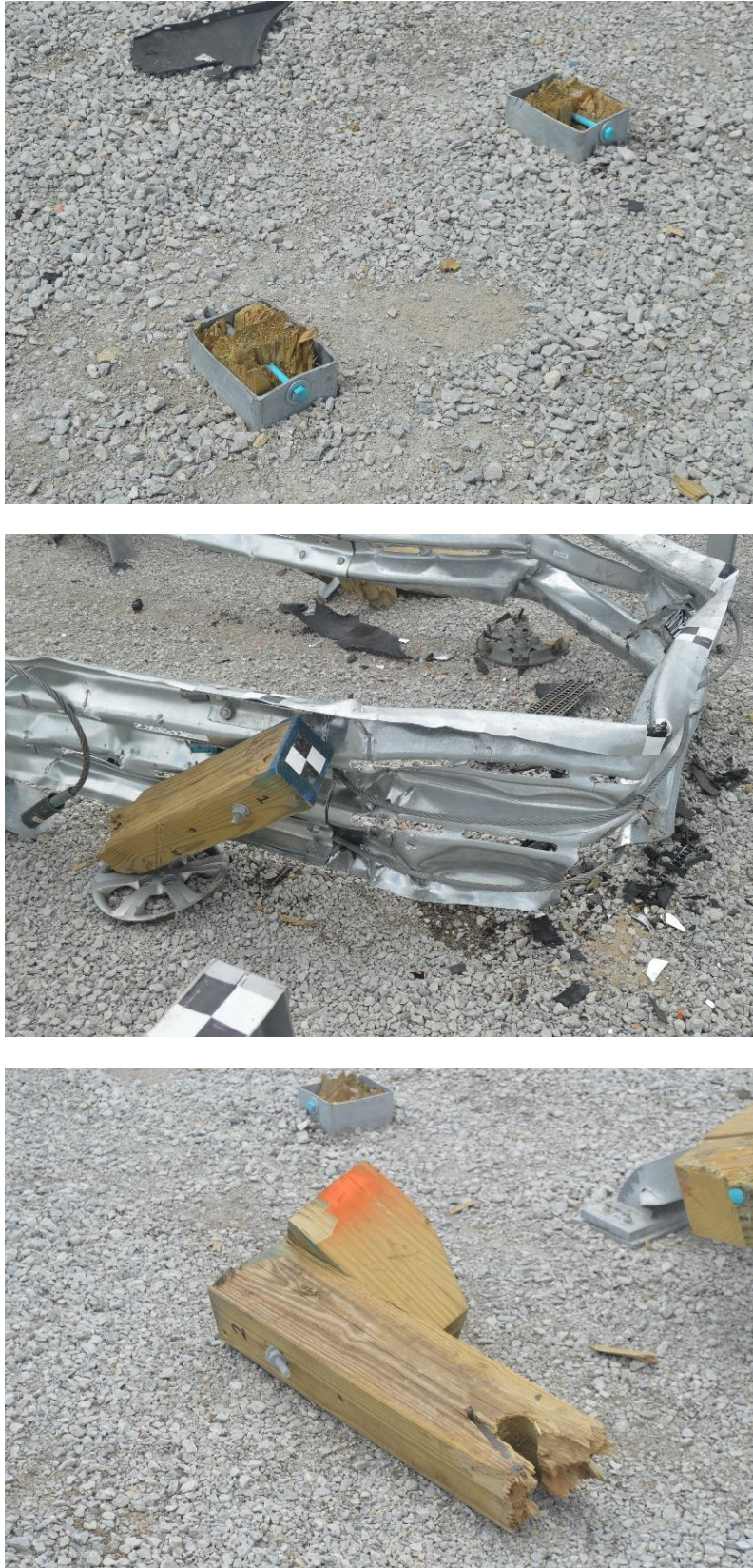
Figure 125. Damage to System at Post Nos. A1 and A2, Test No. MSPBN-5
