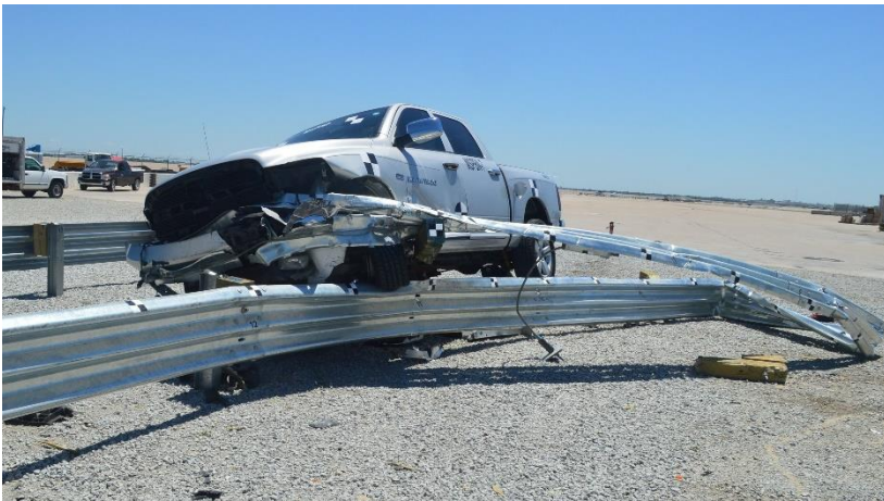
Figure 167. Overview of System Damage with Vehicle Present, Test No. MSPBN-7
