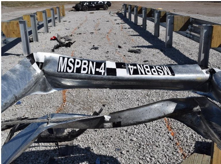
Figure 64. Close Up of Damage to Impact Area, Test No. MSPBN-4
