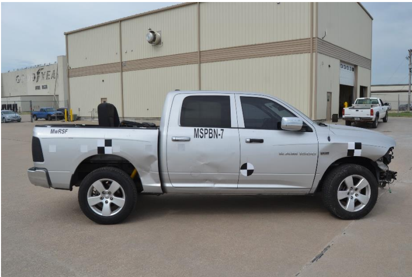
Figure 180. Vehicle Damage, Test No. MSPBN-7
