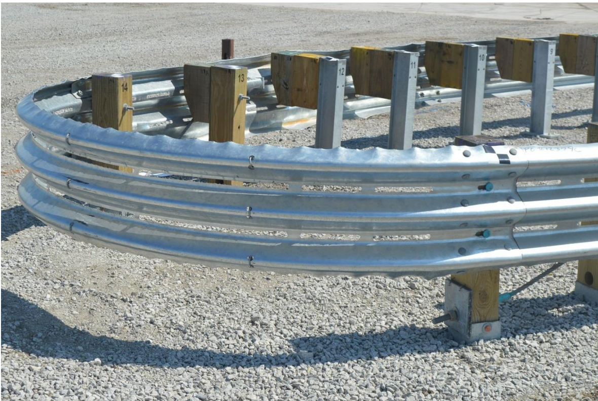
Figure 222. Damage to Impacted Area, Test No. MSPBN-8
