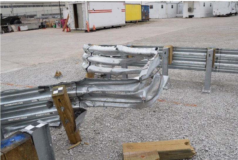
Figure 65. Damage to Post Nos. A1 and A2, Test No. MSPBN-4
