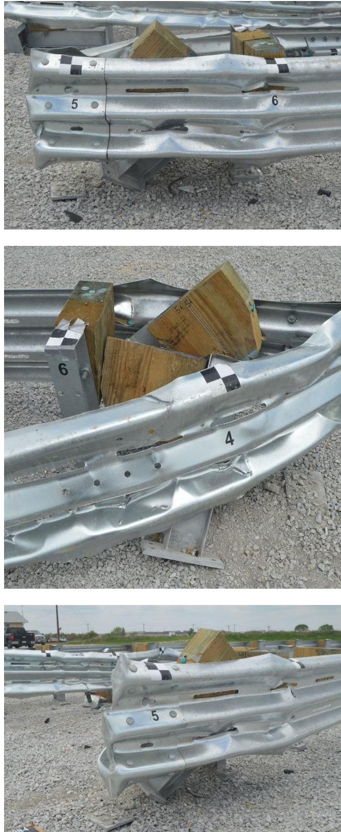
Figure 127. Damage to System at Post Nos. A5 and A6, Test No. MSPBN-5
