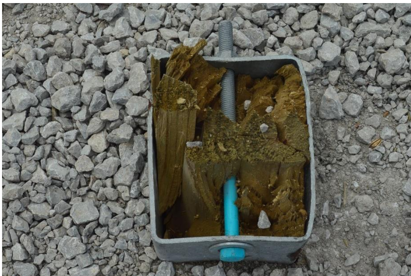
Figure 146. Damage to Post Nos. A1 (middle) and A2 (bottom), Test No. MSPBN-6 183
