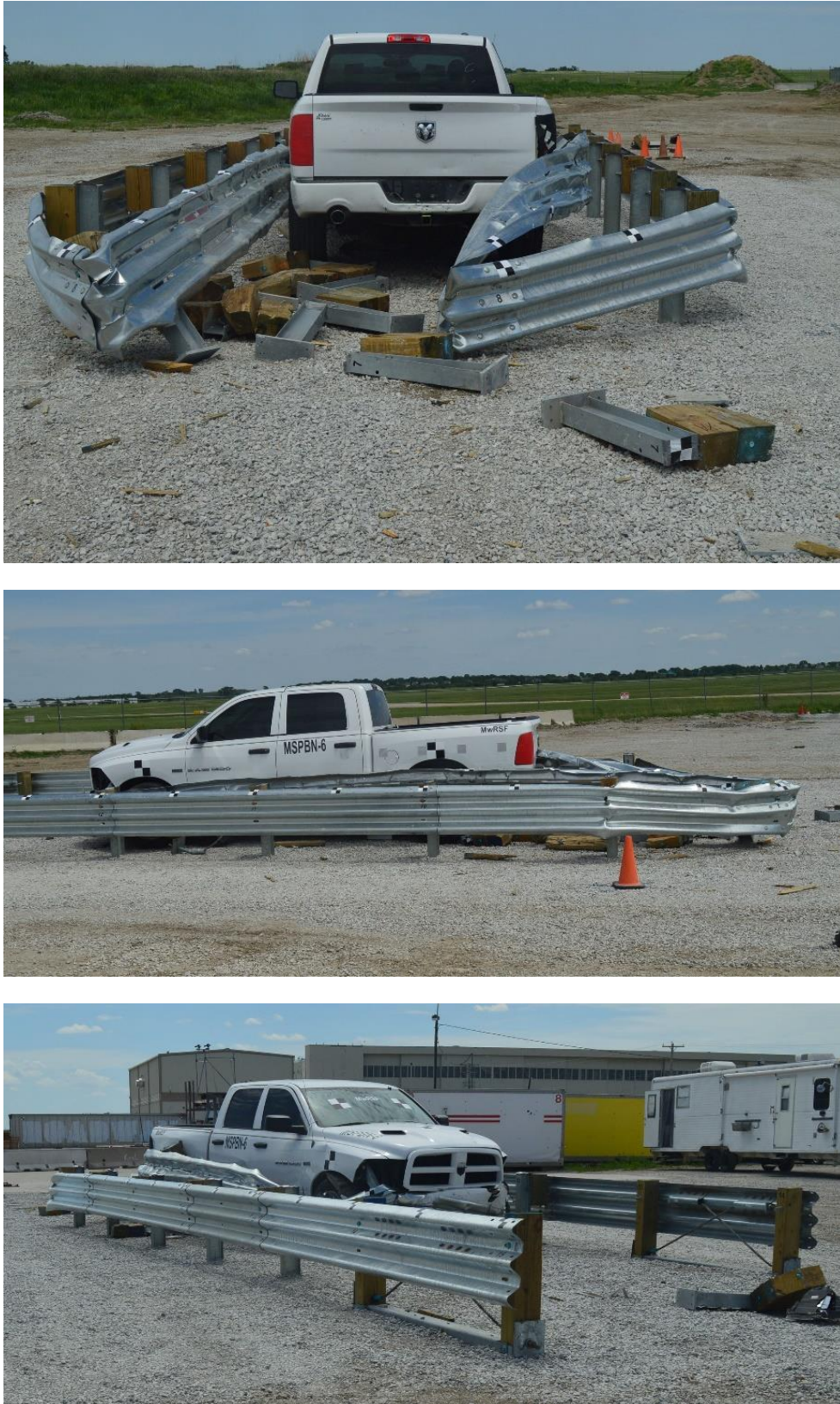
Figure 143. Overview of System Damage with Vehicle Present, Test No. MSPBN-6
