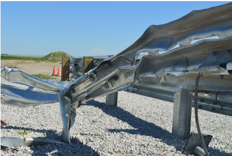
Figure 147. Damage to Rail at Post Nos. A1 and A2, Test No. MSPBN-6
