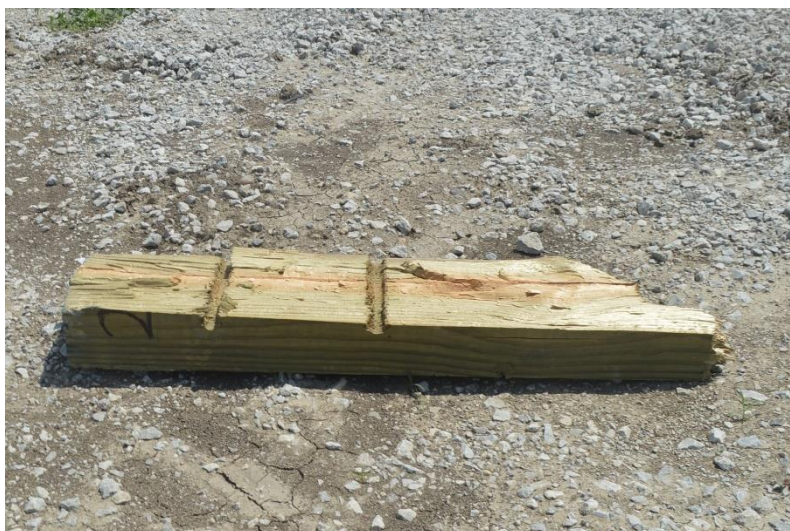
Figure 170. Damage to Post Nos. A1 and A2, Test No. MSPBN-7
