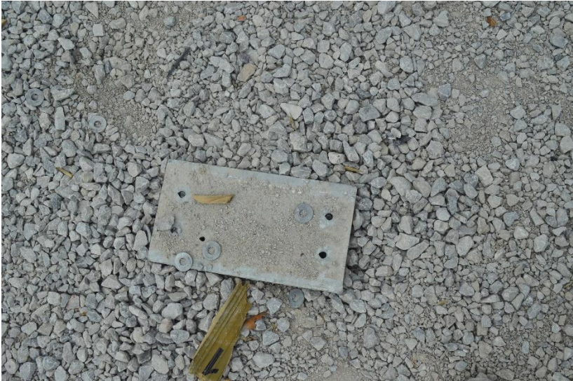
Figure 154. UBSP Post Bases, Test No. MSPBN-6
