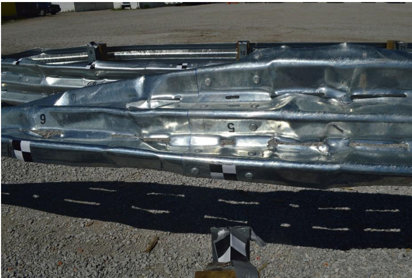
Figure 149. Damage to Rail at Post Nos. A5 through A9, Test No. MSPBN-6
