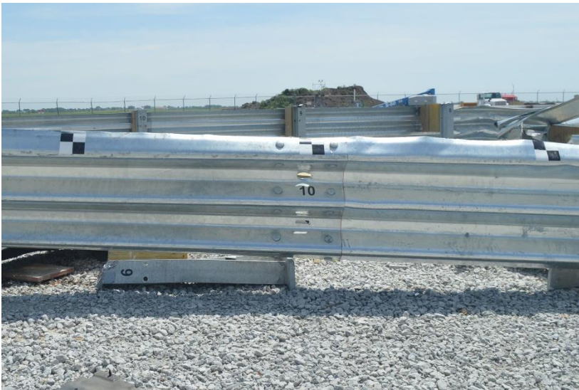
Figure 177. Damage to Rail at Post Nos. B9 through B12, Test No. MSPBN-7
