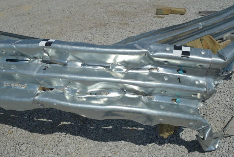
Figure 175. Damage to Rail at Post Nos. B1 through B4, Test No. MSPBN-7
