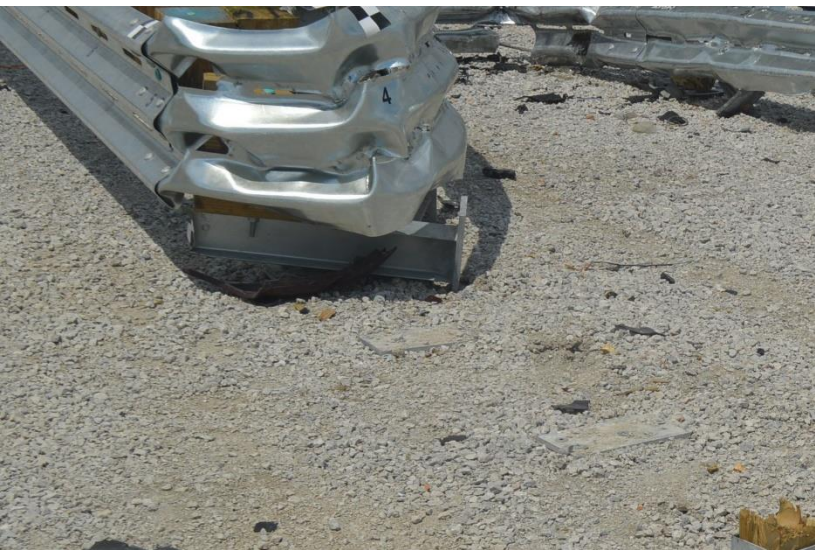
Figure 129. Damage to Post Nos. B3 through B5, Test No. MSPBN-5
