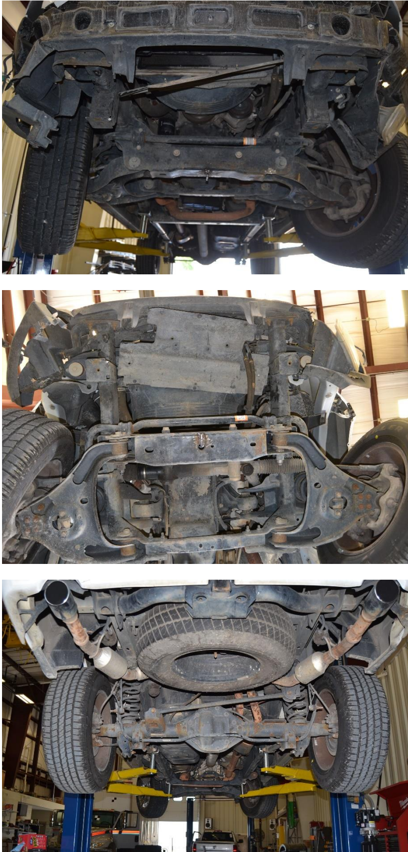
Figure 159. Vehicle Undercarriage Damage, Test No. MSPBN-6
