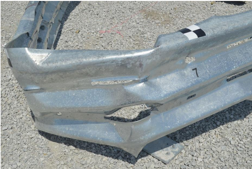
Figure 173. Damage to Rail at Post Nos. A6 through A8, Test No. MSPBN-7
