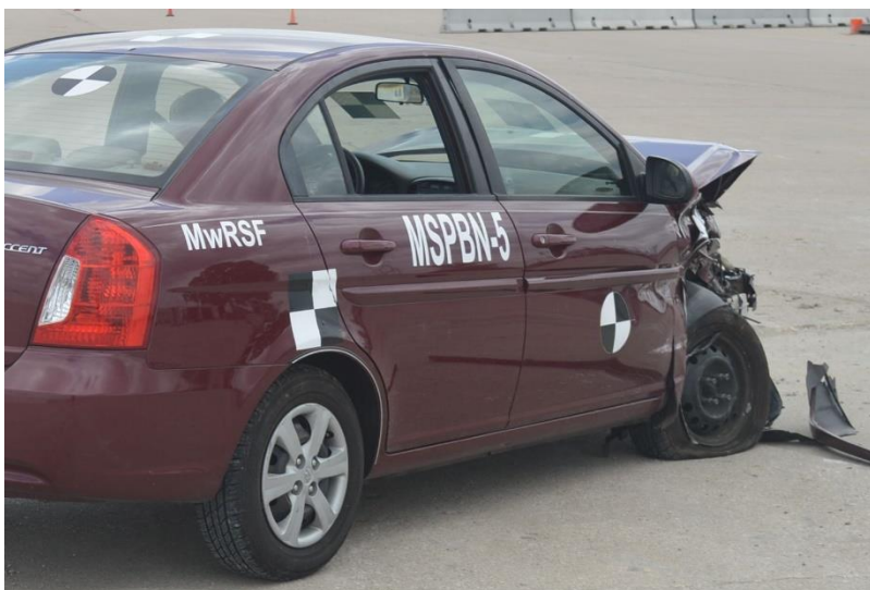
Figure 134. Vehicle Damage, Test No. MSPBN-5
