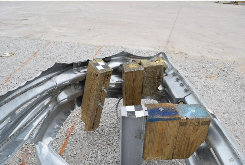
Figure 66. Damage to Post Nos. B1 and B2, Test No. MSPBN-4
