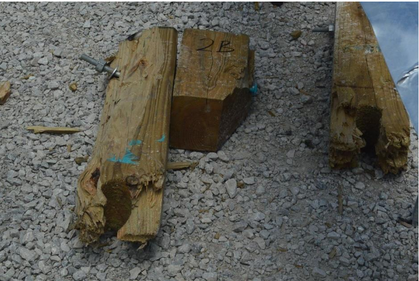
Figure 150. Damage to Post Nos. B1 and B2, Test No. MSPBN-6
