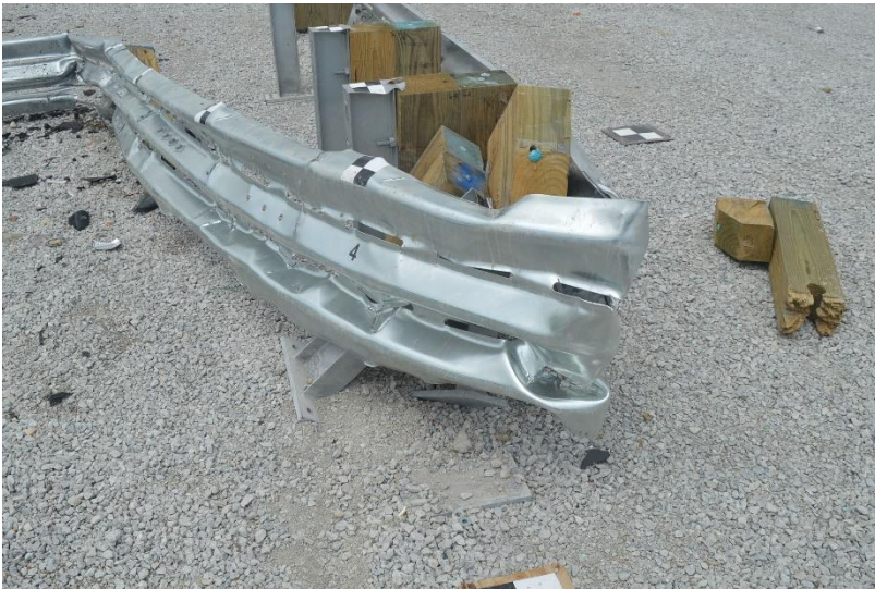
Figure 126. Damage to System at Post Nos. A3 and A4, Test No. MSPBN-5
