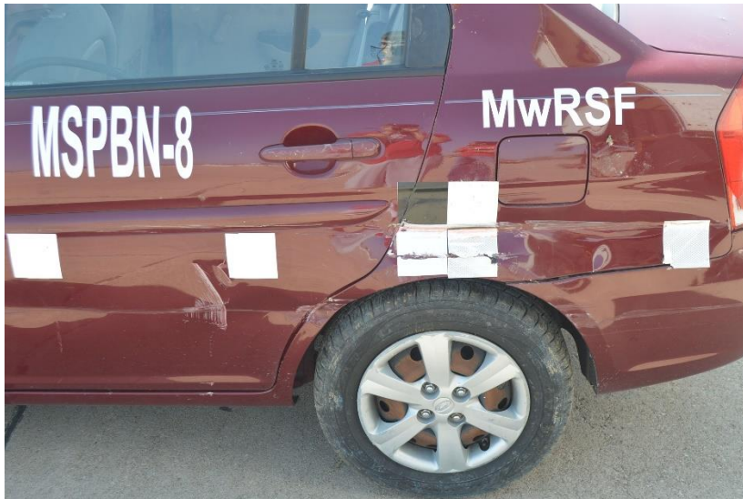
Figure 227. Vehicle Damage, Test No. MSPBN-8
