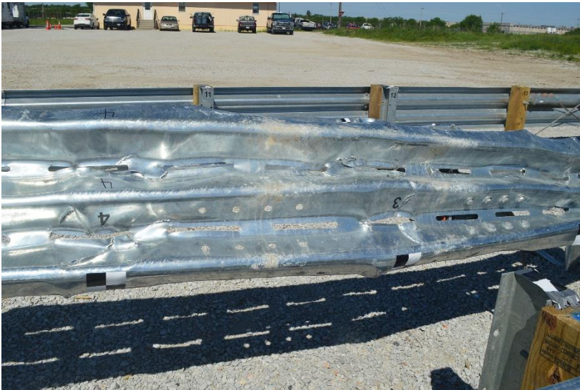
Figure 148. Damage to Rail at Post Nos. A3 and A4, Test No. MSPBN-6
