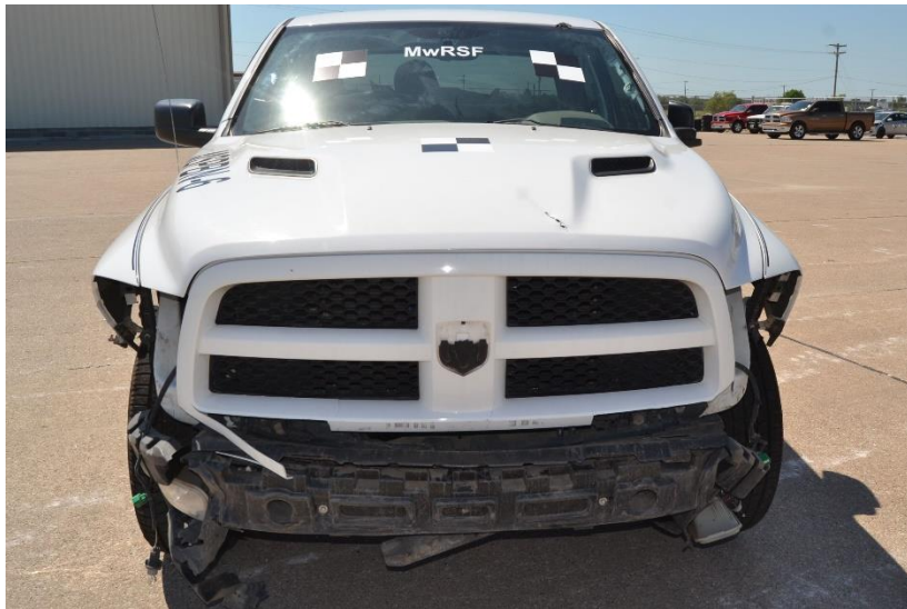
Figure 157. Vehicle Damage, Test No. MSPBN-6
