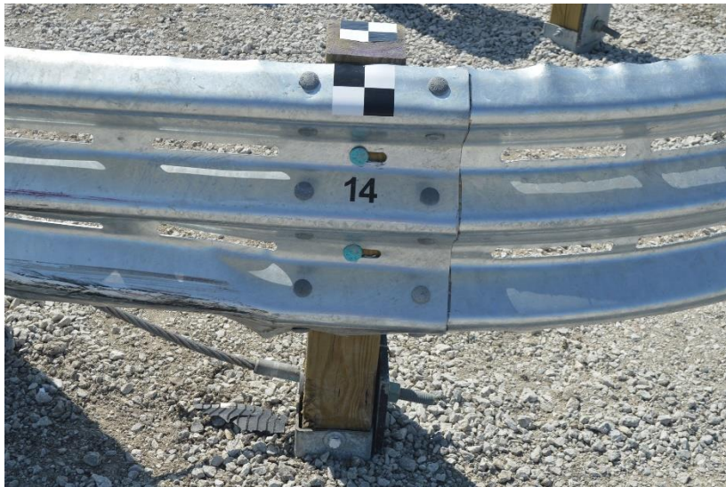
Figure 224. Damage to System at Post Nos. A13 and A14, Test No. MSPBN-8
