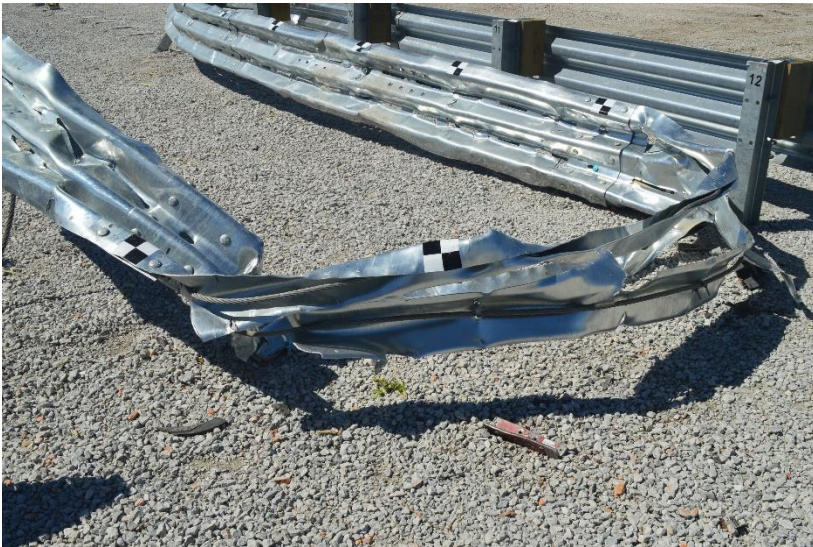
Figure 145. Damage to Impact Location, Test No. MSPBN-6
