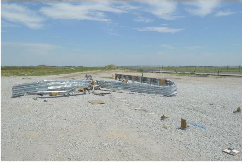
Figure 168. Overview of System Damage without Vehicle Present, Test No. MSPBN-7
