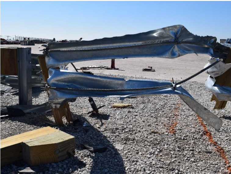
Figure 67. Damage to Impact Location, Test No. MSPBN-4
