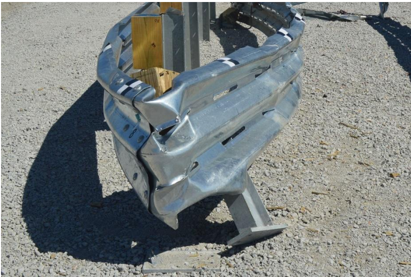
Figure 153. Damage to Railing at Post Nos. B6 through B9, Test No. MSPBN-6
