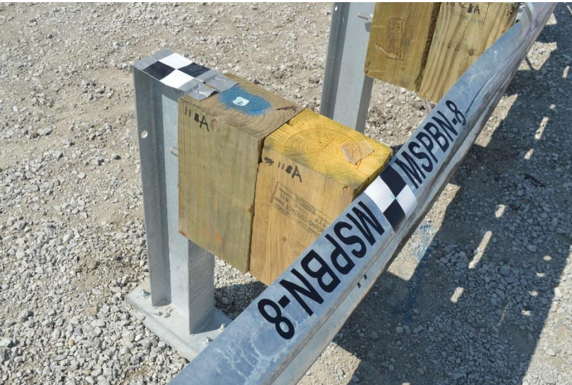
Figure 223. Damage to System at Post Nos. A11 and A12, Test No. MSPBN-8
