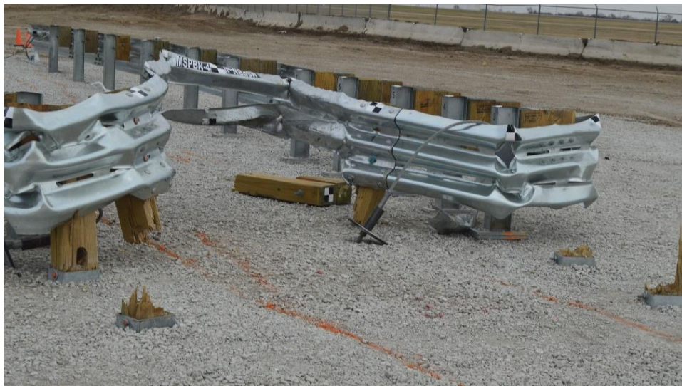
Figure 63. Impact Location Damage, Test No. MSPBN-4
