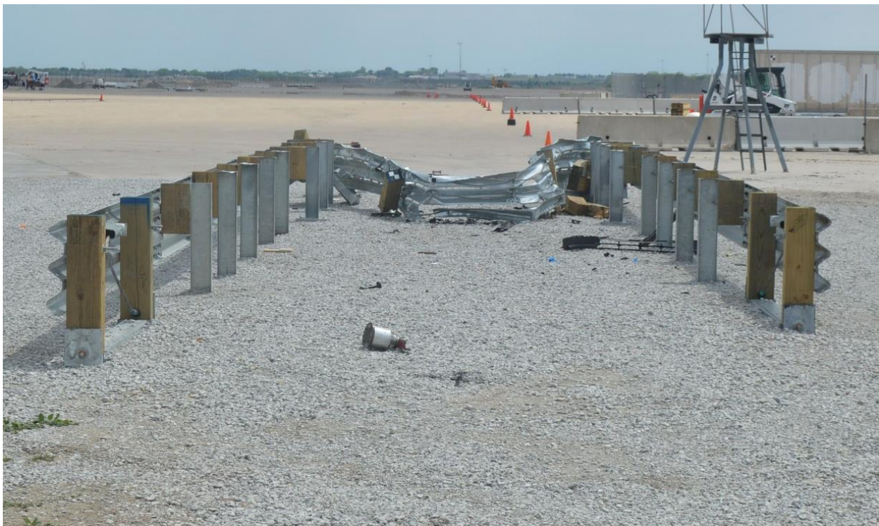
Figure 123. Overview of System Damage, Test No. MSPBN-5
