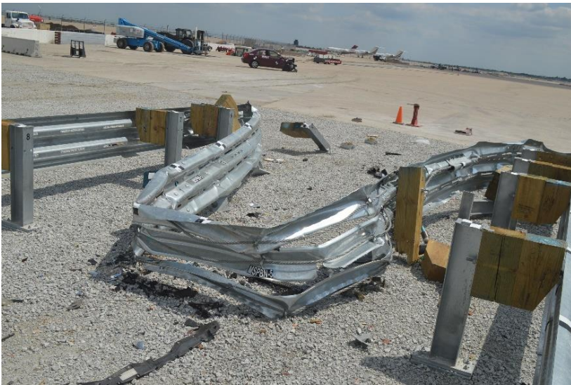
Figure 124. Close-Up of Impacted Area, Test No. MSPBN-5
