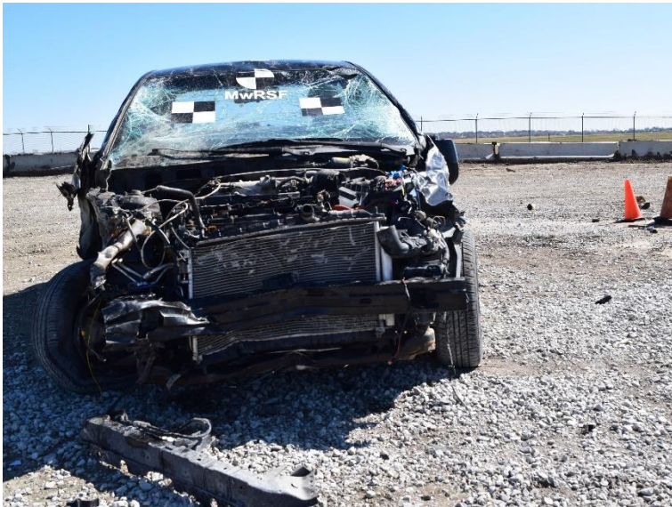
Figure 70. Vehicle Damage, Test No. MSPBN-4
