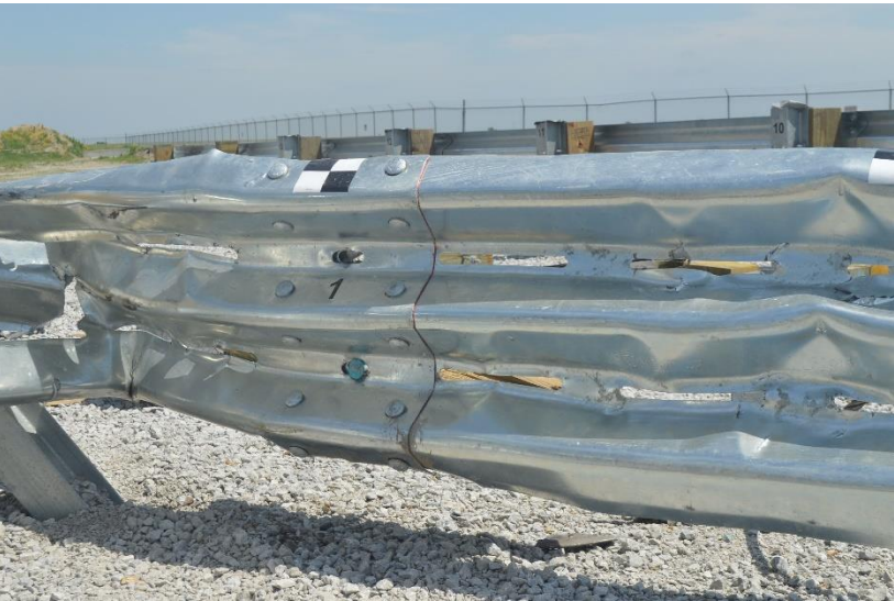
Figure 171. Damage to Rail at Post Nos. A1 through A3, Test No. MSPBN-7
