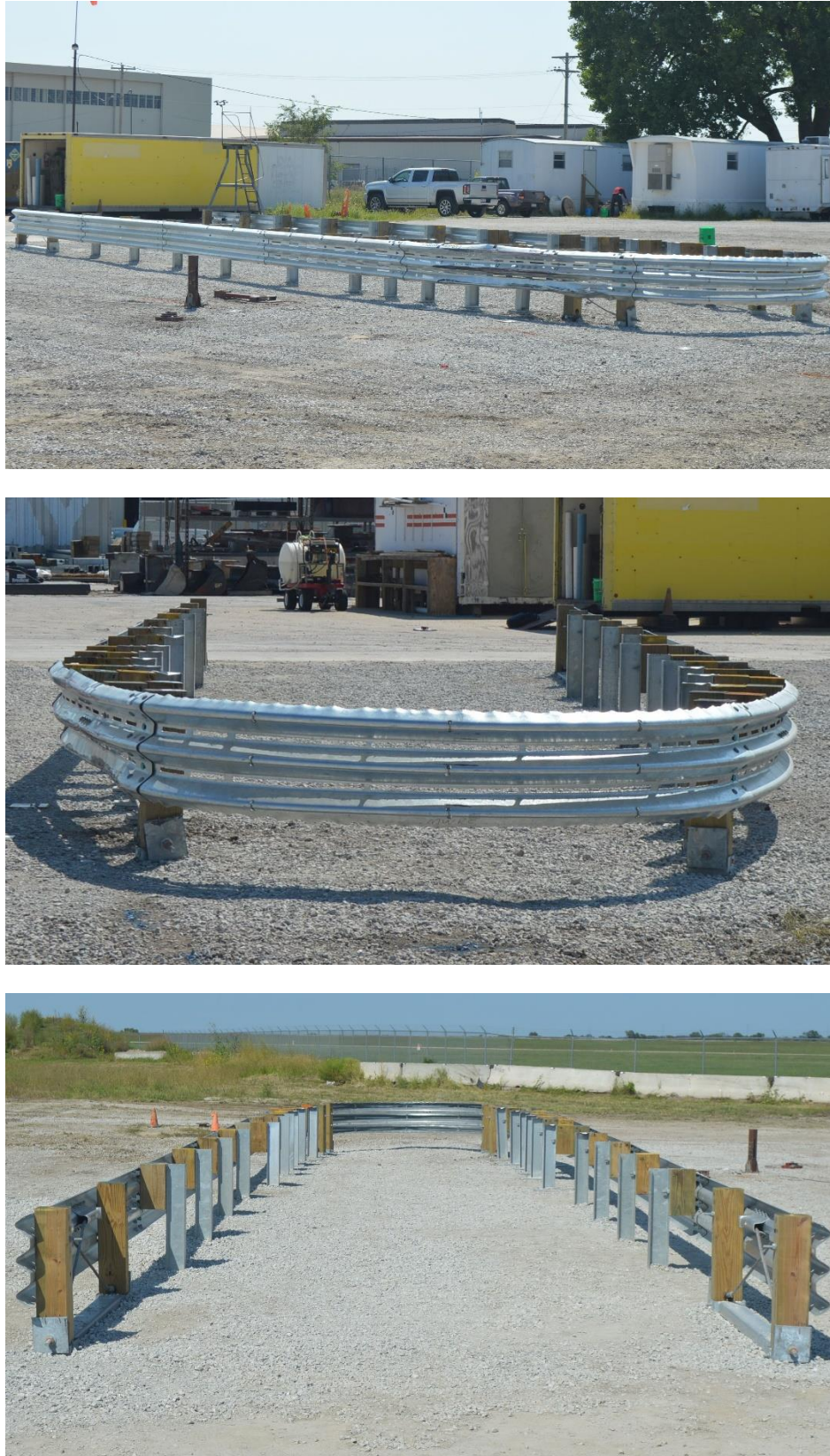
Figure 221. Overview of Damage to System, Test No. MSPBN-8
