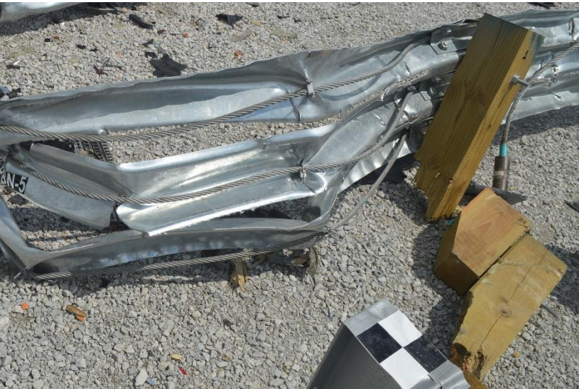
Figure 128. Damage to System at Post Nos. B1 and B2, Test No. MSPBN-5
