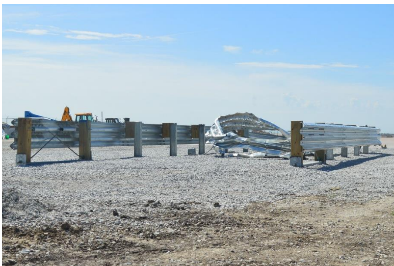
Figure 144. Overview of System Damage with Vehicle Removed, Test No. MSPBN-6.
