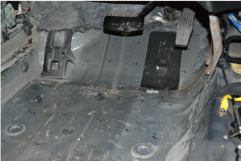
Figure 72. Vehicle Interior Damage, Test No. MSPBN-4
