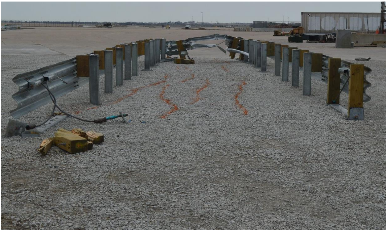
Figure 62. Overview of System Damage, Test No. MSPBN-4
