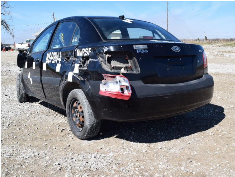
Figure 71. Vehicle Damage, Test No. MSPBN-4
