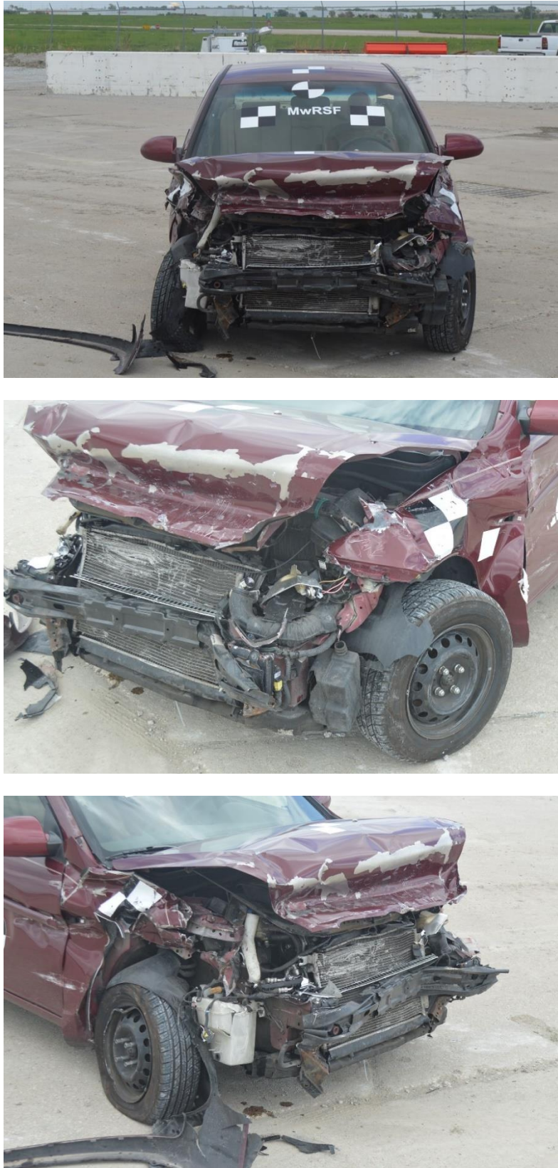
Figure 133. Vehicle Damage, Test No. MSPBN-5
