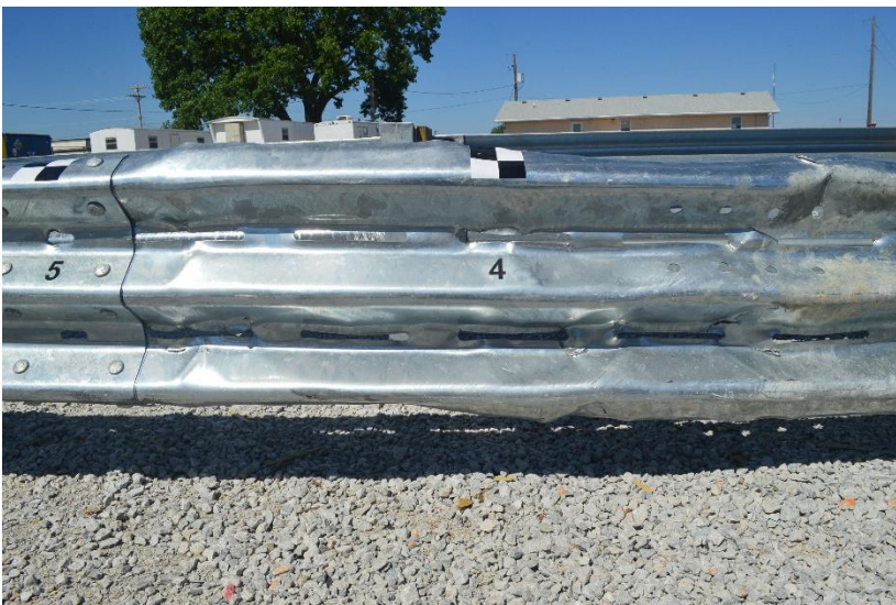
Figure 152. Damage to Rail at Post Nos. B3 through B5, Test No. MSPBN-6
