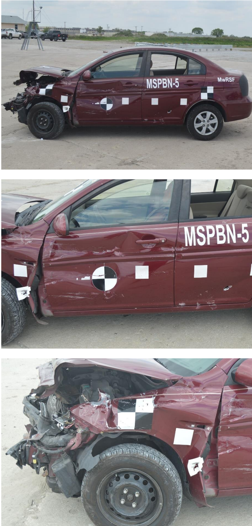
Figure 132. Vehicle Damage, Test No. MSPBN-5
