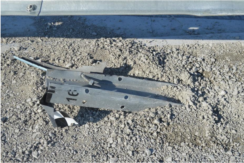
Figure 55. Post Nos. 16 and 17 Damage, Test No. MGSC-7
