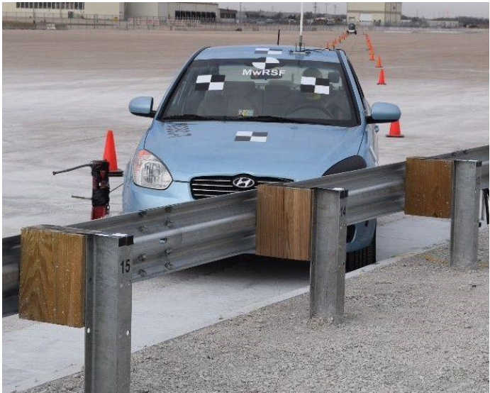
Figure 41. Impact Location, Test No. MGSC-7
