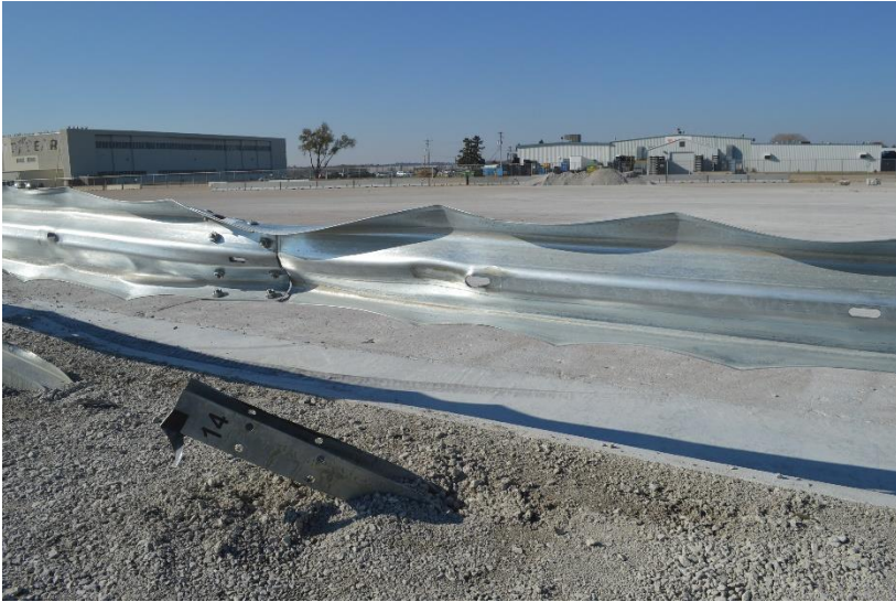
Figure 52. Backside Guardrail Damage, Post Nos. 13 through 16, Test No. MGSC-7
