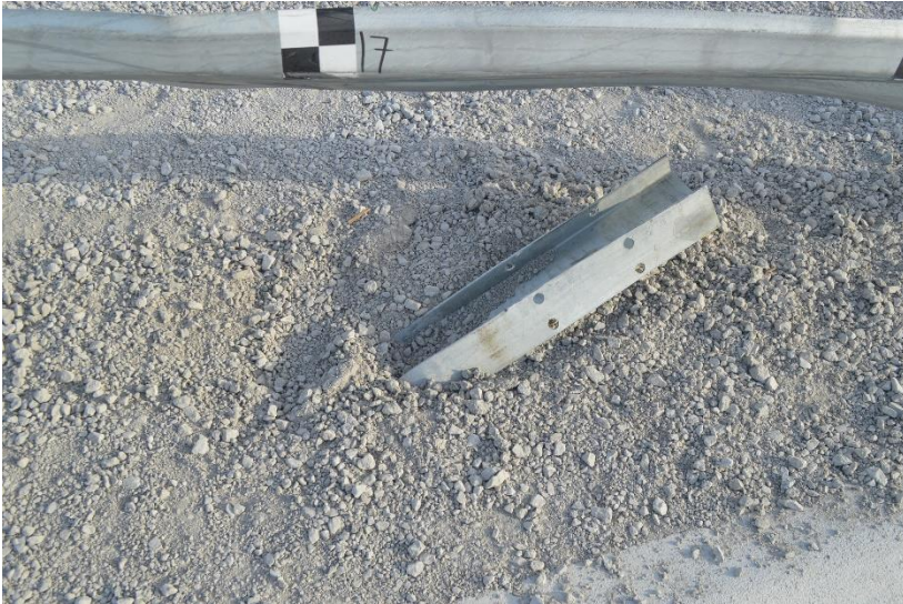
Figure 78. System Damage, Post Nos. 16 through 19, Test No. MGSC-8
