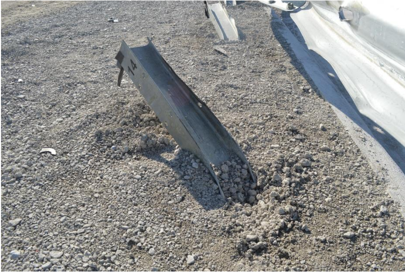
Figure 54. Post Nos. 14 and 15 Damage, Test No. MGSC-7
