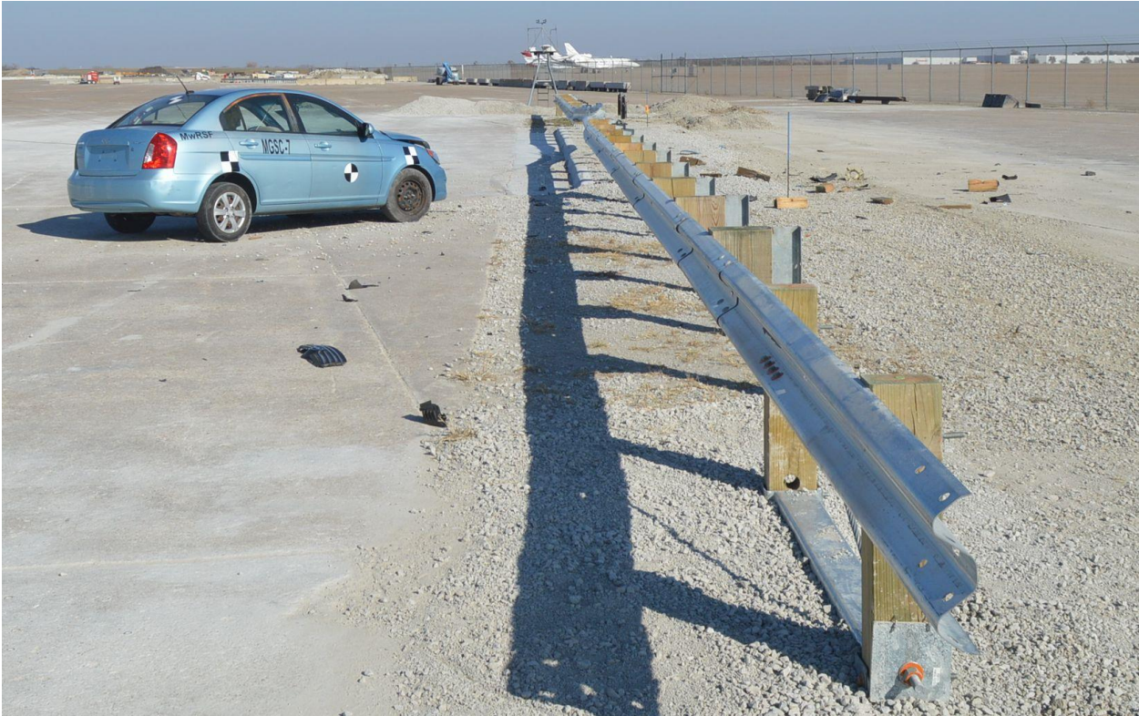
Figure 48. Vehicle Final Position and Trajectory Marks, Test No. MGSC-7
