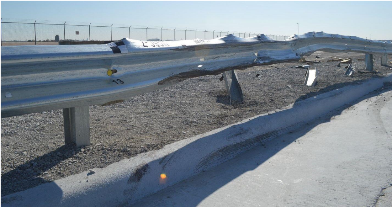
Figure 49. System Damage, Test No. MGSC-7
