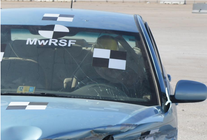
Figure 60. Vehicle Damage, Test No. MGSC-7
