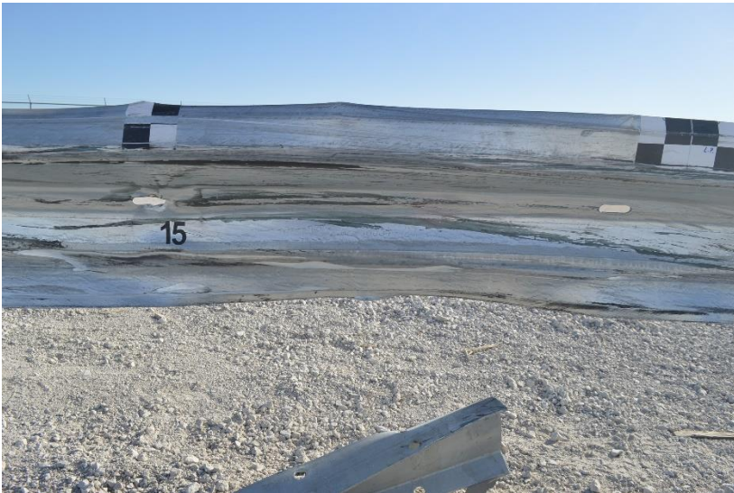
Figure 73. System Damage, Guardrail at Post Nos. 14 through 17, Test No. MGSC-8
