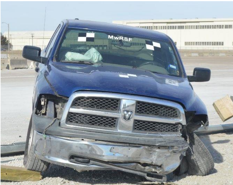
Figure 81. Vehicle Damage, Test No. MGSC-8
