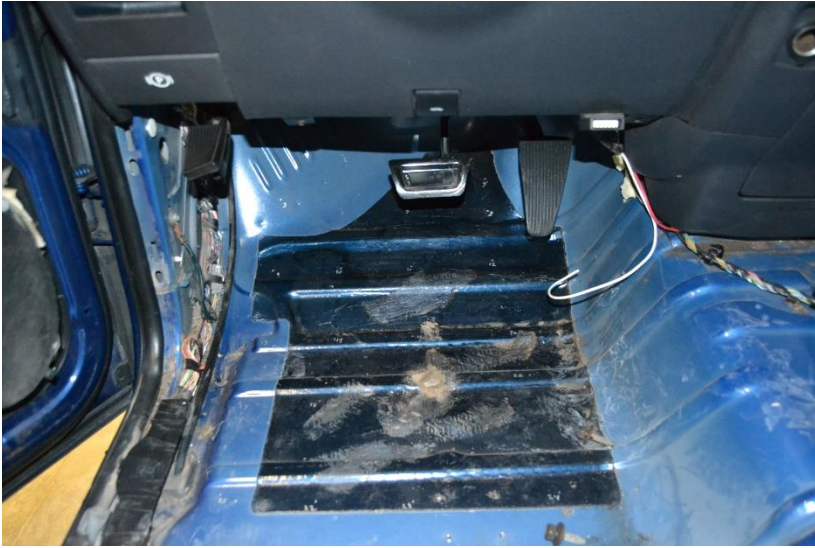
Figure 84. Occupant Compartment Damage, Test No. MGSC-8
