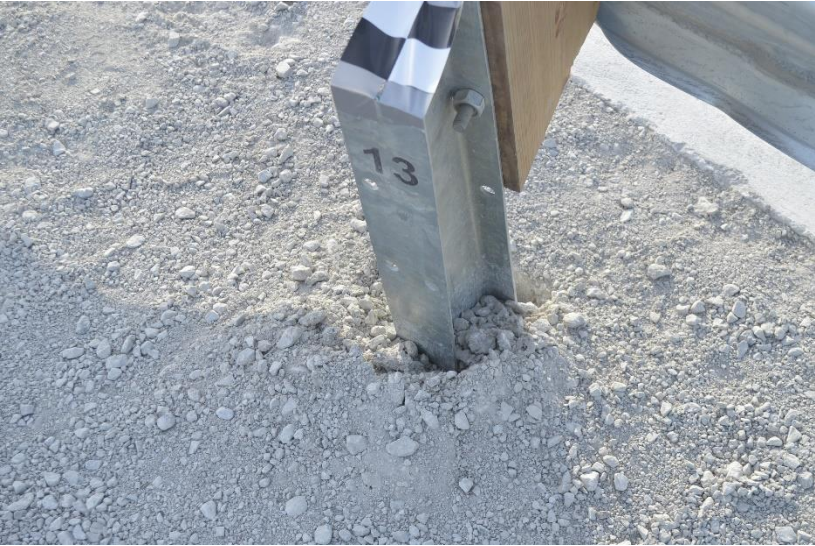
Figure 77. System Damage, Post Nos. 12 through 15, Test No. MGSC-8
