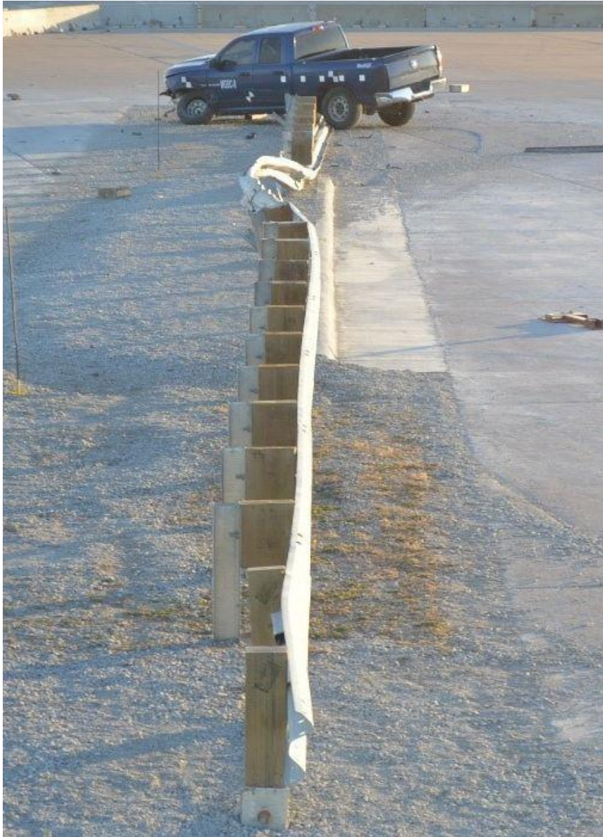
Figure 70. Vehicle Final Position and Trajectory Marks, Test No. MGSC-8
