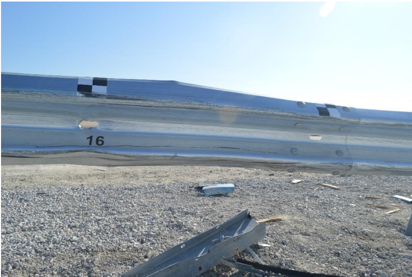
Figure 51. Guardrail Damage, Post Nos. 15 through 18 Test No. MGSC-7
