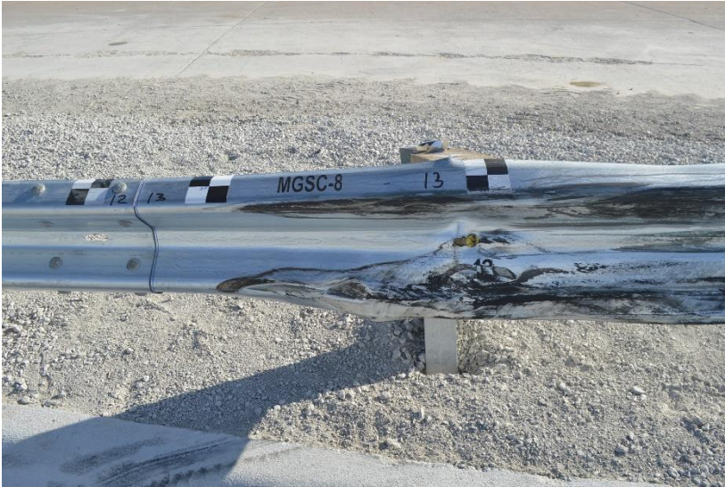
Figure 72. System Damage, Guardrail at Post Nos. 12 through 14, Test No. MGSC-8
