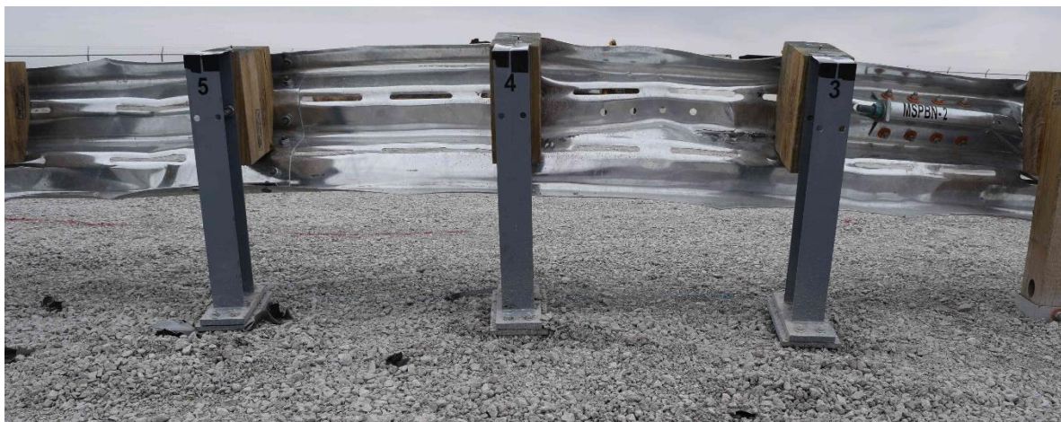
Figure 80. Blockout Damage, Test No. MSPBN-2 100
