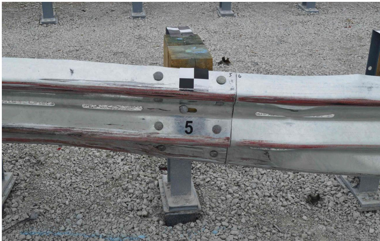
Figure 82. Post Nos. A4 and A5 Damage, Test No. MSPBN-2
