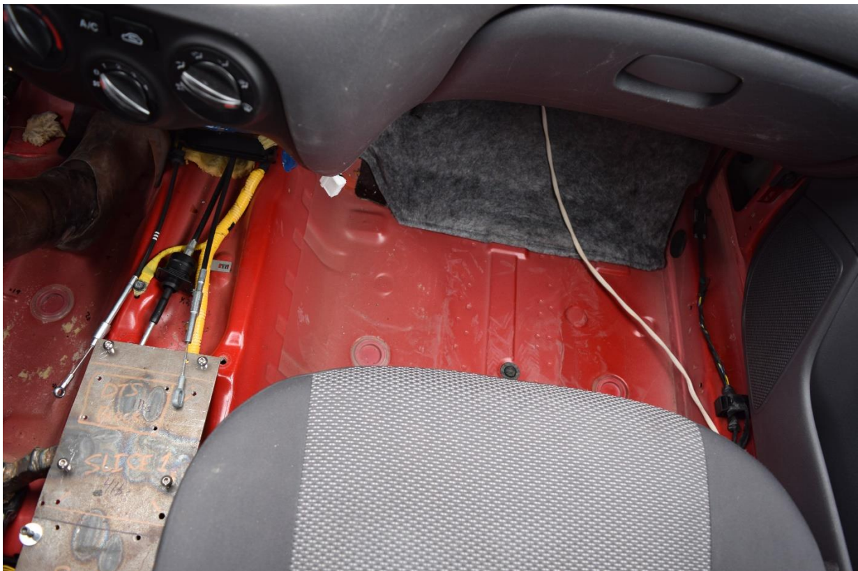
Figure 86. Floorboard Damage, Test No. MSPBN-2
