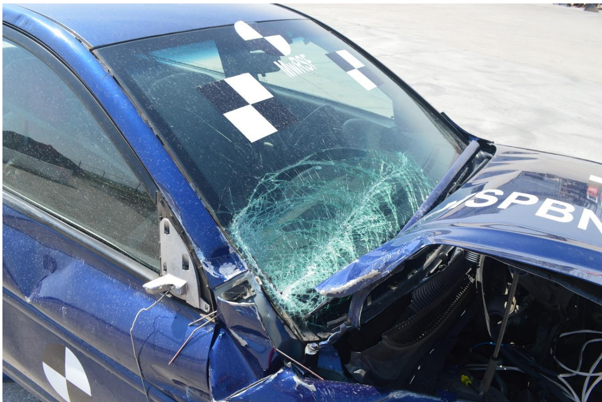
Figure 100. Windshield Damage, Test No. MSPBN-3
