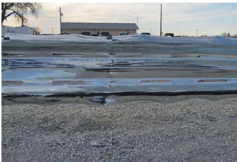
Figure 62. Post Nos. A6 and A7 Damage, Test No. MSPBN-1
