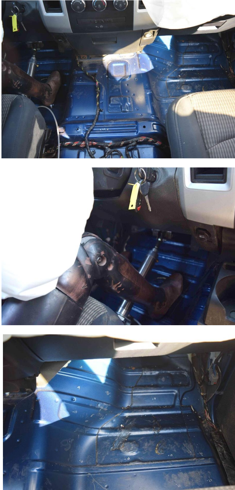
Figure 70. Interior Floorboard Damage, Test No. MSPBN-1
