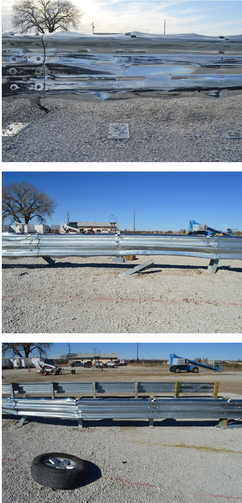
Figure 59. Post Nos. A6 through A13 Damage, Test No. MSPBN-1
