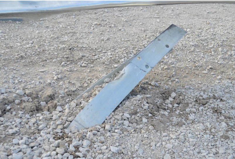
Figure 63. Post Nos. A8 and A9 Damage, Test No. MSPBN-1
