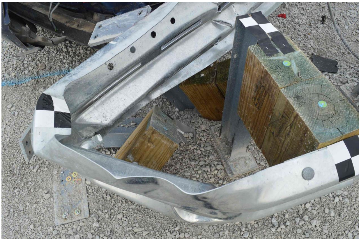
Figure 96. Post Nos. A3, A4, and A5 Damage, Test No. MSPBN-3
