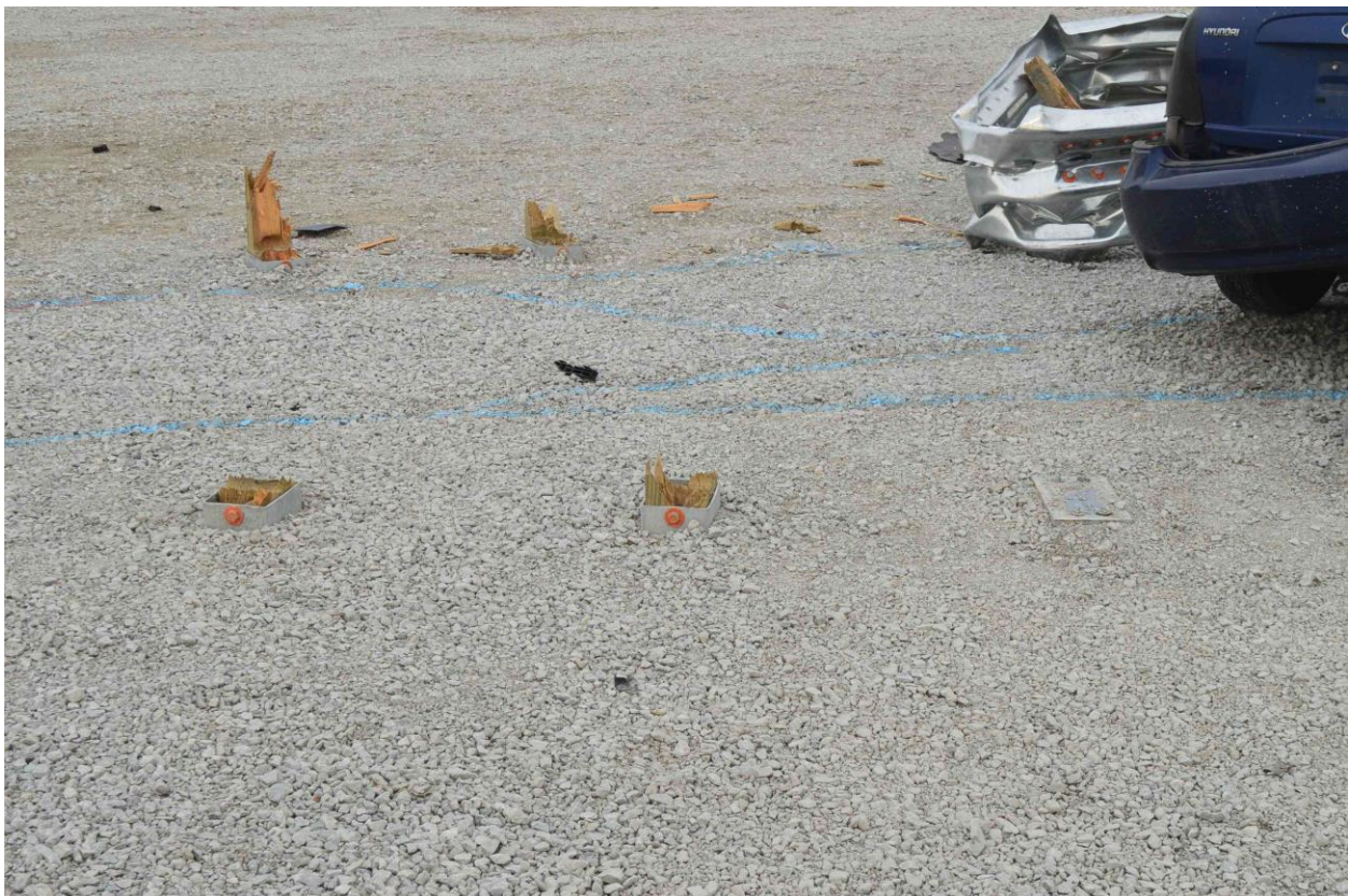
Figure 95. Post Nos. A1, A2, A3, B1, B2, and B3 Damage, Test No. MSPBN-3
