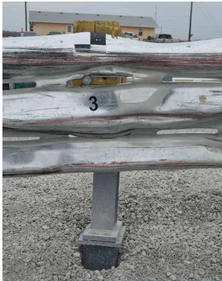
Figure 81. Post Nos. A2 and A3 Damage, Test No. MSPBN-2
