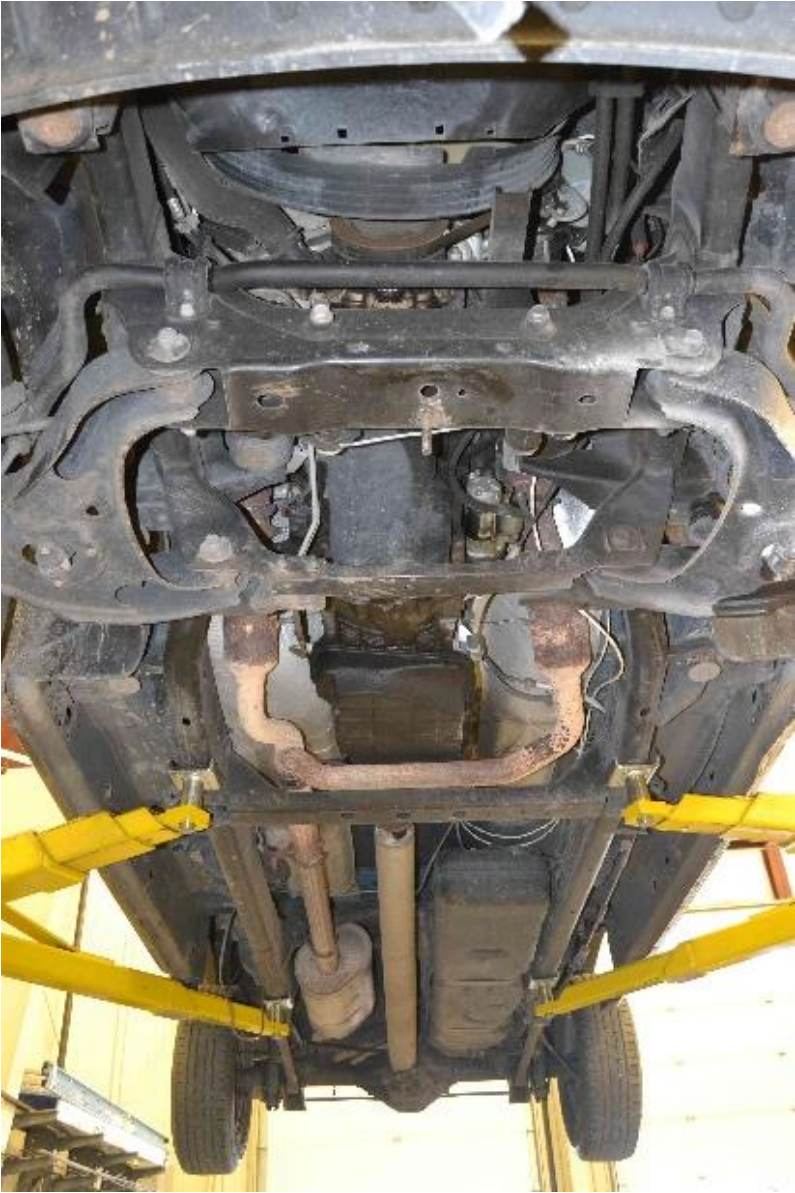
Figure 71. Undercarriage Damage, Test No. MSPBN-1
