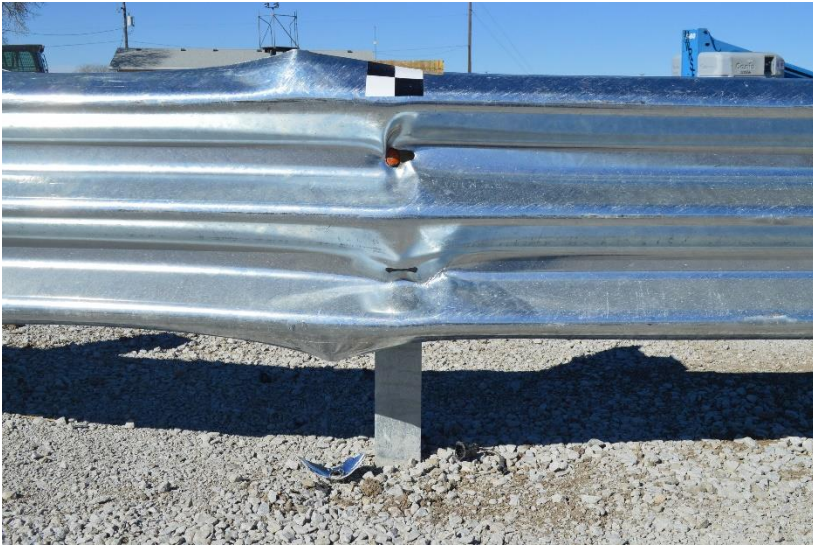
Figure 64. Post Nos. A10 and A11 Damage, Test No. MSPBN-1
