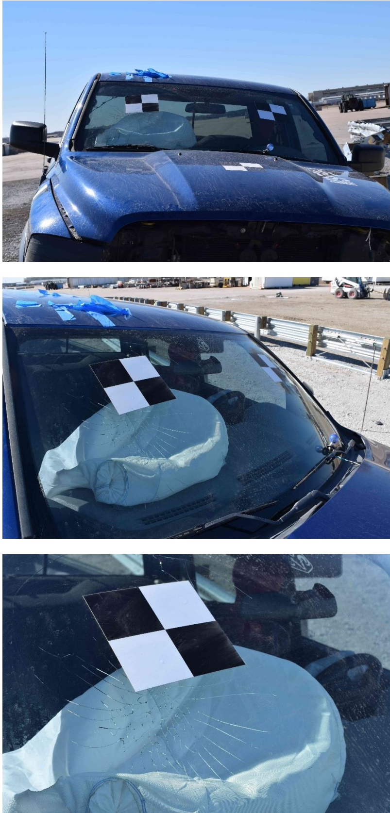
Figure 69. Windshield Damage Test No. MSPBN-1
