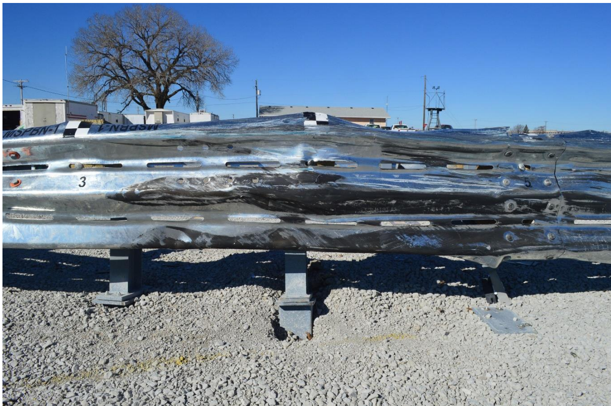
Figure 58. Post Nos. A1 through A5 Damage, Test No. MSPBN-1
