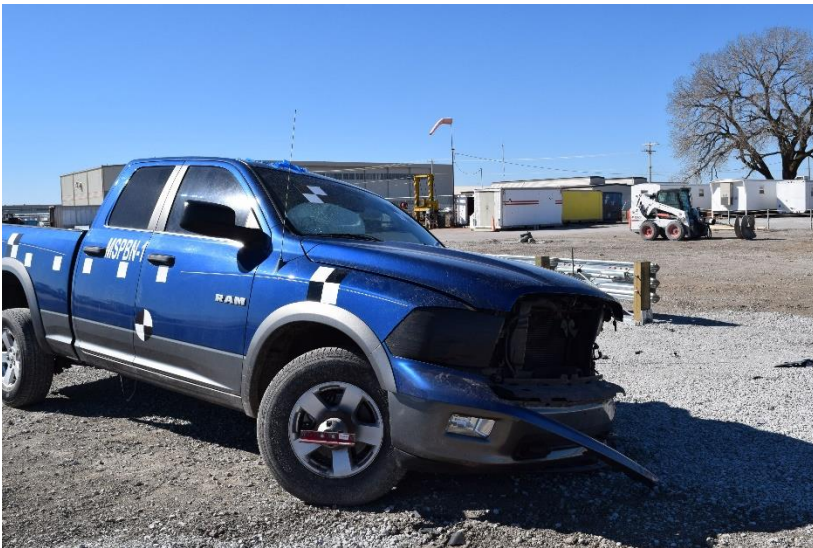
Figure 67. Vehicle Damage, Test No. MSPBN-1
