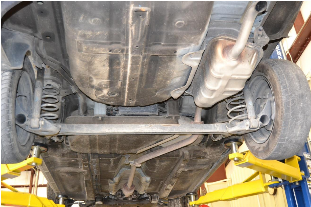
Figure 103. Undercarriage Damage, Test No. MSPBN-3
