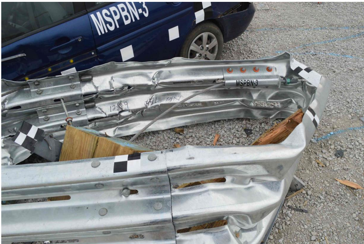
Figure 97. Post nos. B3, B4, and B5 Damage, Test No. MSPBN-3
