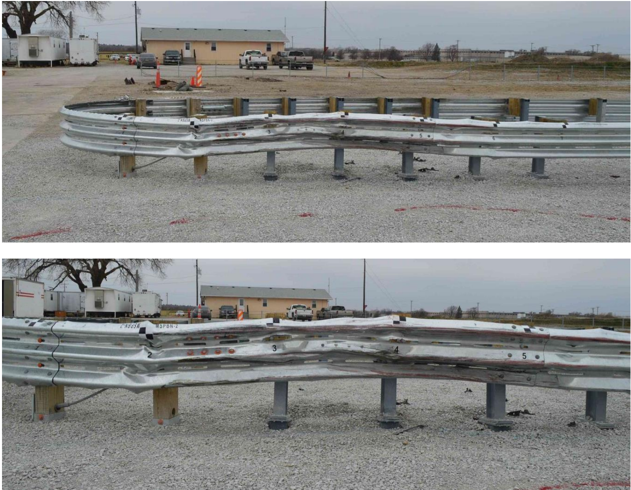
Figure 79. Post nos. A1 through A5 Damage, Test No. MSPBN-2
