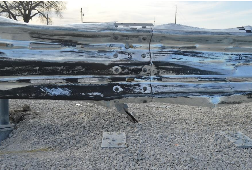
Figure 61. Post Nos. A4 and A5 Damage, Test No. MSPBN-1
