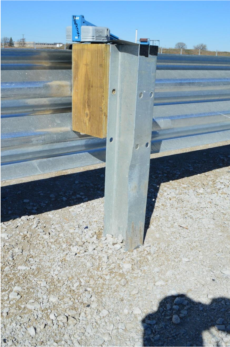
Figure 65. Post No. B9 Damage, Test No. MSPBN-1
