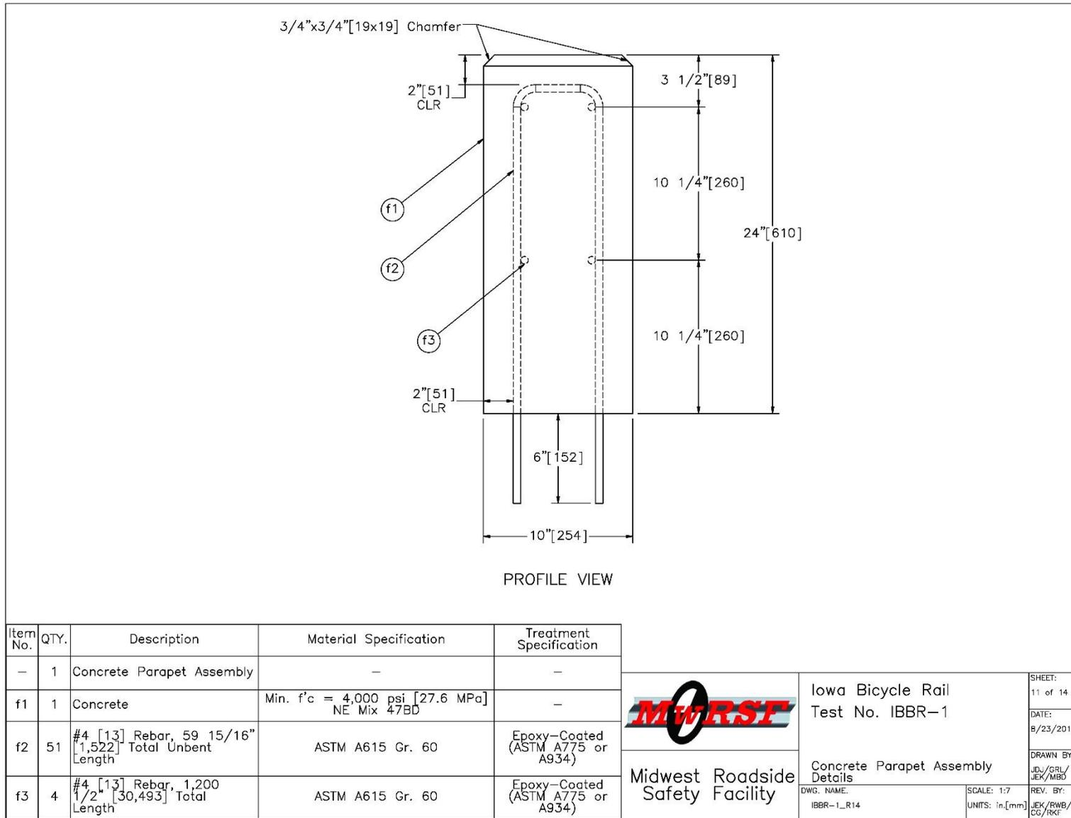
Figure 12. Concrete Parapet Assembly Details, Test No. IBBR-1
