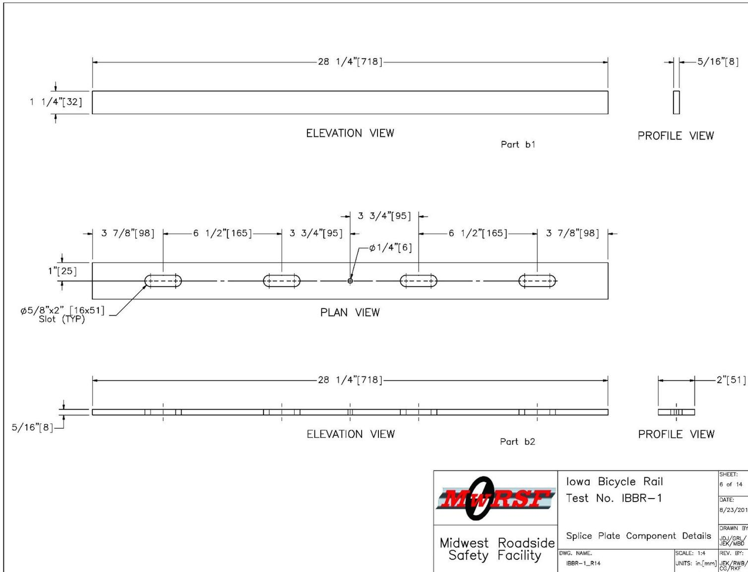
Figure 7. Splice Plate Component Details, Test No. IBBR-1
