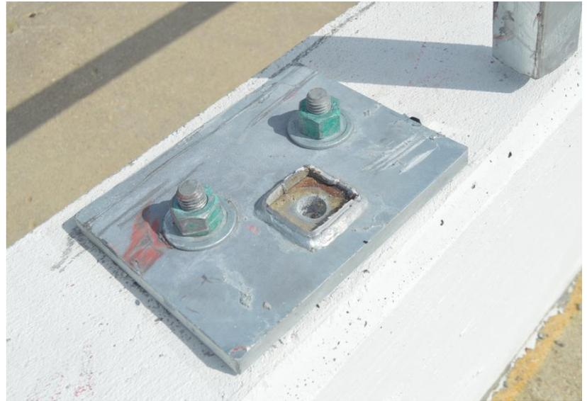
Figure 33. Post No. 4 Damage, Test No. IBBR-1
