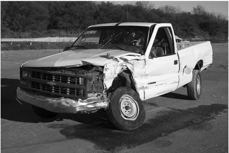
Figure 43. Tapered Tubular Rail Contact, Test No. 401021-3 [24]
