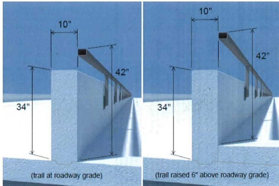
Figure 1. Iowa DOT Alternate Separation Barrier (in service)
