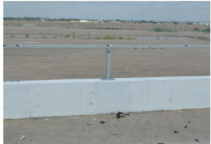
Figure 32. Back Side System Damage, Test No. IBBR-1
