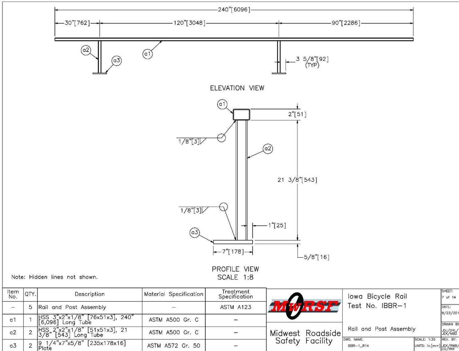
Figure 8. Rail and Post Assembly, Test No. IBBR-1
