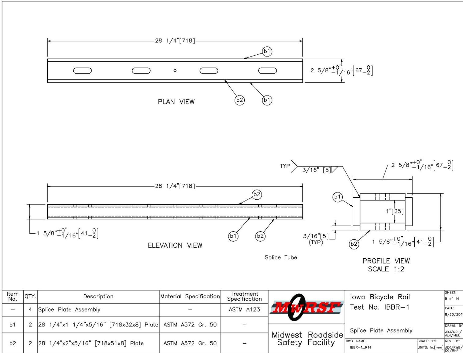
Figure 6. Splice Plate Assembly, Test No. IBBR-1
