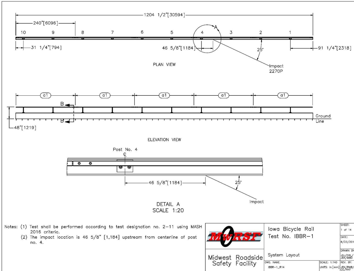
Figure 2. System Layout, Test No. IBBR-1
