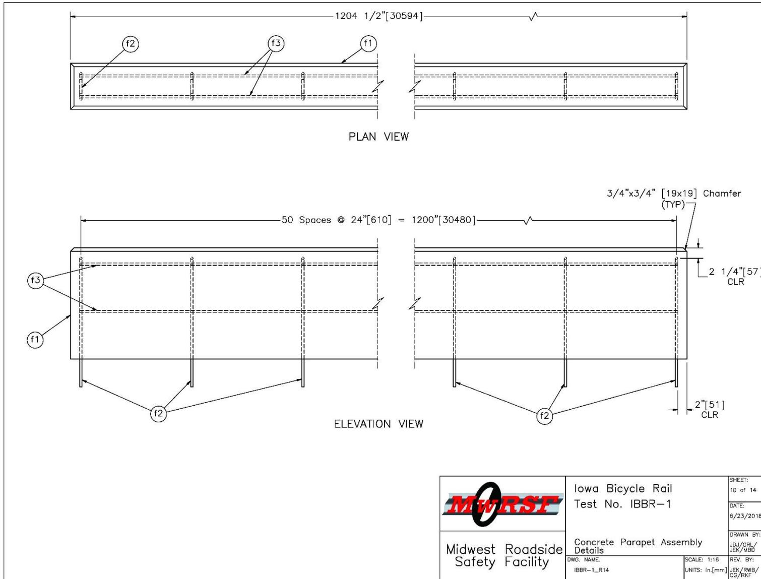
Figure 11. Concrete Parapet Assembly Details, Test No. IBBR-1
