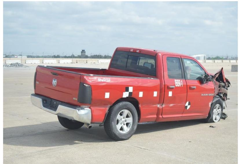
Figure 36. Vehicle Damage, Test No. IBBR-1
