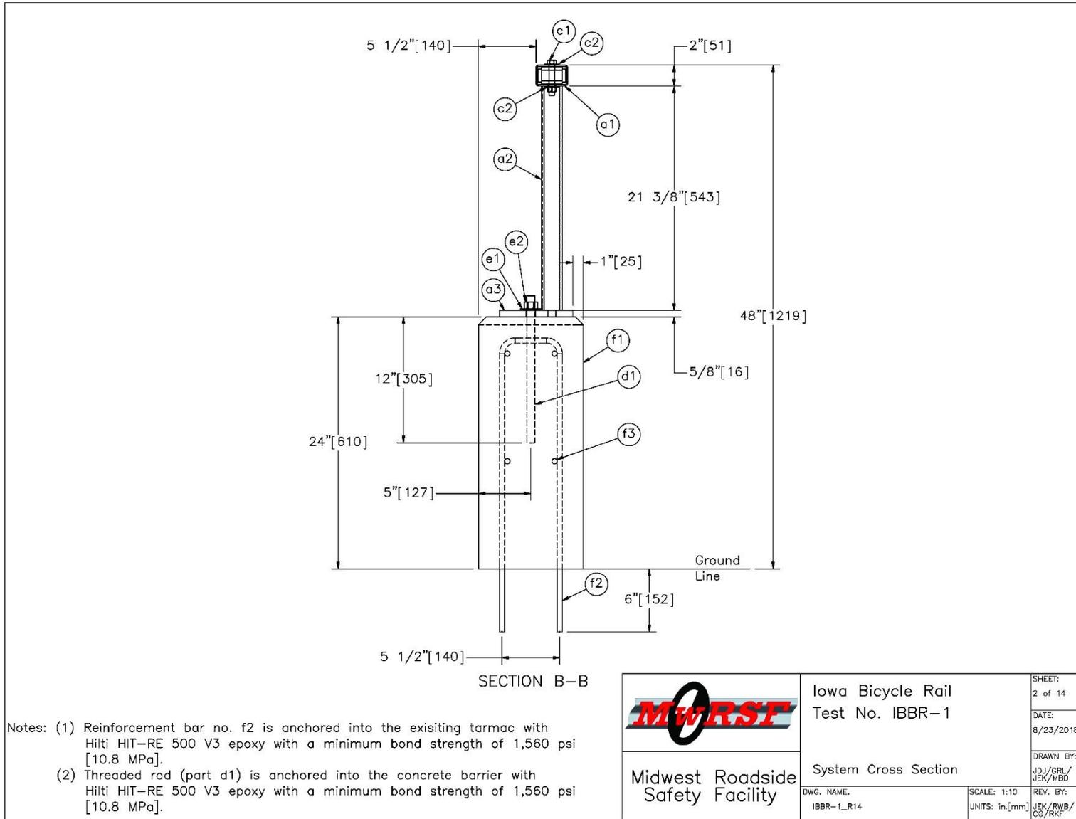
Figure 3. System Cross Section Layout, Test No. IBBR-1
