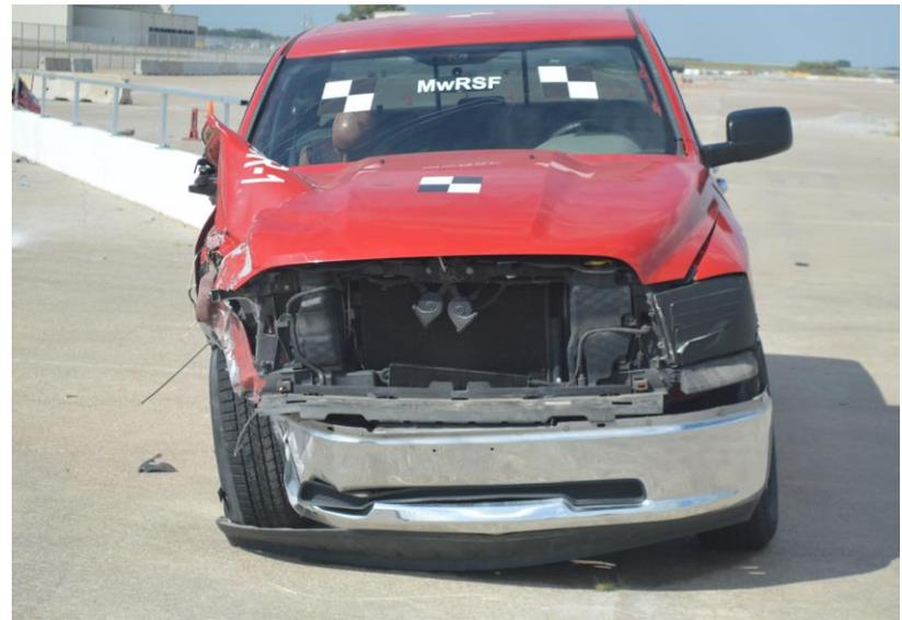
Figure 37. Vehicle Damage, Test No. IBBR-1
