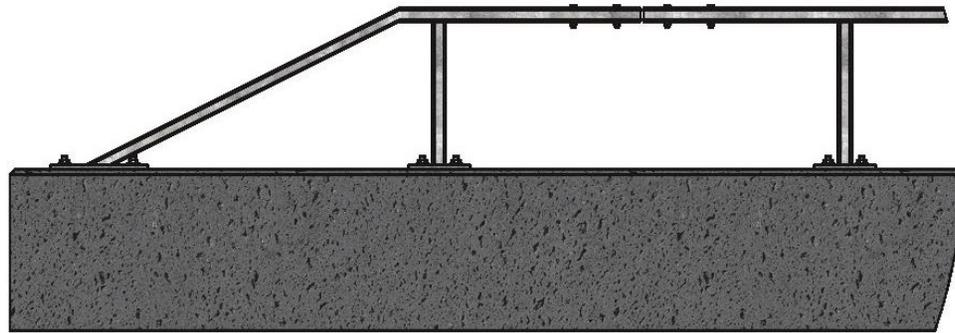
Partially Welded Tube End Termination – Near Side Splice Attachment
