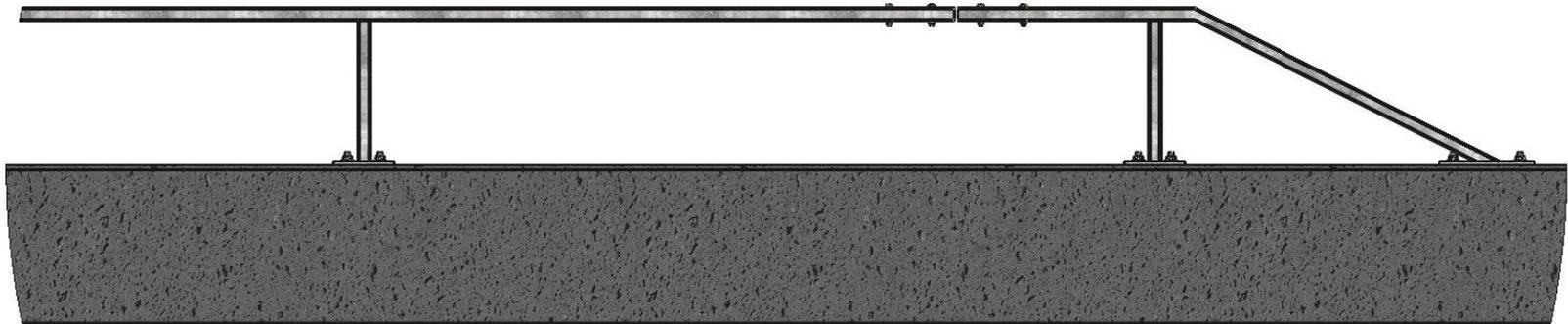
Partially Welded Tube End Termination – Far Side Splice Attachment
