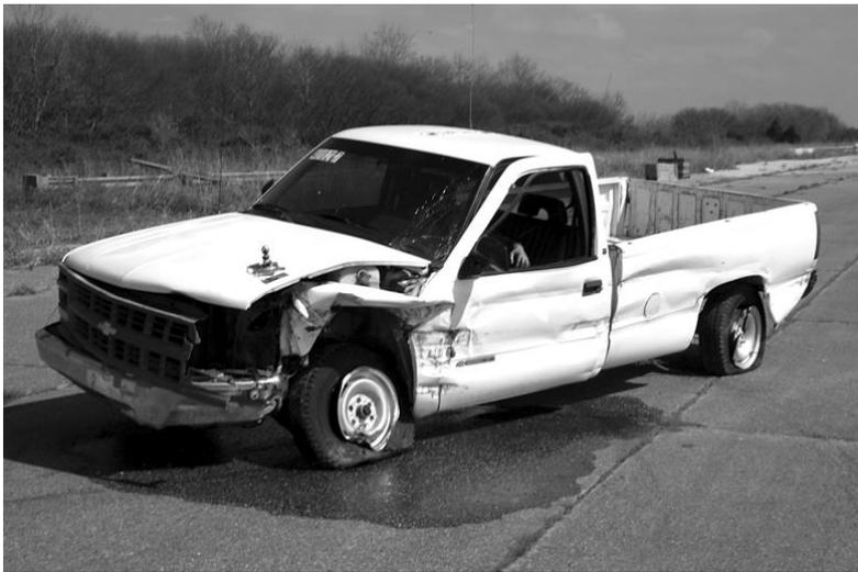
Figure 45. Tapered Tubular Rail Contact, Test No. 401021-7 [24]
