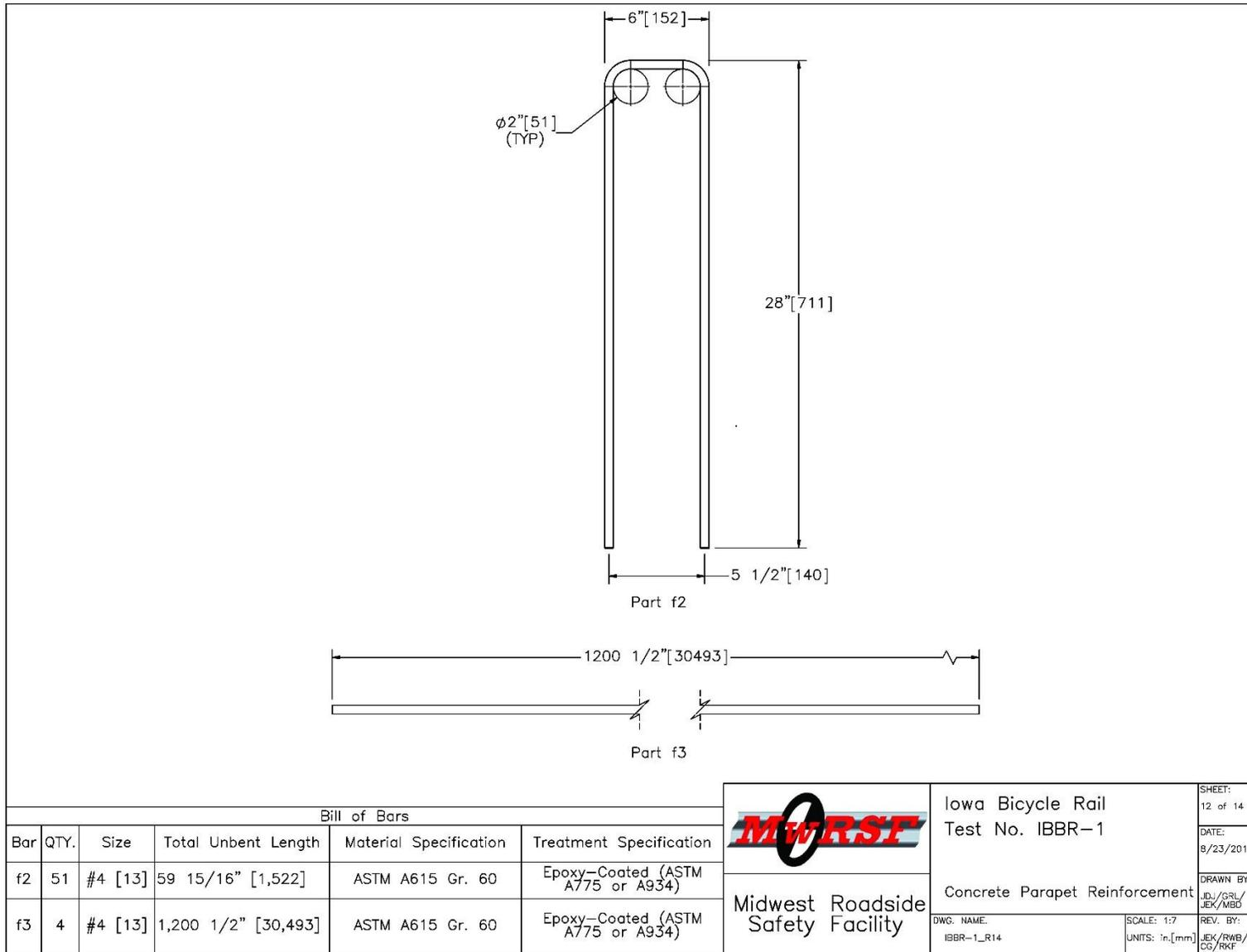
Figure 13. Concrete Parapet Reinforcement, Test No. IBBR-1
