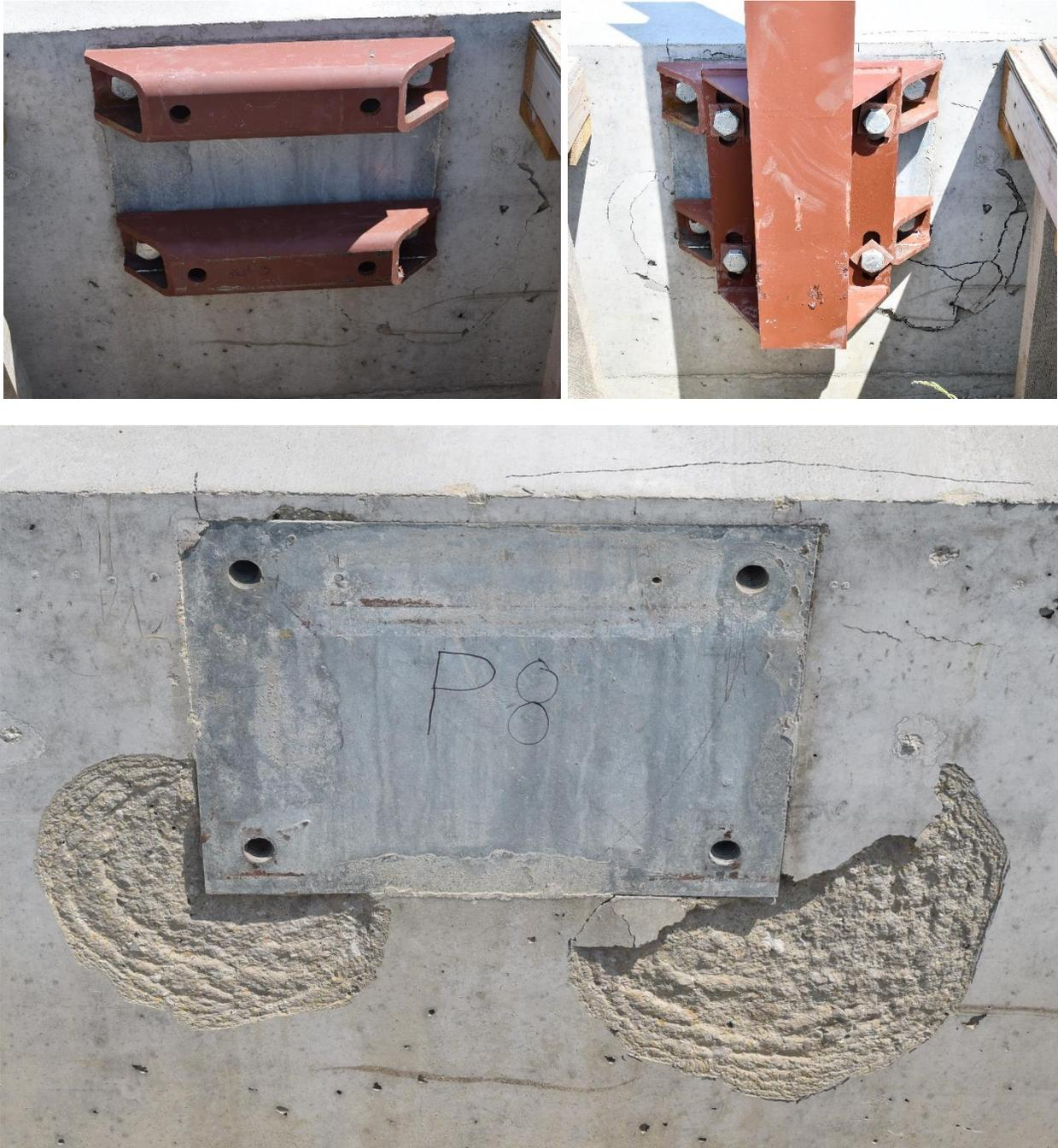
Figure 115. Pre- and Post-Test Sidewall Spalling, Test No. ILOH4-4
