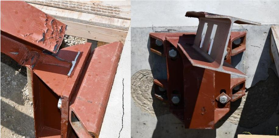
(b) Damage at End of Test
