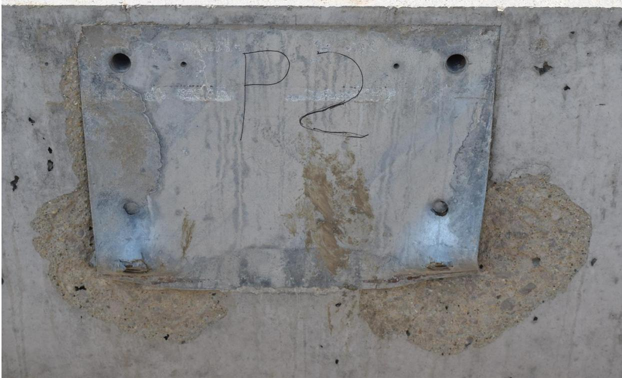
Figure 105. Post-Test Concrete Spalling for Test No. ILOH4-1
