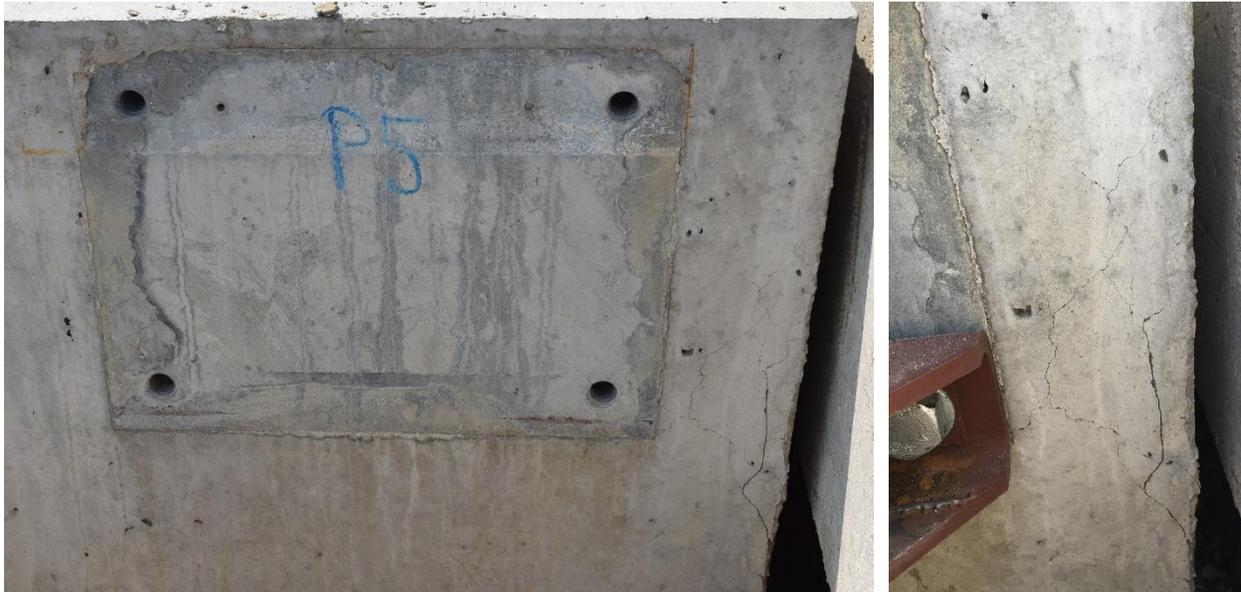
Figure 120. Post-Test Concrete Cracking from Test No. ILOH4-6
