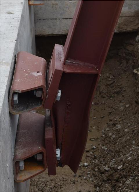
(b) Damage at End of Test
