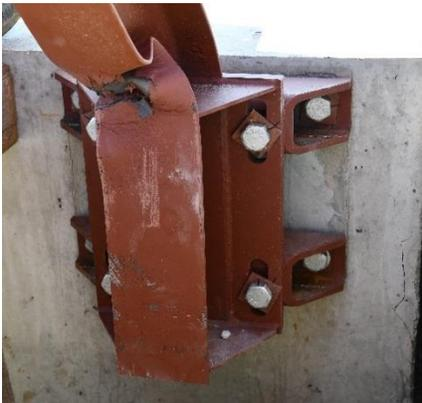
(b) Damage at End of Test
