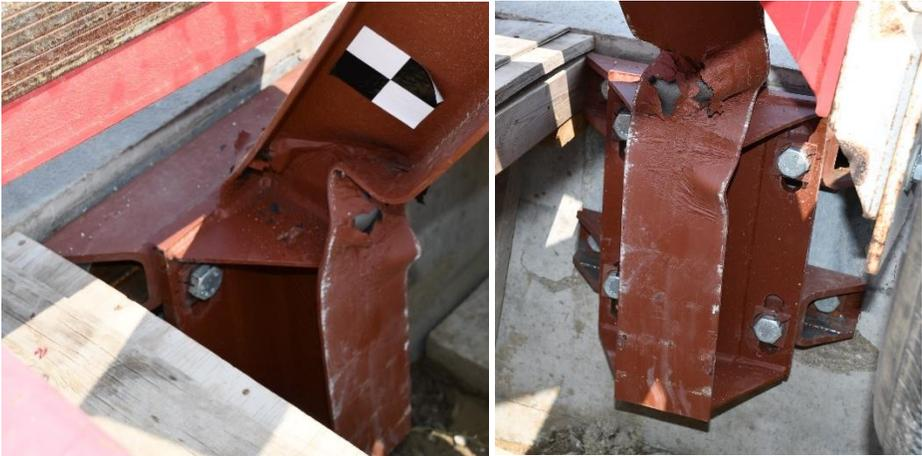
(b) Damage at End of Test
