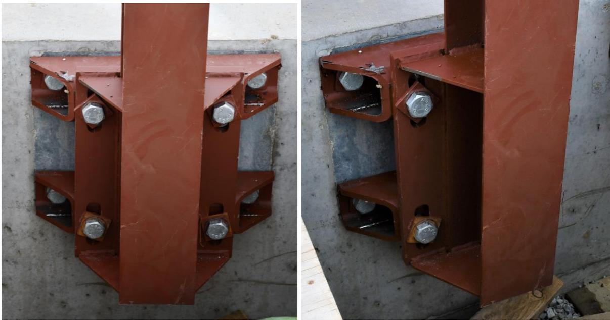
Figure 110. Singular Plate Attachment, Thicker Deck Spacers, and Gussets, Test No. ILOH4-3
