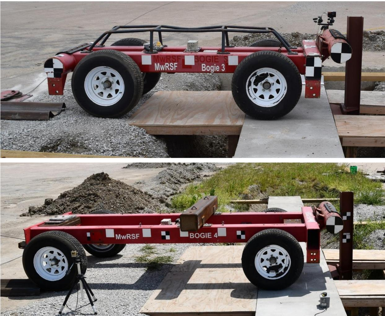
Figure 102. Rigid-Frame Bogie Vehicles
