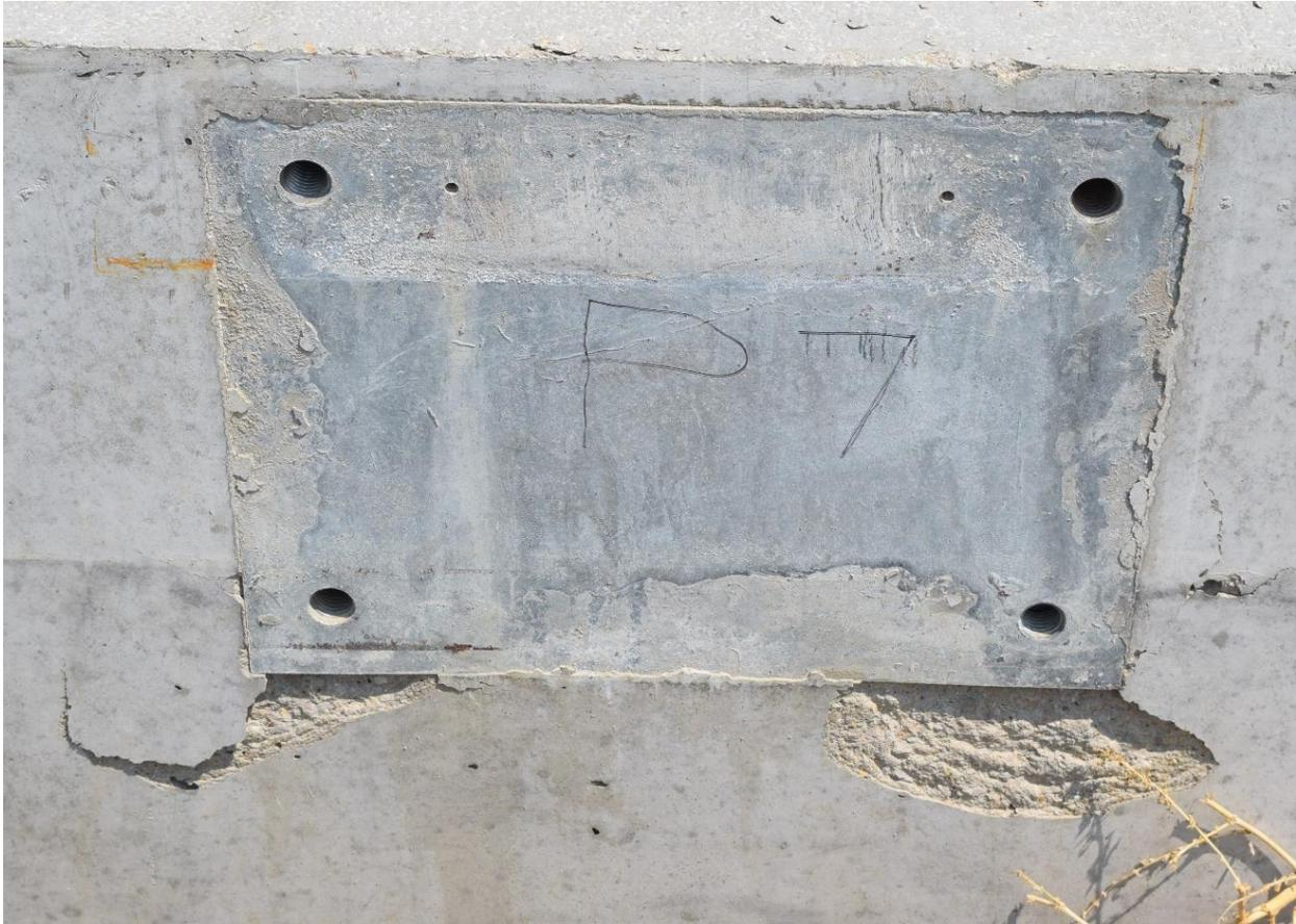
Figure 117. Post-test Concrete Spalling, Test No. ILOH4-5
