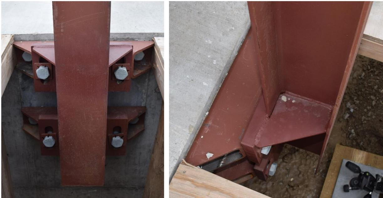
Figure 107. Added Tensile Gussets for Test No. ILOH4-2
