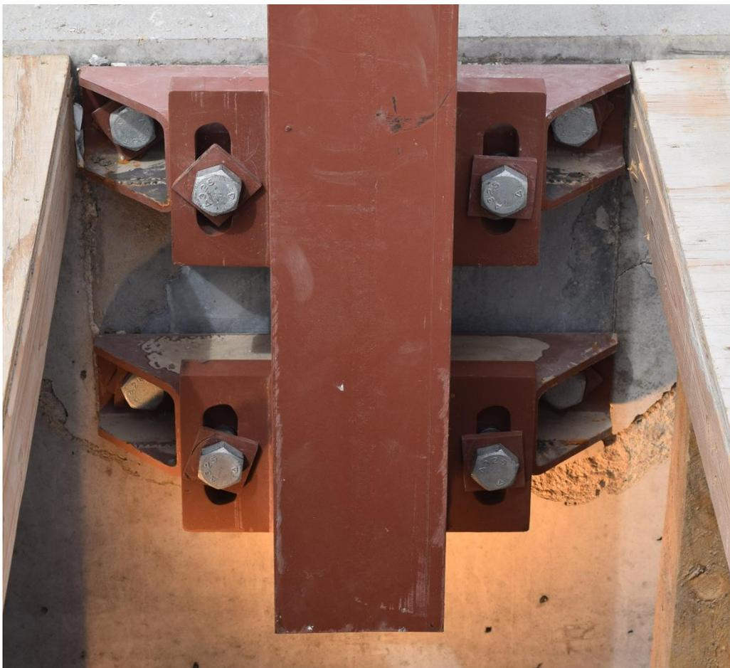
Figure 104. Pre-Test Concrete Spalling for Test No. ILOH4-1
