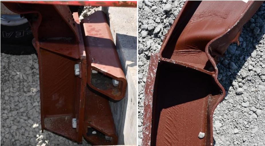
(b) Damage at End of Test
