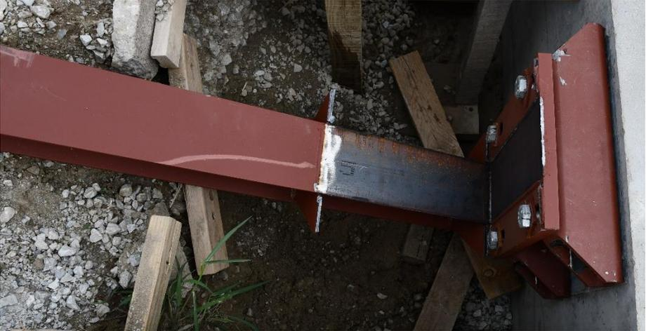
(b) Damage at End of Test
