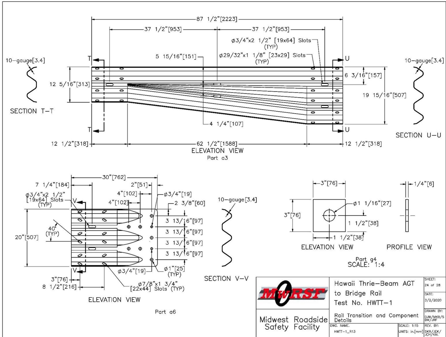
Figure 37. Asymmetric Transition Rail and Terminal Connector Details, Test Nos. HWTT-1 and HWTT-2
