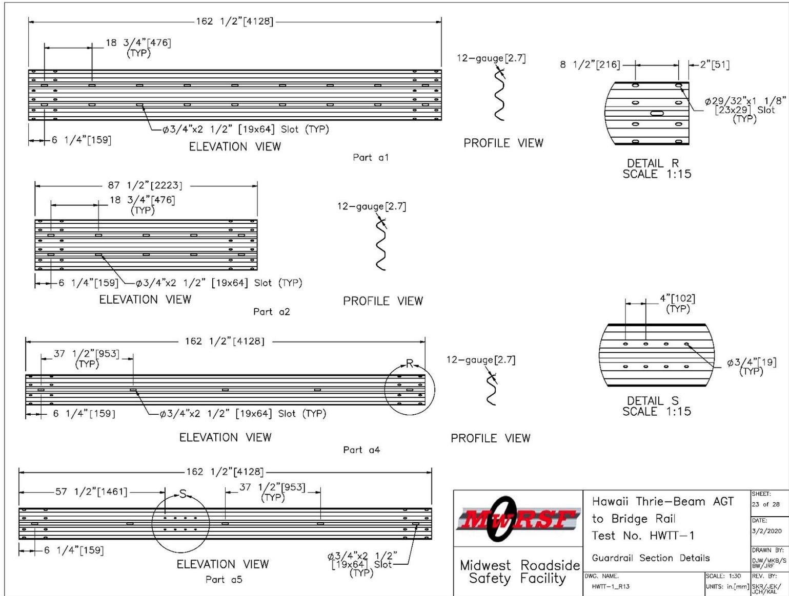
Figure 36. Guardrail Section Details, Test Nos. HWTT-1 and HWTT-2
