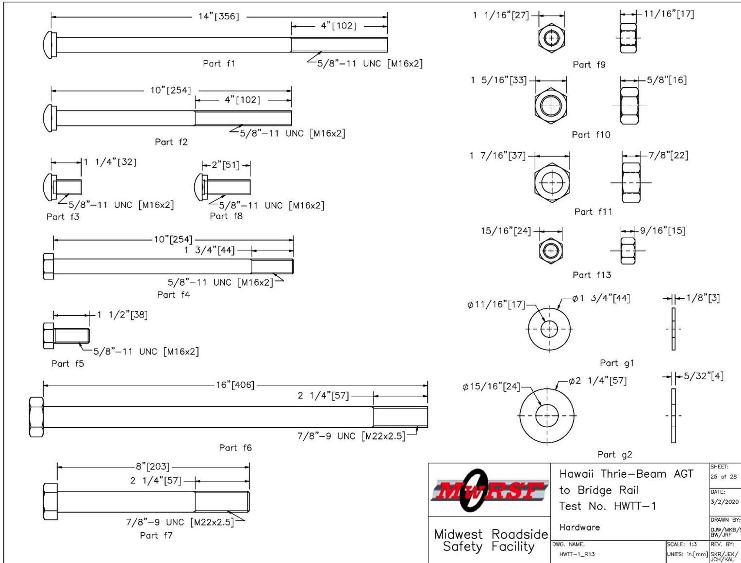
Figure 38. Hardware, Test Nos. HWTT-1 and HWTT-2
