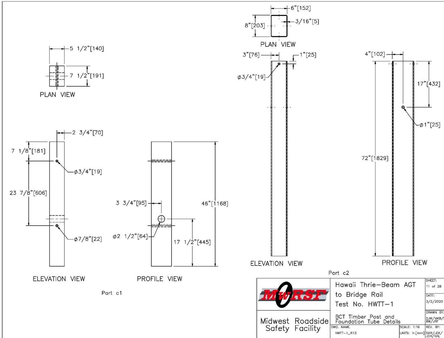
Figure 24. BCT Timber Post and Foundation Tube Details, Test Nos. HWTT-1 and HWTT-2
