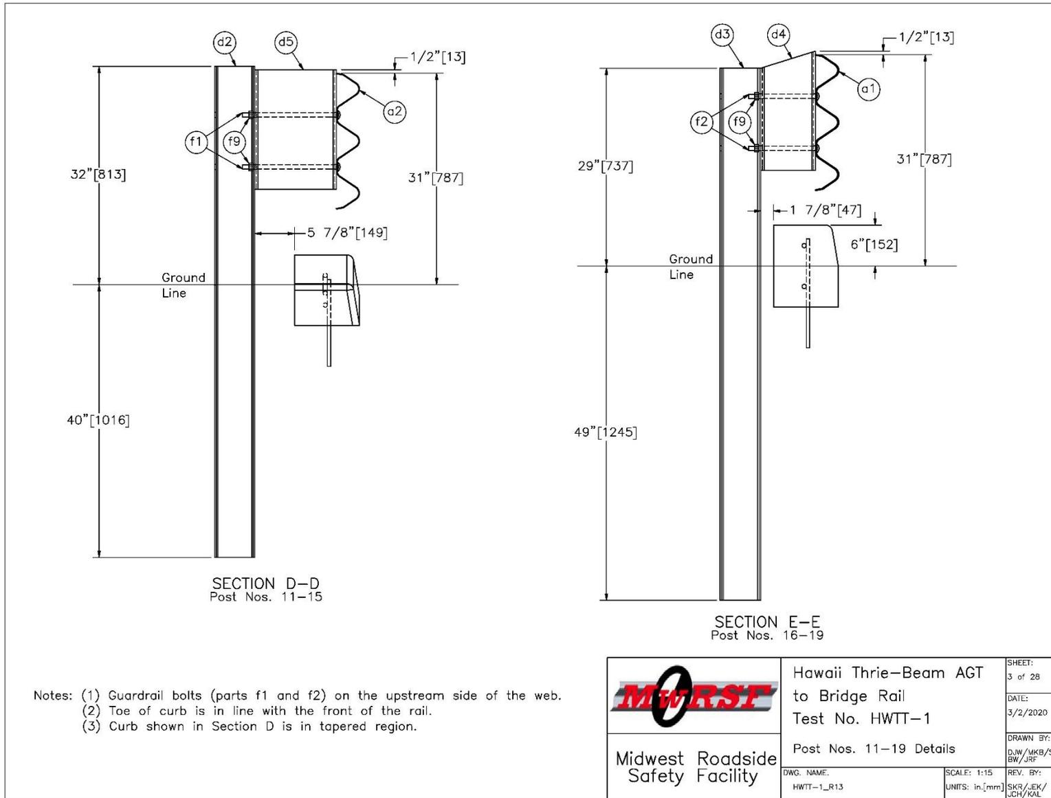
Figure 16. Post Nos. 11 through 19 Details, Test Nos. HWTT-1 and HWTT-2
