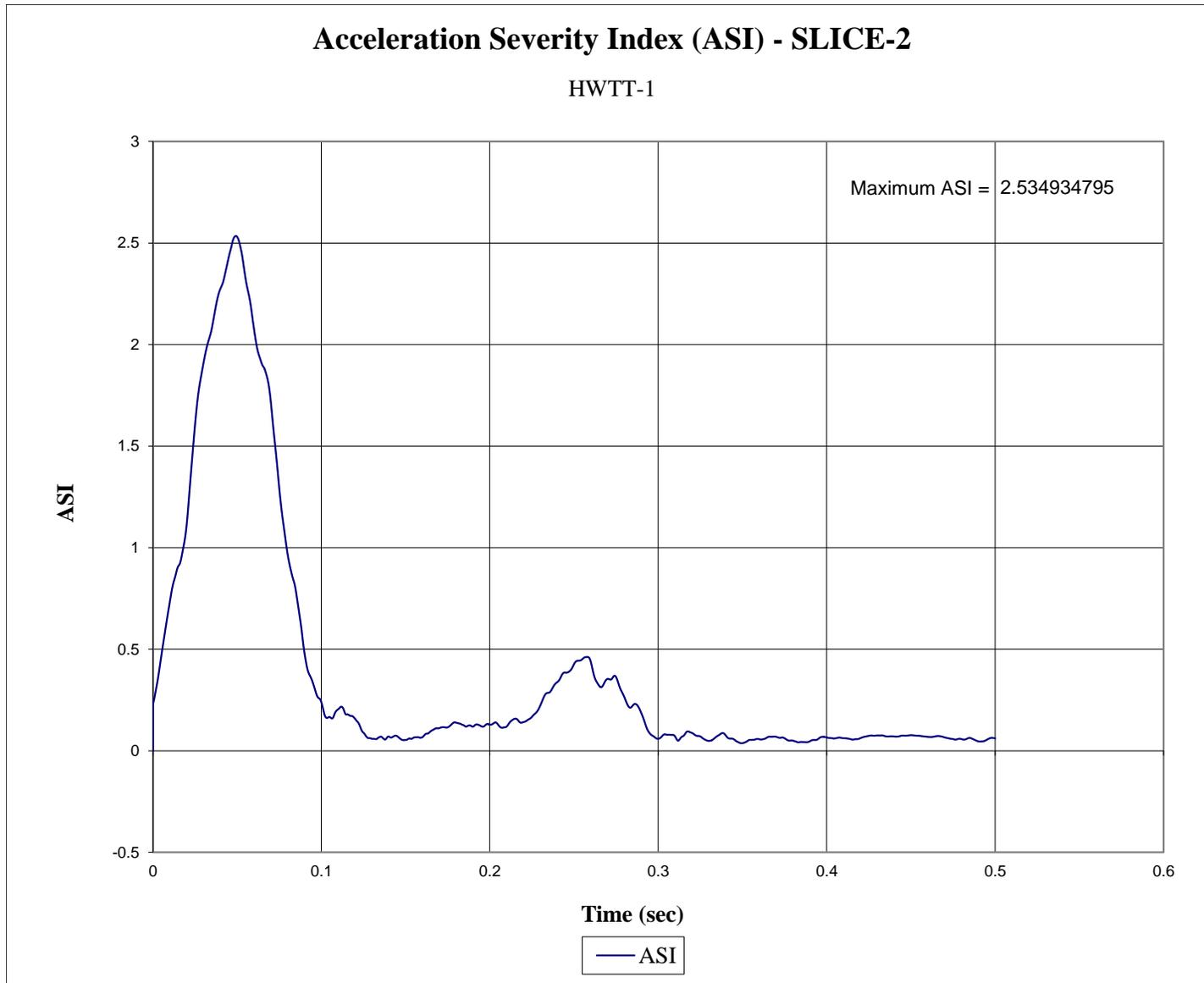
Figure E-16. Acceleration Severity Index (SLICE-2), Test No. HWTT-1
