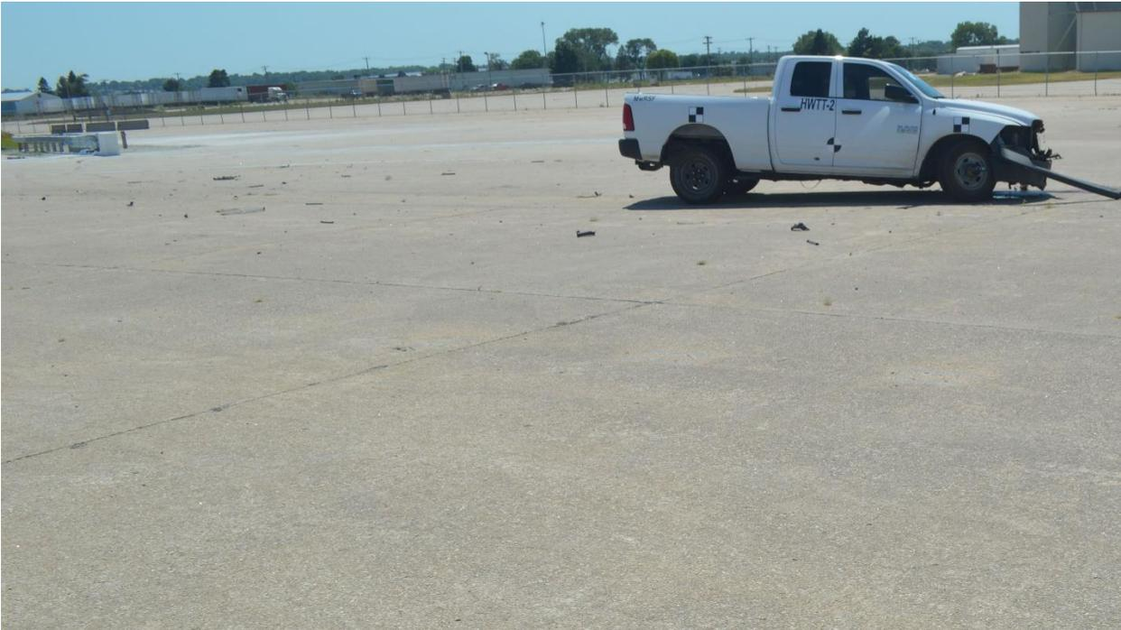
Figure 72. Vehicle Final Position and Trajectory Marks, Test No. HWTT-2
