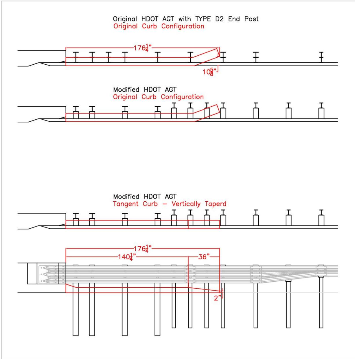
Figure 12. Modified HDOT AGT with Inclusion of MGS Upstream Stiffness Transition
