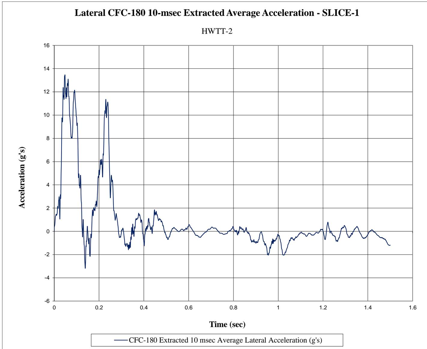
Figure F-12. 10-ms Average Lateral Deceleration (SLICE-1), Test No. HWTT-2
