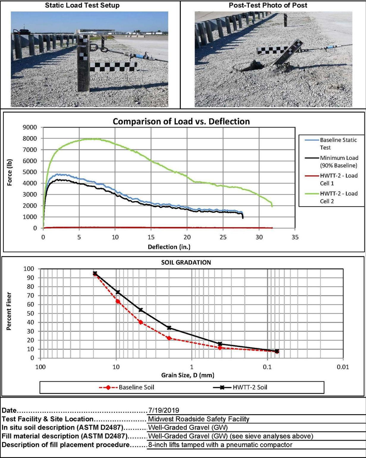
Figure C-4. Static Soil Test, Test No. HWTT-2
