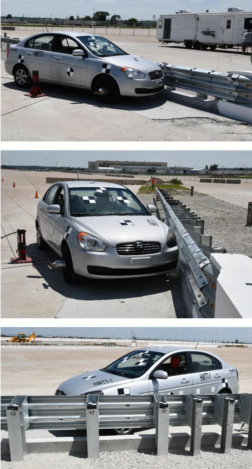
Figure 55. Impact Location, Test No. HWTT-1
