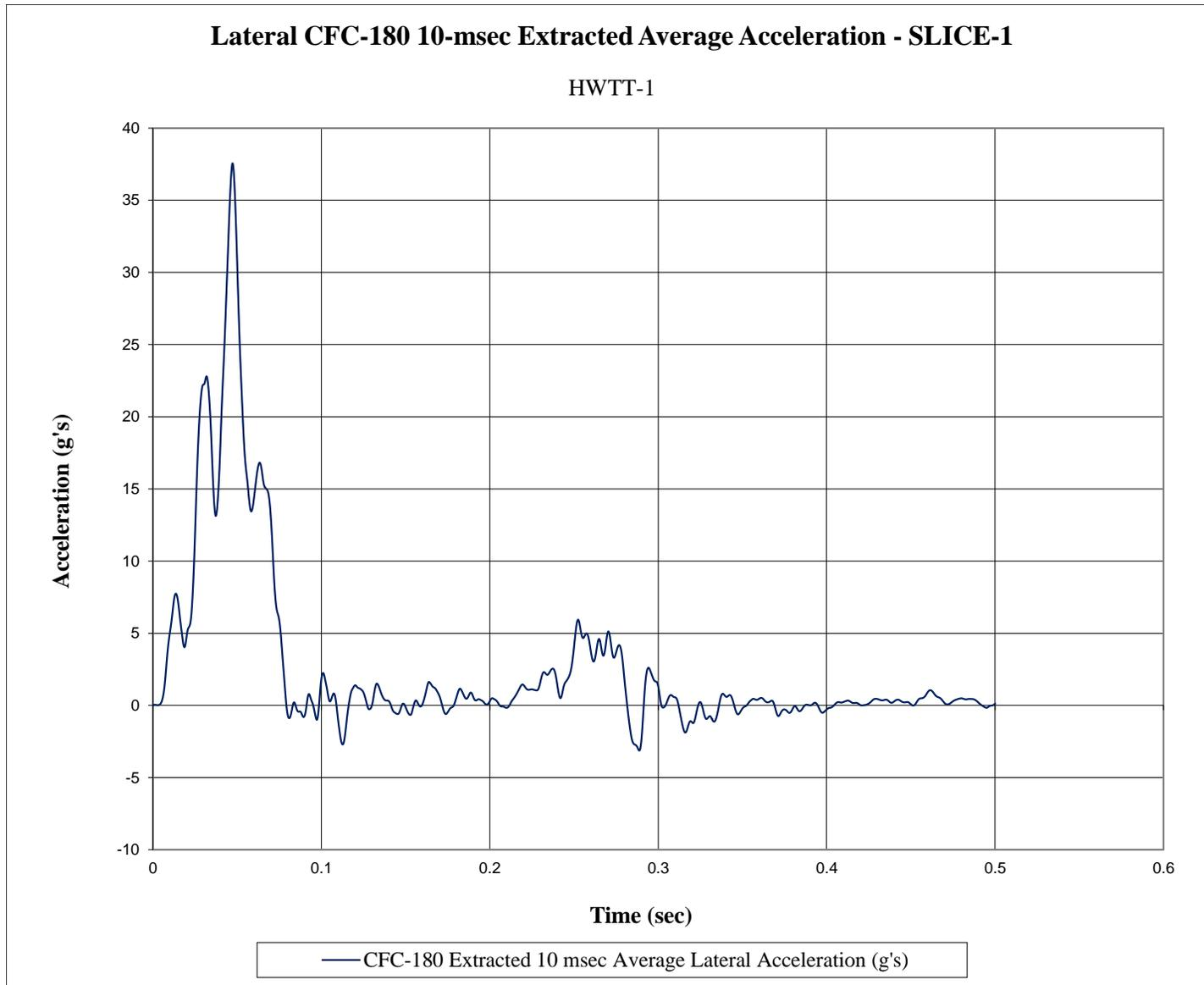
Figure E-4. 10-ms Average Lateral Deceleration (SLICE-1), Test No. HWTT-1
