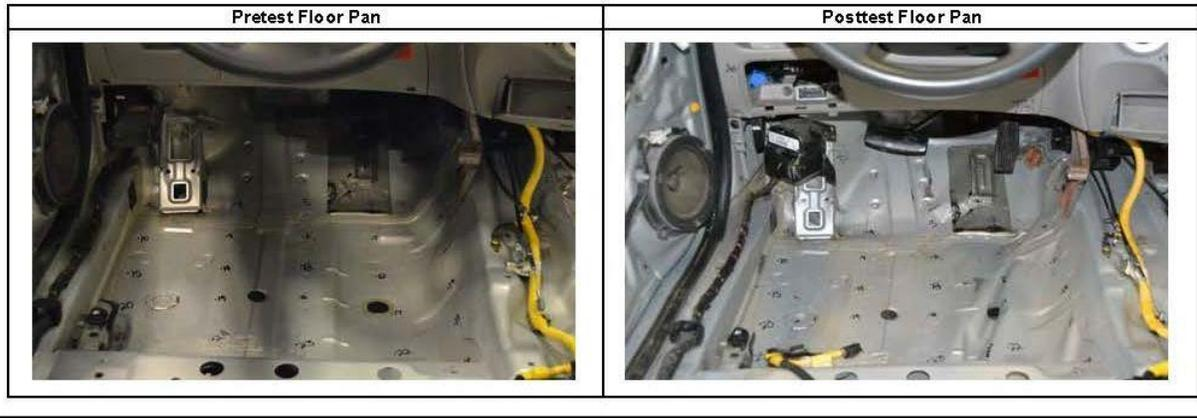
Figure D-1. Floor Pan Deformation Data – Set 1, Test No. HWTT-1
