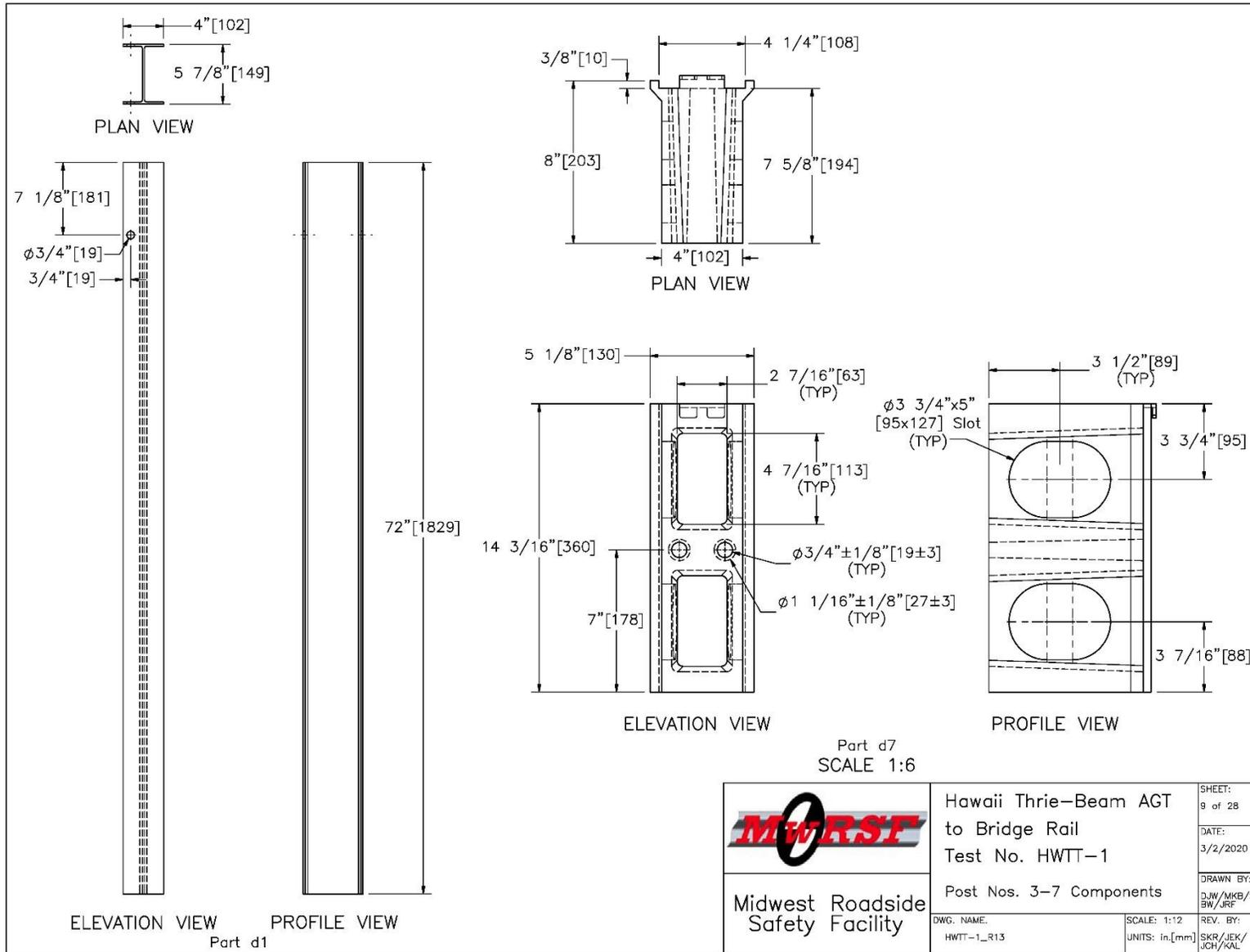
Figure 22. Post Nos. 3 through 7 Components, Test Nos. HWTT-1 and HWTT-2
