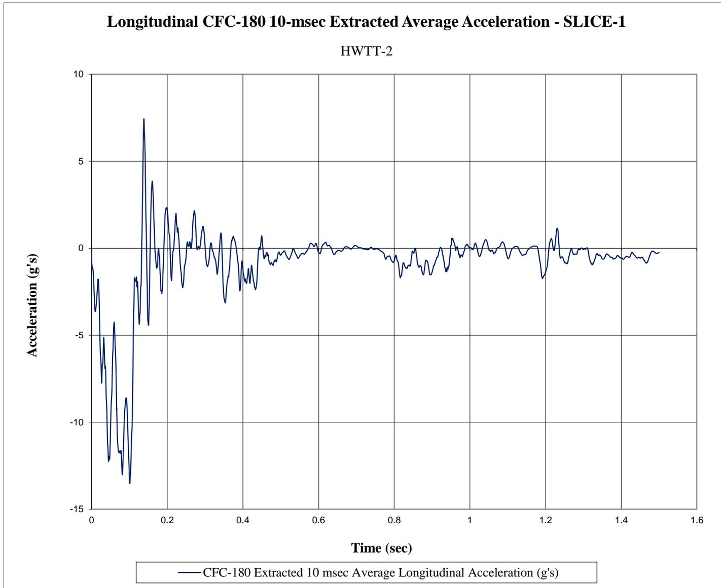
Figure F-9. 10-ms Average Longitudinal Deceleration (SLICE-1), Test No. HWTT-2
