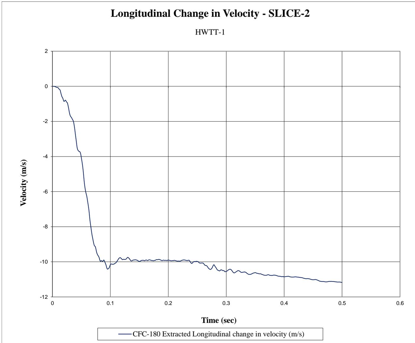
Figure E-10. Longitudinal Occupant Impact Velocity (SLICE-2), Test No. HWTT-1
