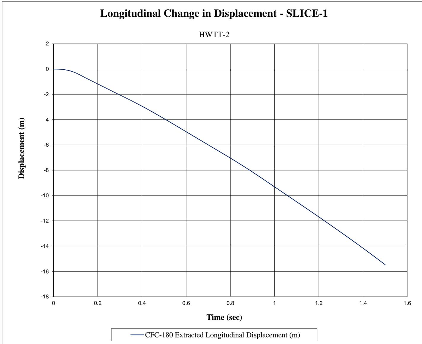
Figure F-11. Longitudinal Occupant Displacement (SLICE-1), Test No. HWTT-2
