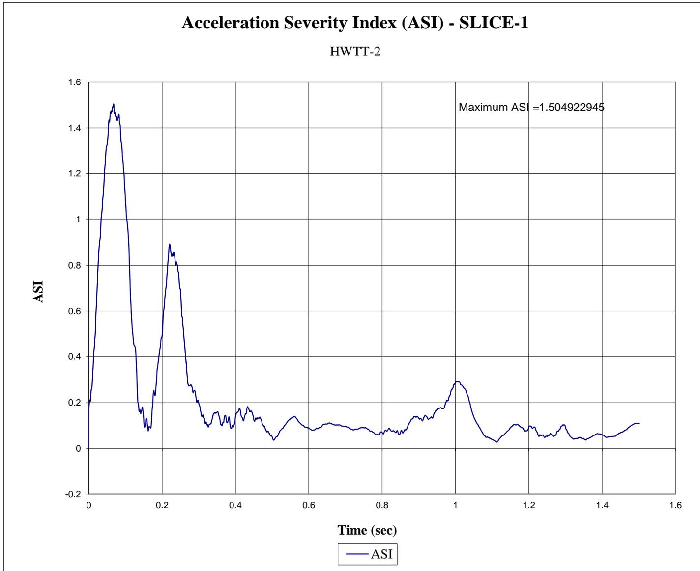
Figure F-16. Acceleration Severity Index (SLICE-1), Test No. HWTT-2
