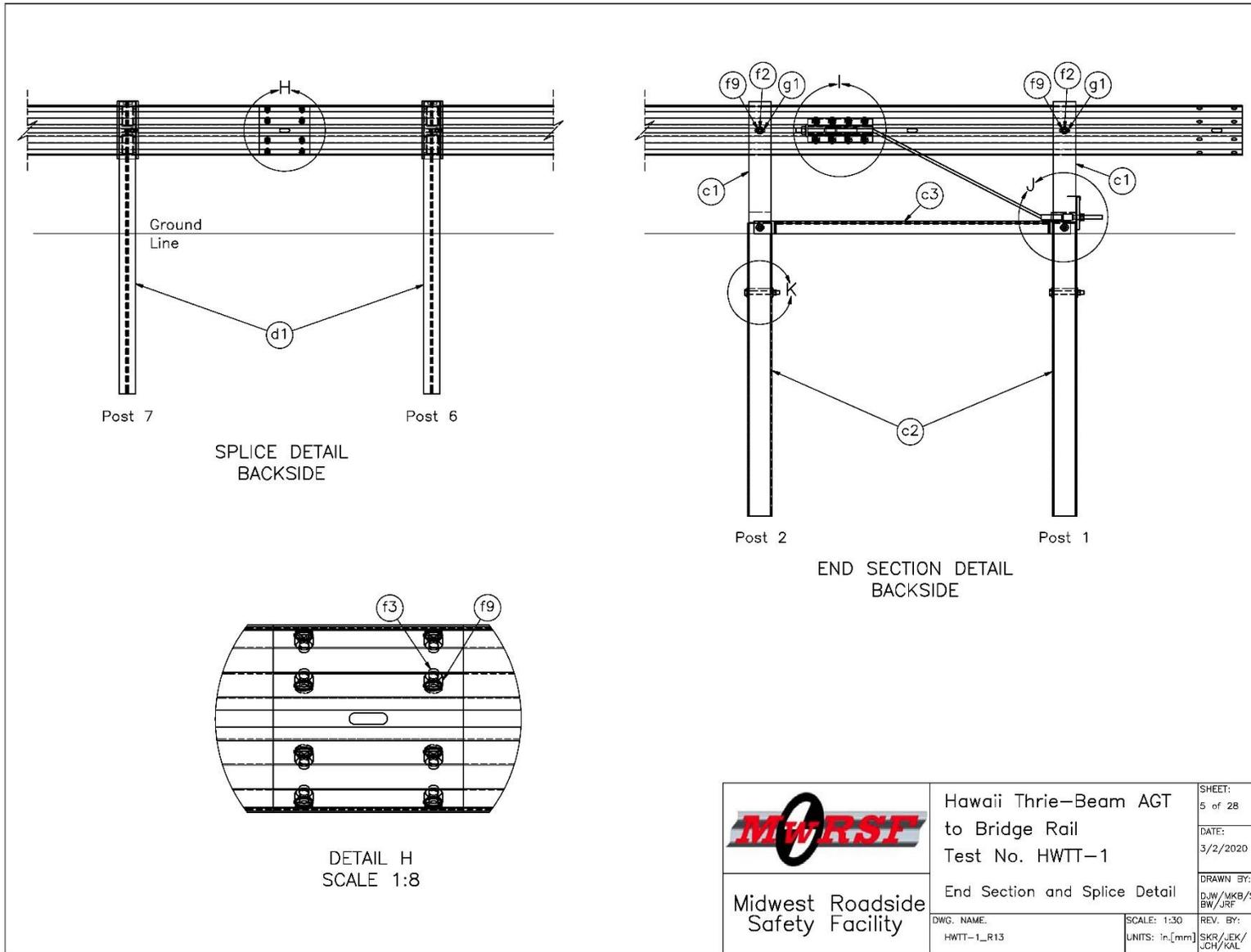
Figure 18. Guardrail End Section and Splice Detail, Test Nos. HWTT-1 and HWTT-2
