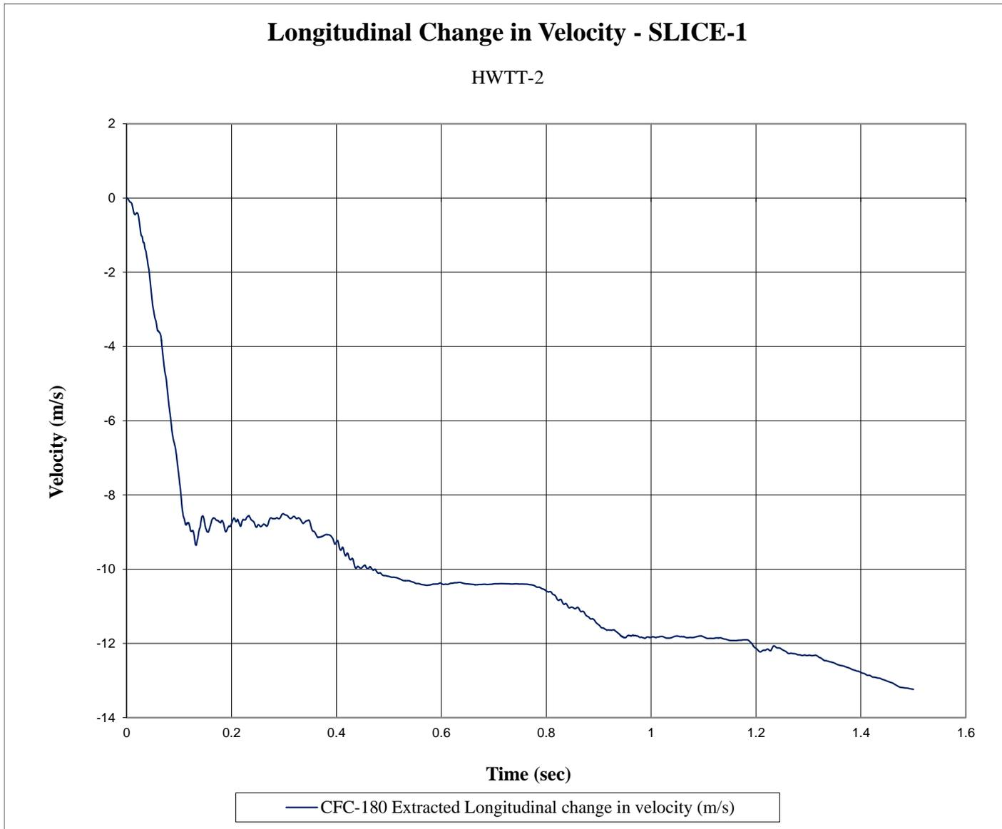
Figure F-10. Longitudinal Occupant Impact Velocity (SLICE-1), Test No. HWTT-2
