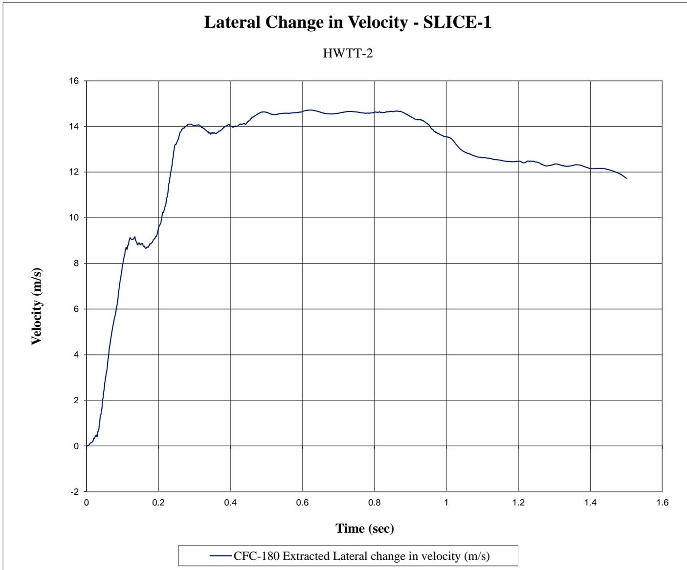
Figure F-13. Lateral Occupant Impact Velocity (SLICE-1), Test No. HWTT-2
