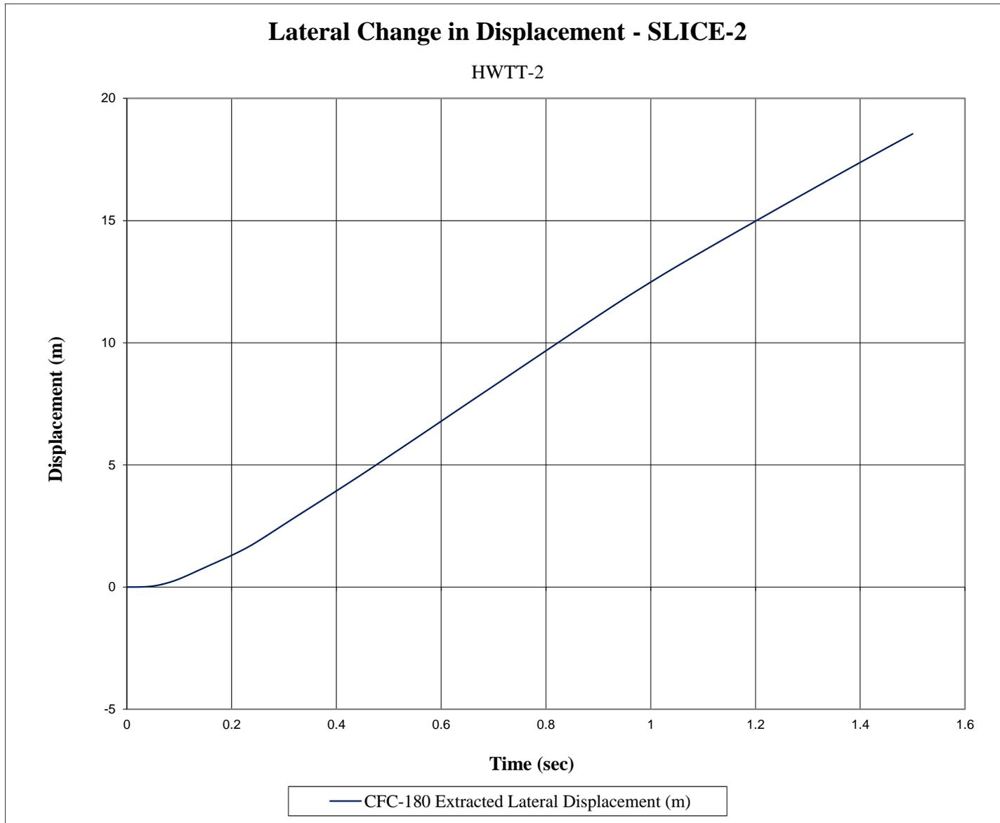
Figure F-6. Lateral Occupant Displacement (SLICE-2), Test No. HWTT-2
