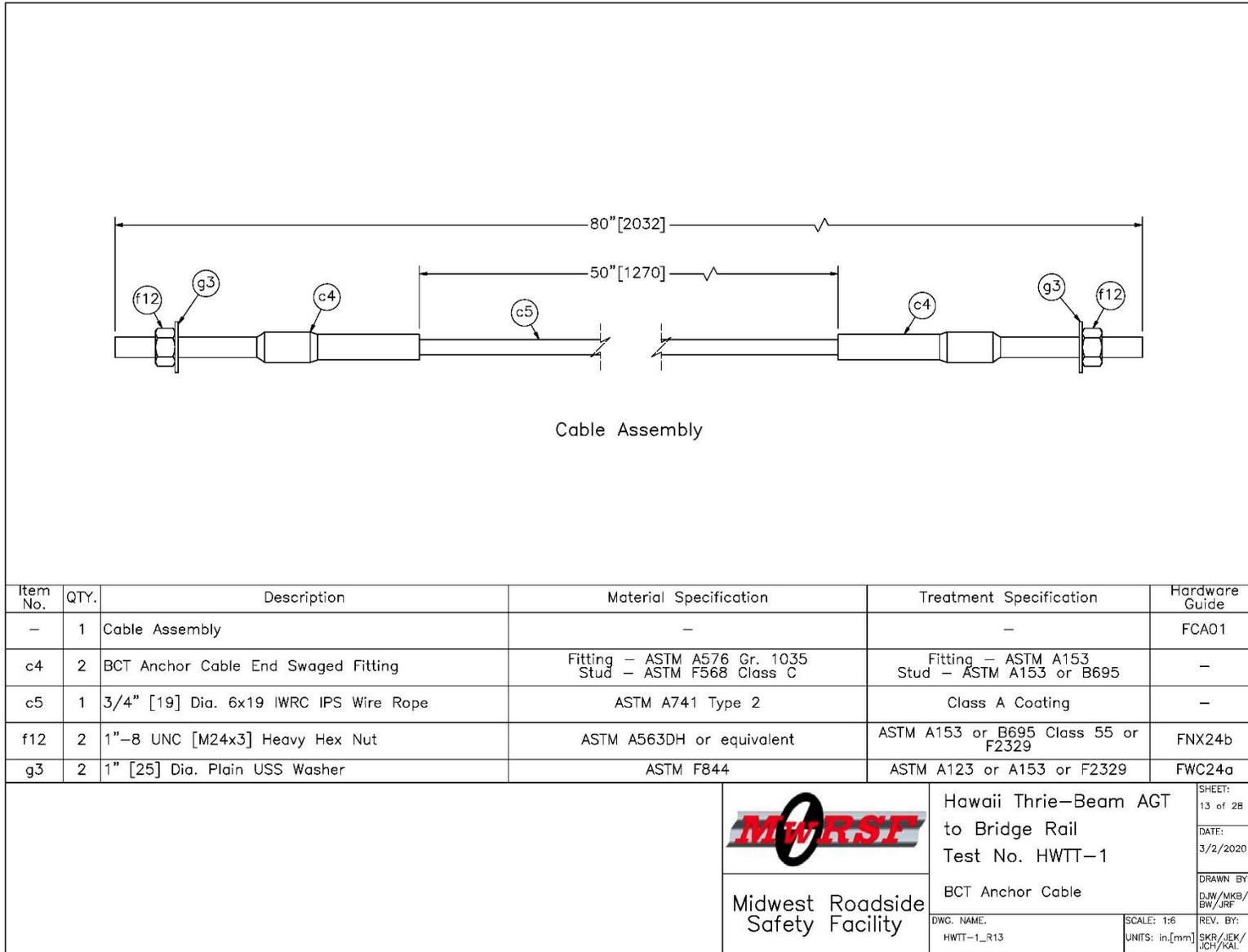
Figure 26. BCT Anchor Cable Details, Test Nos. HWTT-1 and HWTT-2
