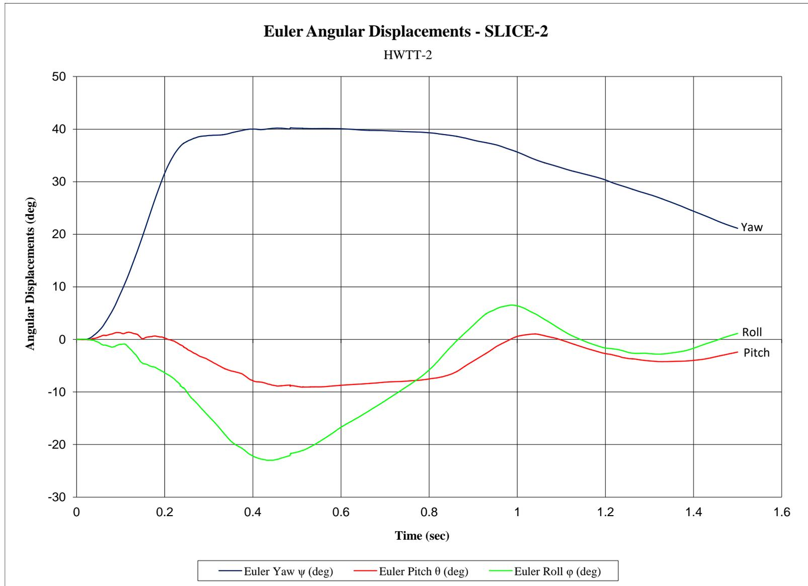
Figure F-7. Vehicle Angular Displacements (SLICE-2), Test No. HWTT-2
