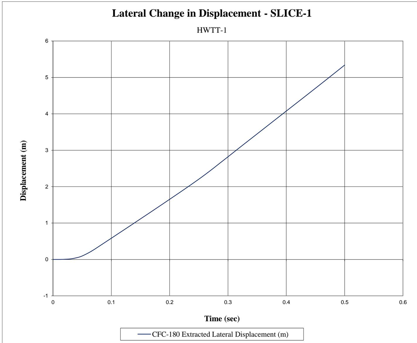
Figure E-6. Lateral Occupant Displacement (SLICE-1), Test No. HWTT-1
