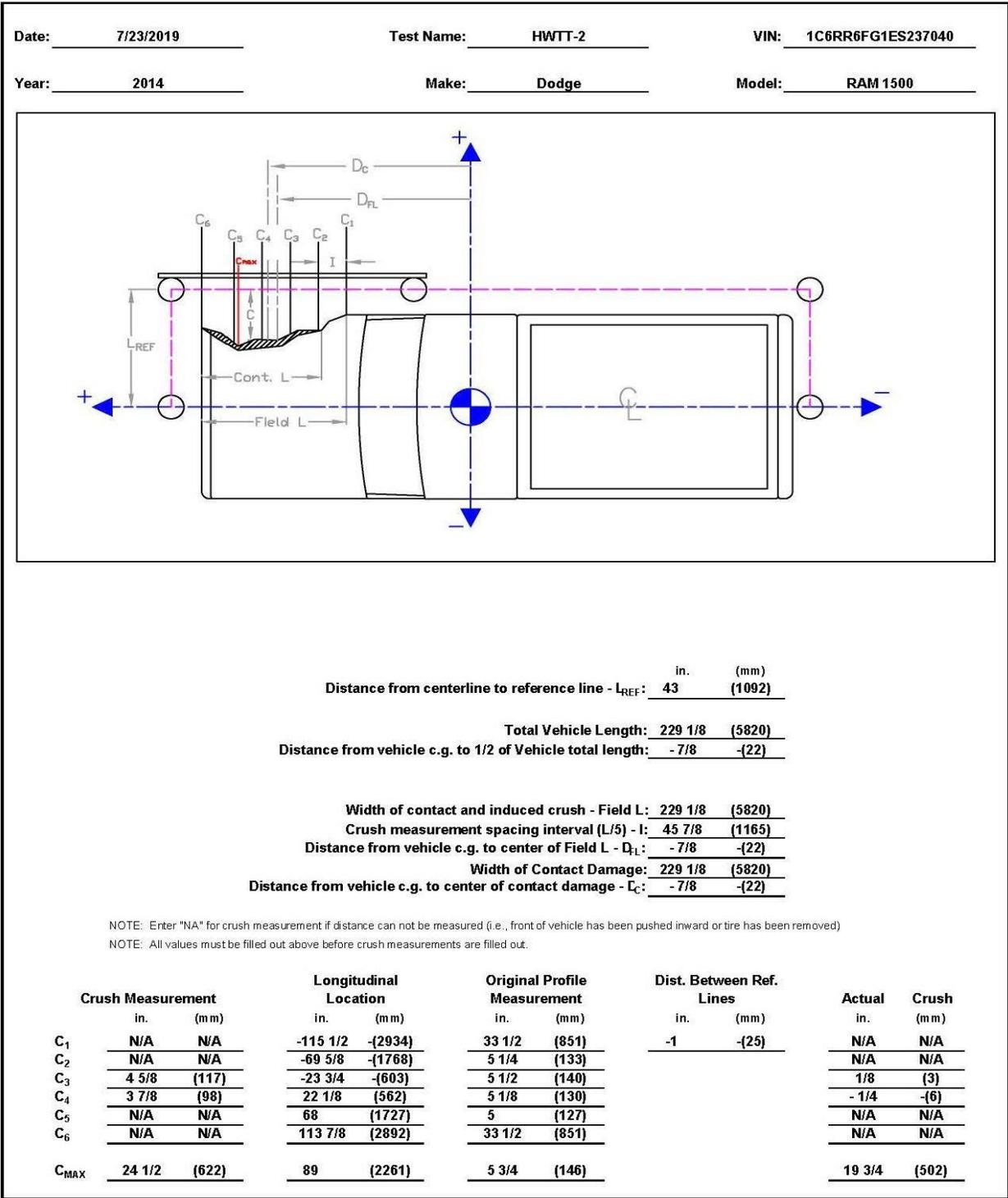
Figure D-13. Exterior Vehicle Crush (NASS) - Side, Test No. HWTT-2
