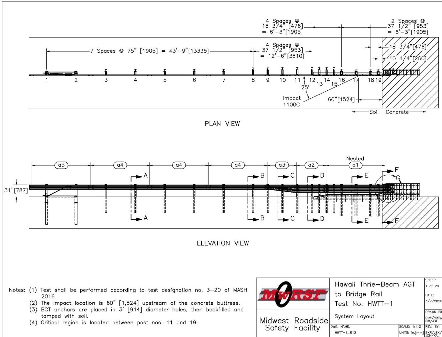
Figure 13. System Layout, Test No. HWTT-1
