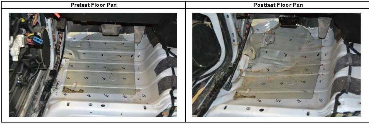
Figure D-7. Floor Pan Deformation Data – Set 1, Test No. HWTT-2
