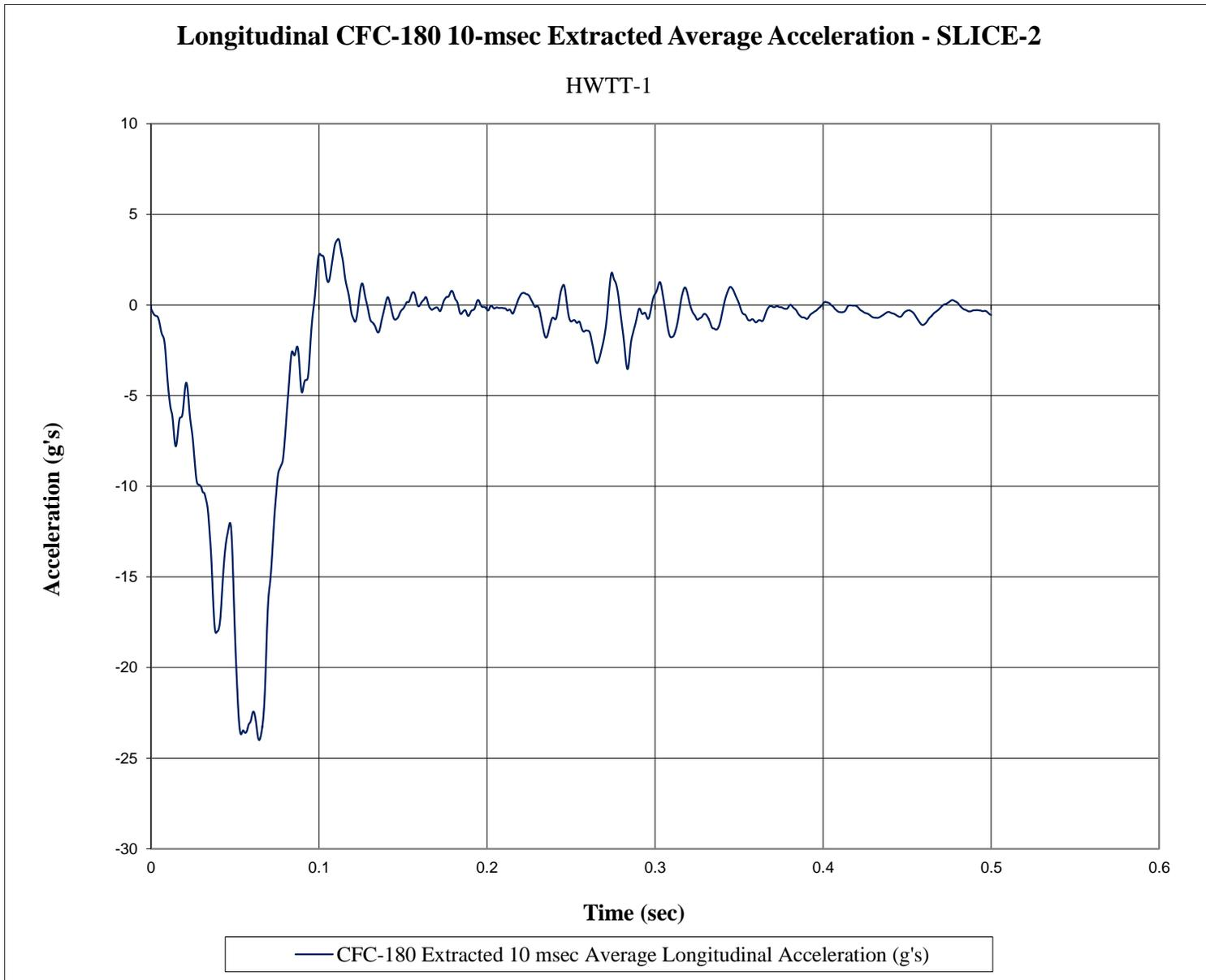
Figure E-9. 10-ms Average Longitudinal Deceleration (SLICE-2), Test No. HWTT-1
