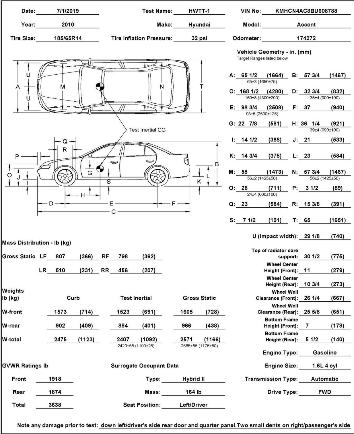
Figure 47. Vehicle Dimensions, Test No. HWTT-1
