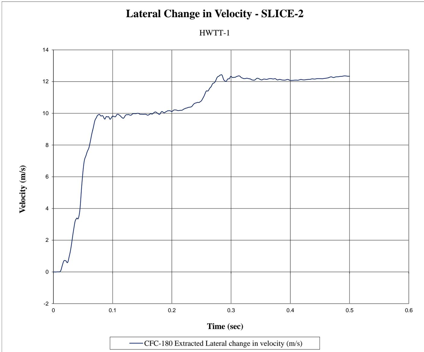
Figure E-13. Lateral Occupant Impact Velocity (SLICE-2), Test No. HWTT-1
