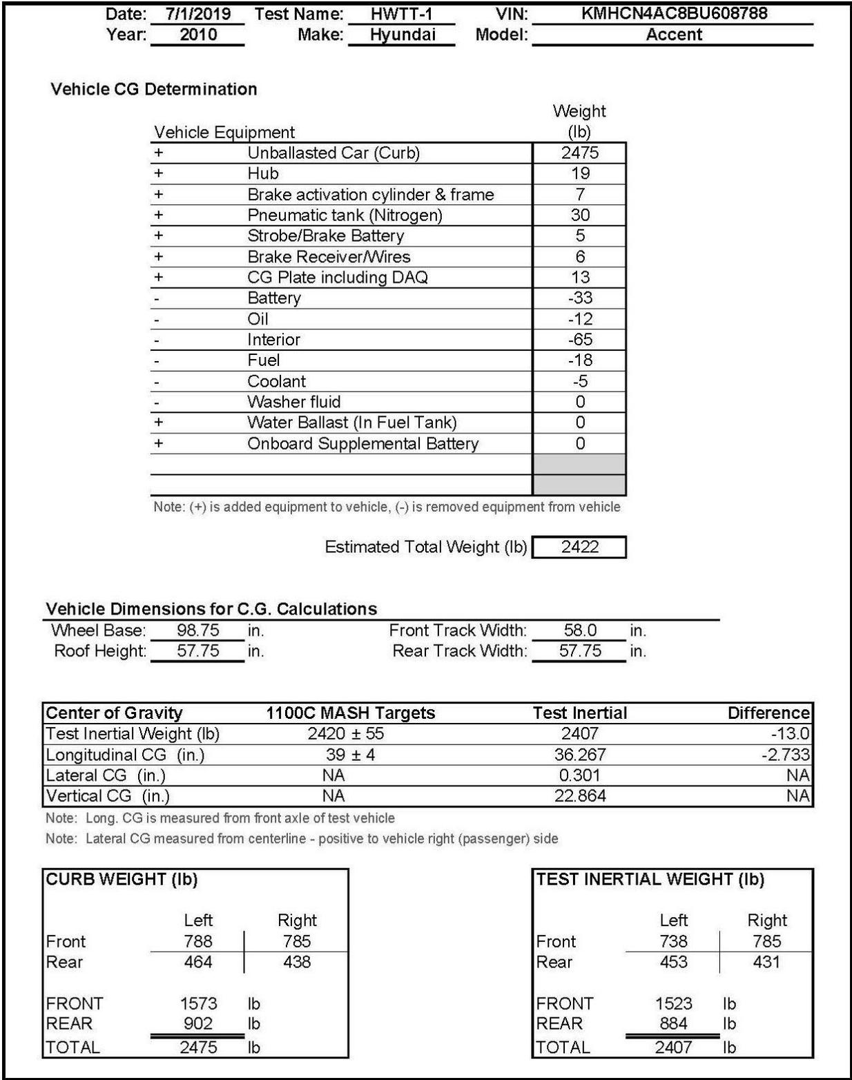
Figure B-1. Vehicle Mass Distribution, Test No. HWTT-1
