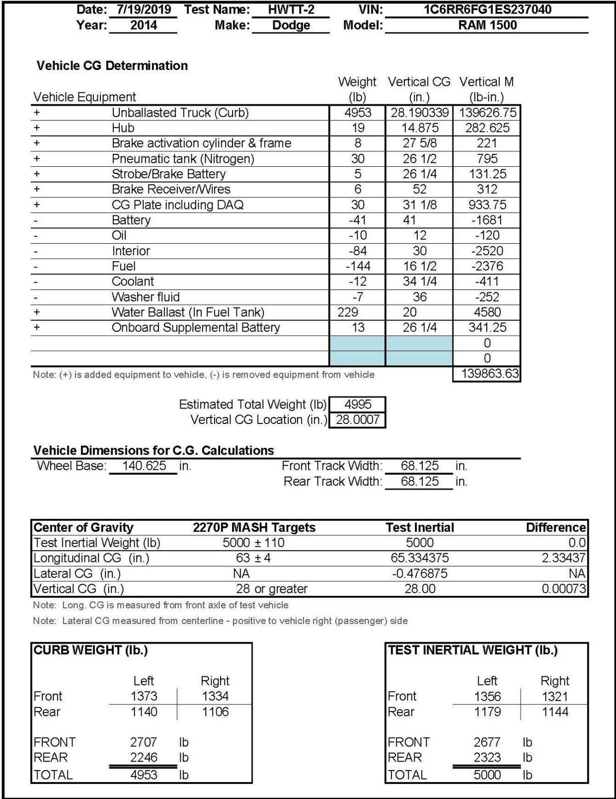
Figure B-2. Vehicle Mass Distribution, Test No. HWTT-2
