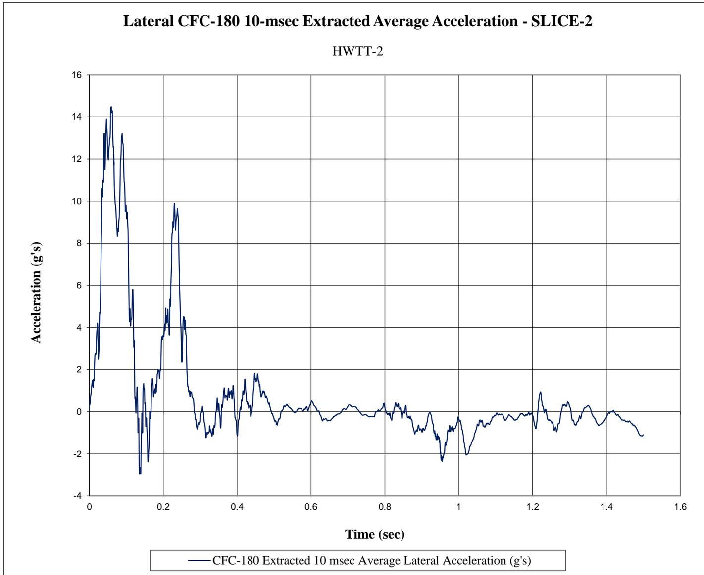
Figure F-4. 10-ms Average Lateral Deceleration (SLICE-2), Test No. HWTT-2
