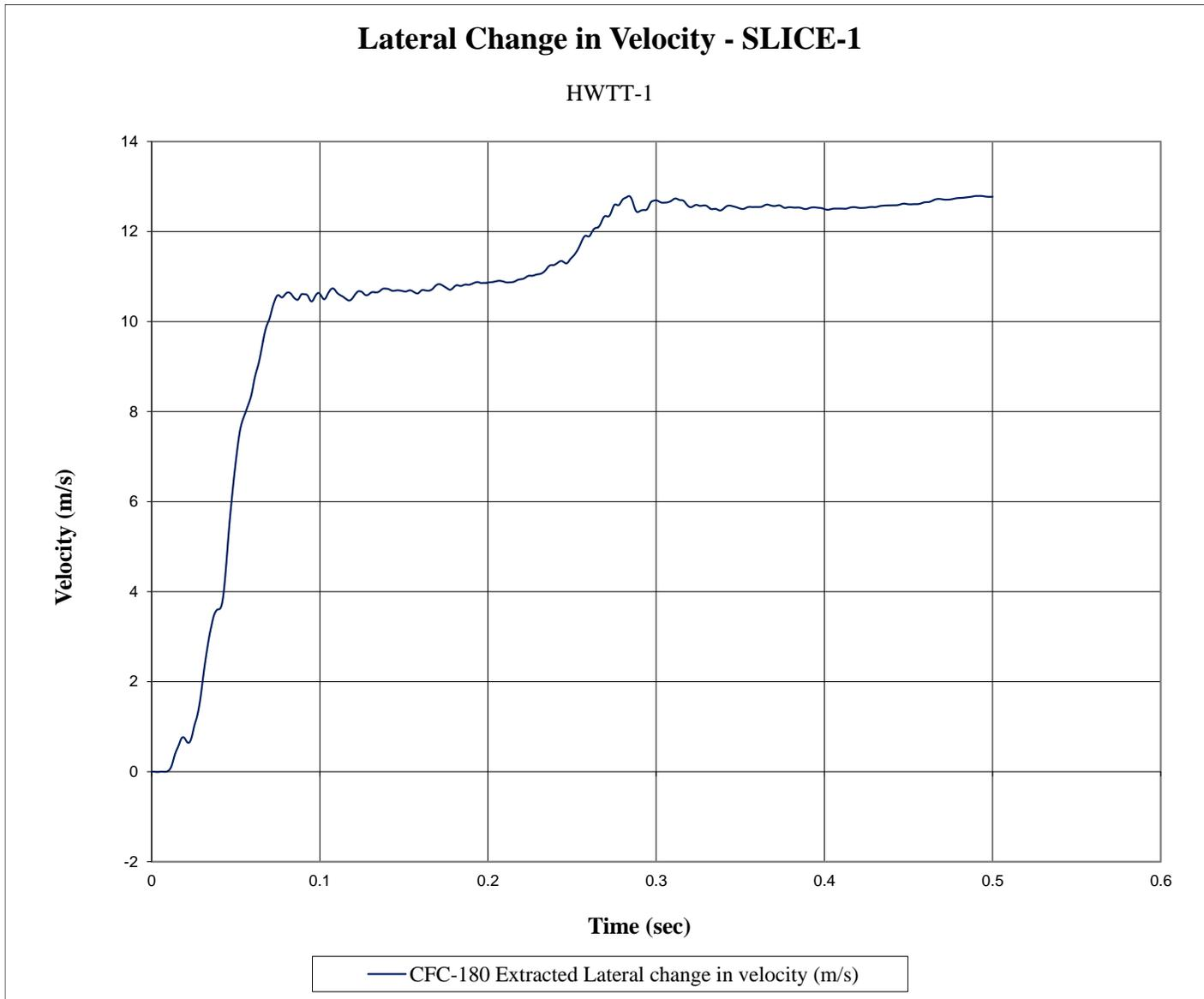
Figure E-5. Lateral Occupant Impact Velocity (SLICE-1), Test No. HWTT-1
