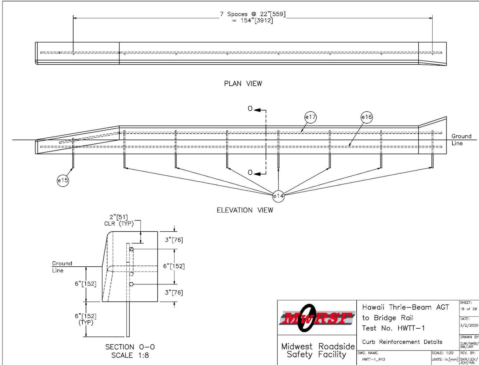
Figure 31. Curb Reinforcement Details, Test Nos. HWTT-1 and HWTT-2
