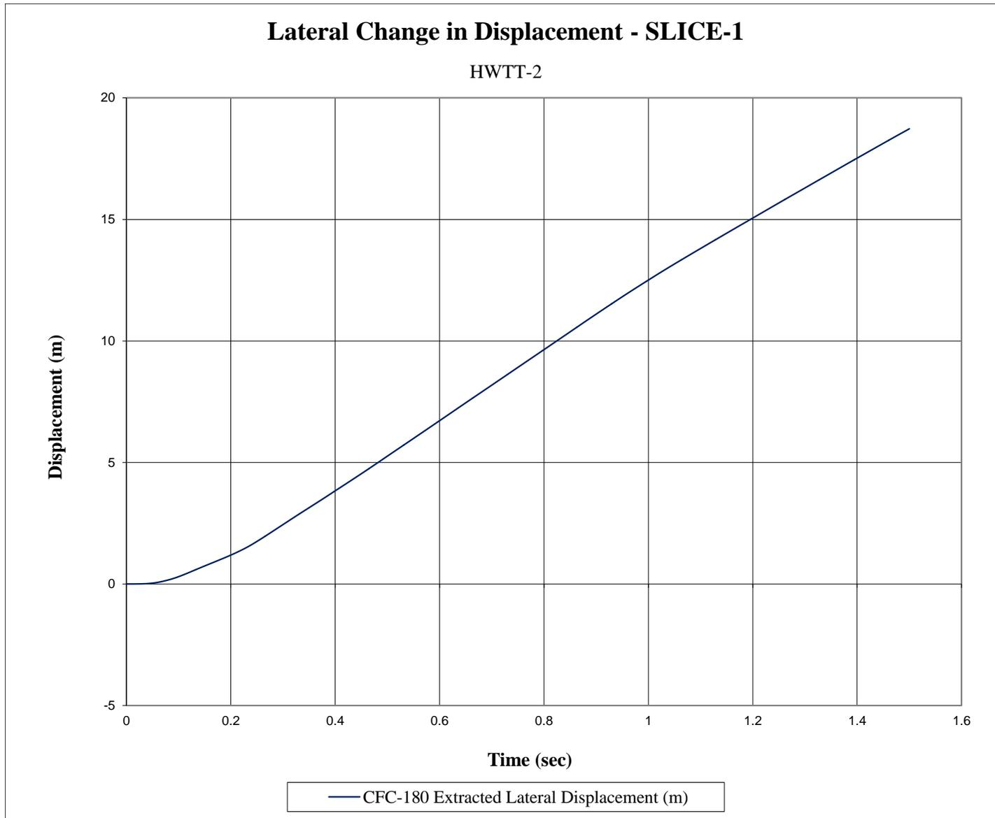
Figure F-14. Lateral Occupant Displacement (SLICE-1), Test No. HWTT-2
