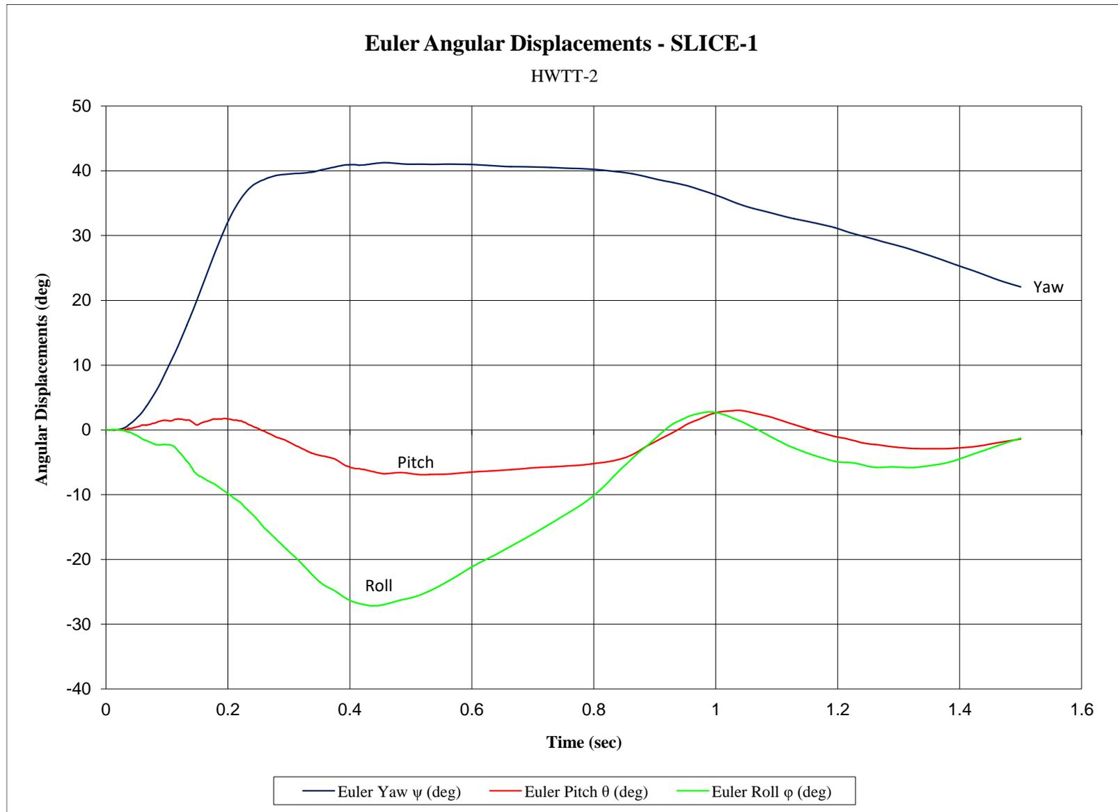
Figure F-15. Vehicle Angular Displacements (SLICE-1), Test No. HWTT-2
