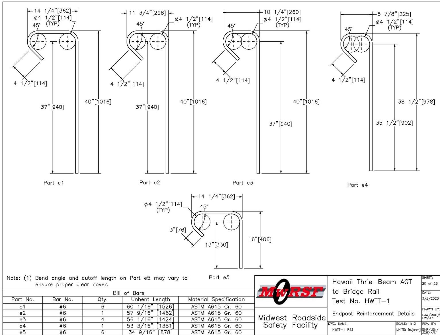
Figure 33. End Post Reinforcement Details, Test Nos. HWTT-1 and HWTT-2
