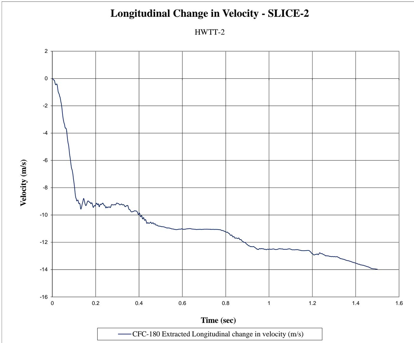
Figure F-2. Longitudinal Occupant Impact Velocity (SLICE-2), Test No. HWTT-2
