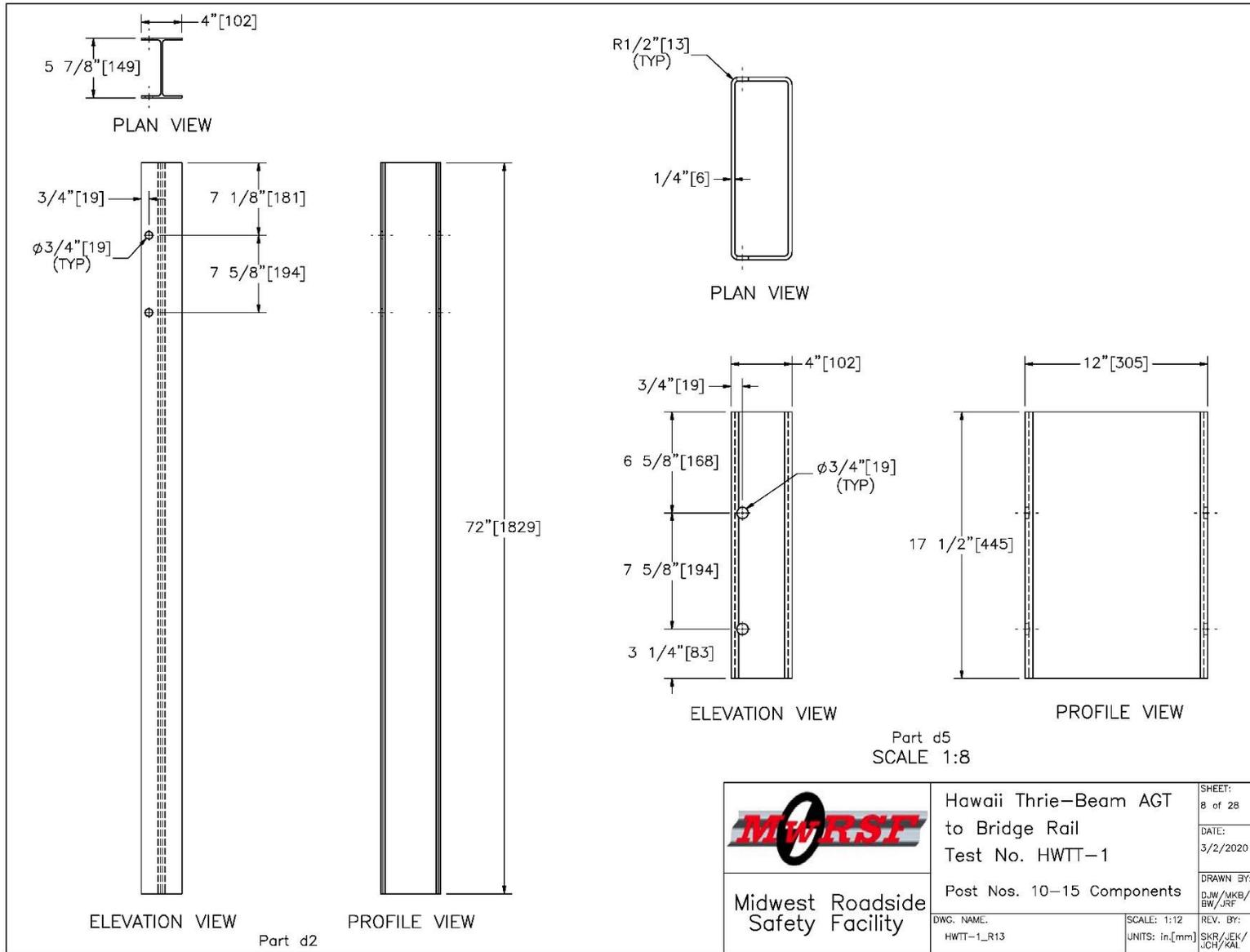
Figure 21. Post Nos. 10 through 15 Components, Test Nos. HWTT-1 and HWTT-2
