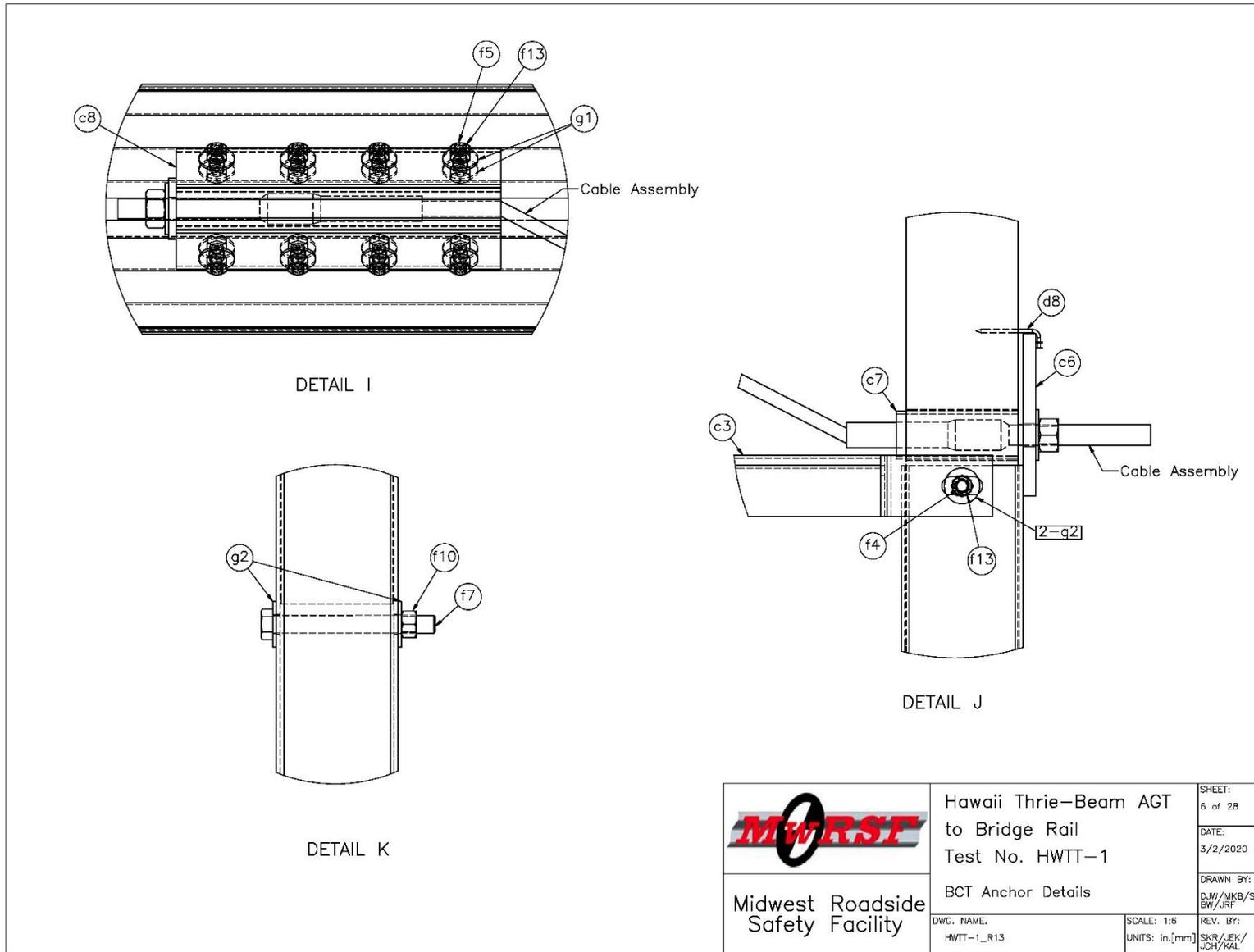
Figure 19. BCT Anchor Details, Test Nos. HWTT-1 and HWTT-2
