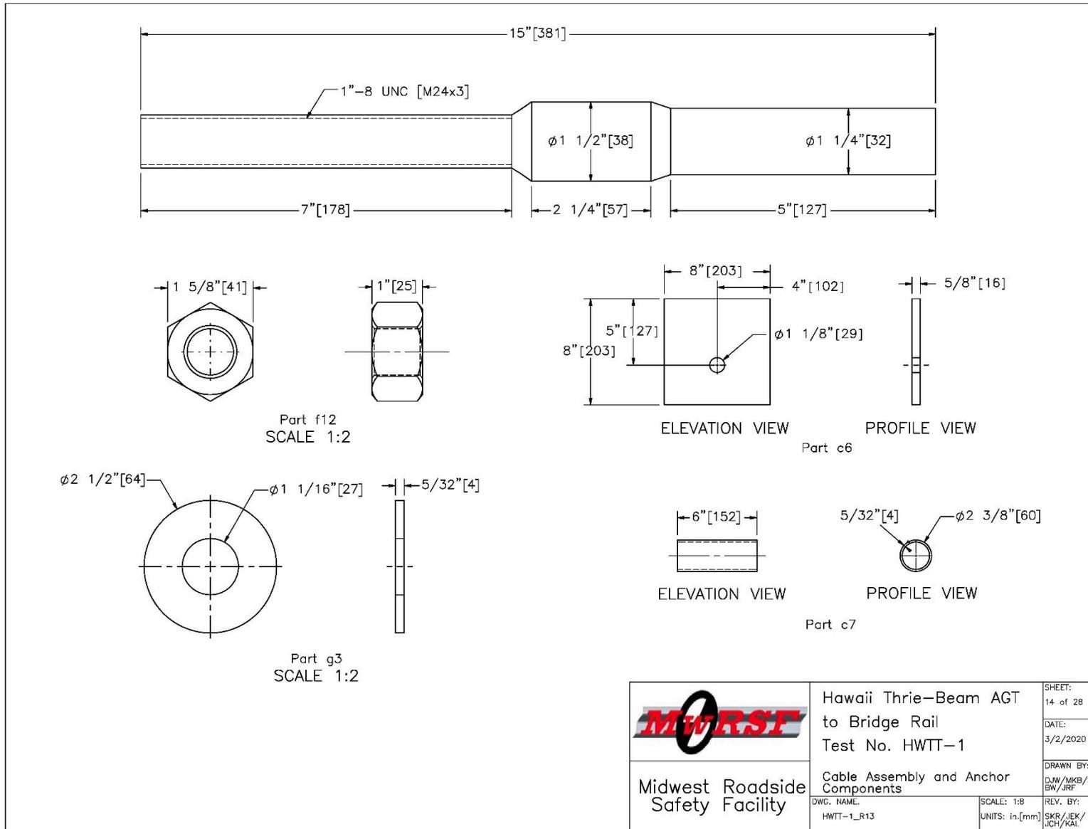
Figure 27. Cable Assembly and Anchor Components, Test Nos. HWTT-1 and HWTT-2
