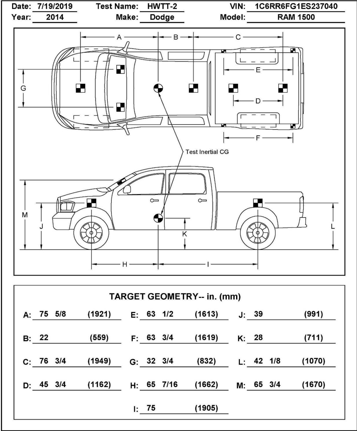
Figure 52. Target Geometry, Test No. HWTT-2
