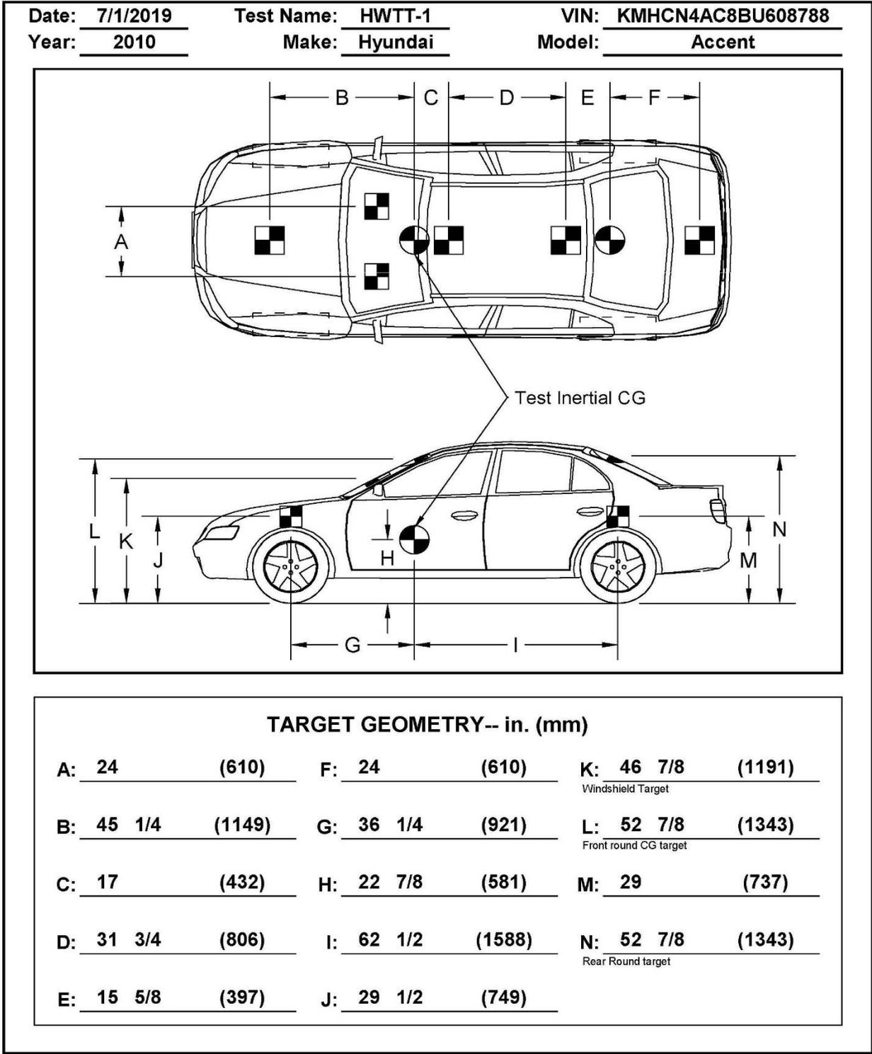
Figure 51. Target Geometry, Test No. HWTT-1
