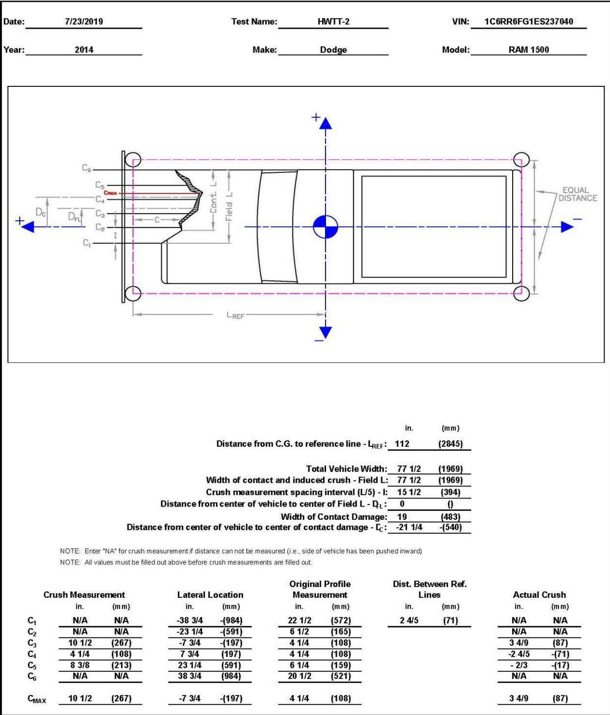
Figure D-12. Exterior Vehicle Crush (NASS) - Front, Test No. HWTT-2
