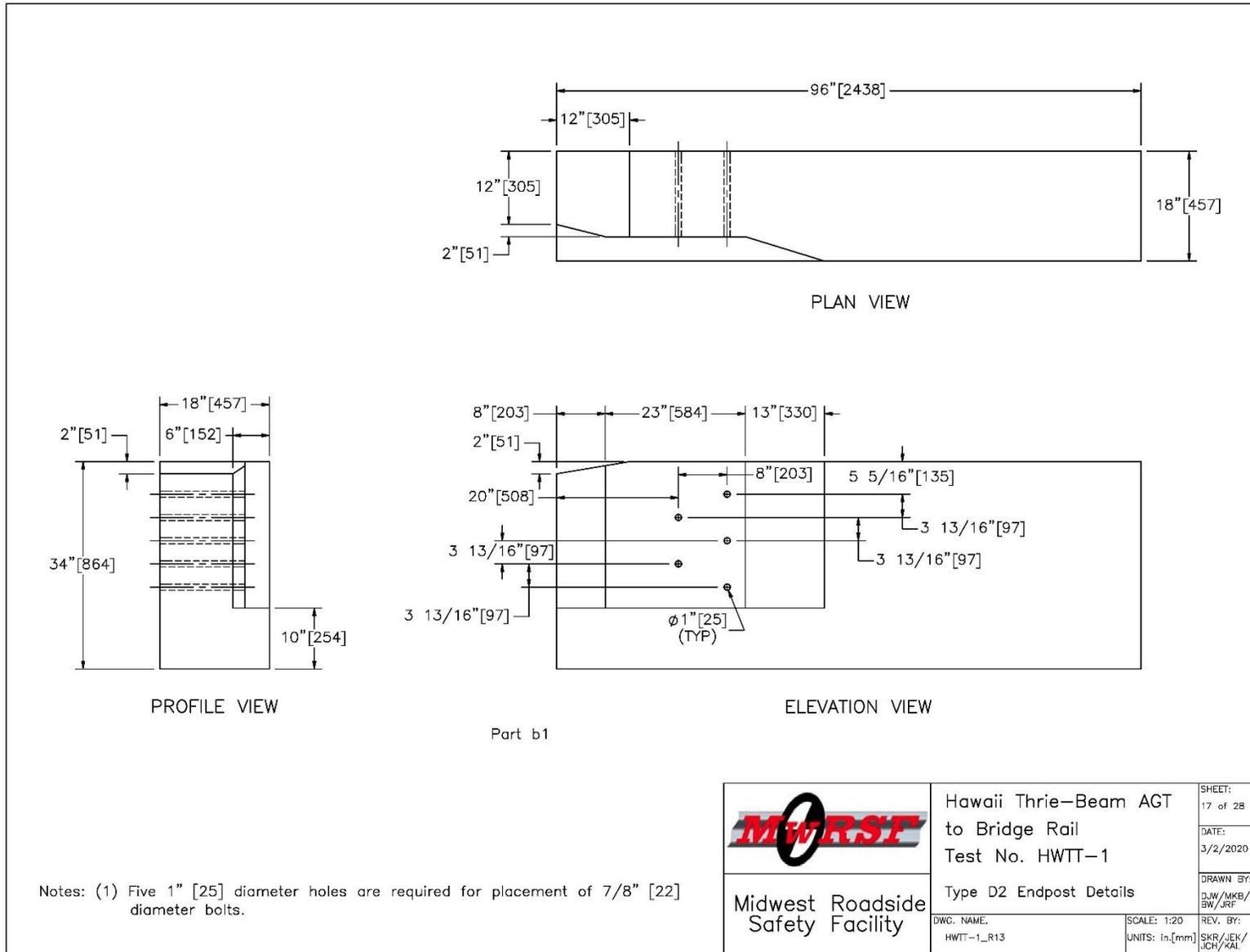
Figure 30. End Post Details, Test Nos. HWTT-1 and HWTT-2
