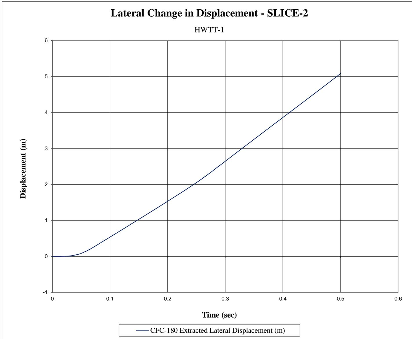
Figure E-14. Lateral Occupant Displacement (SLICE-2), Test No. HWTT-1
