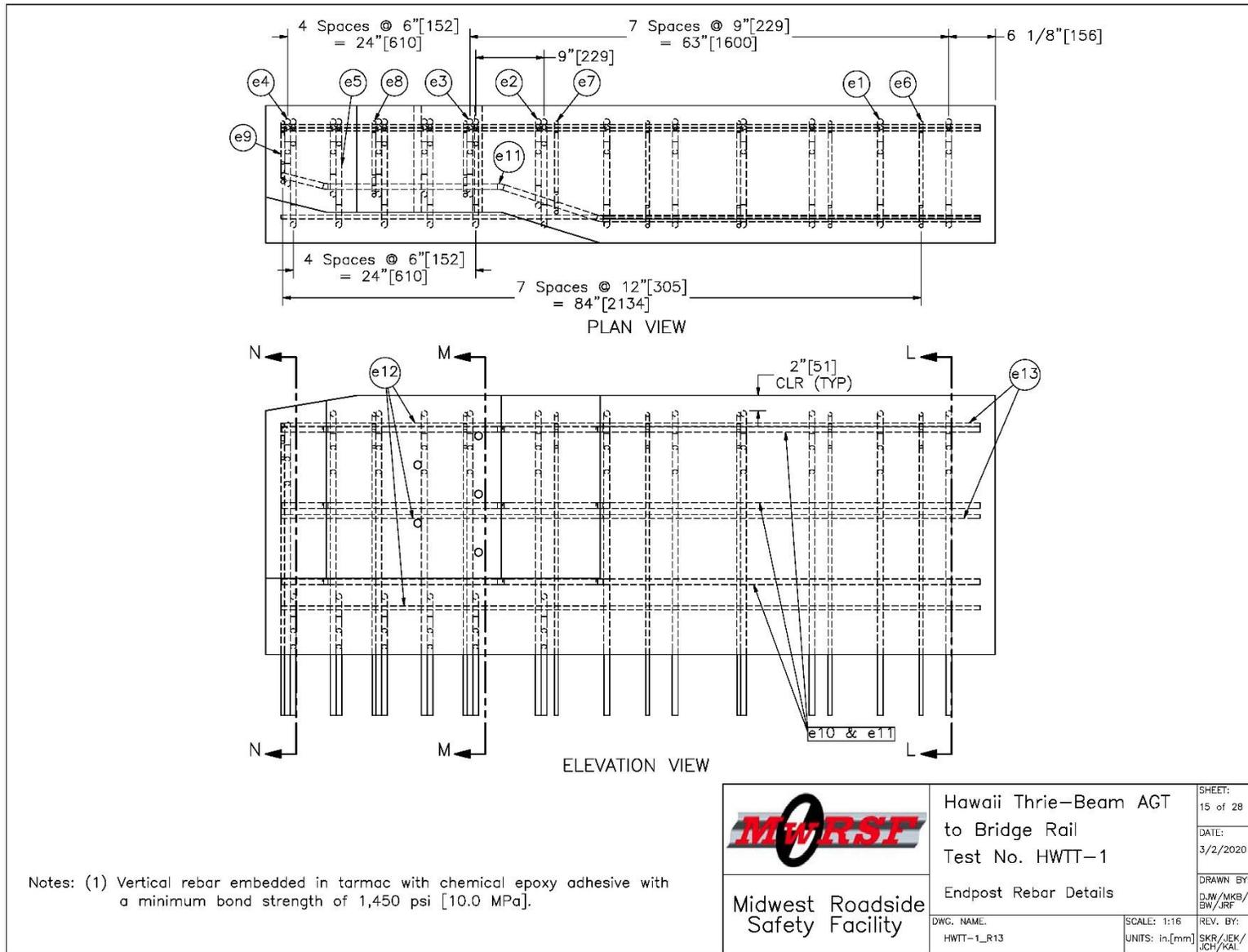
Figure 28. End Post Rebar Details, Test Nos. HWTT-1 and HWTT-2
