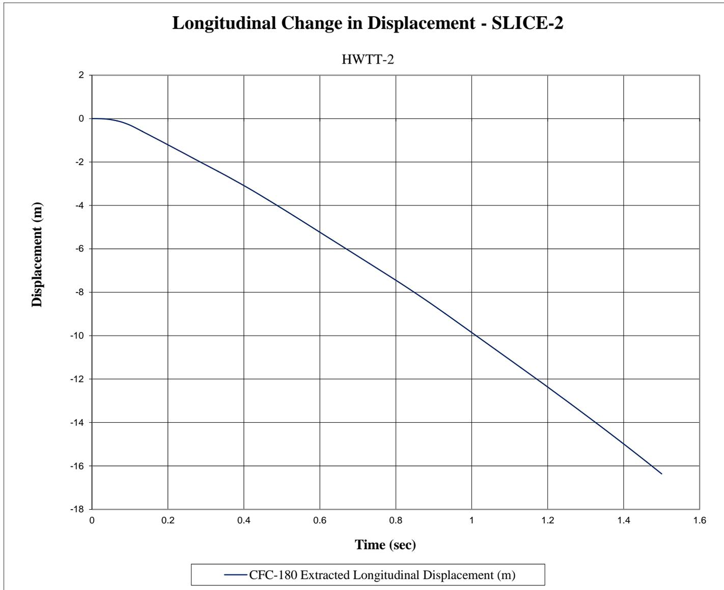
Figure F-3. Longitudinal Occupant Displacement (SLICE-2), Test No. HWTT-2
