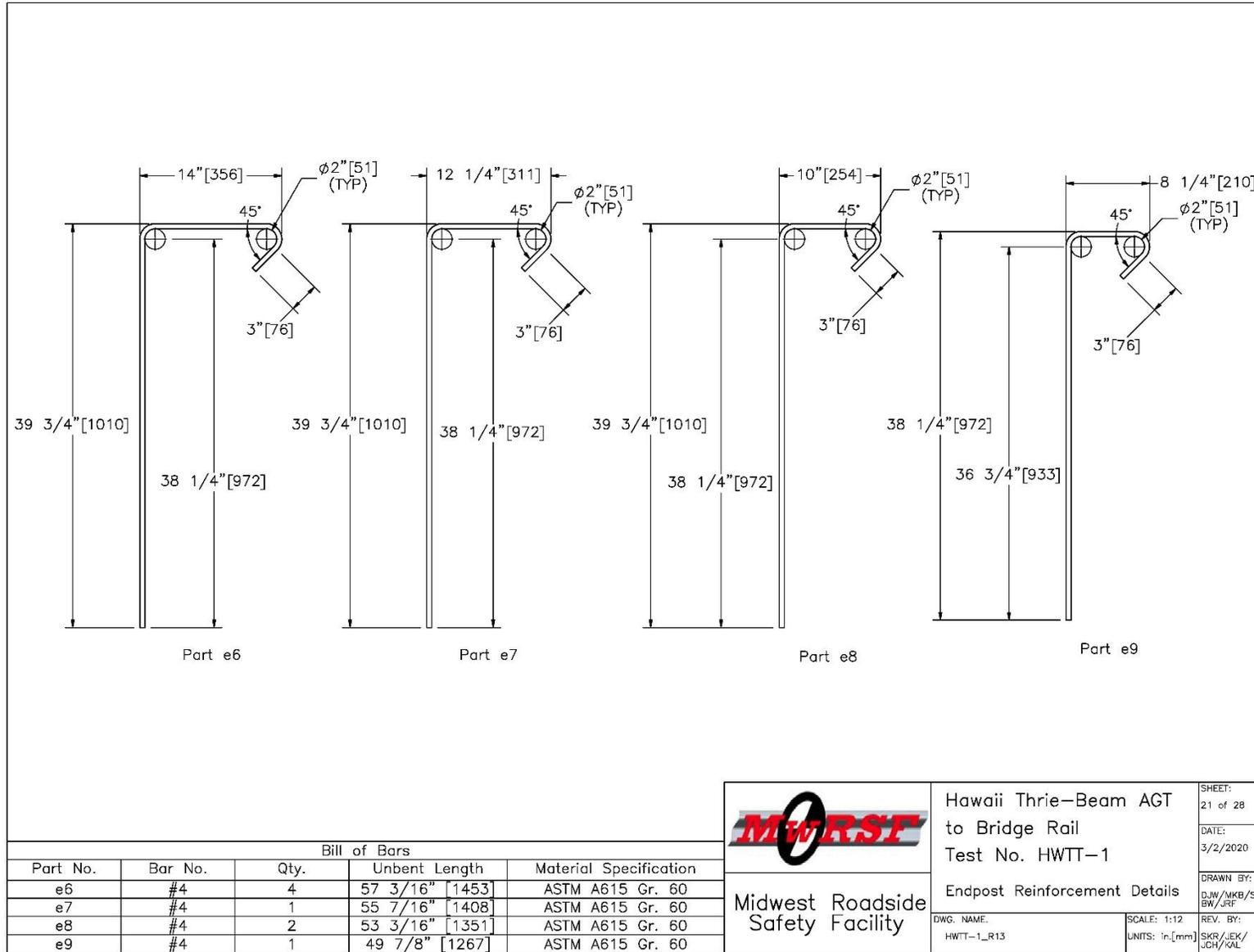
Figure 34. End Post Reinforcement Details, Test Nos. HWTT-1 and HWTT-2
