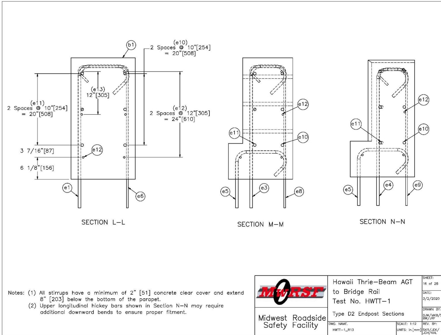
Figure 29. End Post Sections, Test Nos. HWTT-1 and HWTT-2
