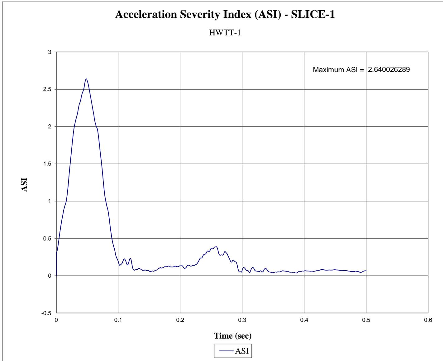
Figure E-8. Acceleration Severity Index (SLICE-1), Test No. HWTT-1
