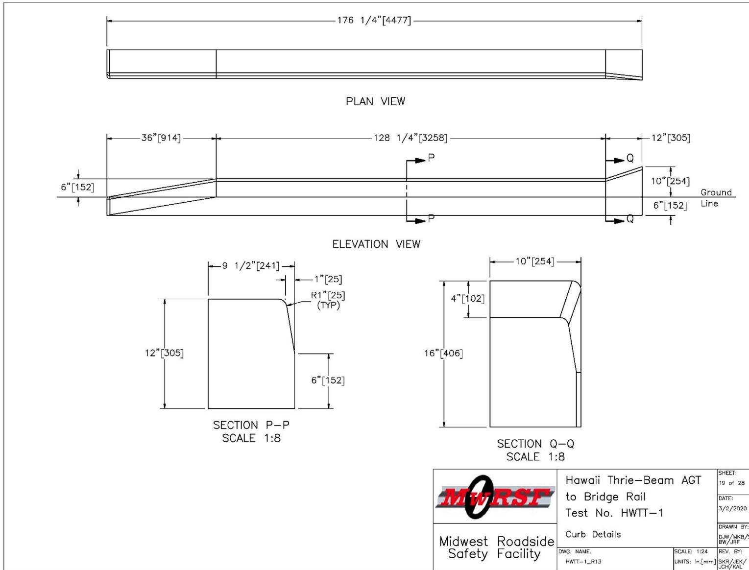
Figure 32. Curb Details, Test Nos. HWTT-1 and HWTT-2
