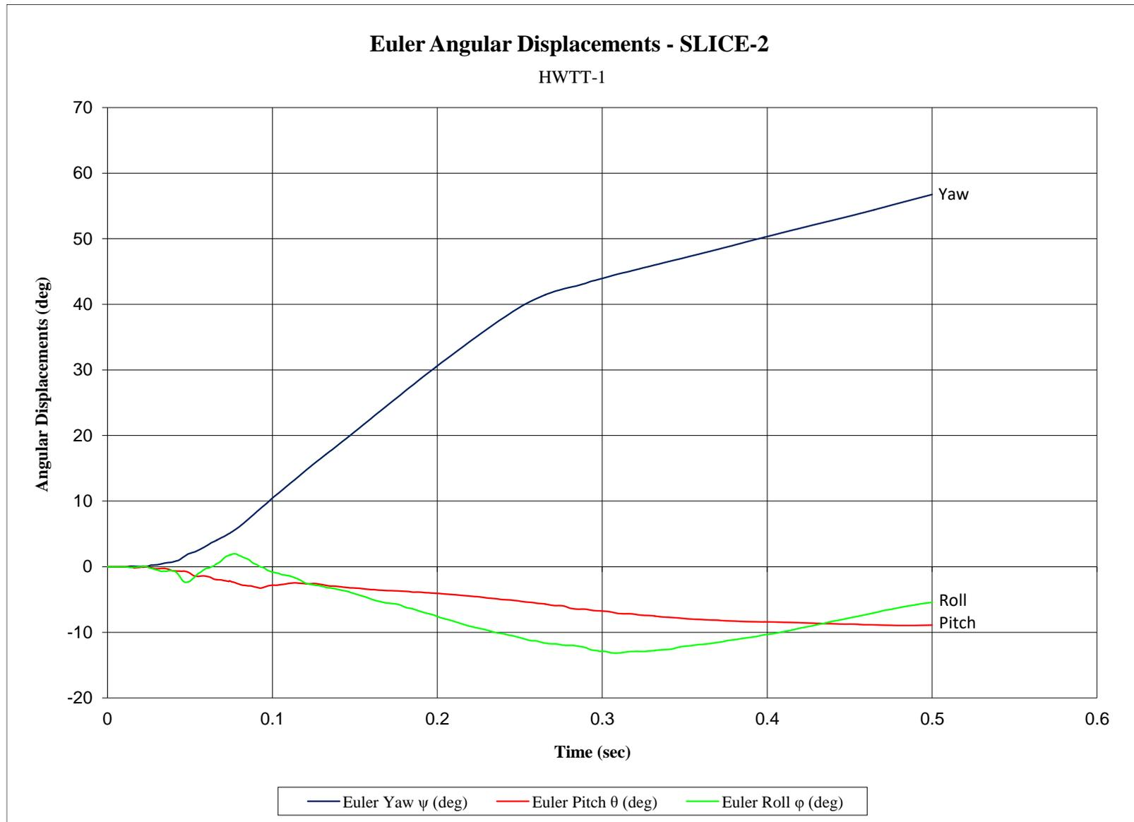
Figure E-15. Vehicle Angular Displacements (SLICE-2), Test No. HWTT-1
