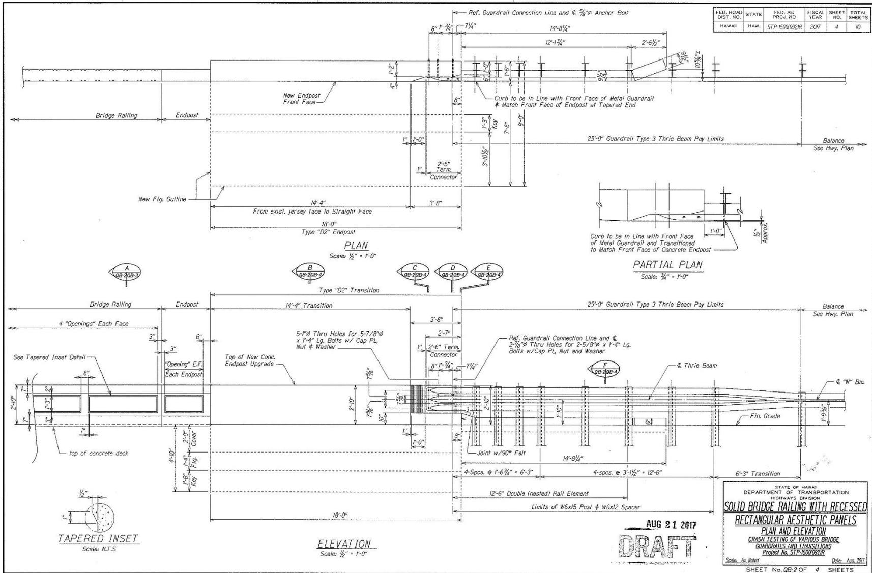
Figure 2. HDOT AGT to 34-in. Tall Bridge Rail Details, Continued
