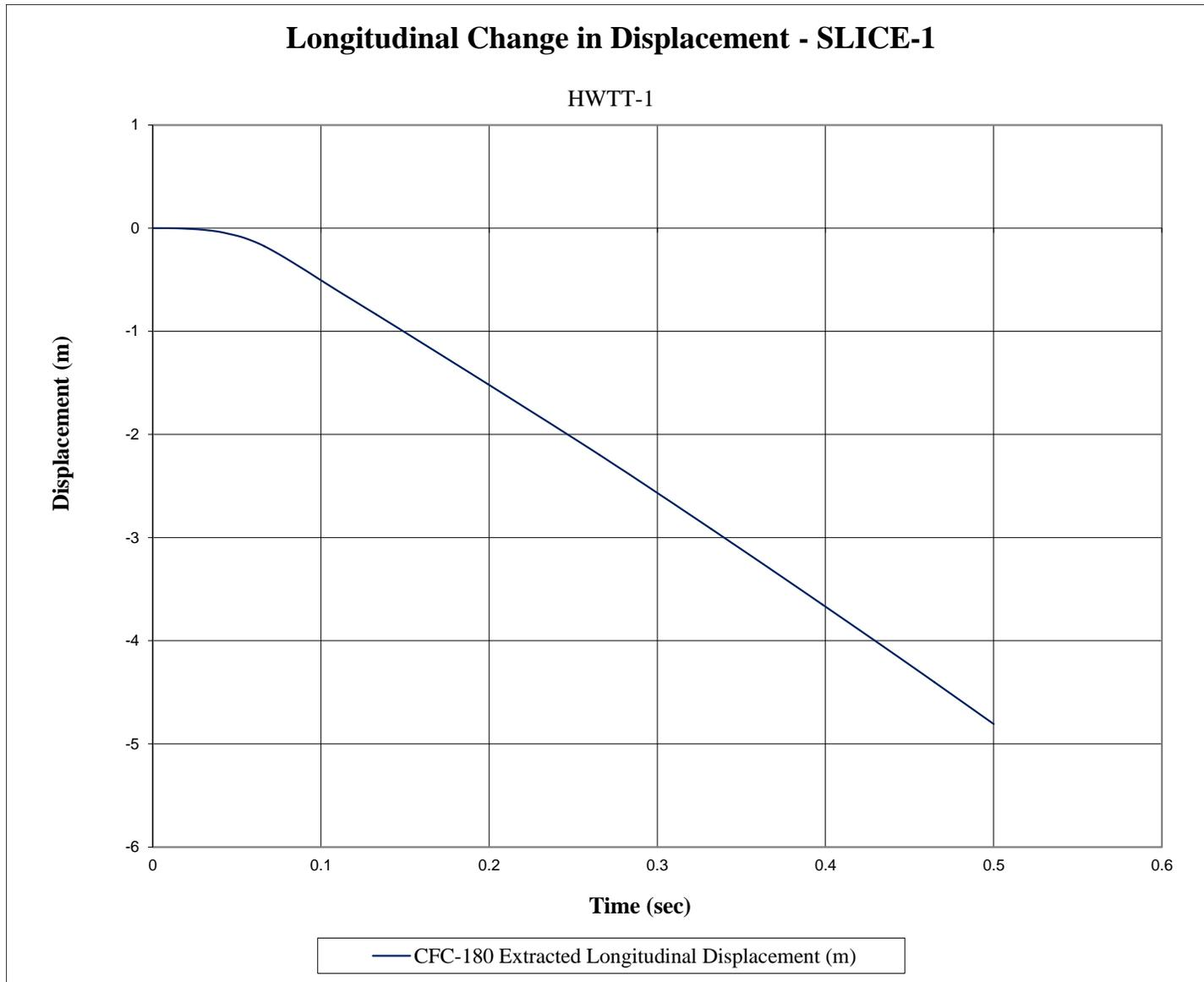
Figure E-3. Longitudinal Occupant Displacement (SLICE-1), Test No. HWTT-1
