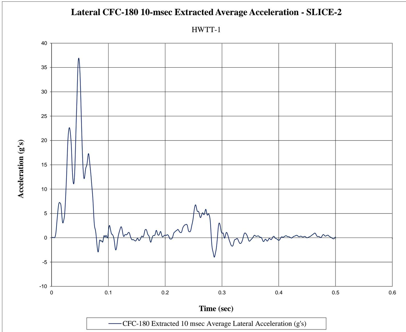
Figure E-12. 10-ms Average Lateral Deceleration (SLICE-2), Test No. HWTT-1
