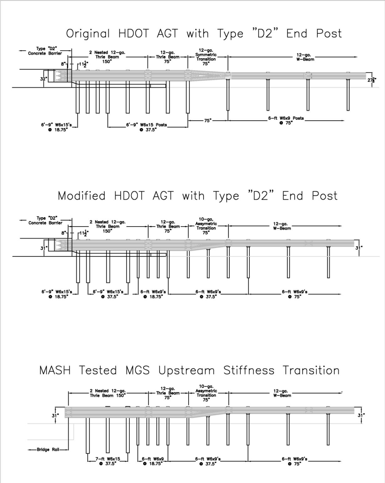
Figure 11. Modified HDOT AGT with Inclusion of MGS Upstream Stiffness Transition
