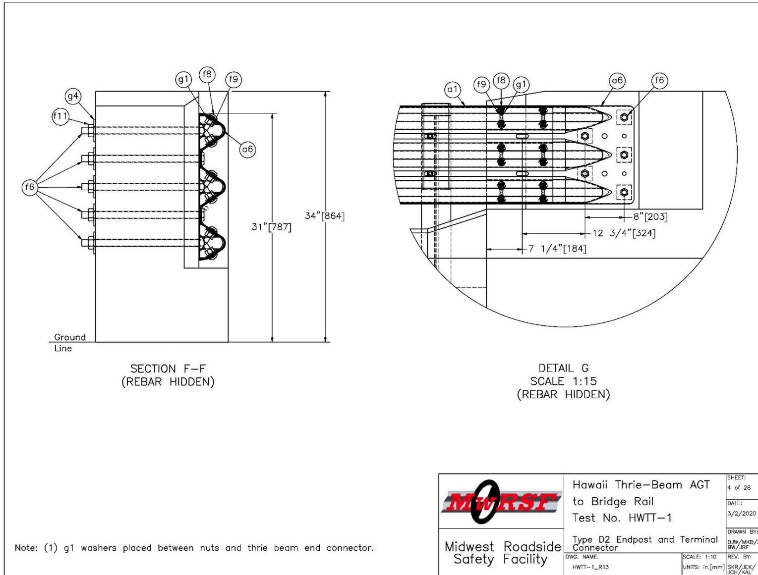
Figure 17. Type D2 End Post and Terminal Connector, Test Nos. HWTT-1 and HWTT-2
