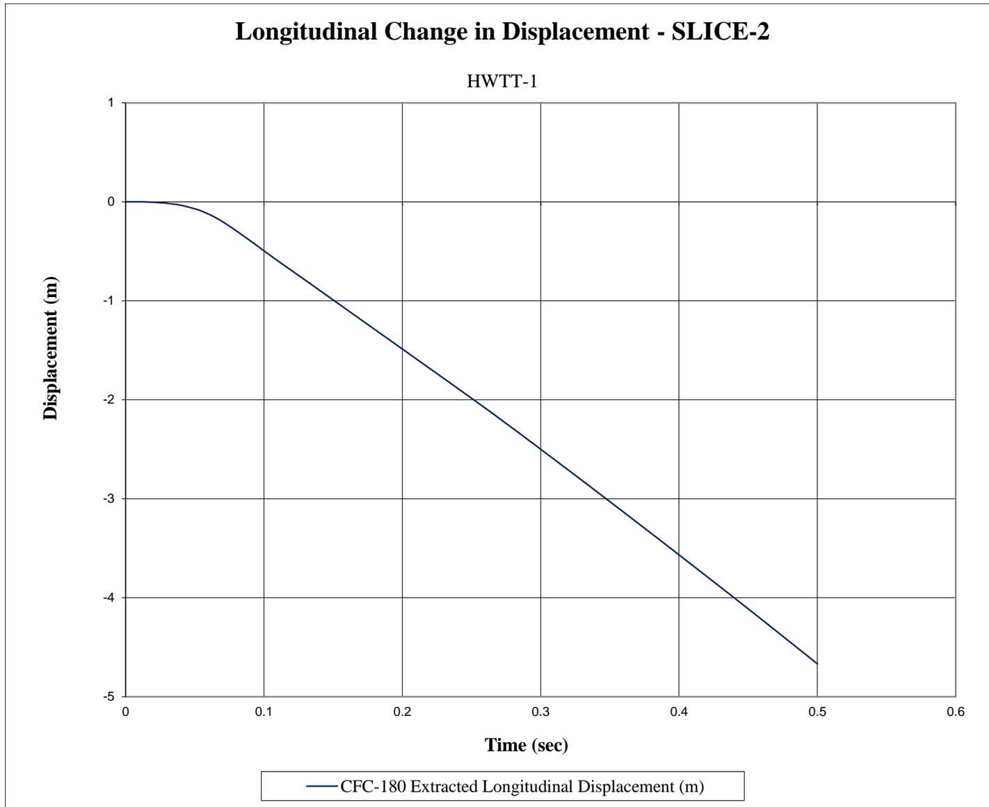
Figure E-11. Longitudinal Occupant Displacement (SLICE-2), Test No. HWTT-1
