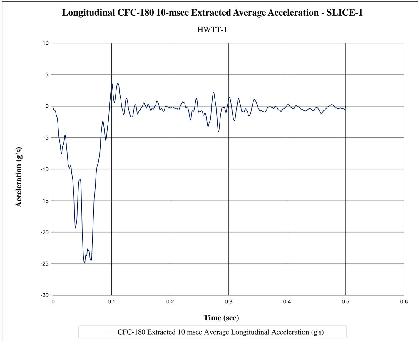
Figure E-1. 10-ms Average Longitudinal Deceleration (SLICE-1), Test No. HWTT-1
