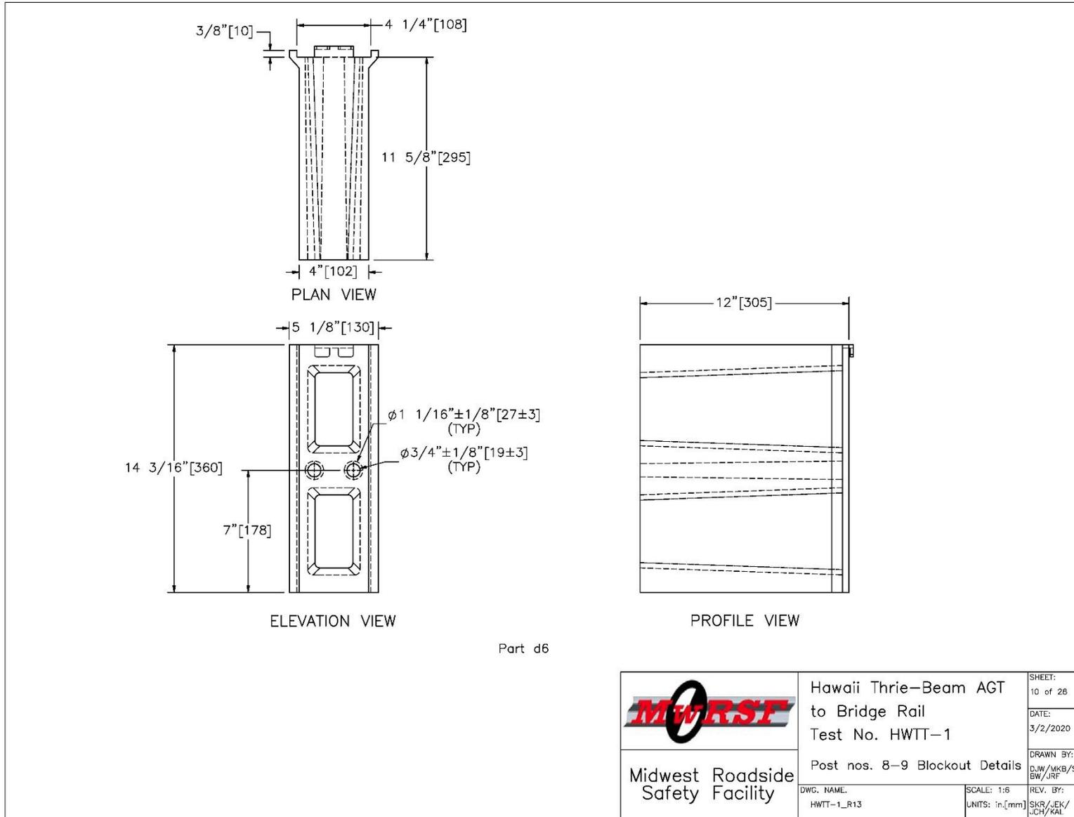
Figure 23. Post Nos. 8 and 9 Blockout Details, Test Nos. HWTT-1 and HWTT-2
