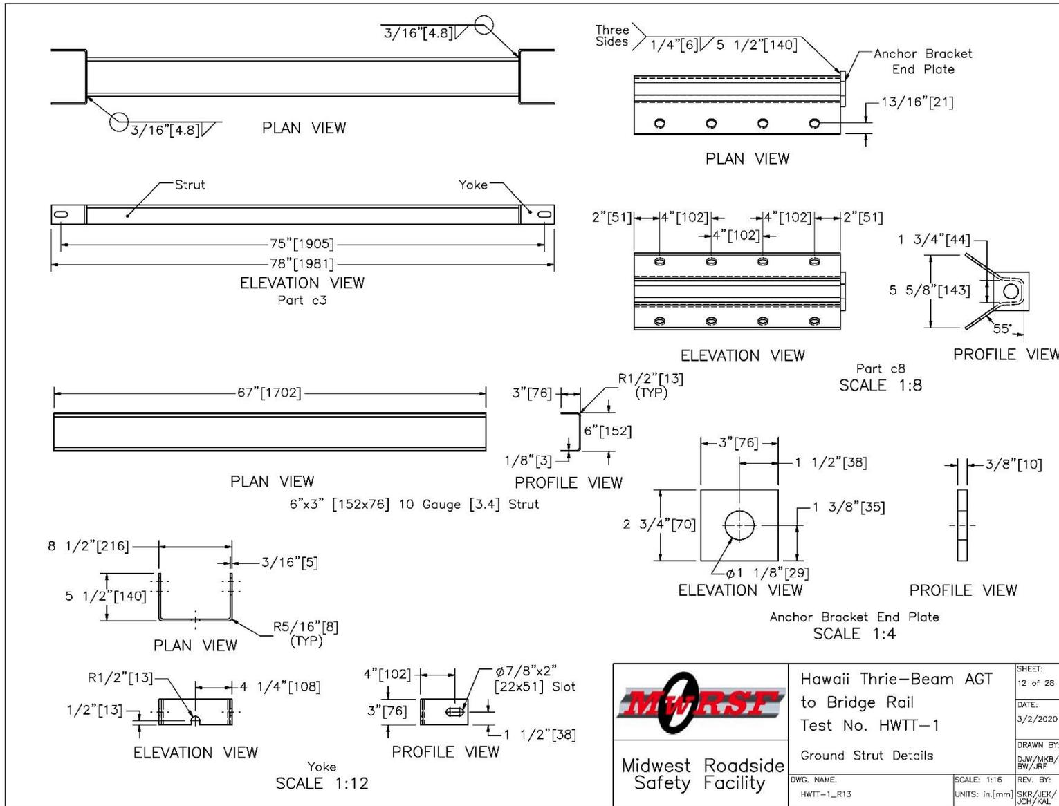
Figure 25. Ground Strut Details, Test Nos. HWTT-1 and HWTT-2
