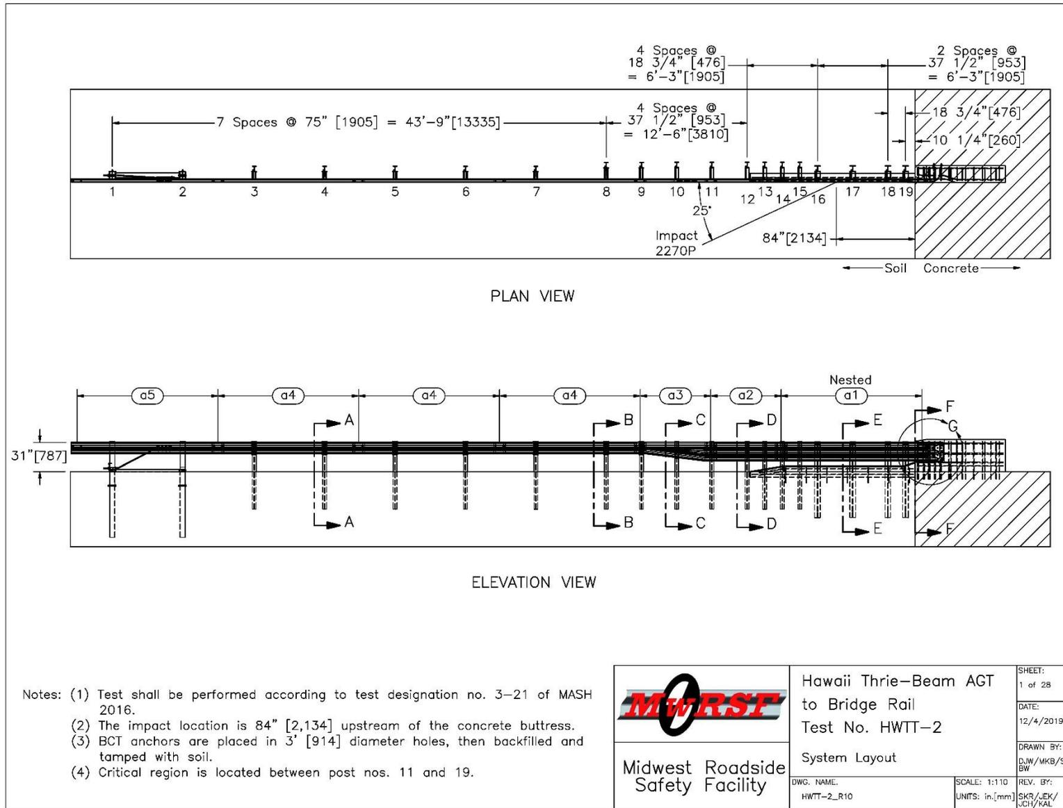
Figure 14. System Layout, Test No. HWTT-2
