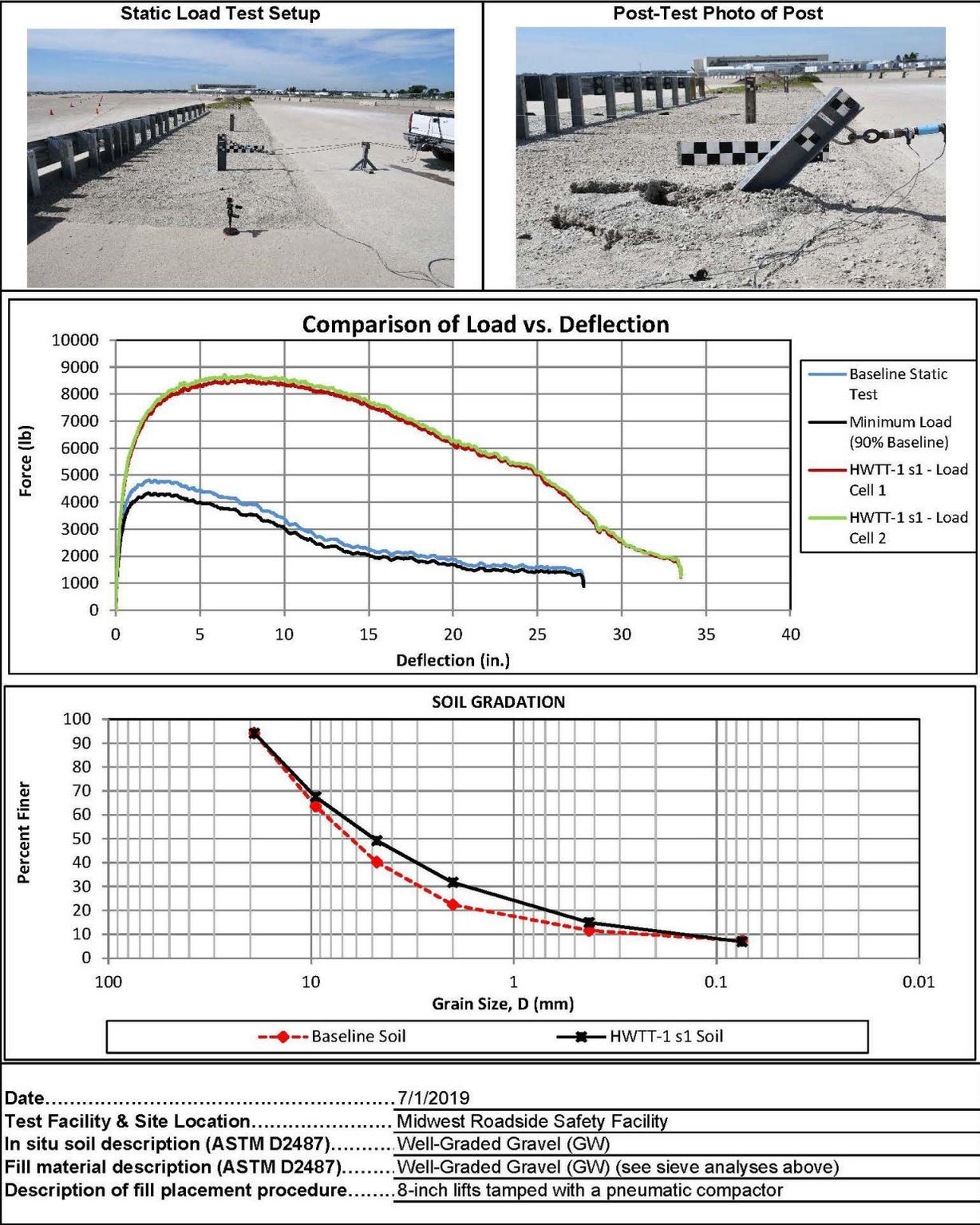
Figure C-2. Static Soil Test, Test No. HWTT-1
