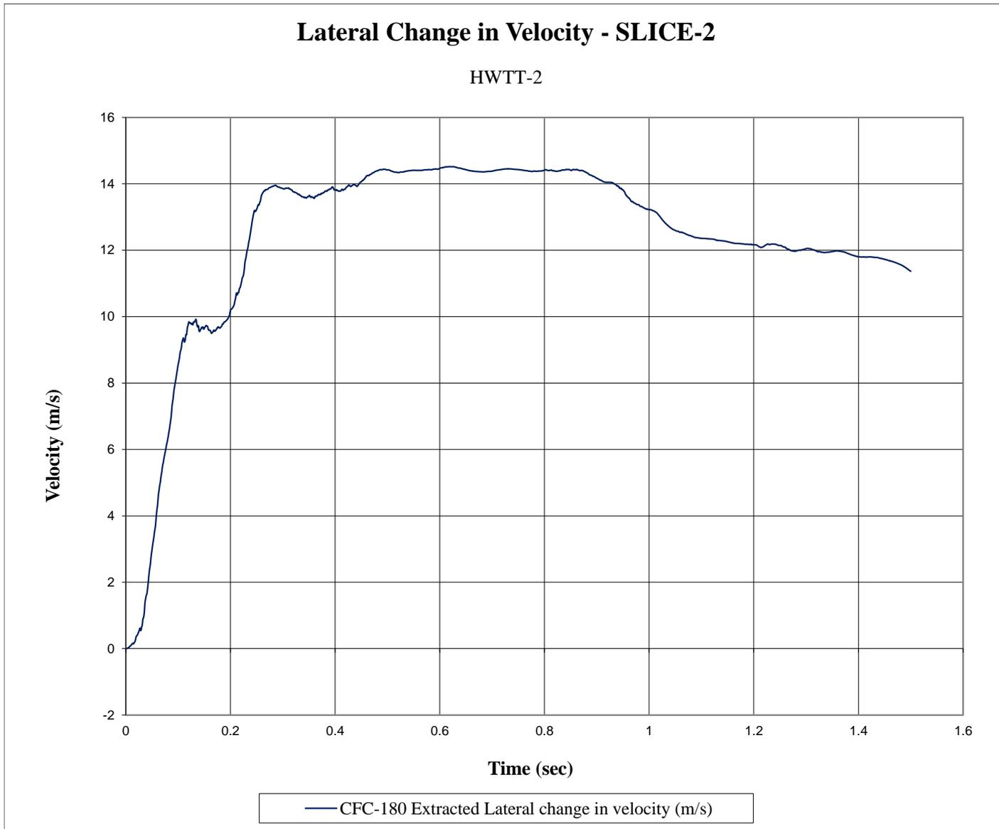
Figure F-5. Lateral Occupant Impact Velocity (SLICE-2), Test No. HWTT-2
