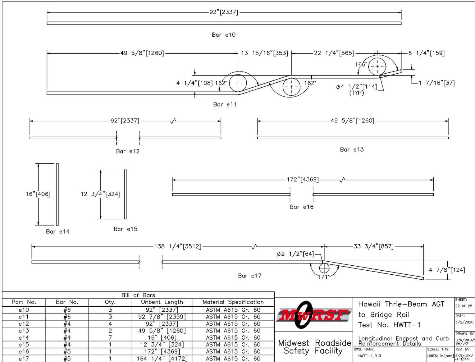
Figure 35. Longitudinal End Post and Curb Reinforcement Details, Test Nos. HWTT-1 and HWTT-2
