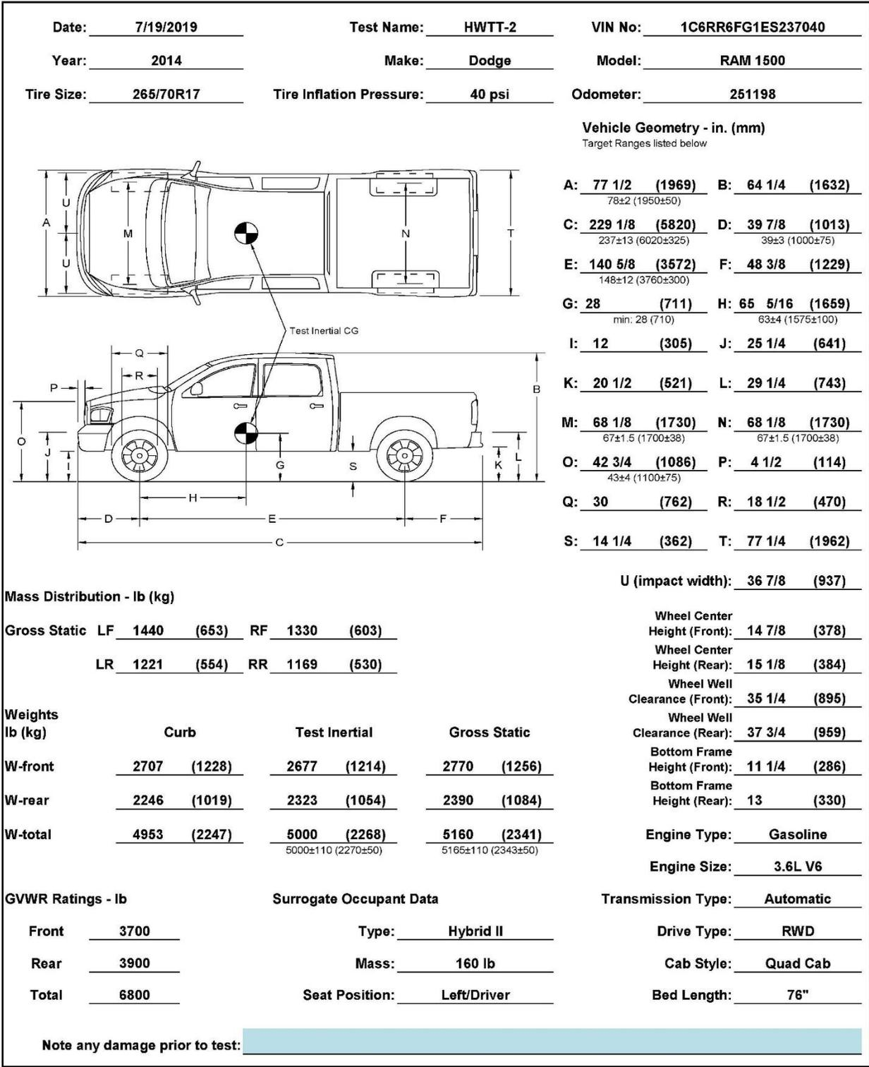
Figure 50. Vehicle Dimensions, Test No. HWTT-2
