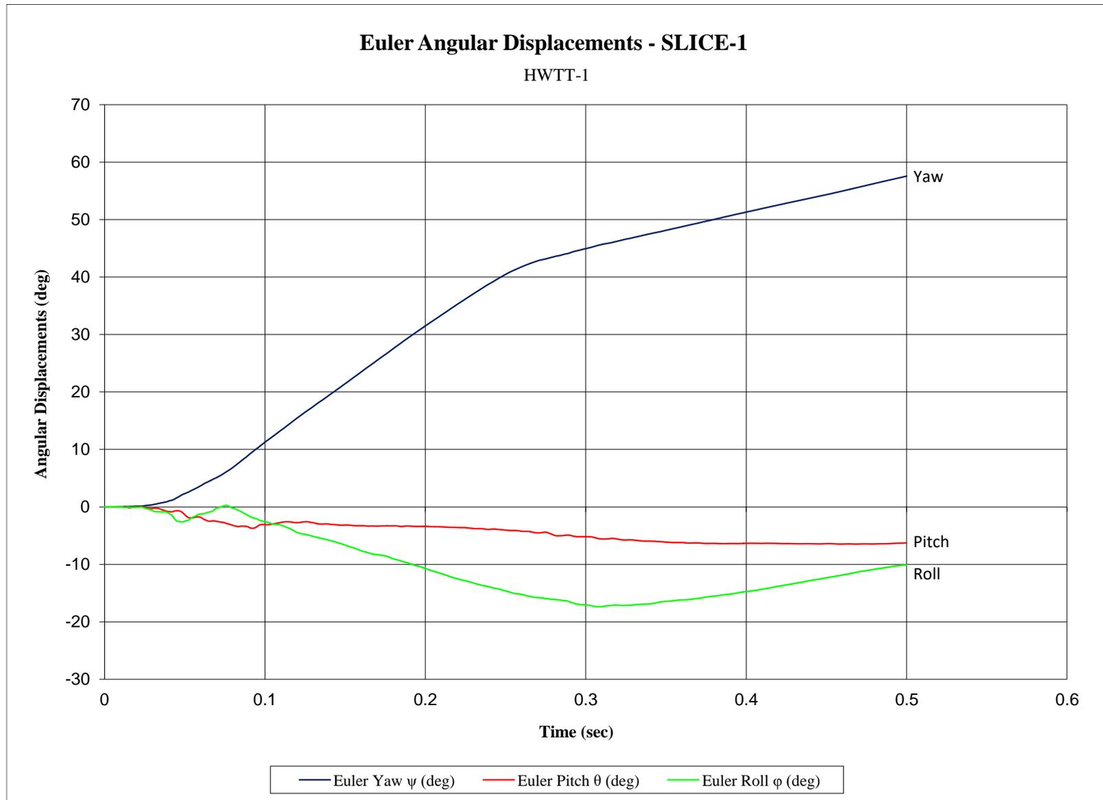
Figure E-7. Vehicle Angular Displacements (SLICE-1), Test No. HWTT-1
