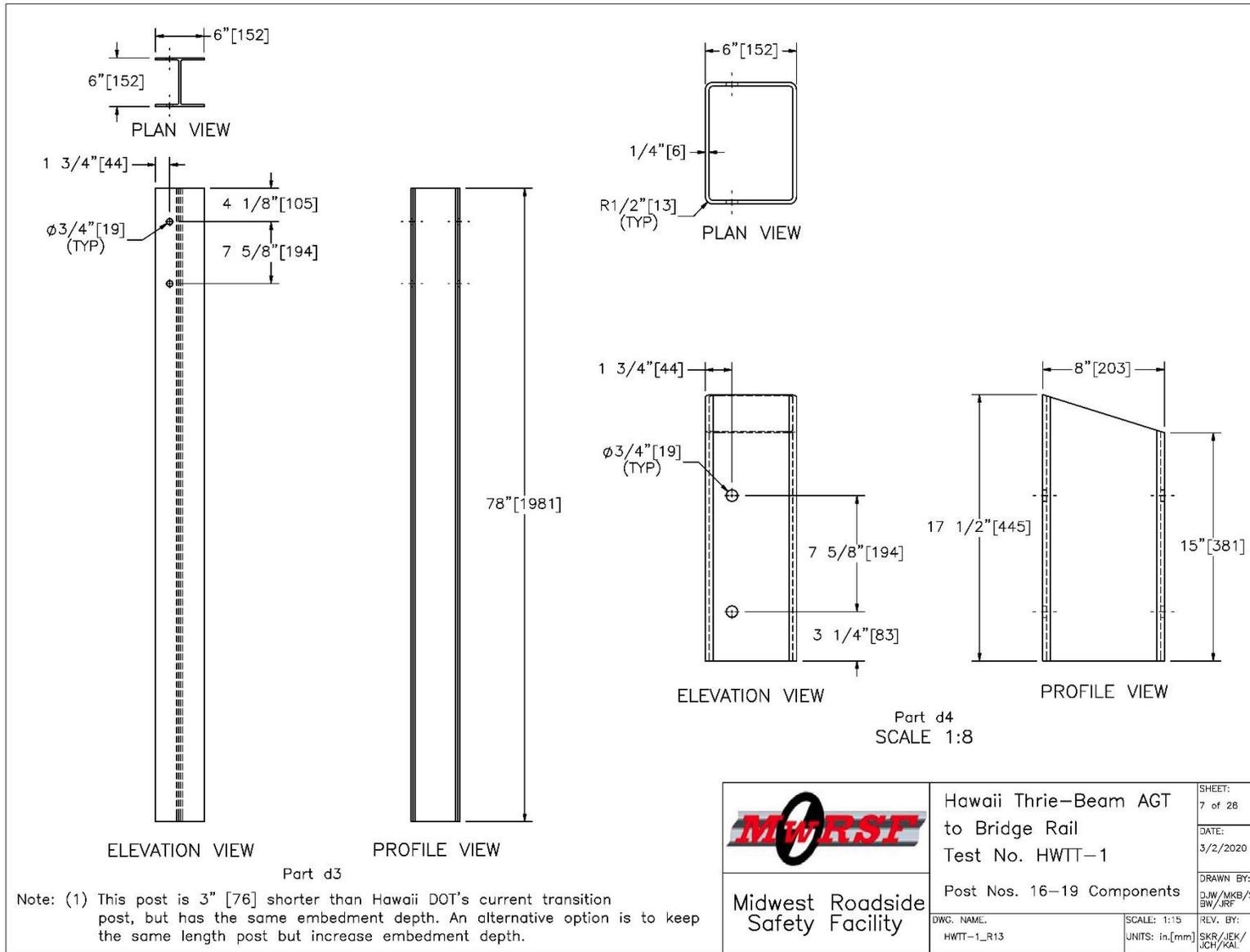
Figure 20. Post Nos. 16 through 19 Components, Test Nos. HWTT-1 and HWTT-2
