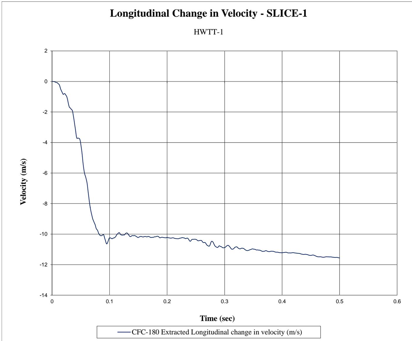
Figure E-2. Longitudinal Occupant Impact Velocity (SLICE-1), Test No. HWTT-1
