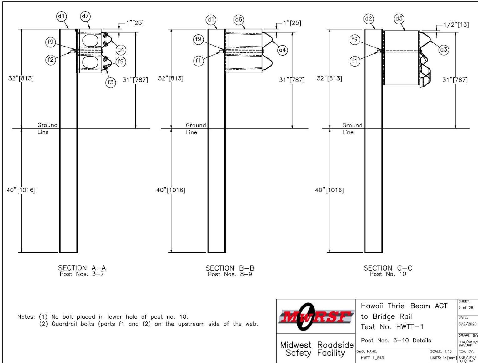
Figure 15. Post Nos. 3 through 10 Details, Test Nos. HWTT-1 and HWTT-2
