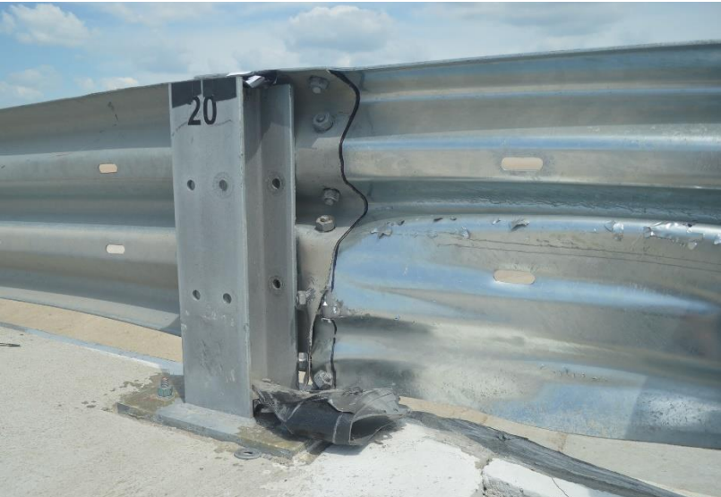
Figure 139. Curb and Post Damage, Test No. HMDT-3
