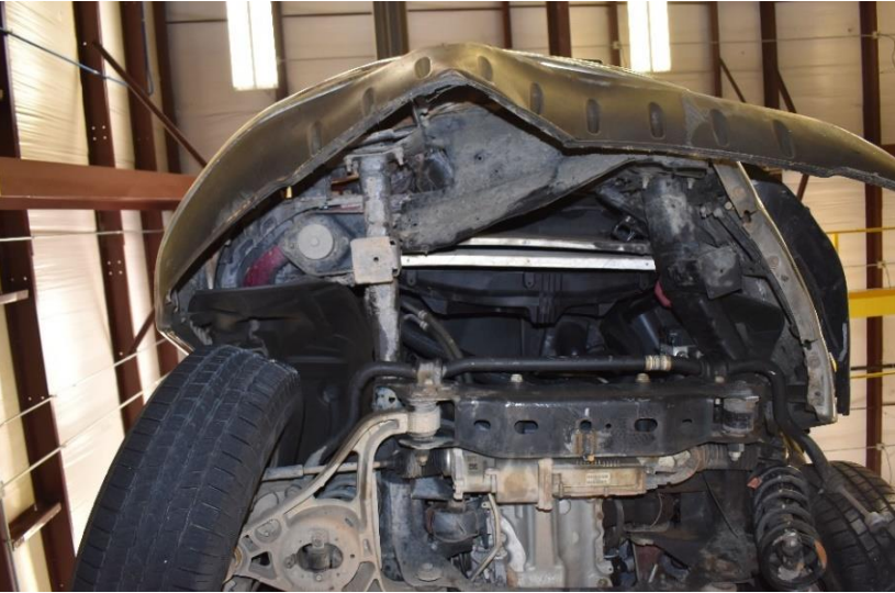
Figure 129. Interior and Undercarriage Damage, Test No. HMDT-2
