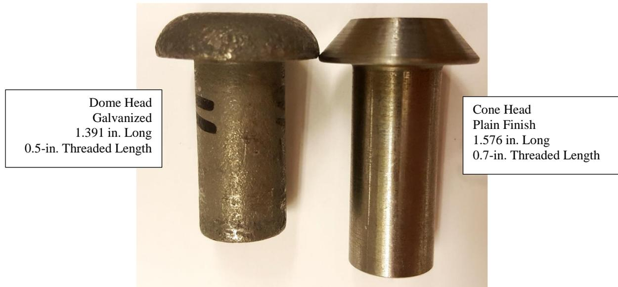
Figure 1. Illustration of Differences between Sleeve Nut Concepts
