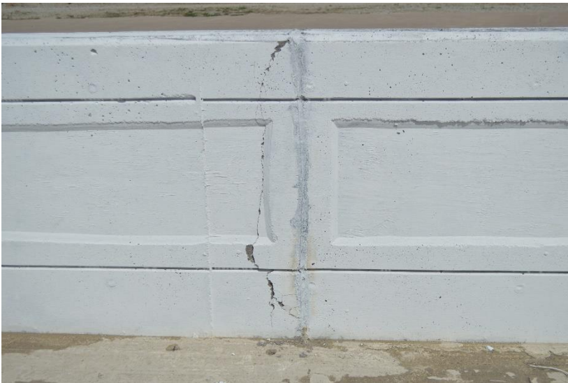
Figure 58. Back-Side System Damage, Test No. H34BR-2
