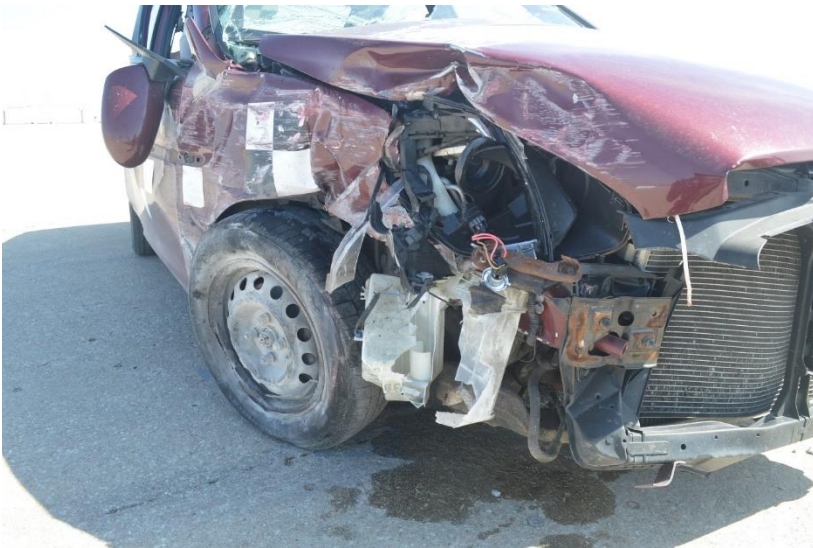
Figure 42. Vehicle Damage, Test No. H34BR-1
