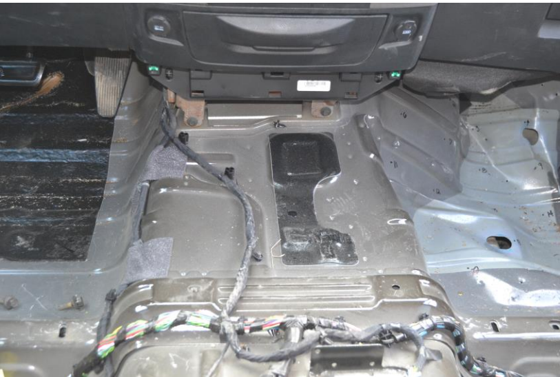
Figure 63. Interior Floorboard Damage, Test No. H34BR-2
