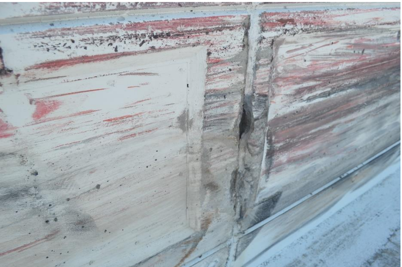
Figure 38. Traffic-Side System Damage, Test No. H34BR-1
