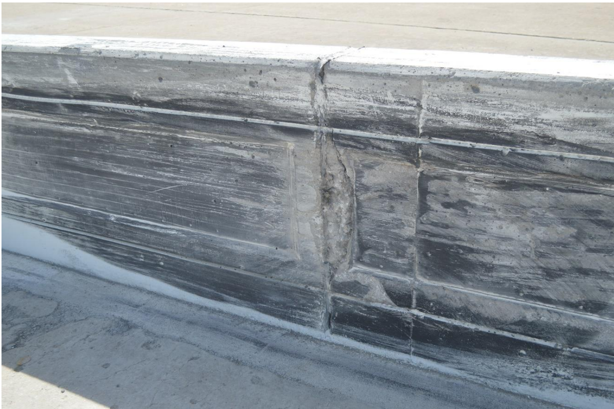
Figure 56. Traffic-Side System Damage, Test No. H34BR-2
