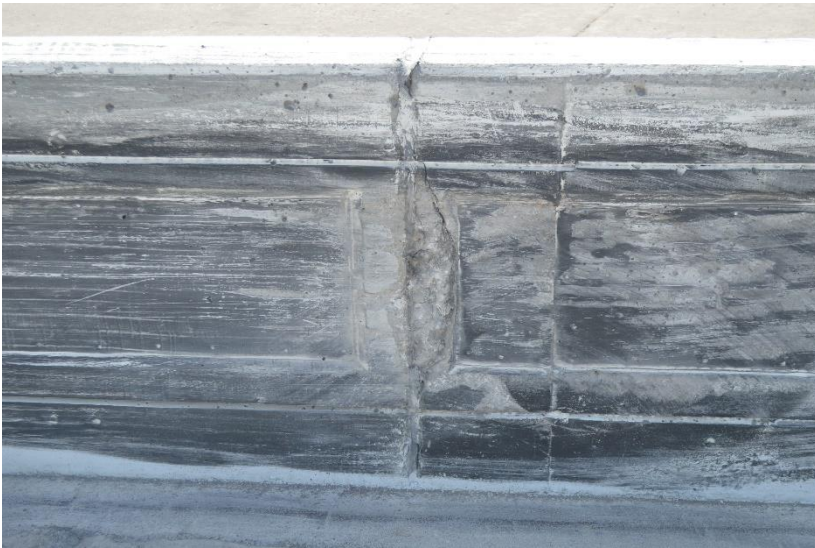
Figure 57. Traffic-Side System Damage, Test No. H34BR-2
