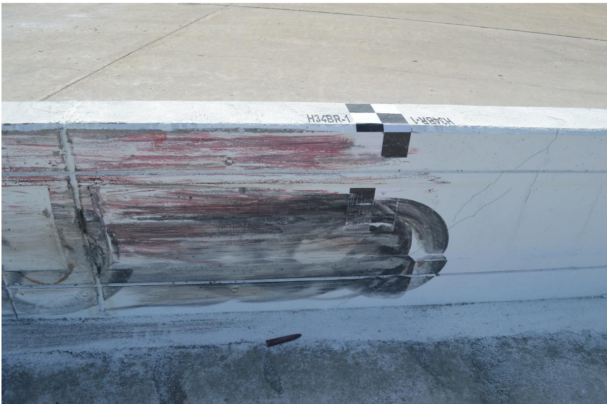
Figure 36. Traffic-Side System Damage, Test No. H34BR-1
