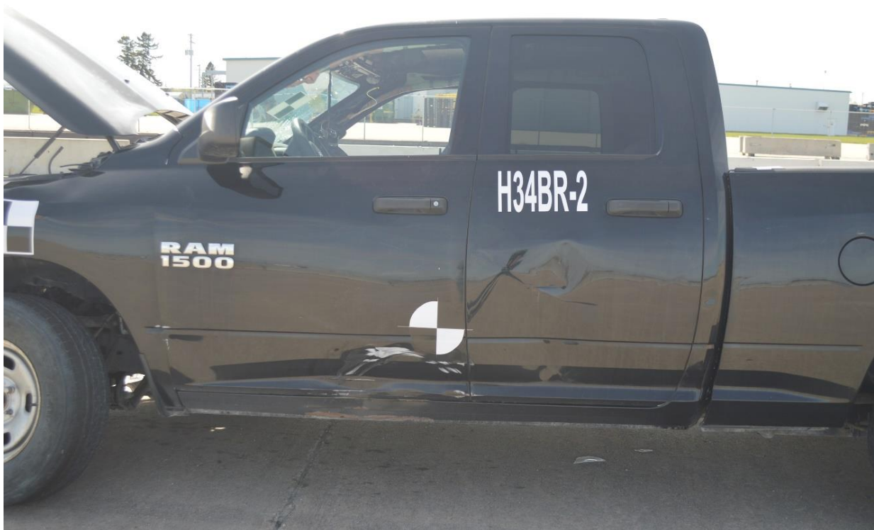
Figure 62. Vehicle Damage, Test No. H34BR-2
