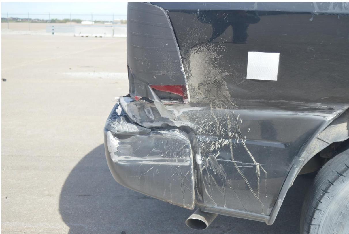
Figure 61. Vehicle Damage, Test No. H34BR-2
