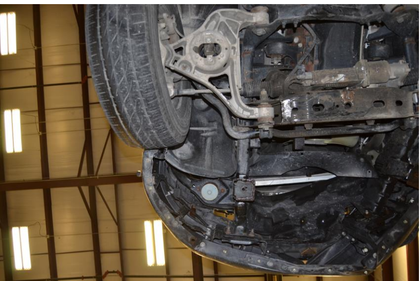
Figure 64. Undercarriage Damage, Test No. H34BR-2
