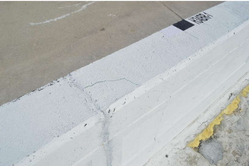
Figure 39. Back-Side System Damage, Test No. H34BR-1
