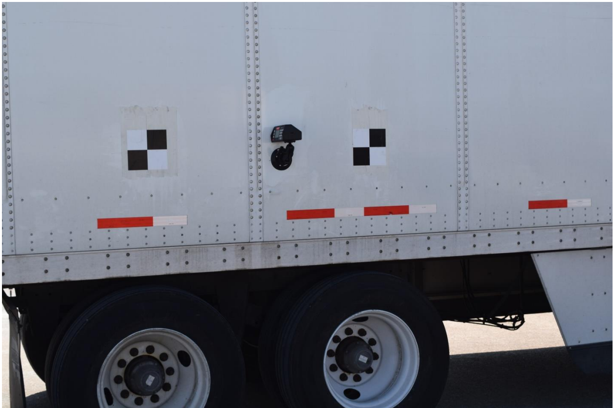
Figure 49. VC4000 Accelerometer Mounted on Trailer
