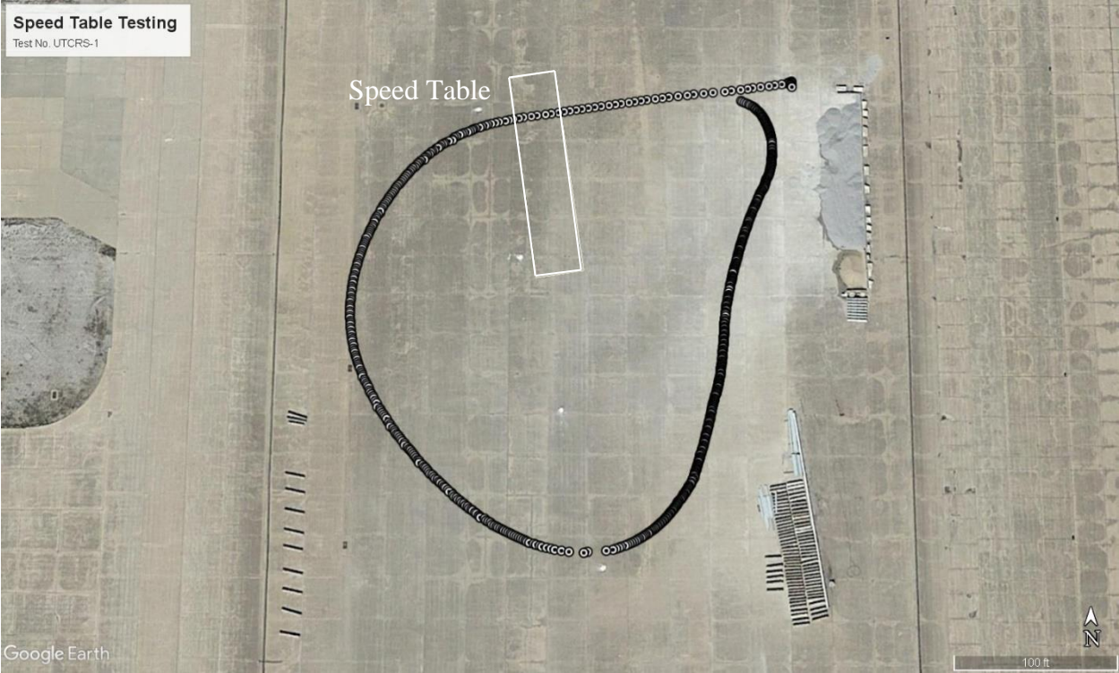
Figure 59. GPS Data Overlaid on Google Earth Image of the Test Site, Test No. UTCRS-1
